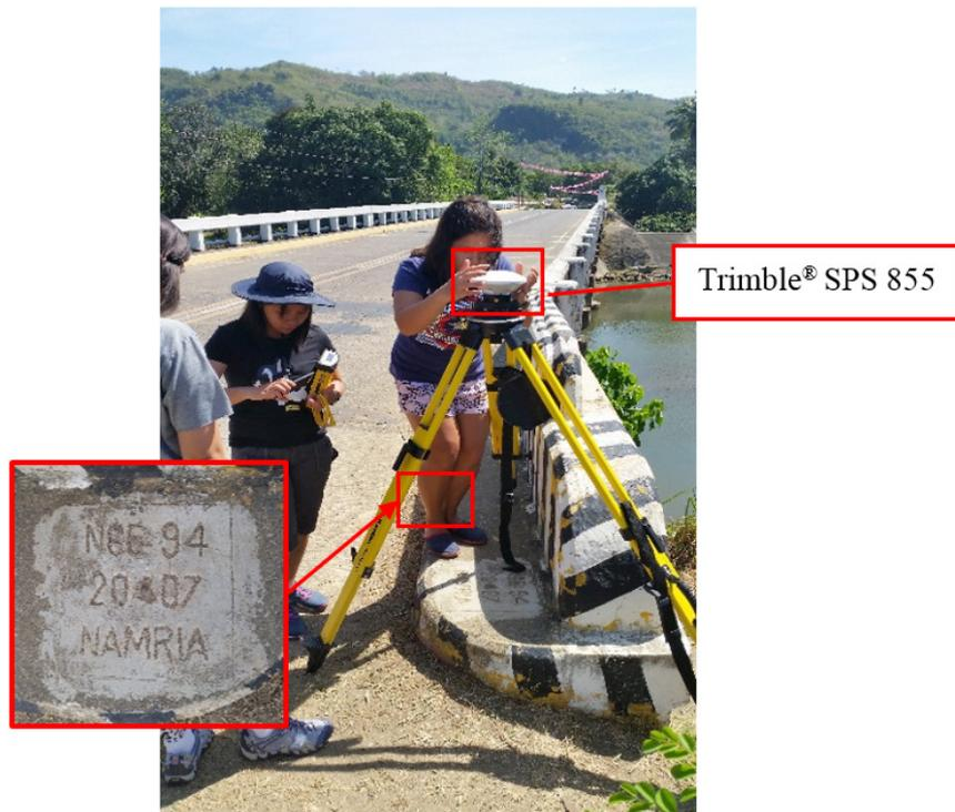
Figure 36. GNSS receiver set-up, Trimble® Zephyr™ Model 2, at NGE-94 in Brgy. Bal-os, Municipality of Basay, Negros Oriental.
