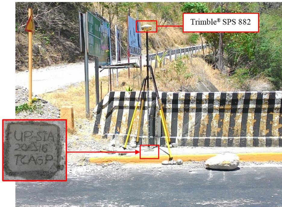
Figure 37. GNSS receiver set-up, Trimble®SPS 882 at control point UP-SIA at Siaton Bridge, Brgy. Caticugan, Municipality of Siaton, Negros Oriental.
