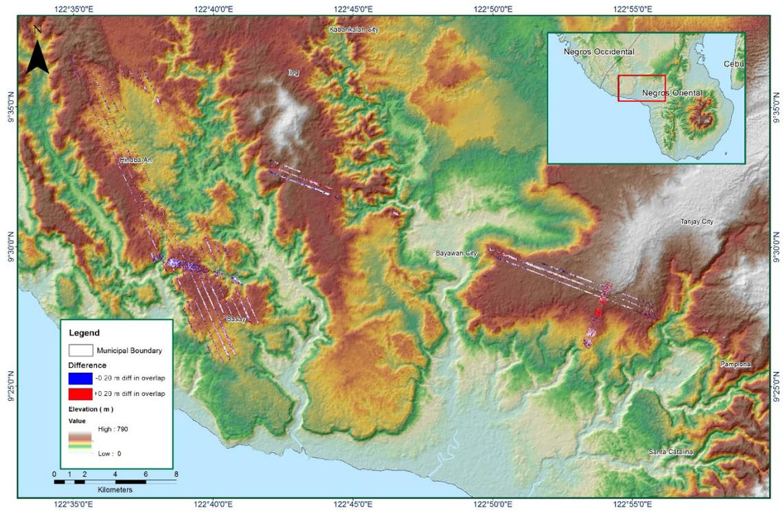
Figure 1.5.7 Elevation difference between flight lines
