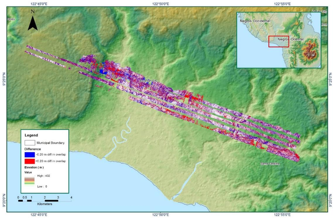
Figure 1.4.7 Elevation difference between flight lines
