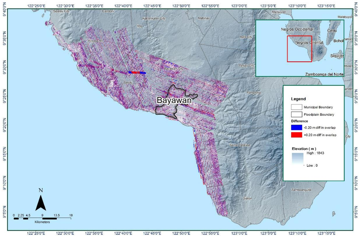
Figure 18. Elevation difference map between flight lines for Bayawan floodplain.
