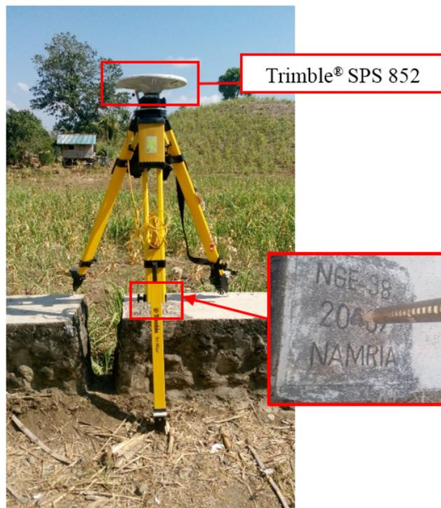
Figure 34. GNSS receiver setup, Trimble® SPS 852, at NGE-98 in Brgy. Kabulacan, Sitio Danao, Municipality of Santa Catalina, Negros Oriental.
