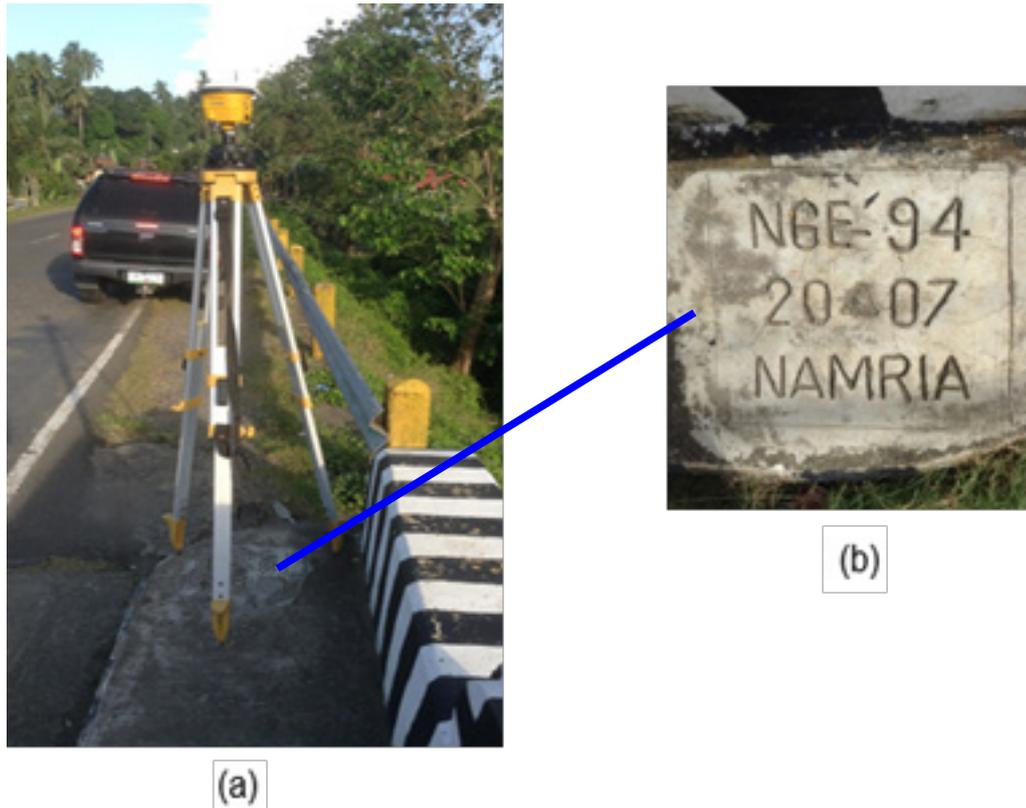
Figure 3. GPS set-up over NGE-94 at the south approach of Tiabanan’s bridge wing wall sidewalk in barangay Bal-Os, Municipality of Basay (a) and NAMRIA reference point NGE-94 (b) as recovered by the field team.
