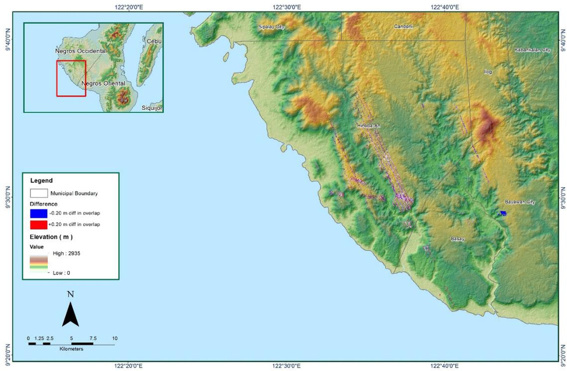
Figure 1.1.7 Elevation Difference between Flight Lines
