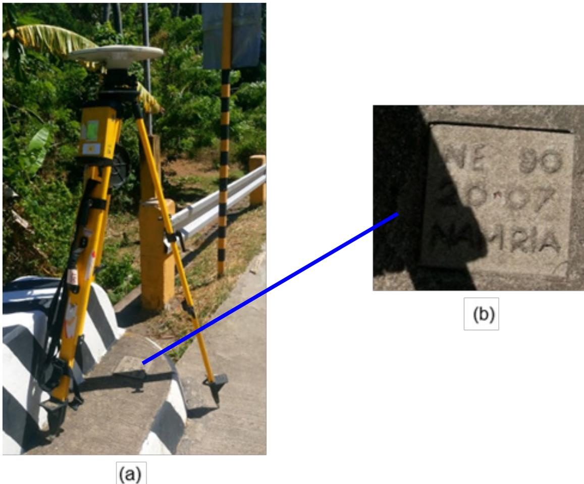
Figure 8. Set-up over NE-90 on a concrete sidewalk of Guinsuan Bridge, 4 meters from the road centerline in Barangay Poblacion under the municipality of Zamboanguita (a) and NAMRIA benchmark NE-90 (b) as recovered by the field team.
