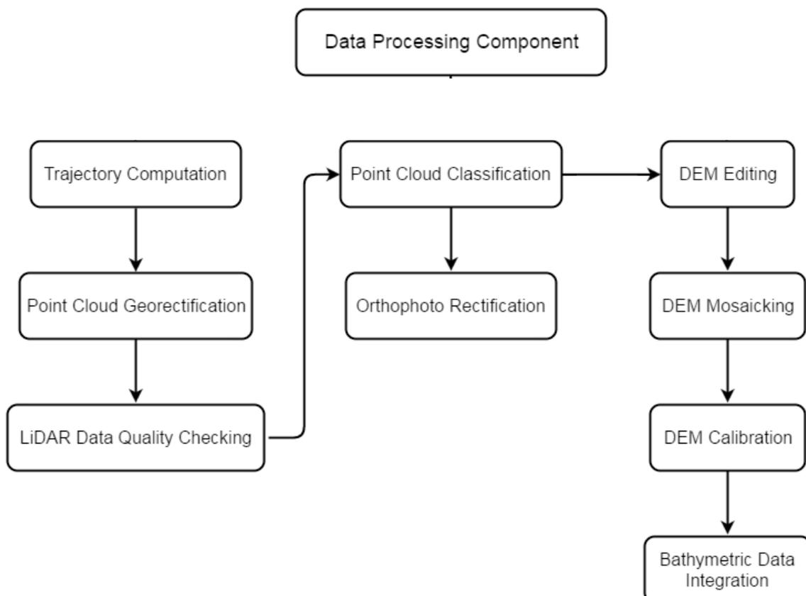
Figure 11. Schematic Diagram for Data Pre-Processing Component.
