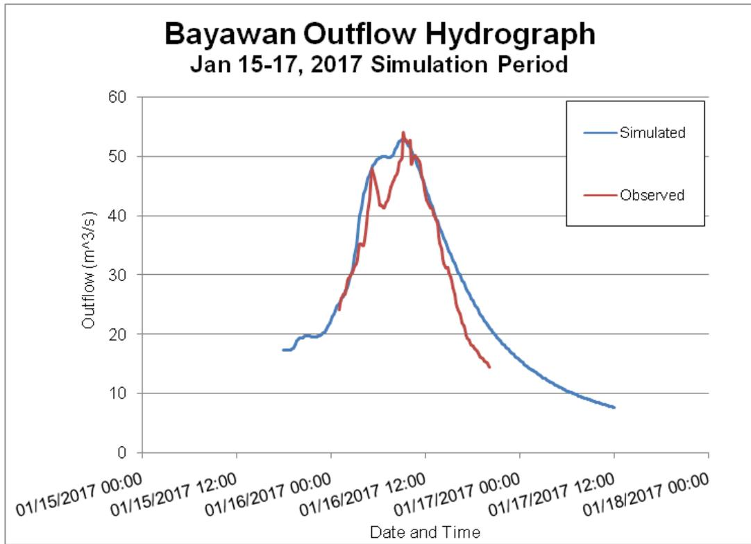
Figure 60. Outflow Hydrograph of Bayawan produced by the HEC-HMS model compared with observed outflow.
