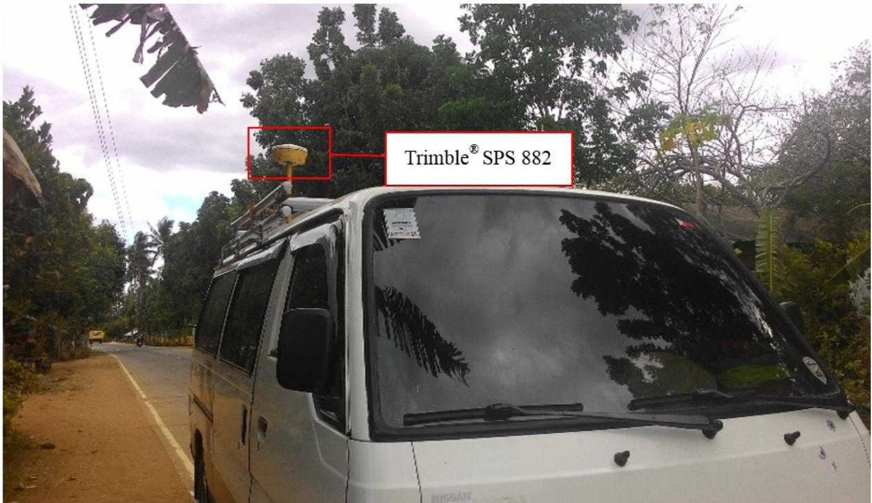
Figure 41. Validation points acquisition survey set-up.
