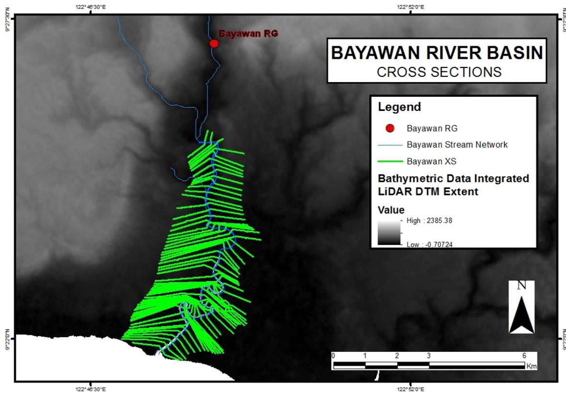
Figure 58. River cross-section of Bayawan River generated through Arcmap HEC GeoRAS tool.
