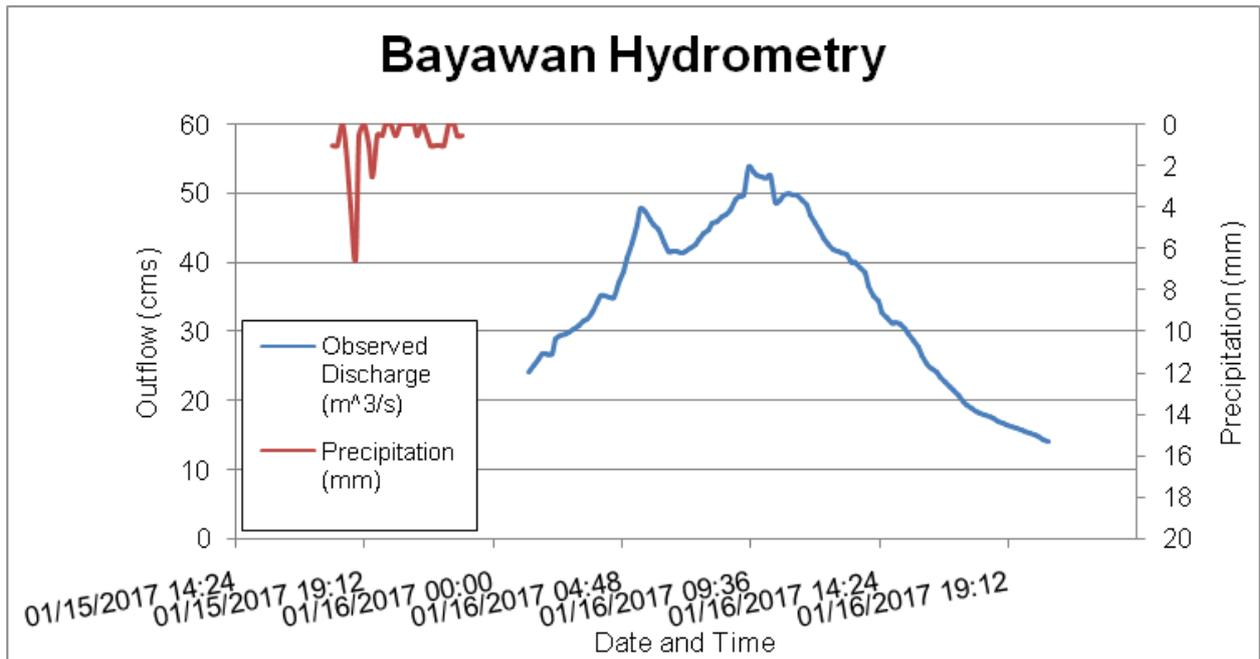
Figure 50. Rainfall and outflow data at Sitio Mantapi, Brgy. Nangka, Bayawan used for modeling.
