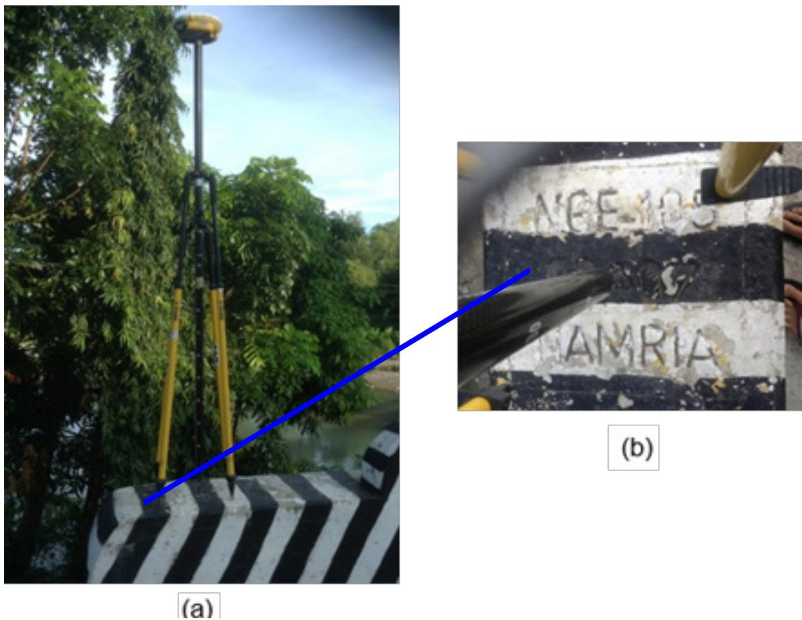
Figure 6. GPS set-up over NGE-105 at top of the bridge wingwall SW of the Bridge main span on the left side of the 1st approach coming from Siaton on the way to Sta. Catalina. The station is located in Barangay Nagbalayen under the municipality of Sta. Catalina (a) and NAMRIA reference point NGE-105 (b) as recovered by the field team.
