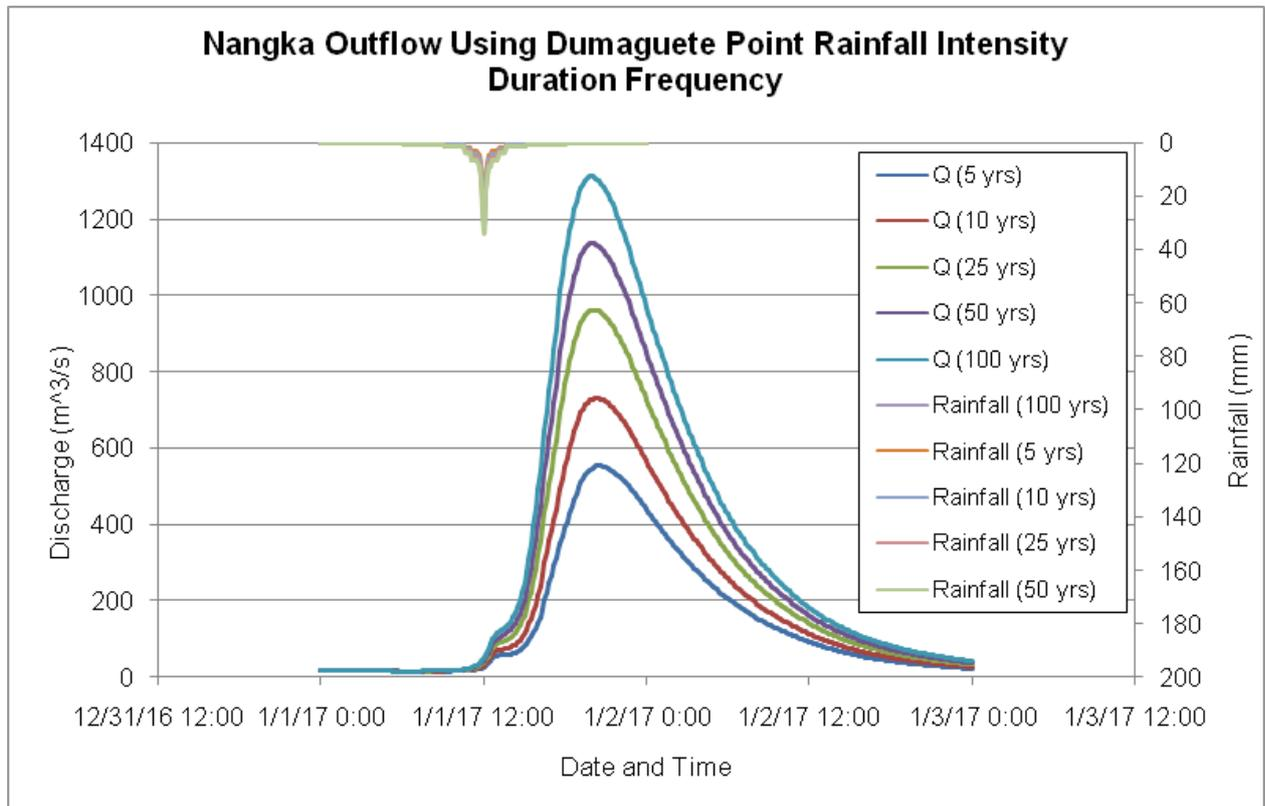
Figure 61. Outflow hydrograph at Sitio Mantapi, Brgy. Nangka, BayawanCity generated using Dumaguete PointRIDF simulated in HEC-HMS.
