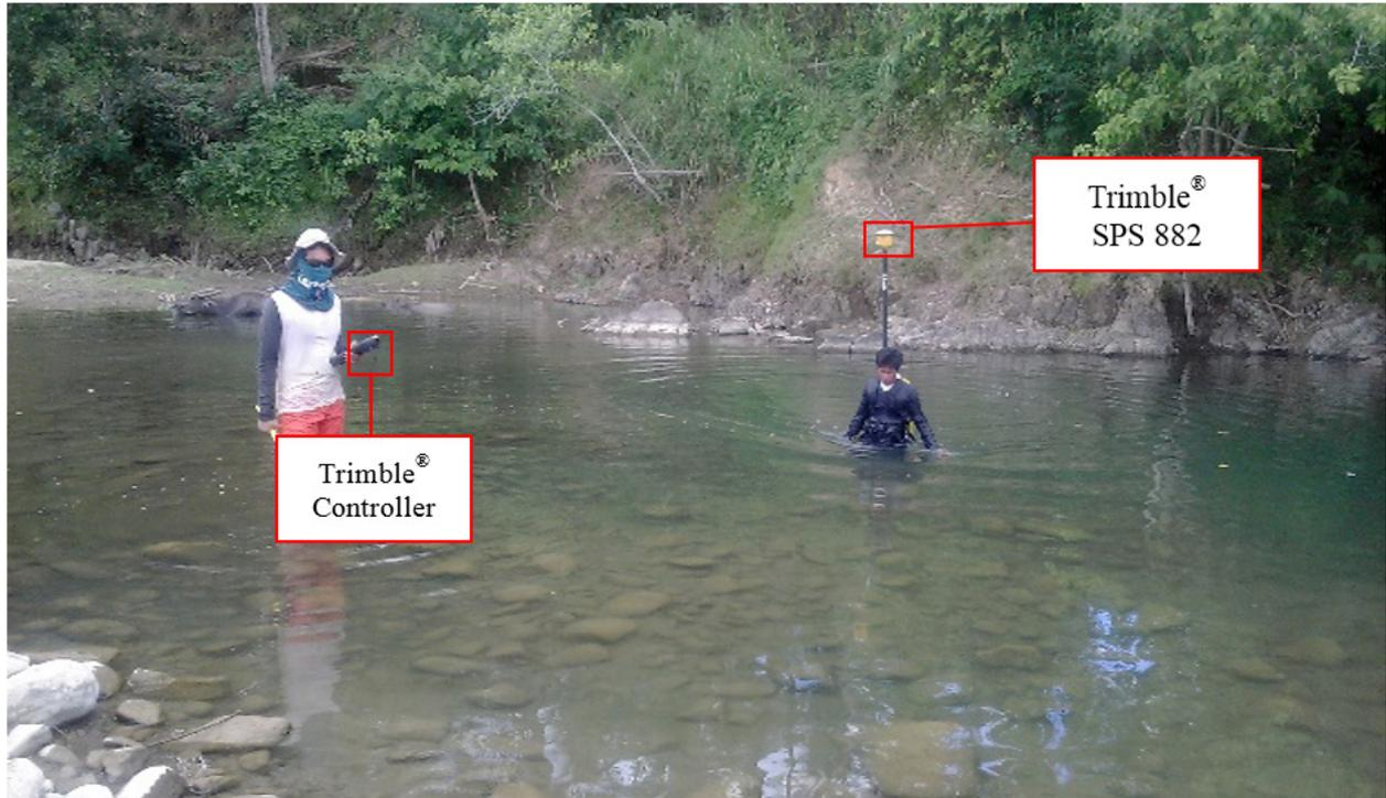
Figure 43. Manual Bathymetric Survey in Bayawan River.
