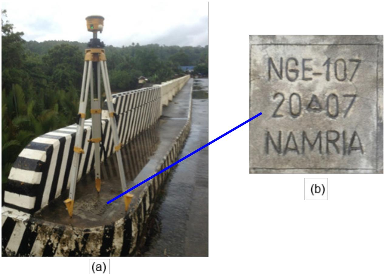
Figure 7. GPS set-up over NGE-107 on a concrete sidewalk on a bridge at KM. 80+569 over Manalongon River in Barangay Manalongon under the municipality of Sta. Catalina (a) and NAMRIA reference point NGE-107 (b) as recovered by the field team.
