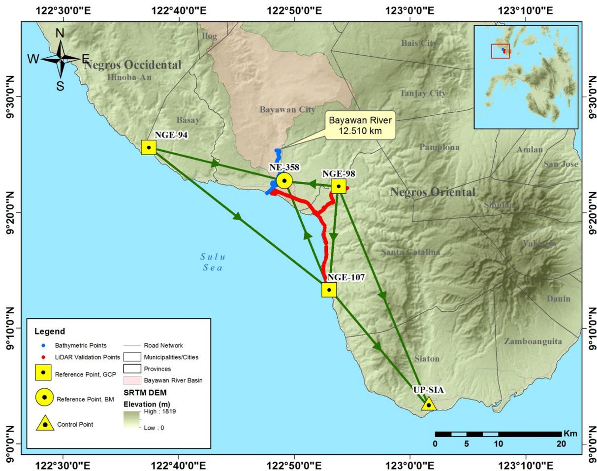
Figure 31. Extent of the bathymetric survey (blue) in Bayawan River and the LiDAR data validation survey (red).
