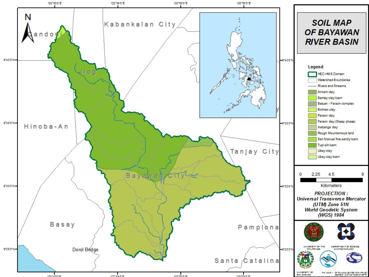
Figure 53. The soil map of the Bayawan River Basin used for the estimation of the CN parameter.
