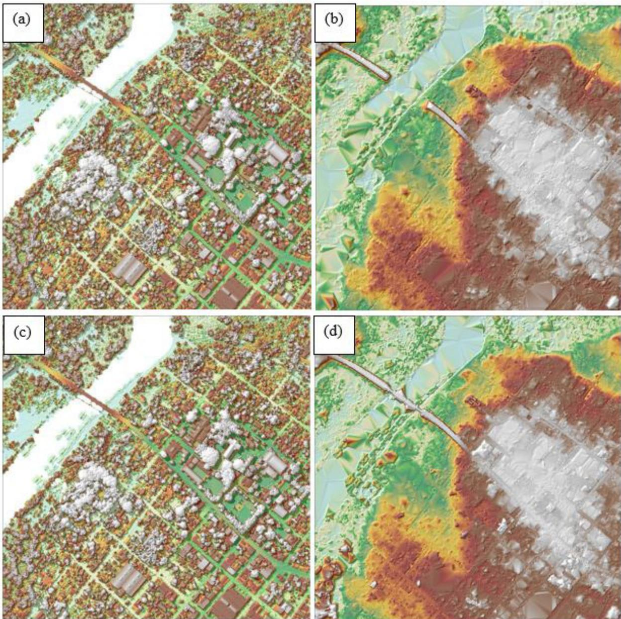
Figure 22. The production of last return DSM (a) and DTM (b) first return DSM (c) and secondary DTM (d) in some portion of Bayawan floodplain.
