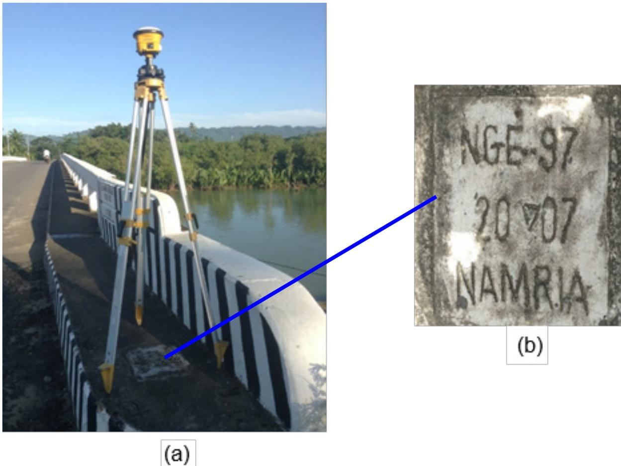
Figure 4. GPS set-up over NGE-97 on the SE corner concrete sidewalk of Bayawan Bridge in Barangay Suba under the municipality of Bayawan (a) and NAMRIA reference point NGE-97 (b) as recovered by the field team.
