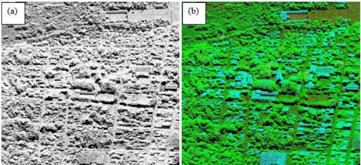
Figure 21. Point cloud before (a) and after (b) classification.
