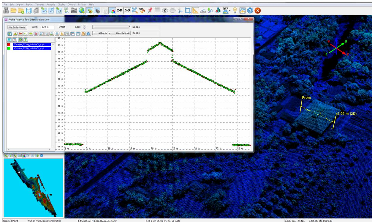
Figure 19. Quality checking for Bayawan flight 7578G using the Profile Tool of QT Modeler.
