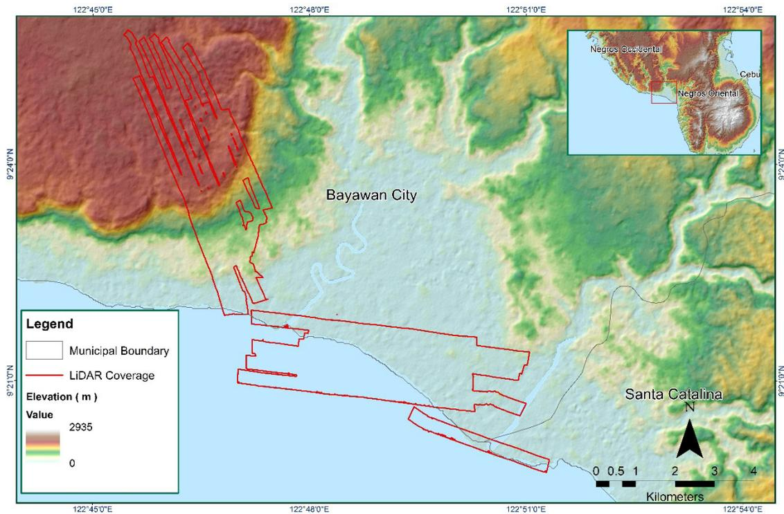
Figure 1.7.4 Coverage of LiDAR data
