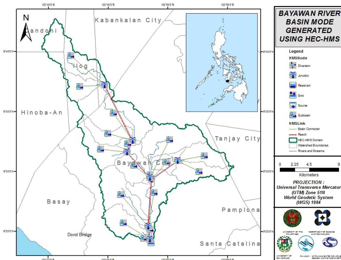
Figure 57. The Bayawan River Basin Model Domain generated using HEC-HMS.
