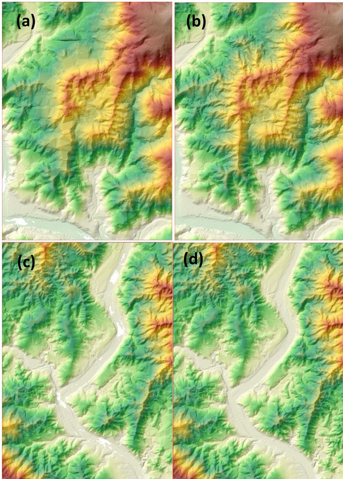
Figure 23. Portions in the DTM of Bayawan floodplain – an interpolated mountain before (a) and after (b) data retrieval; (c) before and (d) after filling data gaps.
