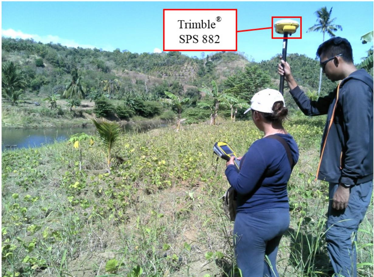
Figure 38. Cross-section survey conducted on Bawayan River in Brgy. Calabnugan, Municipality of Sibulan.
