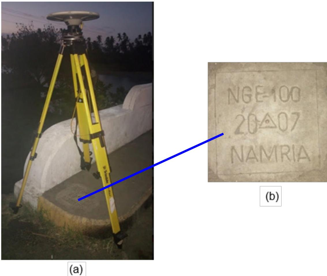
Figure 5. GPS set-up over NGE-100 on the SW of Cawitan Bridge, along Dumaguete-Bayawan national highway (a) and NAMRIA reference point NGE-100 (b) as recovered by the field team.
