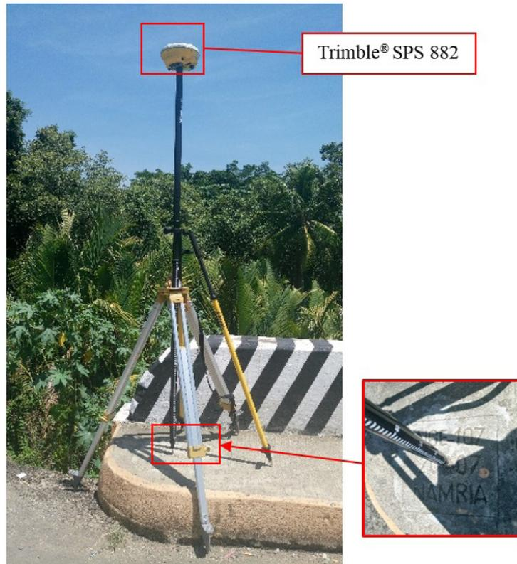
Figure 33. GNSS receiver set-up, Trimble® SPS 882, at NGE-107 at the approach of Manalongon Bridge in Brgy. Manalongon, Municipality of Santa Catalina, Negros Oriental.
