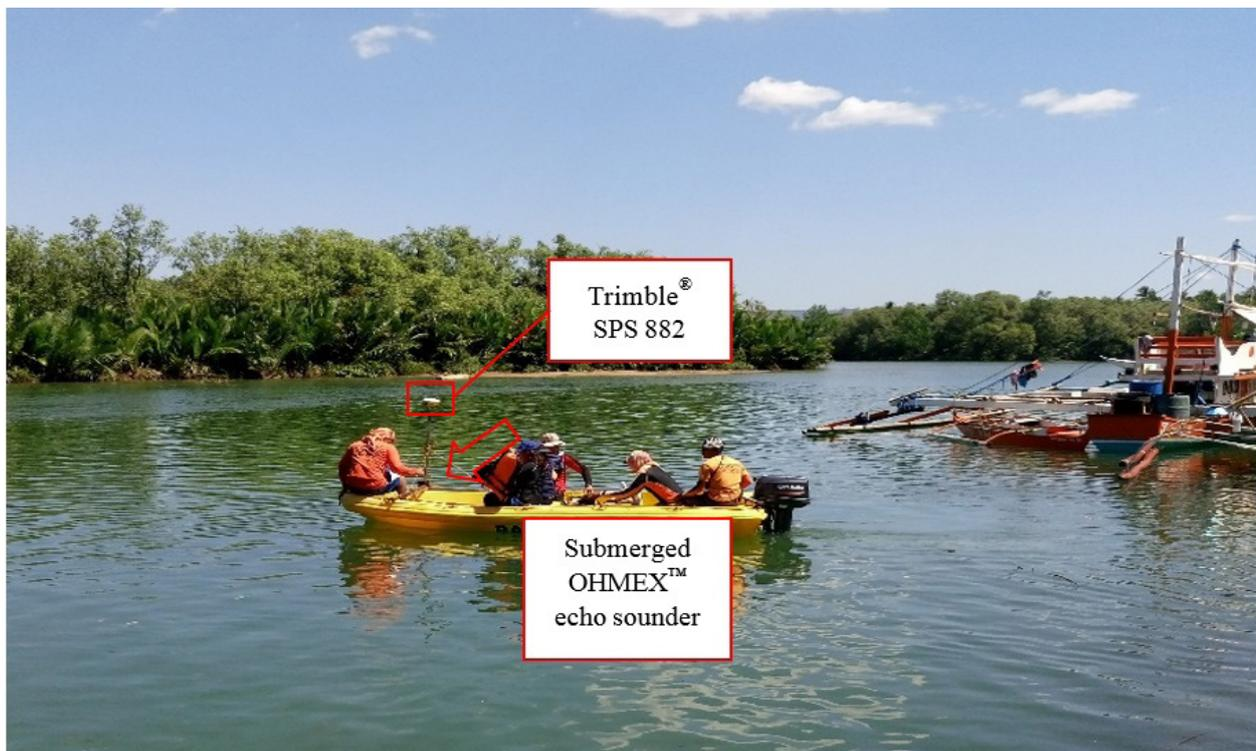
Figure 44. Bathymetric survey using the OHMEX Echosounder.
