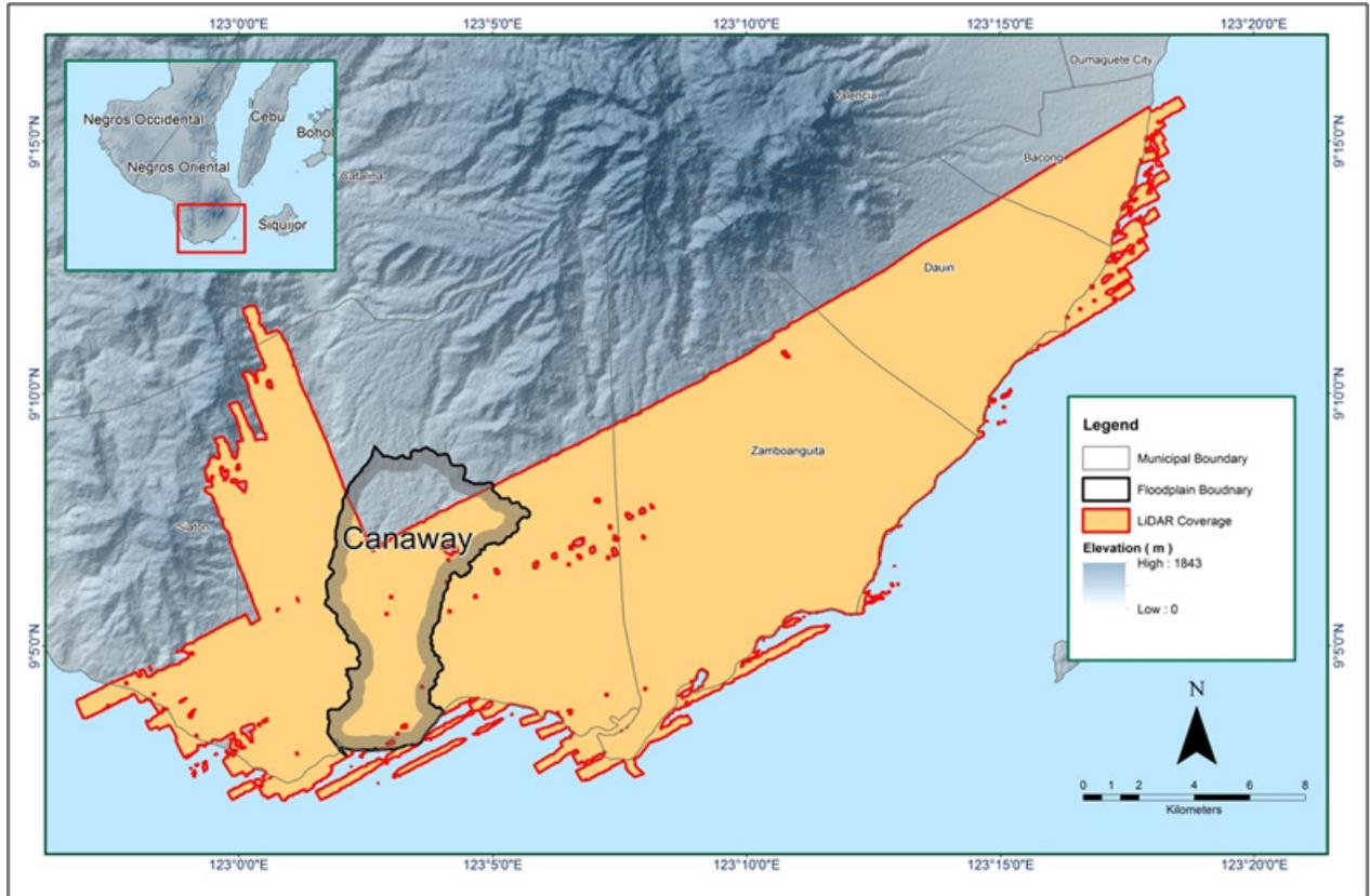
Figure 15. Boundary of the processed LiDAR data on top of a SAR Elevation Data over Canaway Floodplain.
