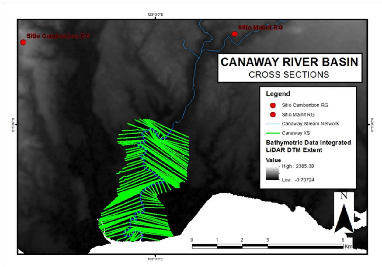
Figure 59 River cross-section of Canaway River generated through Arcmap HEC GeoRAS tool
