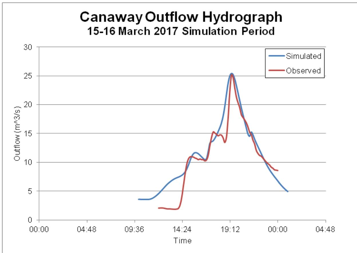
Figure 61 Outflow Hydrograph of Canaway produced by the HEC-HMS model compared with observed outflow
