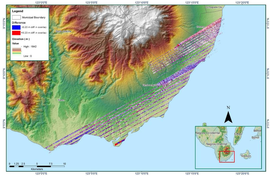
Figure A-8.21 Elevation difference between flight lines
