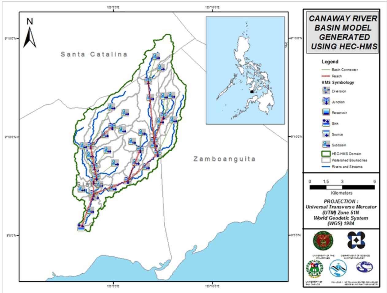
Figure 58 The Canaway River Basin Model Domain generated using HEC-HMS
