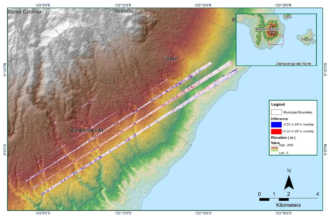
Figure A-8.37 Elevation difference between flight lines
