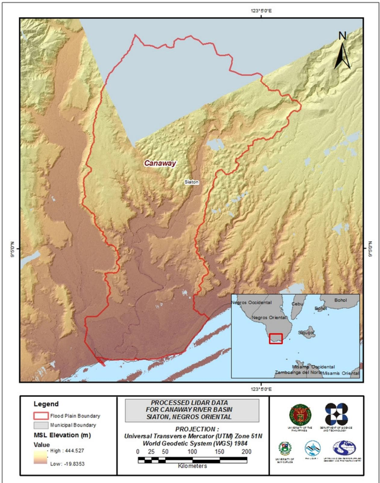
Figure 26. Map of Processed LiDAR Data for Canaway Floodplain
