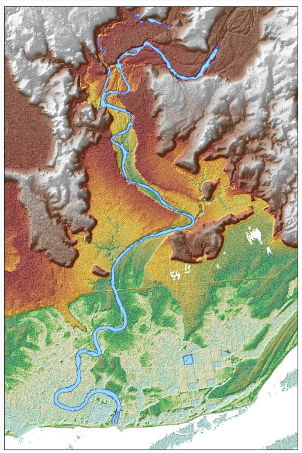
Figure 63 Sample output of Canaway RAS Model
