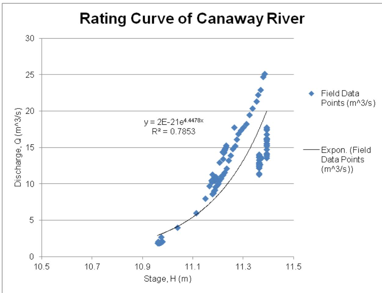
Figure 50 Rating Curve at Canaway River
