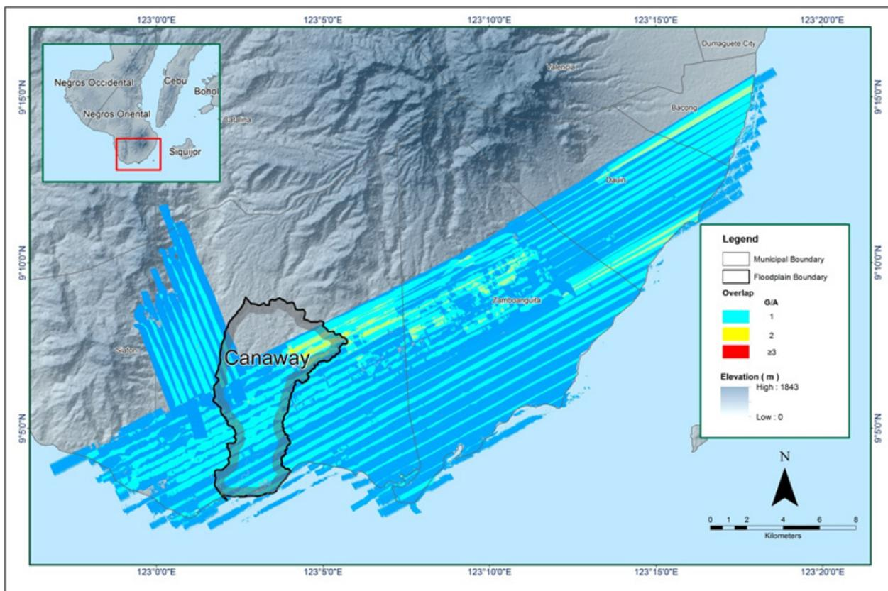
Figure 16. Image of data overlap for Canaway Floodplain
