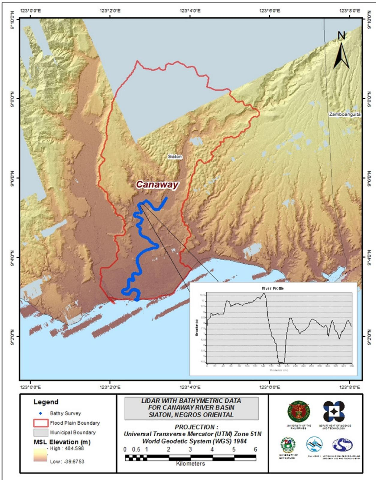
Figure 30. Map of Canaway Floodplain with bathymetric survey points shown in blue
