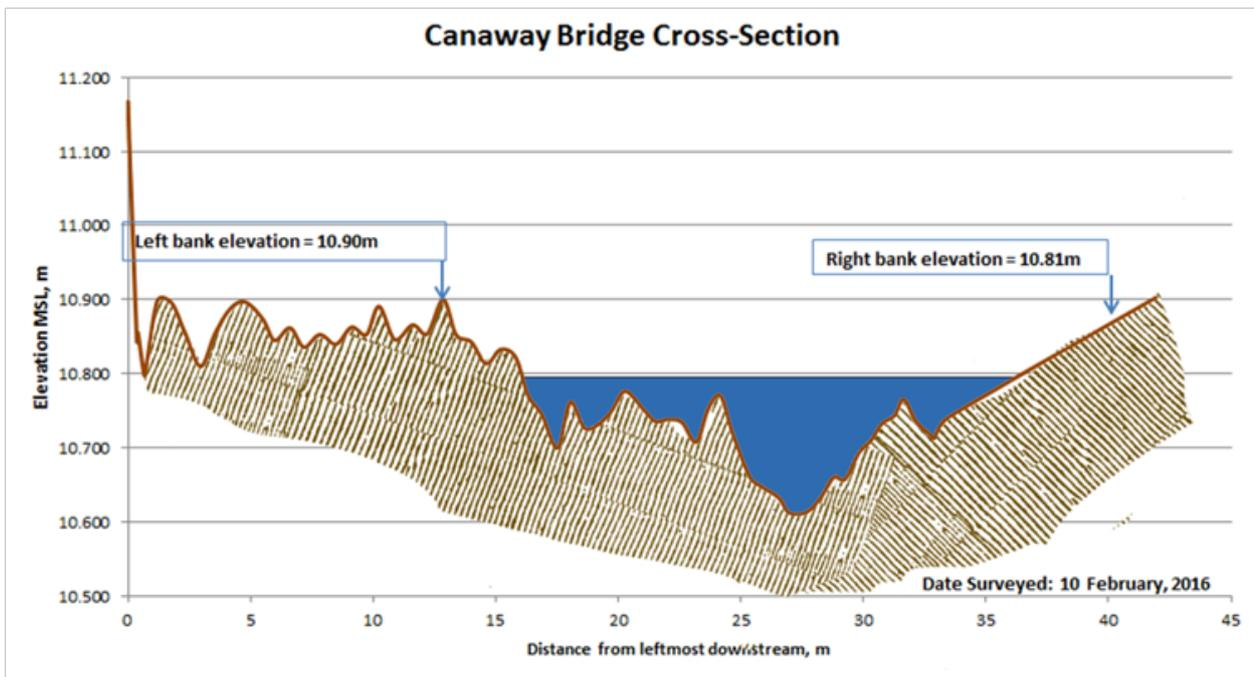
Figure 49 Cross-Section Plot of Canaway Bridge
