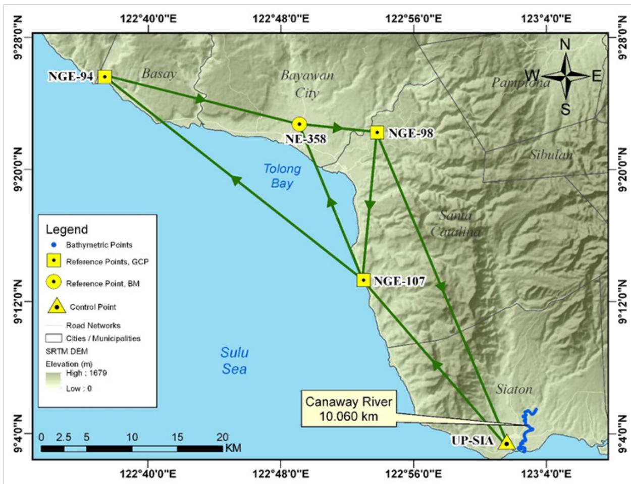
Figure 34 GNSS Network of Canaway River field survey
