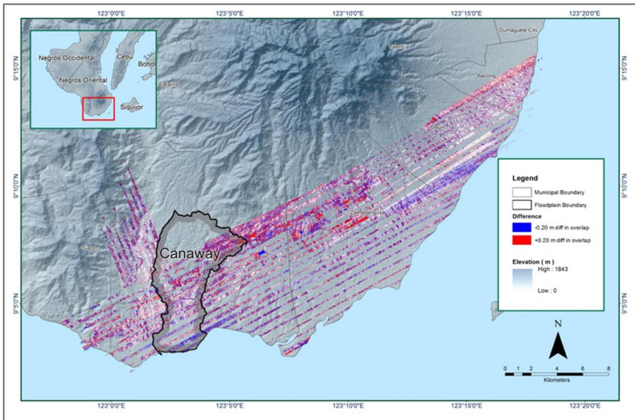
Figure 18. Elevation difference map between flight lines for Canaway Floodplain
