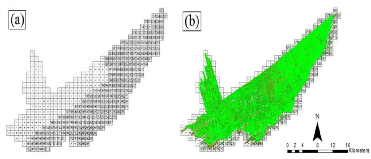
Figure 20. Tiles for Canaway Floodplain (a) and classification results (b) in TerraScan
