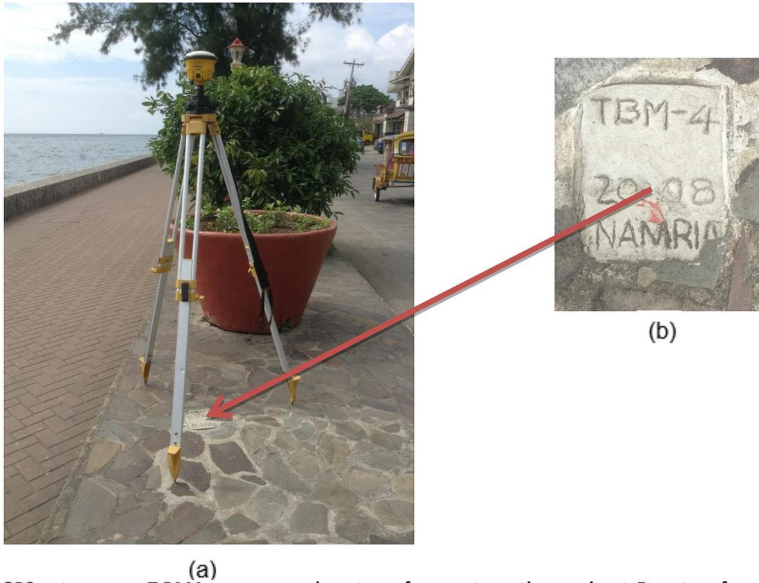
Figure 8 GPS set-up over T-BM4 as recovered on top of concrete pathway about 5 meters from the seawall of Dumaguete City’s boulevard (a) and NAMRIA benchmark T-BM4 (b) as recovered by the field
