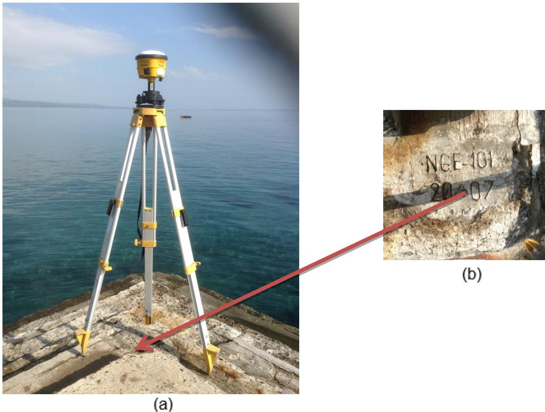
**Figure 5** GPS set-up over NGE-101 on the third step from the top flooring of the pier NE corner in Barangay Poblacion under the Municipality of Sibulan (a) and NAMRIA reference point NGE-101 (b) as recovered by the field team
