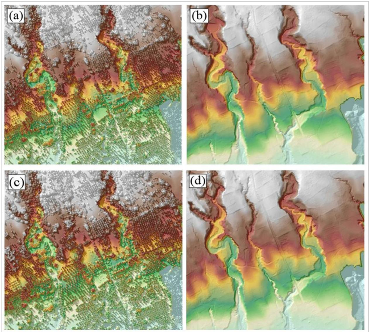
Figure 22. The Production of last return DSM (a) and DTM (b), first return DSM (c) and secondary DTM (d) in some portion of Canaway Floodplain
