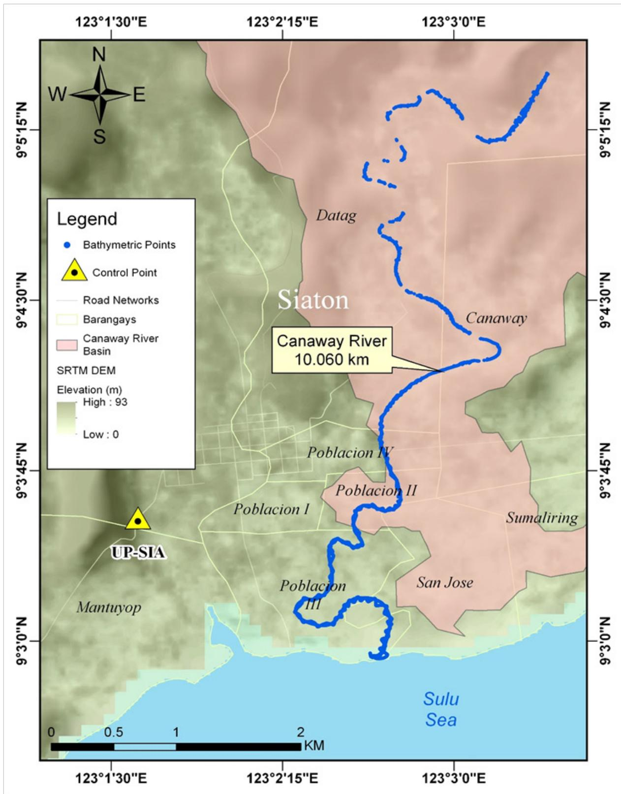
Figure 46 Bathymetric survey of Canaway River
