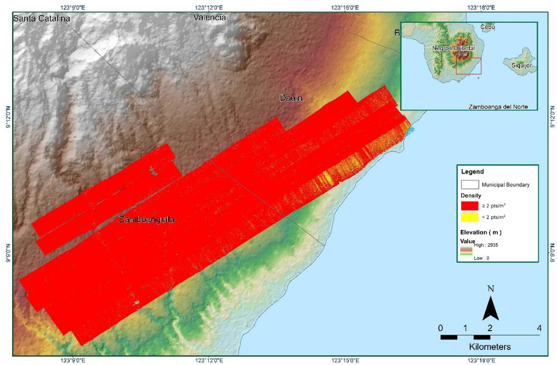
Figure A-8.36 Density map of merged LiDAR data
