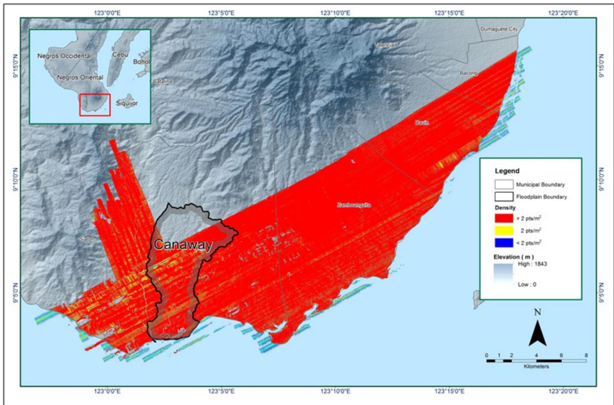
Figure 17. Density map of merged LiDAR data for Canaway Floodplain
