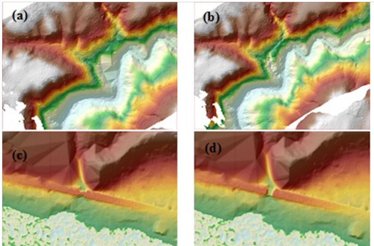
Figure 25. Portions in the DTM of Canaway Floodplain – interpolated area (a) before and (b) after data retrieval; a bridge (c) before and (d) after manual editing.
