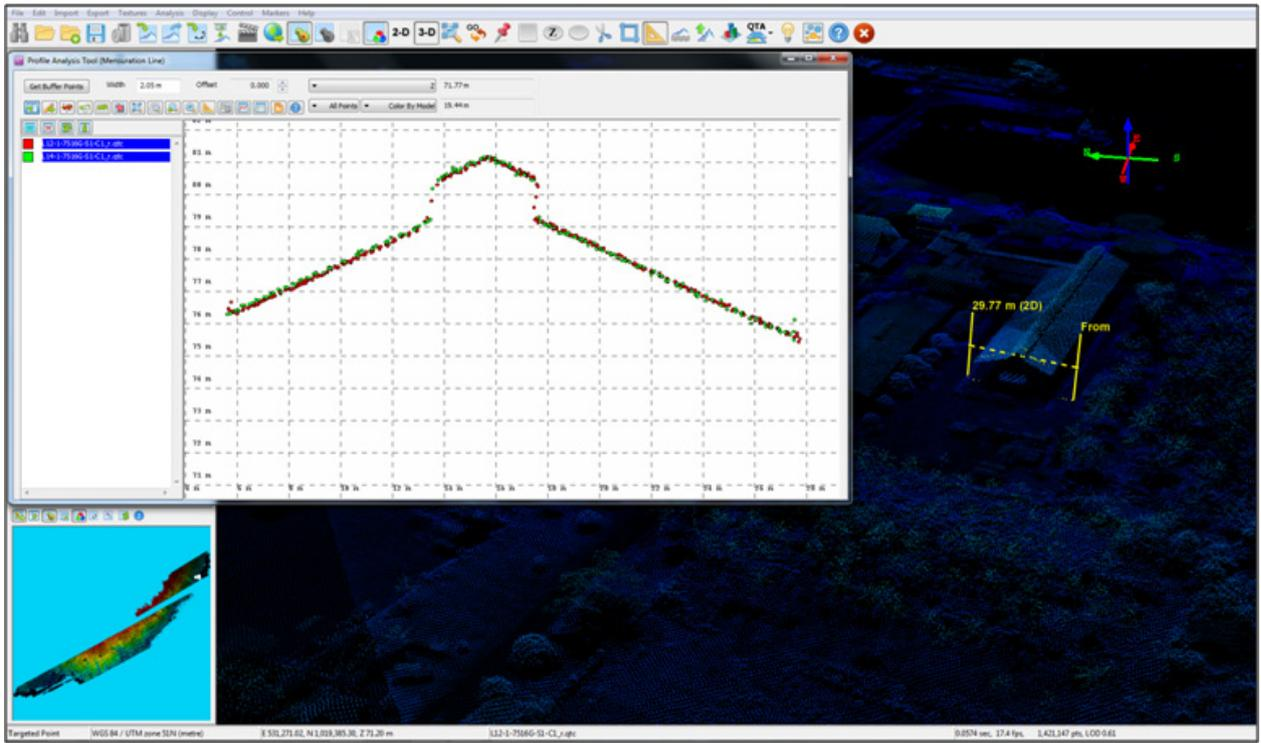
Figure 19. Quality checking for a Canaway flight 7516G using the Profile Tool of QT Modeler
