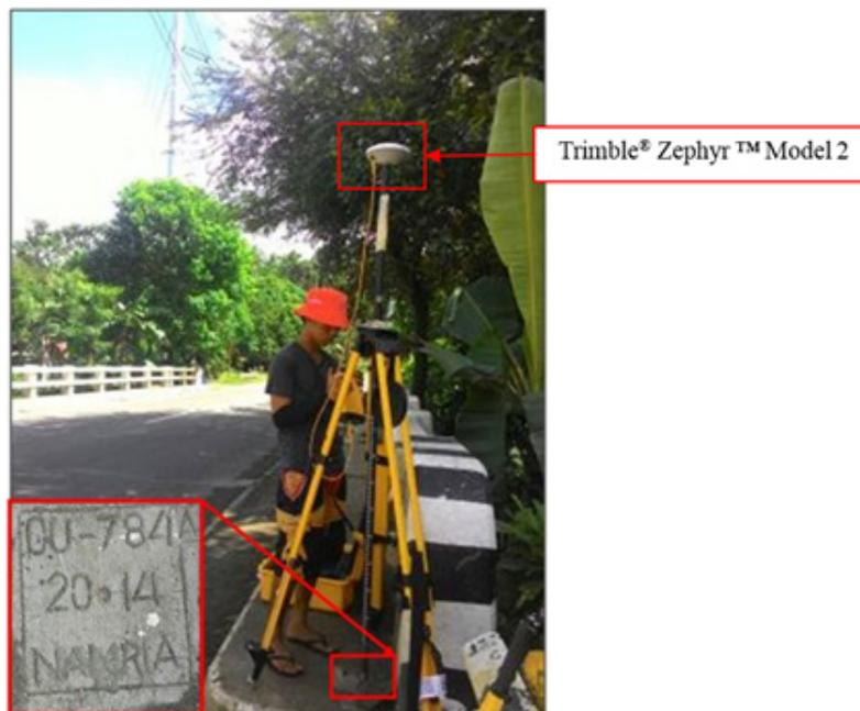
Figure 35. GNSS receiver setup, Trimble® Zephyr™ Model 2, at CU-784 Balud Bridge approach in Brgy. Balud, Toledo City, Cebu.
