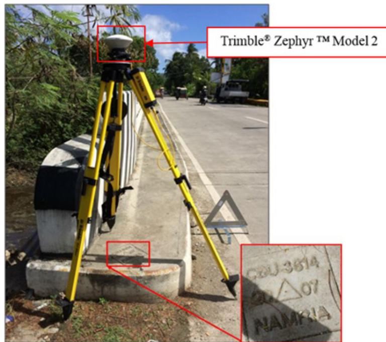
Figure 36. GNSS base receiver setup, Trimble® Zephyr™ Model 2, at CBU-3614, Lapu-Lapu Bridge approach in Brgy. Poblacion, Municipality of Asturias, Cebu.
