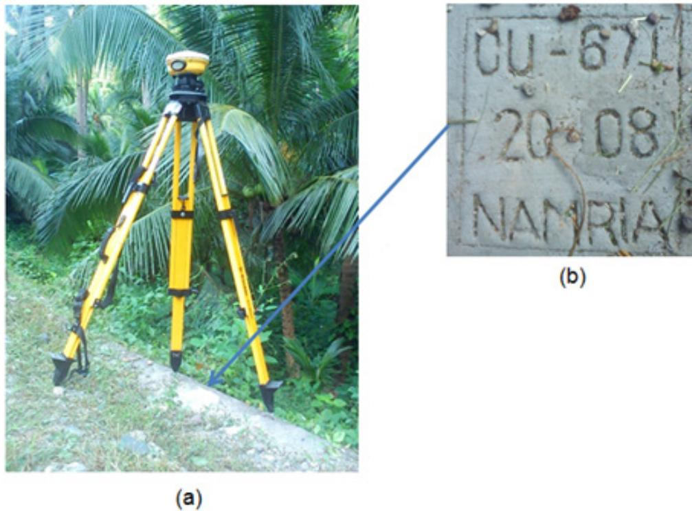
Figure 8. GPS set-up over CU-671 at the right side of the National Road going to Argao Town Proper in Barangay Liki, Sogod, Cebu (a) and NAMRIA reference point CU-671 (b) as recovered by the field team.
