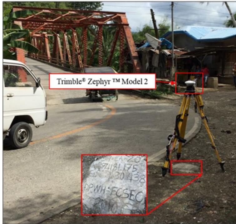
Figure 40. GNSS base receiver setup, Trimble® Zephyr™ Model 2, at DPWHECS in Brgy. Bago, Municipality of Asturias.
