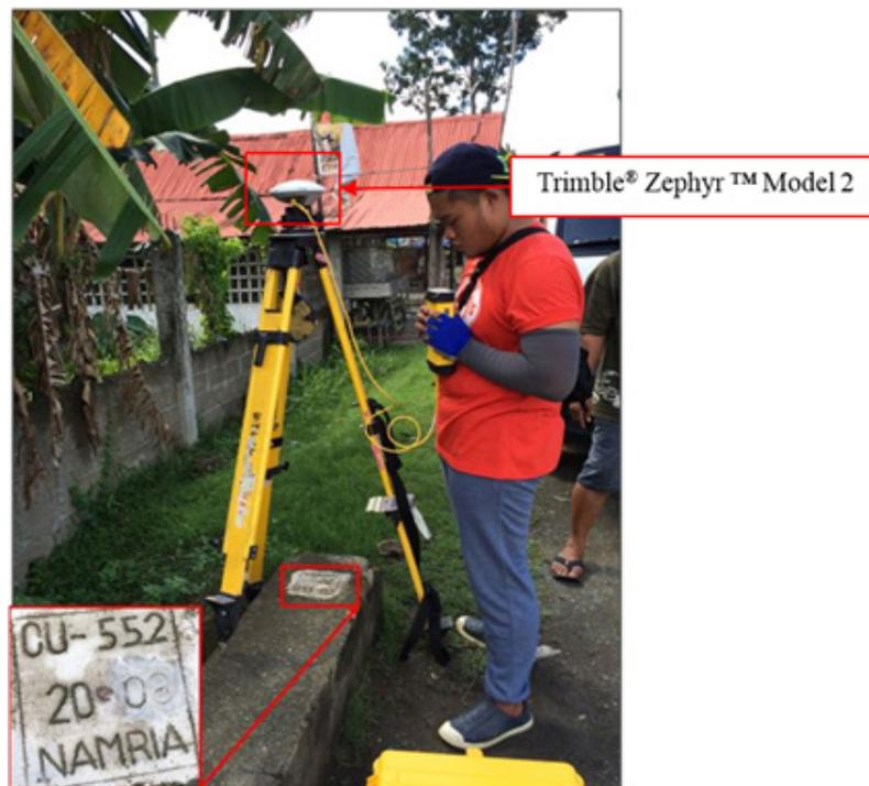
Figure 37. GNSS base setup, Trimble® Zephyr™ Model 2, at CU-552 in Brgy. Cantu-od, Municipality of Balamban.
