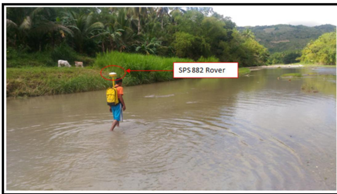
Figure 48. Set up of the bathymetric survey at Guinabasan River.
