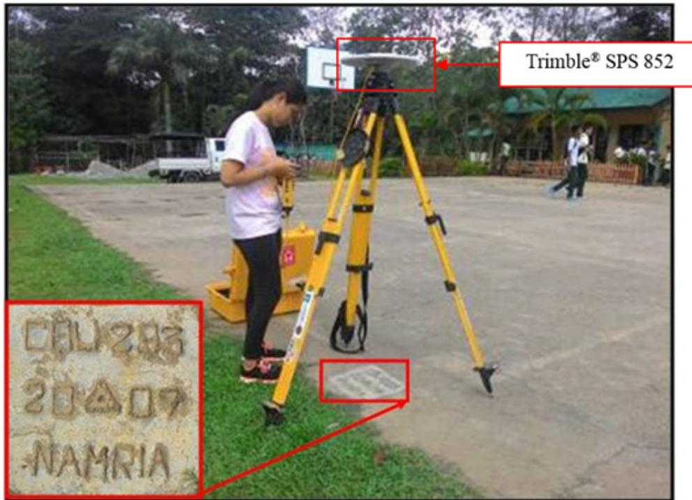
Figure 34. GNSS receiver set-up, Trimble® SPS 852, at CBU-293 in front of Cantabaco National High School in Brgy. Cantabaco, Toledo City, Cebu.
