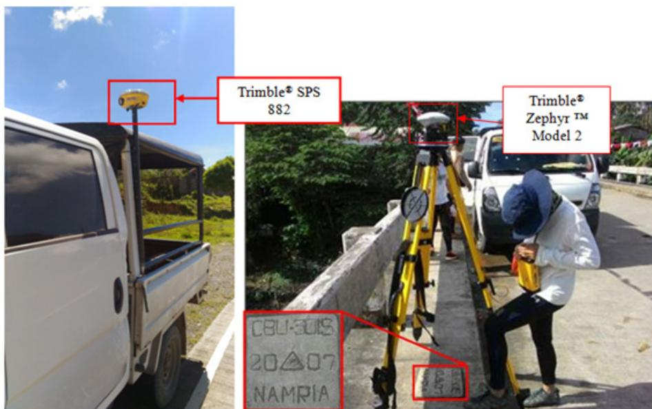
Figure 46. GNSS Receiver Trimble® SPS 882 installed on a vehicle for Ground Validation Survey.
