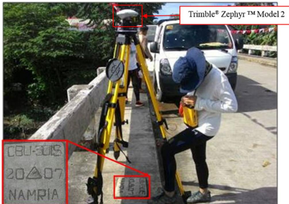
Figure 39. GNSS base setup, Trimble® Zephyr™ Model 2, at CBU-3015 in Santa Lucia Bridge, Brgy. Santa Lucia, Municipality of Asturias.
