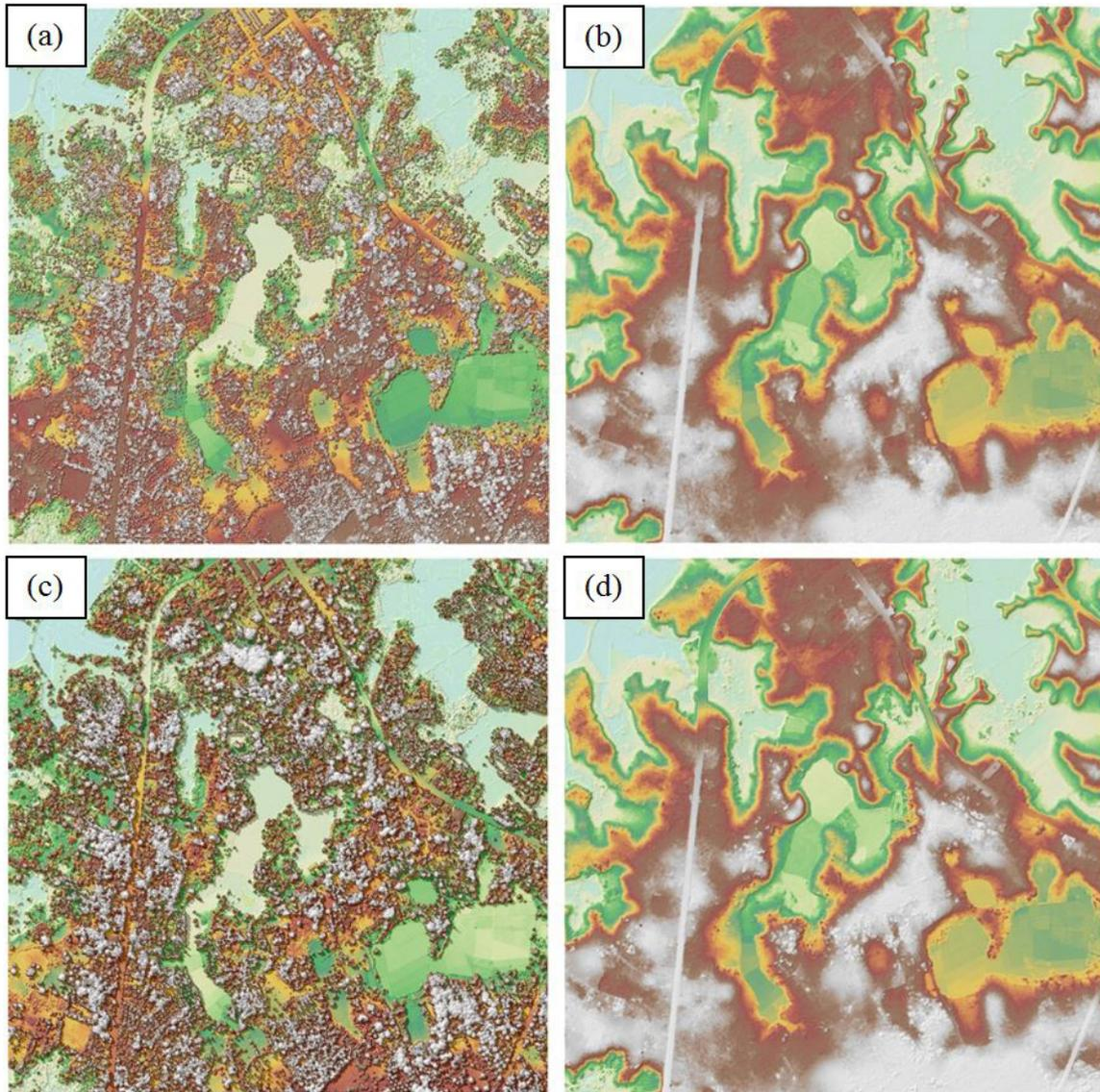
Figure 17. The production of last return DSM (a) and DTM (b), first return DSM (c) and secondary DTM (d) in some portion of Inabanga floodplain.
