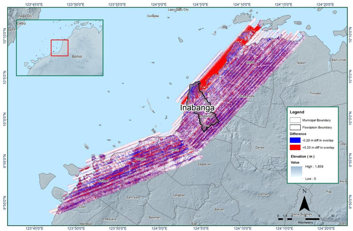
Figure 13. Elevation difference Map between flight lines for the Inabanga Floodplain Survey.
