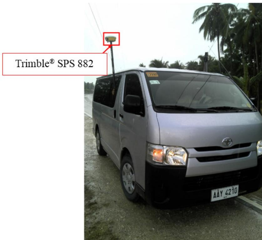
Figure 38. GNSS Receiver Trimble® SPS 882 installed on a vehicle for Ground Validation Survey.
