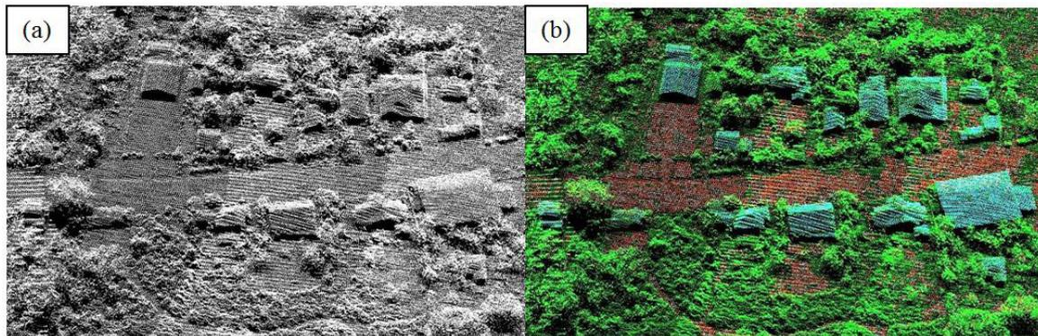
Figure 16. Point cloud before (a) and after (b) classification.
