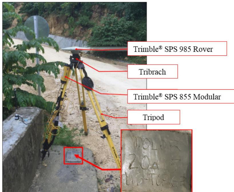
Figure 30. GNSS receiver set up, Trimble® SPS 985 at control point DOLOR, located at the left most (facing downstream) Baguhan Bridge approach, across Inabanga River located in Brgy. Dorol, Municipality of Angilan, Bohol.
