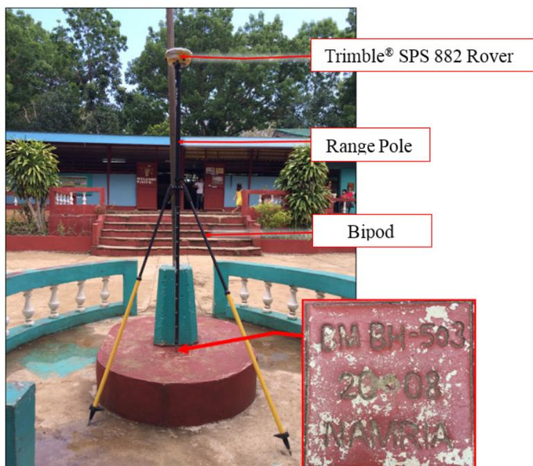
Figure 29. GNSS receiver set up, Trimble® SPS 882 at BH-503 located inside the campus of Dao Elementary School, Brgy. Dao, Municipality of Dauis, Bohol.
