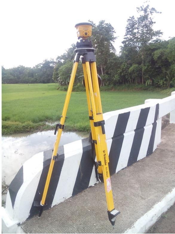
Figure 4. GPS set-up over established point BHL-63A in Hagbuyo Bridge, Brgy, Hagbuyo, San Miguel, Bohol (a).
