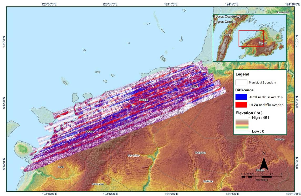
Figure 1.5.7. Elevation difference between flight line
