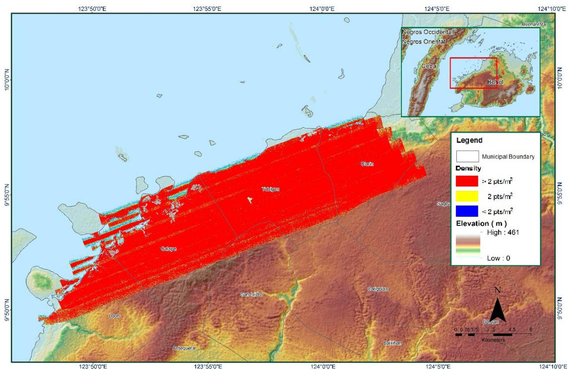
Figure 1.5.6. Density map of merged LiDAR data
