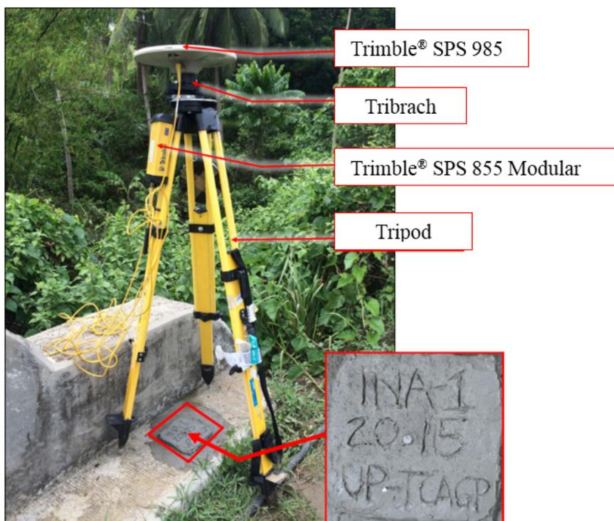
Figure 31. GNSS receiver set up, Trimble® SPS 985 at INA-1 at the Inabanga Bridge approach, Brgy. Baguhan, Inabanga, Bohol.
