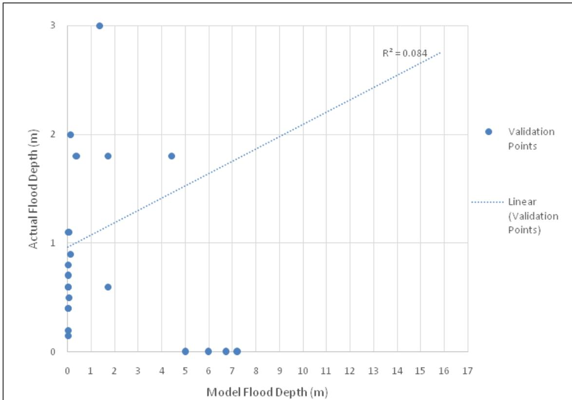
Figure 78. Flood Map depth versus Actual Flood Depth.
