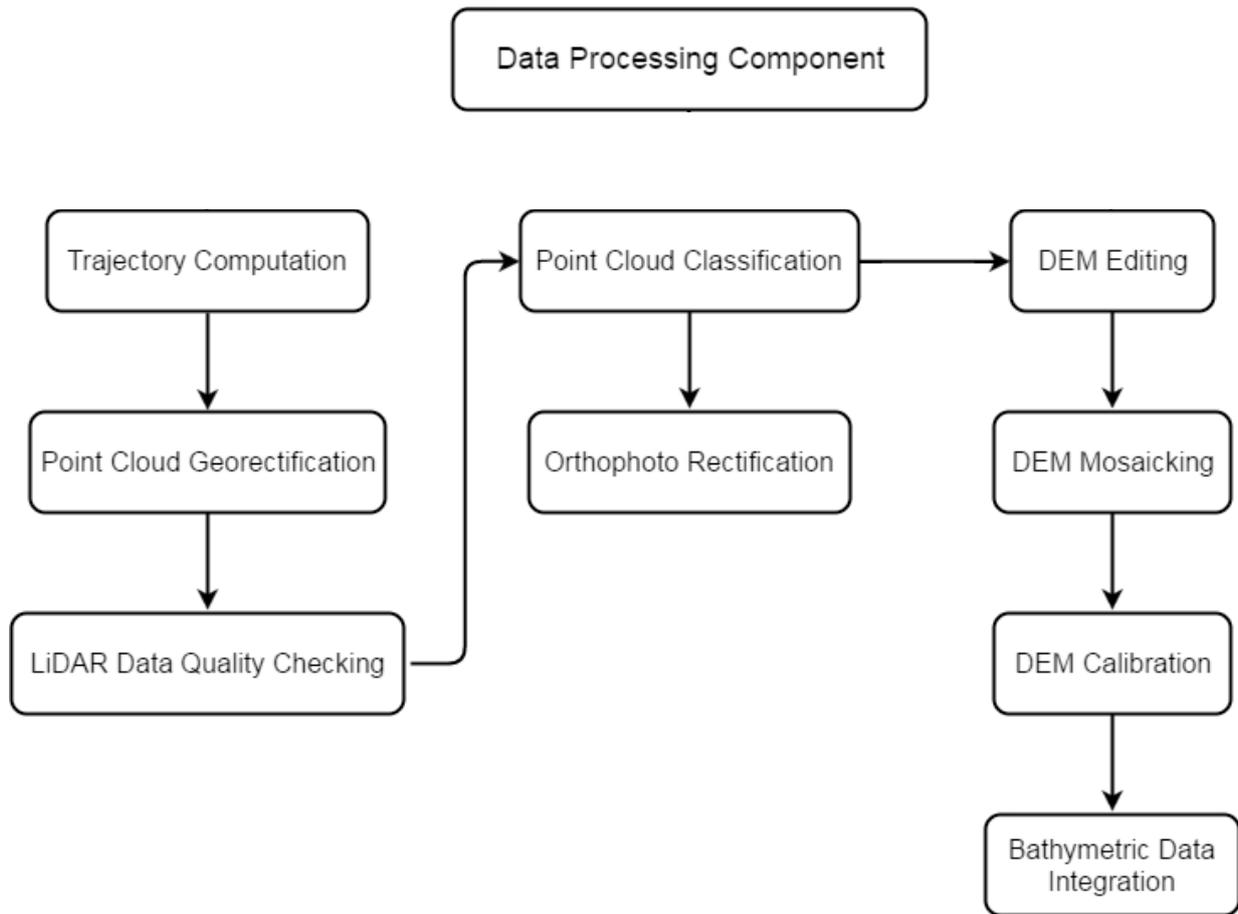
Figure 6. Schematic diagram for the data pre-processing.
