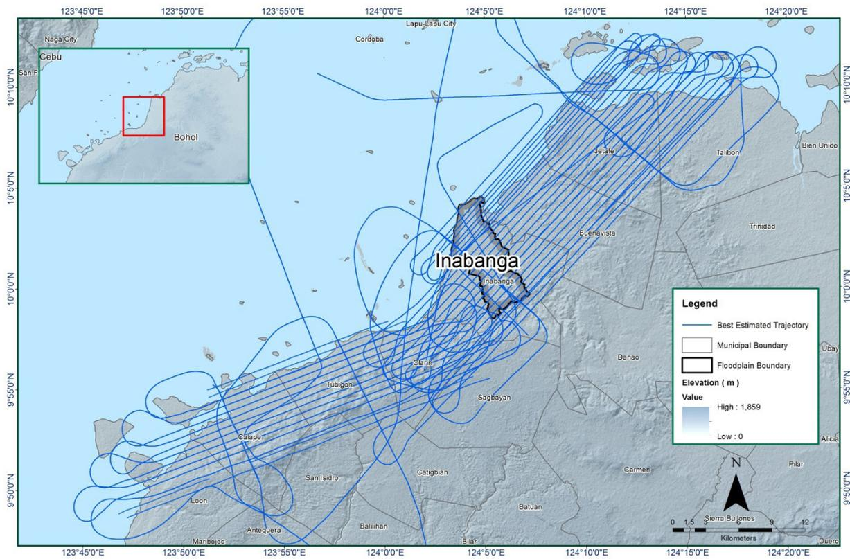
Figure 9. Best Estimated Trajectory of the LiDAR missions conducted over the Inabanga Floodplain.
