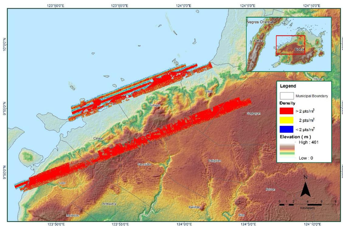
Figure 1.4.4. Density map of merged LiDAR data
