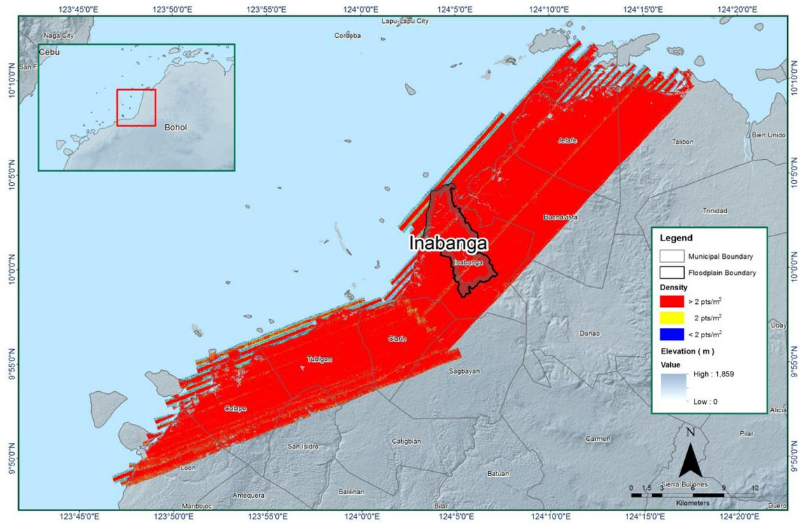
Figure 12. Pulse density map of the merged LiDAR data for Inabanga floodplain.
