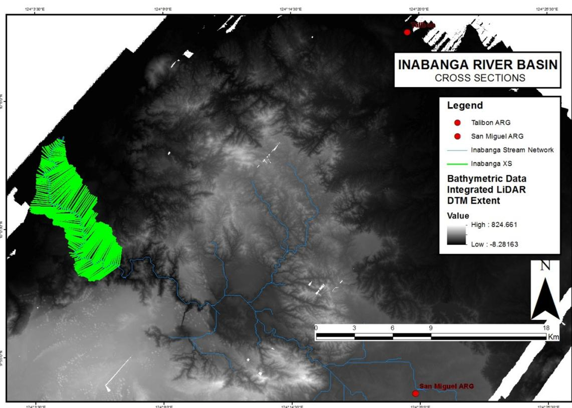
Figure 54. River cross-section of the Inabanga River through the ArcMap HEC GeoRas tool.
