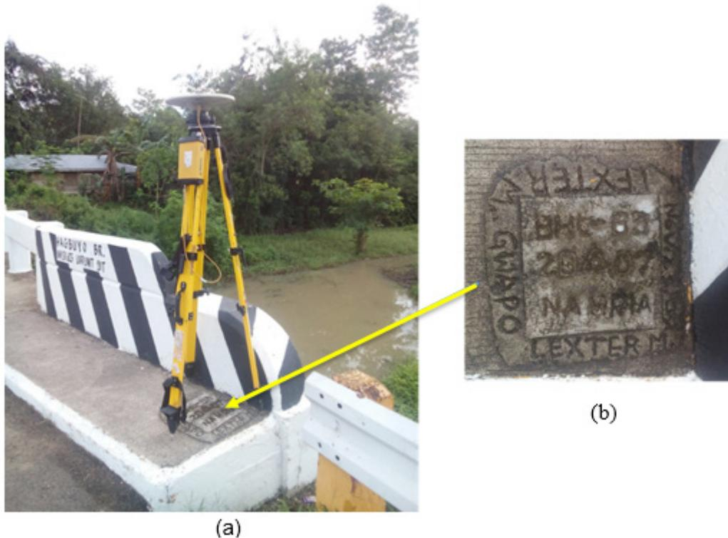
Figure 3. GPS set-up over BHL-63 in Hagbuyo Bridge in Brgy. Hagbuyo, San Miguel, Bohol (a) and NAMRIA reference point BHL-63 (b) as recovered by the team.
