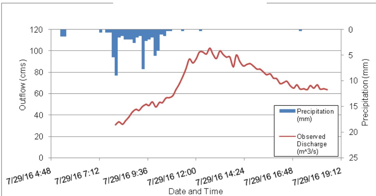
Figure 46. Rainfall and outflow data at Baguhan Bridge, which was used for modeling.
