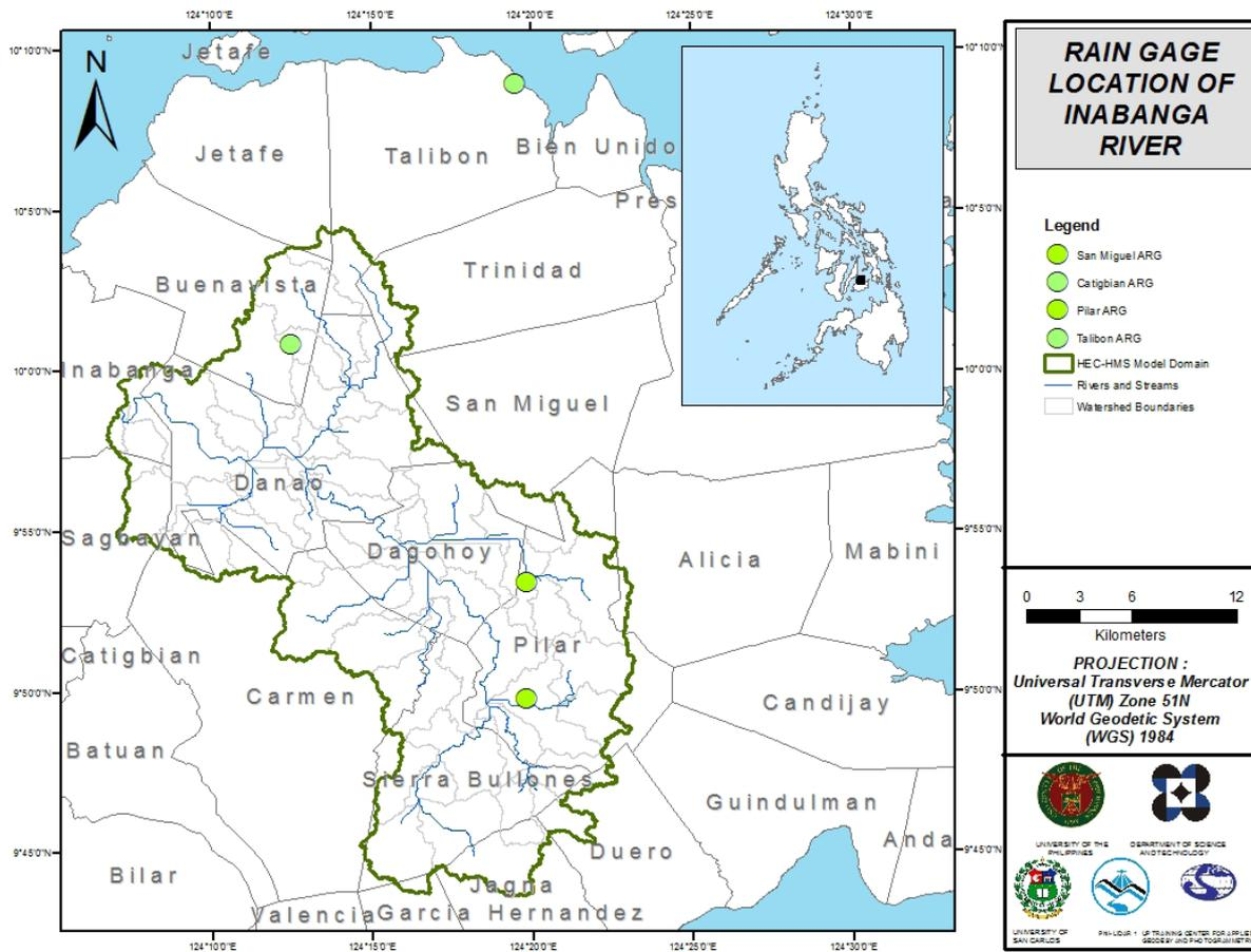
Figure 43. Location Map of the Inabanga HEC-HMS model used for calibration.
