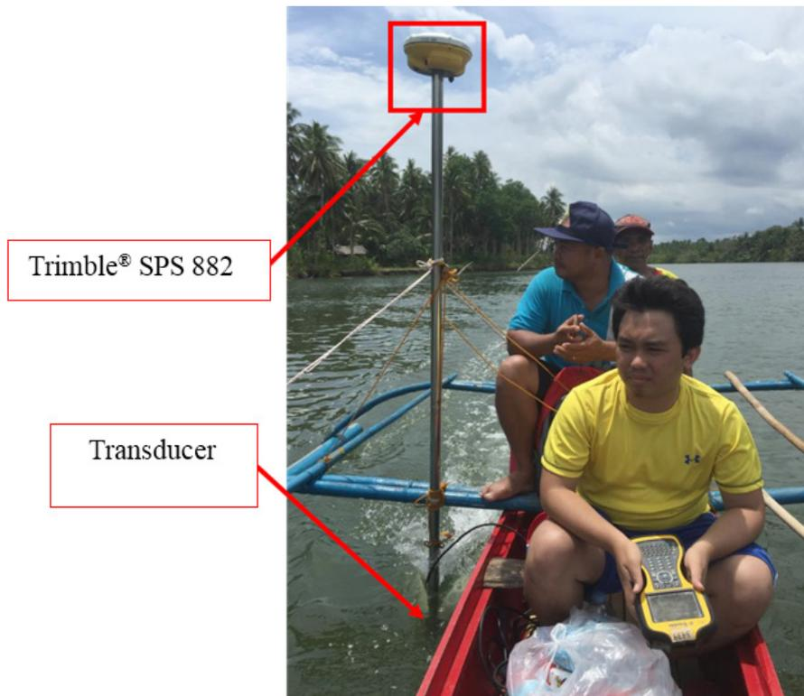
Figure 40. Set up of the bathymetric survey at Inabanga River using Trimble® SPS 882 in GNSS PPK survey technique.
