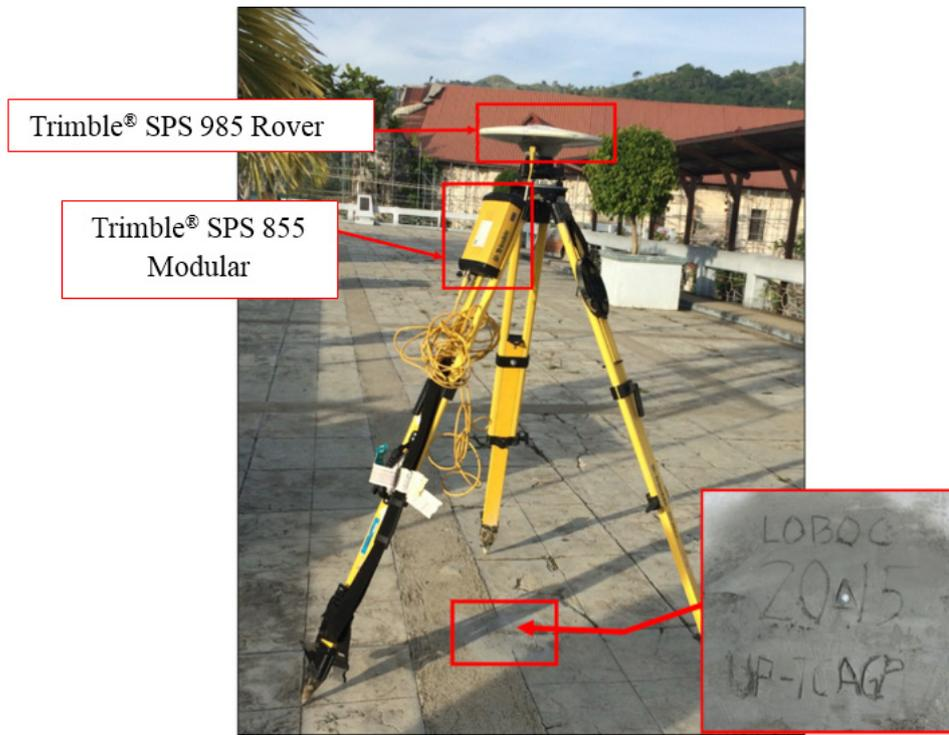
Figure 32. GNSS receiver set up, Trimble® SPS 852 on LOBOC, located on the incomplete bridge across the Loboc River near the municipality town plaza of Loboc in Brgy. Poblacion.
