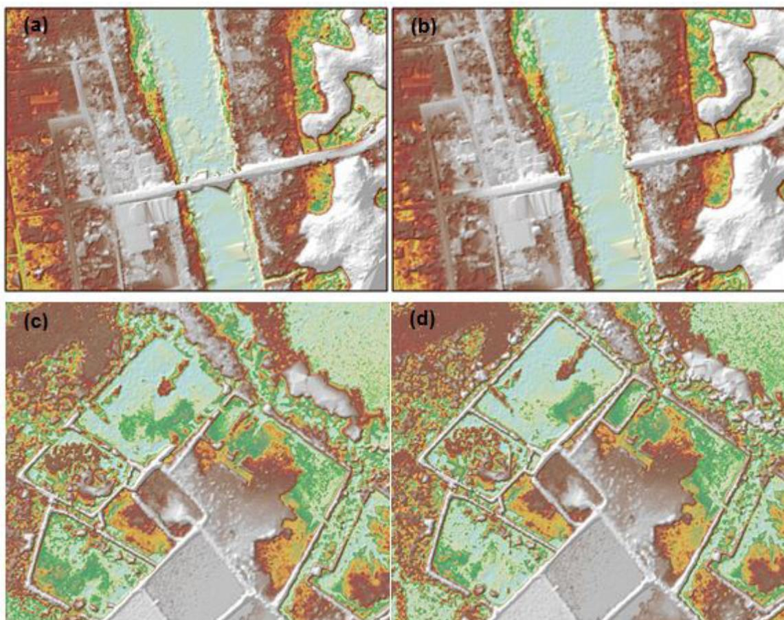
Figure 18. Portions in the DTM of the Inabanga Floodplain – a bridge before (a) and after (b) manual editing; a paddy field before (c) and after (d) data retrieval.
