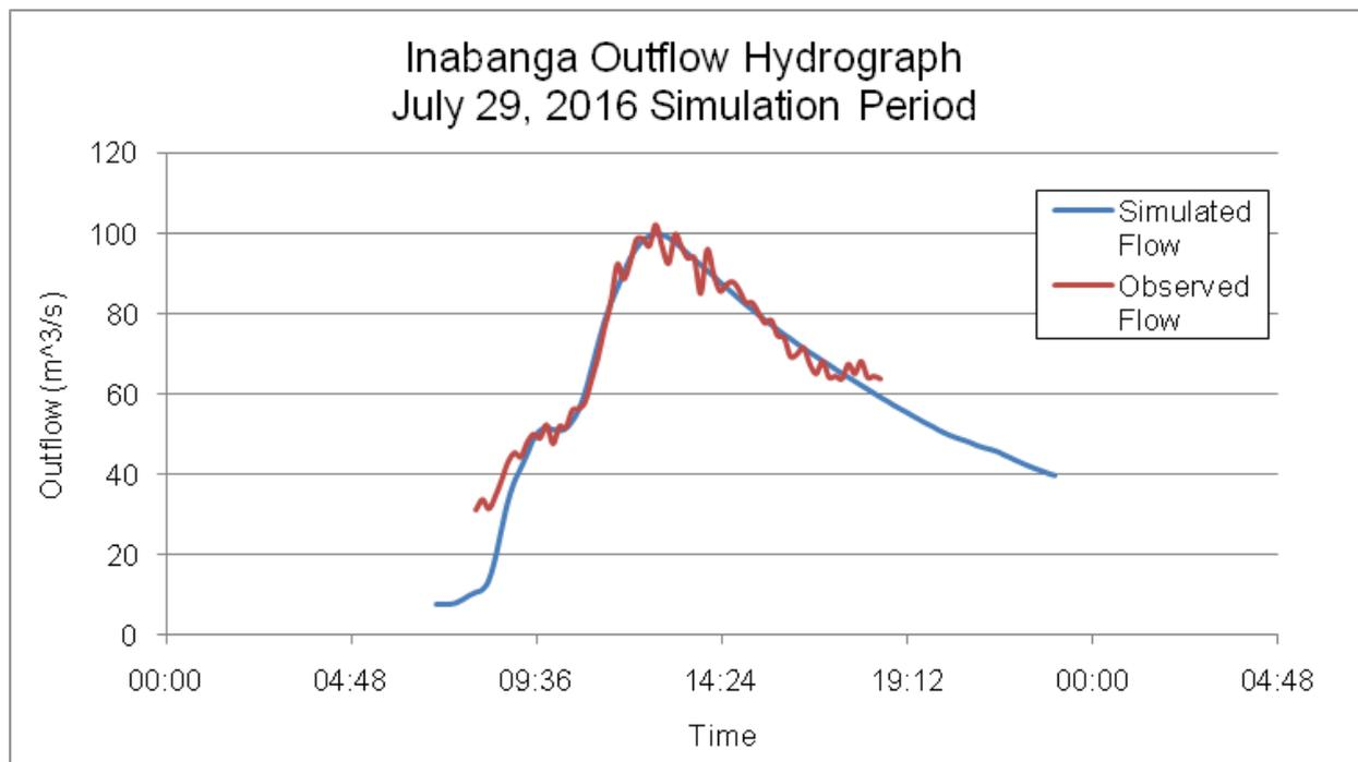
Figure 56. Outflow Hydrograph of Inabanga produced by the HEC-HMS model compared with observed outflow.
