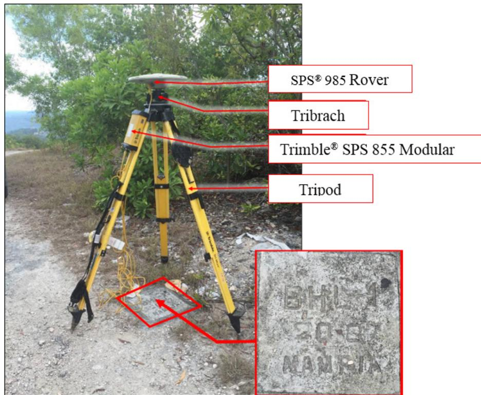
Figure 28. GNSS receiver set up, Trimble® SPS 985 at BHL-01 near a telecommunication antennae in Brgy. Catarman, Municipality of Dauis, Bohol.
