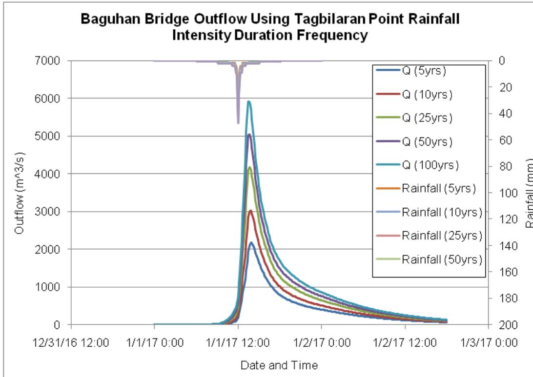
Figure 57. The Outflow hydrograph at the Baguhan Bridge, Inabanga generated using the Tagbilaran Point RIDF simulated in HEC-HMS.
