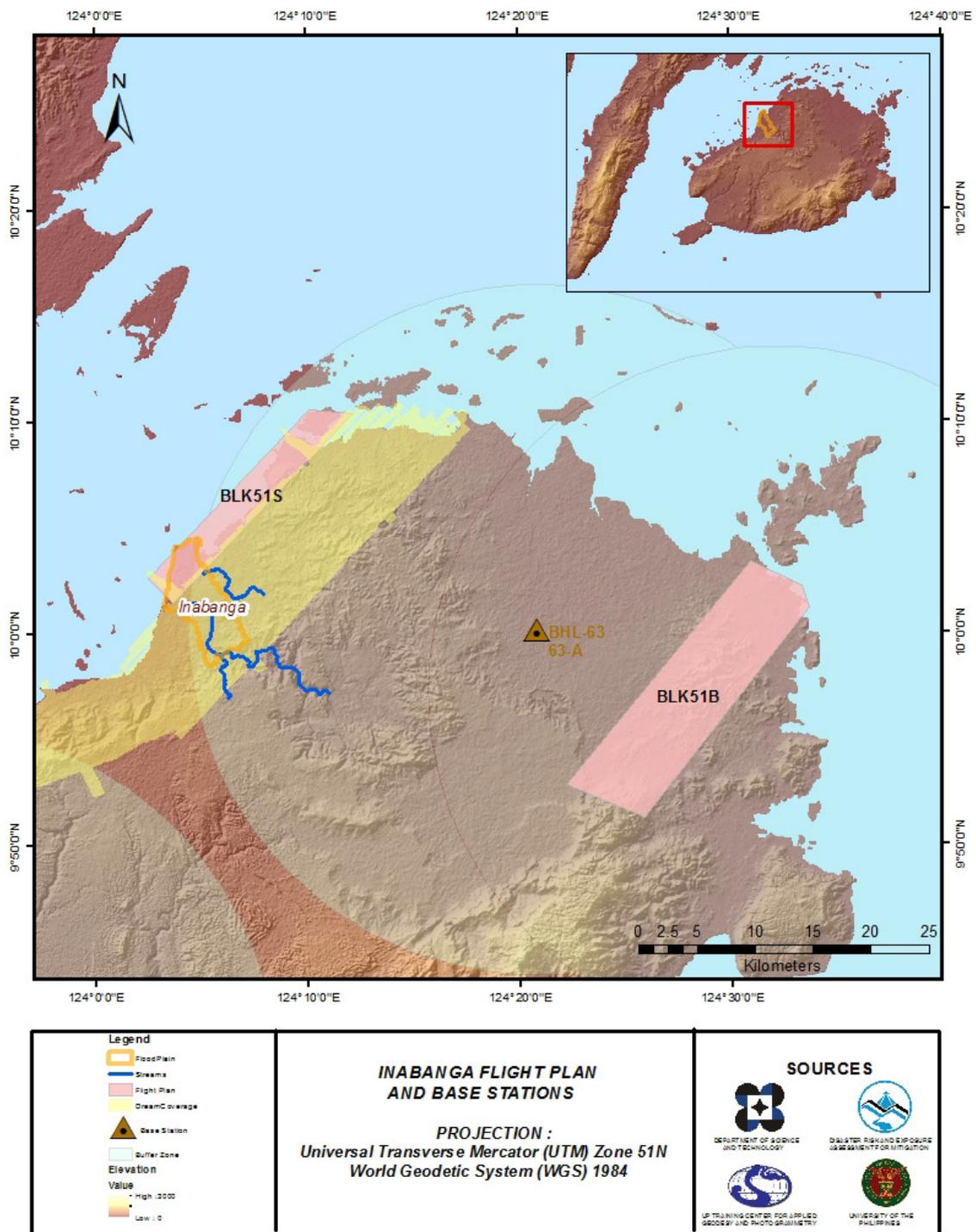
Figure 2. Flight plans and base stations used for Inabanga floodplain using Pegasus LiDAR system.
