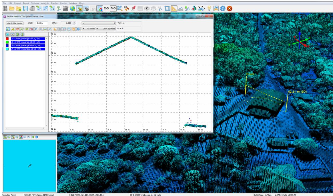
Figure 14. Quality checking for Inabanga flight 3409P using the Profile Tool of QT Modeler.
