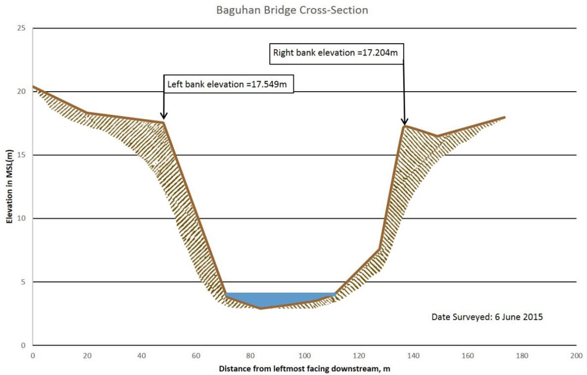
Figure 44. Cross-Section Plot of Baguhan Bridge.
