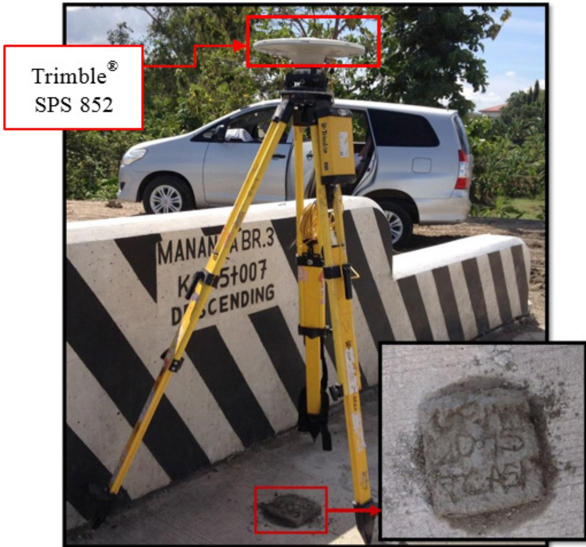
Figure 33. GNSS base receiver, Trimble® SPS 852, at UP-MAN, at the approach of Mananga Bridge in Brgy. Lawaan II, Talisay City, Cebu
