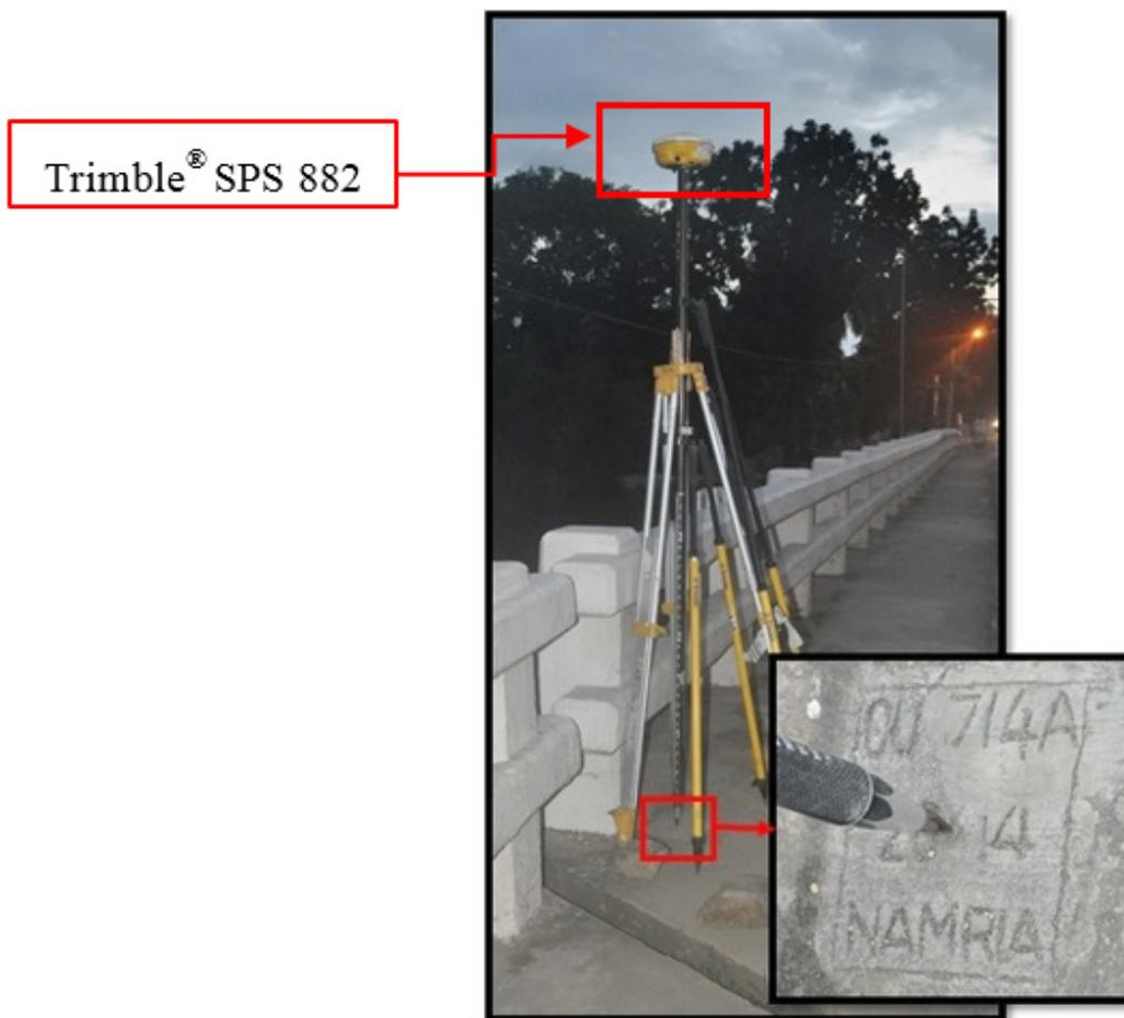
Figure 31. GNSS receiver setup, Trimble® SPS 882, at CU-714A, at the approach of Cotcot Bridge in Brgy. Cotcot, Municipality of Liloan, Cebu
