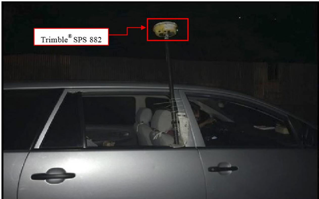
Figure 39. Validation points acquisition survey set up along Kotkot River Basin
