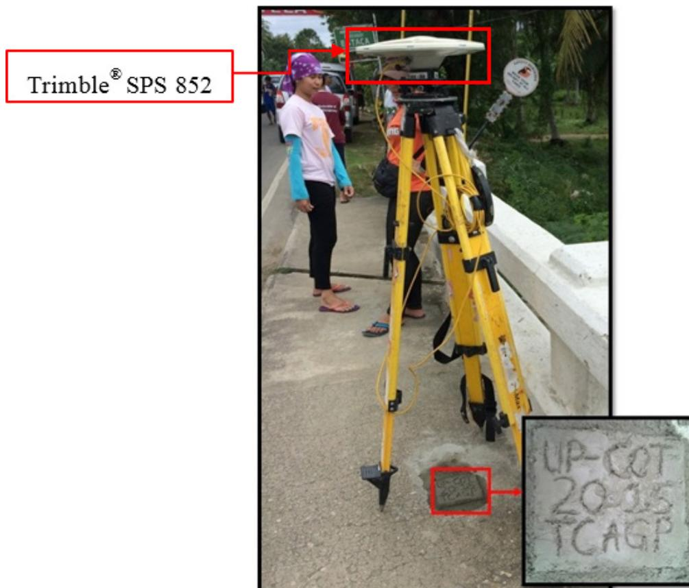
Figure 32. GNSS base receiver, Trimble® SPS 852, at UP-COT, at the approach of Cotcot Bridge in Brgy. Cotcot, Municipality of Liloan, Cebu
