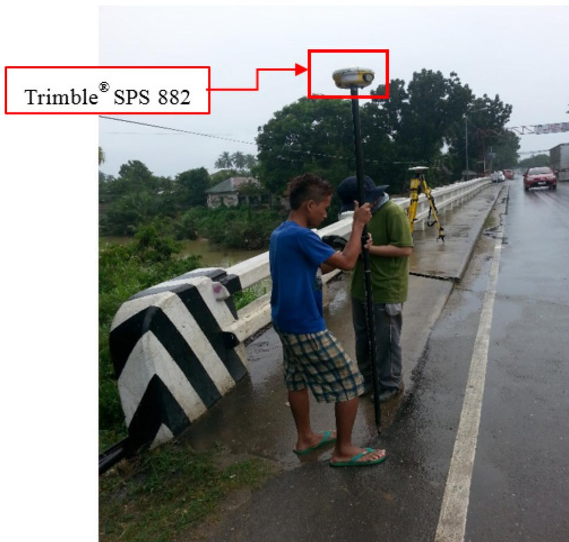
Figure 35. As-built survey of Kotkot Bridge
