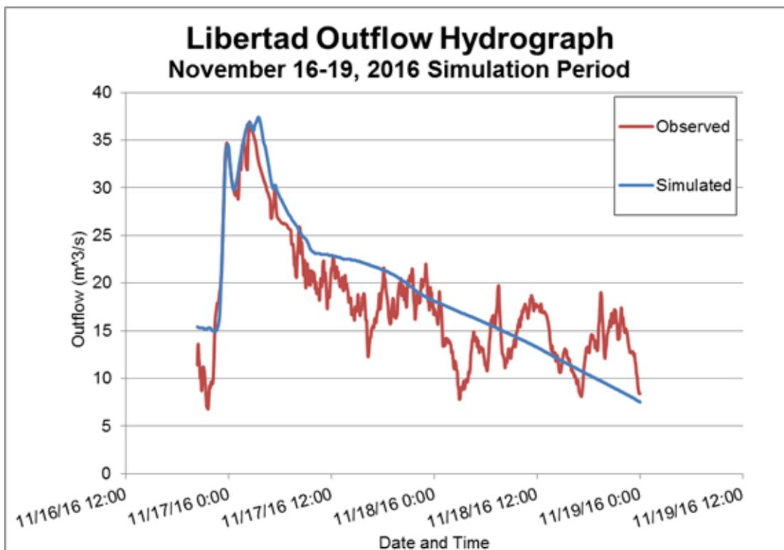
Figure 57. Outflow Hydrograph of Libertad produced by the HEC-HMS model compared with observed outflow.
