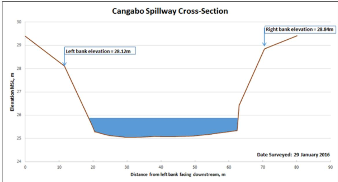
Figure 45. Cross-Section Plot of Cancabo Spillway in Libertad River.
