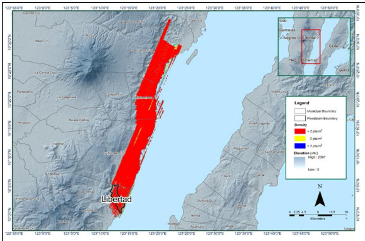
Figure 13. Pulse density map of the merged LiDAR data for Libertad floodplain.
