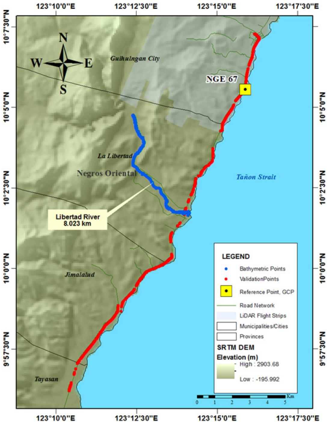
Figure 39. The extent of the LiDAR ground validation survey (in red) for Libertad River Basin.
