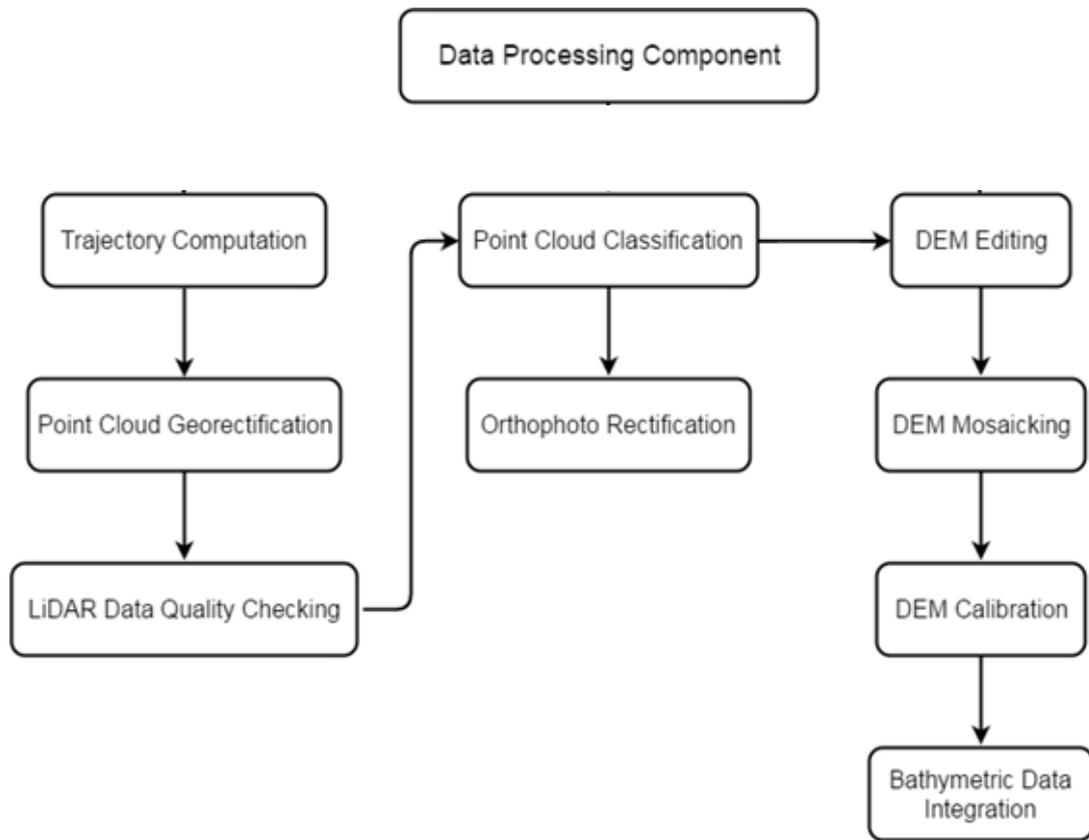
Figure 7. Schematic diagram for the data pre-processing.
