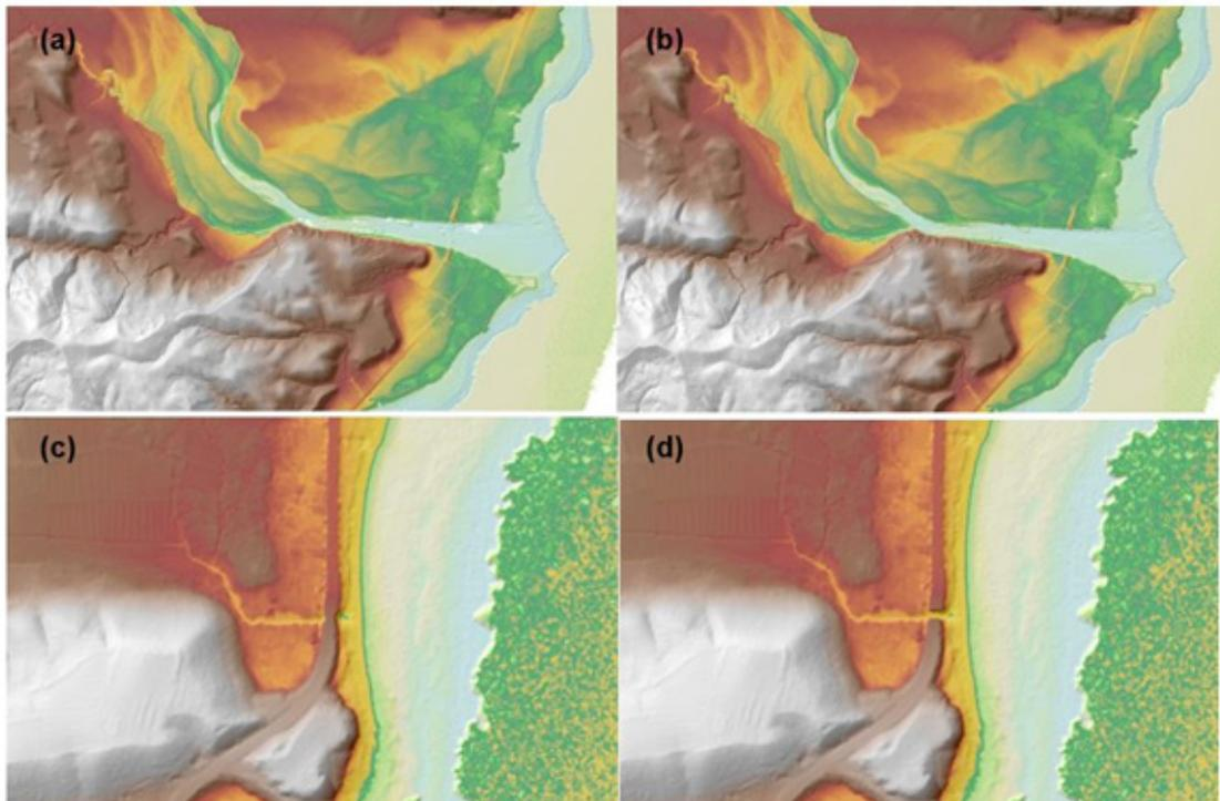
Figure 21. Portions in the DTM of the Libertad Floodplain – before (a) and after (b) filling of data gaps; a bridge before (c) and after (d) manual editing.
