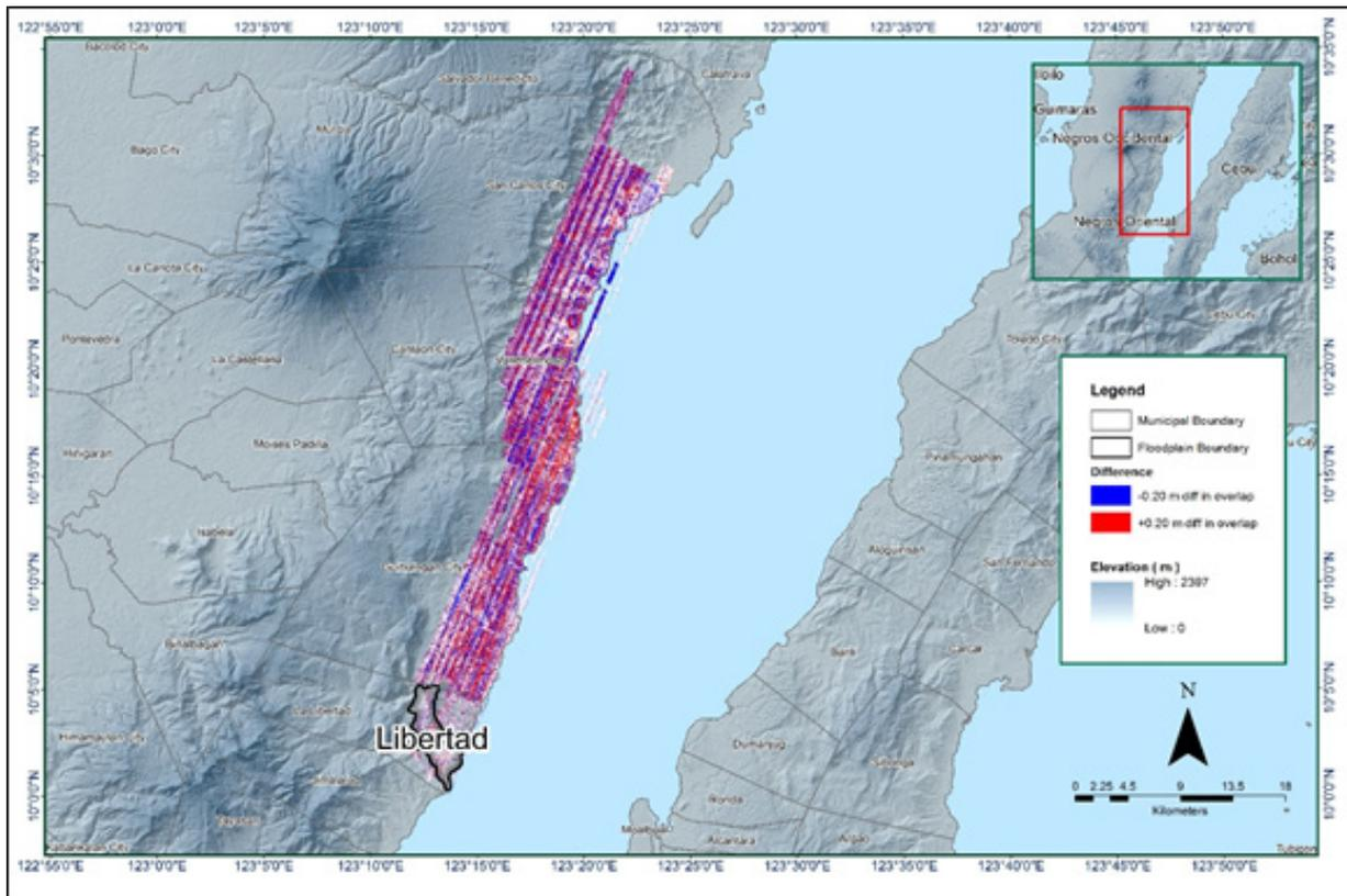
Figure 14. Elevation difference Map between flight lines for the Libertad Floodplain Survey.
