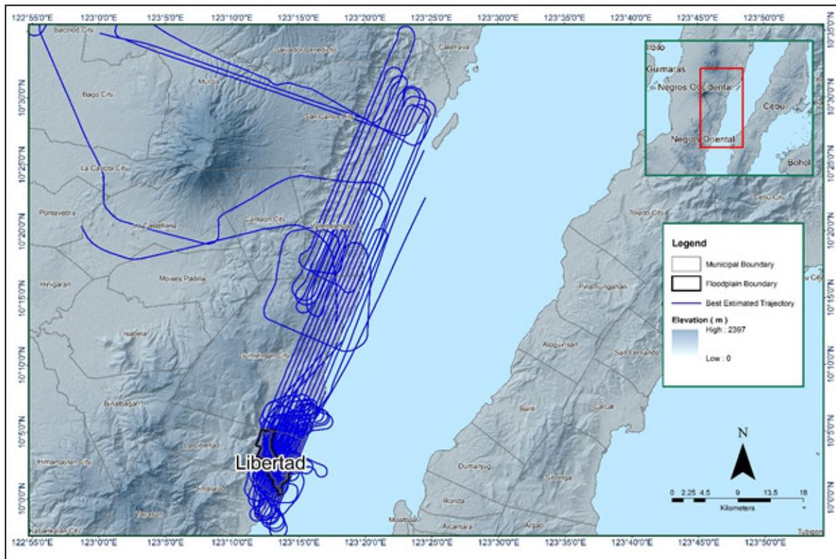
Figure 10. Best Estimated Trajectory of the LiDAR missions conducted over the Libertad.
