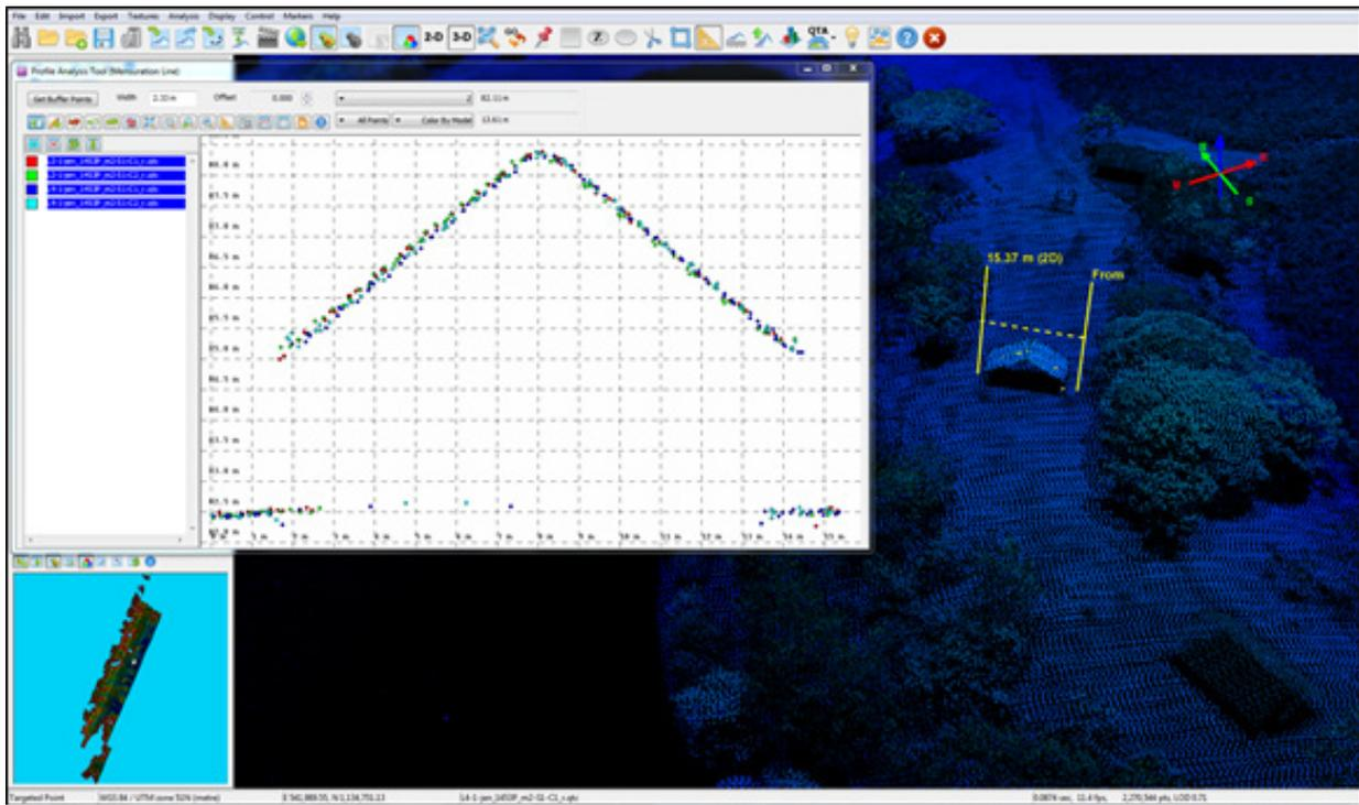
Figure 15. Quality checking for Libertad flight 1453P using the Profile Tool of QT Modeler.
