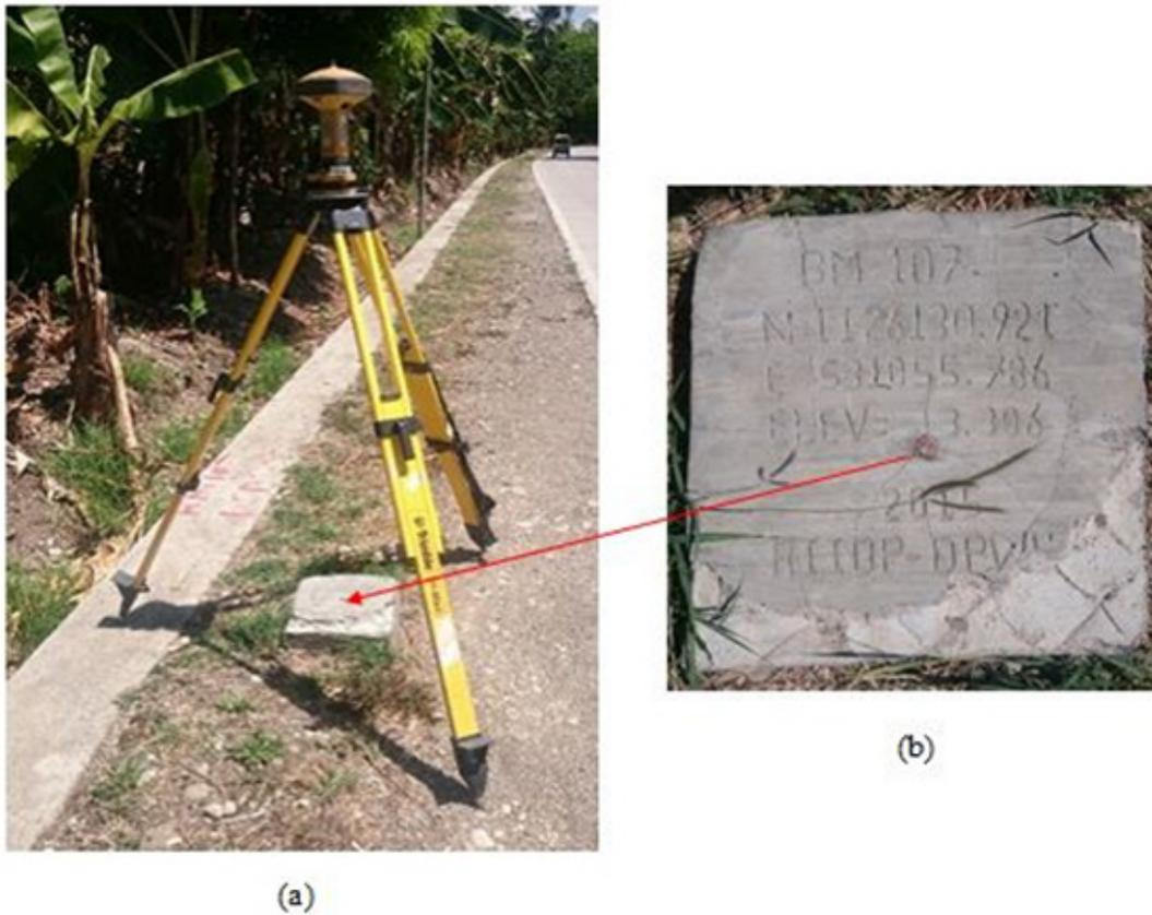
Figure 5. GPS set-up over BM-107 as located at the right side of the national road going to Dumaguete located at Guihulngan, Negros Oriental. (a) and NAMRIA reference point BM-107 (b) as recovered by the field team.
