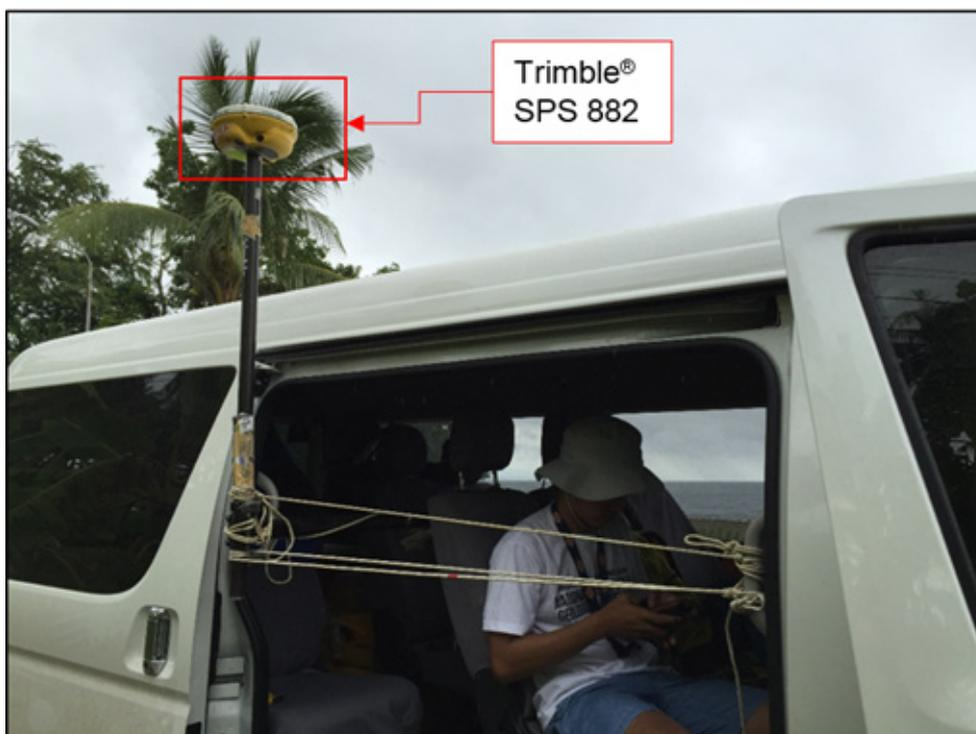
Figure 38. GNSS Receiver Trimble® SPS 882 installed on a vehicle for Ground Validation Survey.
