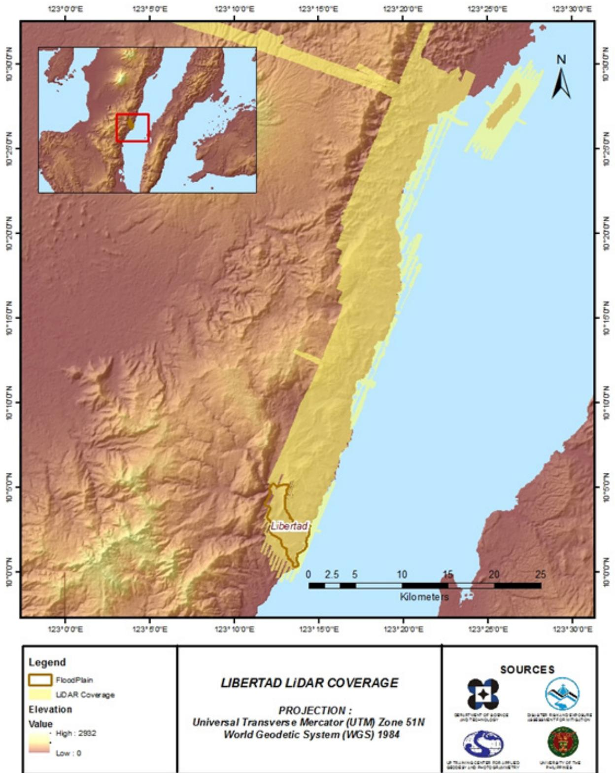
Figure 6. Actual LiDAR survey coverage for Libertad floodplain.
