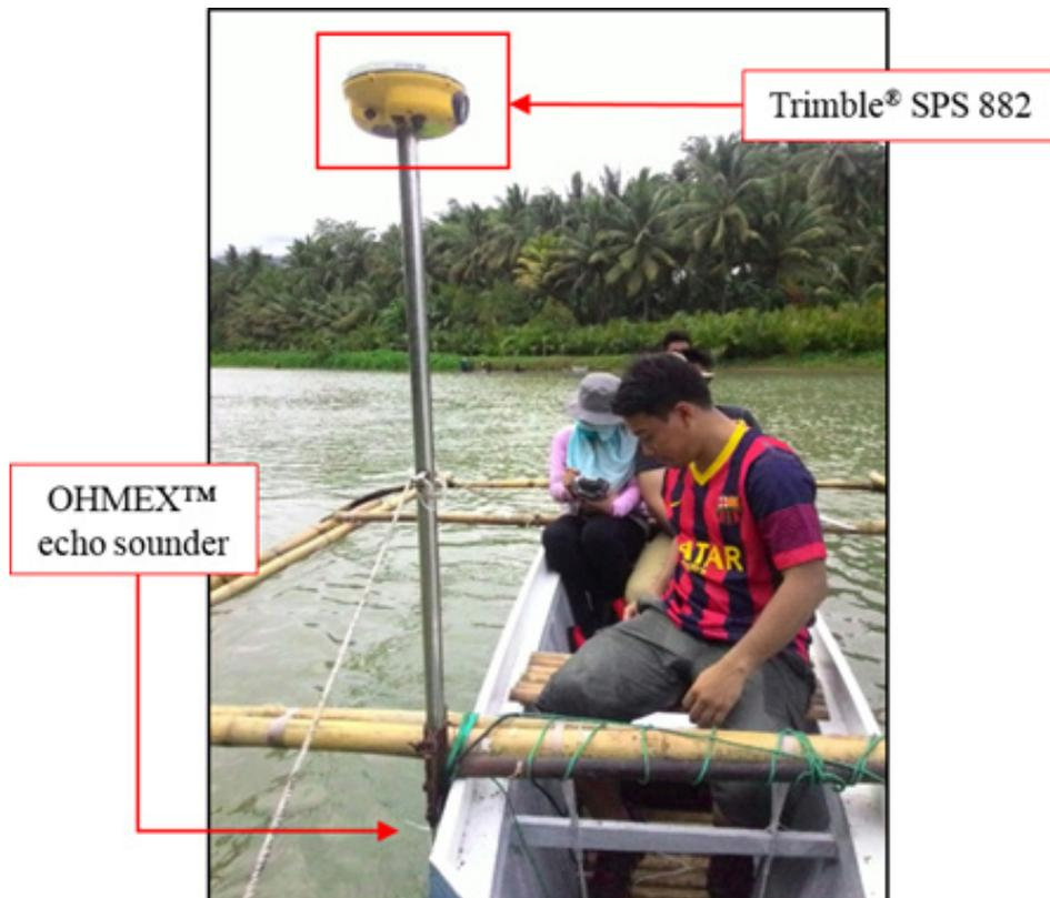
Figure 40. Set up of the bathymetric survey at Libertad River using Trimble® SPS 882 in GNSS PPK survey technique.
