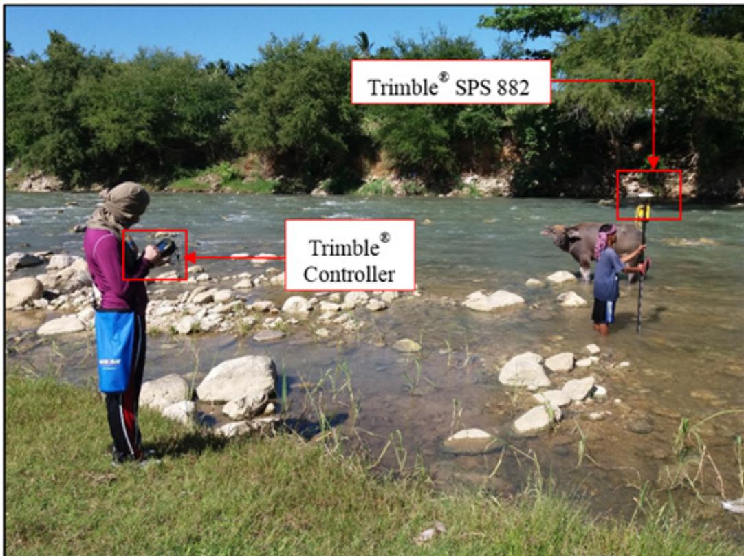
Figure 41. Manual bathymetric survey set-up for Libertad River.
