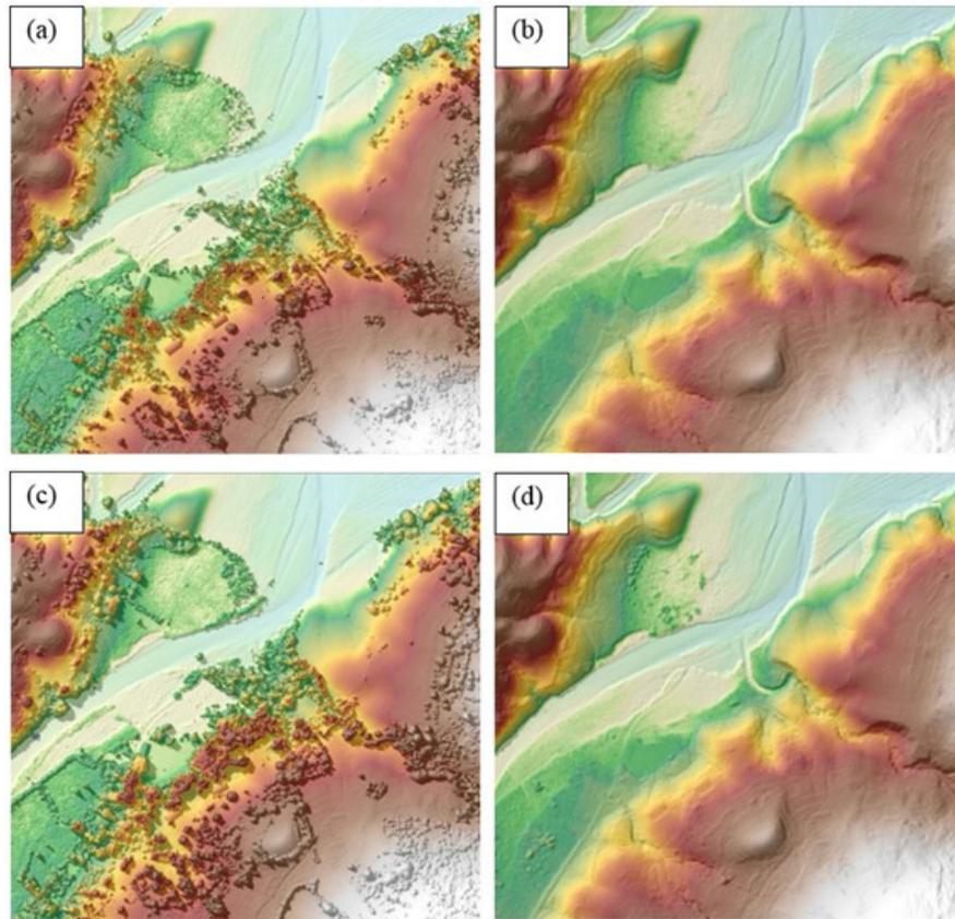
Figure 18. The production of last return DSM (a) and DTM (b), first return DSM (c) and secondary DTM (d) in some portion of Libertad floodplain.
