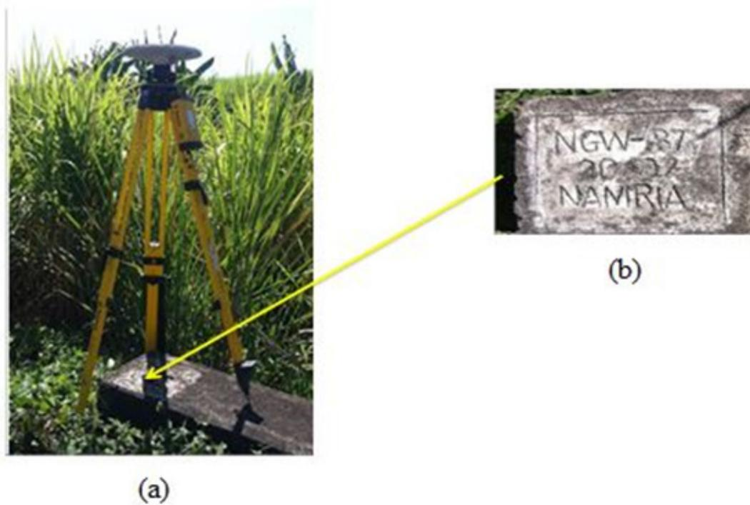
Figure 3. GPS set-up over NGW-87 as recovered at the SE side of Moises Padilla-Canlaon Road and NE of wooden electric post. Station is situated on top of headwall. (a) and NAMRIA reference point NGW-87 (b) as recovered by the field team.
