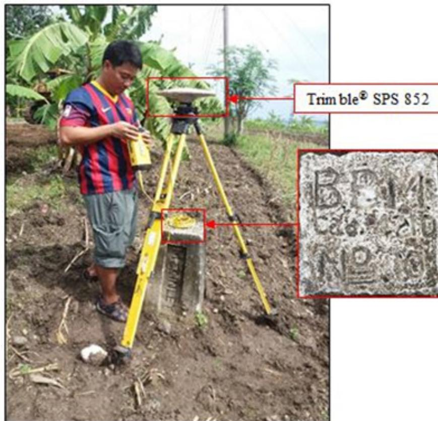
Figure 31. Trimble® SPS 852 base set-up at NGE-67 located along national road in Brgy. Mckinley, Municipality of Libertad.
