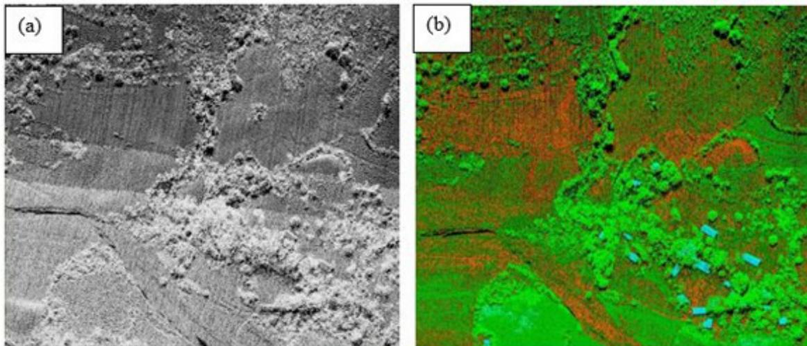
Figure 17. Point cloud before (a) and after (b) classification.
