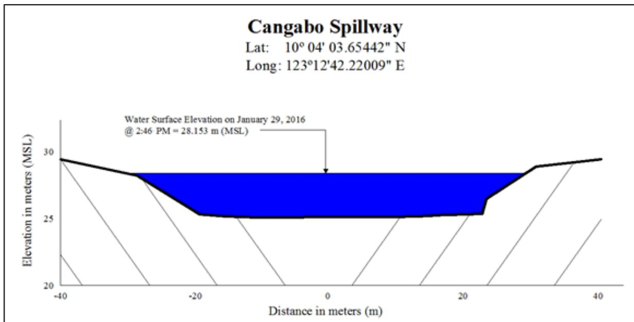
Figure 36. Deployment site, Cangabo Spillway, cross-section diagram
