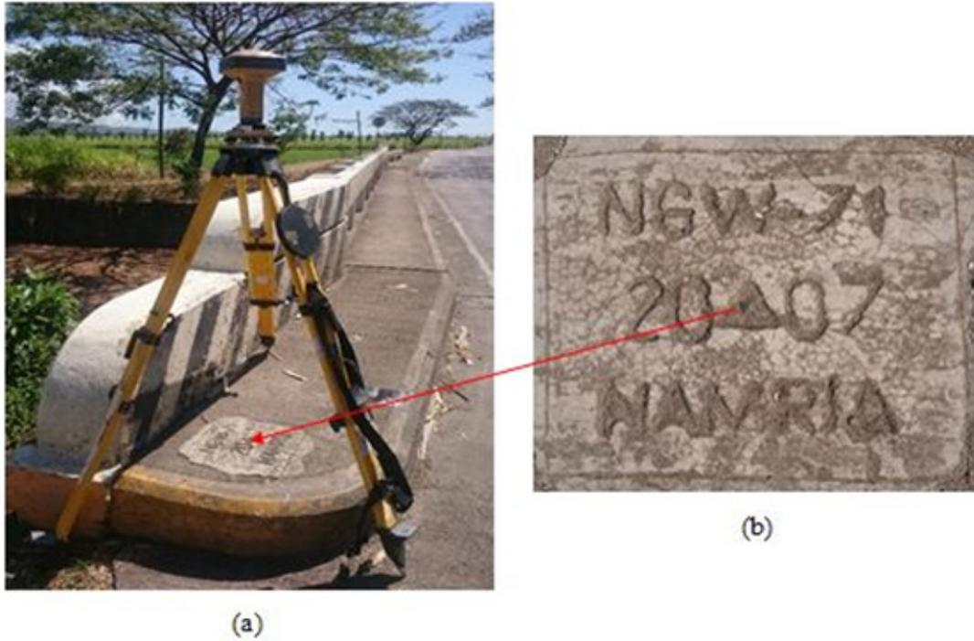
Figure 4. GPS set-up over NGW-71 as recovered in San Carlos, Negros Occidental. The station is located at Higalaman Bridge, at km 148+364.5 along the national road. (a) and NAMRIA reference point NGW-71 (b) as recovered by the field team.
