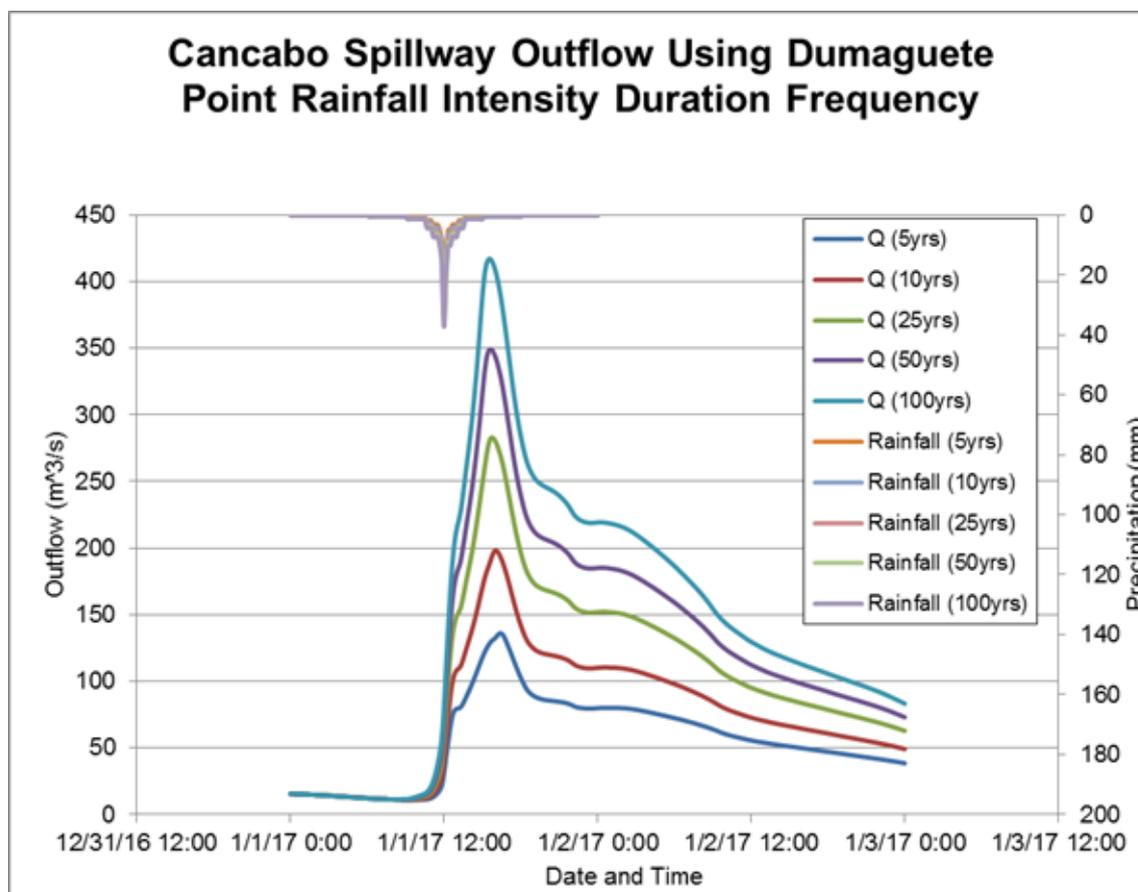
Figure 58. The Outflow hydrograph at the Cancabo Spillway, Libertad generated using the Dumaguete Point RIDF simulated in HEC-HMS.
