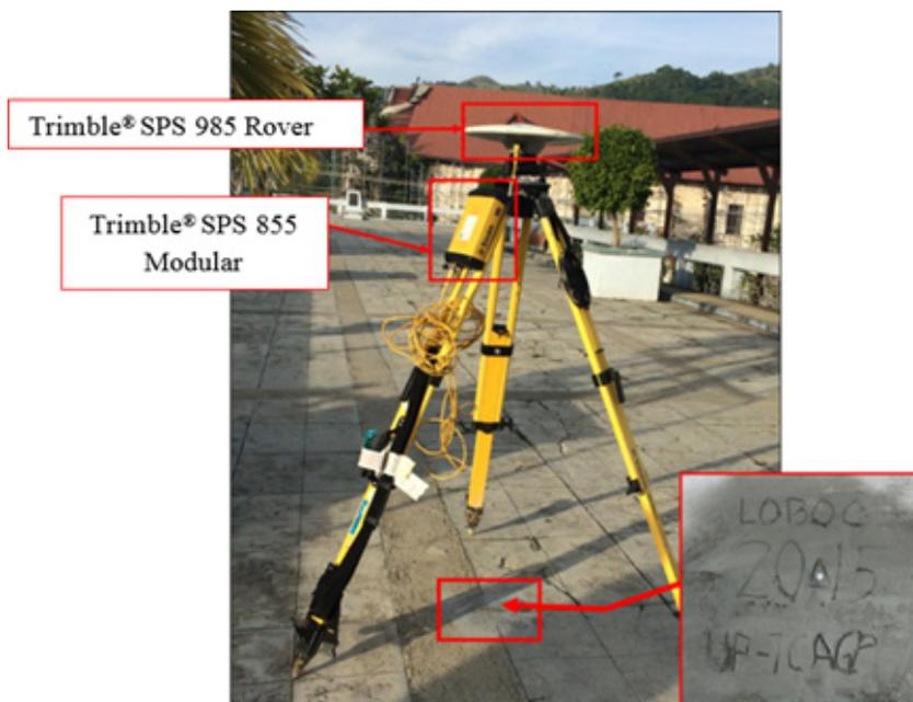
Figure 34. GPS setup of Trimble® SPS 852 on LOBOC, located on the incomplete bridge across the Loboc River near the municipality town plaza of Loboc in Brgy. Poblacion
