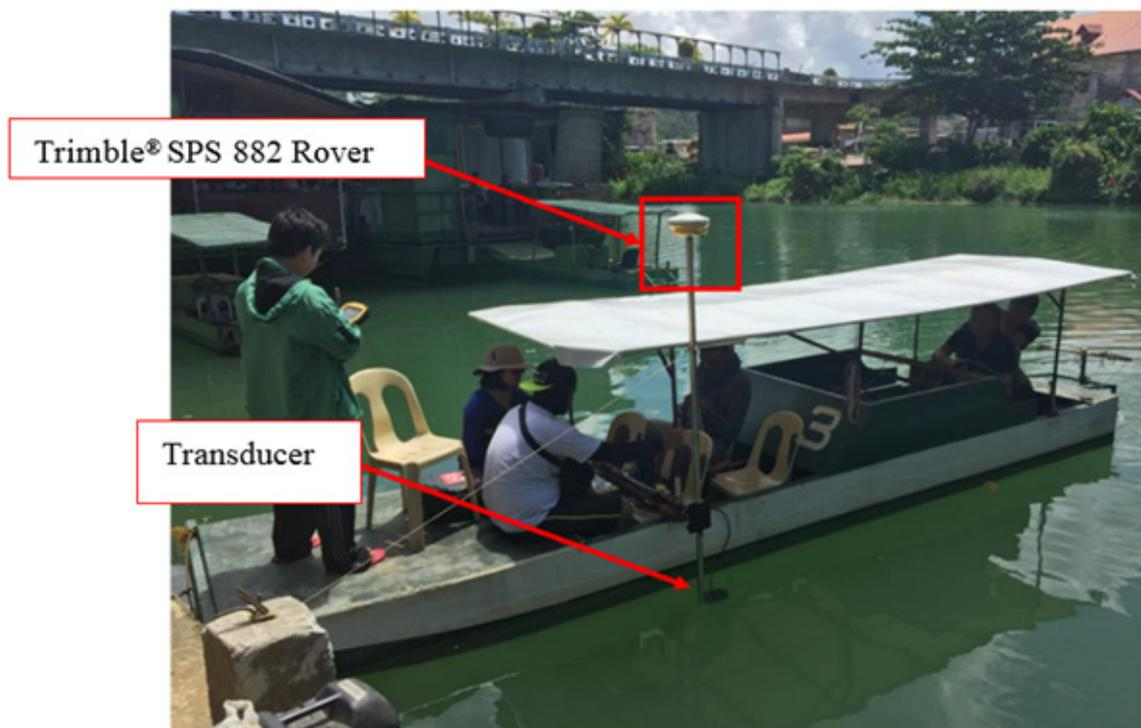
Figure 42. Bathymetric survey in Loboc River
