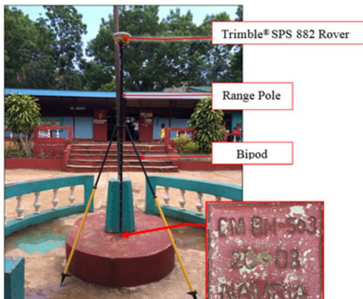
Figure 31. Trimble® SPS 882 GNSS receiver setup at BH-503 located inside the campus of Dao Elementary School, Brgy. Dao, Municipality of Dauis, Bohol
