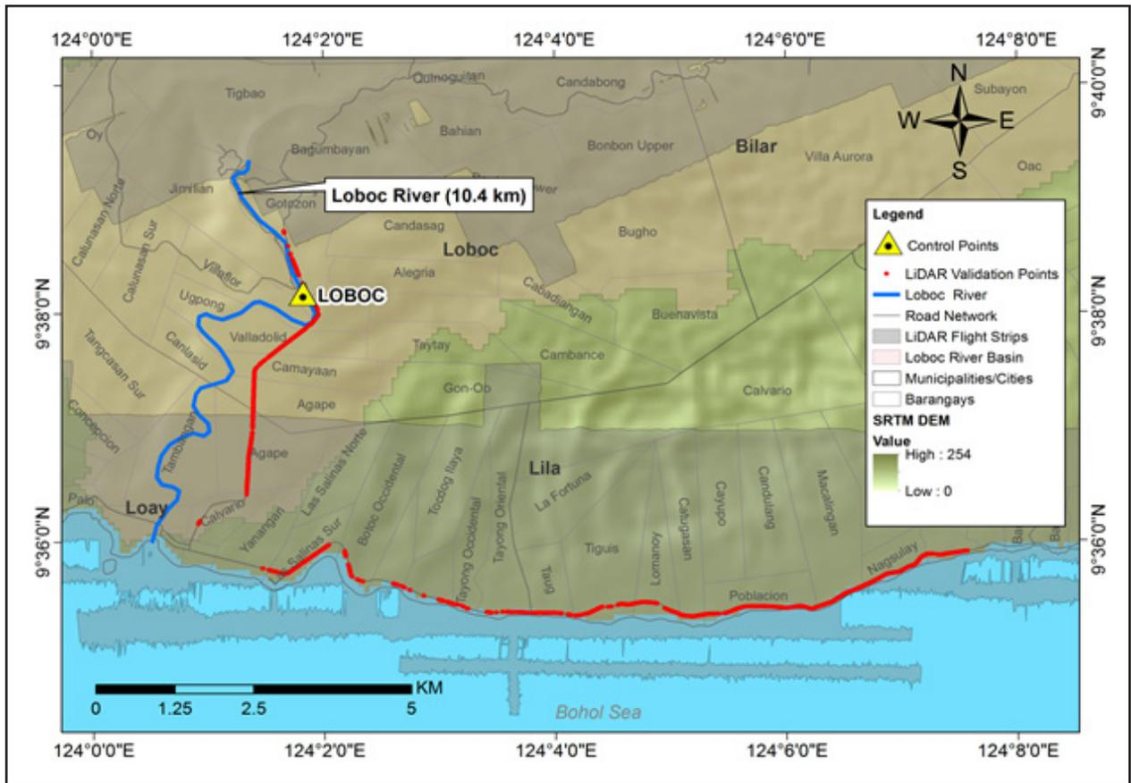
Figure 41. Validation points acquisition survey coverage for Loboc River Basin
