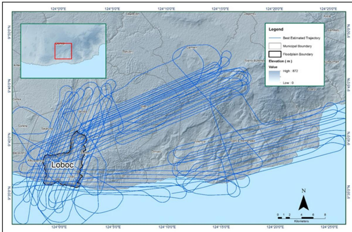
Figure 9. The best estimated trajectory of the LiDAR missions conducted over the Loboc Floodplain
