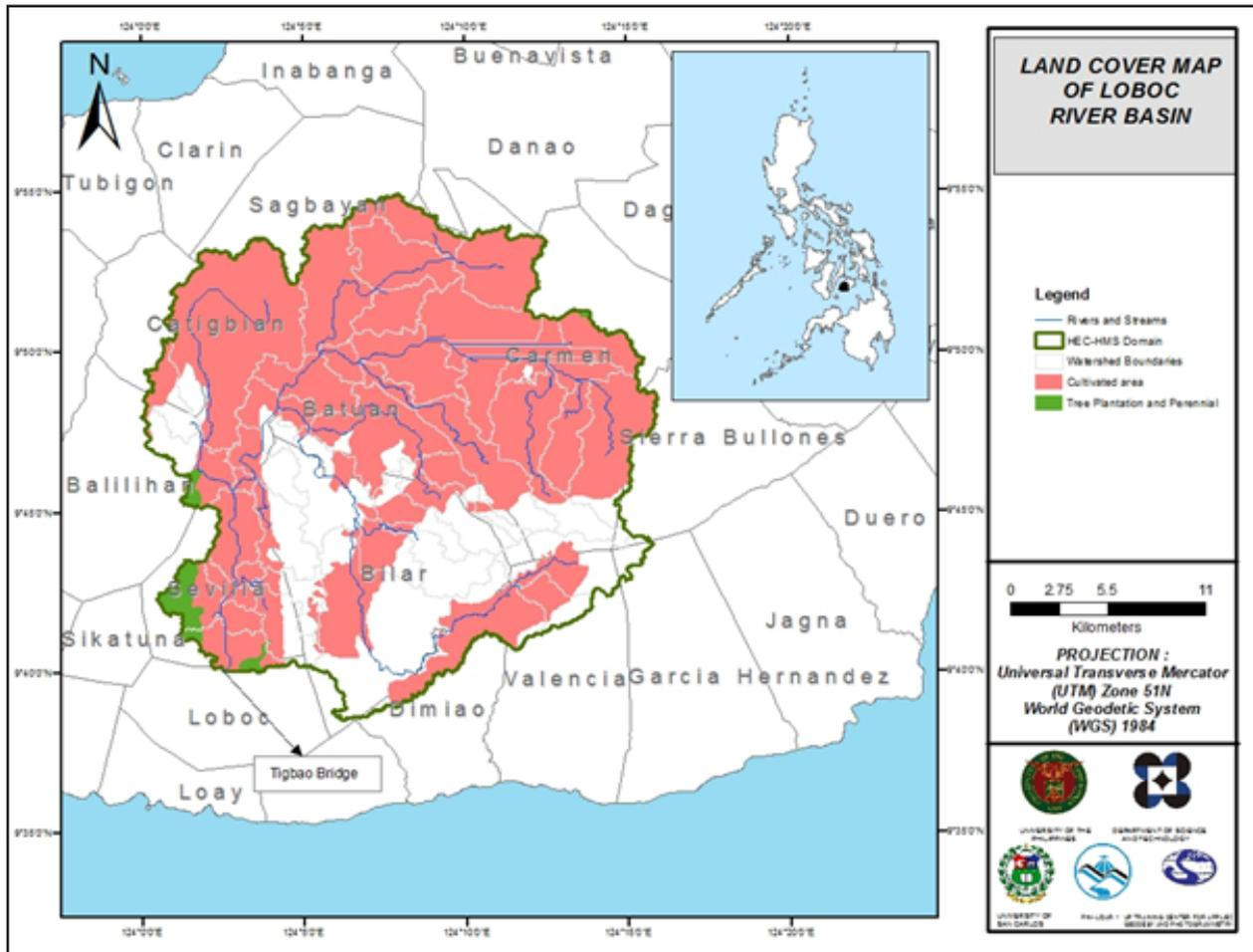
Figure 52. The land cover map of the Loboc River Basin used for the estimation of the CN and watershed lag parameters of the rainfall-runoff model. (Source of data: National Mapping and Resource Information Authority)
