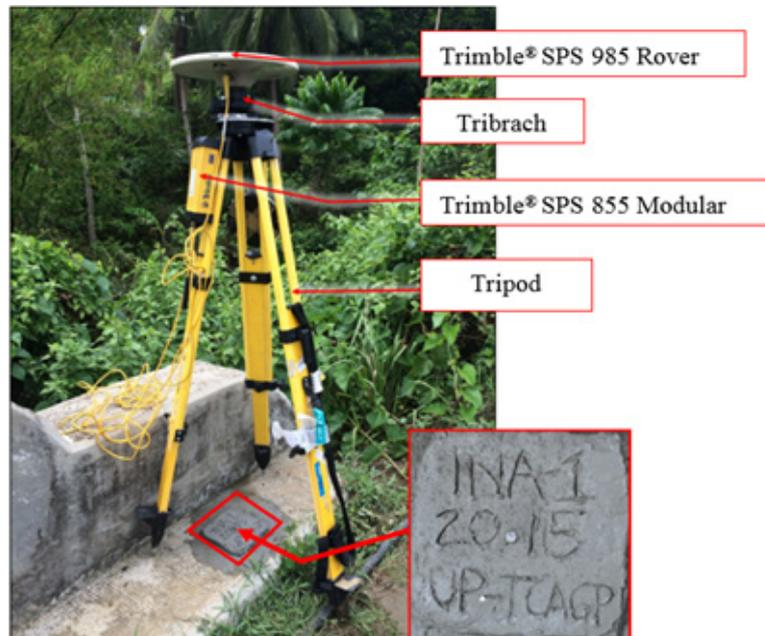
Figure 33. Trimble® SPS 985 GNSS receiver setup at INA-1 at the Inabanga Bridge approach, Brgy. Baguhan, Inabanga, Bohol
