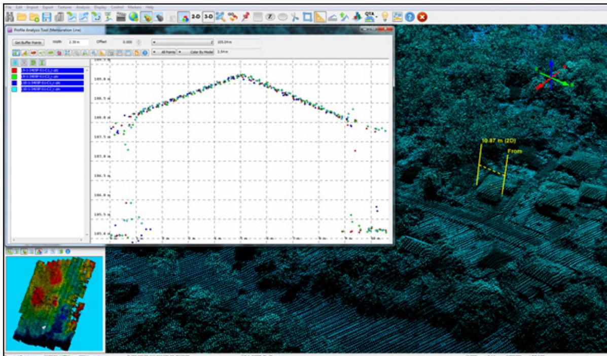
Figure 14. Quality checking for a Loboc flight 3405P using the Profile Tool of QT Modeler.
