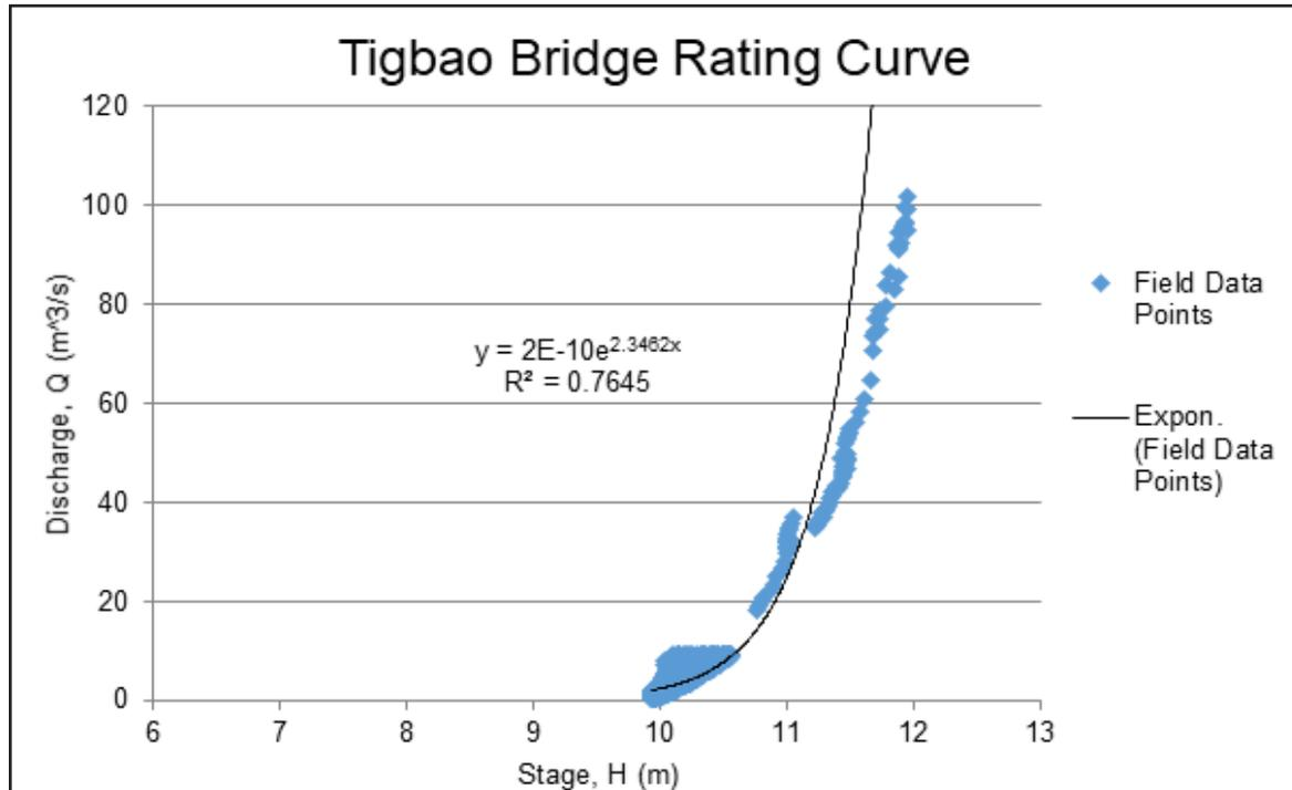
Figure 47. Rating Curve at Tigbao Bridge, Loboc, Bohol
