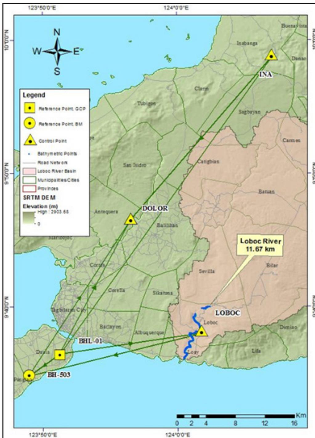
Figure 29. GNSS network covering the Loboc River.
