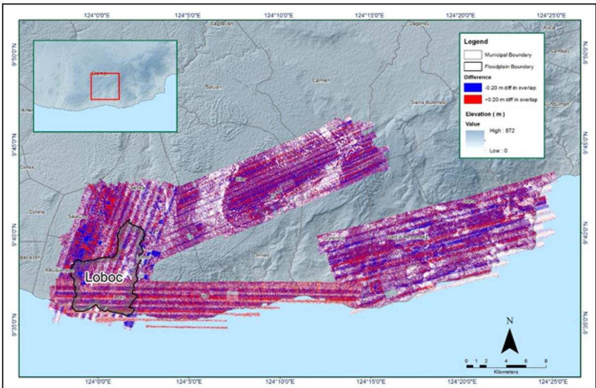
Figure 13. Elevation difference map between flight lines for Loboc floodplain.
