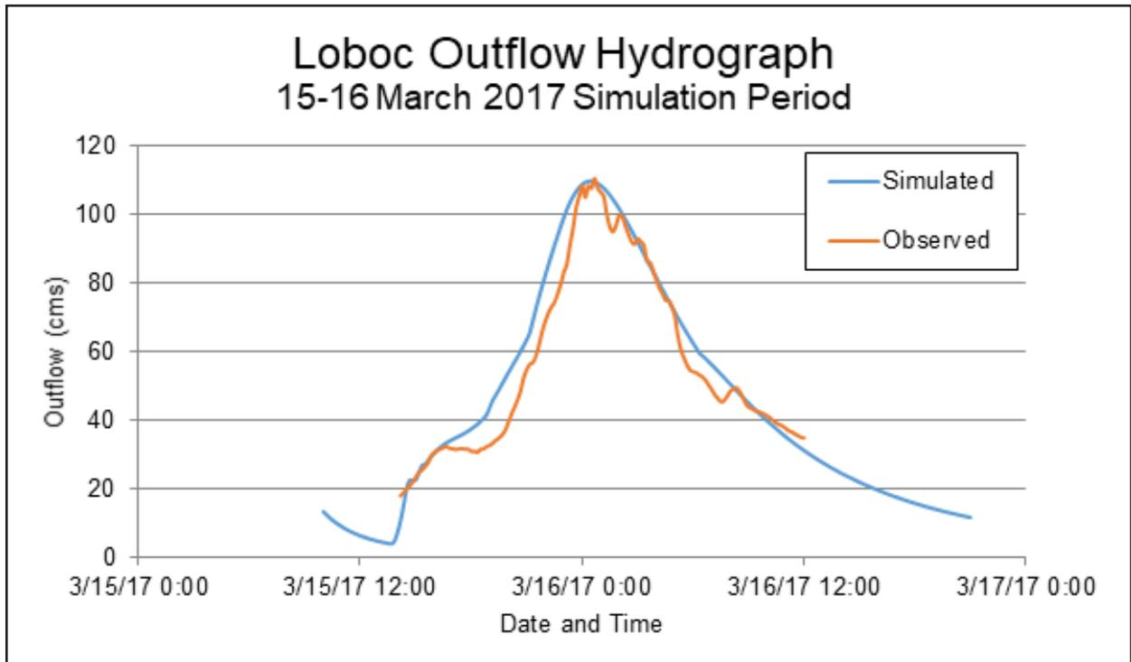
Figure 60. Outflow Hydrograph of Loboc produced by the HEC-HMS model compared with observed outflow.
