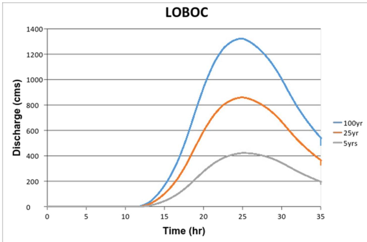
Figure 62. Loboc river generated discharge using 5-, 25-, and 100-year Tagbilaran rainfall intensity-duration-frequency (RIDF) in HEC-HMS
