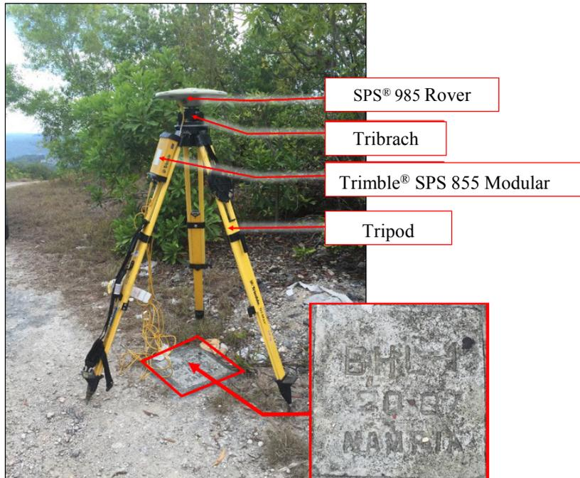
Figure 30. Trimble® SPS 985 GNSS receiver setup at BHL-01 near a telecommunication antennae in Brgy. Catarman, Municipality of Dauis, Bohol
