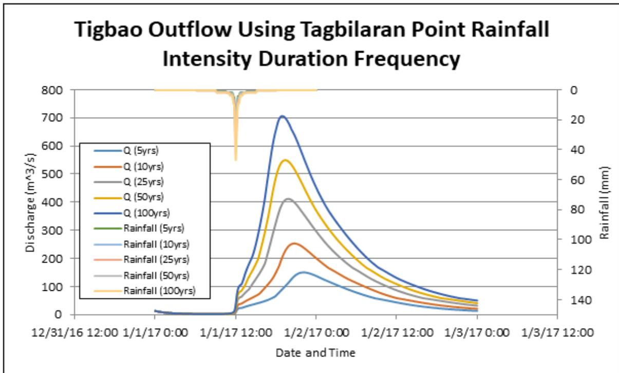
Figure 61. Outflow hydrograph at Tigbao generated using Tagbilaran PointRIDF simulated in HEC-HMS
