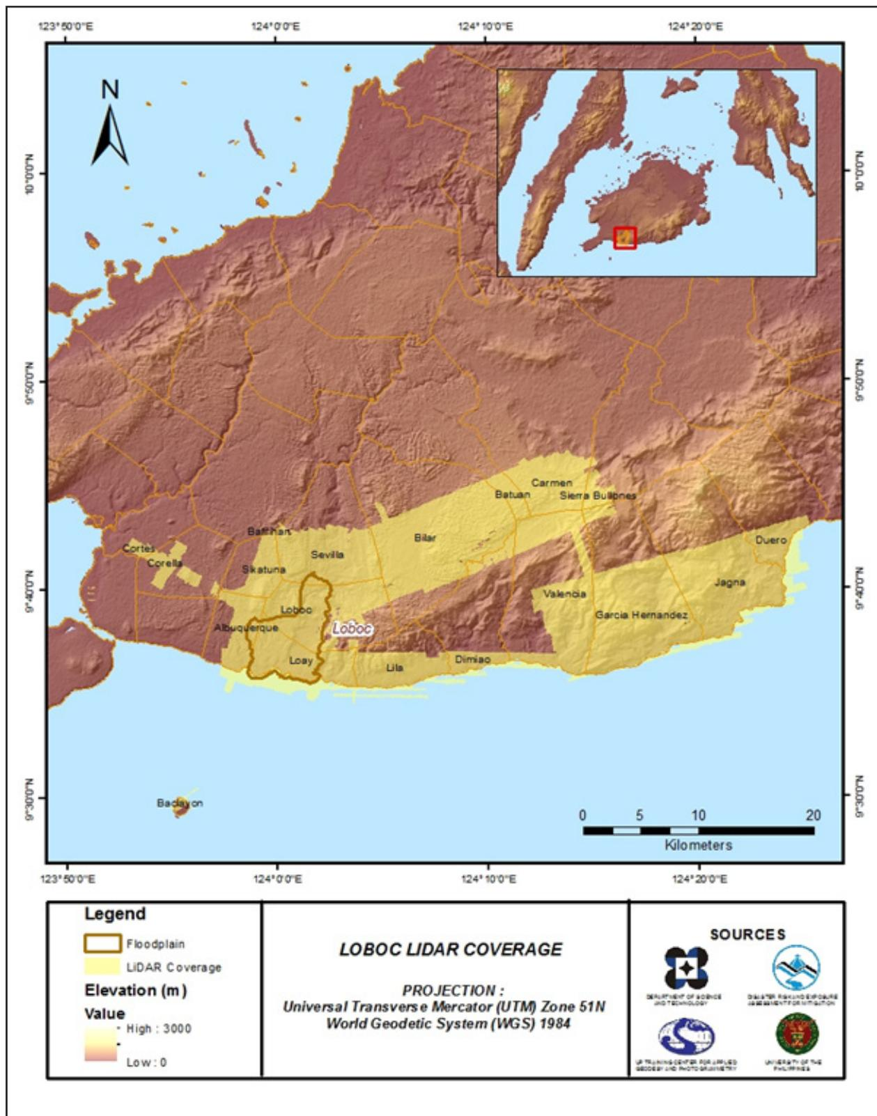
Figure 5. Actual LiDAR data acquisition for Loboc floodplain.
