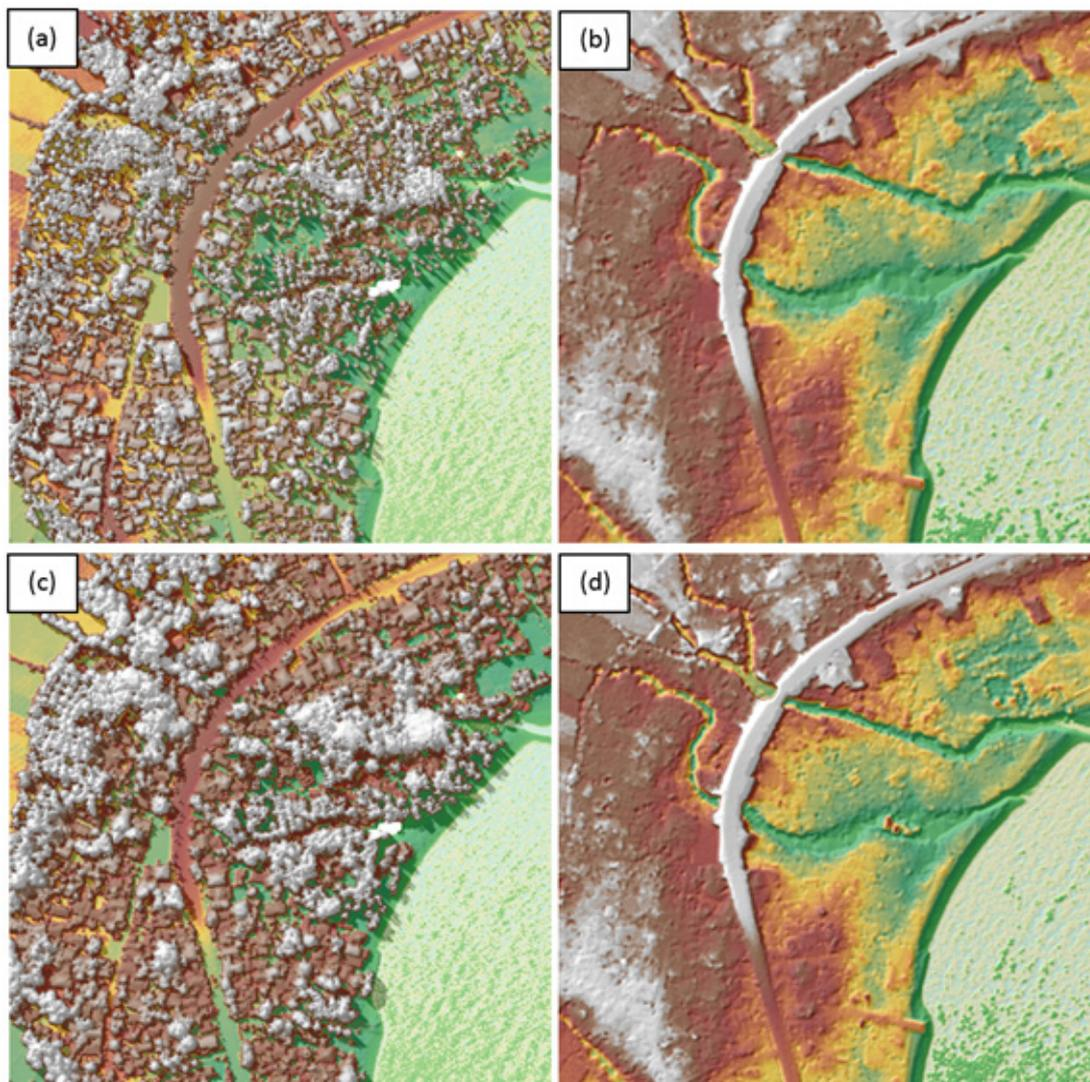
Figure 17. The production of last return DSM (a) and DTM (b), first return DSM (c) and secondary DTM (d) in some portion of Loboc floodplain.
