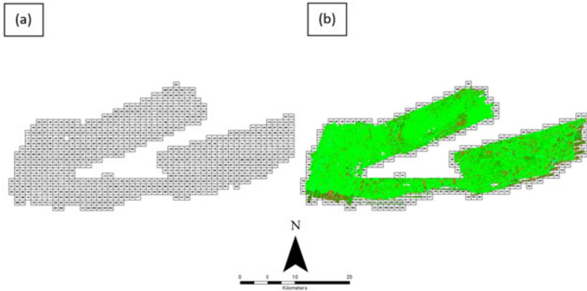
Figure 15. Tiles for Loboc floodplain (a) and classification results (b) in TerraScan.
