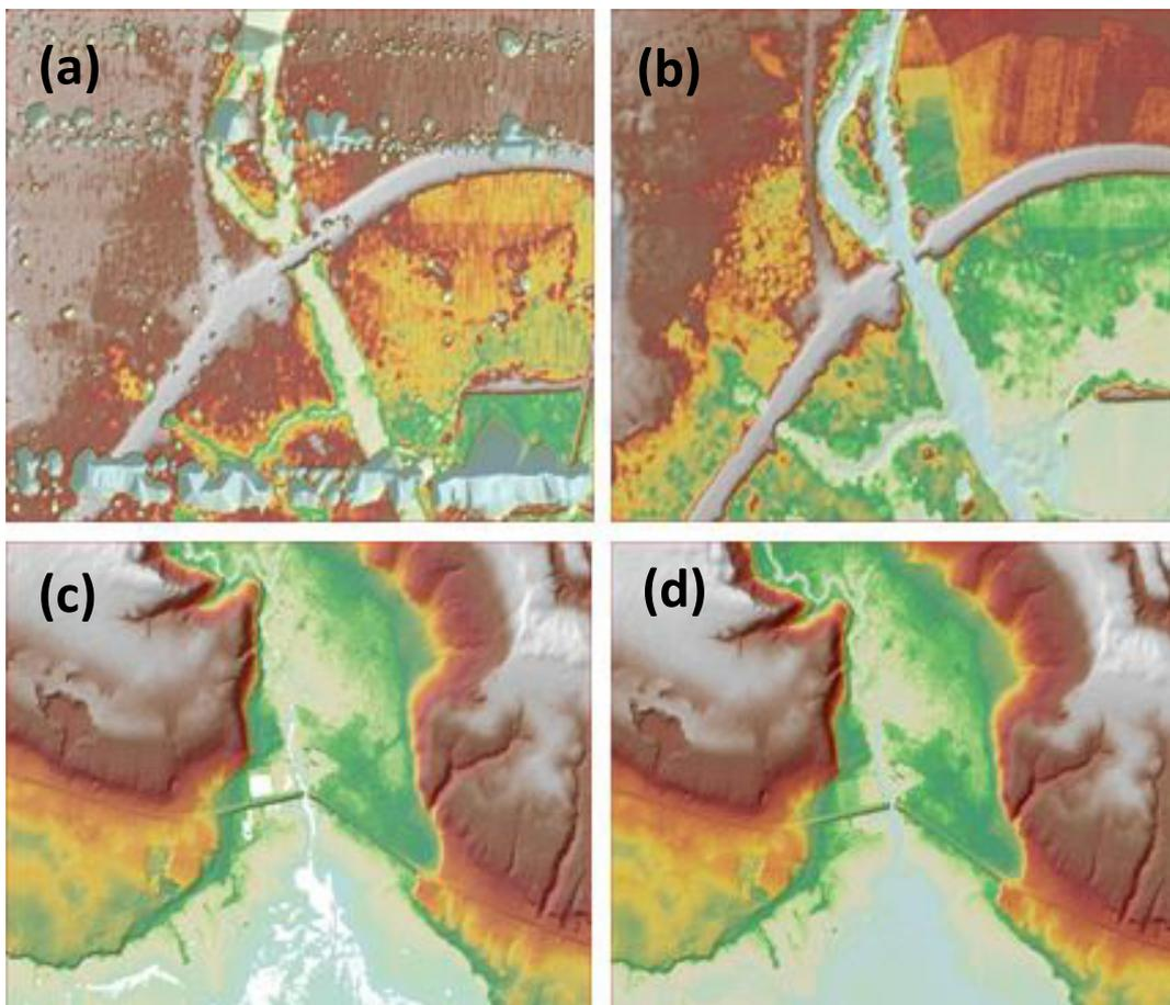
Figure 20. Portions in the DTM of Loboc floodplain – a bridge before (a) and after (b) manual editing; a water surface before (c) and after (d) filling data gaps.
