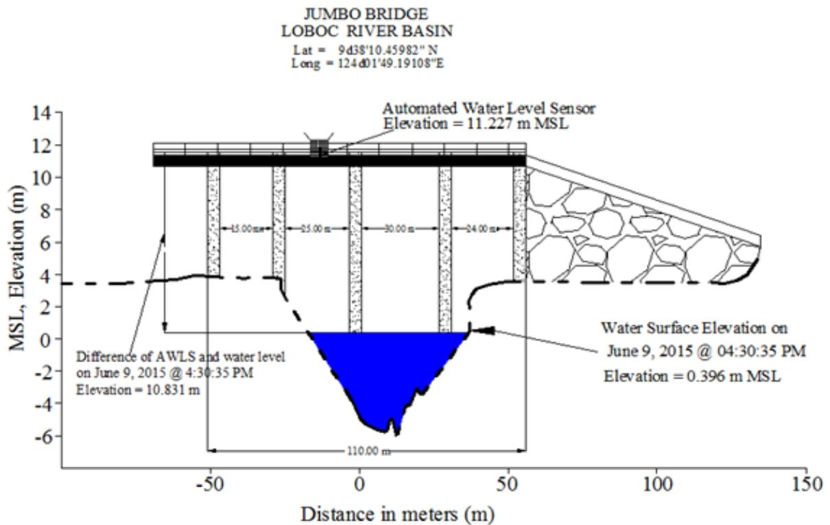
Figure 37. Jumbo Bridge cross-sectional diagram
