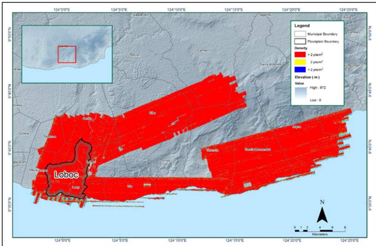
Figure 12. Pulse density map of merged LiDAR data for Loboc floodplain.
