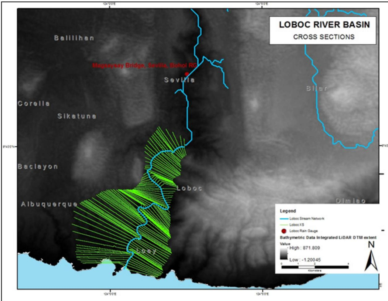
Figure 56. River cross-section of Loboc River generated through Arcmap HEC GeoRAS tool
