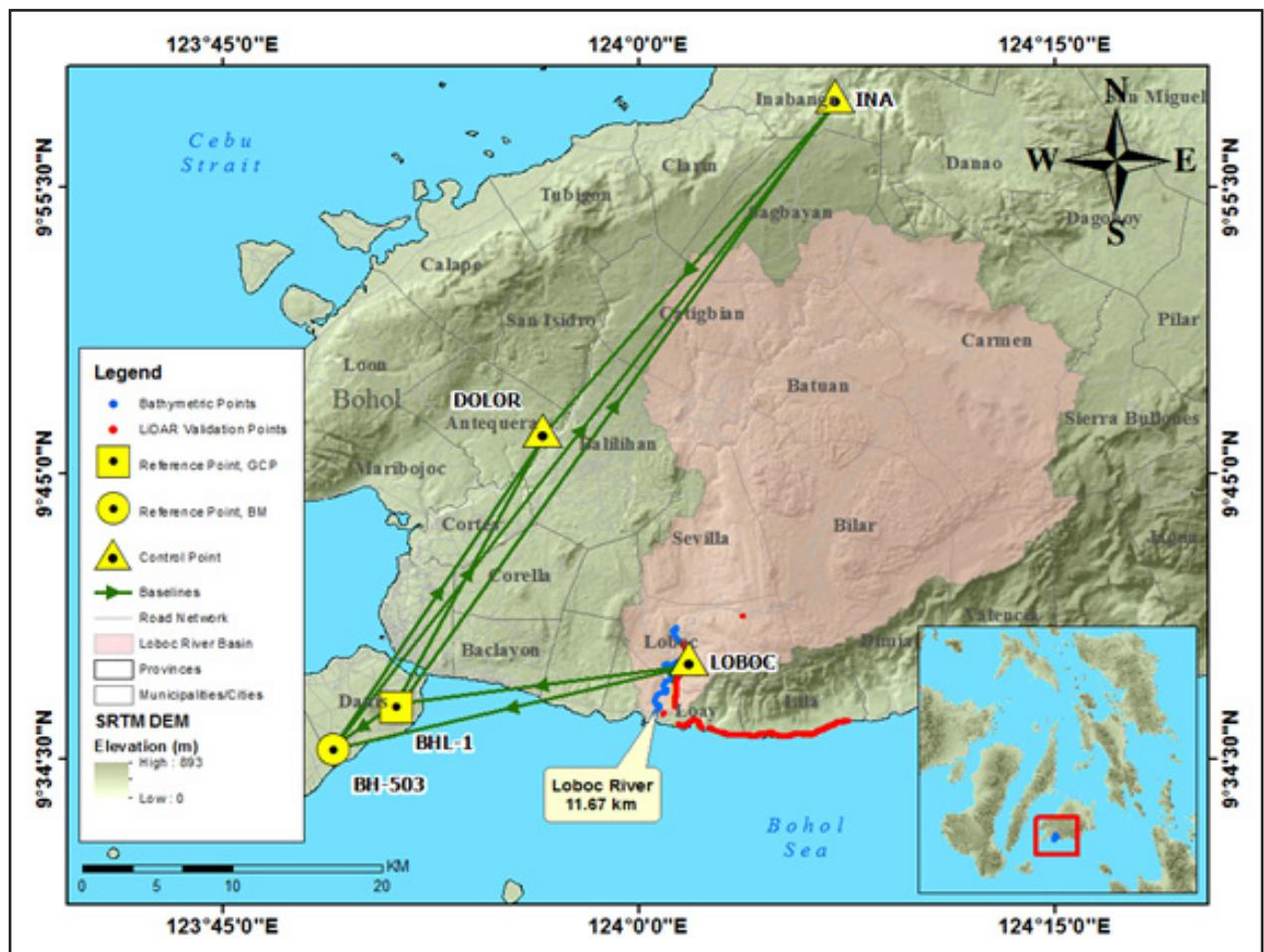
Figure 28. Extent of the bathymetric survey (blue line) in Loboc River and the LiDAR data validation survey (red)
