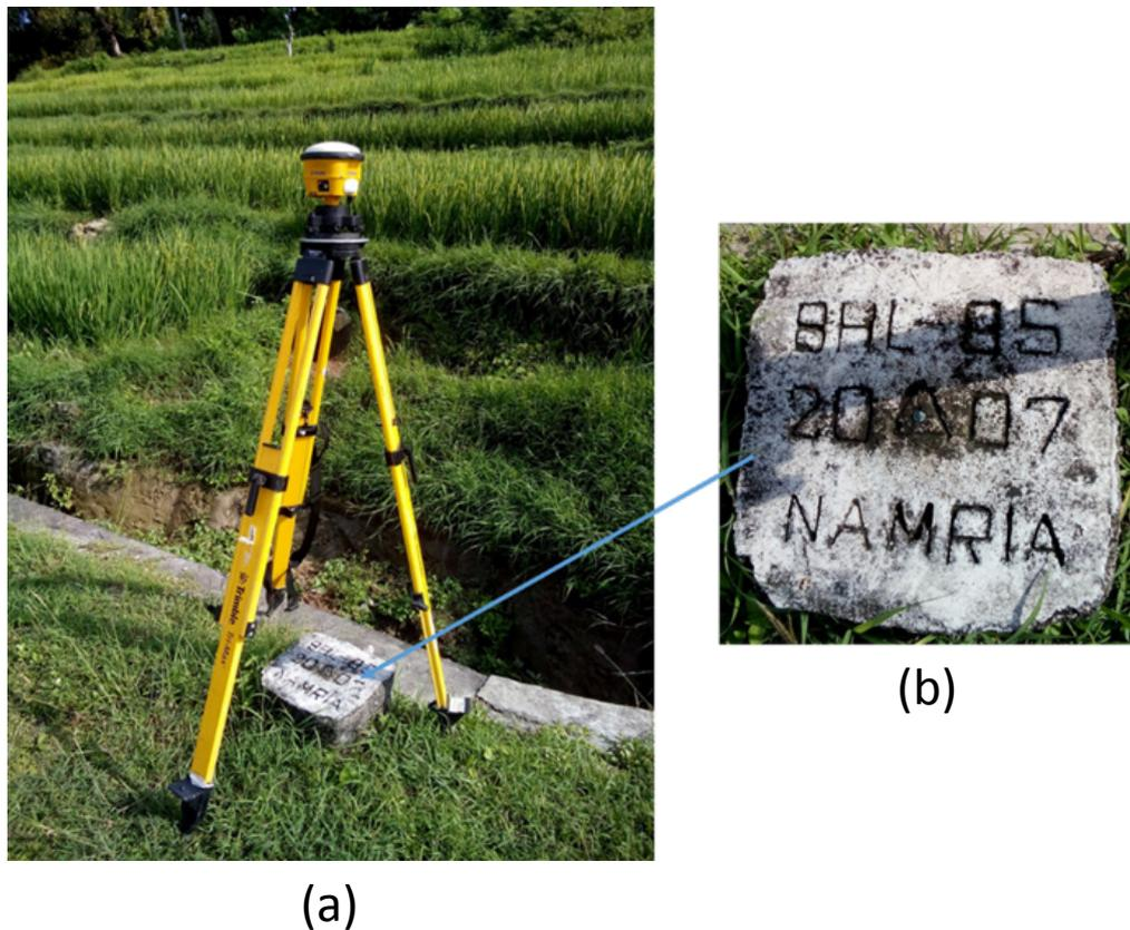
Figure 3. GPS set-up over BHL-95 located at the left side of the road from Lila Town Proper, Lila, Bohol (a) and NAMRIA reference point BHL-95 (b) as recovered by the field team.
