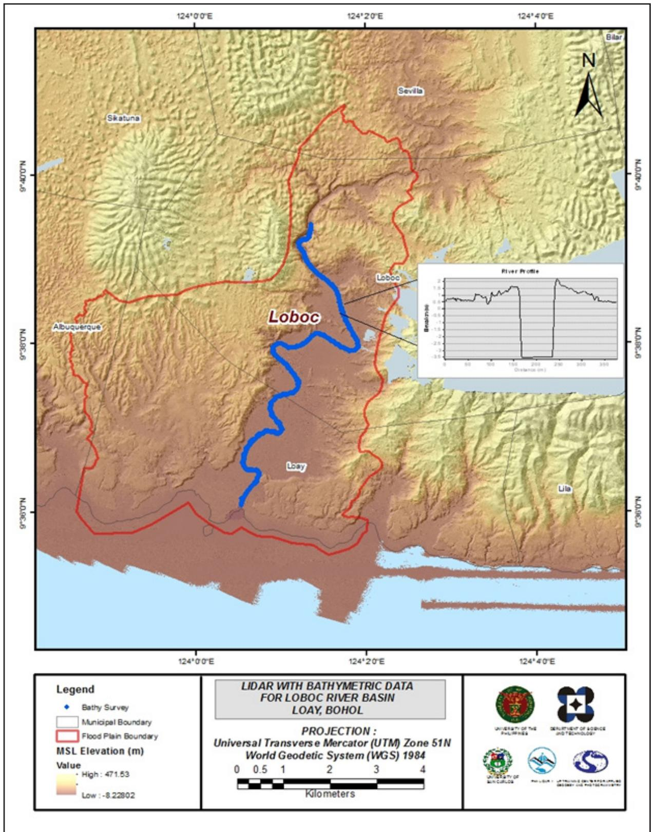
Figure 25. Map of Loboc Flood Plain with bathymetric survey points shown in blue.
