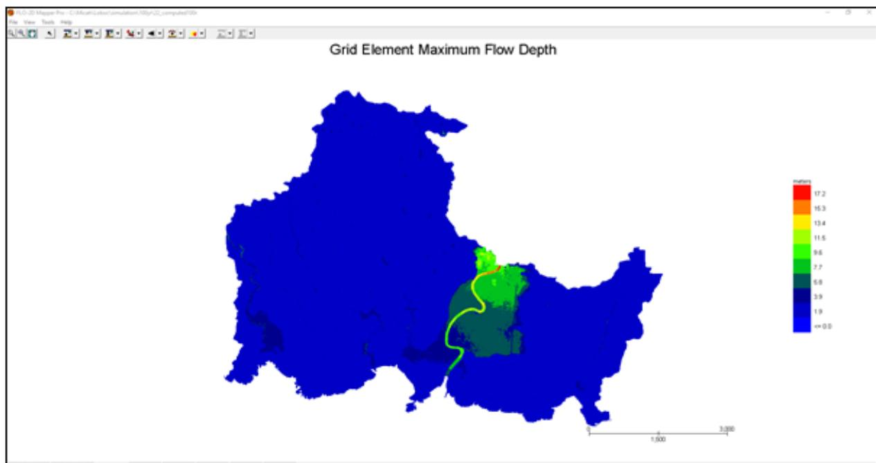
Figure 59. Generated 100-year rain return flow depth map from FLO-2D Mapper
