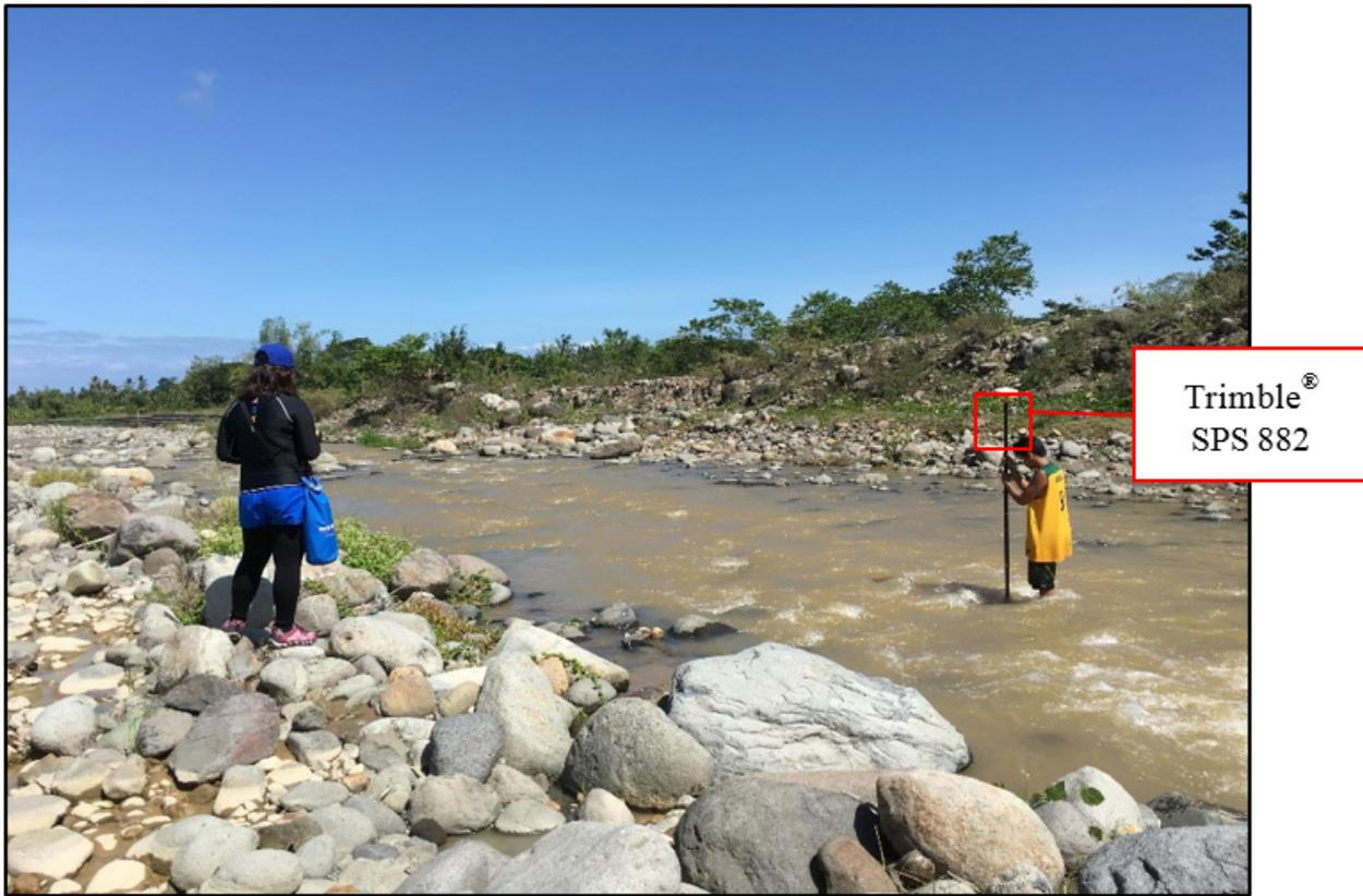
Figure 38. Cross-section survey conducted on Ocoy river in Brgy. Calabnugan, Municipality of Sibulan
