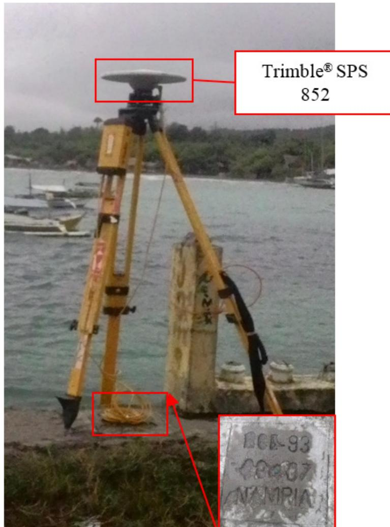
Figure 33. GNSS receiver set-up, Trimble® SPS 852, at NGE-93 in Brgy. Jilocon, Municipality of San Jose, Negros Oriental
