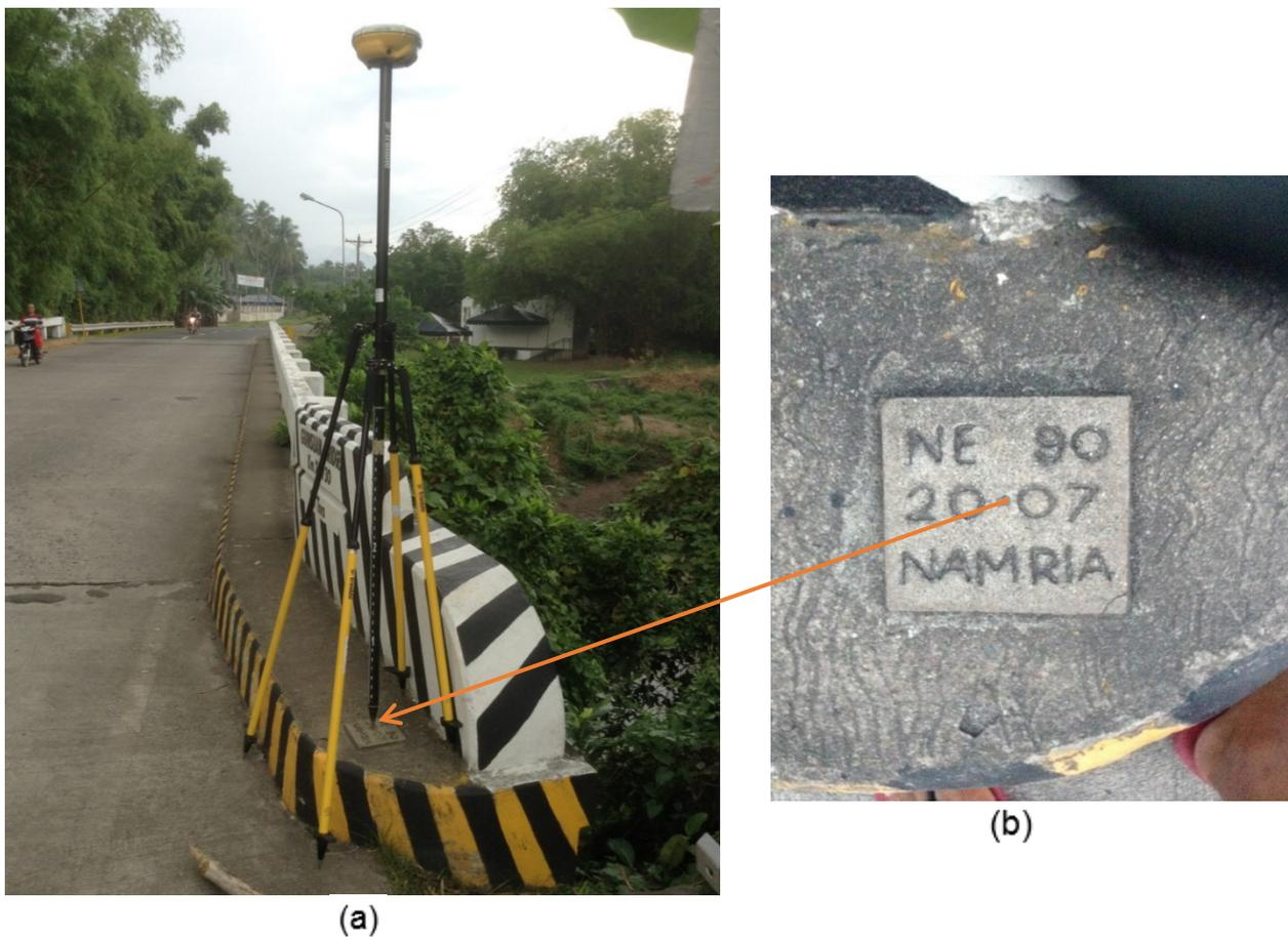
Figure 9. GPS set-up over NE-90 as recovered on the concrete sidewalk of Guinsan Bridge four (4) meters from the road centerline in Brgy. Poblacion under the municipality of Zamboangita. (a) and NAMRIA reference point NE-90 (b) as recovered by the field team.
