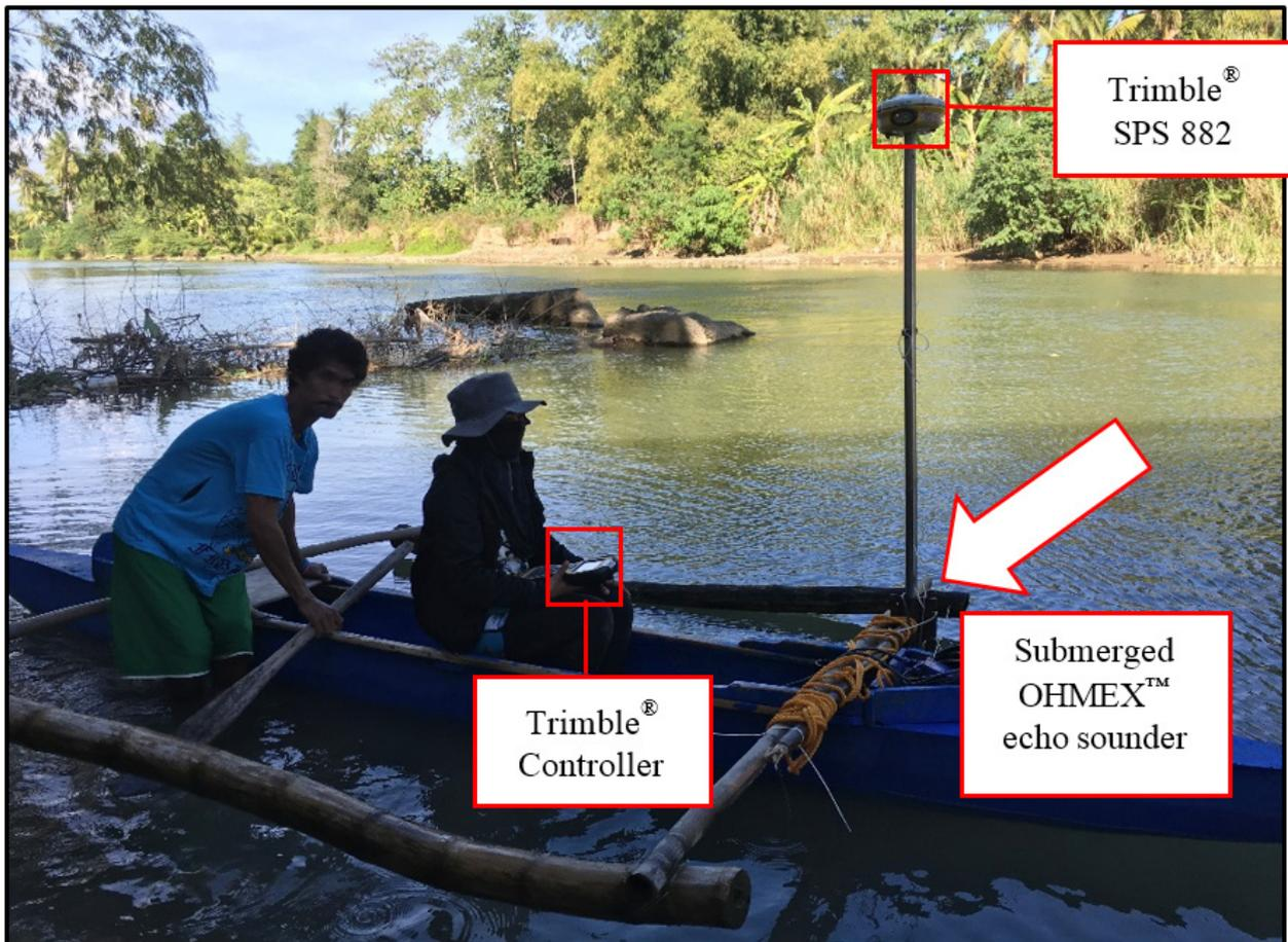
Figure 44. Bathymetric survey in Ocoy River
