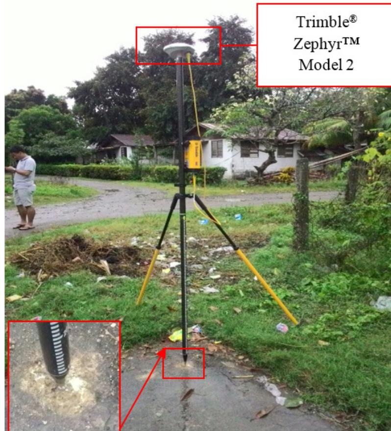
Figure 36. GNSS receiver set-up, Trimble® Zephyr™ Model 2, at UP-TAN in Brgy. Novallas, Tanjay City, Negros Oriental
