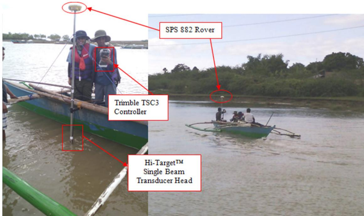
Figure 48. Bathymetric survey using Ohmex™ Echo Sounder along Sapangdaku River
