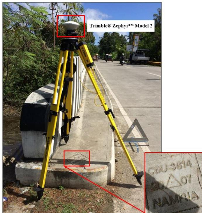
Figure 37. GNSS receiver set-up, Trimble® Zephyr™ Model 2, at CBU-3614, Lapu-lapu Bridge approach in Brgy. Poblacion, Municipality of Asturias, Cebu
