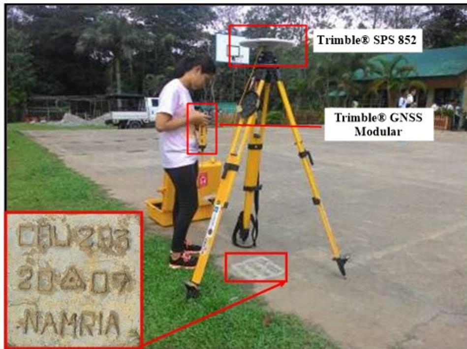
Figure 35. GNSS receiver set-up, Trimble® SPS 852, at CBU-293 in front of Cantabaco National High School in Brgy. Cantabaco, Toledo City, Cebu
