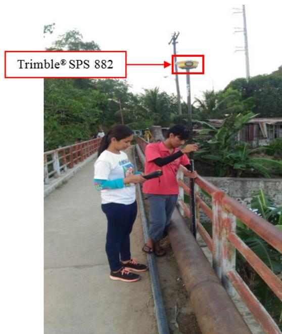
Figure 40. Bridge as-built and cross-section survey at the downstream side of Ilihan Foot Bridge in Brgy. Ilihan, Toledo City, Cebu
