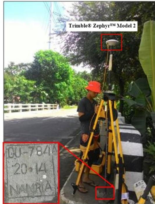
Figure 36. GNSS receiver setup, Trimble® Zephyr™ Model 2, at CU-784 Balud Bridge approach in Brgy. Balud, Toledo City, Cebu
