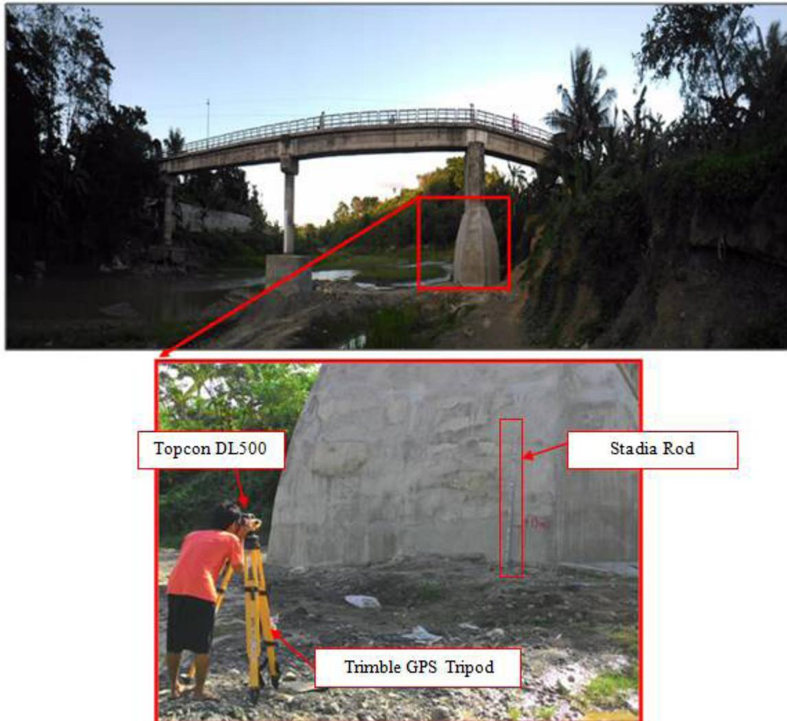
Figure 44. Water level marking using a Digital Level at Ilihan Foot Bridge, Brgy. Ilihan Toledo City
