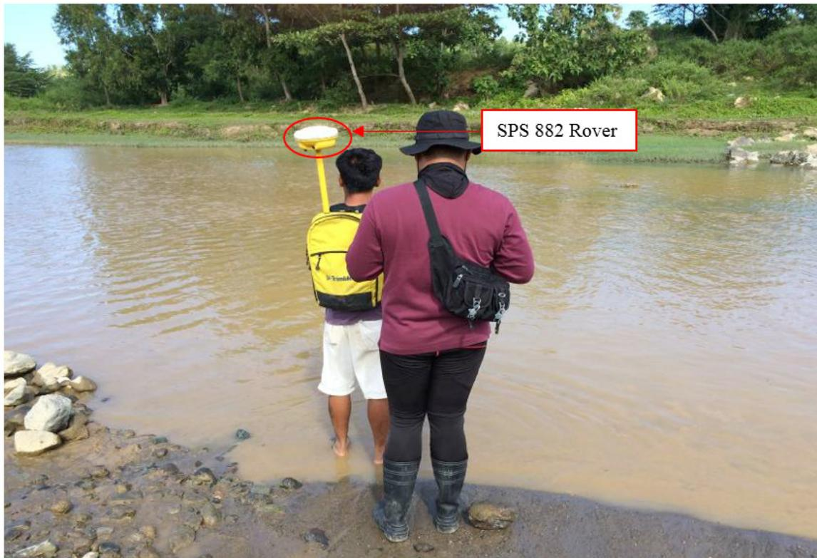
Figure 47. Manual bathymetry along Sapangdaku River
