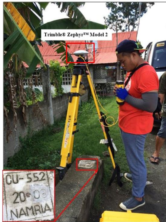
Figure 38. GNSS receiver set-up, Trimble® Zephyr™ Model 2, at CU-552 along the national highway in Brgy. Cantuod, Balamban, Cebu
