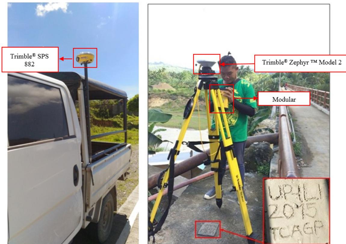
Figure 45. Validation points acquisition survey set-up
