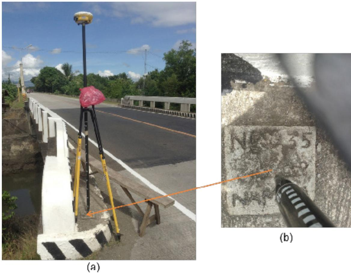
Figure 5. GPS set-up over NE-135 in Busuang Bridge on top of concrete sidewalk in Barangay Bio-os under the municipality of Amlan (a) and NAMRIA reference point NE-135 (b) as recovered by the field team.
