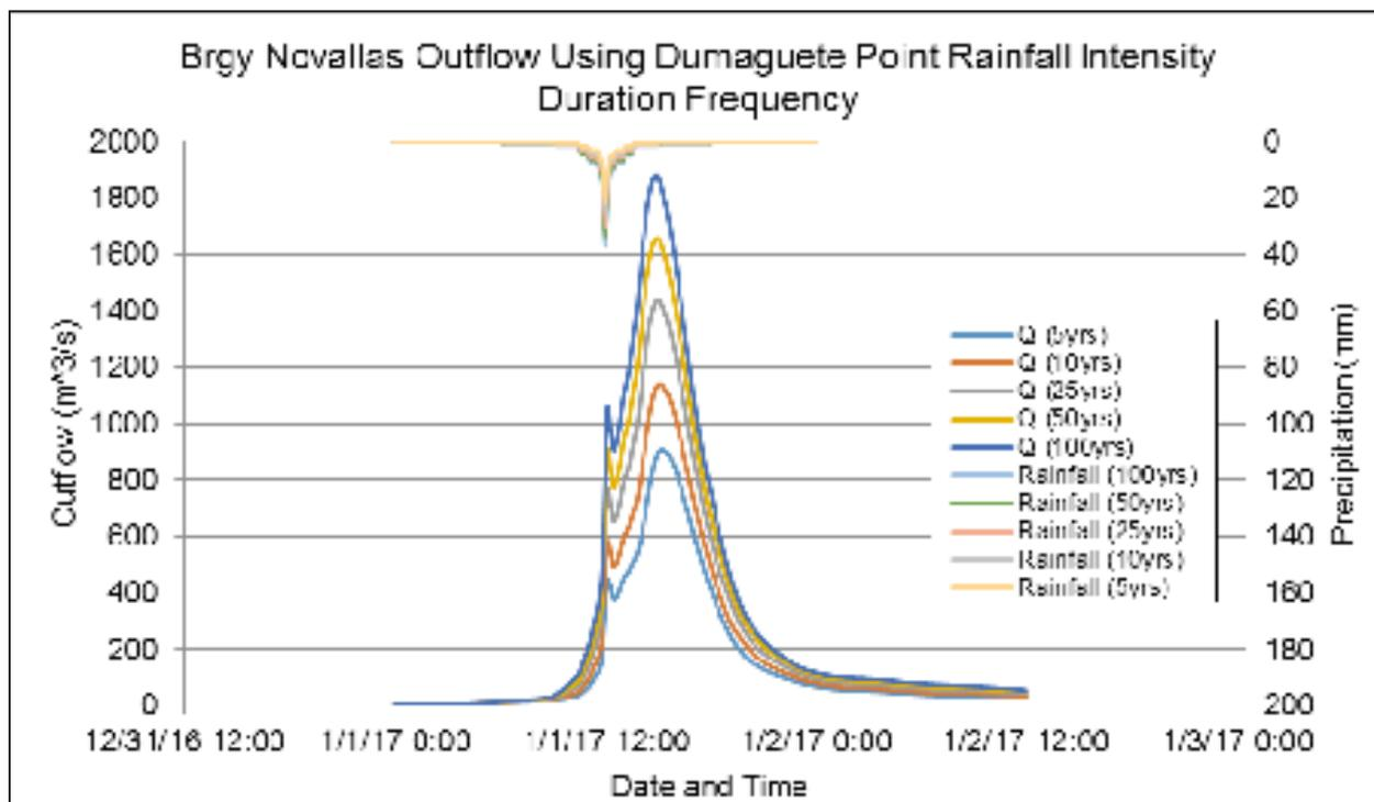
Figure 59. Outflow hydrograph at Brgy. Novallas, Tanjay City generated using Dumaguete Point RIDF simulated in HEC-HMS
