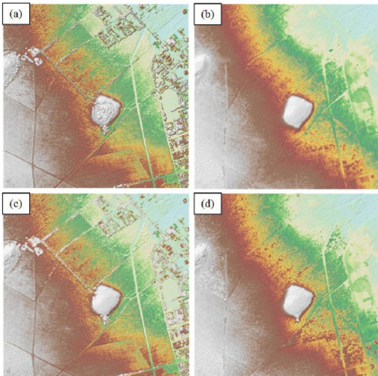
Figure 19. The production of last return DSM (a) and DTM (b), first return DSM (c) and secondary DTM (d) in some portion of Tanjay Floodplain.
