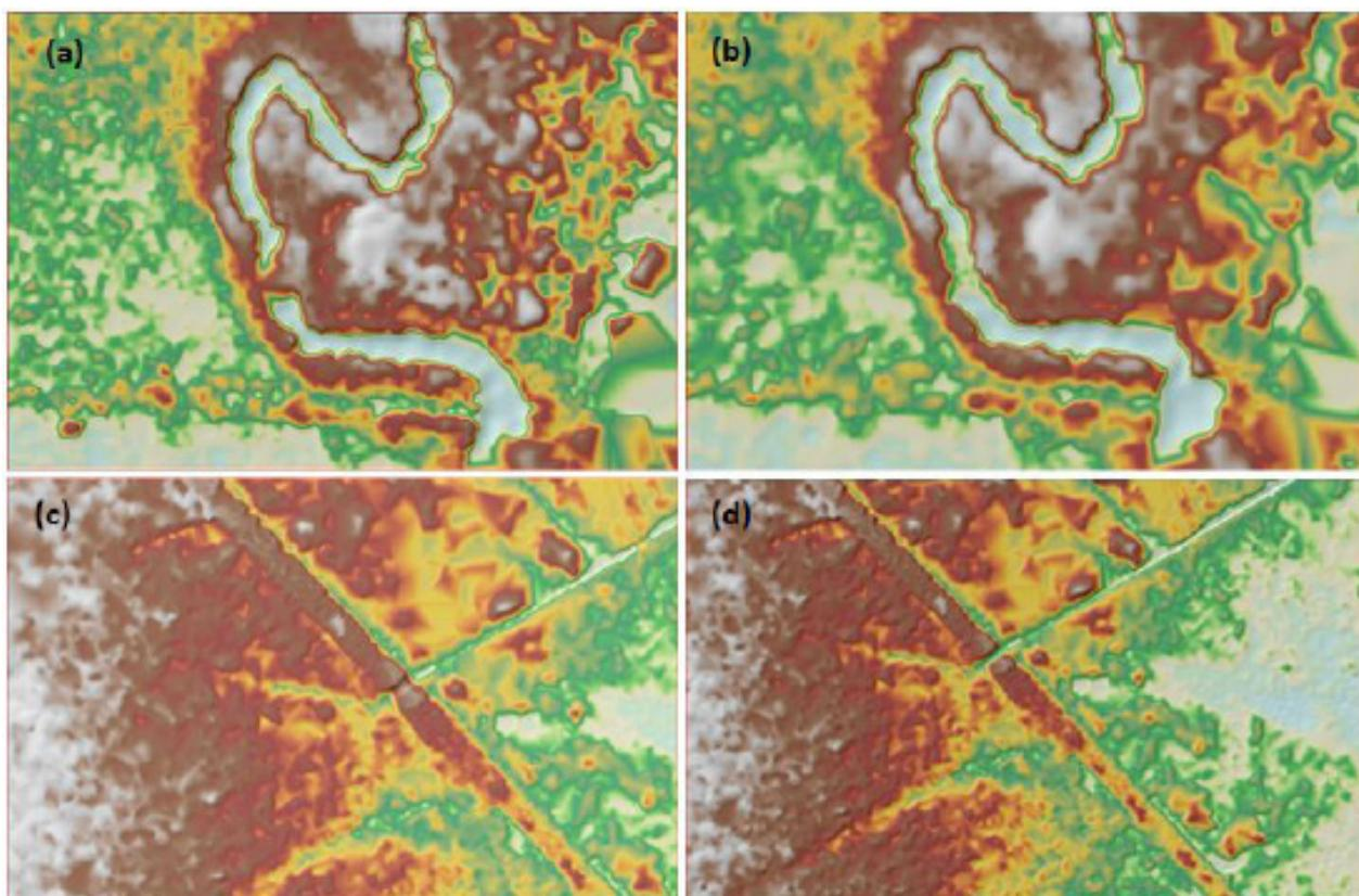
Figure 22. Portions in the DTM of Tanjay Floodplain – (a) before and (b) after editing; (c) before and (d) after bridge removal.
