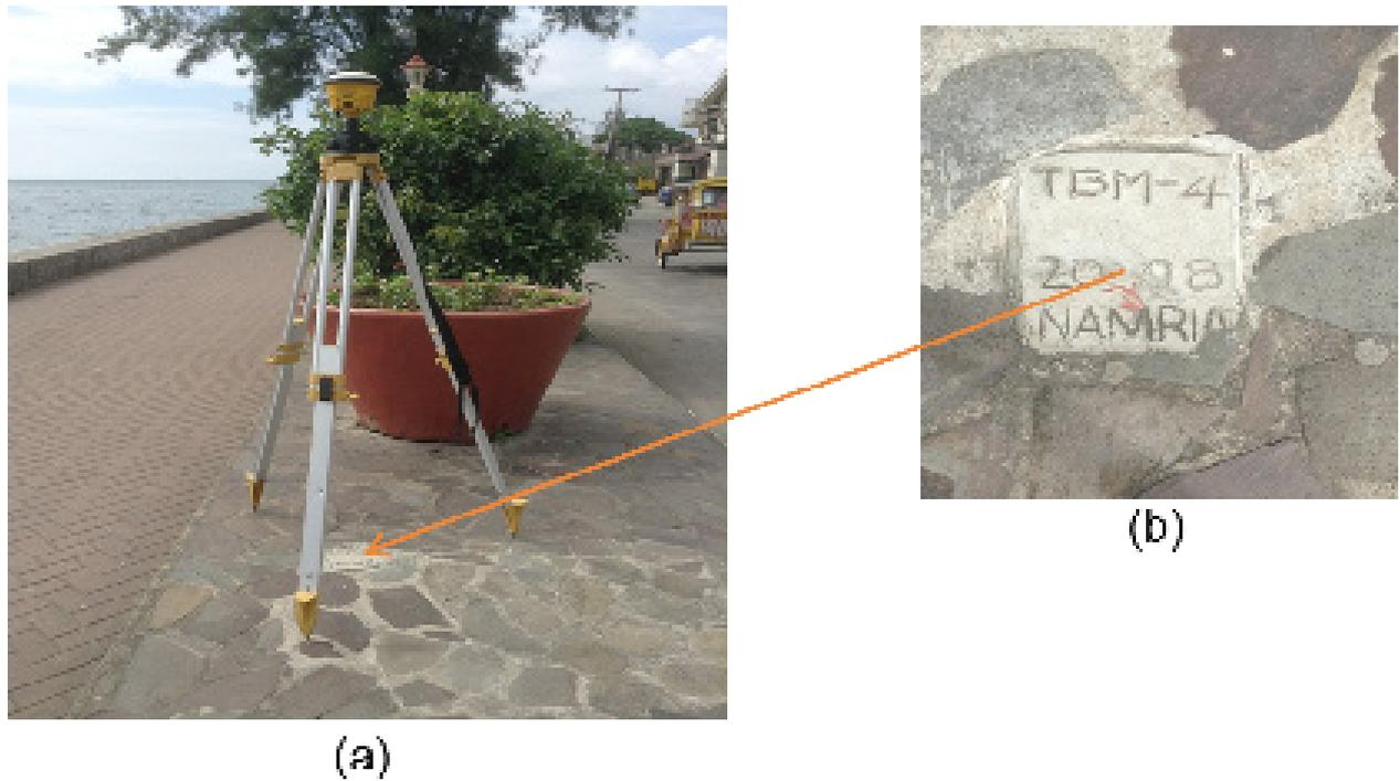
Figure 3. GPS set-up over TBM-4 on top of concrete pathway about 5 meters from the seawall of Dumaguete City’s boulevard (a) and NAMRIA reference point TBM-4 (b) as recovered by the field team.
