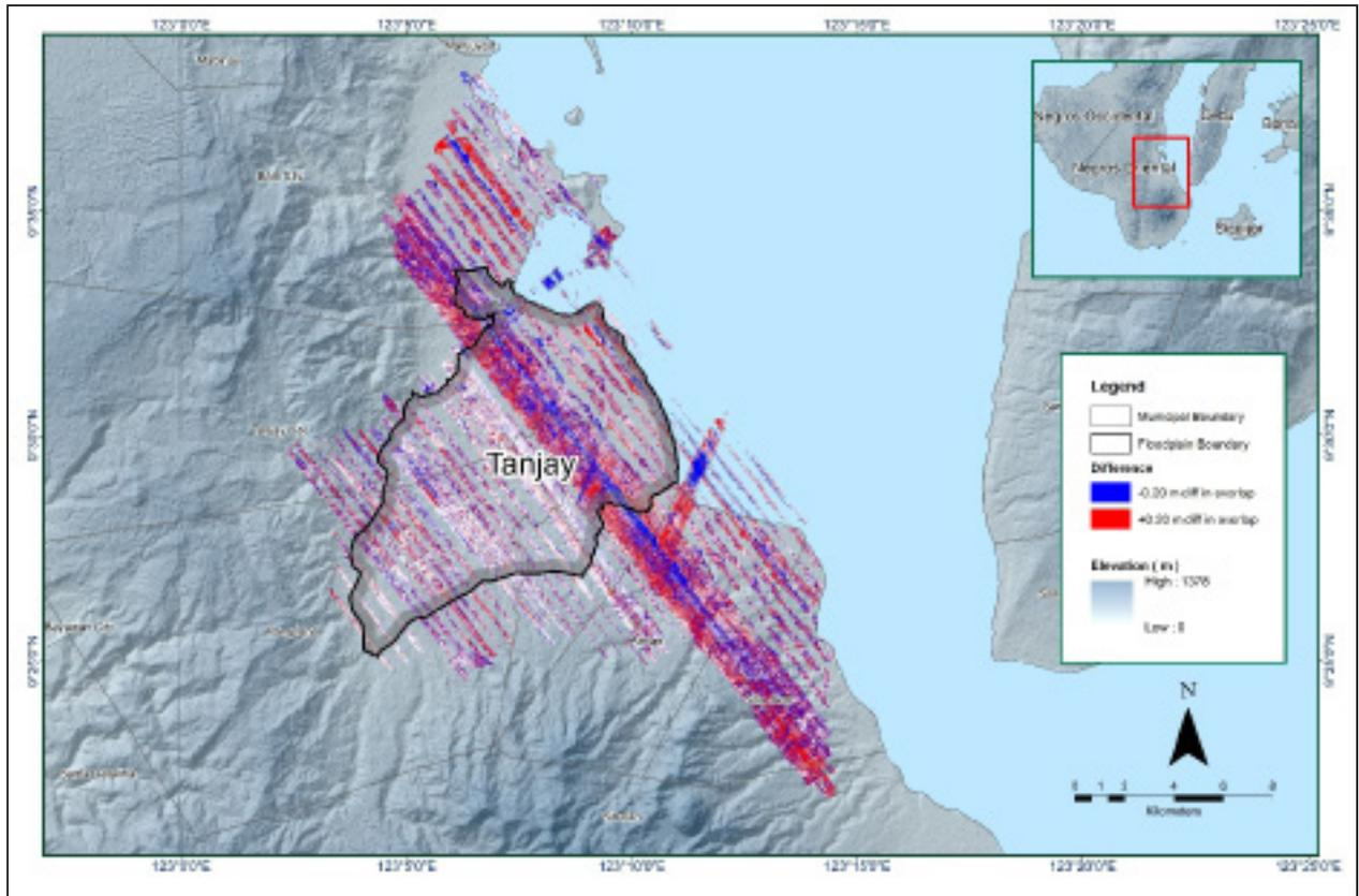
Figure 15. Elevation difference map between flight lines for Tanjay Floodplain.
