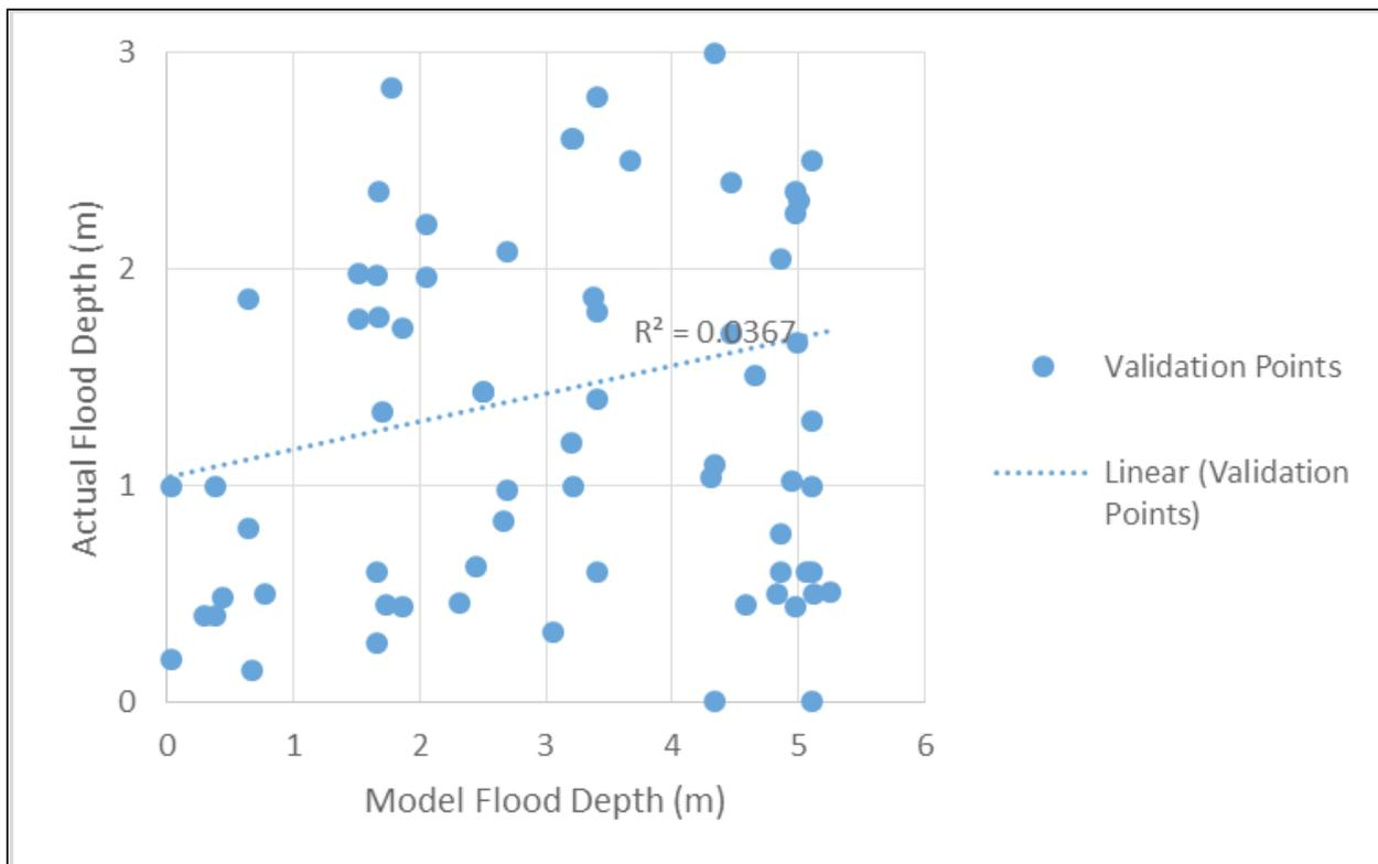
Figure 77. Flood map depth vs. actual flood depth
