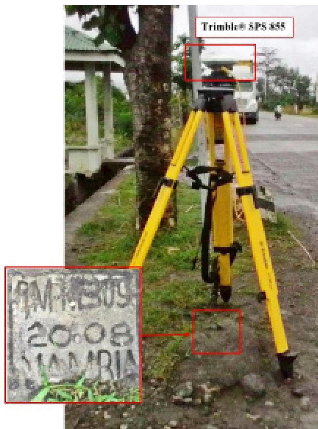
Figure 34. GNSS base set up, Trimble® SPS 855, at NE-309, a BM used as a marker, located on top of a rock along Western Nautical Highway in Brgy. San Jose, City of Tanjay, Negros Oriental
