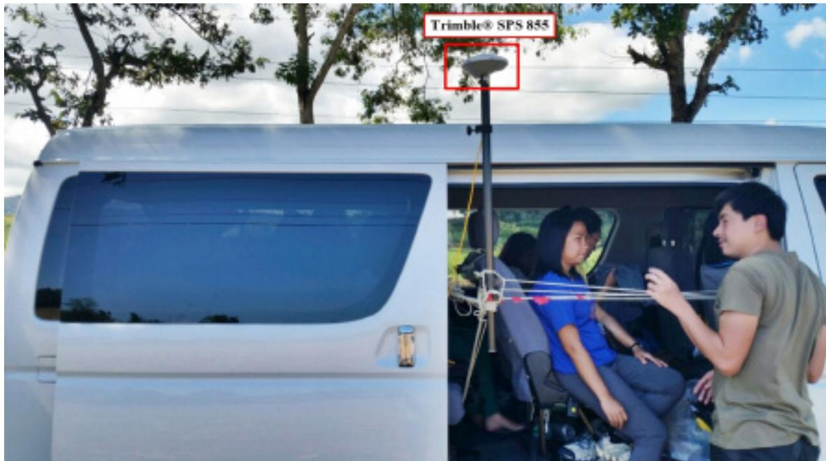
Figure 40. Validation points acquisition survey set-up
