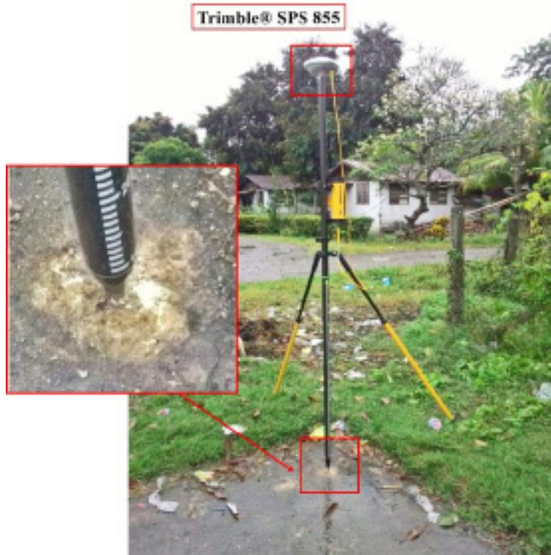
Figure 35. GNSS receiver set up, Trimble® SPS 855, at UP-TAN, an established control point located in Brgy. Novallas, Tanjay City, Negros Oriental
