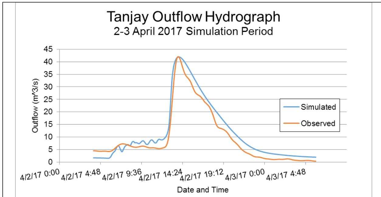
Figure 58. Outflow Hydrograph of Tanjay produced by the HEC-HMS model compared with observed outflow.
