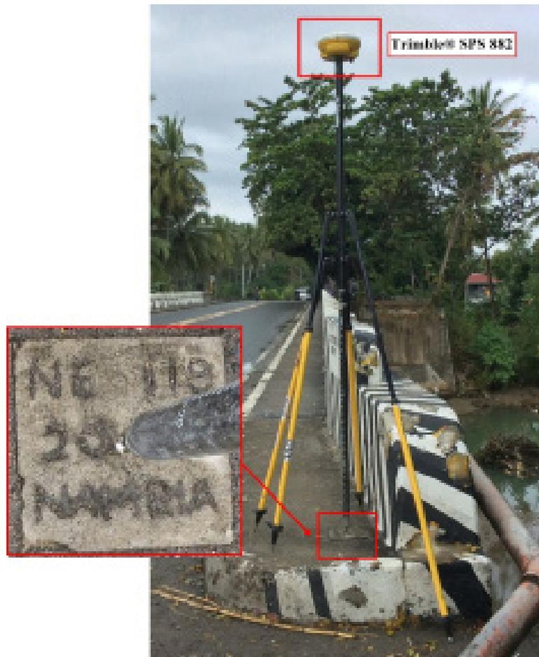
Figure 32. GNSS receiver setup, Trimble® SPS 882, at NE-119 at the approach of Ocoy Bridge in Brgy. Campaclan, Municipality of Sibulan, Negros Oriental
