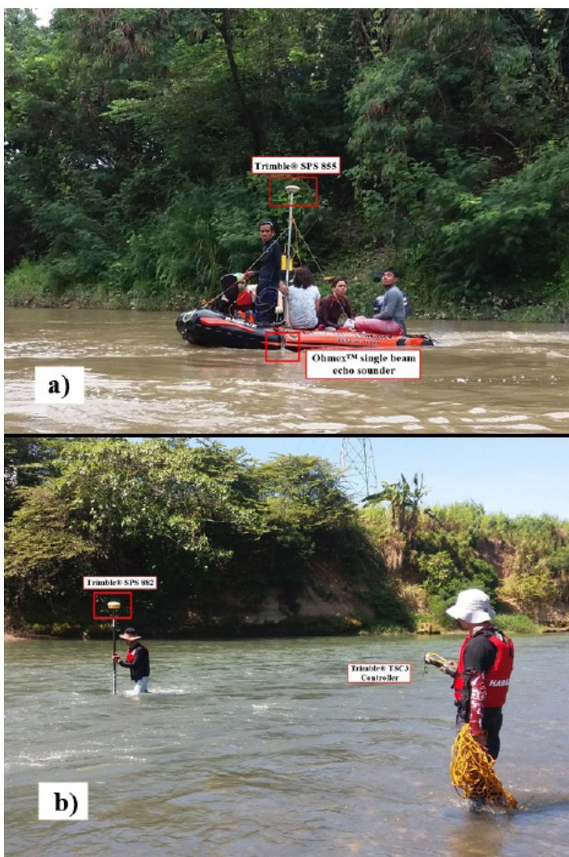
Figure 42. Bathymetric survey of ABSD at Tanjay River using a Hi-Target™ GNSS Rover Receiver
