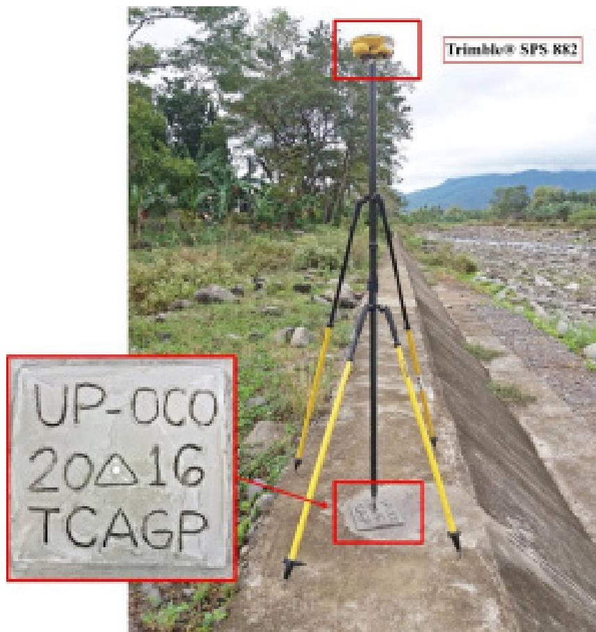
Figure 36. GNSS receiver set-up, Trimble® SPS 882 at control point UP-OCO near the abutment of Sibulan Bridge Brgy. Calabnugan, Municipality of Sibulan, Negros Oriental
