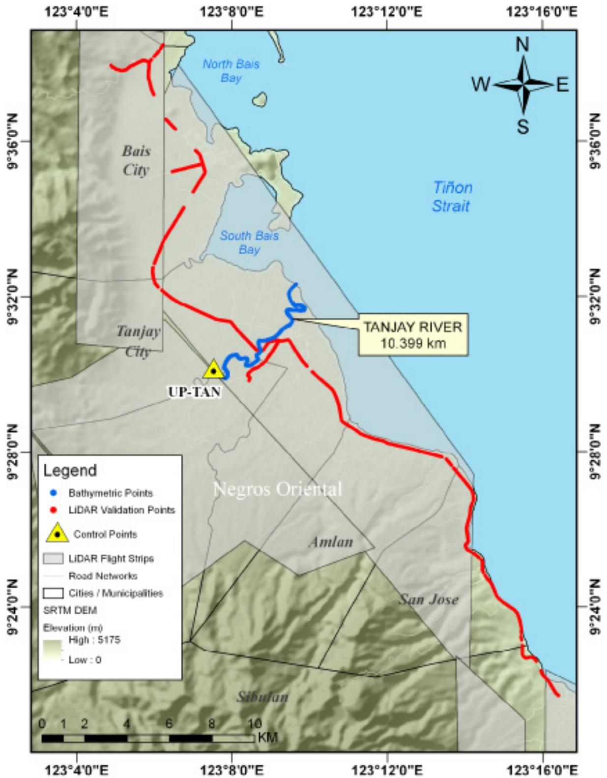
Figure 41. LiDAR Validation points acquisition survey for Tanjay River Basin
