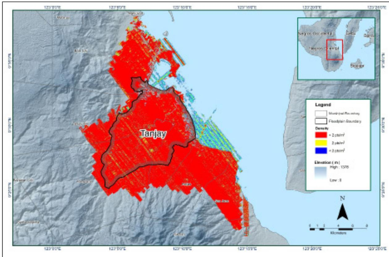
Figure 14. Pulse density map of merged LiDAR data for Tanjay Floodplain.
