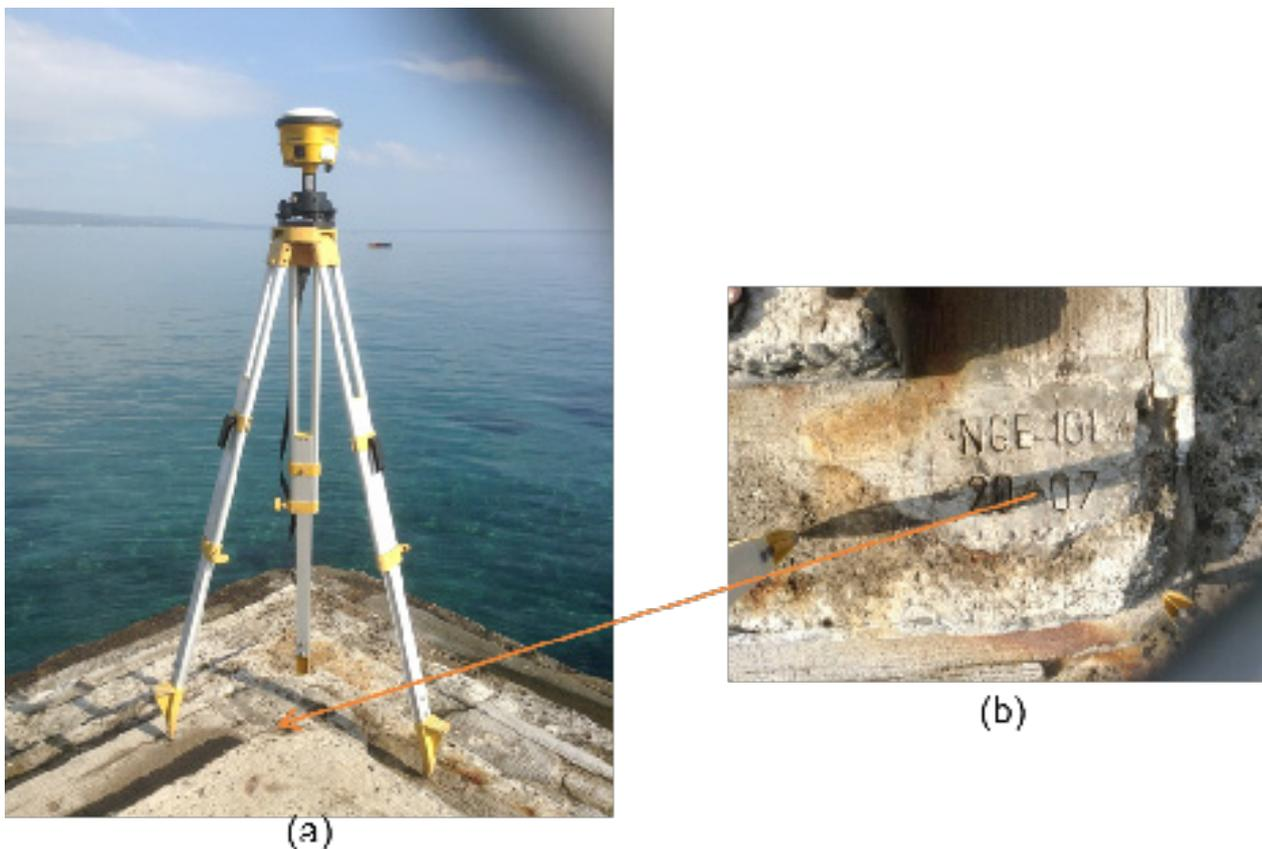
Figure 4. GPS set-up over NGE-101 on the third step from the top flooring of the pier NE corner in barangay Poblacion under the municipality of Sibulan (a) and NAMRIA reference point NGE-101 (b) as recovered by the field team.
