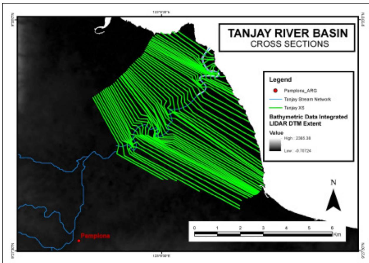
Figure 56. River cross-section of Tanjay River generated through Arcmap HEC GeoRAS tool
