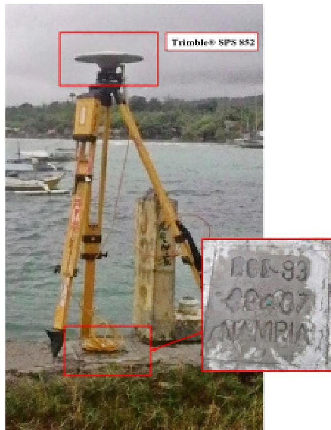
Figure 33. GNSS receiver set-up, Trimble® SPS 852, at NGE-93 in Brgy. Jilocon, Municipality of San Jose, Negros Oriental
