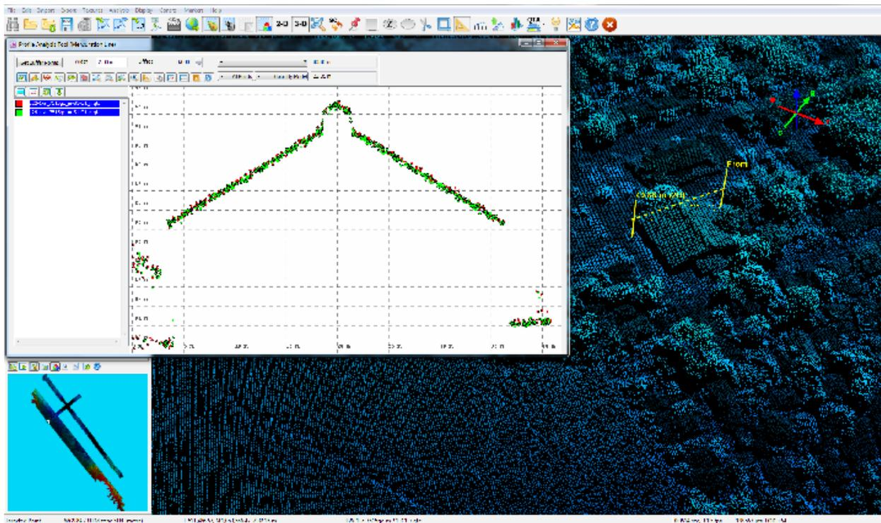
Figure 16. Quality checking for Tanjay Flight 7515G using the Profile Tool of QT Modeler.
