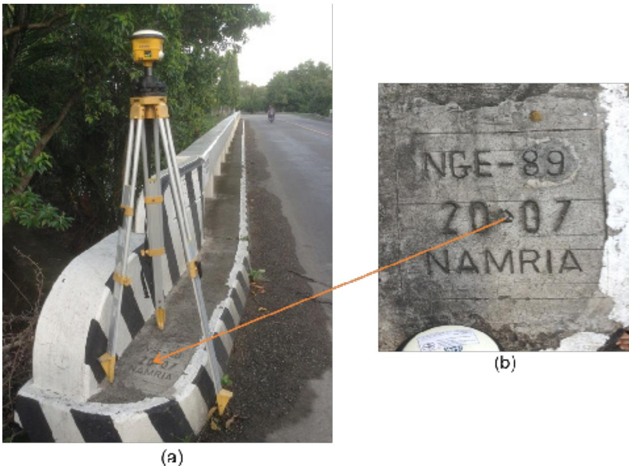
Figure 6. GPS set-up over NGE-89 on the SE corner of Bio-os Bridge in Barangay Bio-os under the municipality of Amlan (a) and NAMRIA reference point NGE-89 (b) as recovered by the field team.
