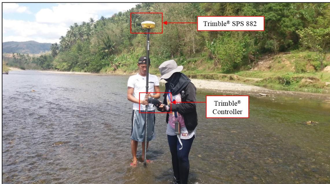
Figure 40. Manual bathymetry set-up for Tiabanan River survey
