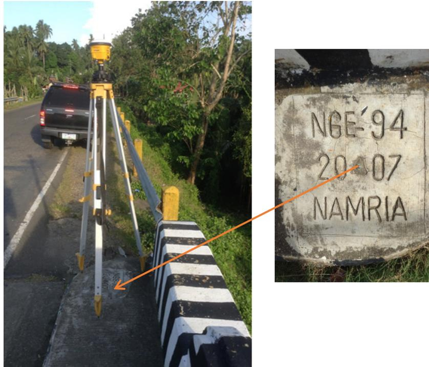
Figure 3. GPS set-up over NGE-94 on the south approach of Tiabanan’s bridge wingwall sidewalk in Barangay Bal-OS under the municipality of Basay (a) and NAMRIA reference point NGE-94 (b) as recovered by the field team.
