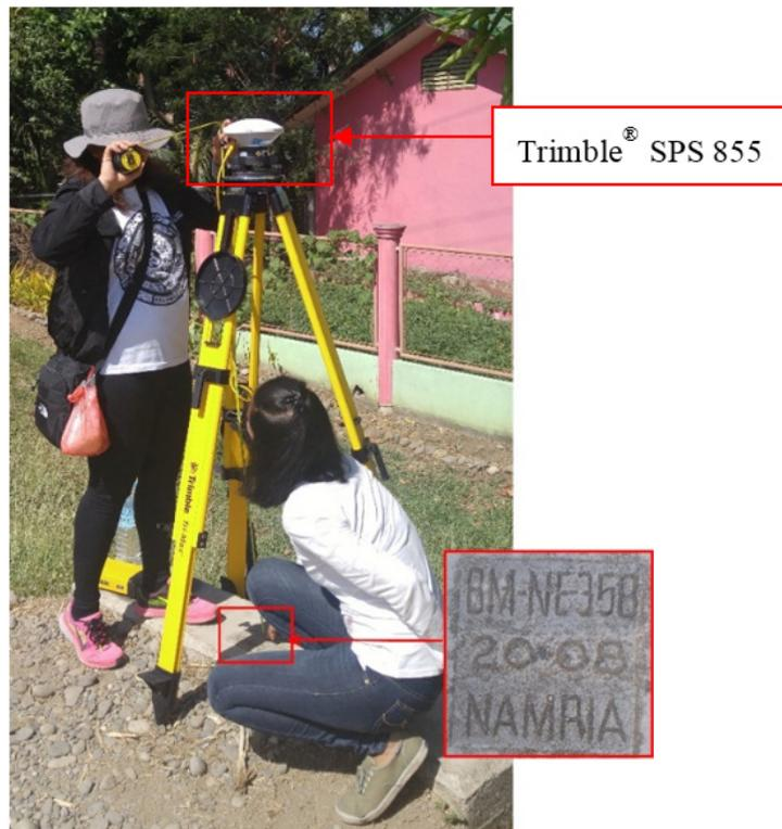
Figure 30. GNSS base set up, Trimble® SPS 855, at NE-358, a first-order BM, located on a culvert along Sta. Caalina-Bayawan Road in Brgy. Ubos, Bayawn City, Negros Oriental
