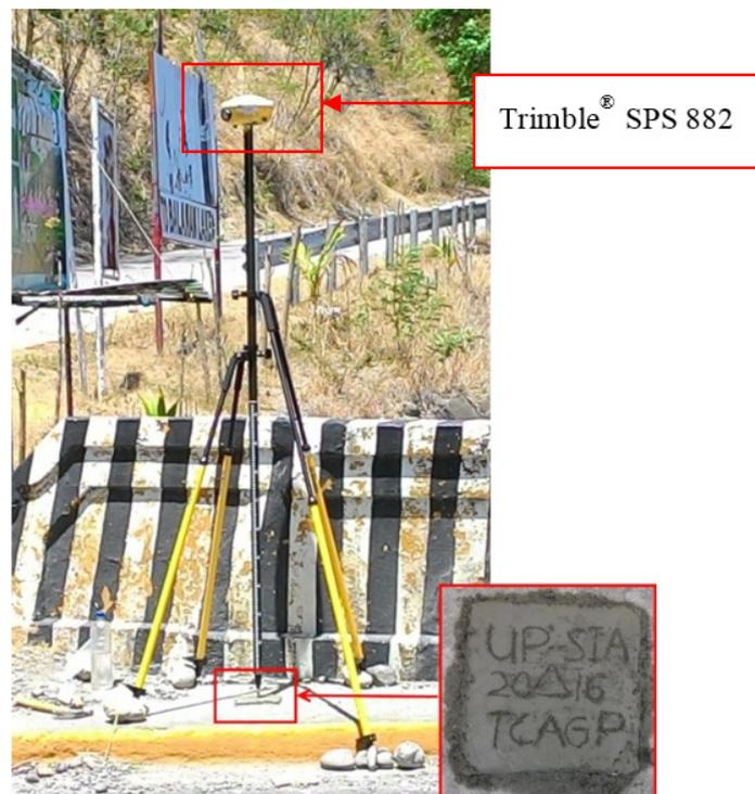
Figure 32. GNSS receiver set up, Trimble® SPS 882, at UP-SIA, an established control point, located at the approach of Siaton Bridge in Brgy. Caticugan, Siaton, Negros Oriental
