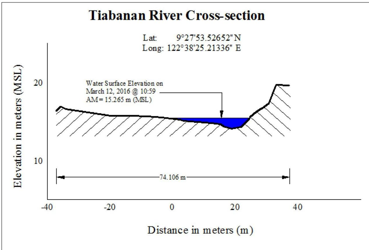
Figure 35. Tiabanan River Cross-section Diagram
