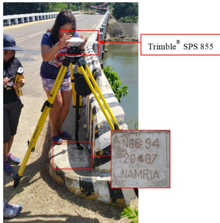
Figure 31. GNSS base set up, Trimble® SPS 855, at NGE-94, a GCP used as marker, located at the approach of Tiabanan Bridge in Brgy. Bongalonan, Basay, Negros Oriental
