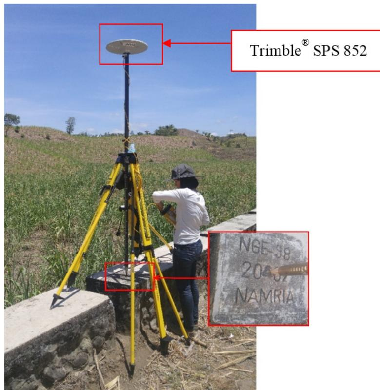
Figure 28. GNSS base set up, Trimble® SPS 852, at NGE-98 a second-order GCP located on top of a concrete block along Sta. Catalia-Pamplona Provincial Road in Brgy. Caranoche, Sta. Catalina, Negros Oriental
