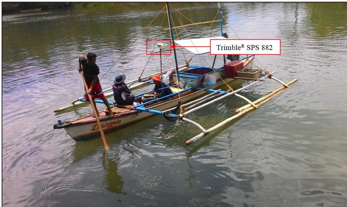
Figure 39. Bathymetry by boat set-up for Tiabanan River survey
