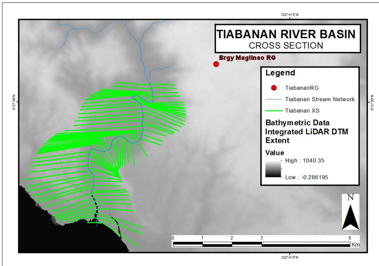
Figure 54. River cross-section of Tiabanan River generated through Arcmap HEC GeoRAS tool
