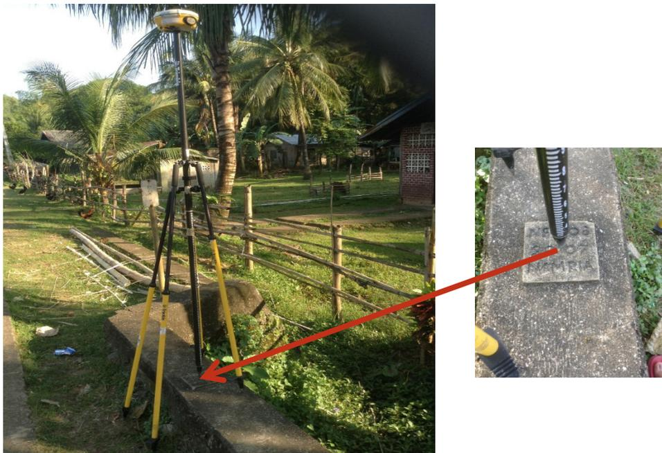
Figure 4. GPS set-up over NE-08 on top center of reinforced concrete pipe culvert about 7 meters from the roadline located in the municipality of Basay, Barangay Nagbualao along the national road going to Hinoba-An (a) and NAMRIA reference point NE-08 (b) as recovered by the field team.
