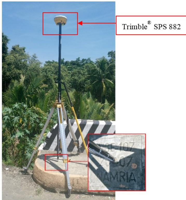
Figure 29. GNSS base set up, Trimble® SPS 882, at NE-107, a second-order GCP located at the approach of Manalongon Bridge in Brgy. Manalongon, Sta. Catalina, Negros Oriental
