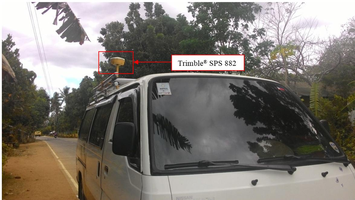
Figure 37. Validation points acquisition survey set-up
