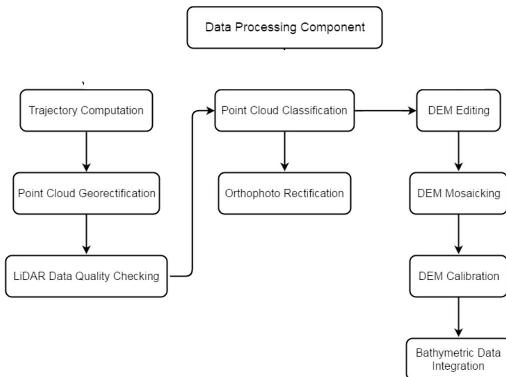
Figure 6. Schematic Diagram for Data Pre-Processing Component
