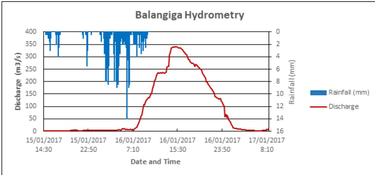
Figure 57. Rainfall and outflow data at the Balangiga Bridge used for modeling
