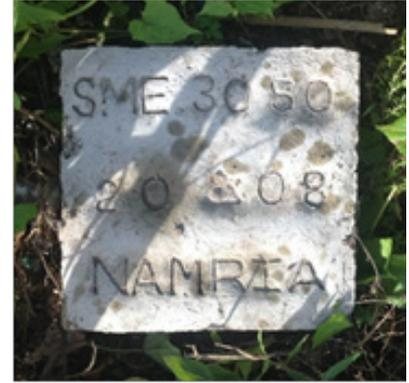
Figure 6. (a) GPS set-up over SME-3050 inside the premises of Central Elementary School, Barangay Poblacion, Guiuan, Eastern Samar, and (b) NAMRIA reference point SME-3050, as recovered by the field team
