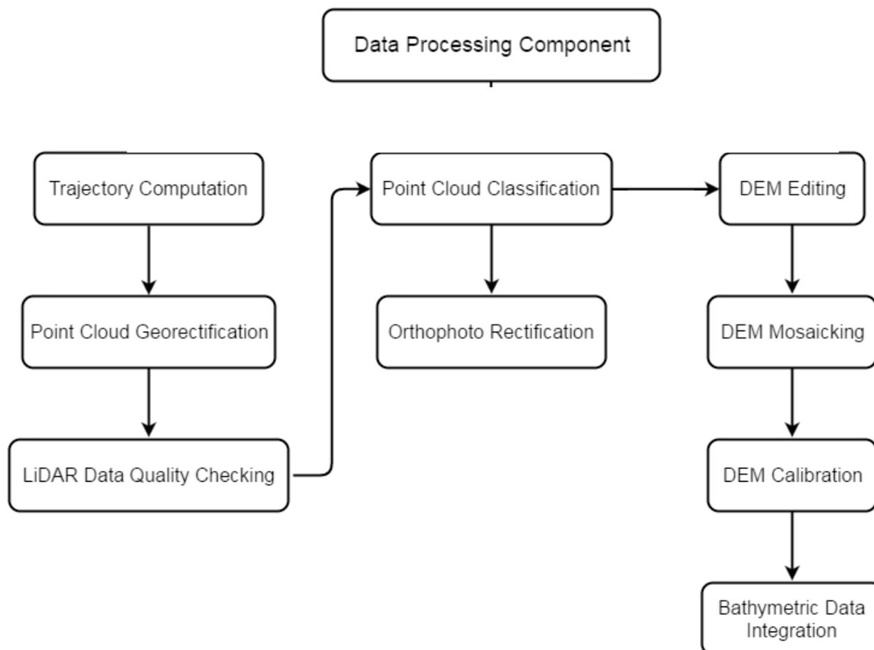
Figure 11. Schematic diagram for the Data Pre-Processing Component
