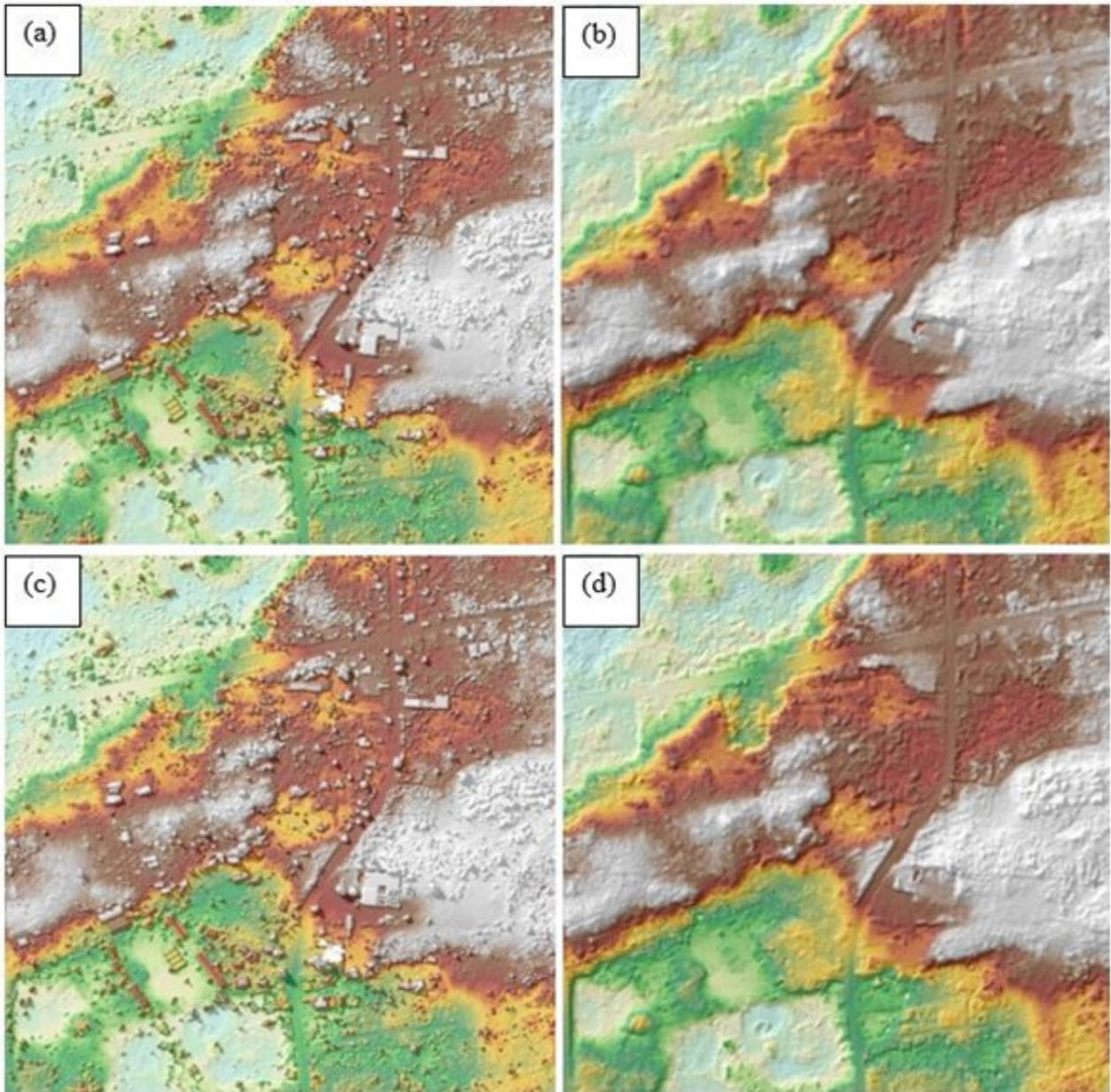
Figure 22. The production of last return DSM (a) and DTM (b), first return DSM (c) and secondary DTM (d) in some portion of the Balangiga Floodplain
