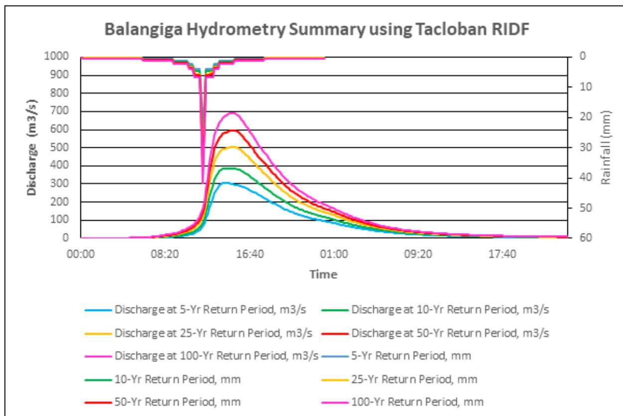
Figure 68. Outflow hydrograph at the Balangiga Station, generated using the Tacloban RIDF simulated in HEC-HMS
