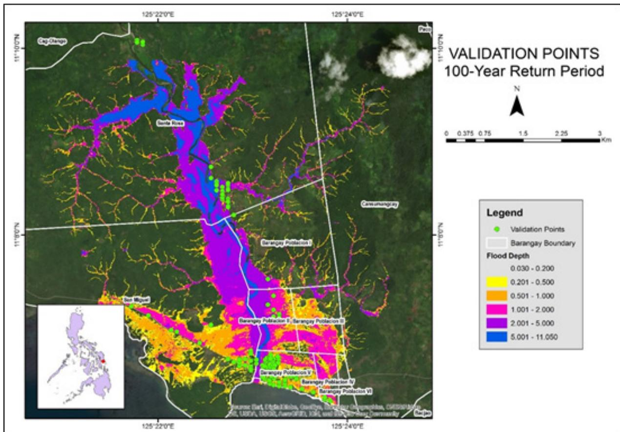
Figure 83. Validation points for a 100-year flood depth map of the Balangiga Floodplain
