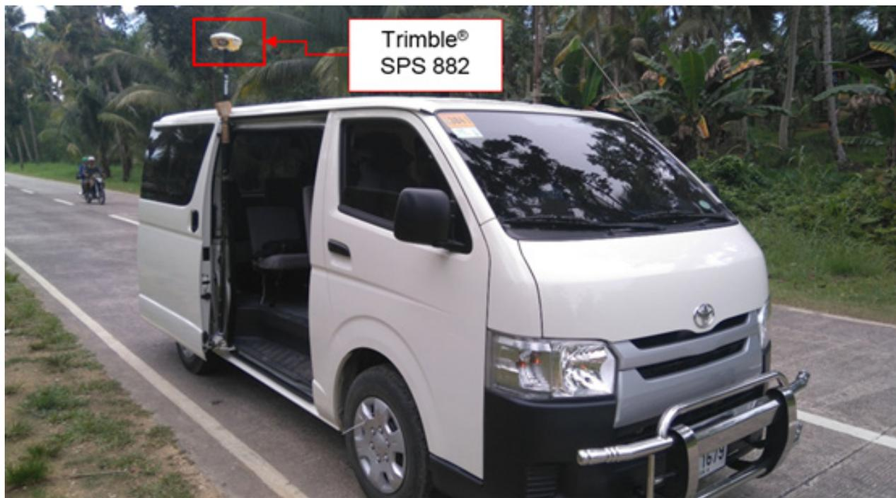
Figure 48. Validation points acquisition survey set-up along the Balangiga River Basin
