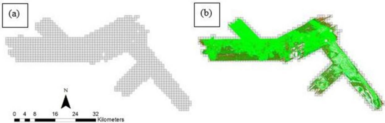
Figure 20. The coverage of the Balangiga Floodplain Survey (a) the tile system (b) depicts the classification results in TerraScan.
