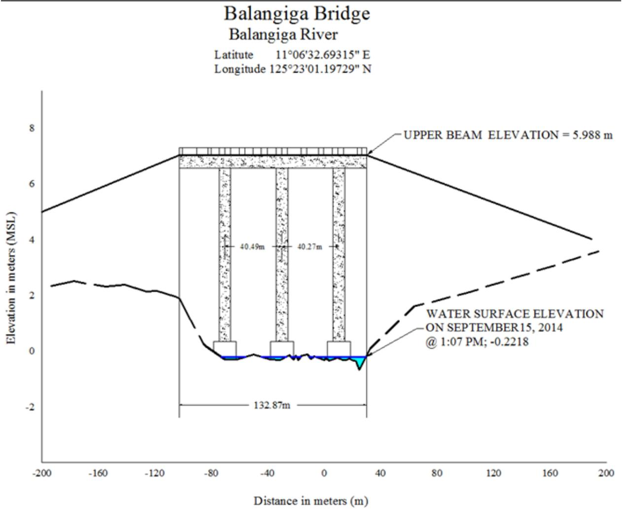
Figure 45. Balangiga Bridge cross-section diagram
