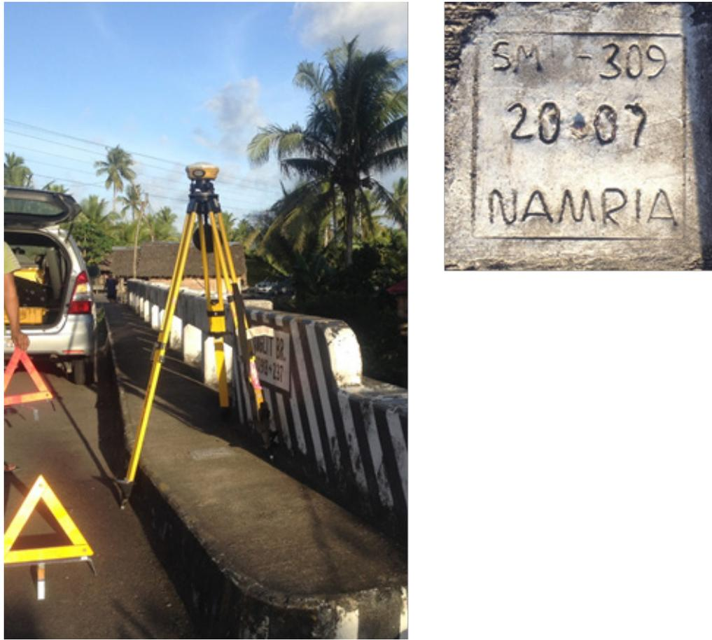
Figure 8. (a) GPS set-up over SM-309 located at the Dalid Bridge along the national highway in Barangay San Pascual, Sta. Rita, Samar, and (b) NAMRIA reference point SM-309, as recovered by the field team
