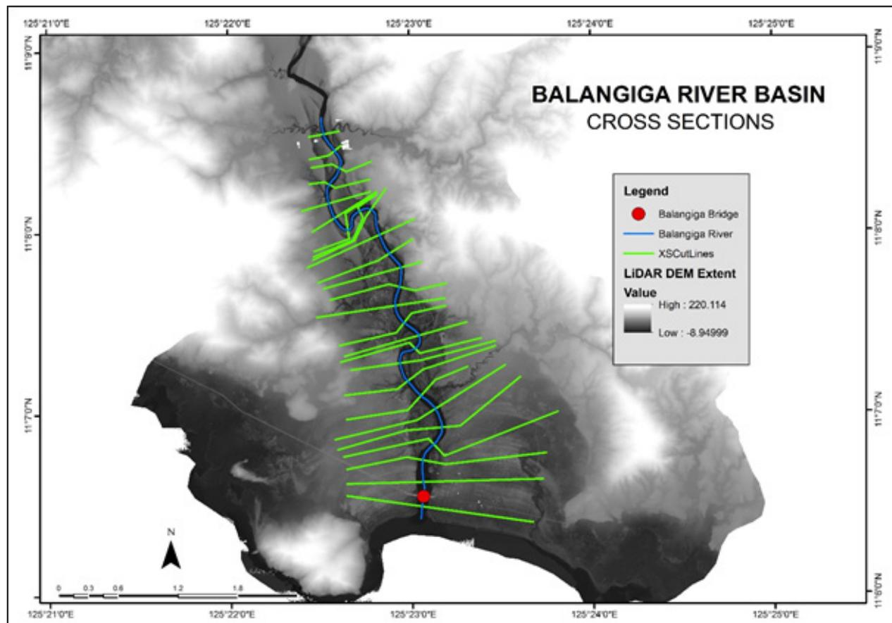
Figure 65. Cross-section of the Balangiga River generated through the ArcMap HEC GeoRAS tool
