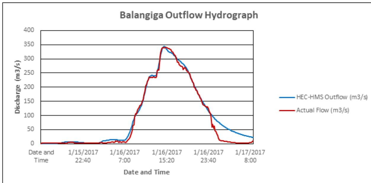
Figure 67. Outflow Hydrograph of the Balangiga Bridge generated in the HEC-HMS model, compared with observed outflow
