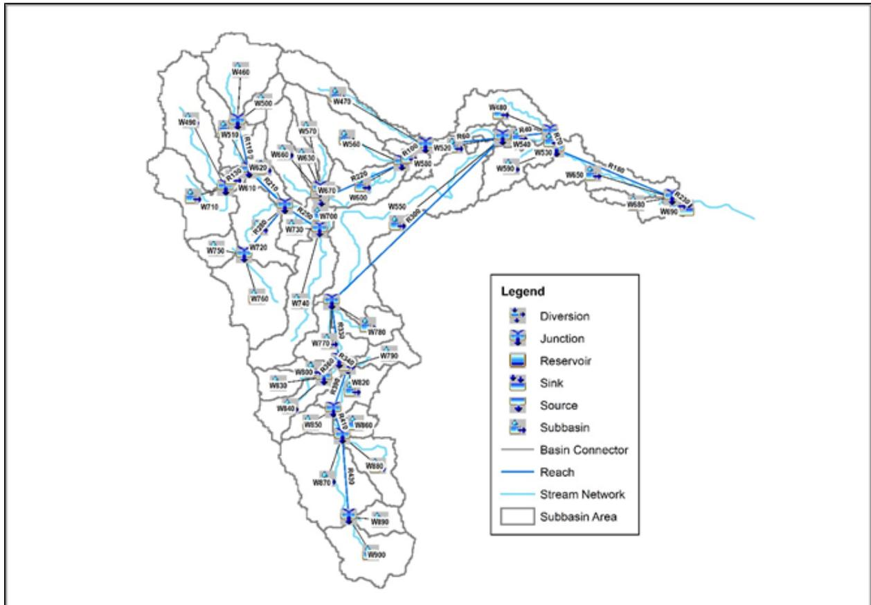
Figure 64. The Balangiga River Basin model generated using HEC-HMS
