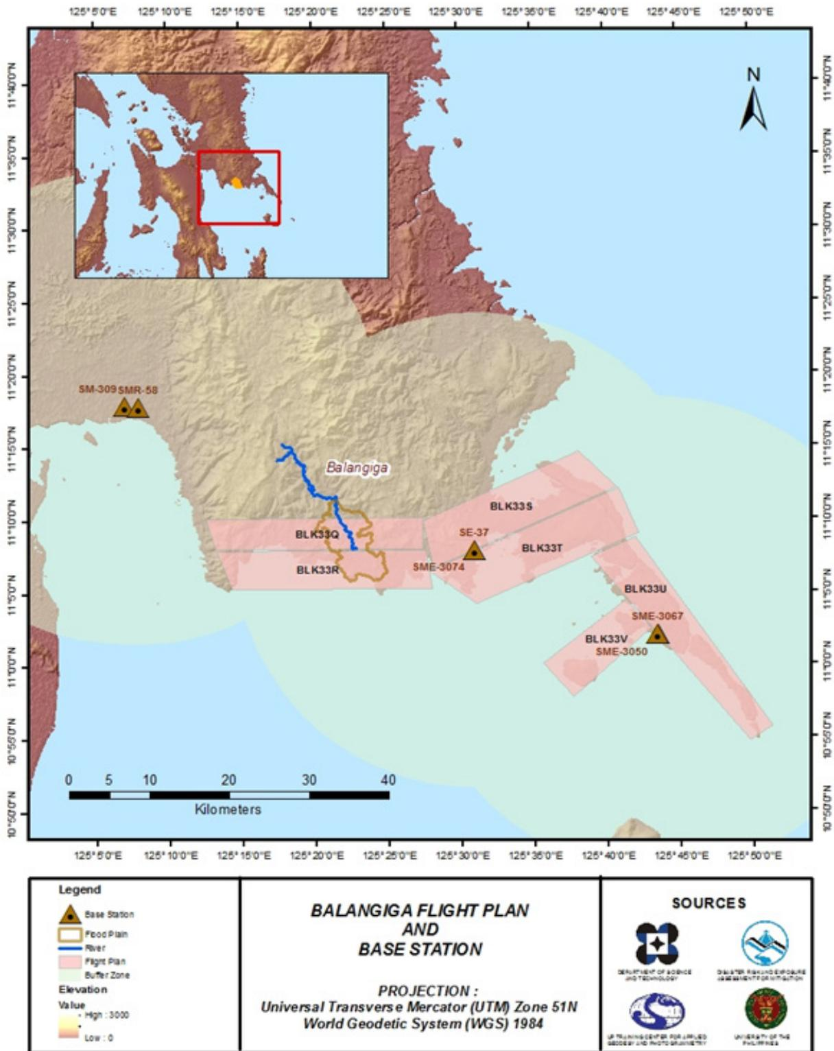
Figure 2. Flight Plan and base stations used for the Balangiga Floodplain survey using Aquarius sensor.
