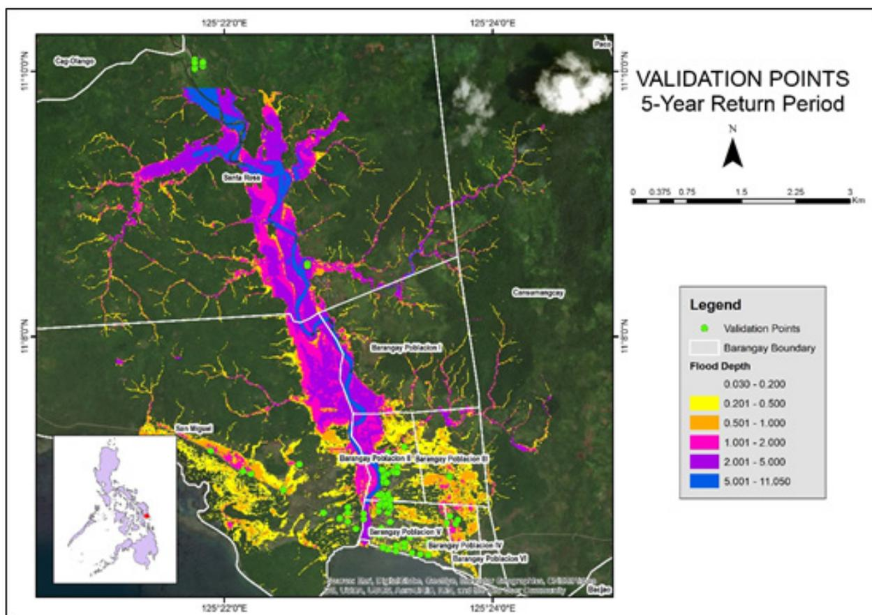
Figure 82. Validation points for 5-year flood depth map of the Balangiga Floodplain
