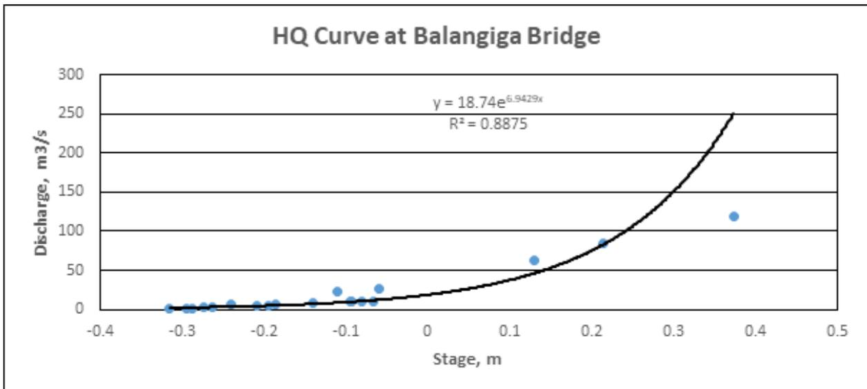
Figure 56. Rating curve at the Balangiga Bridge
