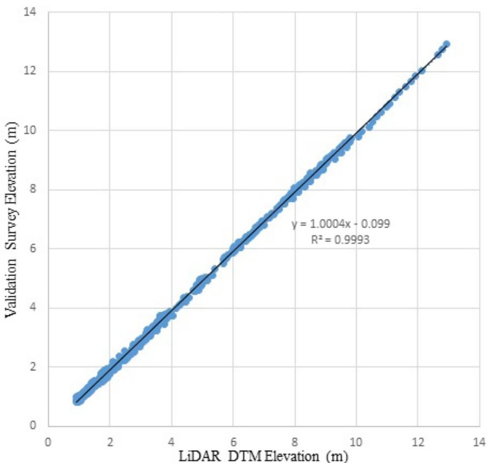
Figure 29. Correlation plot between the validation survey points and the LiDAR data
