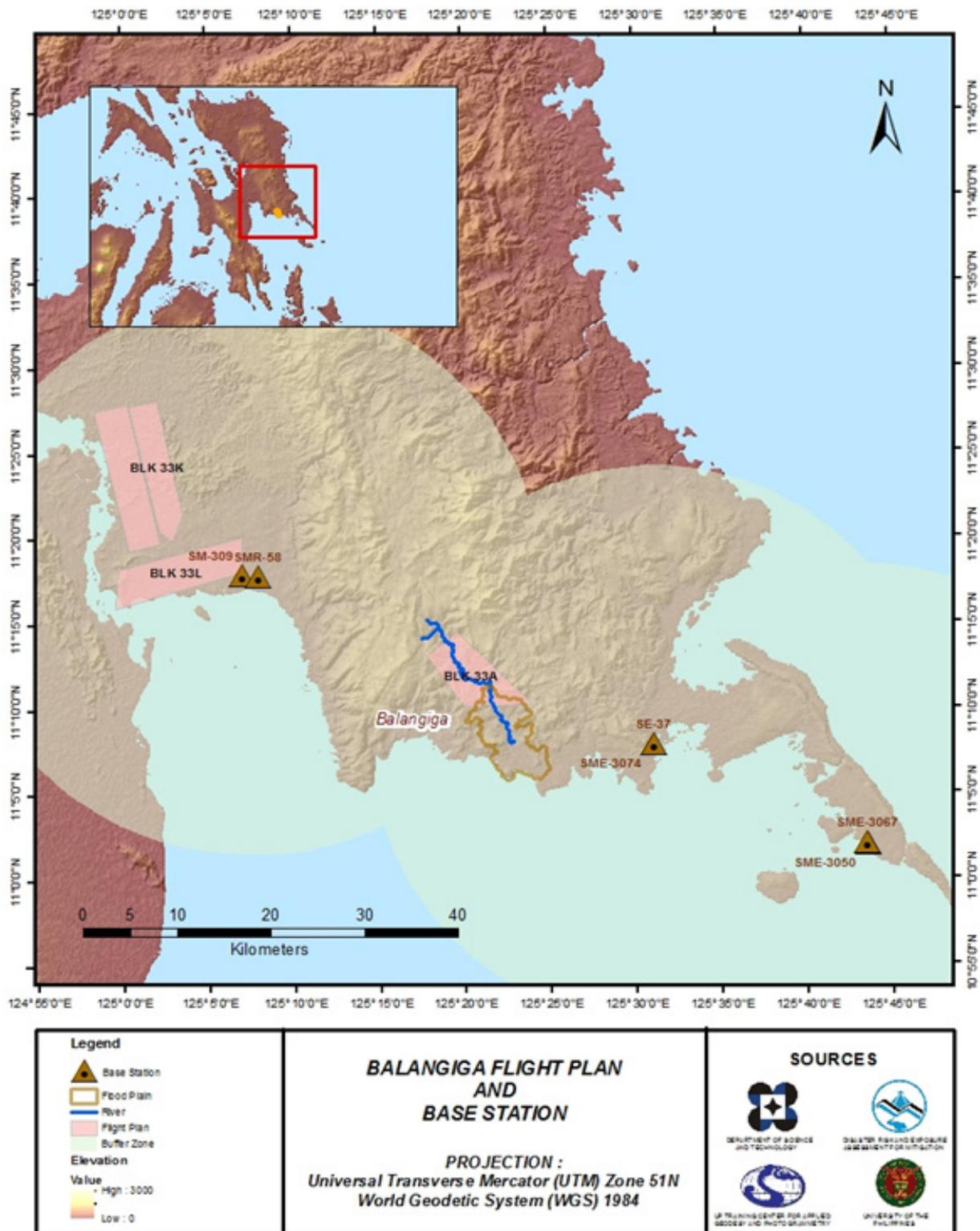
Figure 3. Flight plans and base stations used to cover the Balangiga Floodplain using the Gemini LiDAR system
