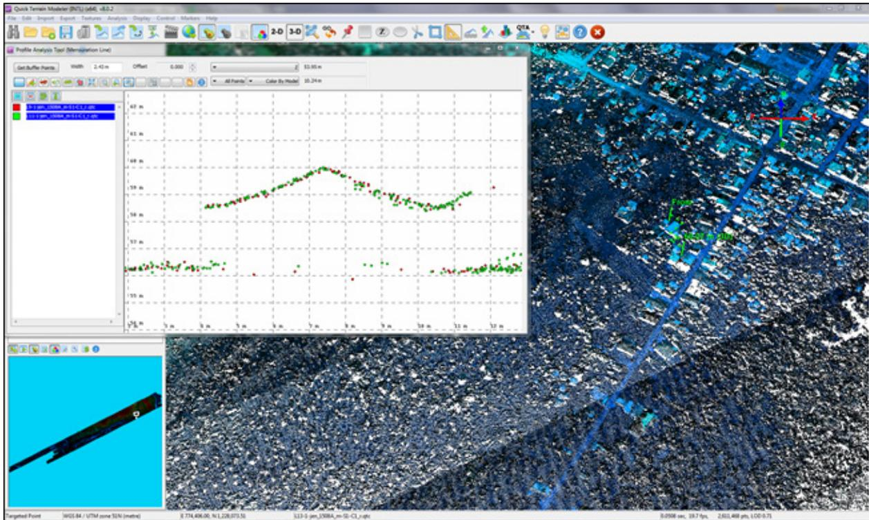
Figure 19. Quality checking for Balangiga flight 1508A using the Profile Tool of QT Modeler
