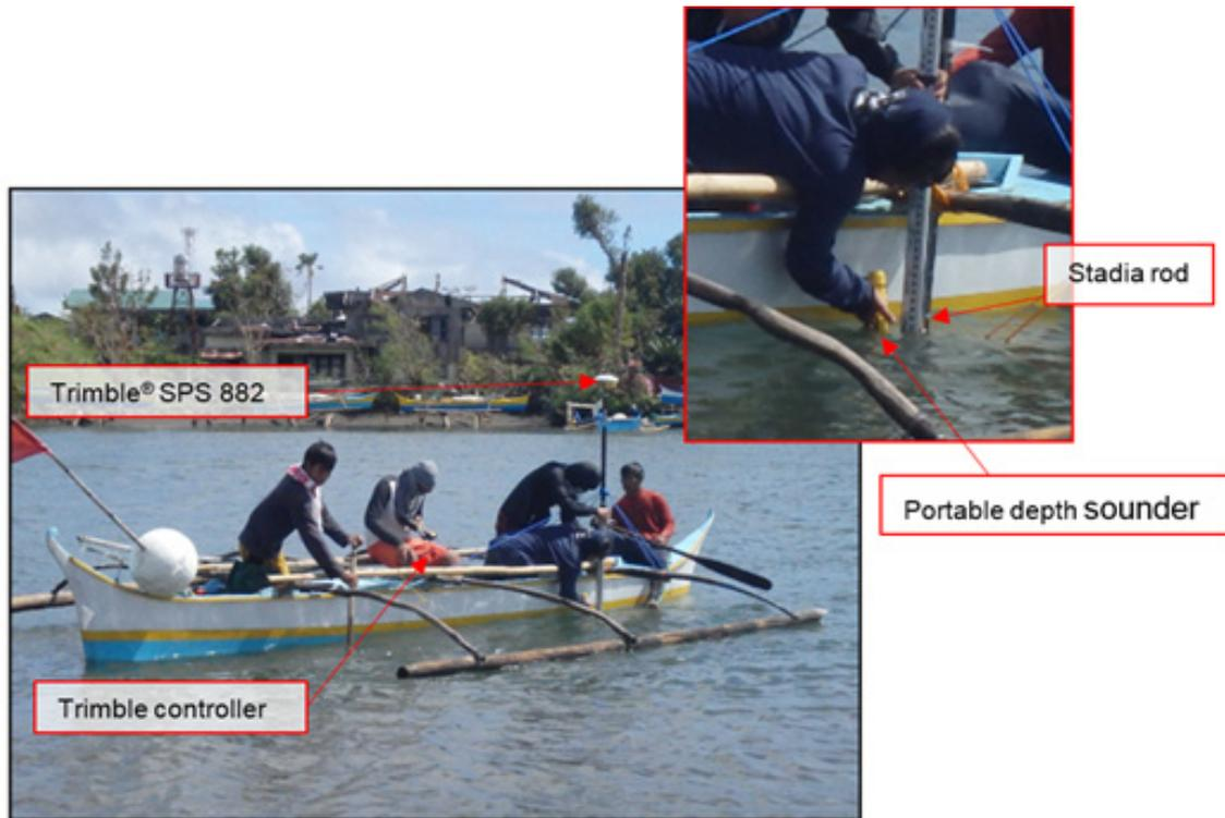
Figure 51. Manual bathymetric survey using a portable depth sounder and stadia deployment for depth-checking in the Balangiga River
