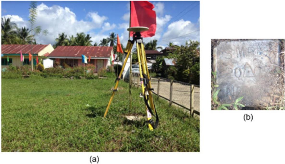
Figure 4. (a) GPS set-up over SMR-58 located inside Serum Elementary School, Barangay Serum, Basey, and (b) NAMRIA reference point SMR-58, as recovered by the field team
