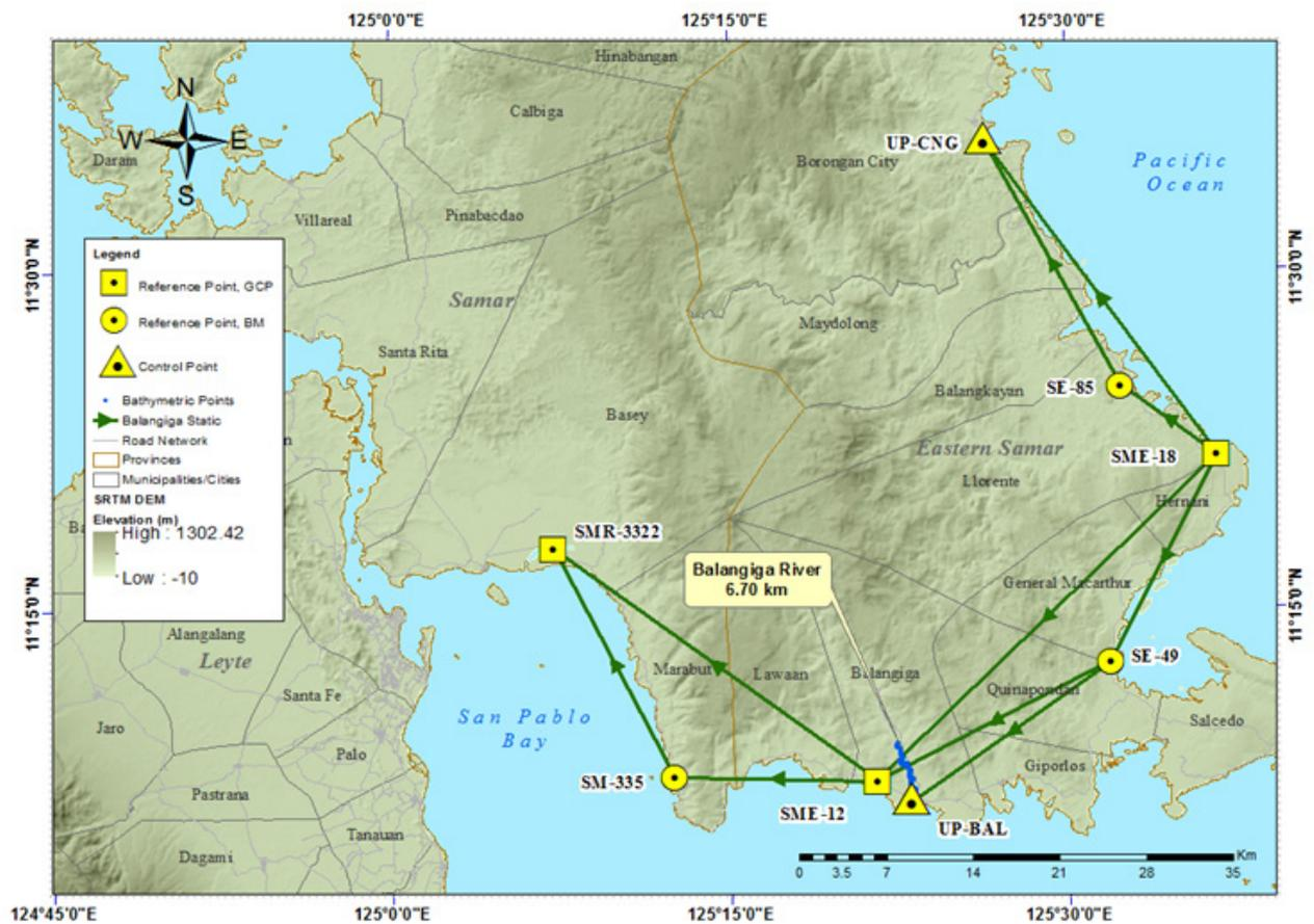
Figure 34. GNSS network of the Balangiga River field survey
