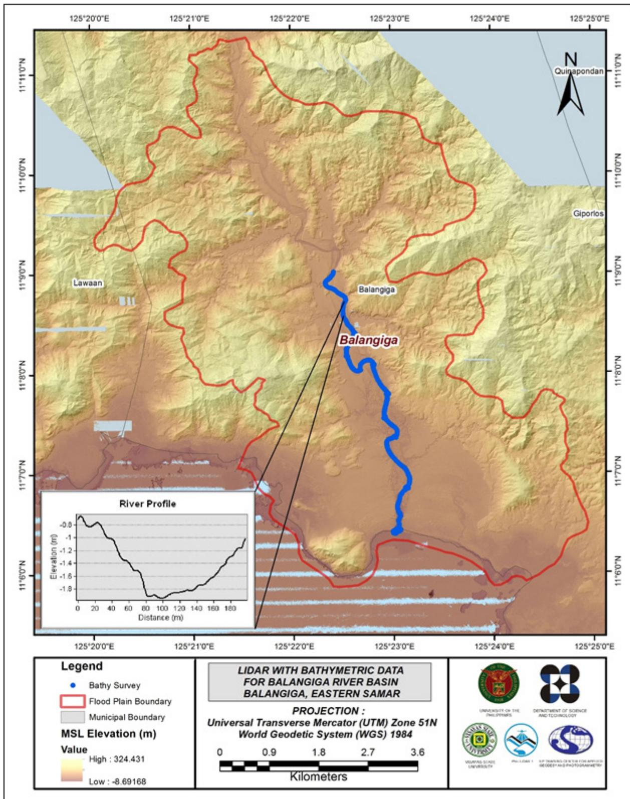
Figure 30. Map of the Balangiga Floodplain, with bathymetric survey points shown in blue
