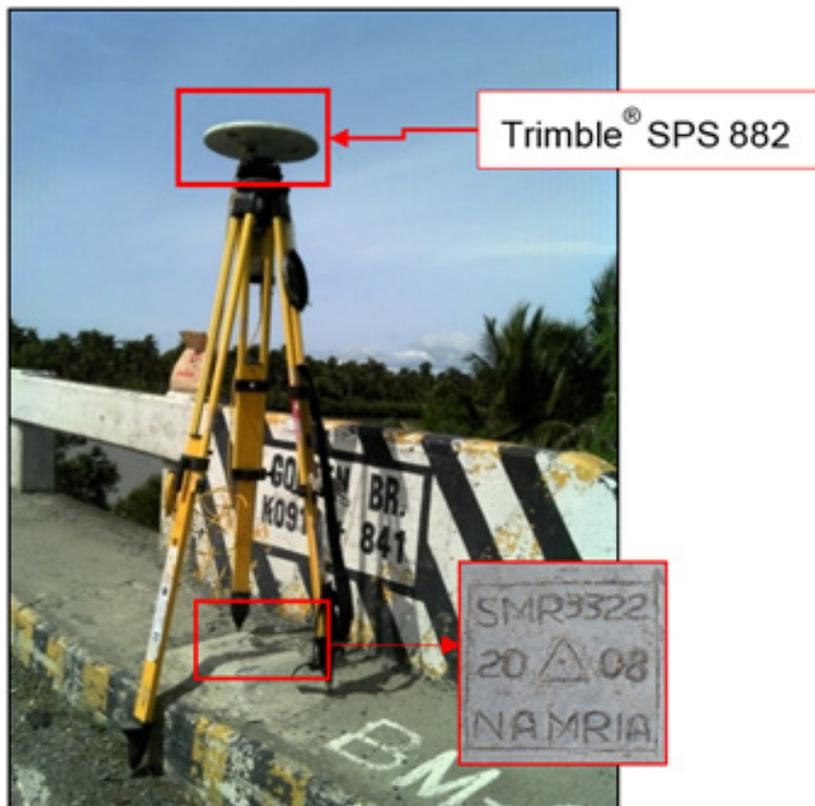
Figure 38. GNSS base occupation, Trimble® SPS 882, at SMR-3322, located at the approach of the Golden Bridge in Barangay Binongtu-an, Municipality of Basey, Samar
