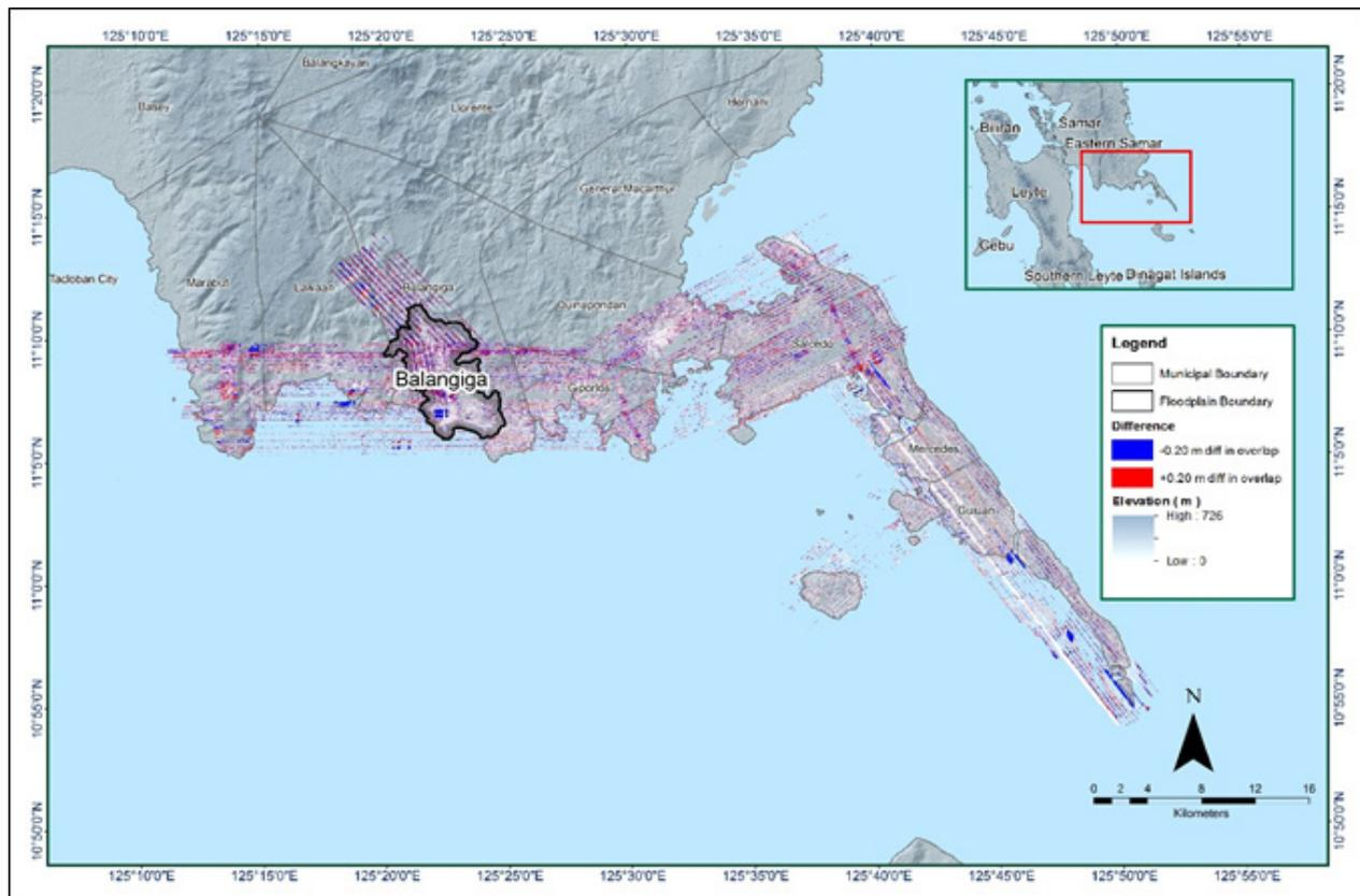
Figure 18. Elevation difference map between flight lines for the Balangiga Floodplain
