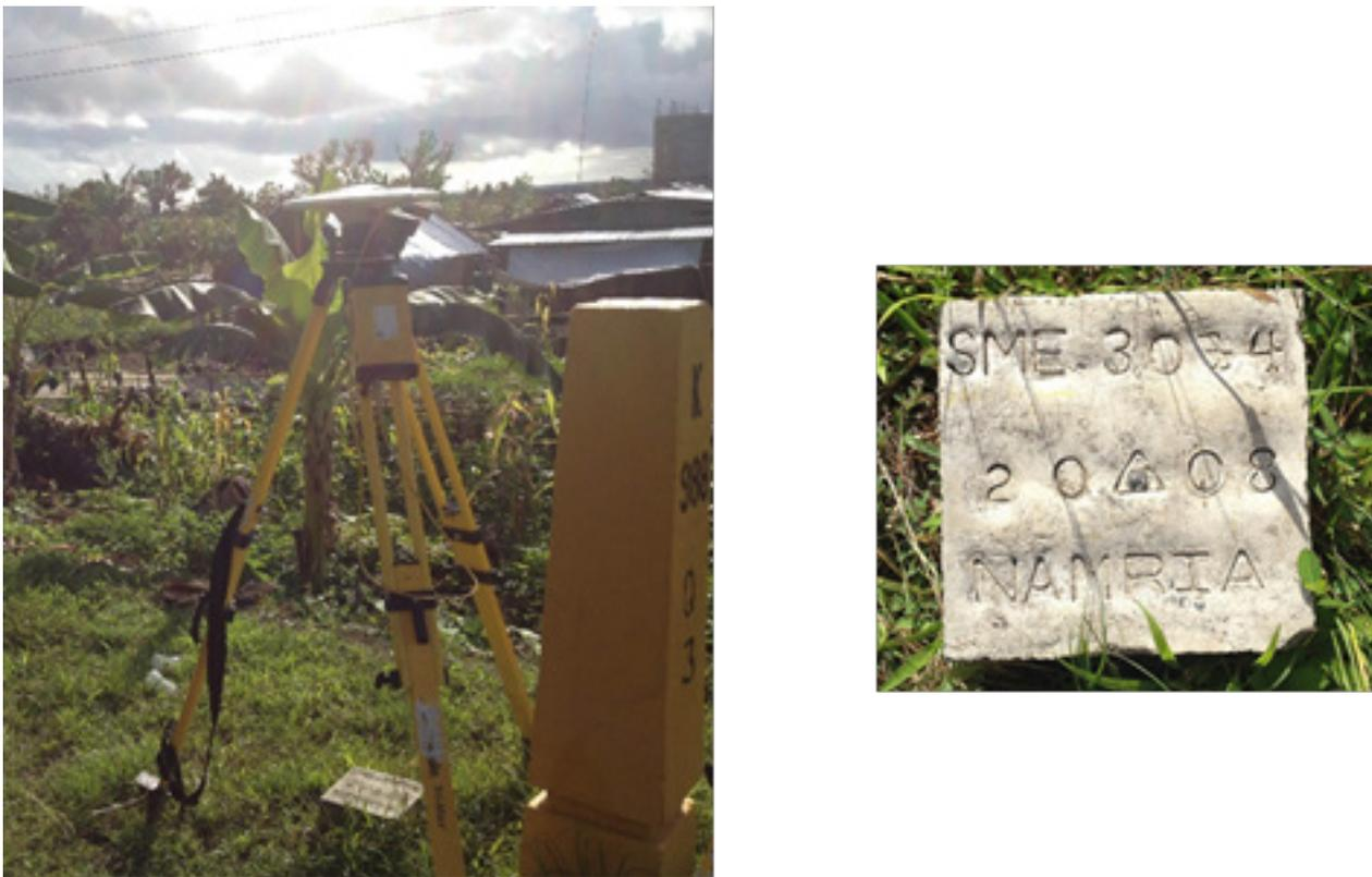
Figure 5. (a) GPS set-up over SME-3074 near KM Post No. 988 in Quinapondan, Eastern Samar court, and (b) NAMRIA reference point SME-3074, as recovered by the field team
