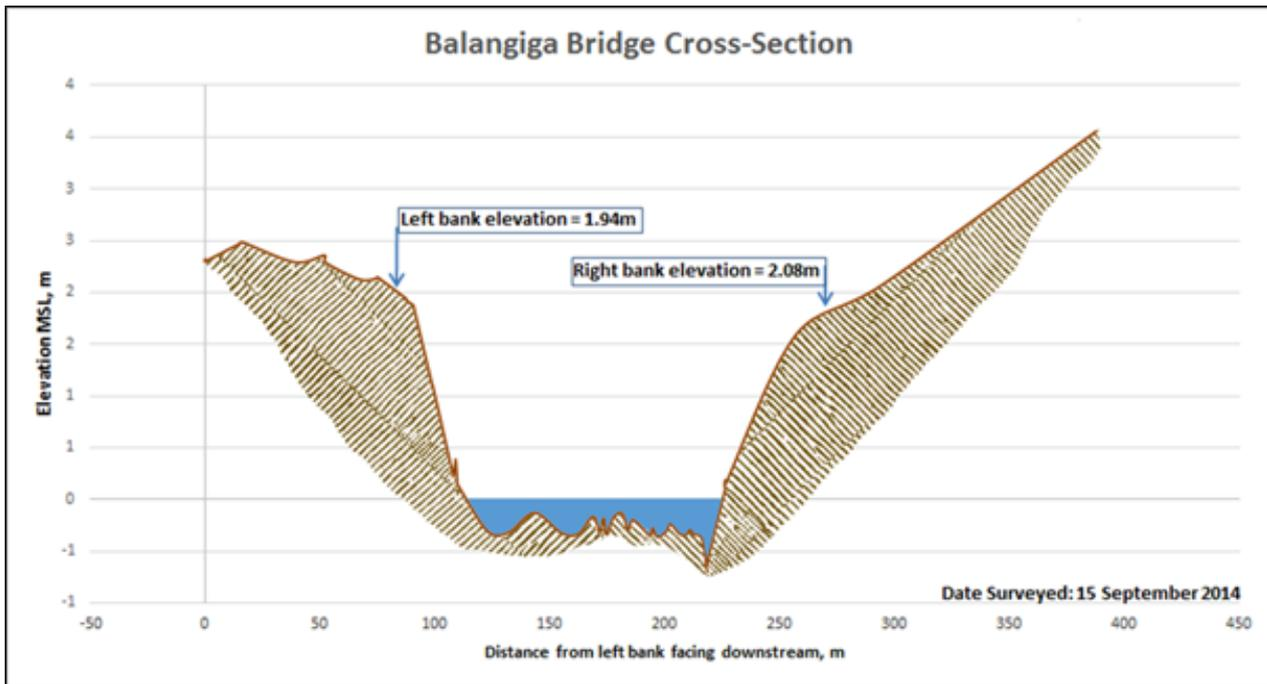
Figure 55. Cross-section plot of the Balangiga Bridge
