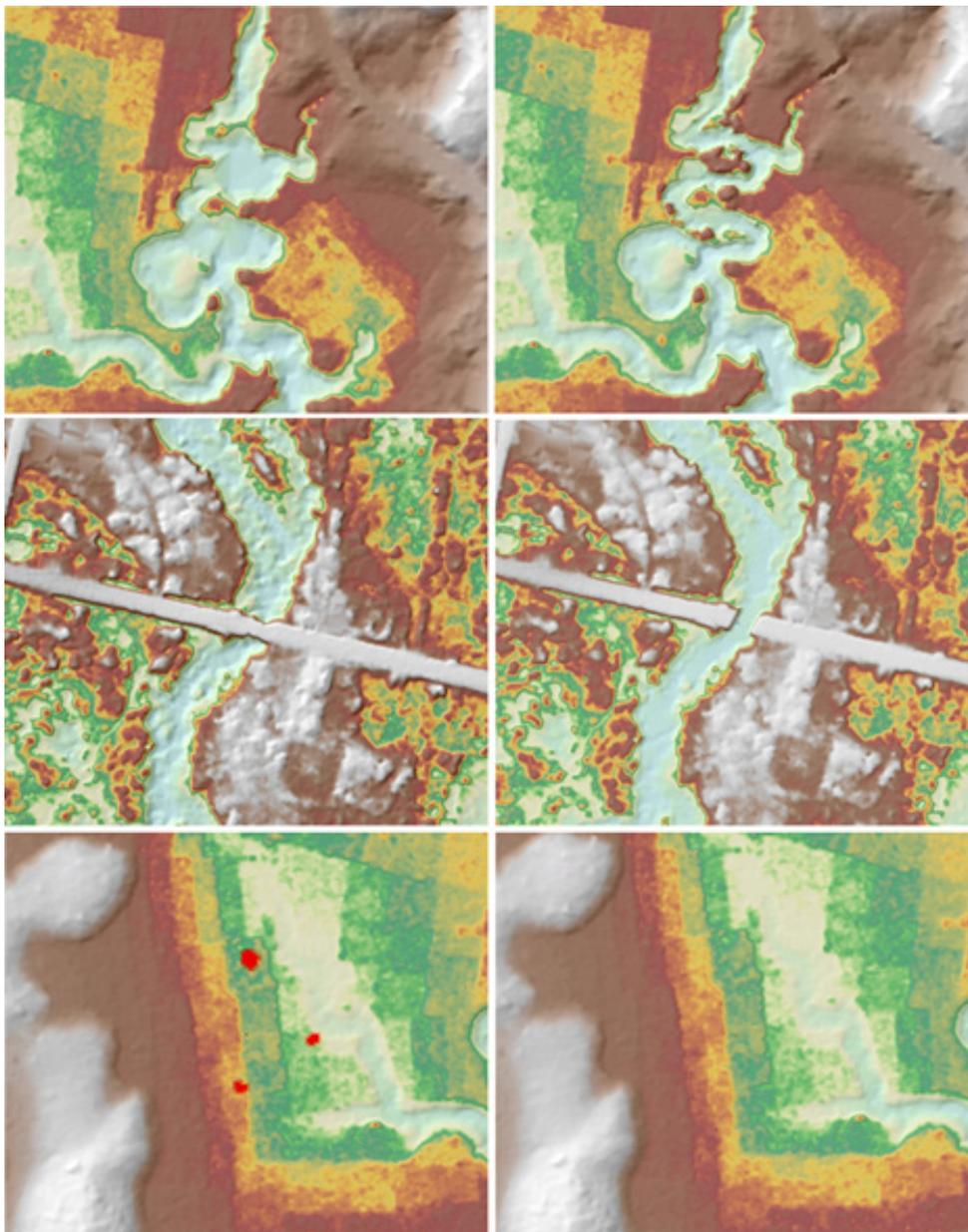
Figure 25. Portions in the DTM of Balangiga Floodplain – a river embankment (a) before and (b) after data retrieval; a bridge (c) before and (d) after manual editing; and data gaps in a paddy field (e) before and (f) after manual editing
