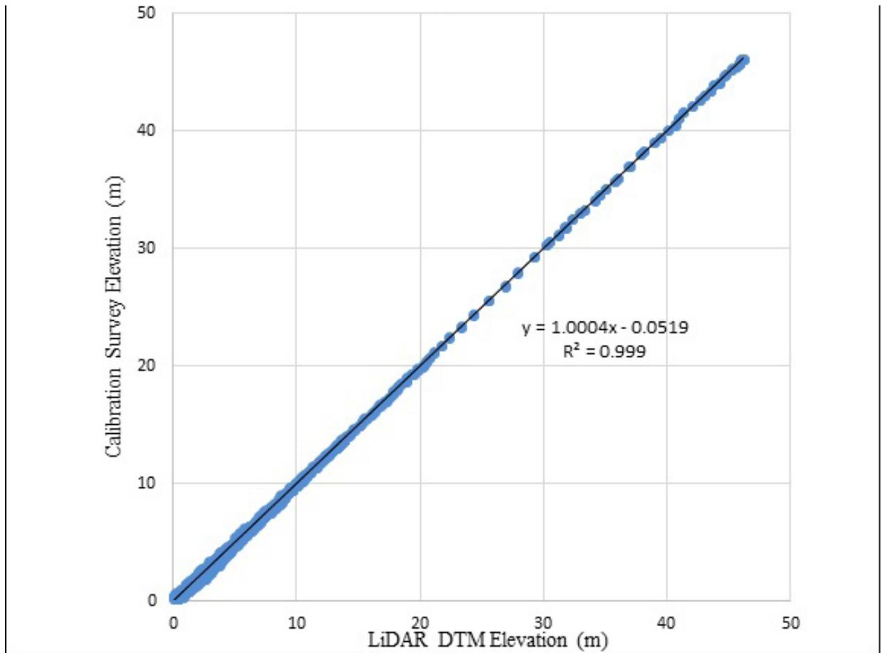
Figure 28. Correlation plot between the calibration survey points and the LiDAR data
