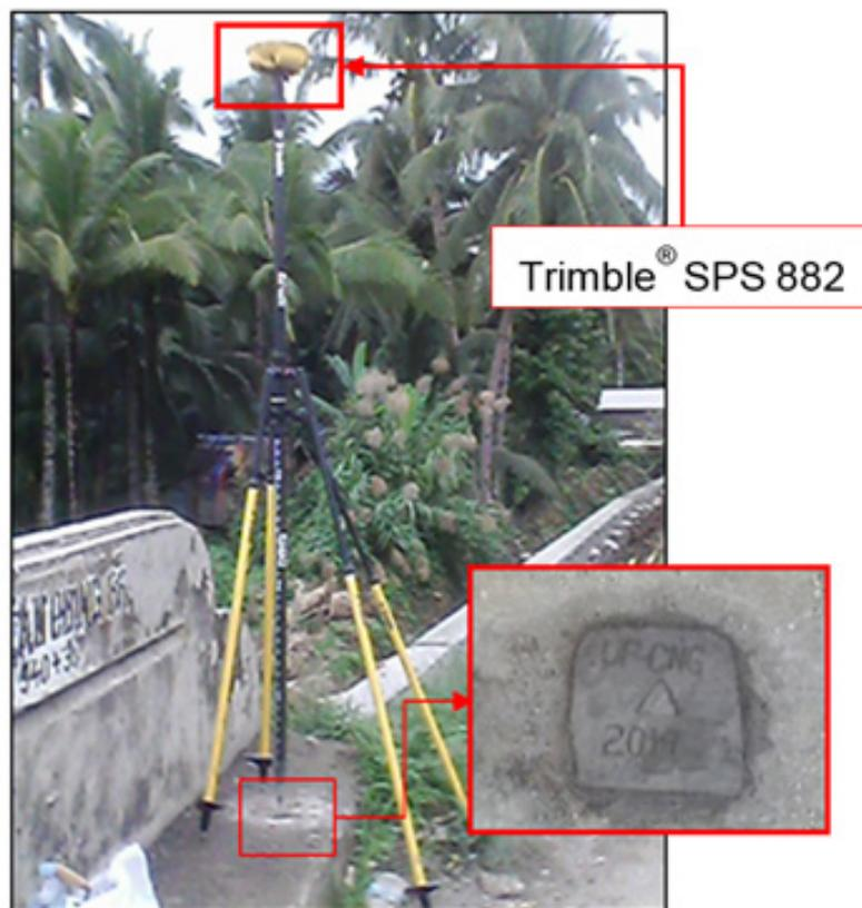
Figure 41. GNSS receiver occupation, Trimble® SPS 882, at UP-CNG, located at the approach of the Can-Obing Bridge in Barangay Can-Along, Borongan City, Eastern Samar
