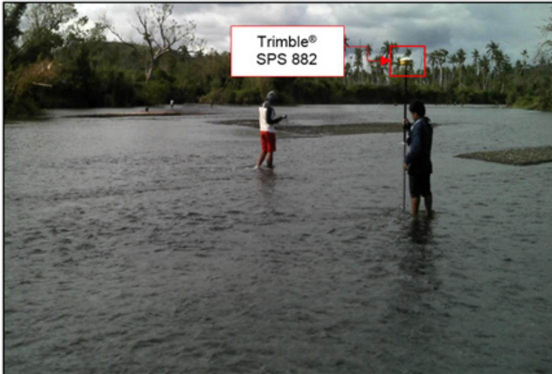
Figure 50. Actual execution of manual bathymetric survey in the Balangiga River
