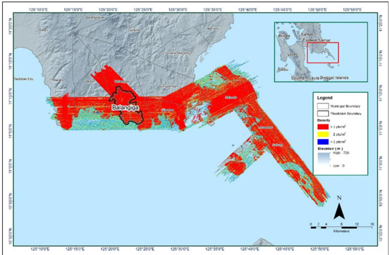
Figure 17. Pulse density map of merged LiDAR data for the Balangiga Floodplain
