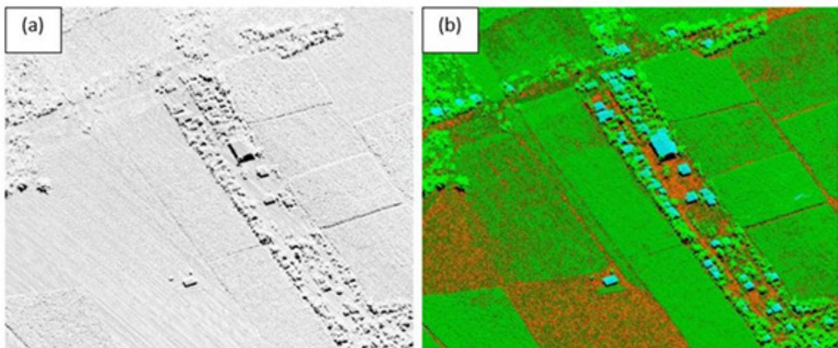
Figure 21. Point cloud (a) before and (b) after classification
