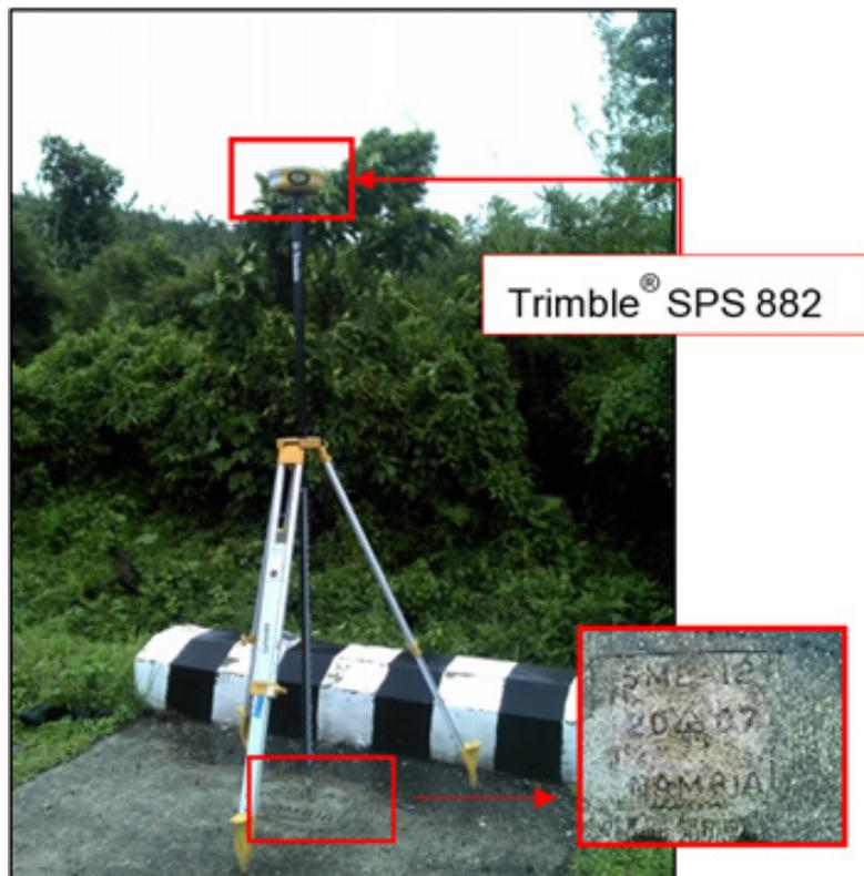
Figure 37. GNSS receiver occupation, Trimble® SPS 882, at SME-12 in Barangay San Miguel, Municipality of Balangiga, Eastern Samar
