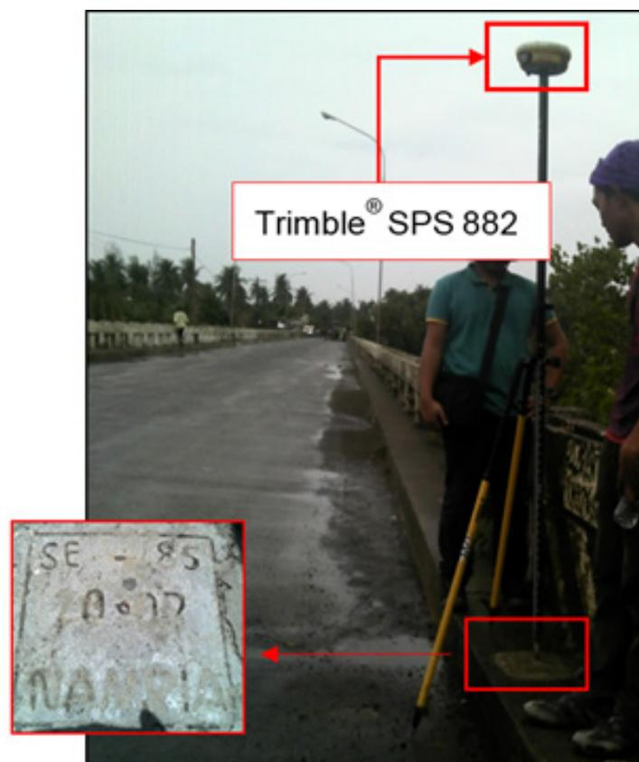
Figure 36. GNSS receiver, Trimble® SPS 882, at SE-85, located at the approach of the Llorente Bridge in Barangay 11, Municipality of Lorente, Eastern Samar
