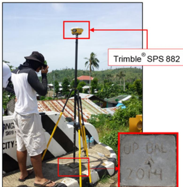
Figure 42. GNSS receiver occupation, Trimble® SPS 882, at control point UP-BAL, at the approach of the Balangiga Bridge in Barangay Poblacion V, Balangiga, Eastern Samar
