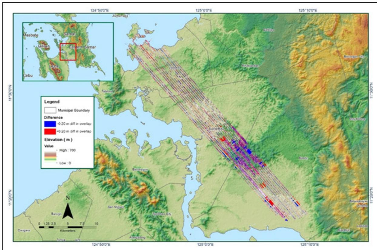
Figure A 8.14 Elevation difference between flight lines
