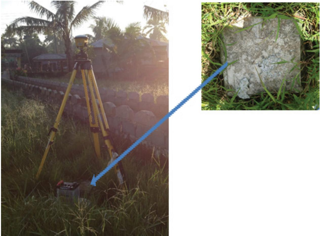
Figure 6. GPS set-up over SMR-56 at Cabacungan Elementary School in Barangay Cabacungan, Sta. Rita, Samar (a) and NAMRIA reference point SMR-56 (b) as recovered by the field team.
