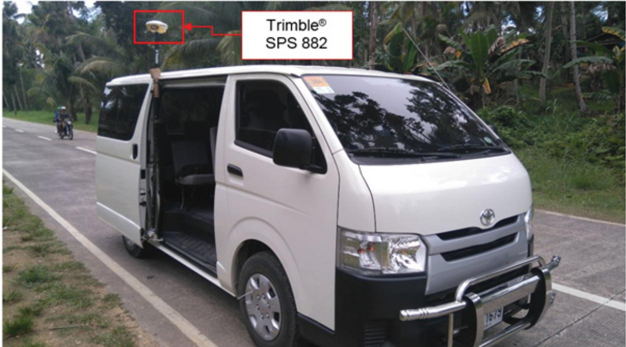
Figure 49. Validation points acquisition survey set-up along Balangiga River Basin
