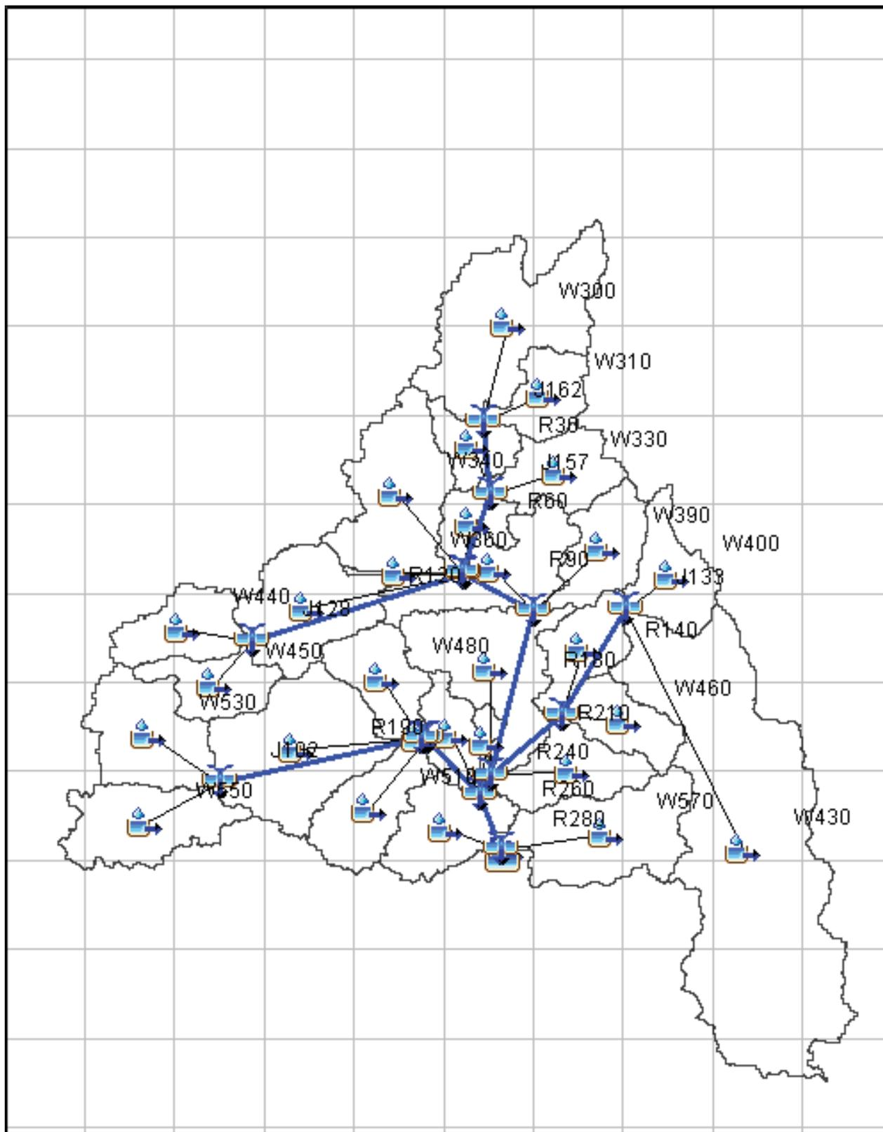
Figure 65. The Basesy river basin model generated using HEC-HMS
