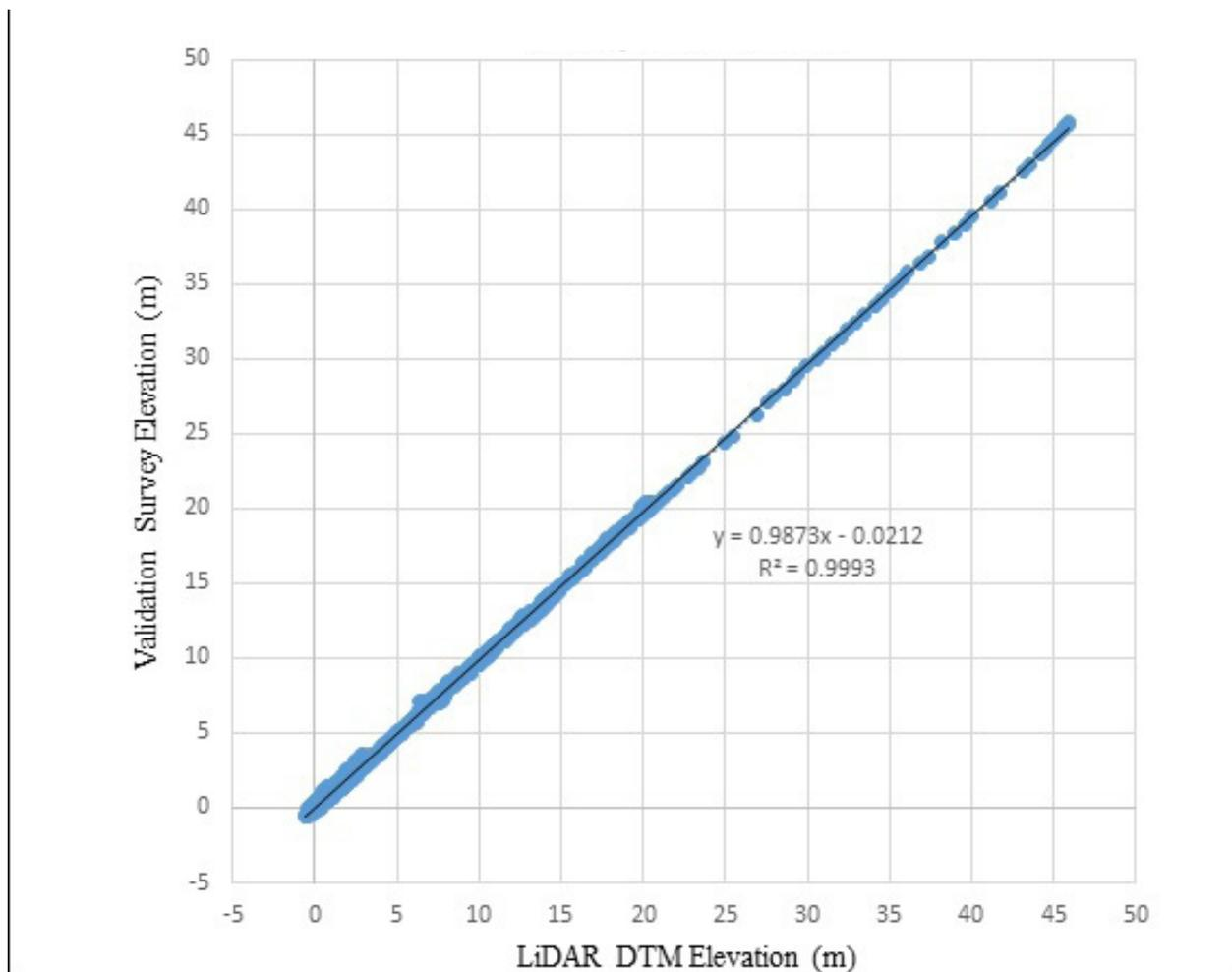
Figure 30. Correlation plot between validation survey points and LiDAR data.
