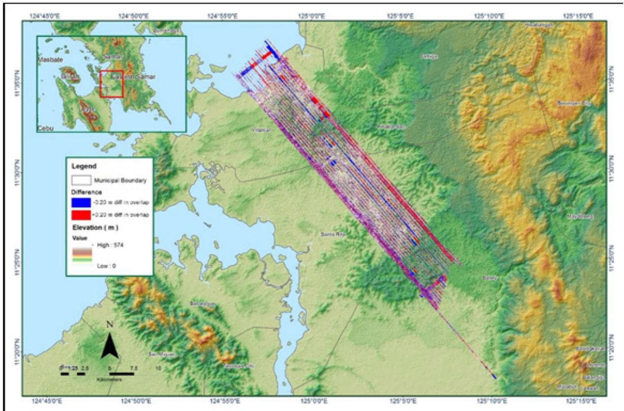
Figure A 8.7 Elevation difference between flight lines
