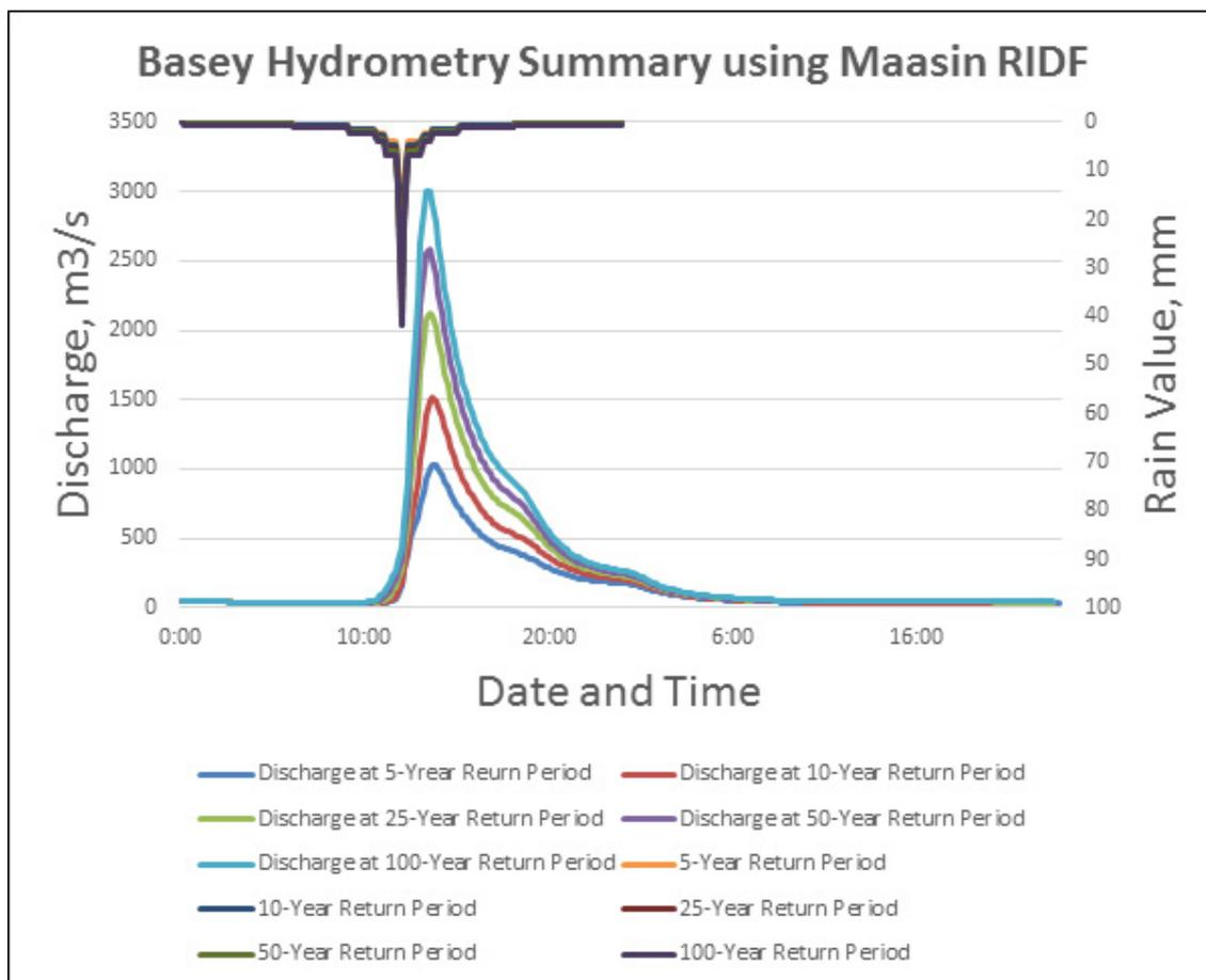
Figure 69. Outflow hydrograph at Basesy Station generated using Tacloban RIDF simulated in HEC-HMS
