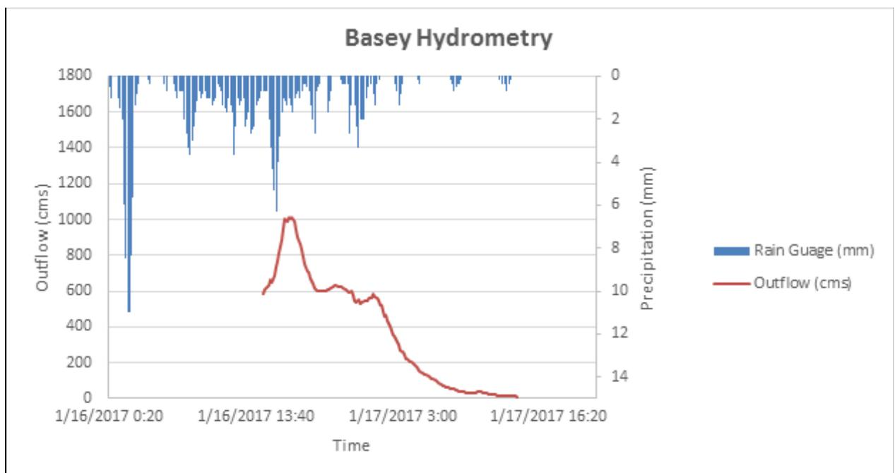
Figure 58. Rainfall and outflow data at Basey used for modeling
