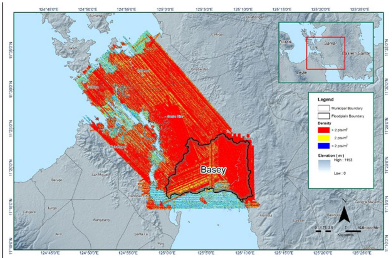
Figure 18. Pulse density map of merged LiDAR data for Basey Floodplain.
