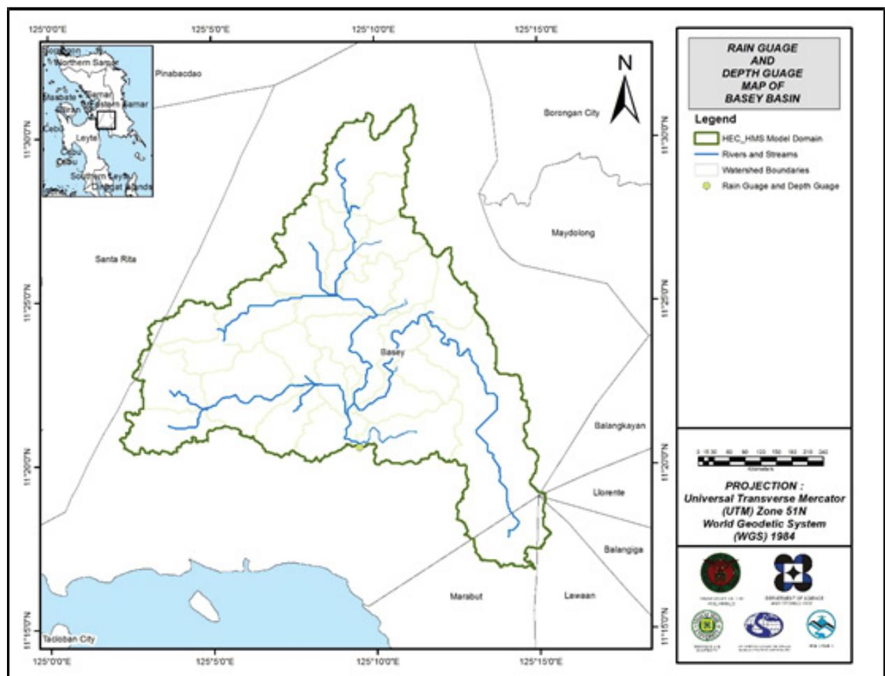
Figure 55. The location map of Basey HEC-HMS model used for calibration
