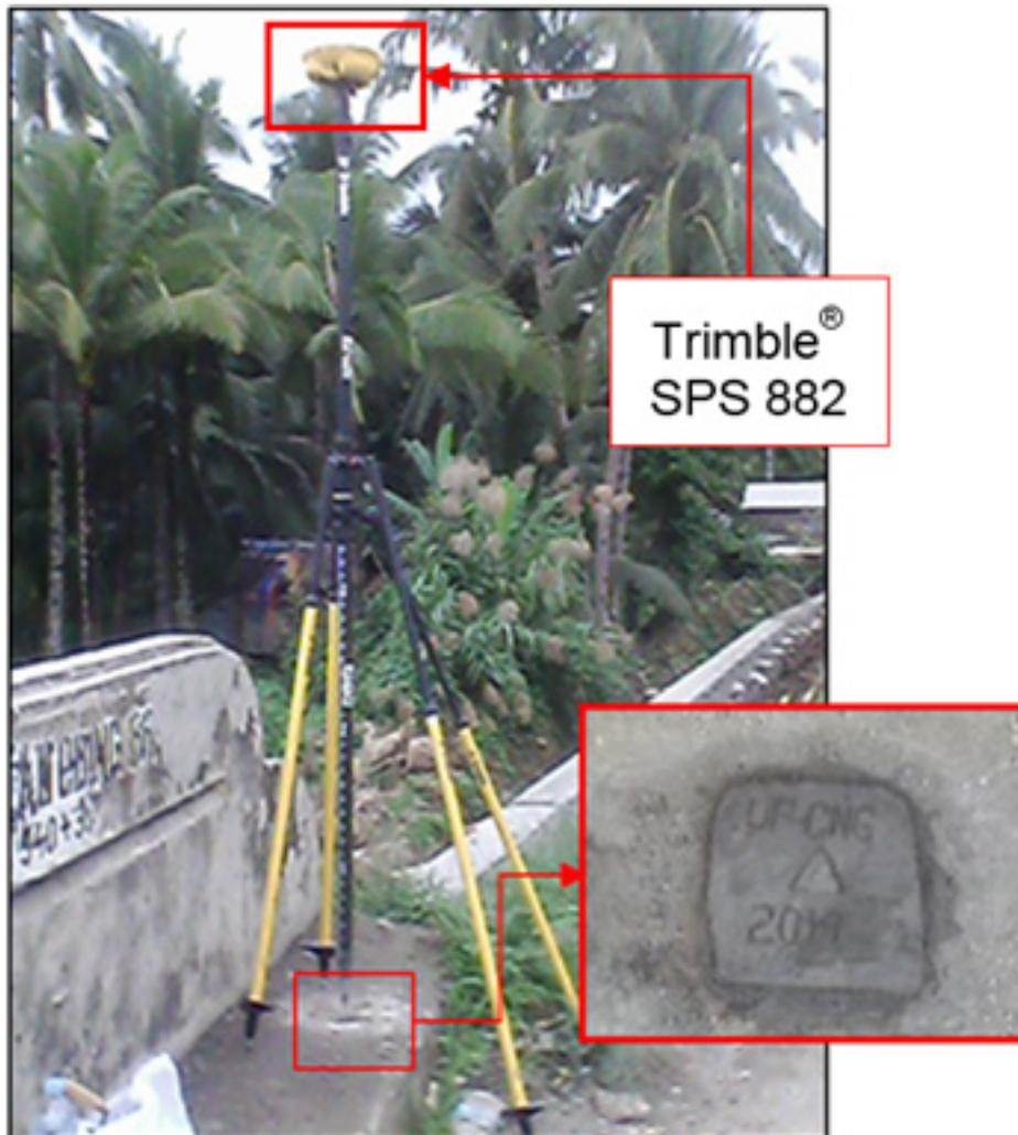
*Figure 42. GNSS receiver occupation, Trimble® SPS 882, at UP-CNG, located at the approach of Can-Obing Bridge in Brgy. Can-Abong, Borongan City, Eastern Samar*
