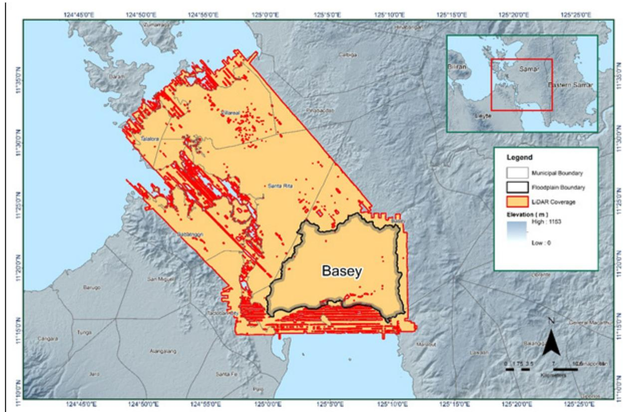
Figure 16. Boundary of the processed LiDAR data over Basey Floodplain
