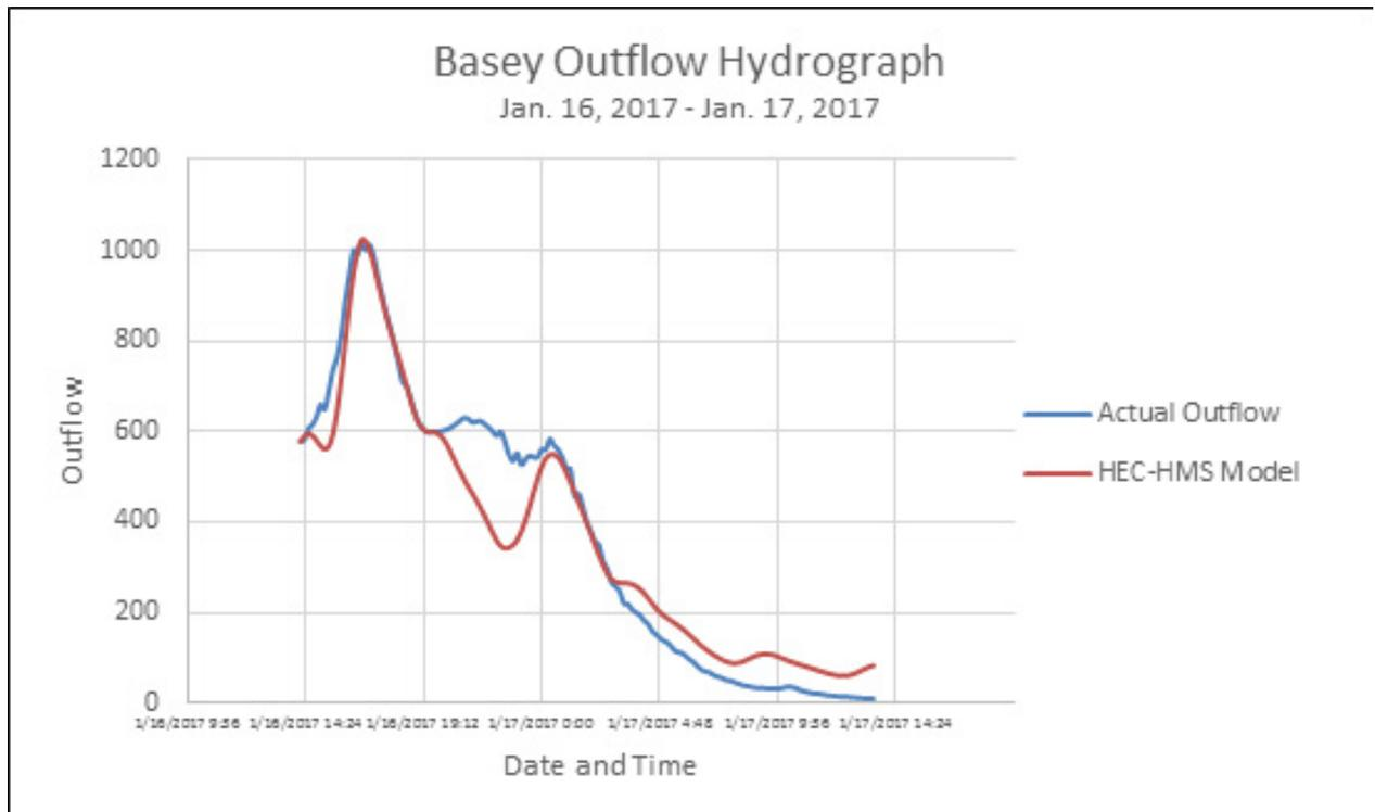
Figure 68. Outflow Hydrograph of Basey produced by the HEC-HMS model compared with observed outflow
