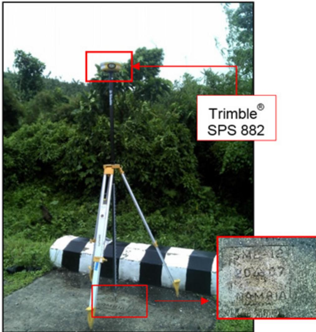
*Figure 38. GNSS receiver occupation, Trimble® SPS 882, at SME-12 in Brgy. San Miguel, Mun. of Balangiga, Eastern Samar*
