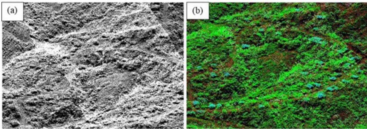
Figure 22. Point cloud before (a) and after (b) classification.
