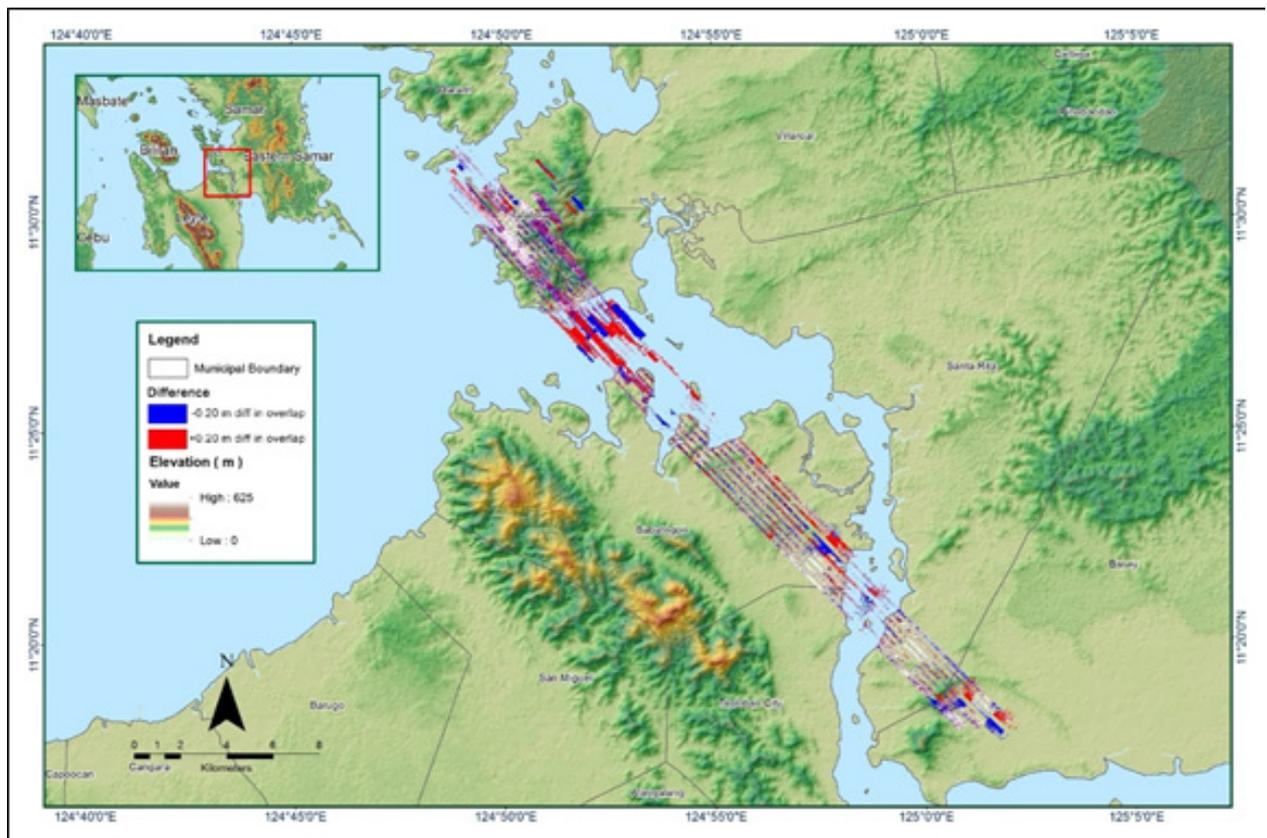
Figure A 8.35 Elevation difference between flight lines
