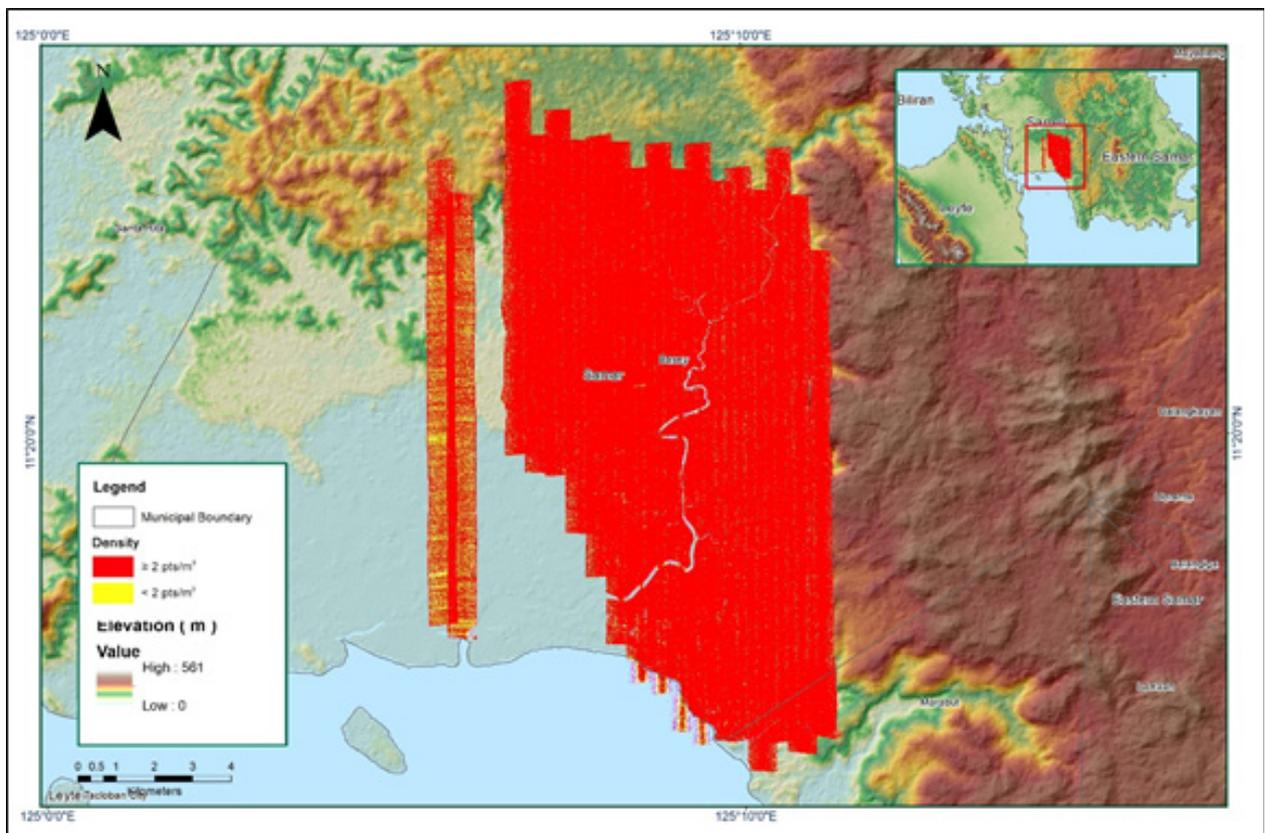
Figure A 8.60 Density map of merged LiDAR data
