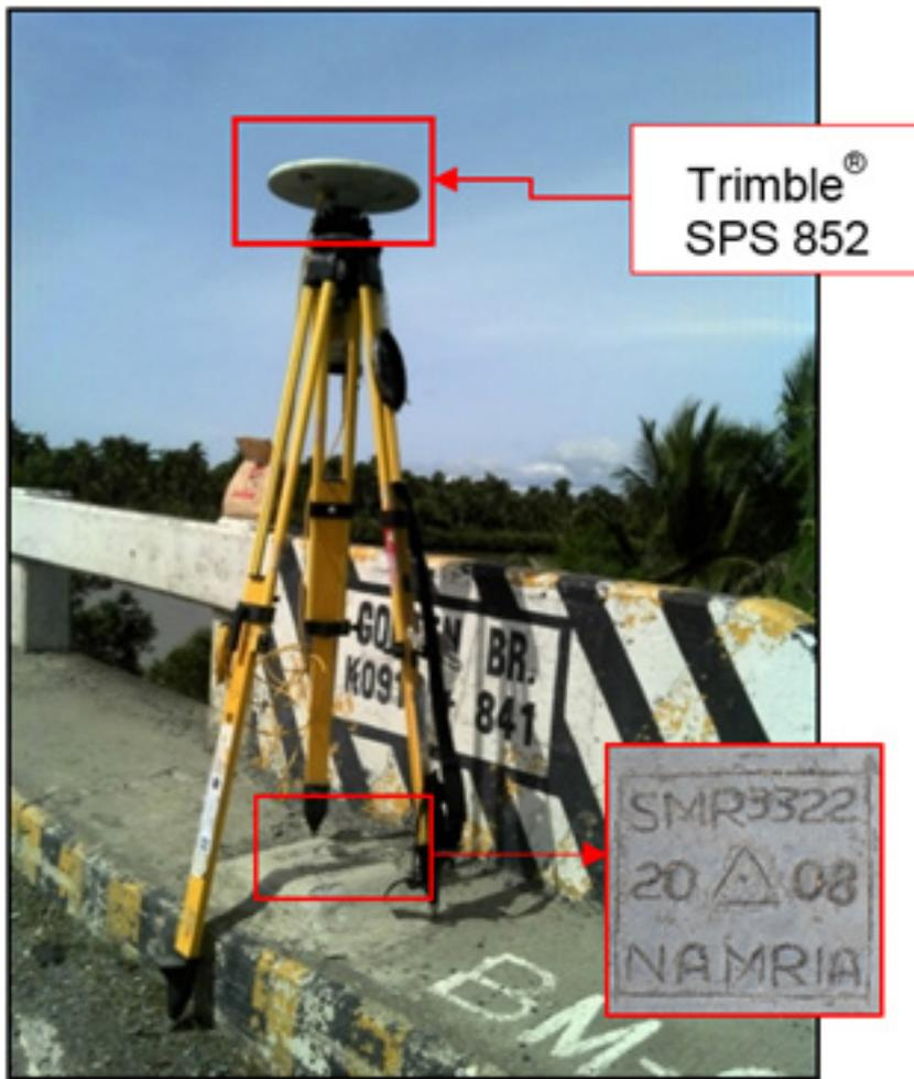
Figure 39. GNSS base occupation, Trimble® SPS 852, at SMR-3322, located at the approach of Golden Bridge in Brgy. Binongtu-an, Mun. of Basey, Samar
