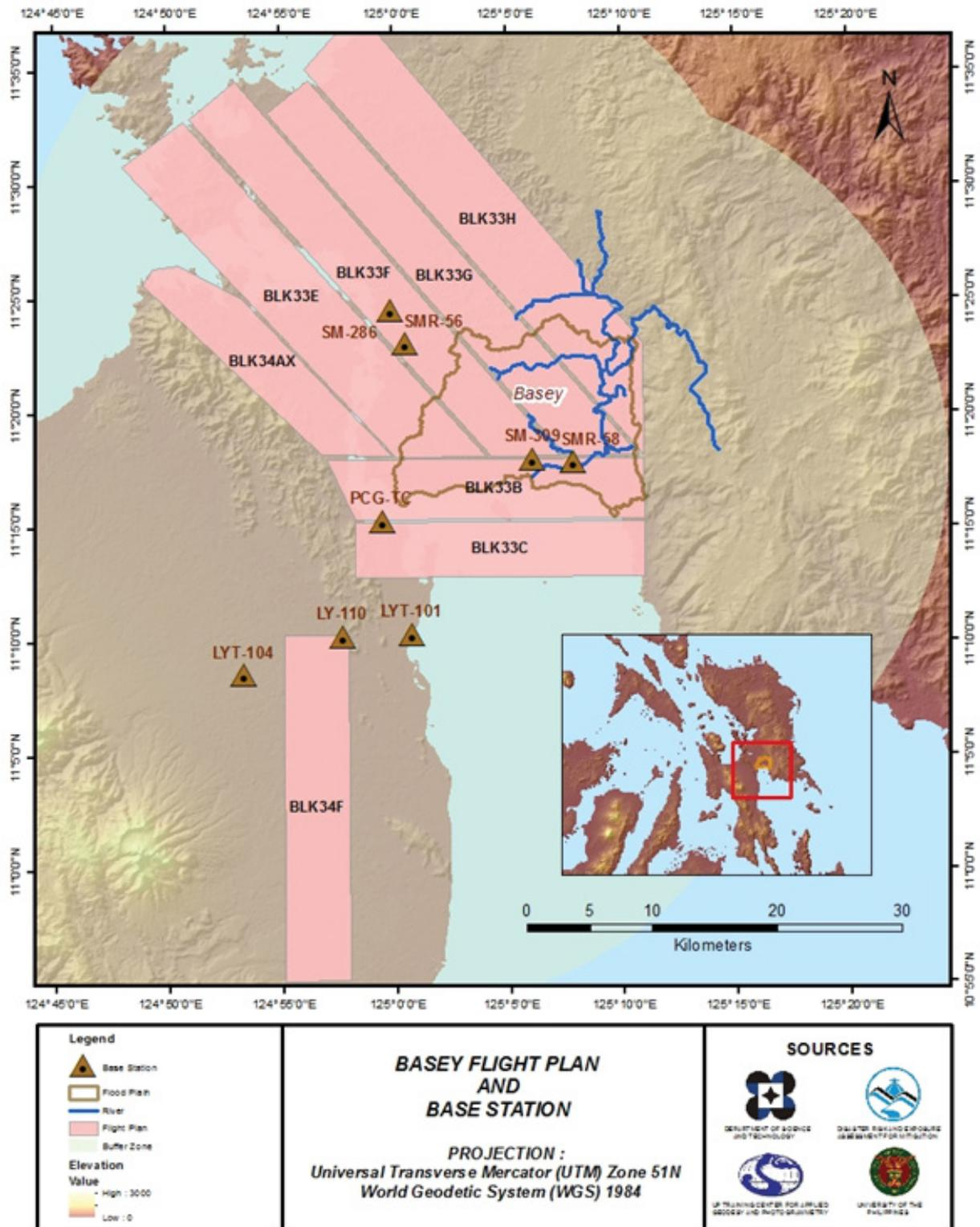
Figure 2. Flight plan and base stations used for Basey Floodplain using Aquarius LiDAR system.
