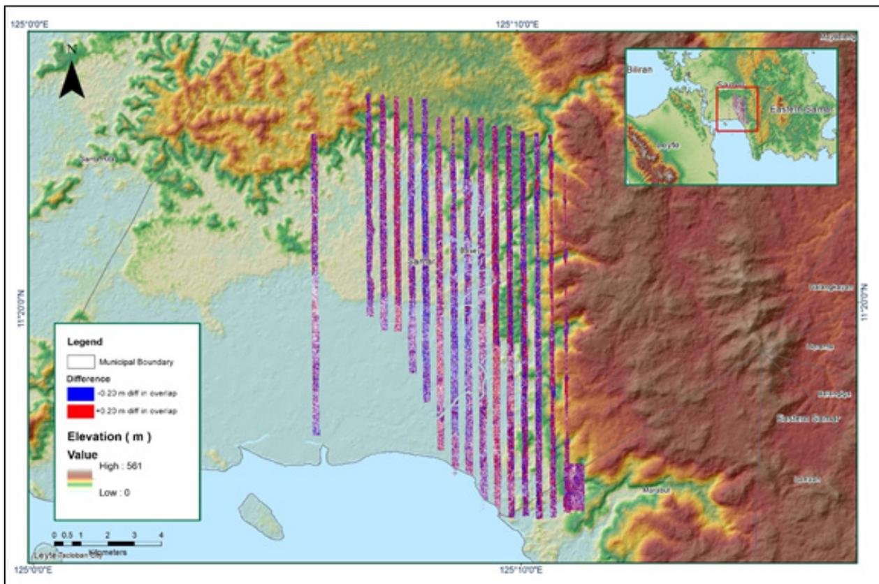
Figure A 8.61 Elevation difference between flight lines
