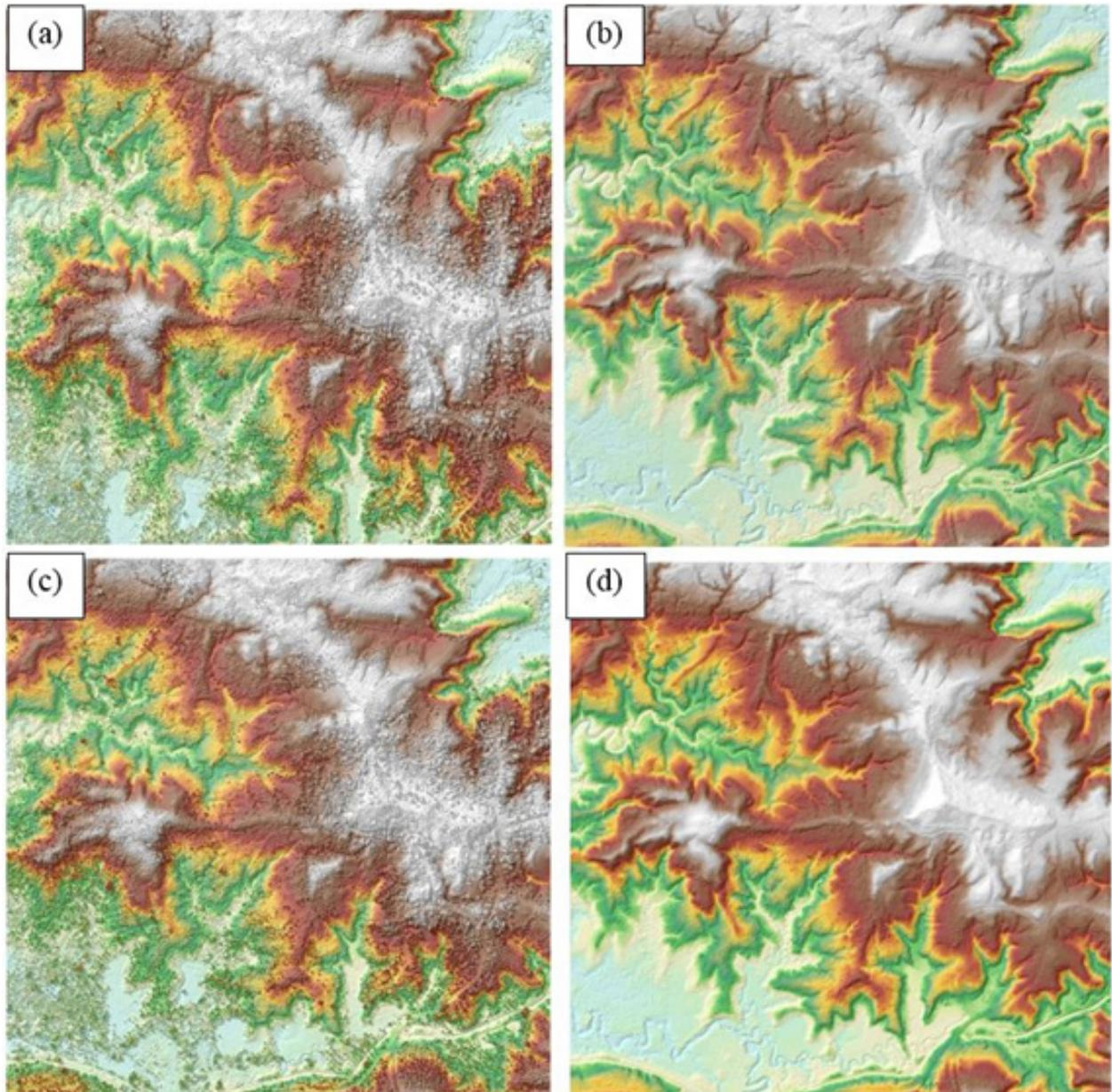
Figure 23. The production of last return DSM (a) and DTM (b), first return DSM (c) and secondary DTM (d) in some portion of Basey Floodplain.
