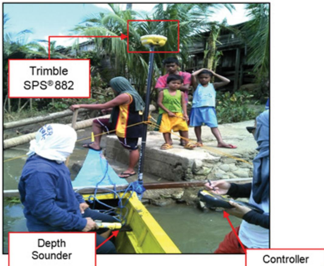
Figure 51. Setting up- Manual Bathymetry in Basey River
