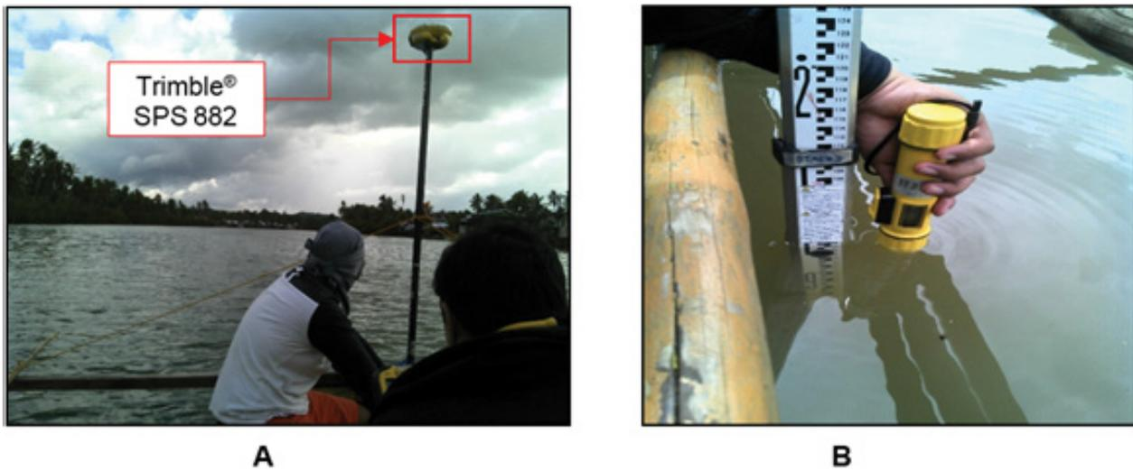
Figure 52. A) Actual Execution of Bathymetric Survey in Basey River, (B) depth checking using portable depth sounder and stadia rod
