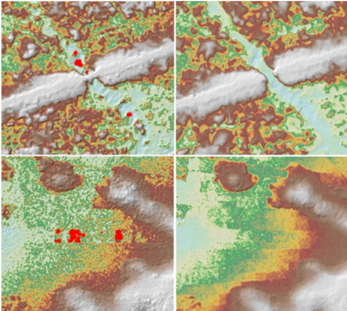
Figure 26. Portions in the DTM of Basey floodplain – a bridge and other obstructions on the river before (a) and after (b) manual editing; a flat area near the river before (c) and after (d) manual editing.
