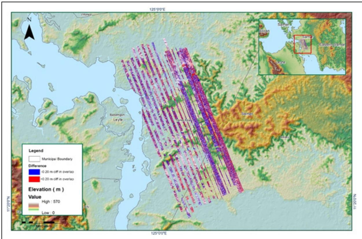
Figure A 8.42 Elevation difference between flight lines
