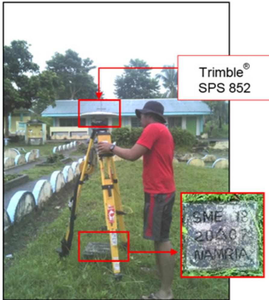
Figure 36. GNSS base receiver setup, Trimble® SPS 852 at SME-18, located inside San Jose Elem. School, Brgy. Canciledes, Municipality of Hernani, Eastern Samar
