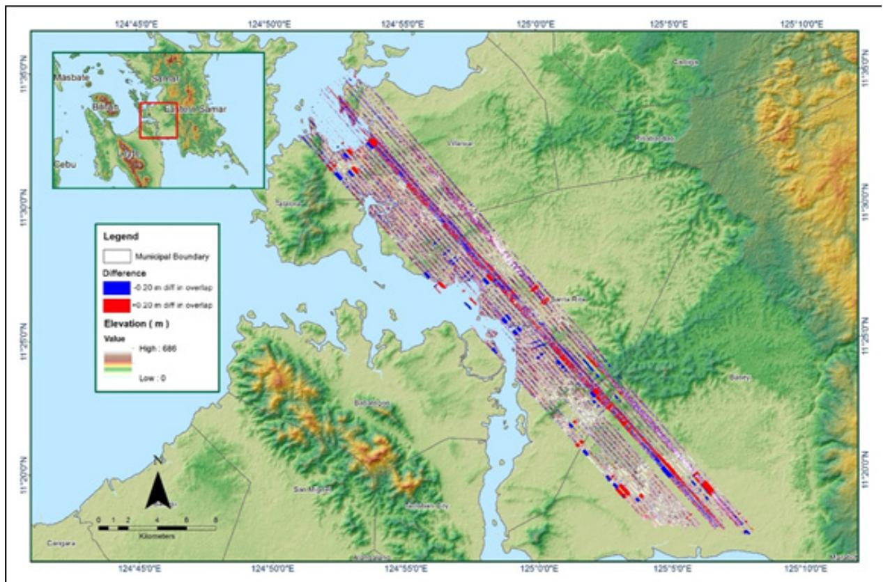
Figure A 8.21 Elevation difference between flight lines
