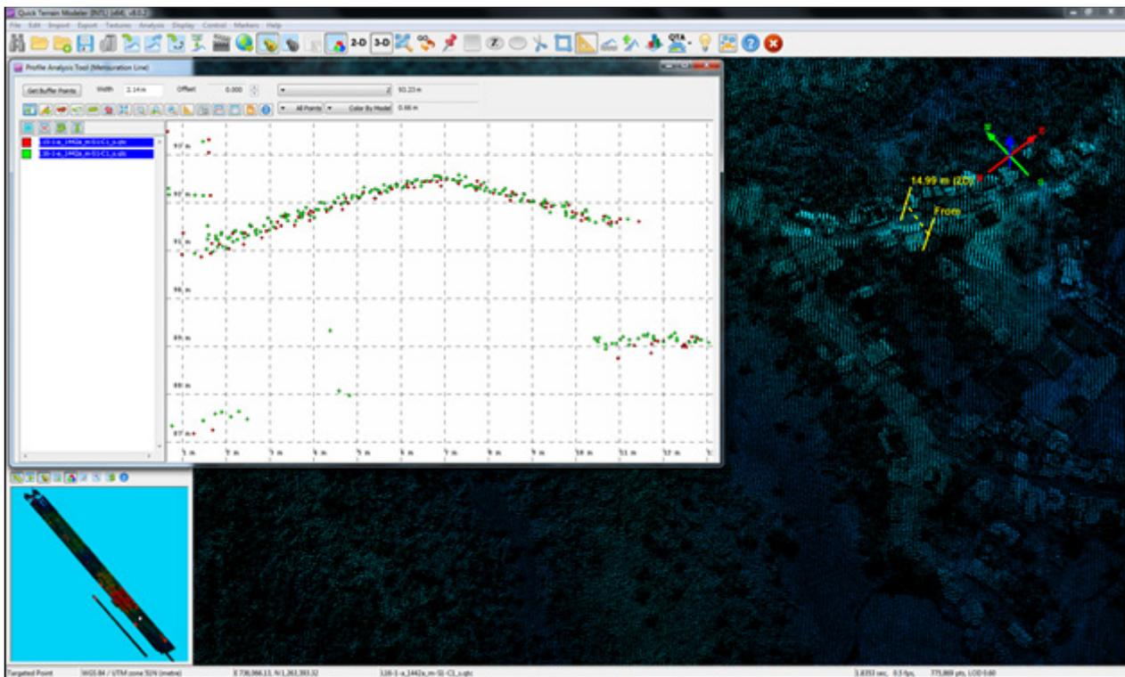
Figure 20. Quality checking for a Baisey flight 1442A using the Profile Tool of QT Modeler.
