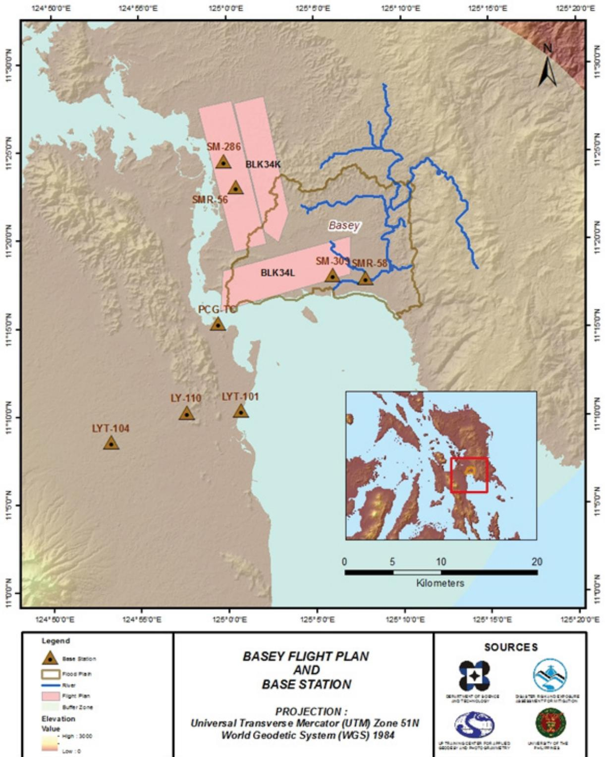
Figure 3. Flight plan and base stations used to cover Basey Floodplain using Gemini LiDAR system.
