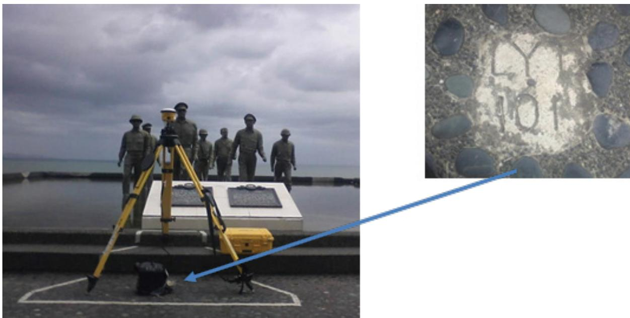
Figure 4. GPS set-up over LYT-101 within the premises of MacArthur's Landing Memorial Park, Palo, Leyte (a) and NAMRIA reference point LYT-101 (b) as recovered by the field team.
