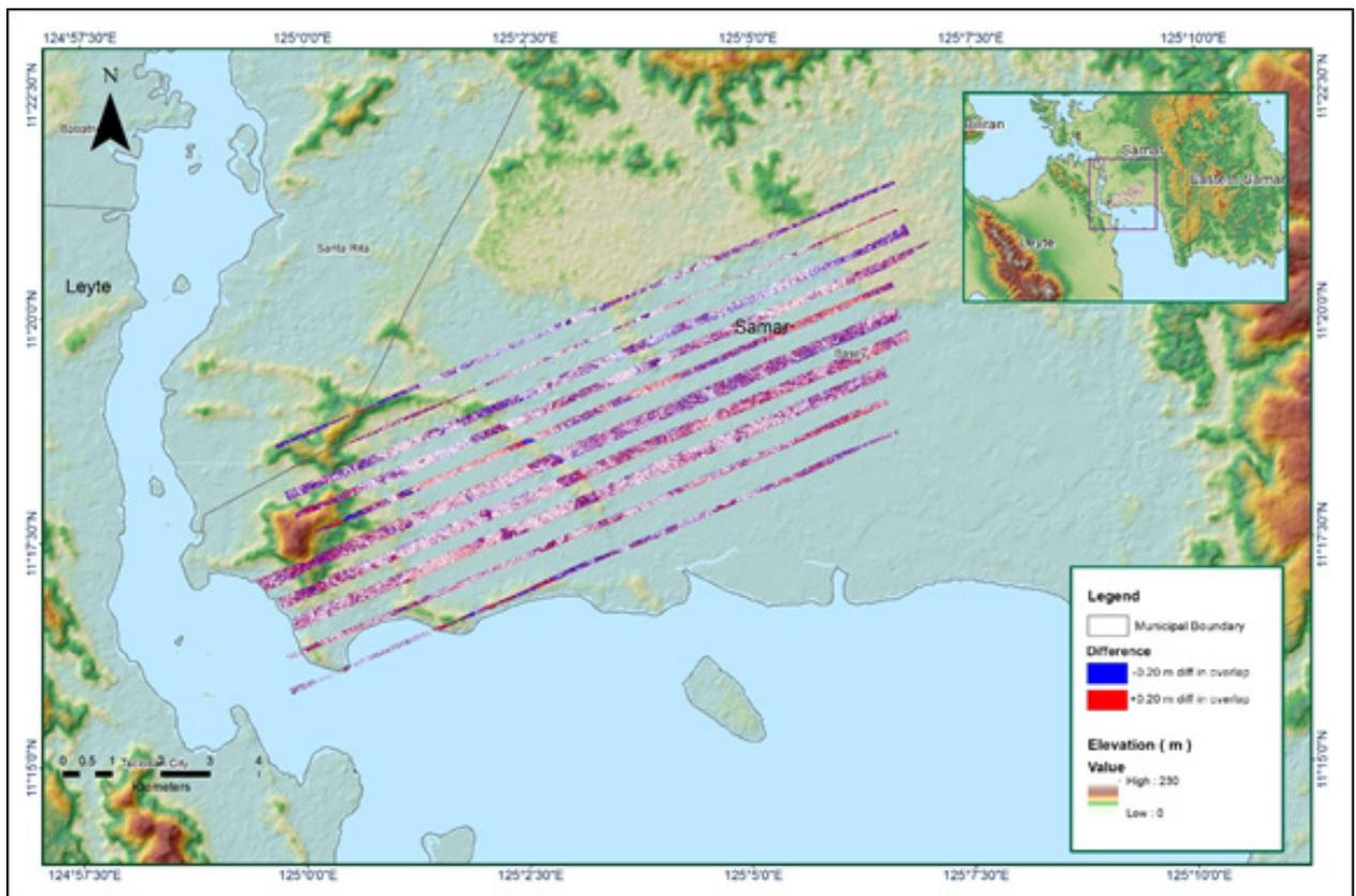
Figure A 8.49 Elevation difference between flight lines
