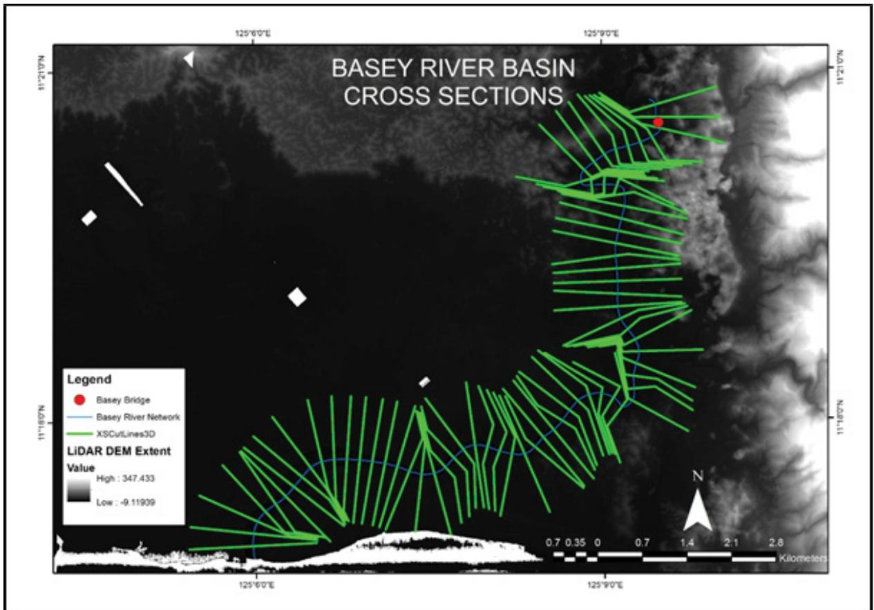
Figure 66. River cross-section of Basey River generated through Arcmap HEC GeoRAS tool
