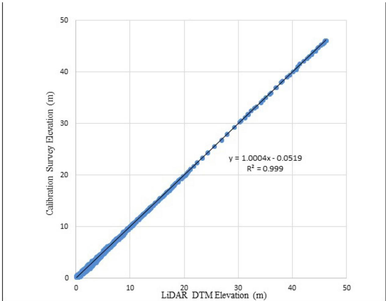
Figure 29. Correlation plot between calibration survey points and LiDAR data
