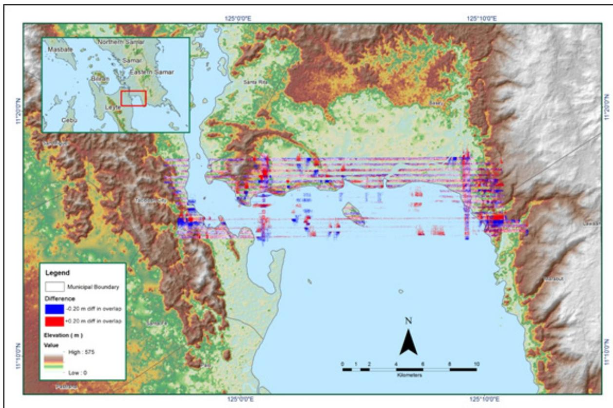
Figure A 8.81 Elevation difference between flight lines
