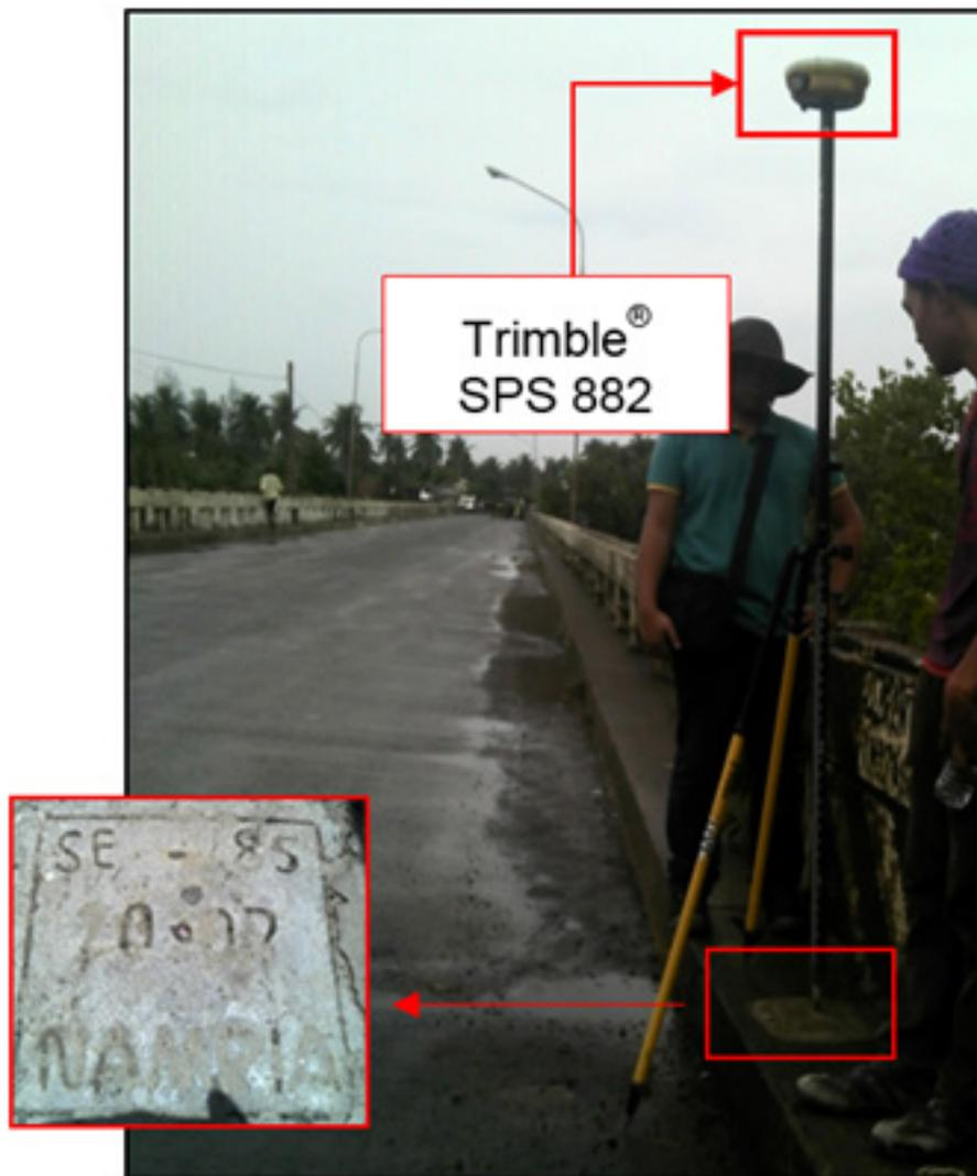
Figure 37. GNSS receiver, Trimble® SPS 882, at SE-85, located at the approach of Llorente Bridge in Bry. 11, Mun. of Llorente, Eastern Samar
