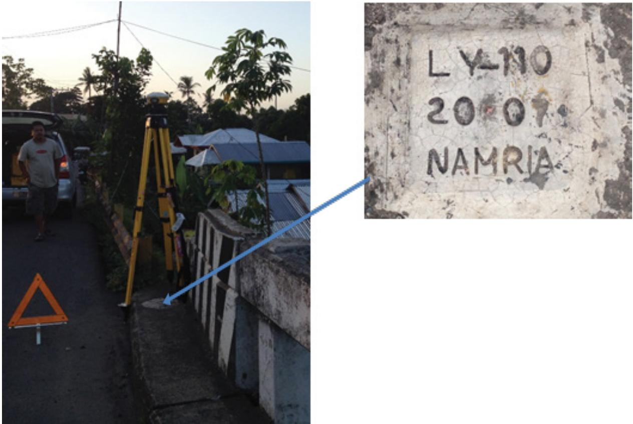
Figure 8. GPS set-up over LY-110 located along Palo-Pastrana Road, Pastrana, Leyte (a) and NAMRIA reference point LY-110 (b) as recovered by the field team.
