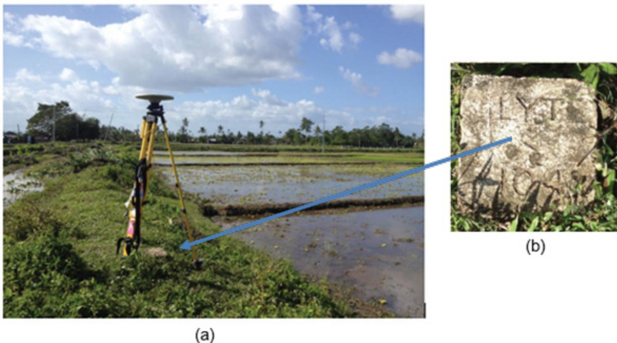
Figure 5. GPS set-up over LYT-104 located and re-established along rice paddy trail, approximately 90 meters from the centerline, east side of Pastrana-Santa Fe Road, District IV, Pastrana, Leyte (a) and NAMRIA reference point LYT-104 (b) as recovered by the field team
