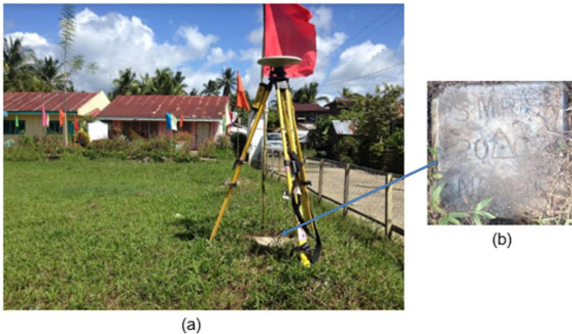
Figure 7. GPS set-up over SMR-58 located inside Serum Elementary School, Brgy. Serum, Basey (a) and NAMRIA reference point SMR-58 (b) as recovered by the field team.
