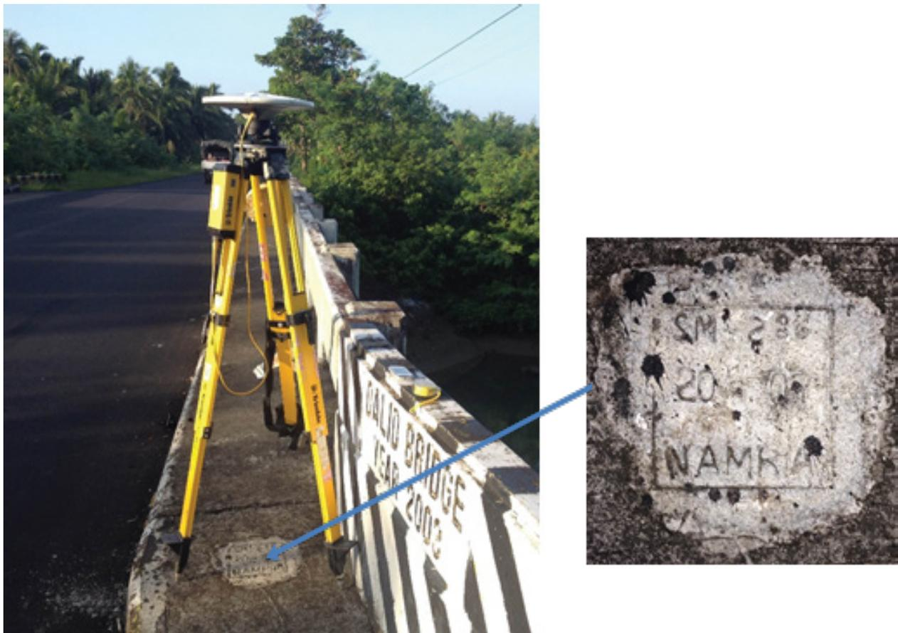
Figure 9. GPS set-up over SM-286 located at Dalid bridge along national highway in Brgy. San Pascual, Sta. Rita, Samar (a) and NAMRIA reference point SM-286 (a) as recovered by the field team.
