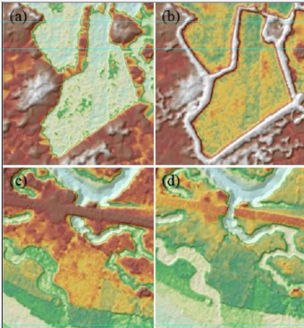
Figure 24. Portions in the DTM of Cadac-an Floodplain – a fishpond embankment before (a) and after (b) data retrieval and a bridge before (c) and after (d) manual editing
