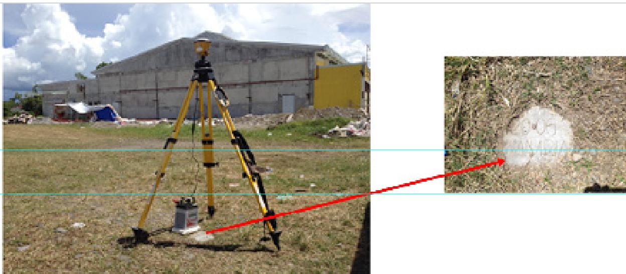
Figure 3. GPS set-up over LYT-93 as recovered within the premises of Abuyog Municipal Hall, Brgy. Sto. Abuyog, Leyte (a) and NAMRIA reference point LYT-93 (b) as recovered by the field team
