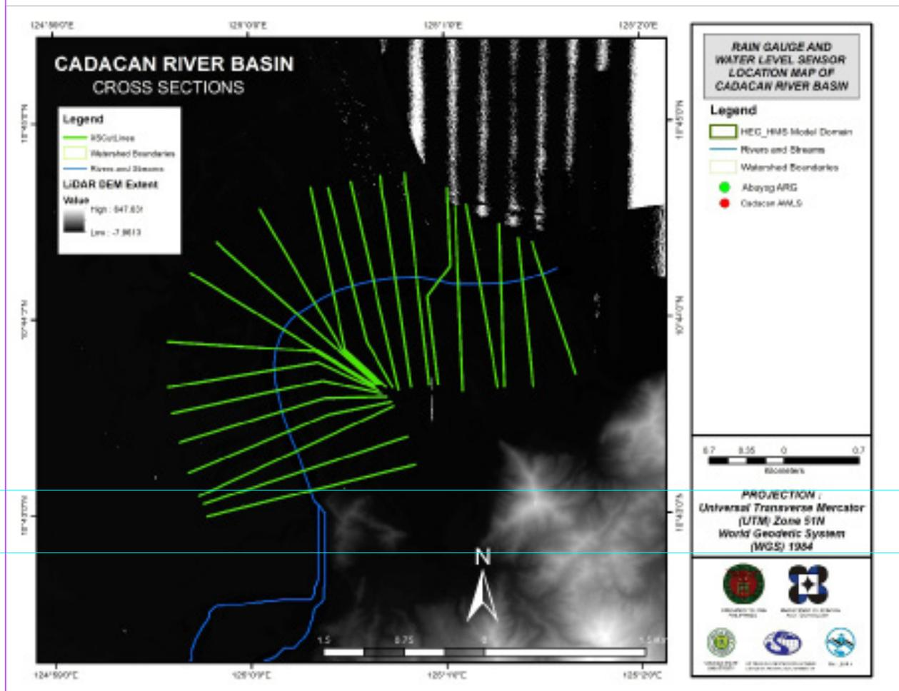
Figure 61. River cross-section of Cadac River generated through Arcmap HEC GeoRAS tool
