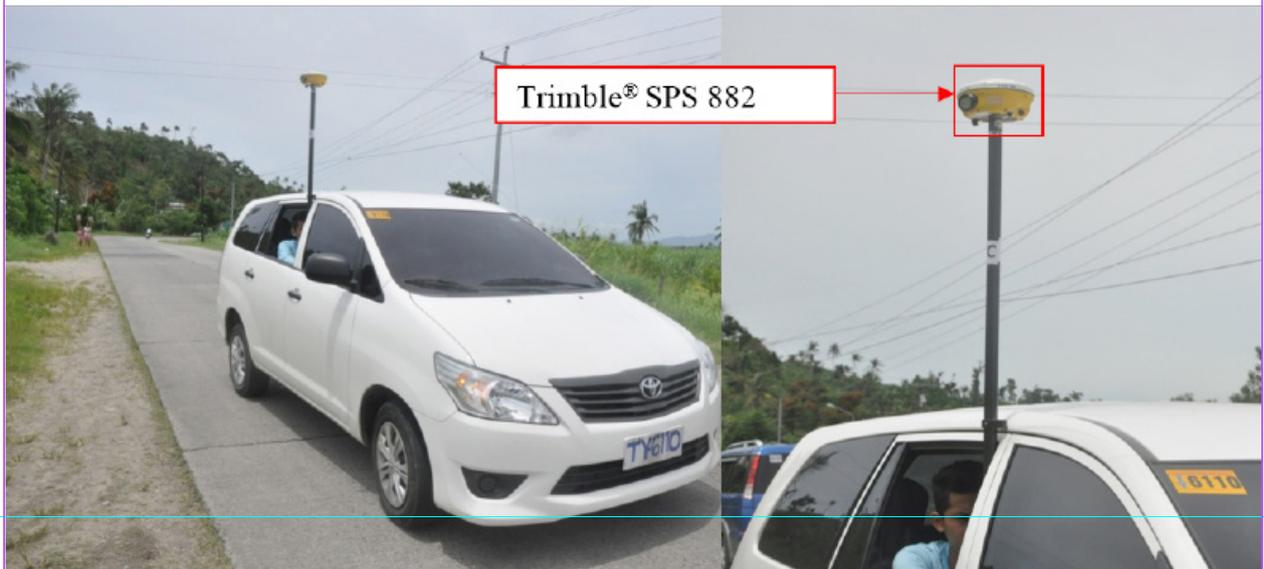
Figure 43. Validation points acquisition survey using Trimble® SPS 882 in Leyte
