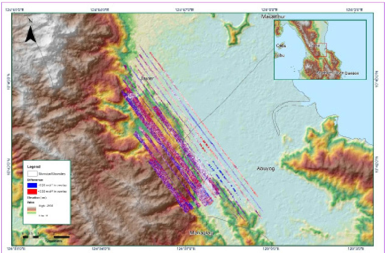
Figure 1.3.7. Elevation difference between flight lines
