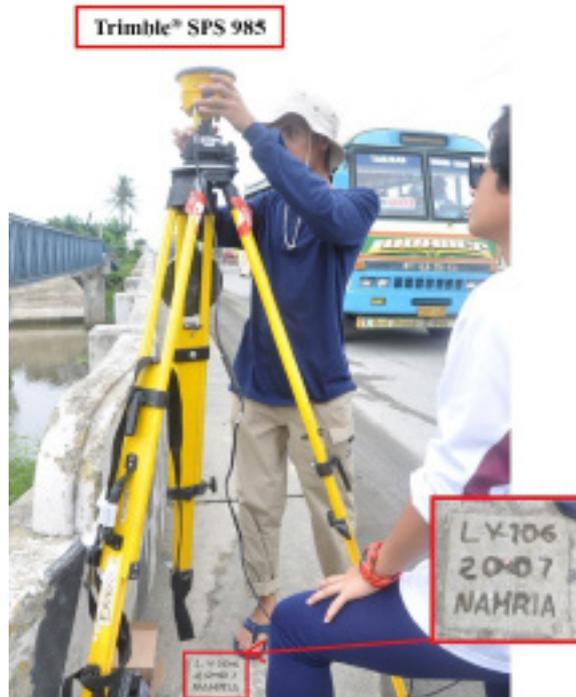
Figure 34. GNSS base set up, Trimble® SPS 985, at LY-106, located at the approach of Bernard Reed Bridge along Maharlika Highway , Brgy. Luntad, Municipality of Palo, Leyte
