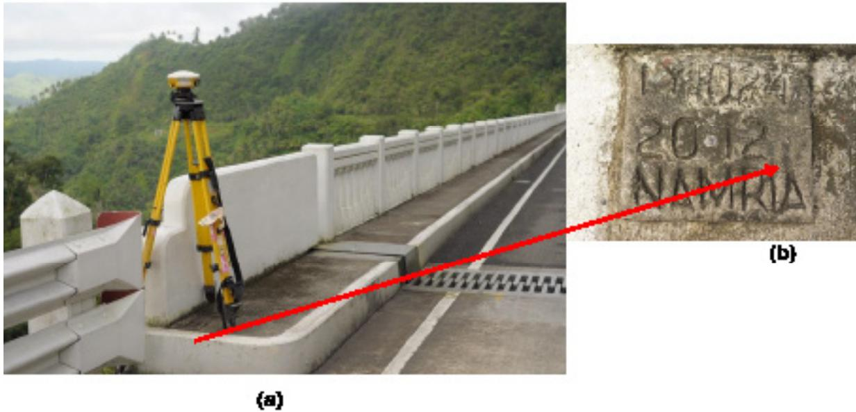
Figure 7. GPS set-up over LY-1024 located at the SE end of the sidewalk of Agas-agas Bridge at KM post 1006 + 972.6 and 4 meters from the road centerline.(a) and NAMRIA reference point LY-1024 (b) as recovered by the field team
