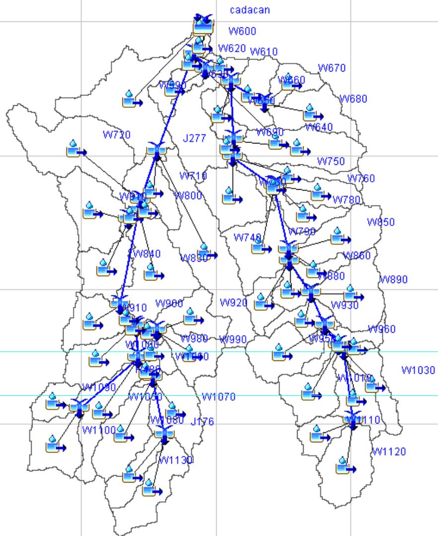
Figure 60. The Cadacan River Basin model generated using HEC-HMS
