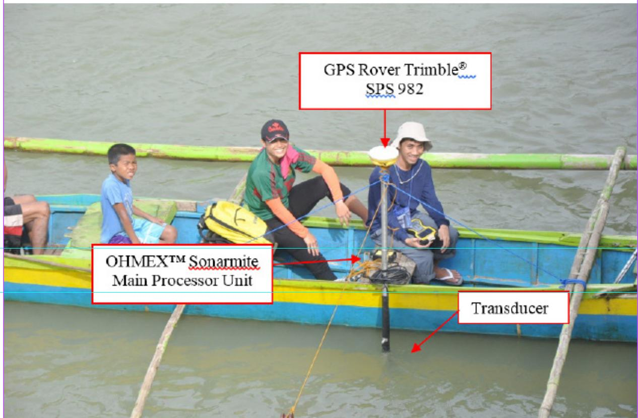
Figure 47. Bathymetric survey along Cadacan River
