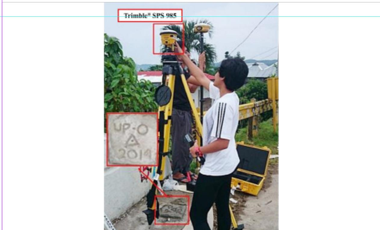
Figure 37. GNSS receiver set up, Trimble® SPS 985, at UP-O, an established control point, located at the bridge approach of the Ormoc Merida Bridge along Ormoc-Merida-Isabel-Palompon Road in Brgy. Liloan, City of Ormoc, Province of Leyte
