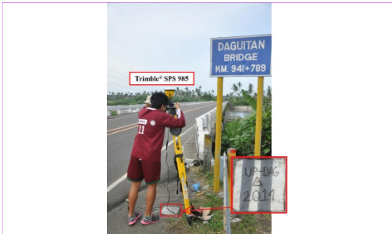
Figure 36. GNSS receiver set up, Trimble® SPS 985, at UP-DAG, an established control point, located at the bridge approach of the Daguitan Bridge along Maharlika Highway in Brgy. Fatima, Municipality of Dulag, Province of Leyte
