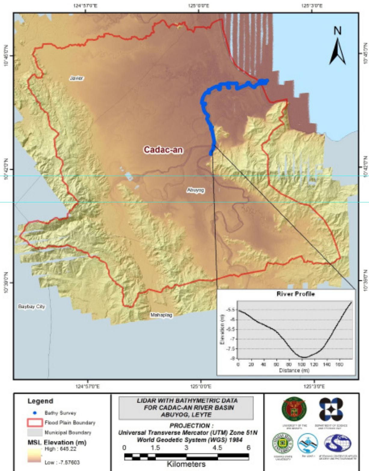
Figure 29. Map of Cadac-an Floodplain with bathymetric survey points shown in blue
