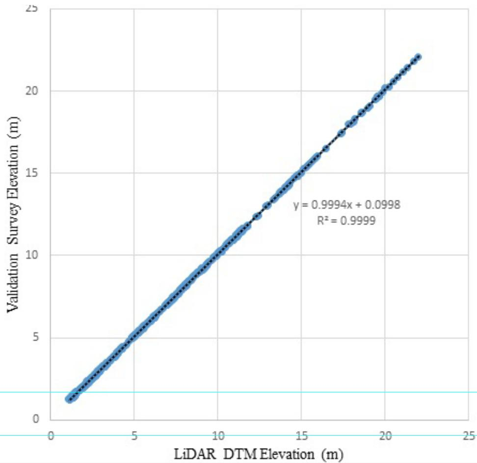
Figure 28. Correlation plot between validation survey points and LiDAR data
