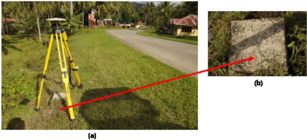
Figure 6. GPS set-up over LYT-757 as recovered on the opposite side of the kilometer post 997 in Barangay Mahayahay, Leyte. (a) and NAMRIA reference point LYT-757 (b) as recovered by the field team
