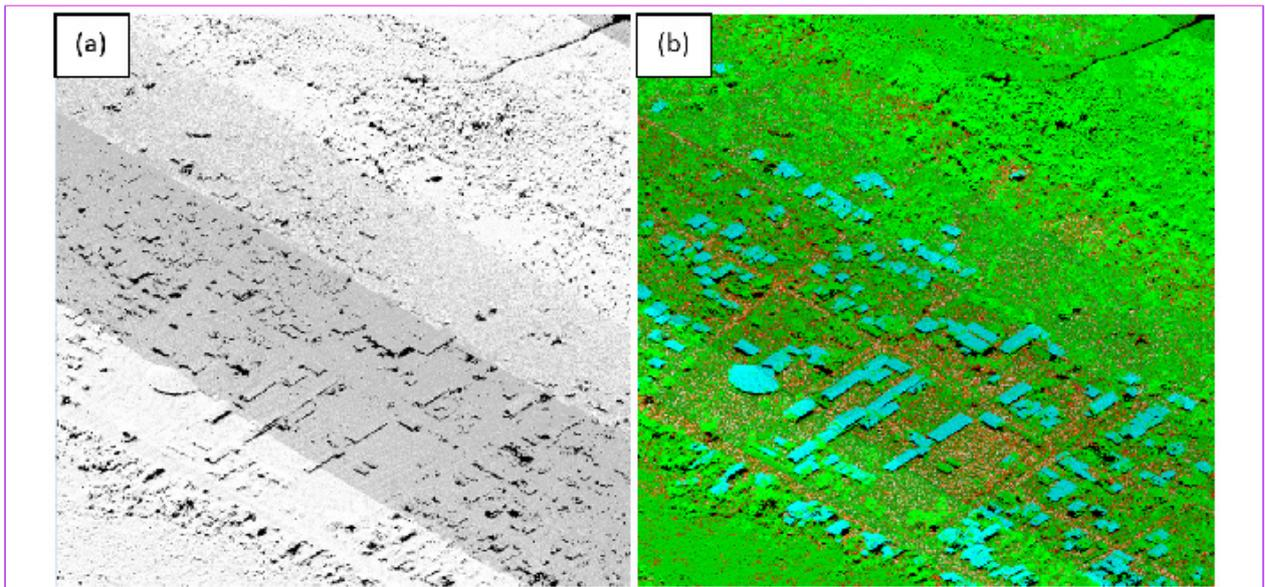
Figure 20. Point cloud before (a) and after (b) classification
