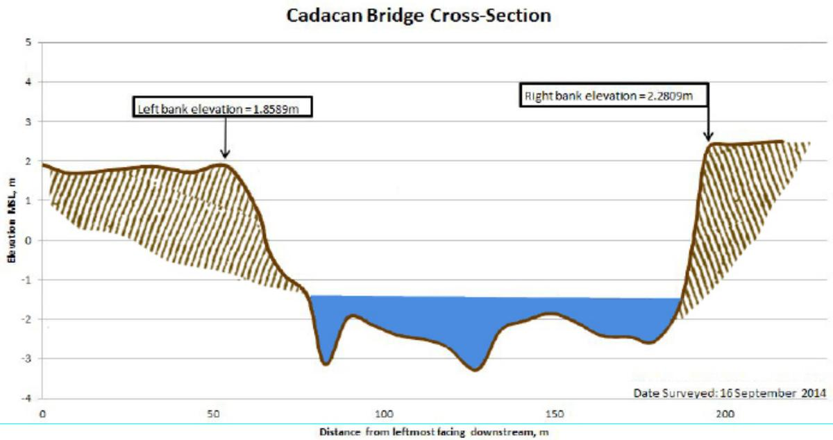
Figure 51. Cross-Section Plot of Cadacan Bridge
