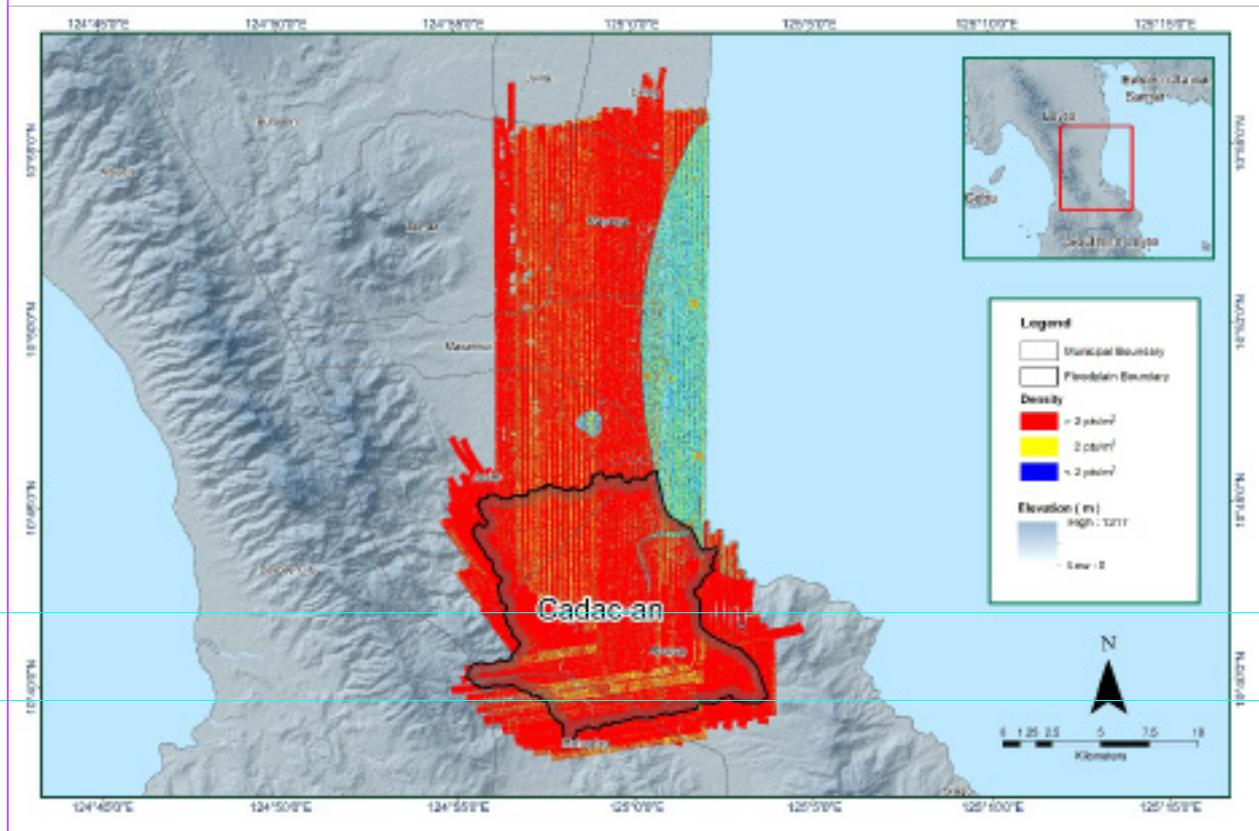
Figure 16. Pulse density map of merged LiDAR data for Cadac-an Floodplain
