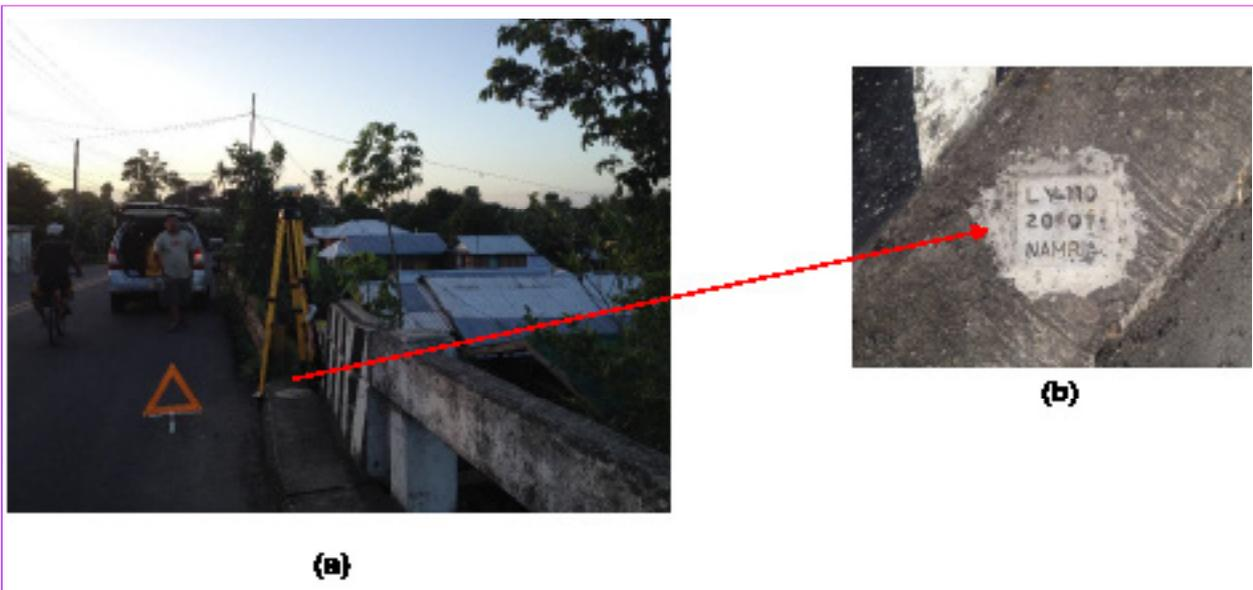
Figure 8. GPS set-up over LY-110 located on a bridge about 225 meters of km post 919, Libertad, Leyte. (a) and NAMRIA reference point LY-110 (b) as recovered by the field team
