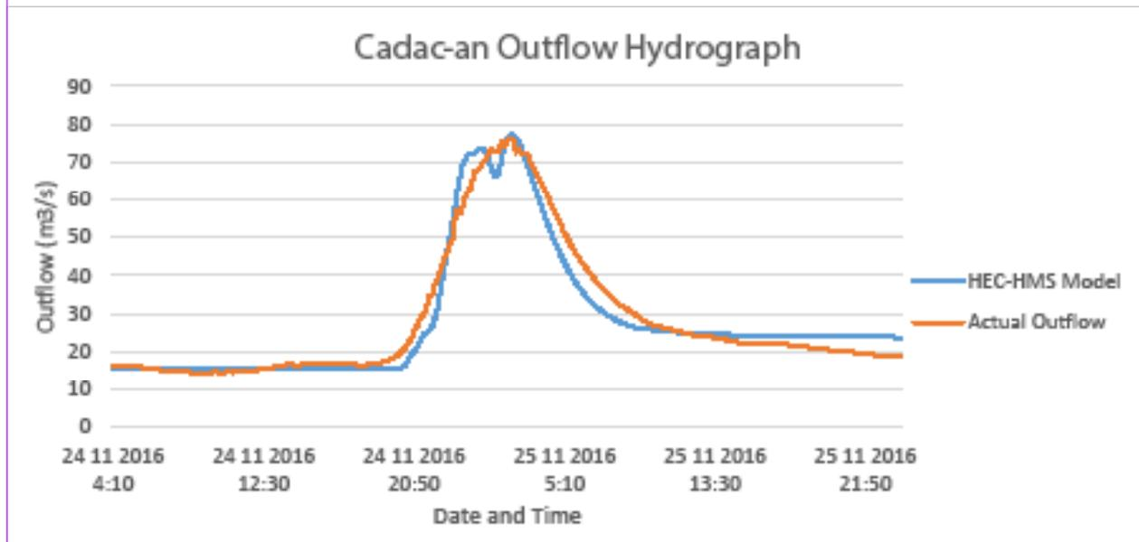
Figure 63. Outflow Hydrograph of Cadacan produced by the HEC-HMS model compared with observed outflow
