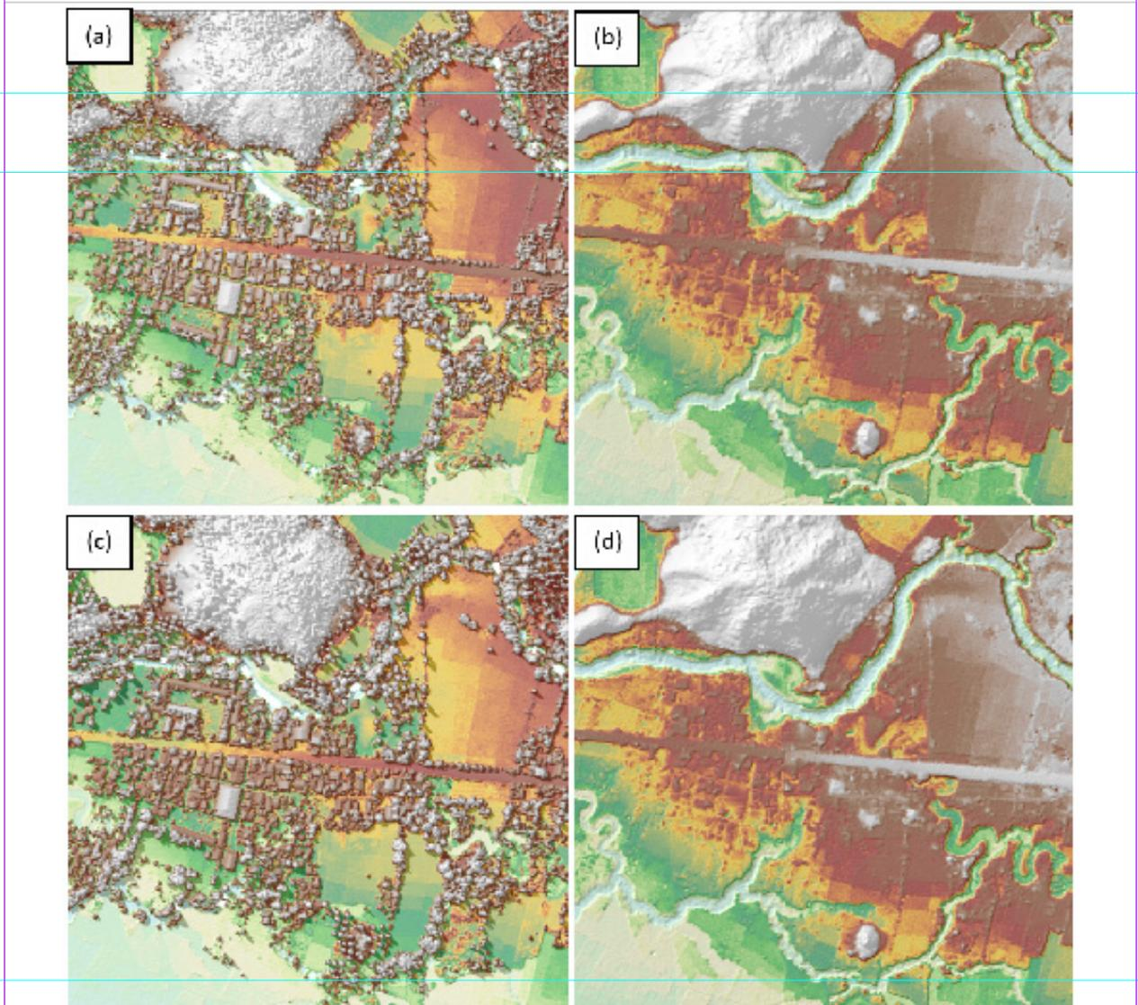
Figure 21. The production of last return DSM (a) and DTM (b), first return DSM (c) and secondary DTM (d) in some portion of Cadac-an Floodplain
