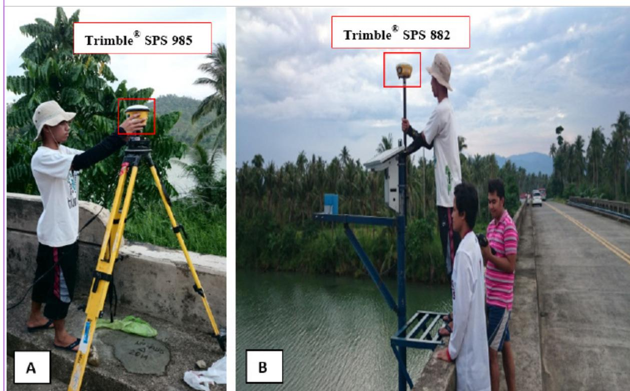
Figure 39. (A) Base set-up at UP-ABG and (B) Acquiring AWLS elevation at Cadacan Bridge, Abuyog, Leyte
