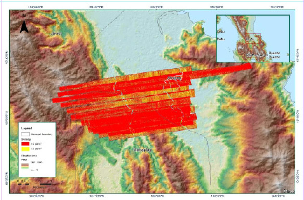
Figure 1.4.6. Density map of merged LiDAR data
