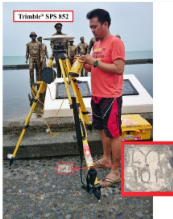
Figure 33. GNSS base set up, Trimble® SPS 852, at LYT-101, located at the General McArthur Shrine in Brgy. Candahog, Municipality of Palo, Leyte
