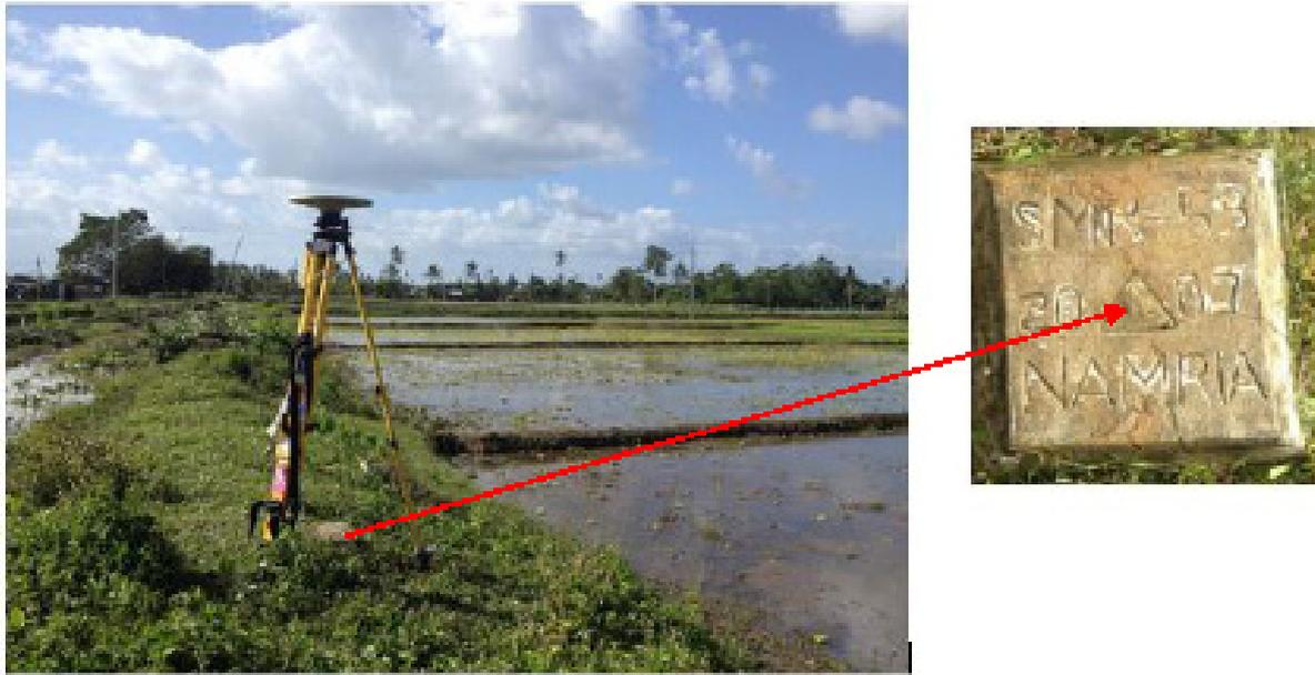
Figure 4. GPS set-up over LYT-104 as recovered and re-established along rice paddy trail, approximately 90 meters from the centerline, east side of Pastrana-Santa Fe Road, District IV, Pastrana, Leyte (a) and NAMRIA reference point LYT-104 (b) as recovered by the field team
