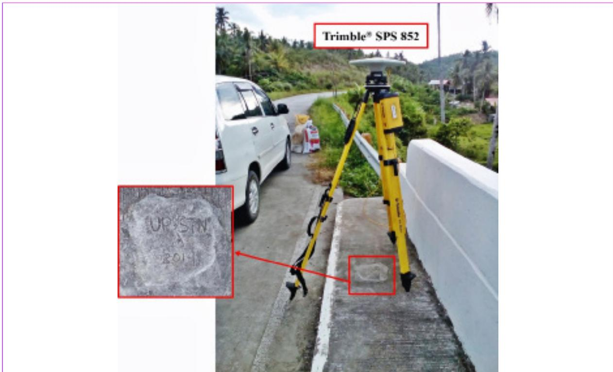
Figure 38. GNSS base set up, Trimble® SPS 852, at UP-STN, an established control point, located at Calaycalay Bridge approach in Brgy. Poblacion Zone 12, City of Baybay, Leyte
