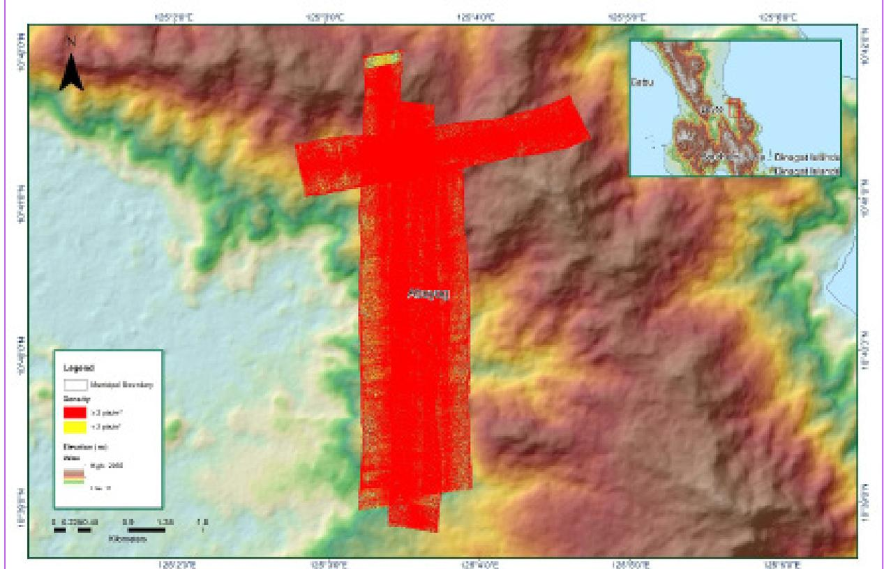
Figure 1.6.6. Density map of merged LiDAR data
