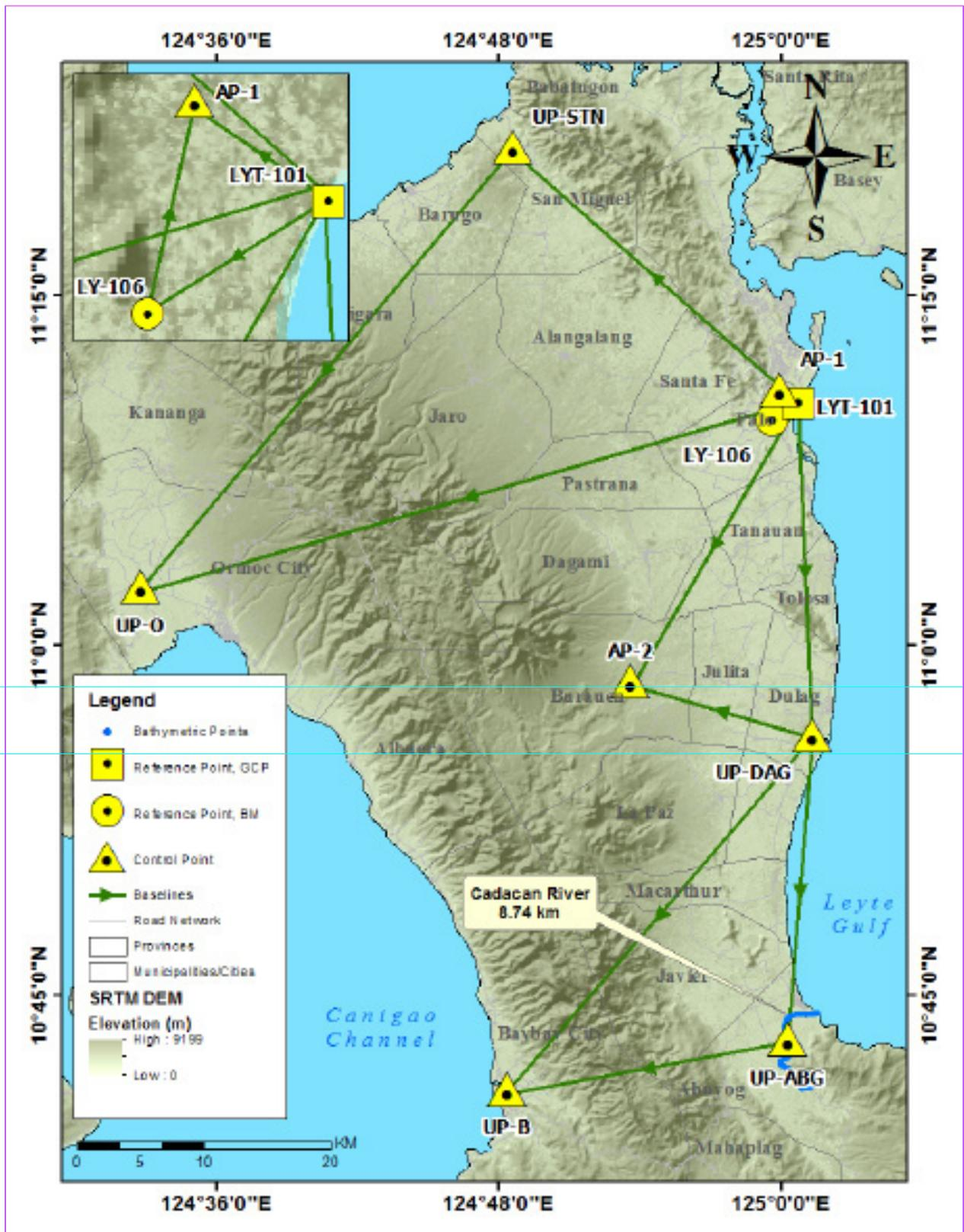
Figure 32. GNSS network for Cadacac River Survey
