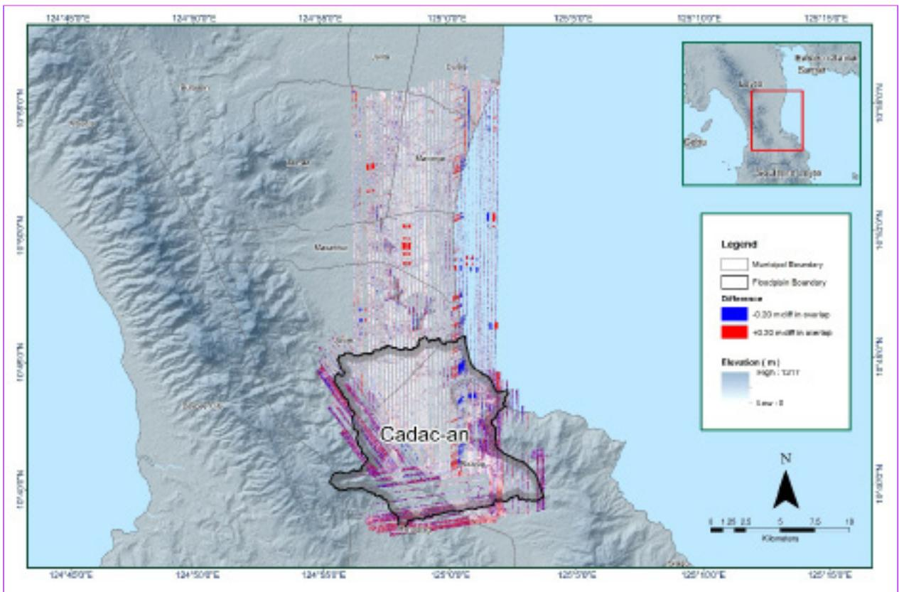
Figure 17. Elevation difference map between flight lines for Cadac-an Floodplain
