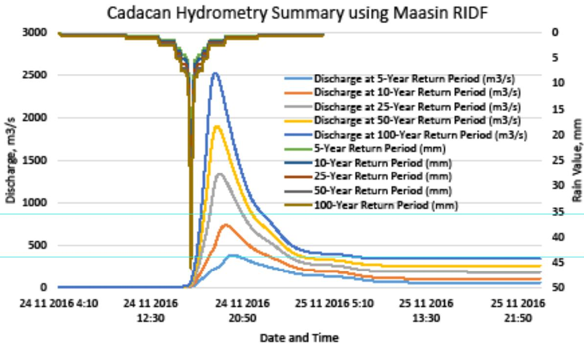
Figure 64. Outflow hydrograph at Cadacan Station generated using Maasin RIDF simulated in HEC-HMS
