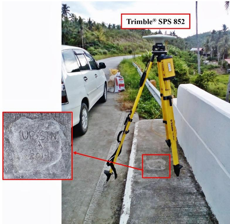
Figure 39. GNSS base set up, Trimble® SPS 852, at UP-STN, an established control point, located at Pagbanganan Bridge approach in Brgy. Brgy. Poblacion Zone 12, City of Baybay, Leyte
