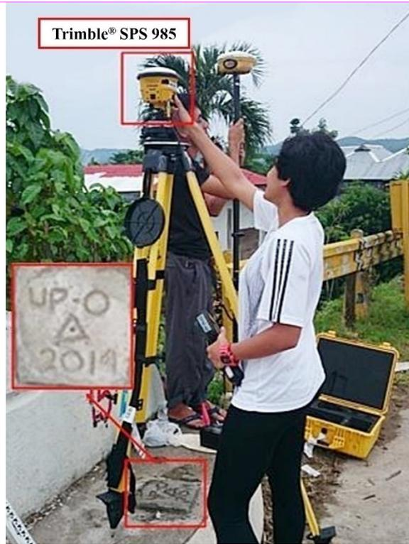
Figure 38. GNSS receiver set up, Trimble® SPS 985, at UP-O, an established control point, located at the bridge approach of the Ormoc Merida Bridge along Ormoc-Merida-Isabel-Palompon Road in Brgy. Liloan, City of Ormoc, Province of Leyte.
