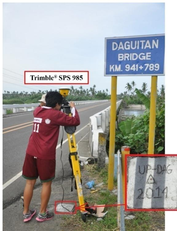
Figure 37. GNSS receiver set up, Trimble® SPS 985, at UP DAG, an established control point, located at the bridge approach of the Daguitan Bridge along Maharlika Highway in Brgy. Fatima, Municipality of Dulag, Province of Leyte
