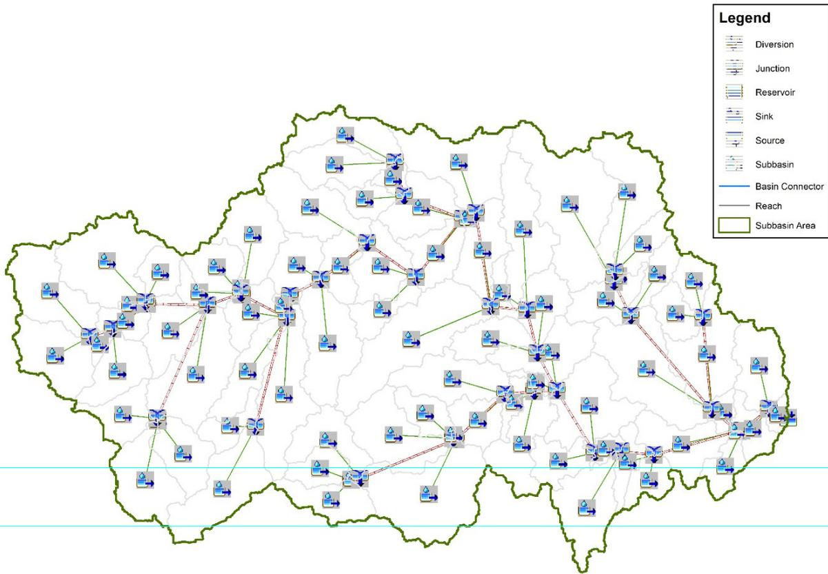
Figure 55. The Dolore river basin model generated using HEC-HMS
