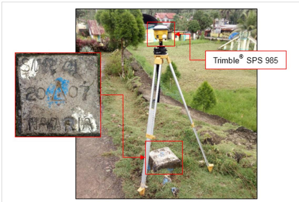
Figure 27. GNSS base set up, Trimble® SPS 985, at SMR-41, located 20 m SW from the flagpole in Bagacay Elementary School playground in Brgy. Bagacay, Hinabangan, Eastern Samar
