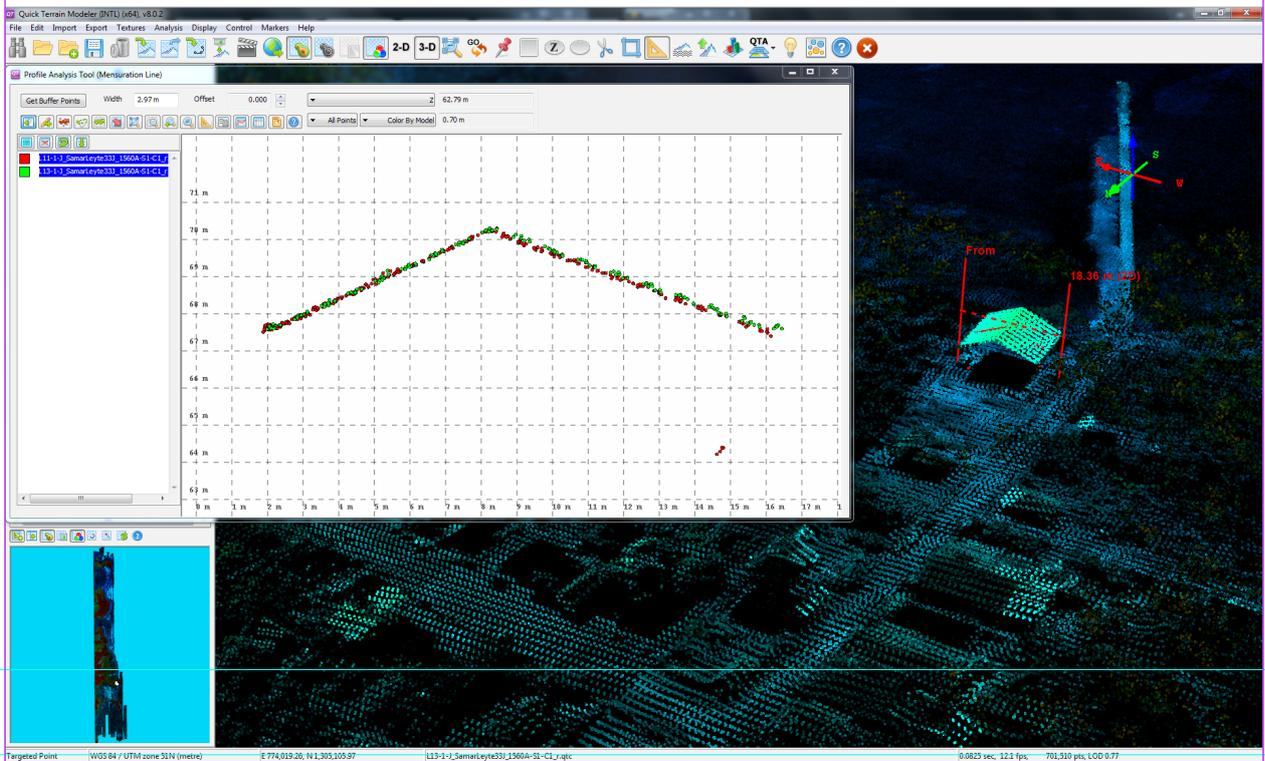
Figure 13. Quality checking for a Dolores flight 1560A using the Profile Tool of QT Modeler.
