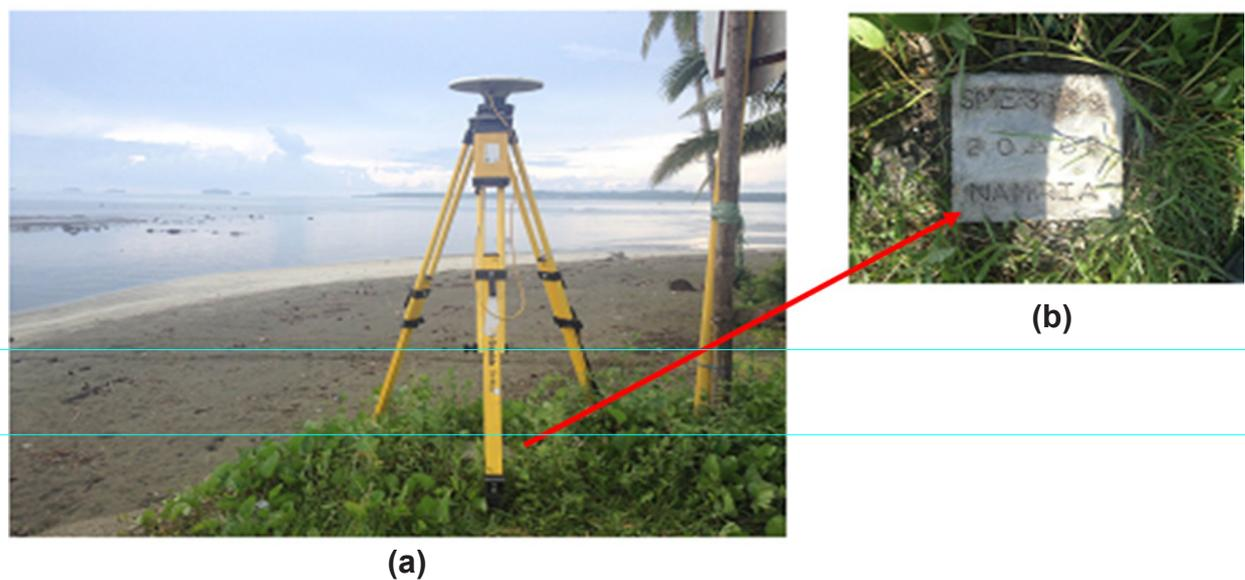
Figure 3. GPS set-up over SME-3139 located along the highway in Brgy. Sto. Nino, Dolores, Eastern Samar (a) and NAMRIA reference point SME-3139 (b) as recovered by the field team.
