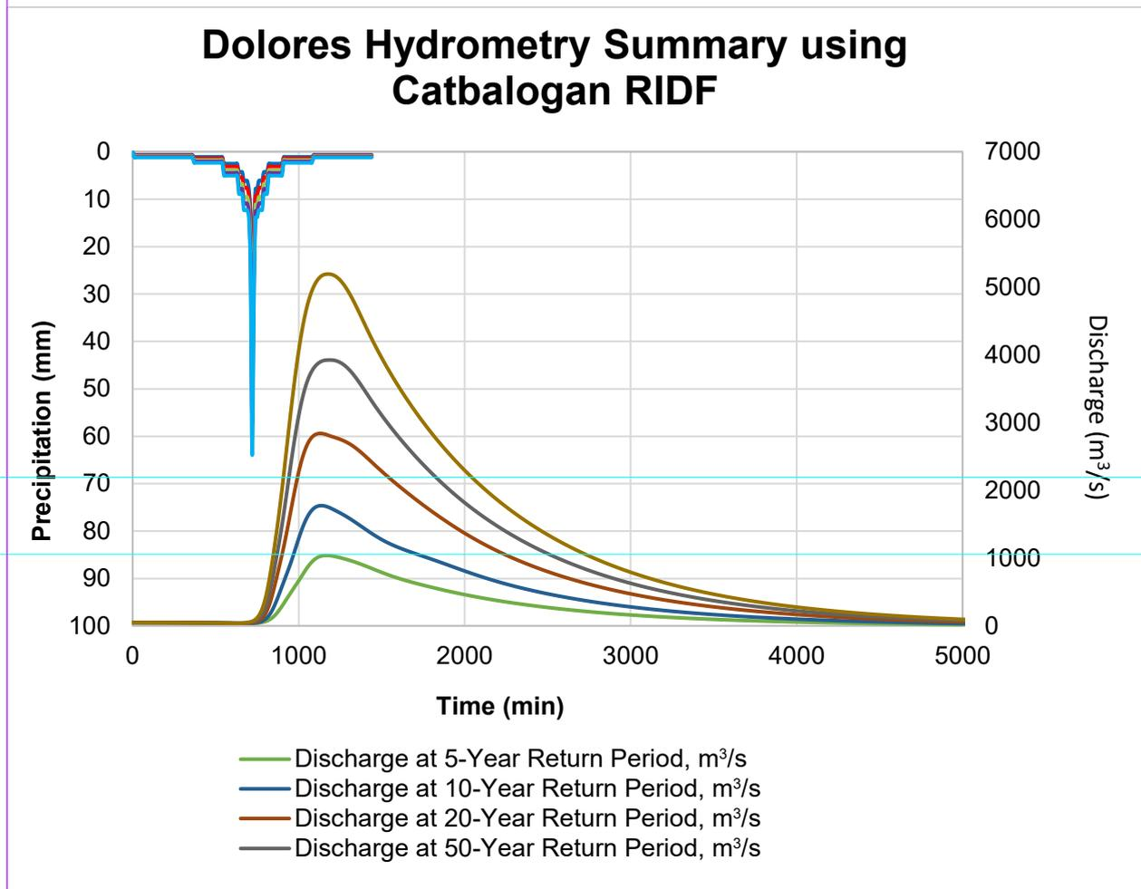
Figure 59. Outflow hydrograph at Dolores Station generated using Catbalogan RIDF simulated in HEC-HMS
