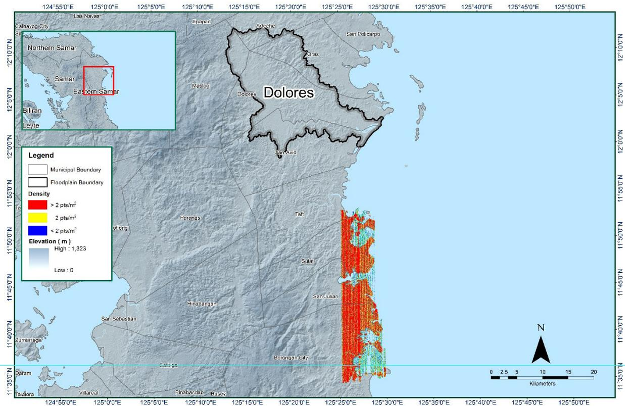
Figure 11. Pulse density map of merged LiDAR data for Dolores Floodplain.
