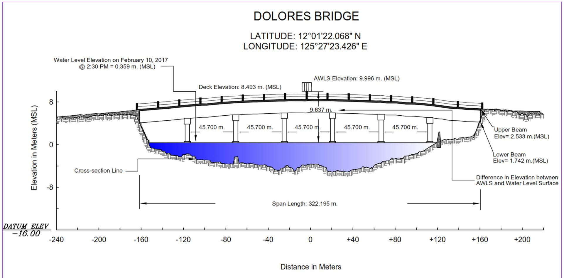
Figure 33. Dolores Bridge Cross-section Diagram
