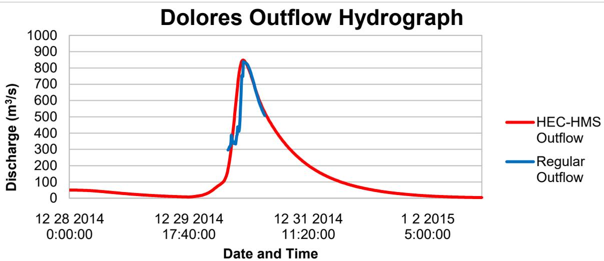
Figure 58. Outflow Hydrograph of Dolores Bridge generated in HEC-HMS model compared with observed outflow
