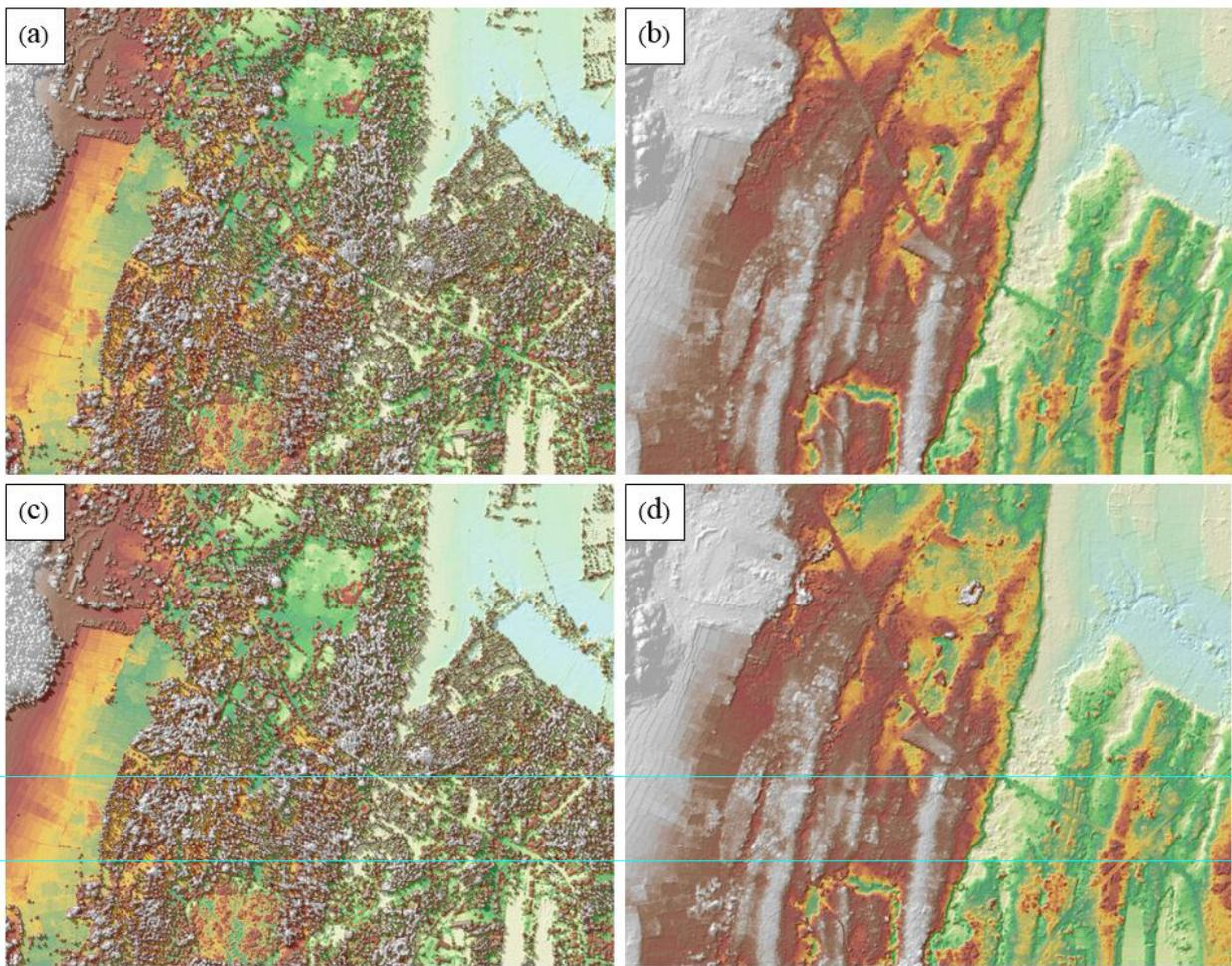
Figure 16. The Production of last return DSM (a) and DTM (b), first return DSM (c) and secondary DTM (d) in some portion near Dolores Floodplain.
