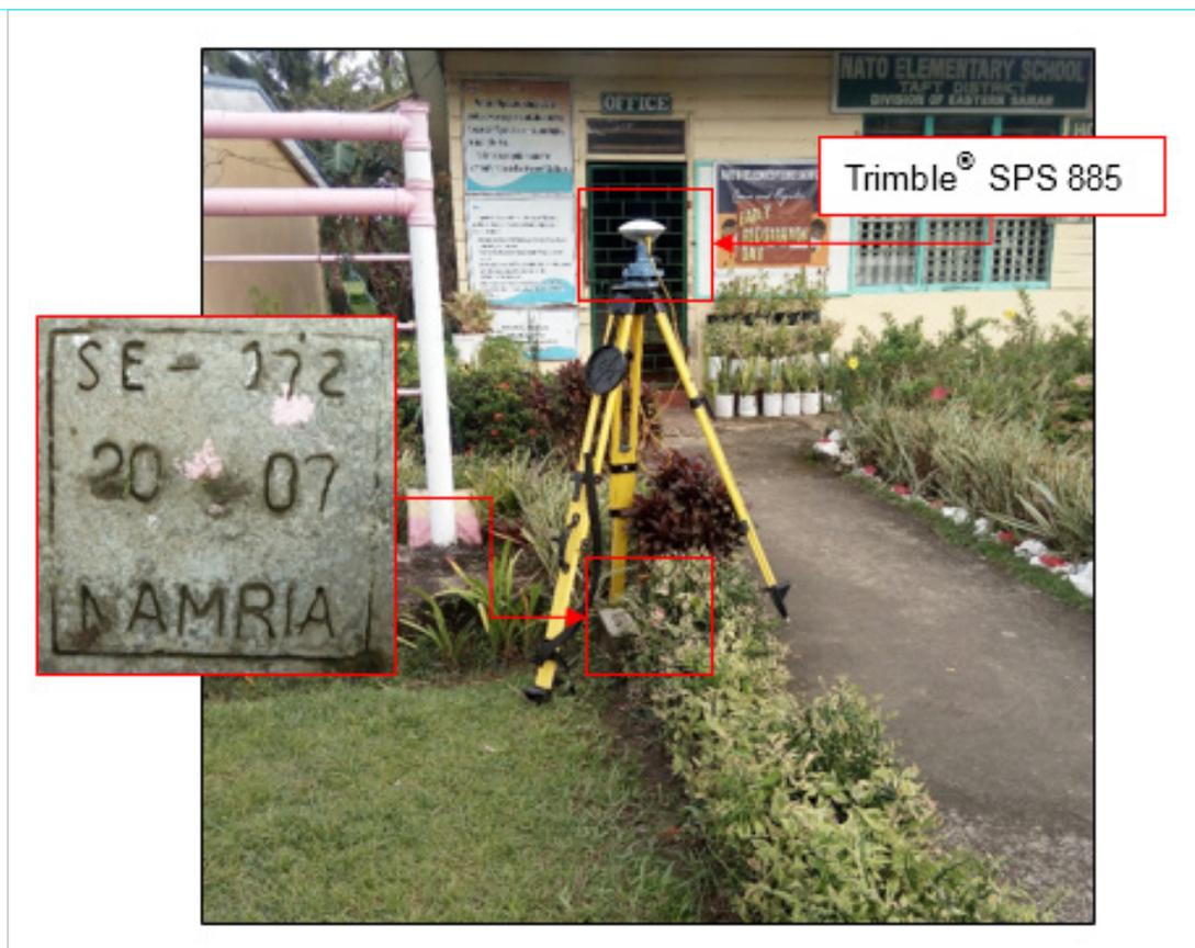
Figure 28. GNSS receiver set up, Trimble® SPS 885, at SE-172, located beside the walkway leading to the office of Nato Elementary School in Brgy. Nato, Taft, Eastern Samar
