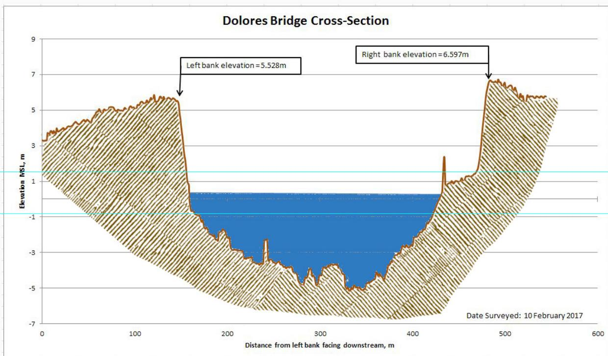
Figure 46. Cross-Section Plot of Dolores Bridge
