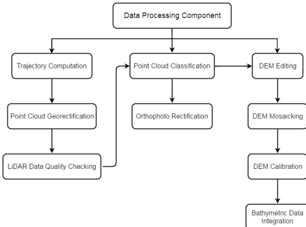
Figure 5. Schematic diagram for the Data Pre-Processing Component
