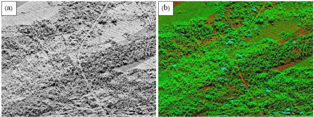
Figure 15. Point cloud before (a) and after (b) classification.
