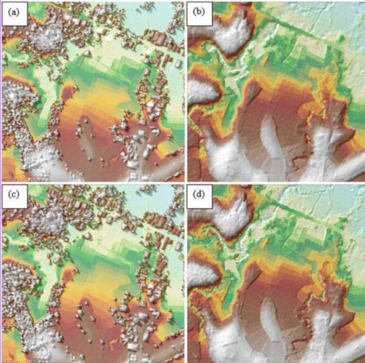
Figure 15. The production of last return DSM (a) and DTM (b), first return DSM (c) and secondary DTM (d) in some portion of Gandara floodplain.
