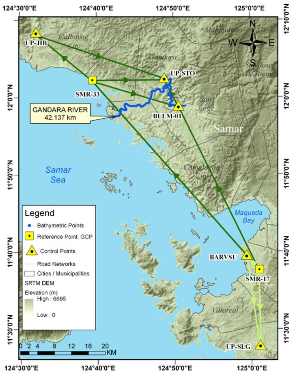
Figure 27. The GNSS Network established in the Gandara River Survey.
