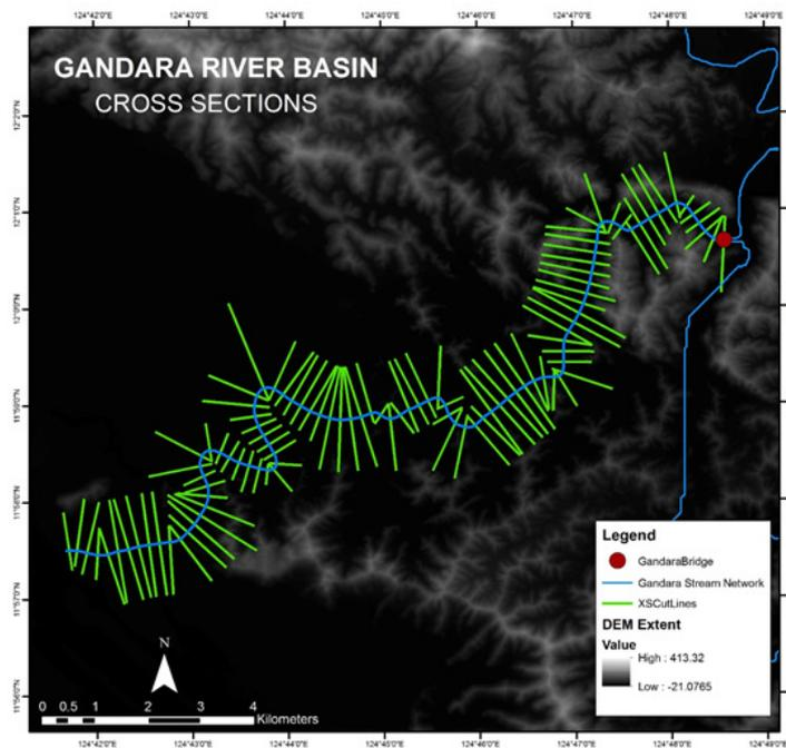
Figure 61. River cross-section of the Gandara River through the ArcMap HEC GeoRAS tool.
