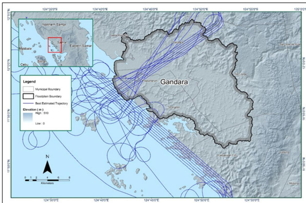
Figure 7. Best Estimated Trajectory of the LiDAR missions conducted over the Gandara Floodplain.
