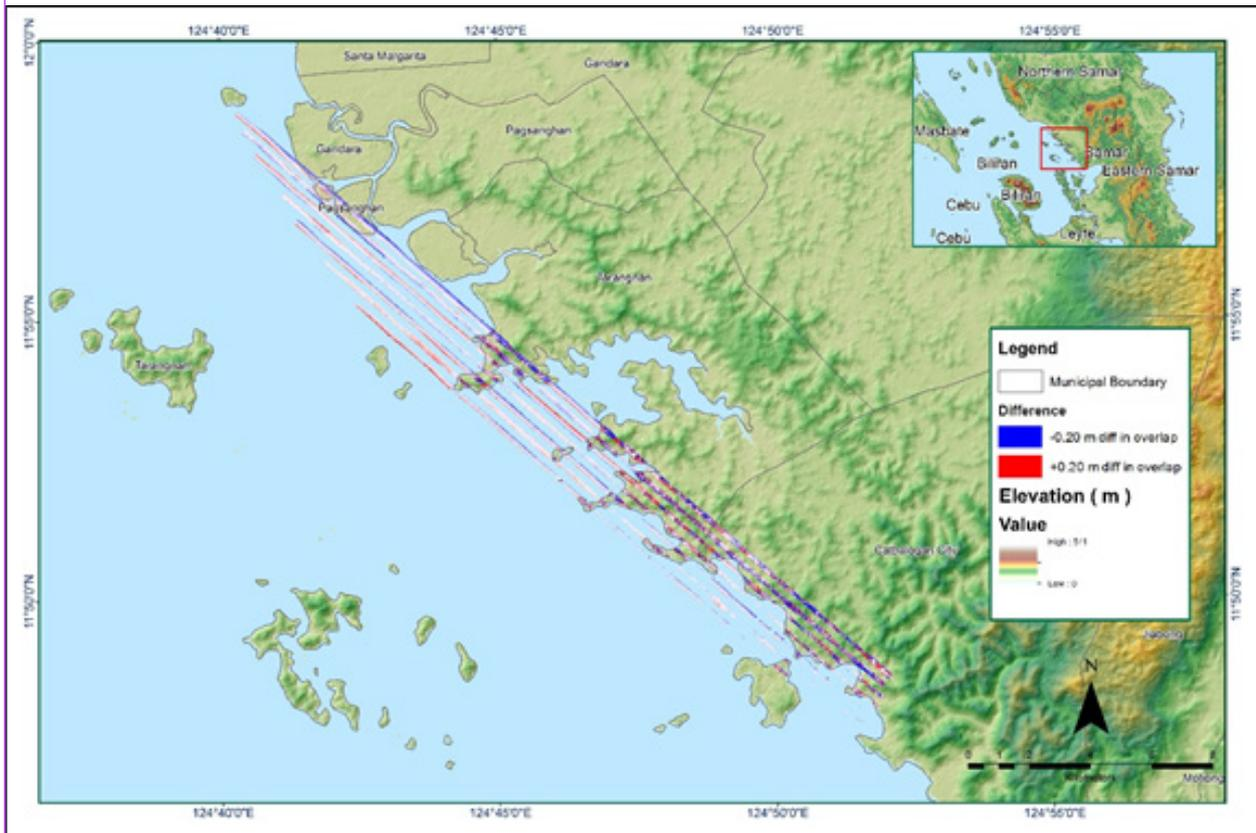
Figure A-8.9. Elevation difference between flight lines
