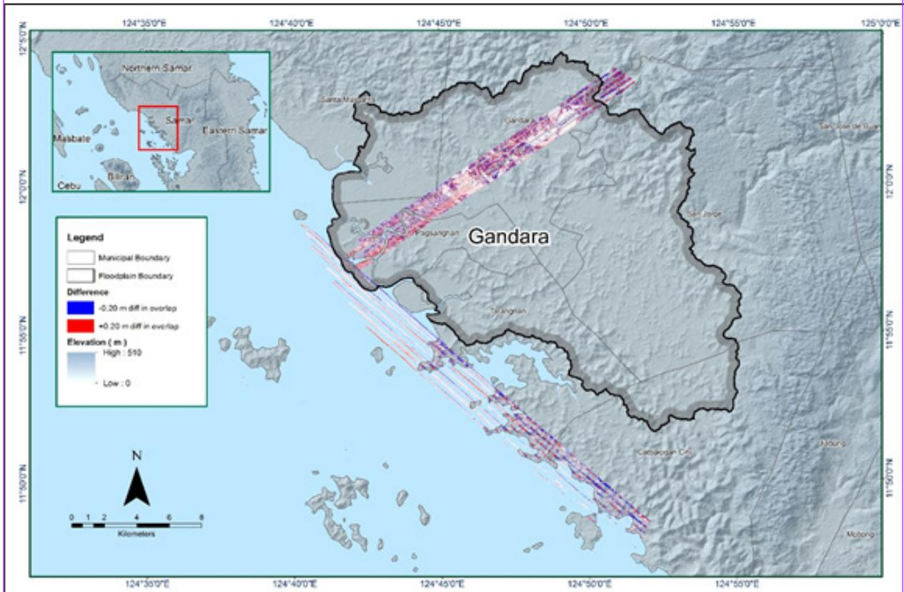
Figure 11. Elevation difference Map between flight lines for the Gandara Floodplain Survey.
