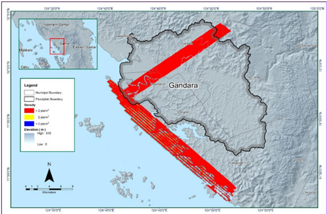
Figure 10. Pulse density map of the merged LiDAR data for Gandara floodplain.
