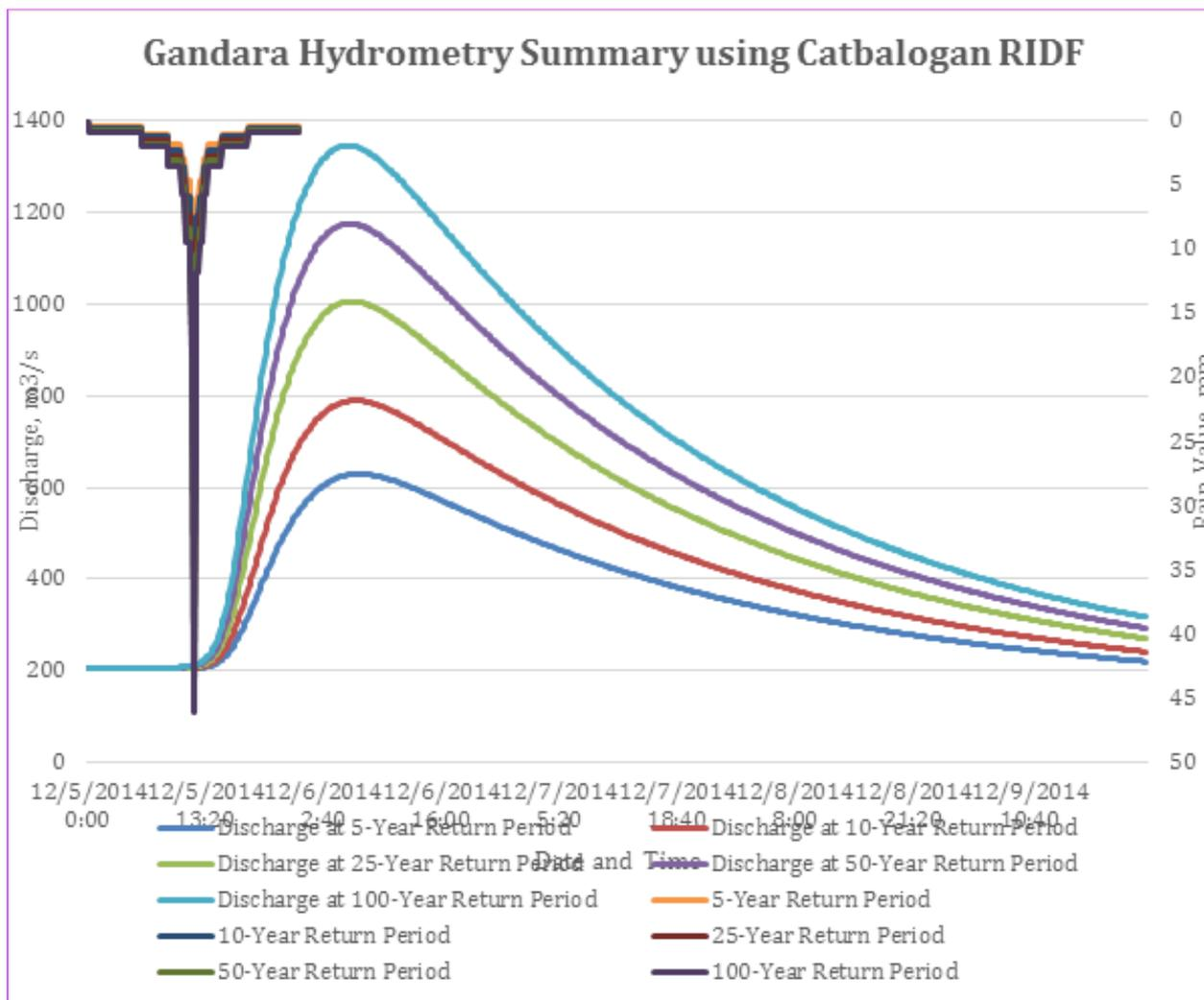
Figure 64. The Outflow hydrograph at the Gandara Station, generated using the Catbalogan RIDF simulated in HEC-HMS.
