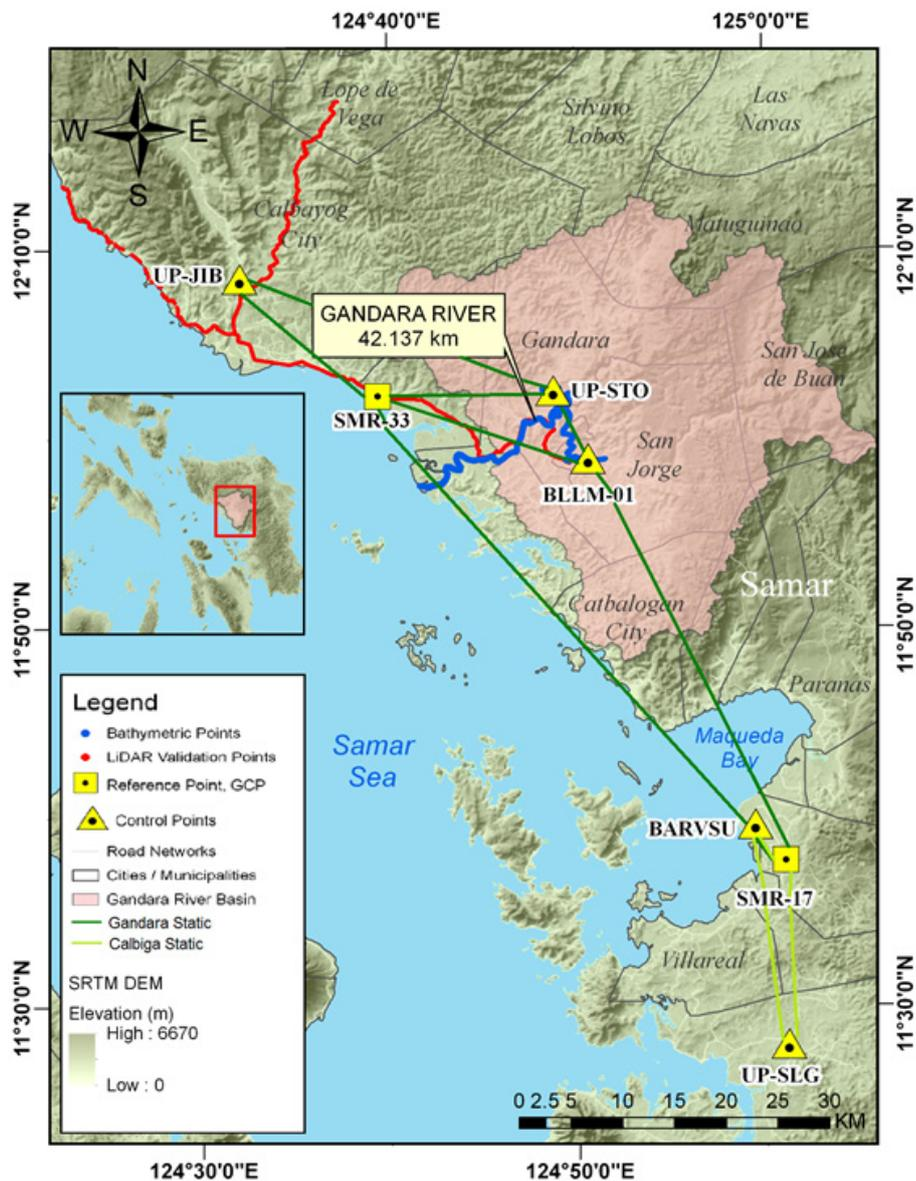
Figure 26. Extent of the bathymetric survey (in blue line) in Gandara River and the LiDAR data validation survey (in red).
