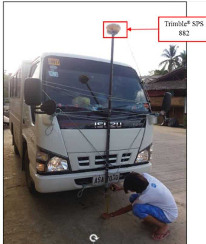
Figure 41. GNSS Receiver Trimble® SPS 882 installed on a vehicle for Ground Validation Survey.
