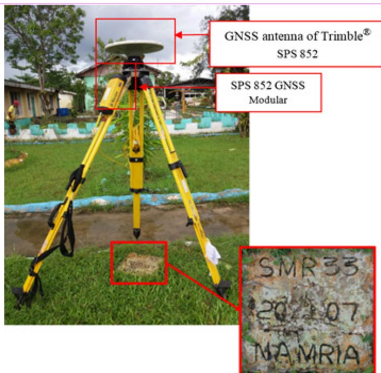
Figure 29. Trimble® SPS 852 set-up at SMR-33 located inside the compound of Sta. Margarita Elementary School in Brgy. Monbon, Municipality of Sta. Margarita, Samar.
