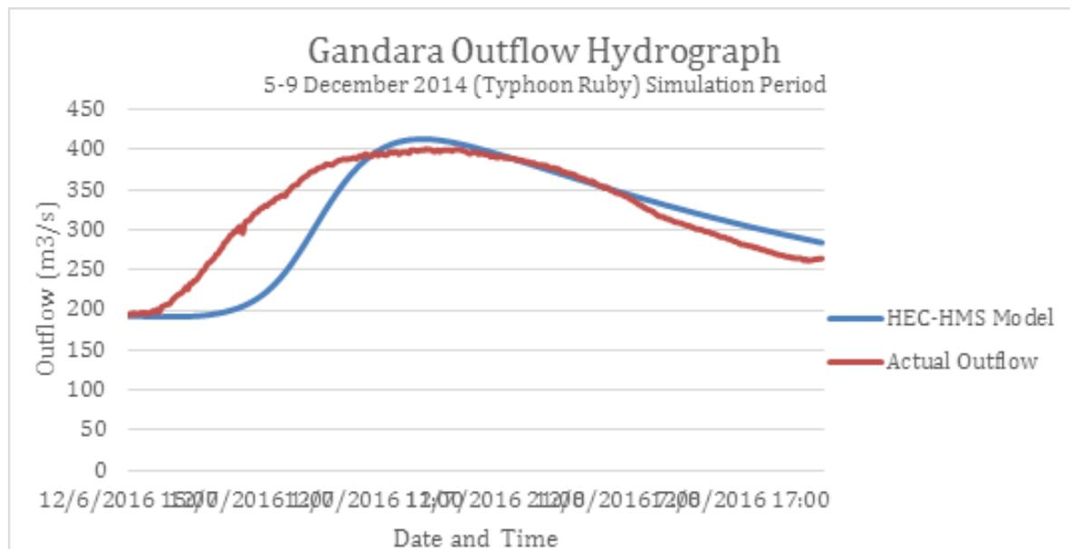
Figure 63. Outflow Hydrograph of Gandara Bridge produced by the HEC-HMS model compared with observed outflow.
