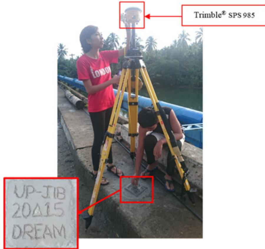
Figure 31. Trimble SPS® 985 set-up at UP-JIB, Jibatang Bridge approach in Brgy. Oquendo, Calbayog City, Samar
