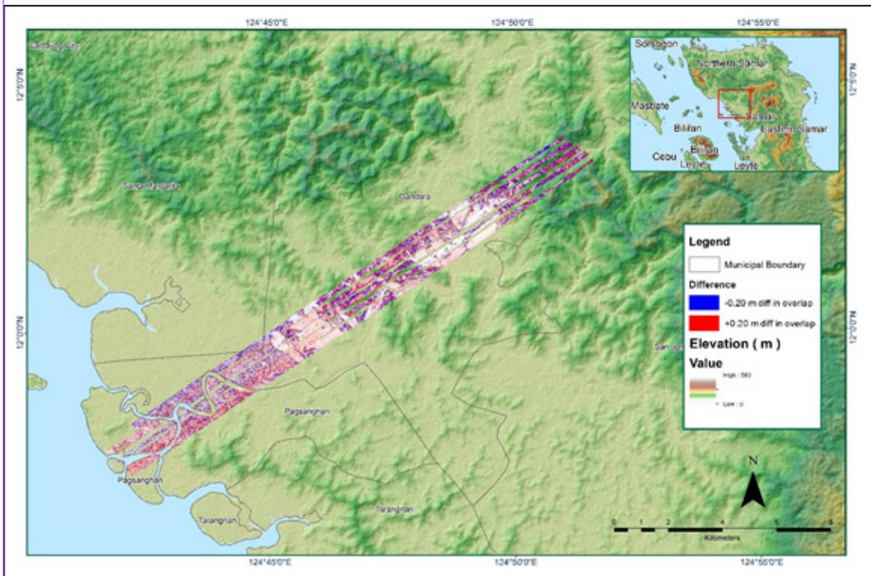
Figure A-8.18 Elevation difference between flight lines
