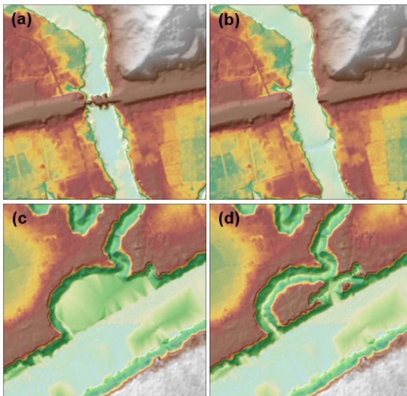
Figure 18. Portions in the DTM of the Gandara Floodplain – a river embankment before (a) and after (b) data retrieval; a bridge before (c) and after (d) manual editing.
