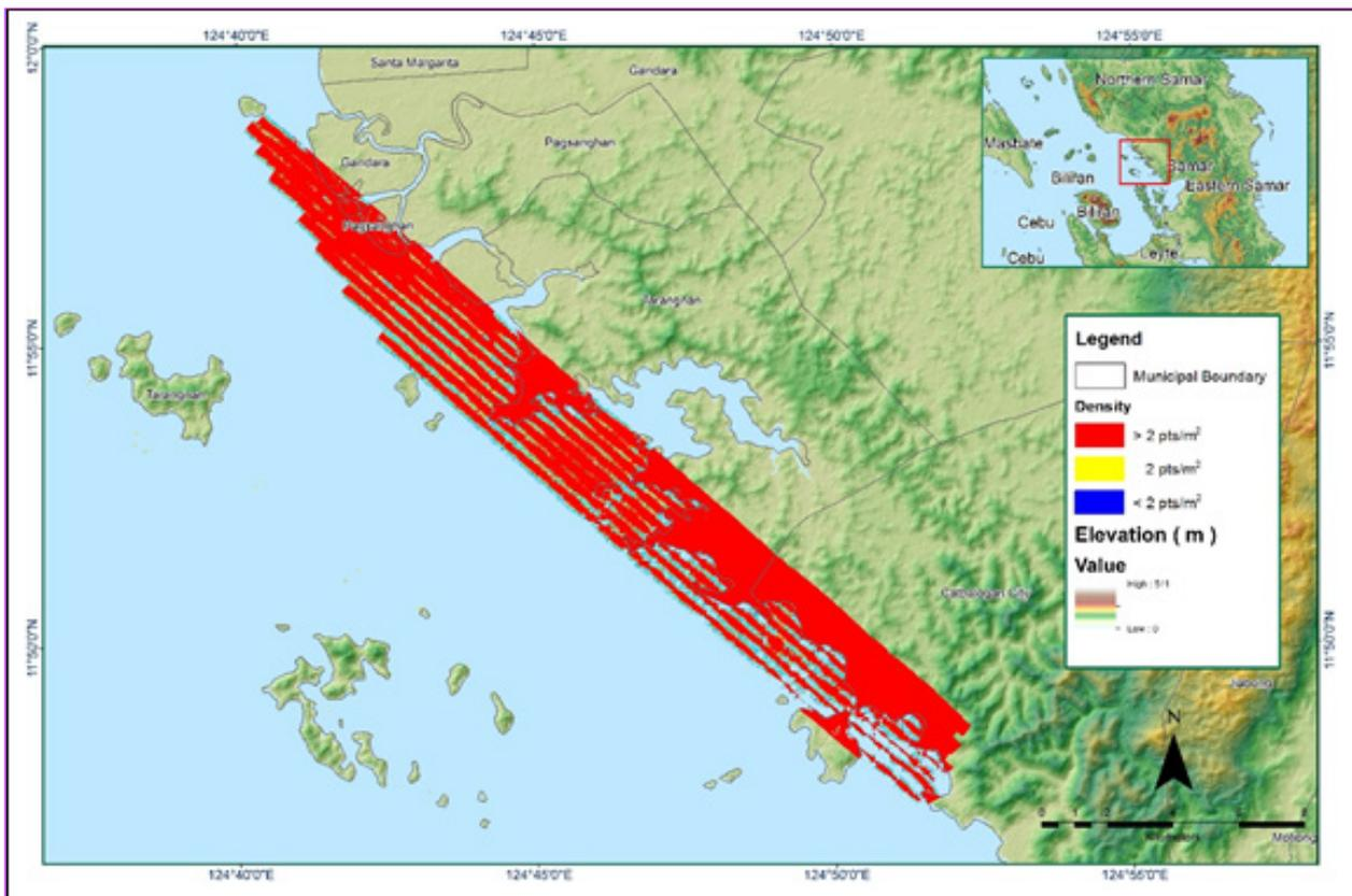
Figure A-8.8. Density map of merged LiDAR data
