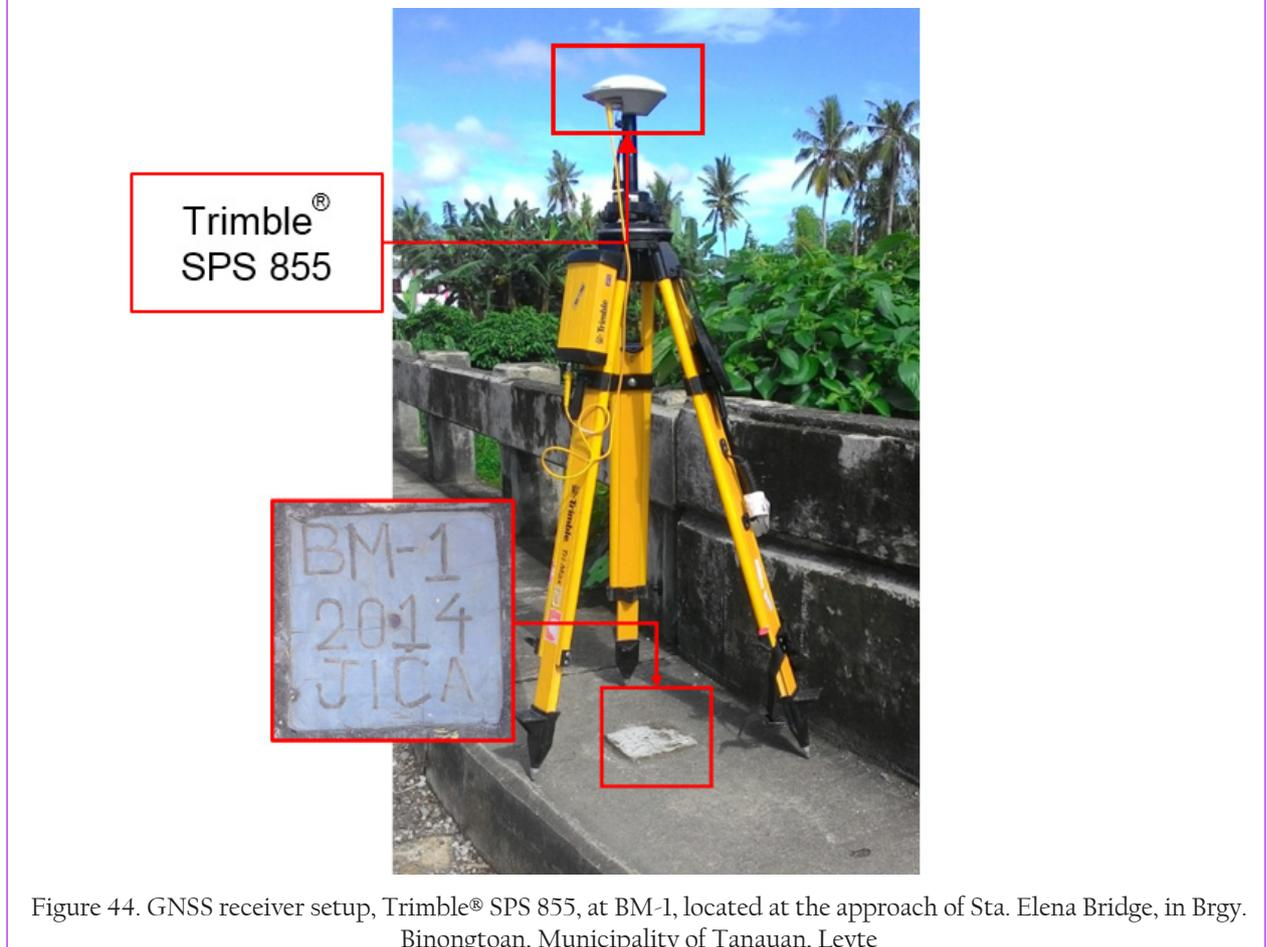
Figure 44. GNSS receiver setup, Trimble® SPS 855, at BM-1, located at the approach of Sta. Elena Bridge, in Brgy. Binongtoan, Municipality of Tanauan, Leyte
