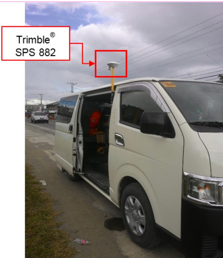
Figure 51. Validation points acquisition survey set up along Guinarona River Basin
