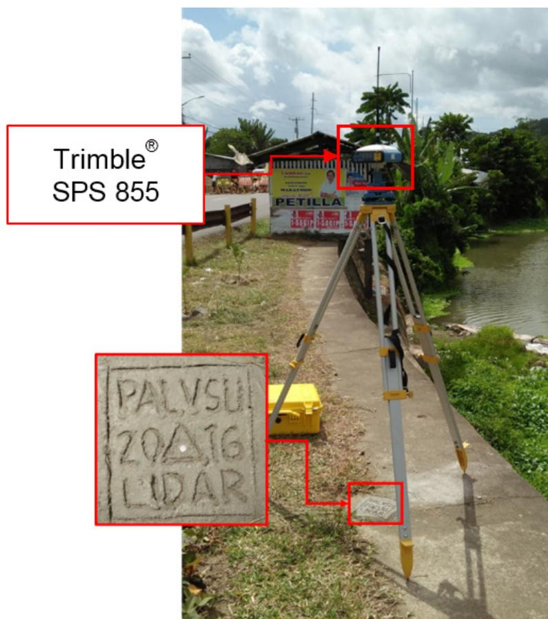
Figure 42. GNSS receiver setup, Trimble® SPS 855, at PAL-VSU, located on top of revetment along Bangon River in Brgy. Arado, Municipality of Palo, Leyte
