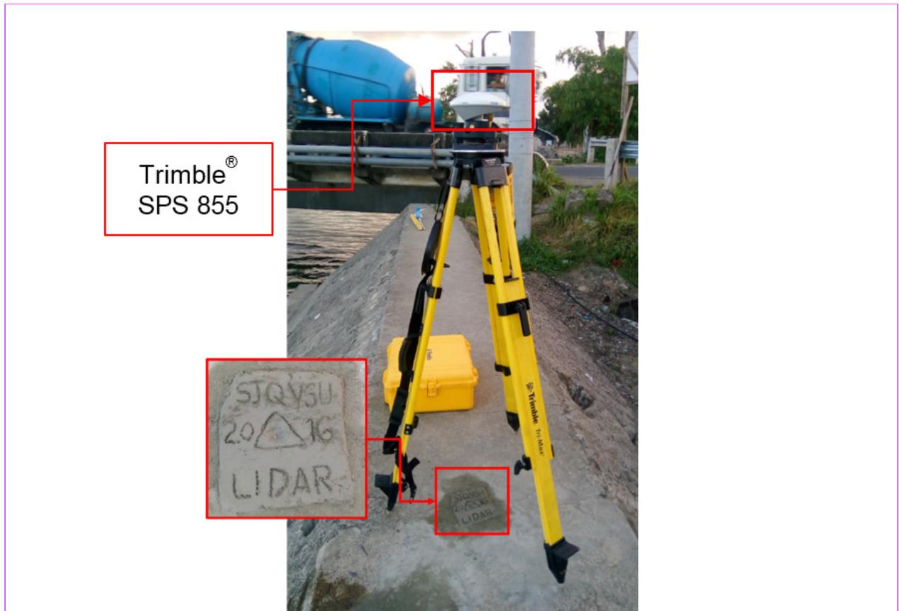
Figure 43. GNSS receiver setup, Trimble® SPS 855, at SJQ-VSU, located near the approach of San Joaquin Bridge, in Brgy. San Joaquin, Municipality of Palo, Leyte
