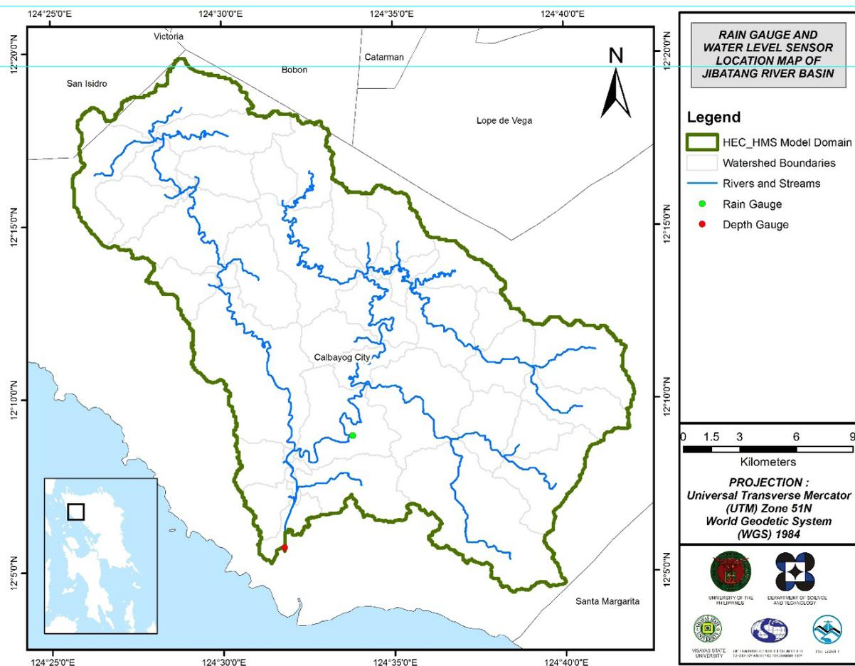
Figure 44. Location map of Jibatang HEC-HMS model used for calibration
