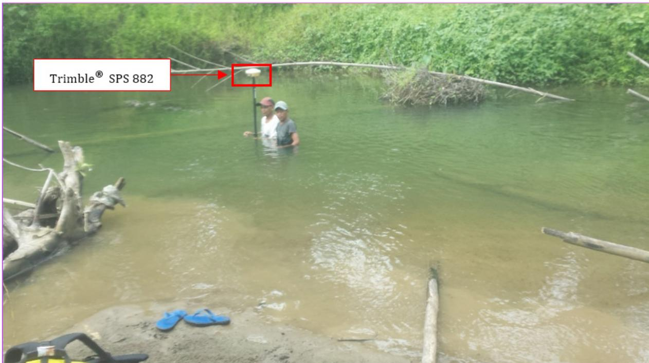
Figure 39. Manual bathymetry along the Jibatang River
