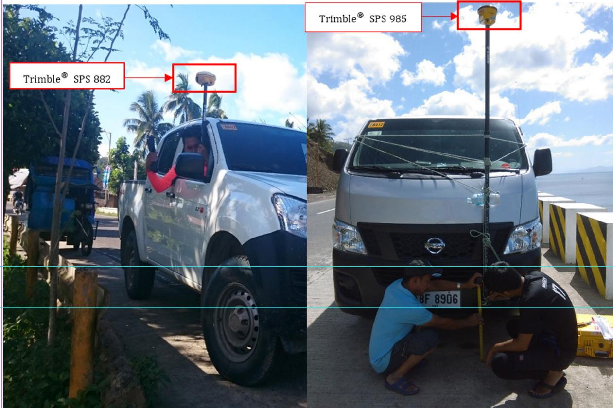
Figure 36. Validation points acquisition survey set-up
