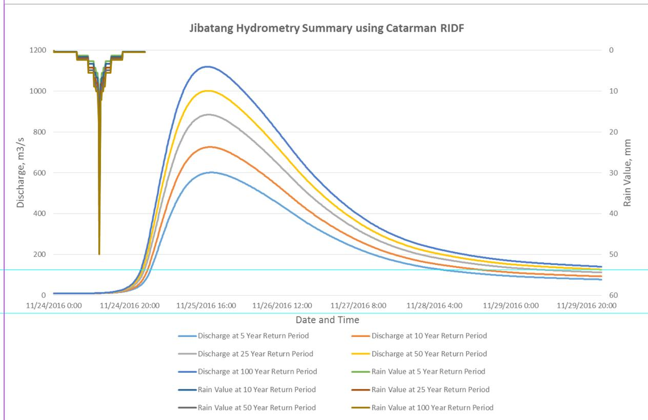
Figure 58. Outflow hydrograph at the Jibatang Station generated using the Catarman RIDF, simulated in HEC-HMS
