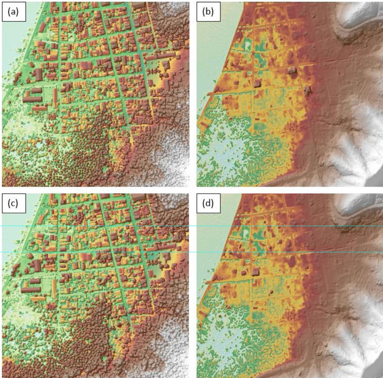
Figure 15. The production of last return (a) DSM and (b) DTM; and, (c) first return DSM and (d) secondary DTM in some portion near the Jibatang floodplain
