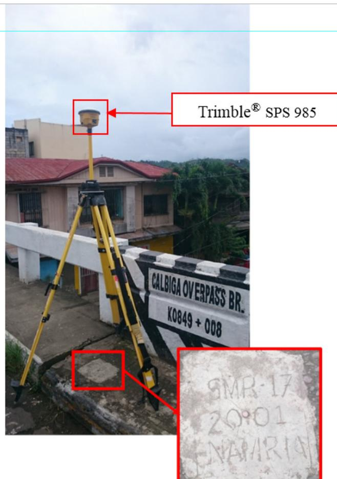
Figure 26. GNSS receiver set-up, Trimble® SPS 985, at SMR-17, located at the Calbiga overpass Bridge approach in Barangay Macaalan, Municipality of Calbiga, Samar
