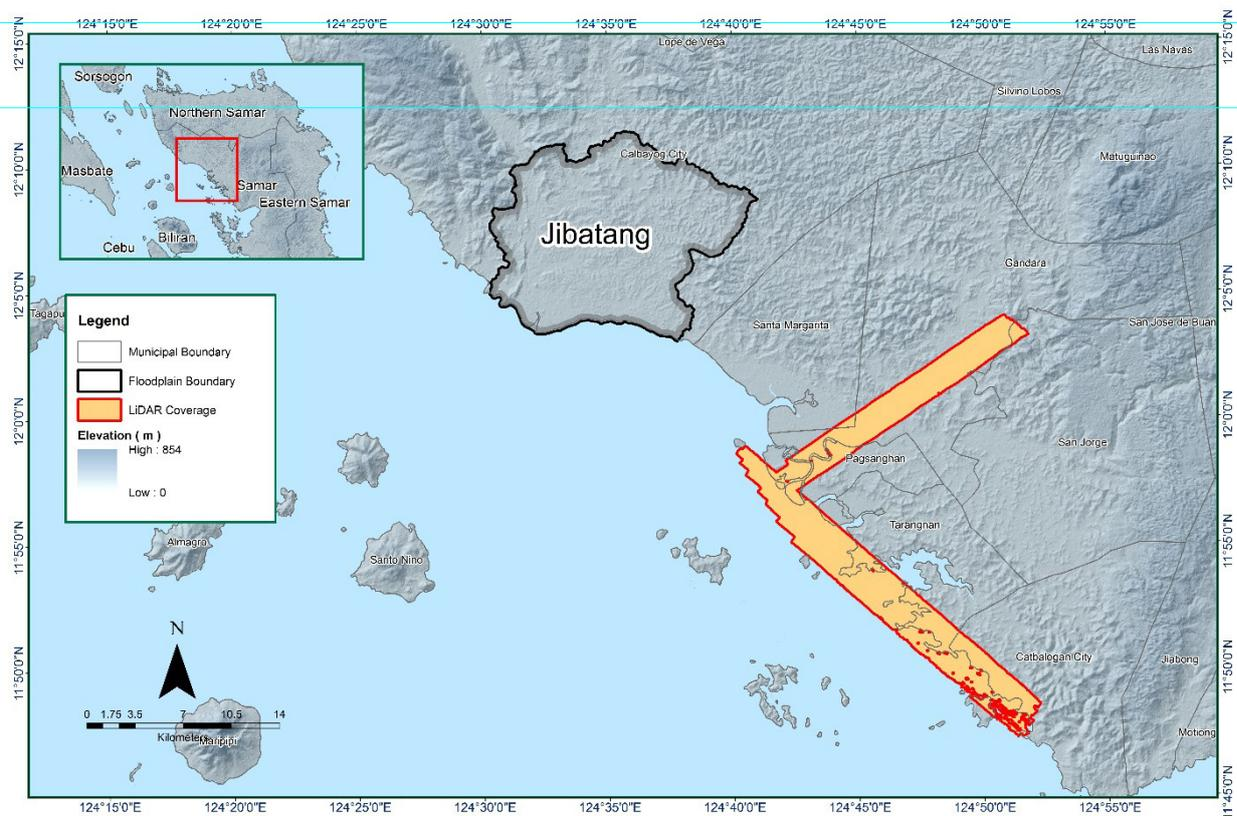
Figure 8. Boundaries of the processed LiDAR data over the Jibatang floodplain
