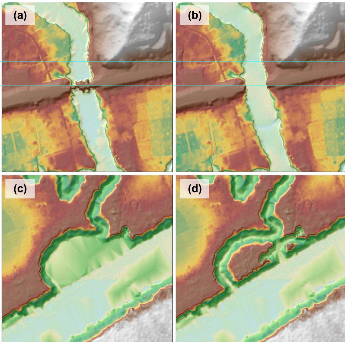
Figure 18. Portions in the DTM of blocks neighboring the Jibatang floodplain – a bridge (a) before and (b) after manual editing; and a river embankment (c) before and (d) after data retrieval
