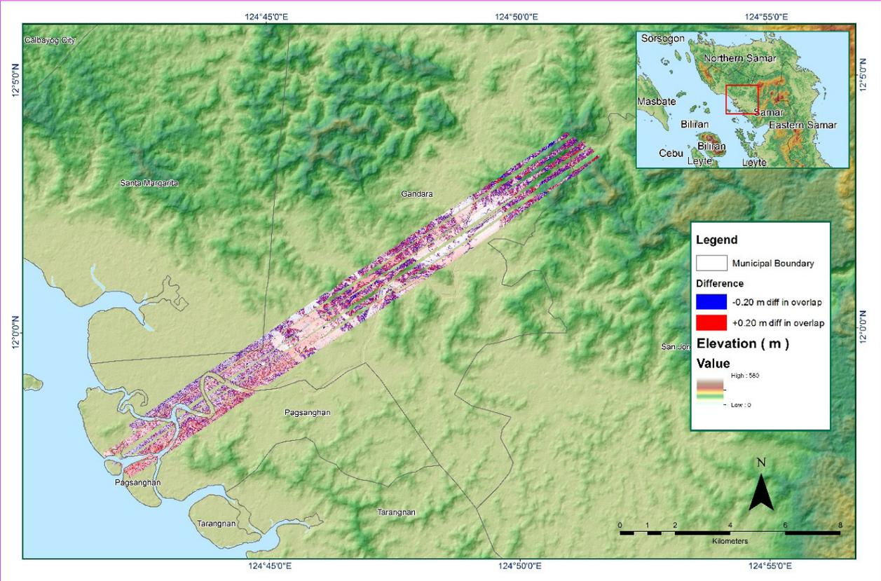
Figure A-8.18. Elevation difference between flight lines
