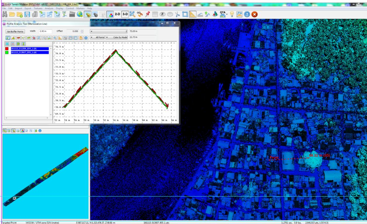
Figure 12. Quality checking for Jibatang flight 10225L using the Profile Tool of QT Modeler
