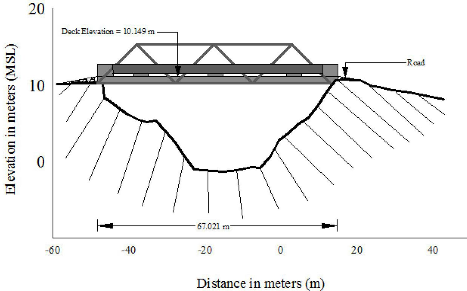
Figure 33. Cagbayang Bridge cross-section diagram
