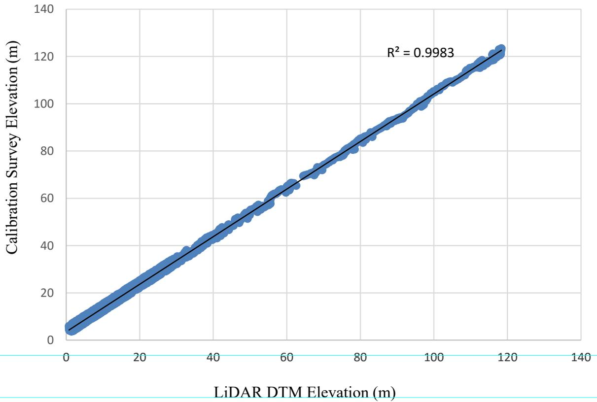
Figure 21. Correlation plot between the calibration survey points and the LiDAR data
