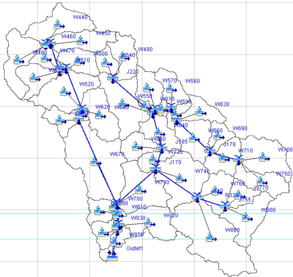
Figure 54. The Jibatang River Basin model generated in HEC-HMS
