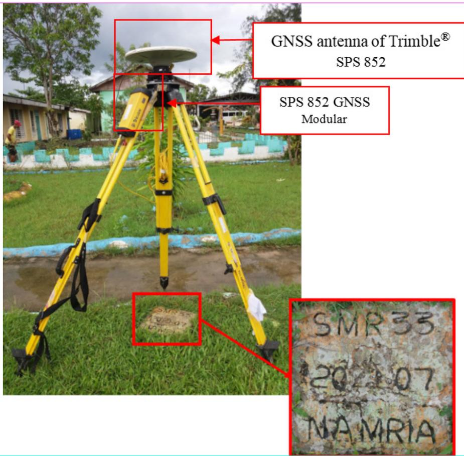
Figure 27. GNSS receiver set-up, Trimble® SPS 852, at SMR-33, inside the compound of Sta. Margarita Elementary School in Barangay Monbon, Municipality of Sta. Margarita, Samar
