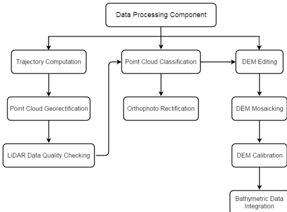
Figure 4. Schematic diagram for the Data Pre-Processing Component
