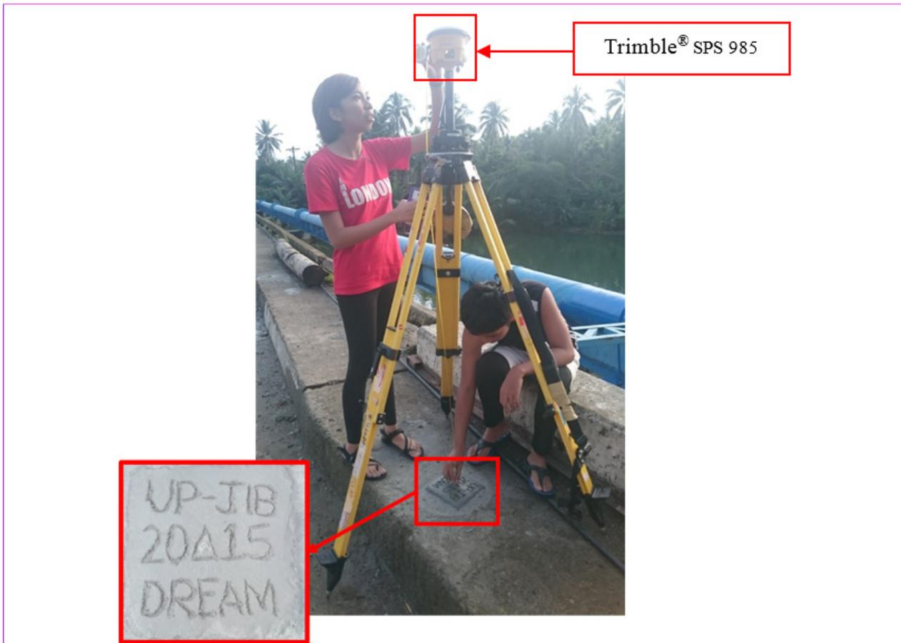
Figure 29. GNSS receiver set-up, Trimble® SPS 985, at UP-JIB, at the Jibatang Bridge approach in Barangay Oquendo, Calbayog City, Samar
