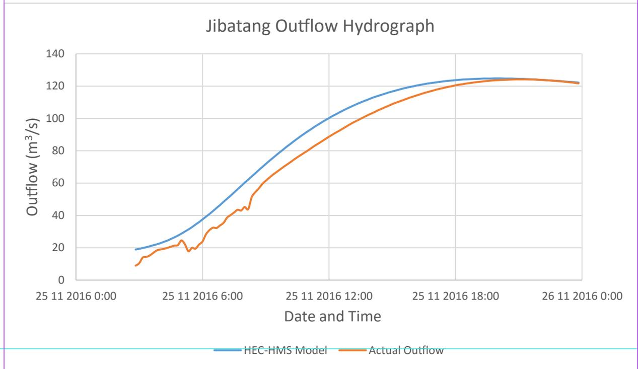
Figure 57. Outflow hydrograph of the Jibatang Bridge generated in HEC-HMS model, compared with observed outflow
