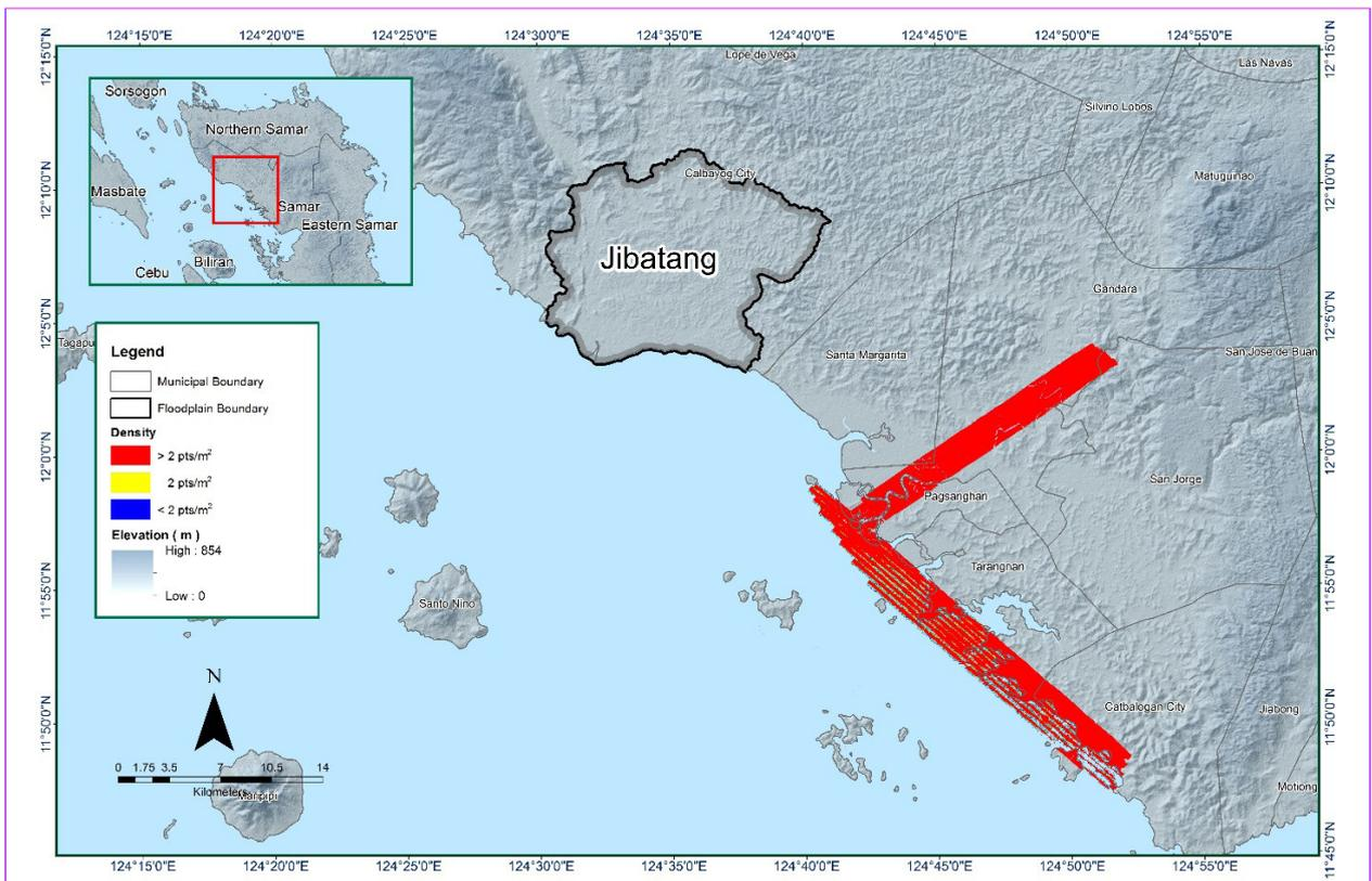
Figure 10. Pulse density map of merged LiDAR data for the Jibatang floodplain
