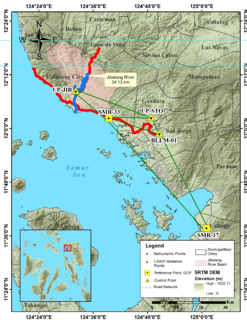
Figure 24. Extent of the bathymetric survey (in blue line) in the Jibatang River and the LiDAR data validation survey (in red)
