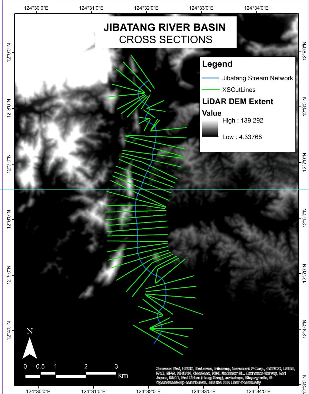
Figure 55. River cross-section of the Jibatang River generated through the ArcMap HEC GeoRAS tool
