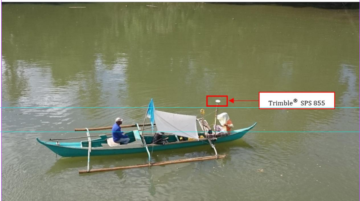
Figure 38. Bathymetric survey using OHMEX™ single beam Echo Sounder along the Jibatang River
