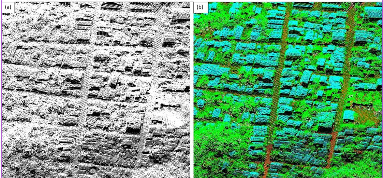
Figure 14. Point cloud (a) before and (b) after classification
