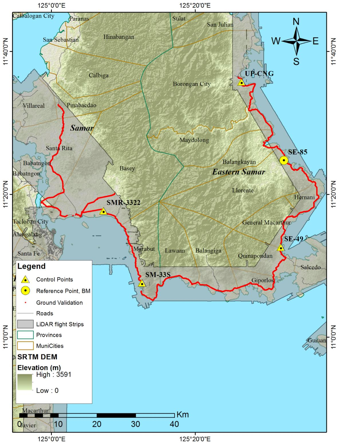
Figure 44. LiDAR ground validation survey along Samar and Eastern Region
