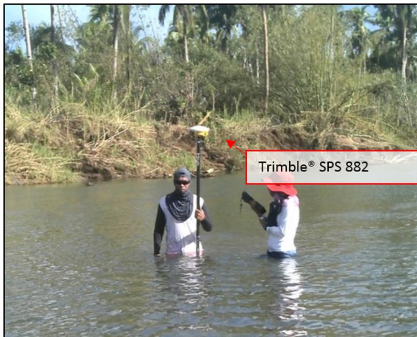
Figure 46. Bathymetric survey in upstream Lorente River
