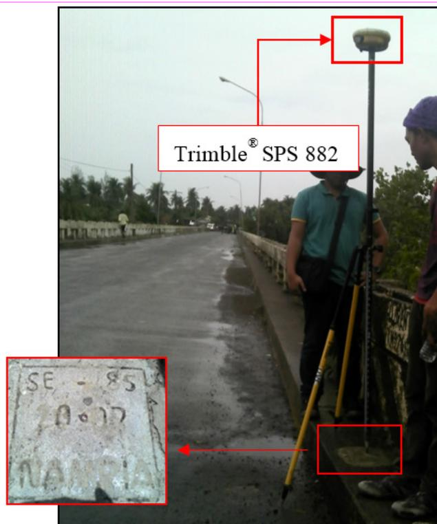
**Figure 33.** GNSS receiver, Trimble® SPS 882, at SE-85, located at the approach of Lorente Bridge in Brgy. 11, Mun. of Lorente, Eastern Samar
