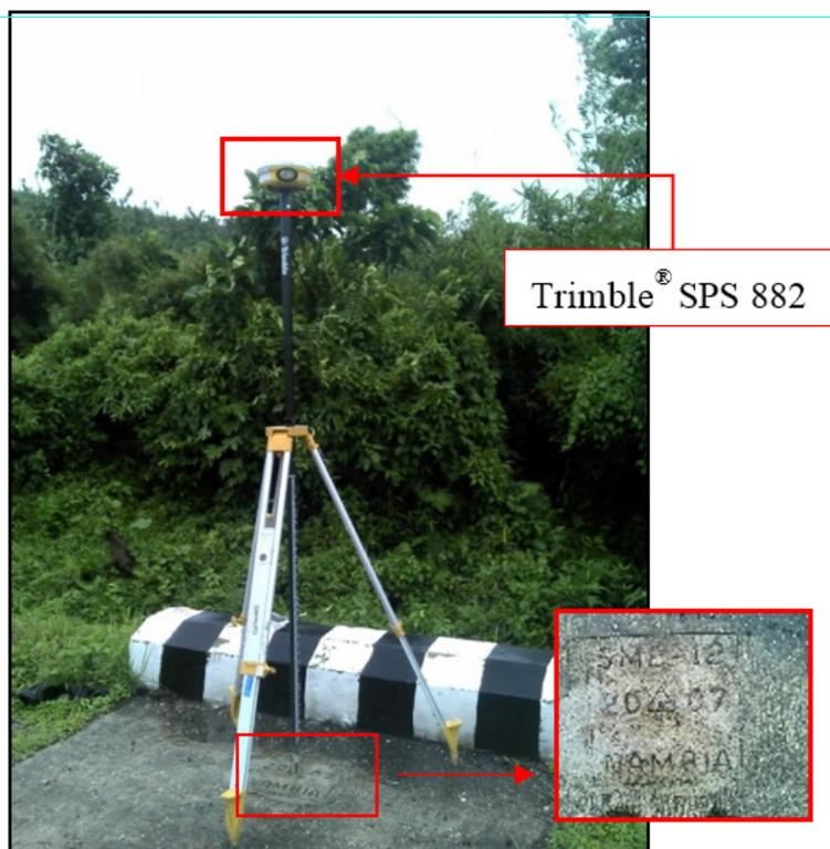
**Figure 34.** GNSS receiver occupation, Trimble® SPS 882, at SME-12 in Brgy. San Miguel, Mun. of Balangiga, Eastern Samar
