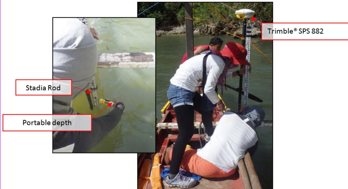
Figure 45. Bathymetric survey using portable depth sounder and stadia rod deployment for depth checking in Lorente River
