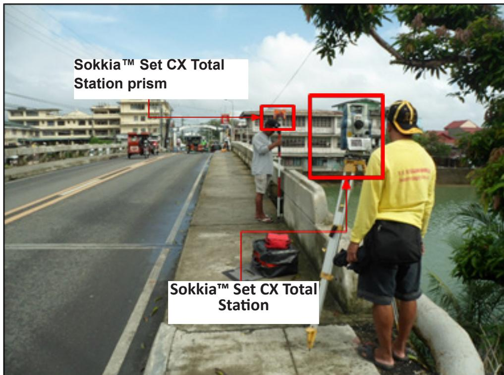
Figure 41. As-built survey of Loom Bridge
