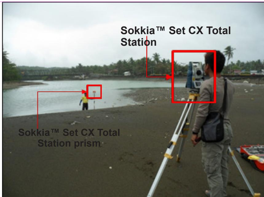
Figure 51. Manual bathymetric survey of HONS along Loom River
