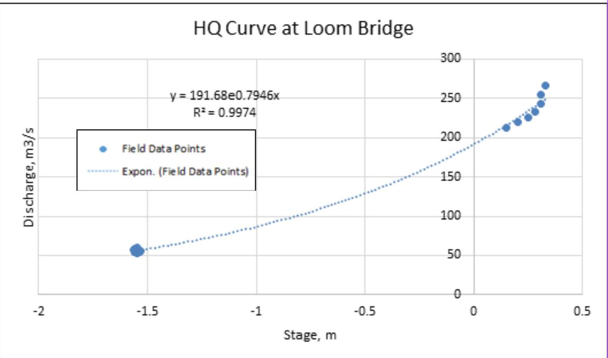
Figure 58. Rating Curve at Loom Bridge, Loom, Samar
