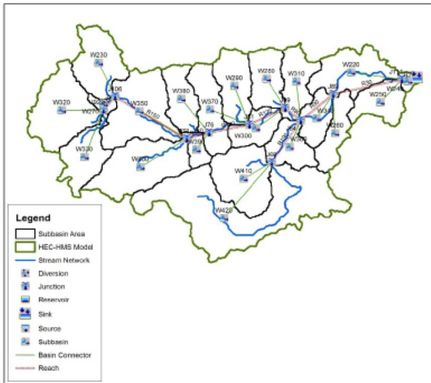
Figure 66. The Loom river basin model generated using HEC-HMS
