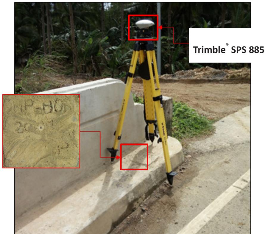
Figure 33. GNSS receiver set up, Trimble® SPS 885, at UP-BOR, located at the approach of a bridge along the National Highway in Brgy. Can-Abong, Borongan City, Eastern Samar.
