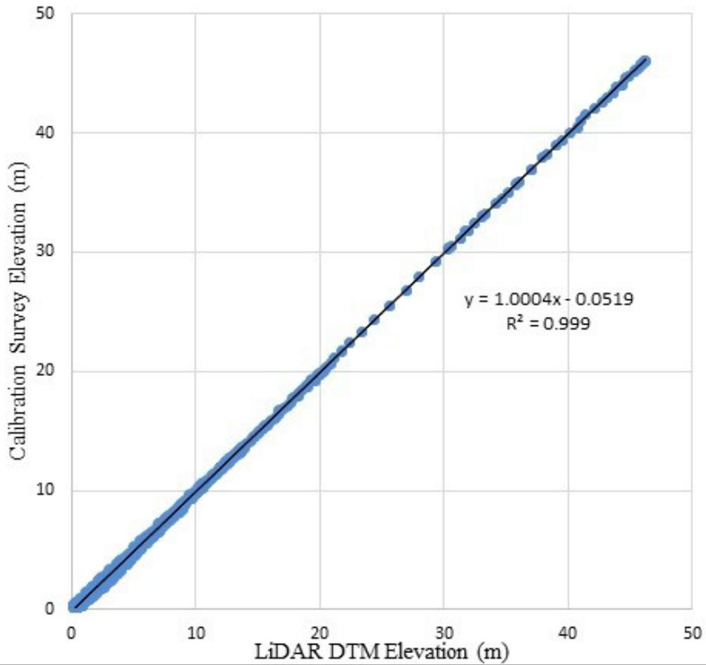
Figure 25. Correlation plot between calibration survey points and LiDAR data.
