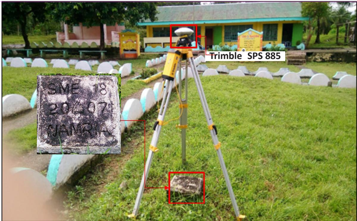
Figure 32. GNSS base set up, Trimble® SPS 885, at SME-18, located 20 m W from the entrance of San Jose Elementary School in Brgy. San Jose, Hernani, Eastern Samar.
