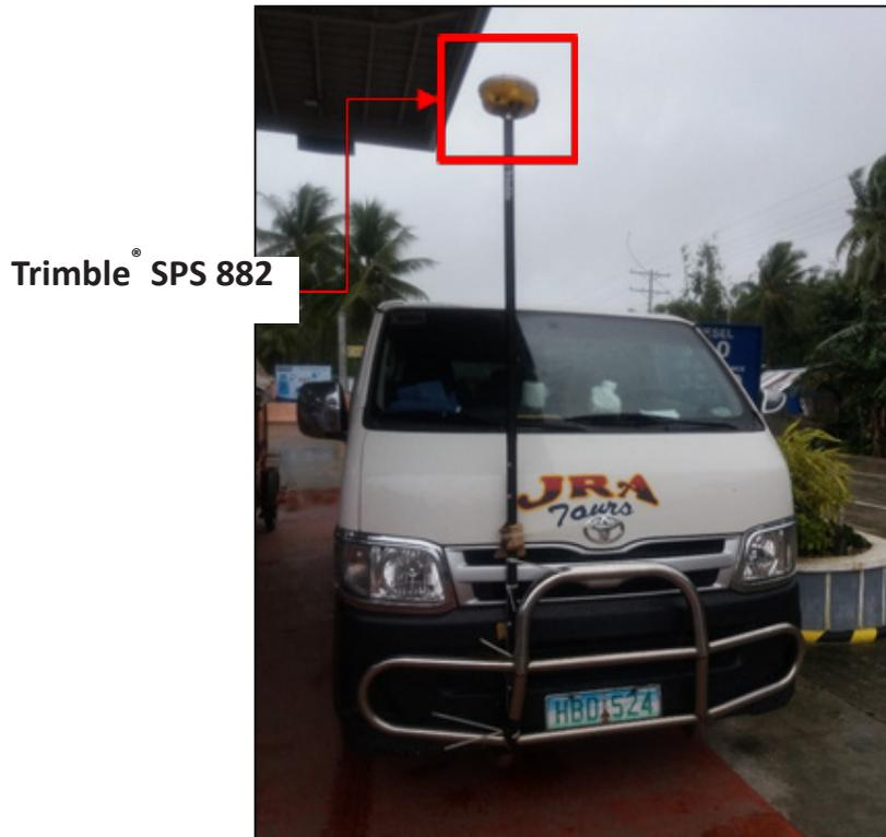
Figure 48. Validation points acquisition survey set-up for Loom River
