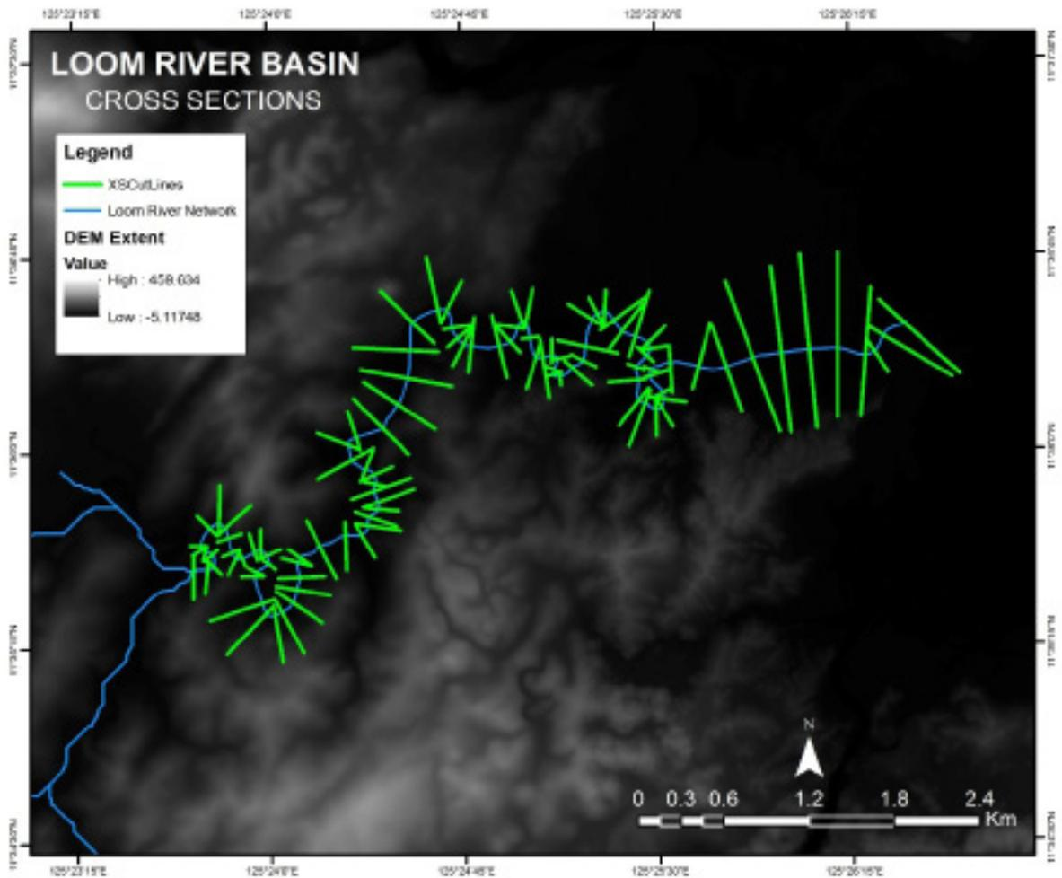
Figure 67. River cross-section of Loom River generated through Arcmap HEC GeoRAS tool
