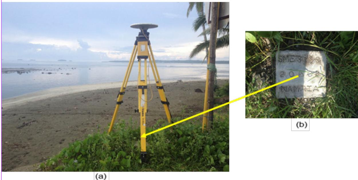
Figure 3. GPS set-up over SME-3139 located along the highway in Brgy. Sto. Nino, Sulat, Eastern Samar (a) and NAMRIA reference point SME-3139 (b) as recovered by the field team.
