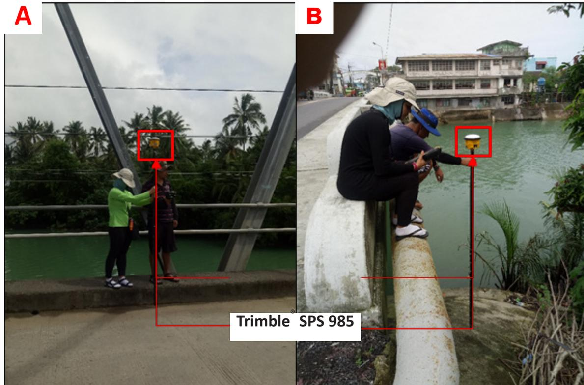
Figure 45. Gathering of random cross-section points along (A) Detour Bridge and (B) Loom Bridge
