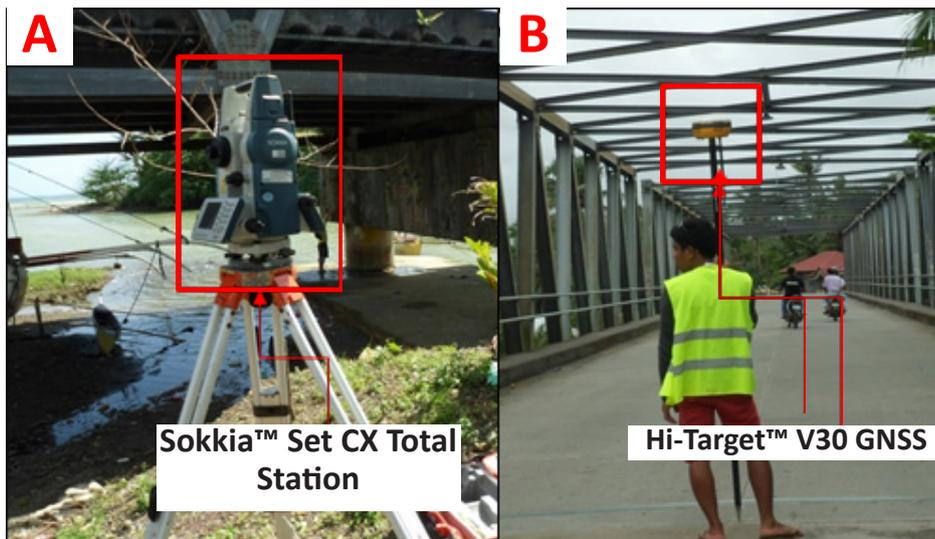
Figure 36. (A) Cross-section and (B) As-built survey of Detour Bridge
