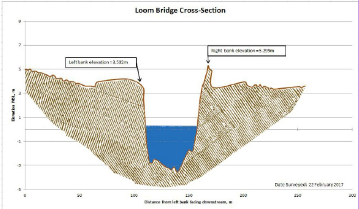
Figure 57. Cross-Section Plot of Loom Bridge
