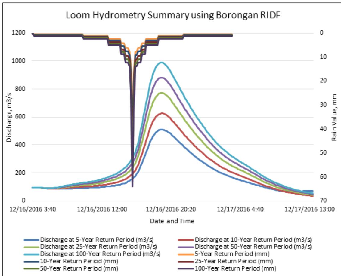
Figure 70. Outflow hydrograph at Loom Station generated using Borongan RIDF simulated in HEC-HMS
