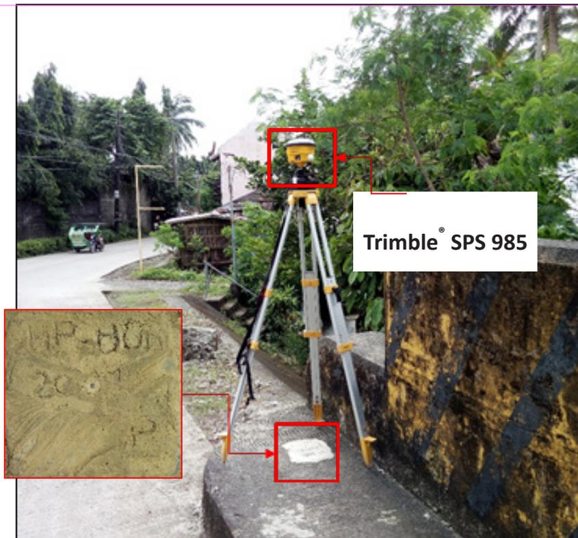
Figure 34. GNSS receiver set up, Trimble® SPS 985, at UP-LOO-1, located at the approach of Detour Bridge in Brgy. Alang-alang, Borongan City, Eastern Samar.
