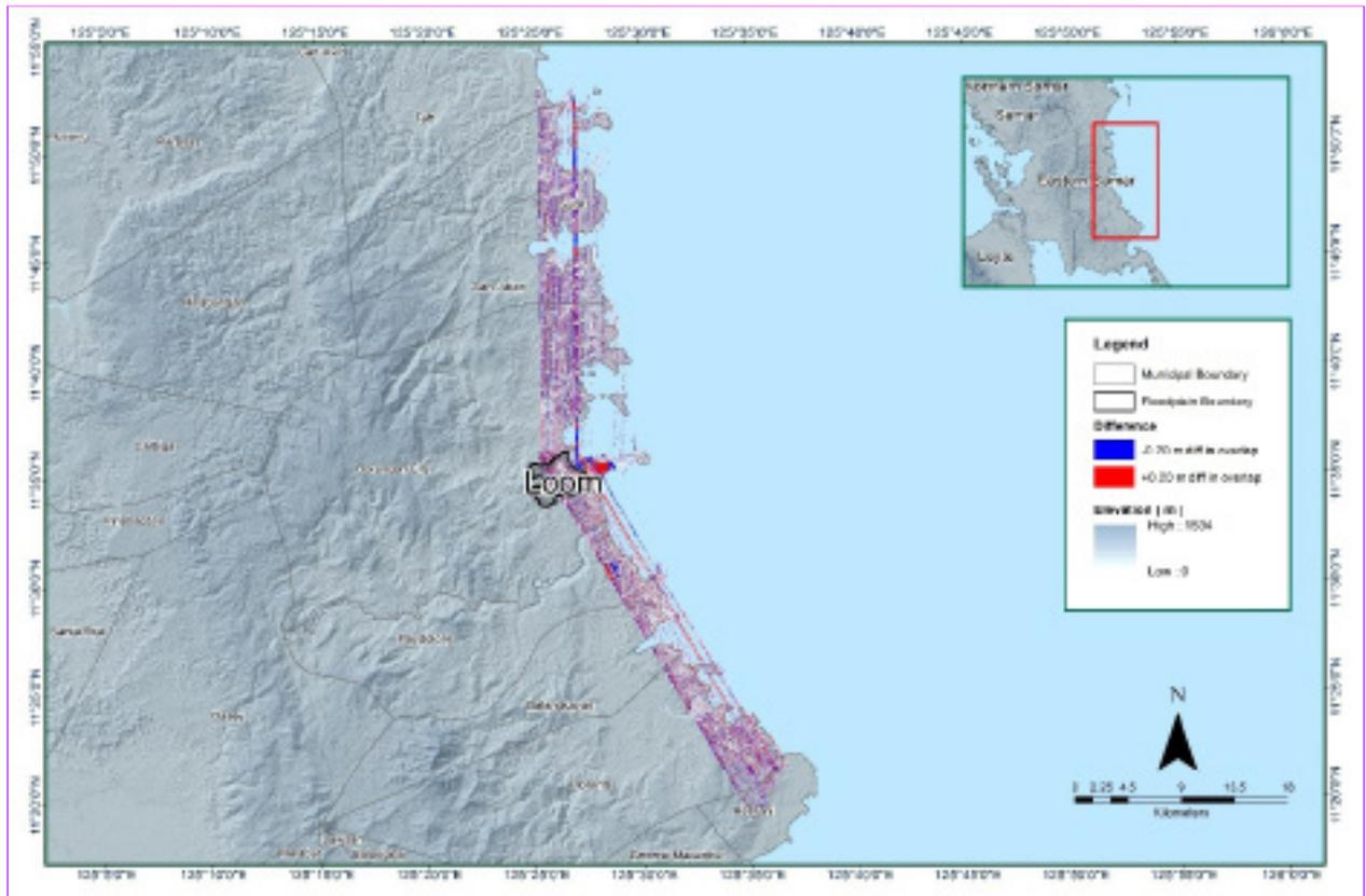
Figure 15. Elevation difference map between flight lines for Loom floodplain.
