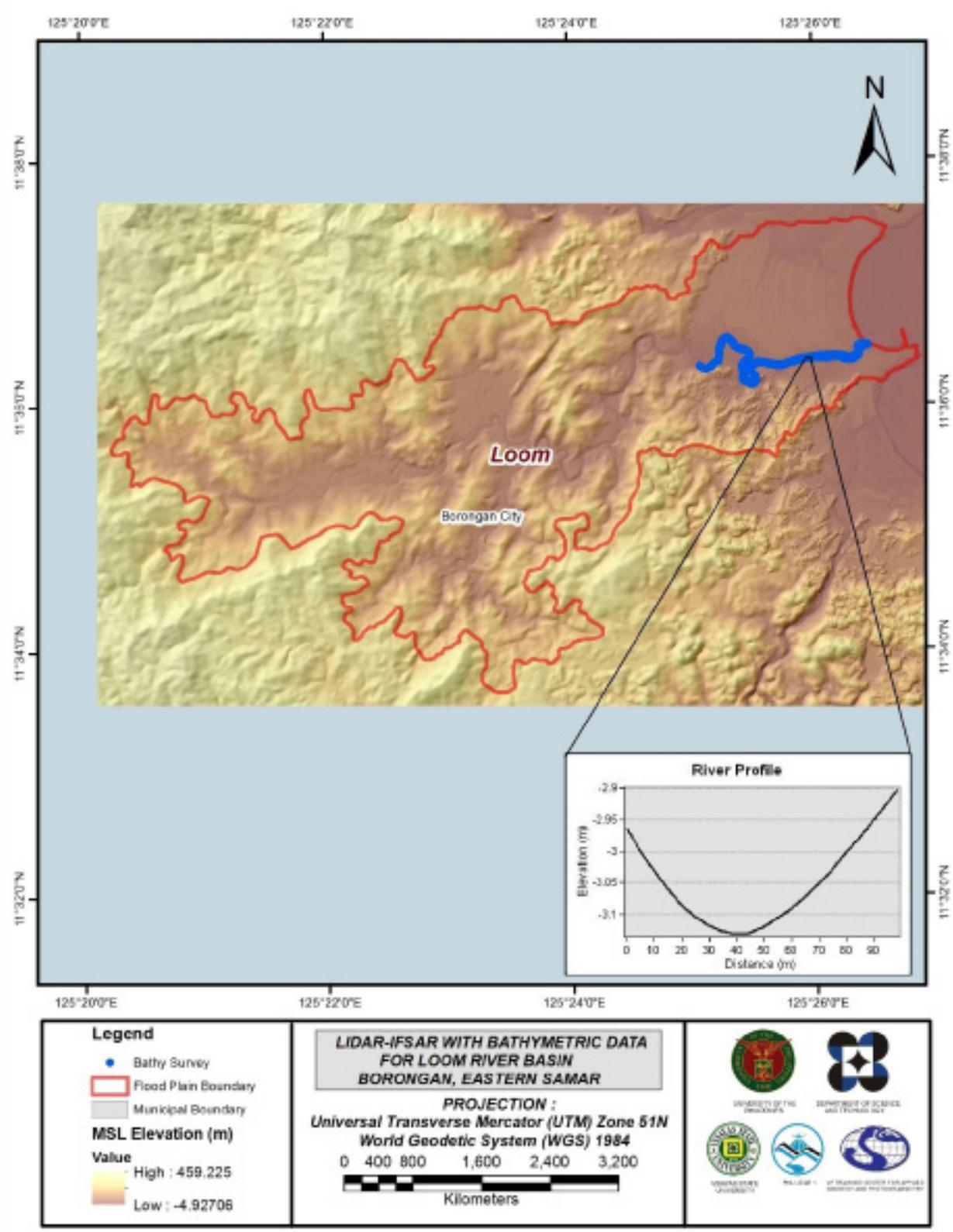
Figure 27. Map of Loom Flood Plain with bathymetric survey points shown in blue.
