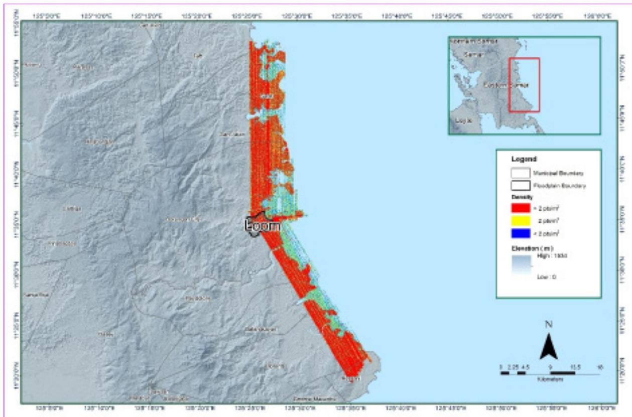
Figure 14. Density map of merged LiDAR data for Loom floodplain.
