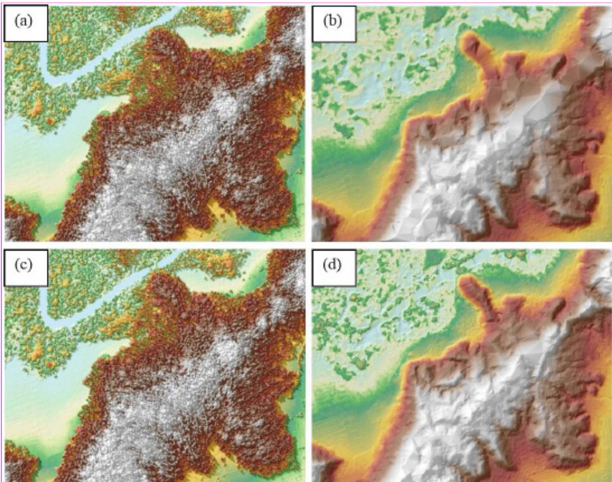
Figure 19. The production of last return DSM (a) and DTM (b), first return DSM (c) and secondary DTM (d) in some portion of Loom Floodplain.
