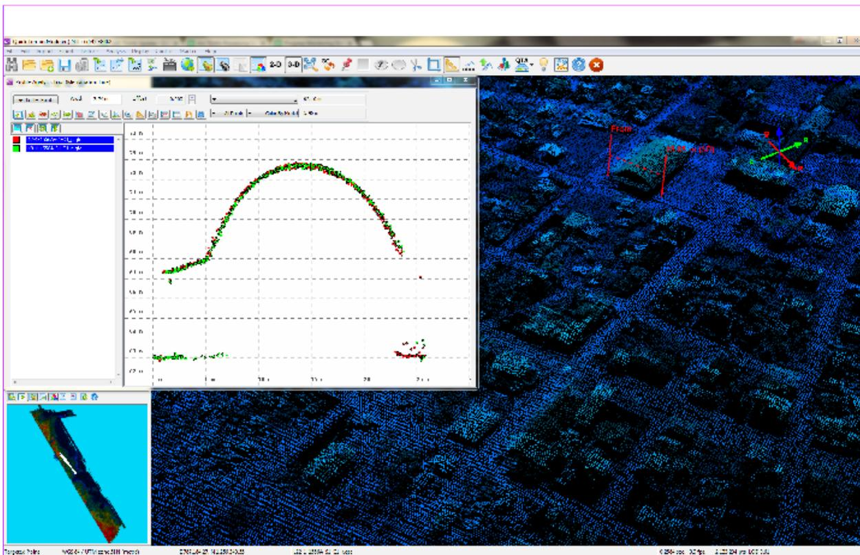
Figure 16. Quality checking for Loom flight 1556A using the Profile Tool of QT Modeler.
