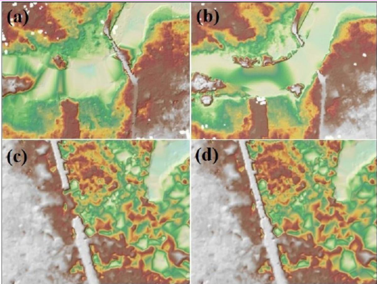
Figure 22. Portions in the DTM of Loom floodplain – a bridge before (a) and after (b) manual editing; and a road before (c) and after (d) data retrieval.
