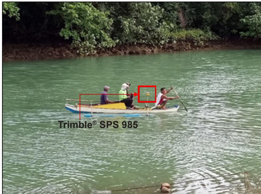
Figure 52. Gathering of random bathymetric points along Loom River
