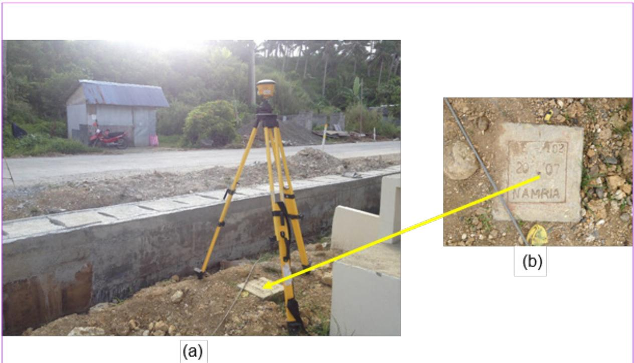
Figure 6. GPS set-up over SE-102 located along the National Highway, in front of Maydolong High School, in Maydolong, Eastern Samar (a) and NAMRIA reference point SE-102 (b) as recovered by the field team.
