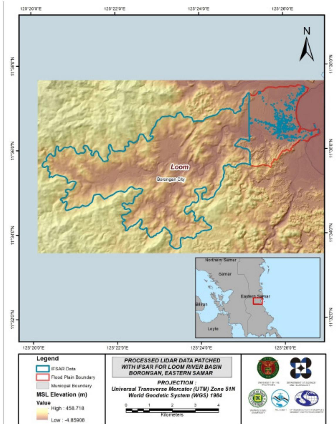
Figure 23. Map of Processed LiDAR Data for Loom Floodplain
