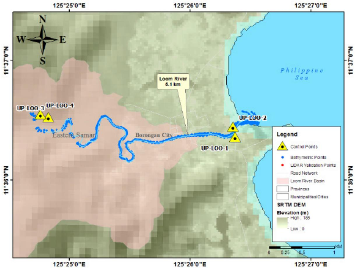
Figure 53. Bathymetric survey of Loom River
