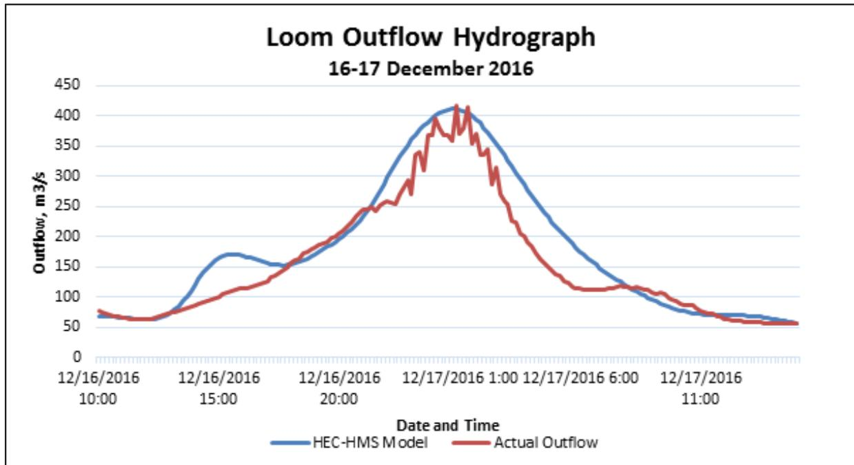
Figure 69. Outflow Hydrograph of Loom produced by the HEC-HMS model compared with observed outflow
