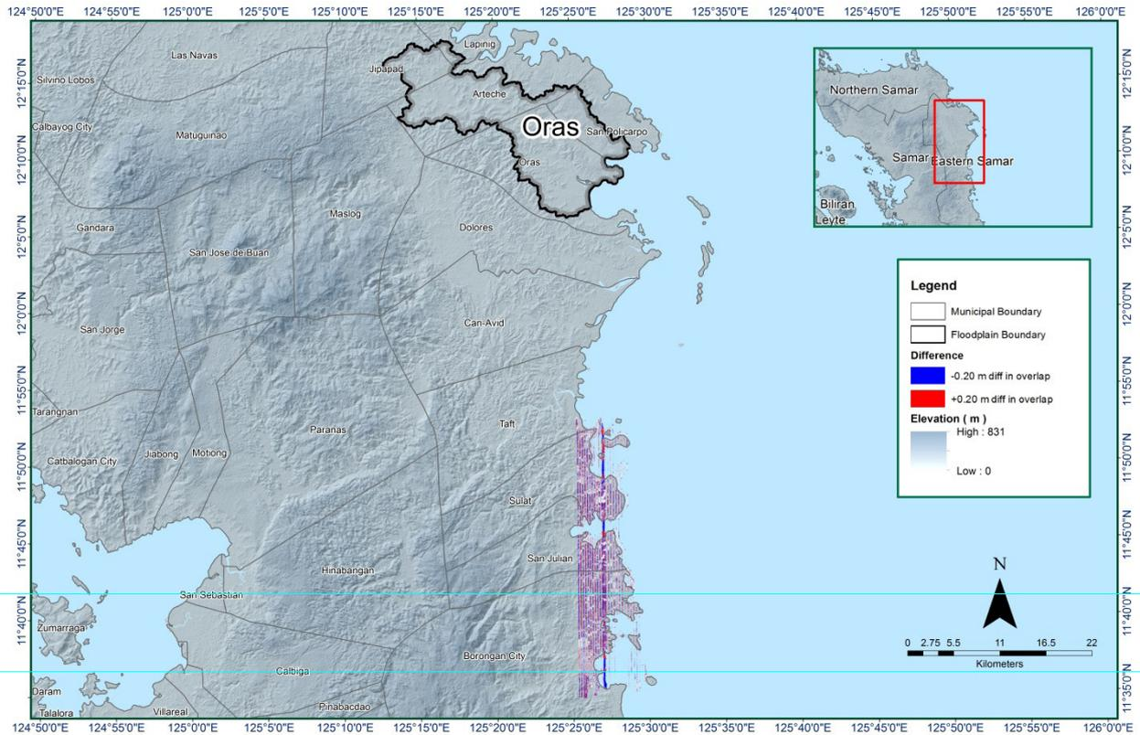
Figure 11. Elevation difference map between flight lines for Oras floodplain.
