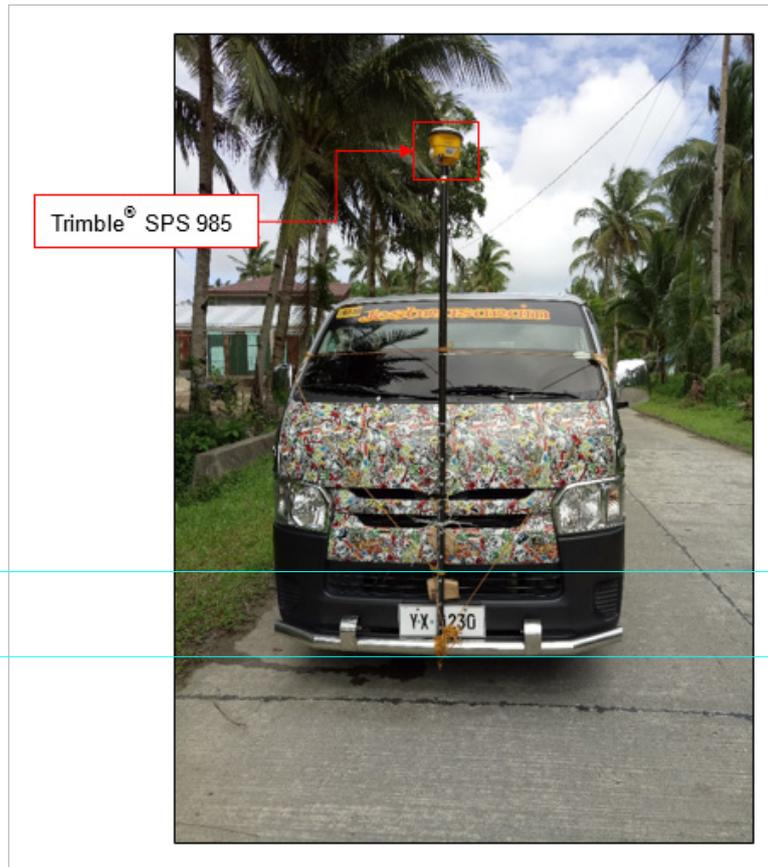
Figure 39. Validation points acquisition survey set-up for Oras River.
