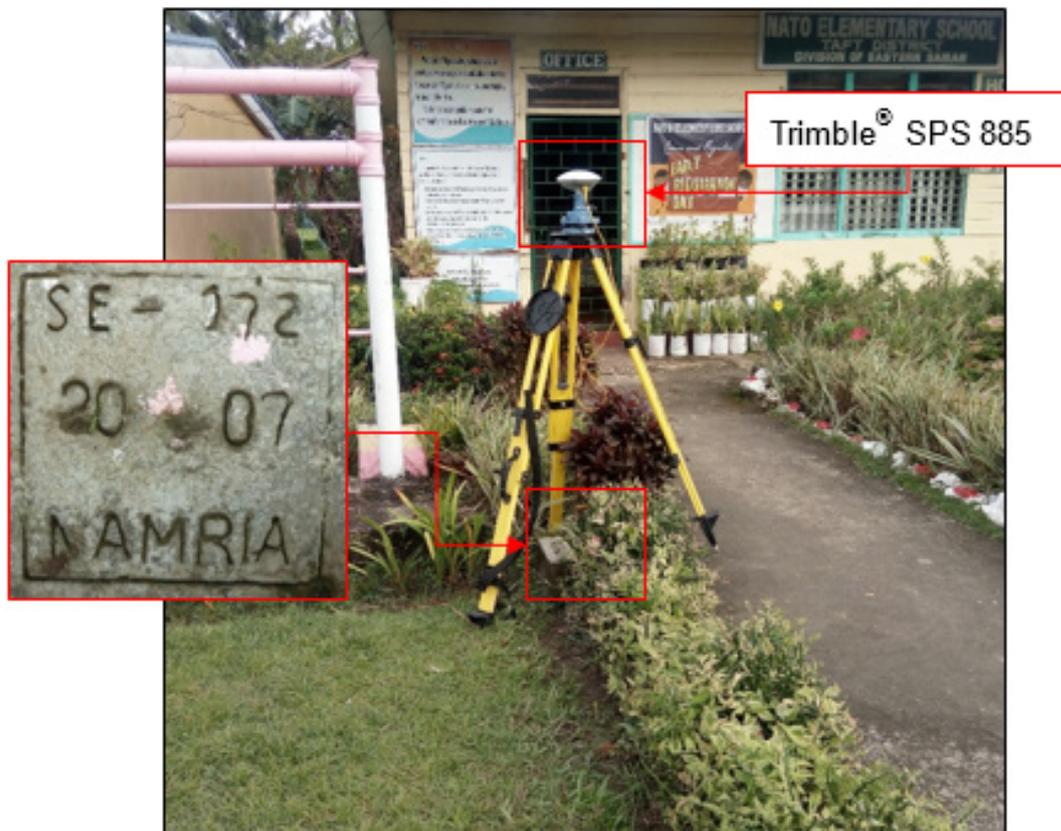
Figure 29. GNSS receiver set up, Trimble® SPS 885, at SE-172, located beside the walkway leading to the office of Nato Elementary School in Brgy. Nato, Taft, Eastern Samar
