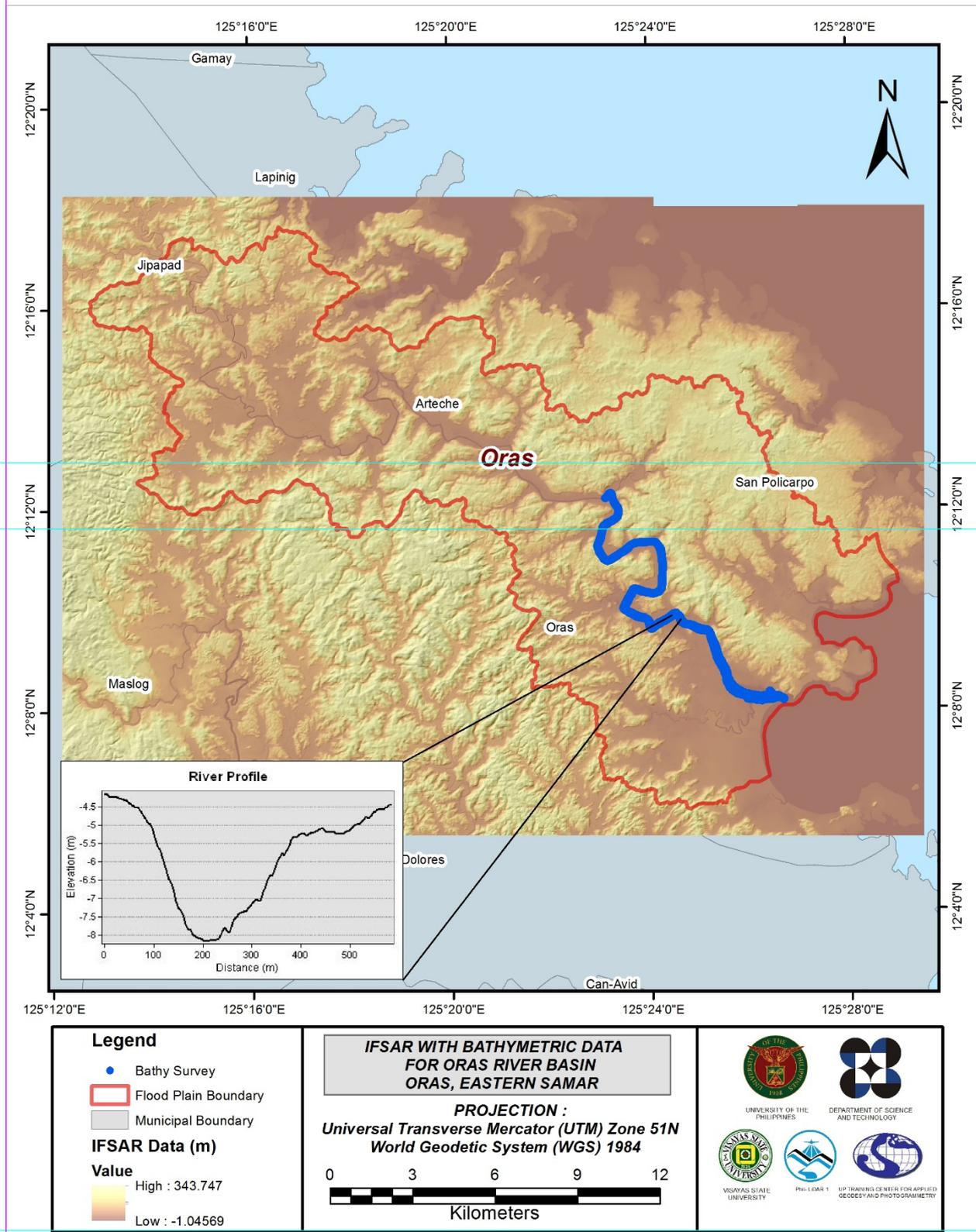
Figure 23. Map of Oras Flood Plain with bathymetric survey points shown in blue.
