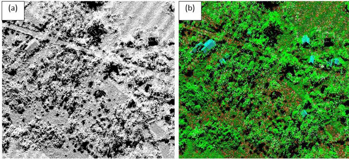
Figure 14. Point cloud before (a) and after (b) classification.
