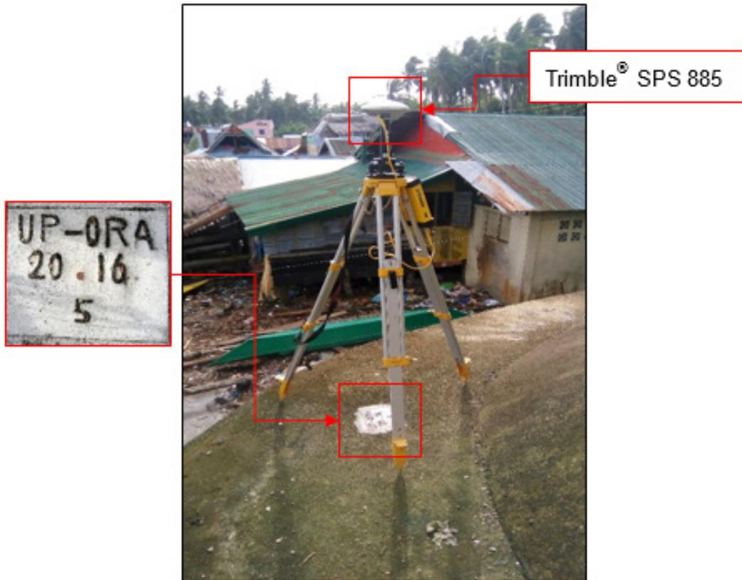
Figure 30. GNSS receiver set up, Trimble® SPS 885, at UP-ORA-5, located at the top of bridge abutment in Brgy. Tawagan, Oras, Eastern Samar
