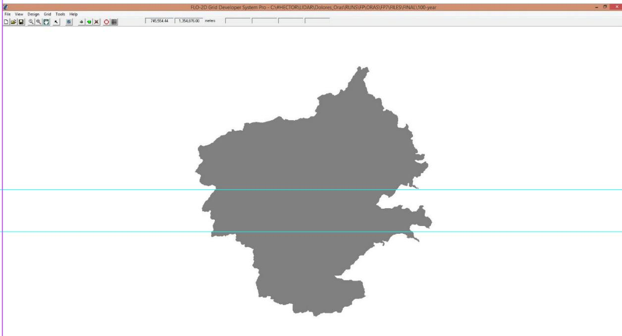
Figure 58. Screenshot of subcatchment with the computational area to be modeled in FLO-2D GDS Pro
