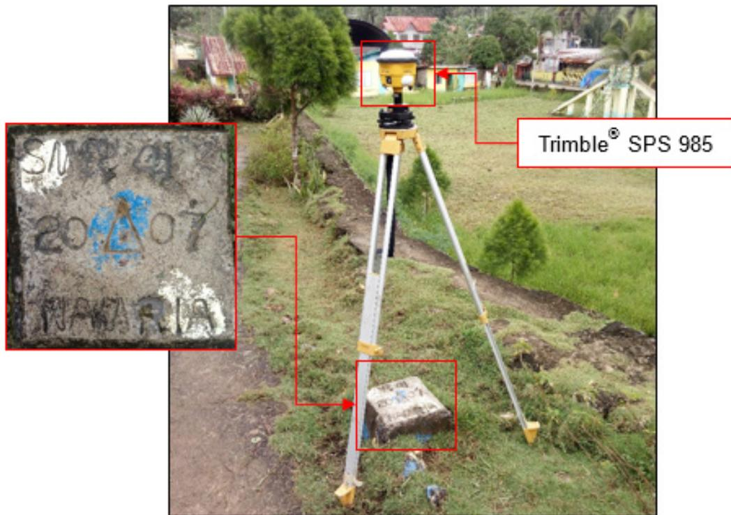
Figure 28. GNSS base set up, Trimble® SPS 985, at SMR-41, located 20 m SW from the flagpole in Bagacay Elementary School playground in Brgy. Bagacay, Hinabangan, Eastern Samar
