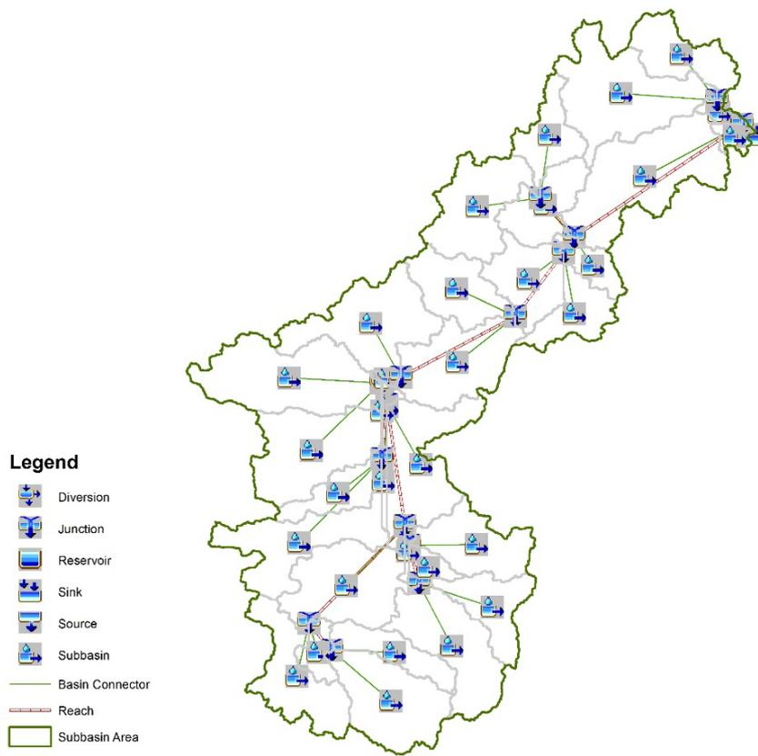
Figure 56. The Oras Hydrologic Model generated in HEC-GeoHMS
