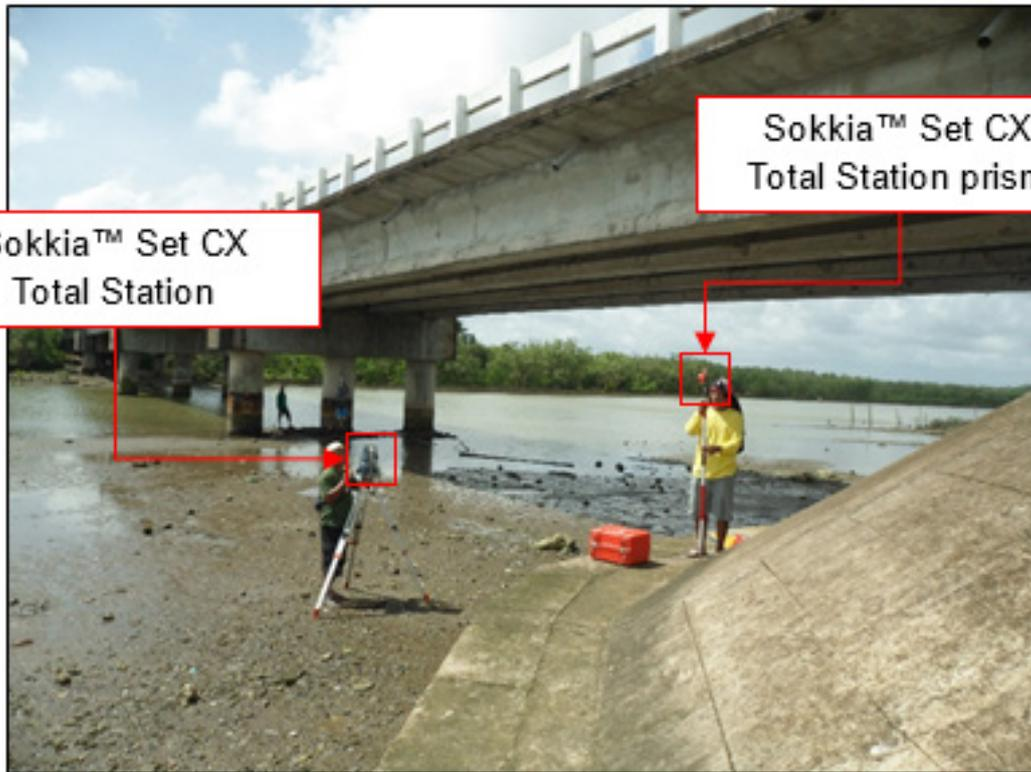
Figure 32. As-built survey of Oras Bridge
