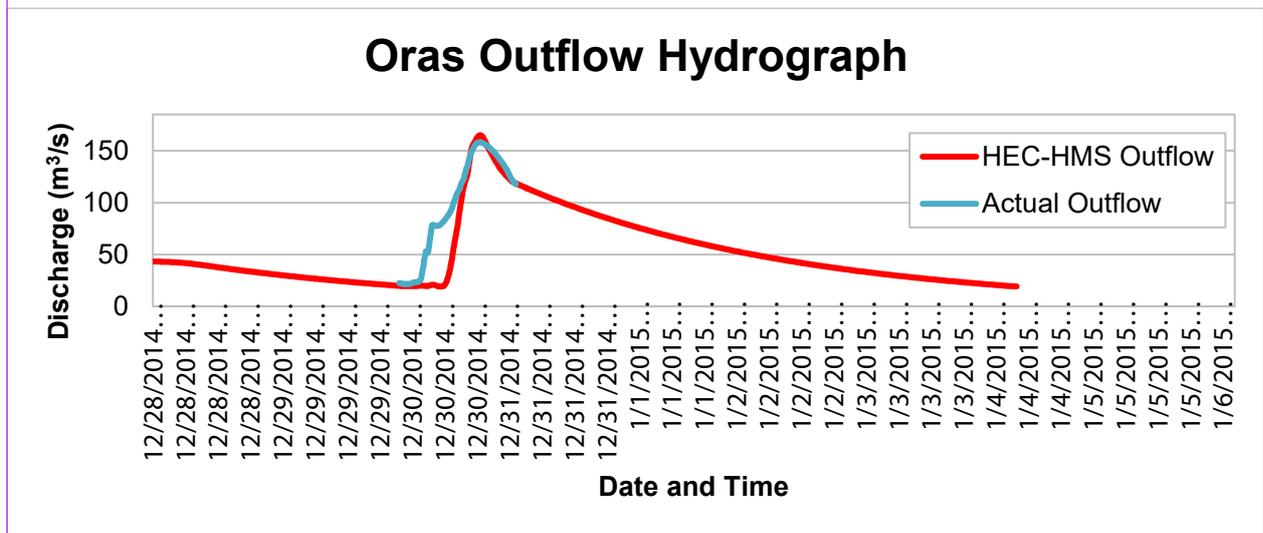
Figure 59. Outflow Hydrograph of Oras Bridge generated in HEC-HMS model compared with observed outflow
