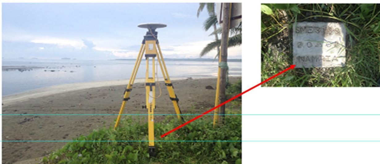
Figure 2. GPS set-up over SME-3139 located along the highway in Brgy. Sto. Nino, Oras, Eastern Samar (a) and NAMRIA reference point SME-3139 (b) as recovered by the field team.
