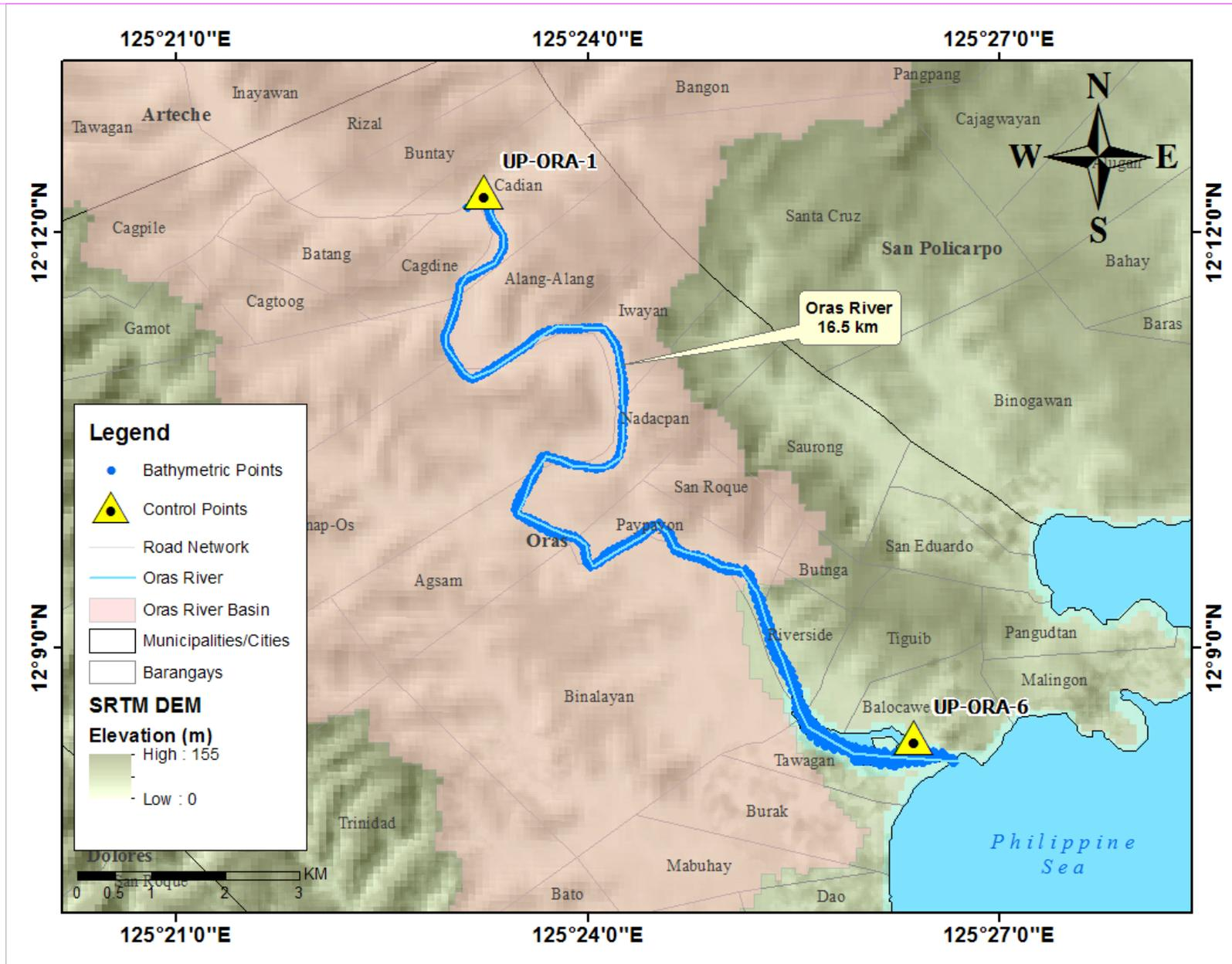
Figure 43. Bathymetric survey of Oras River
