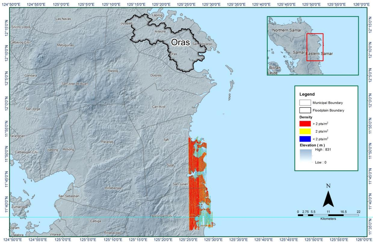
Figure 10. Density map of merged LiDAR data for Oras floodplain.
