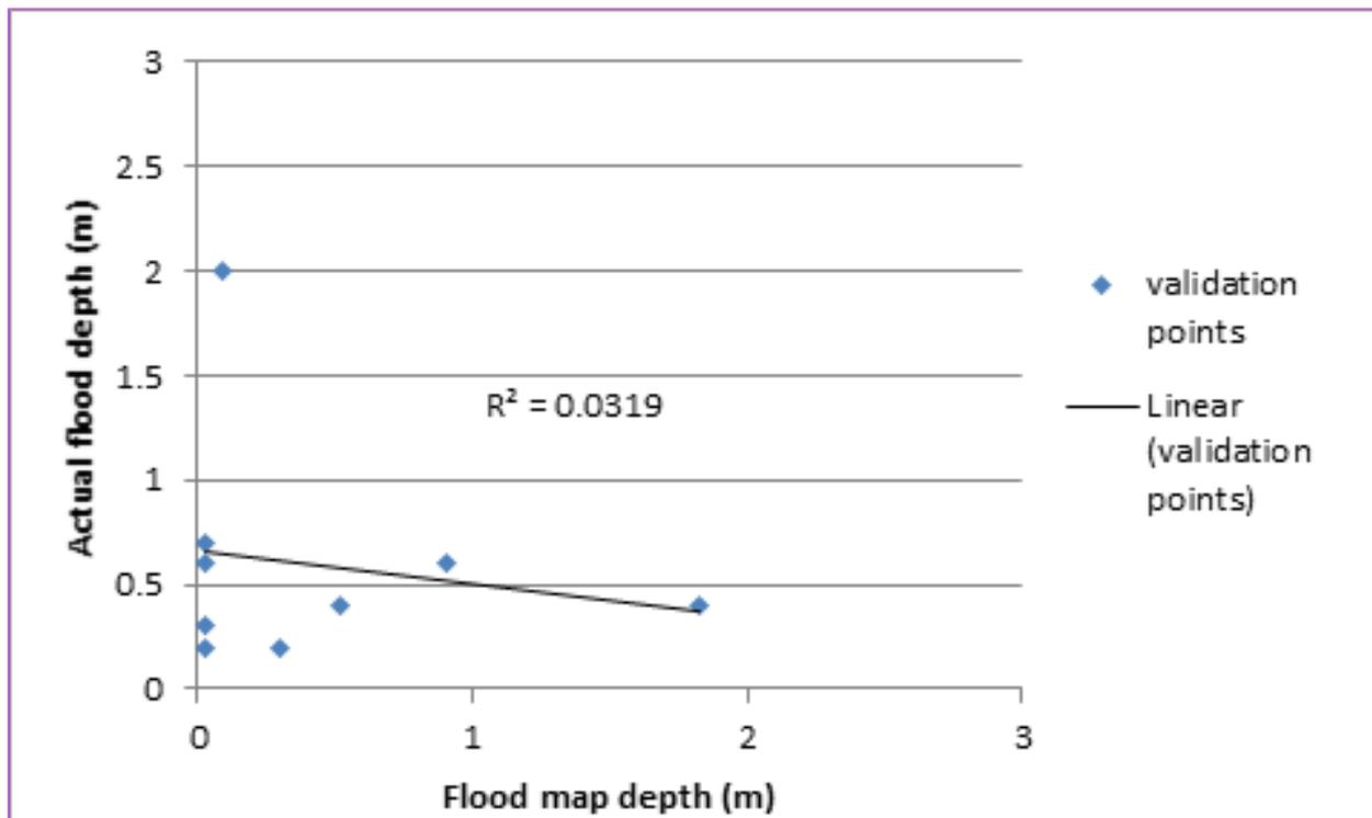
Figure 78. Flood map depth vs. actual flood depth for 100-year RP validation
