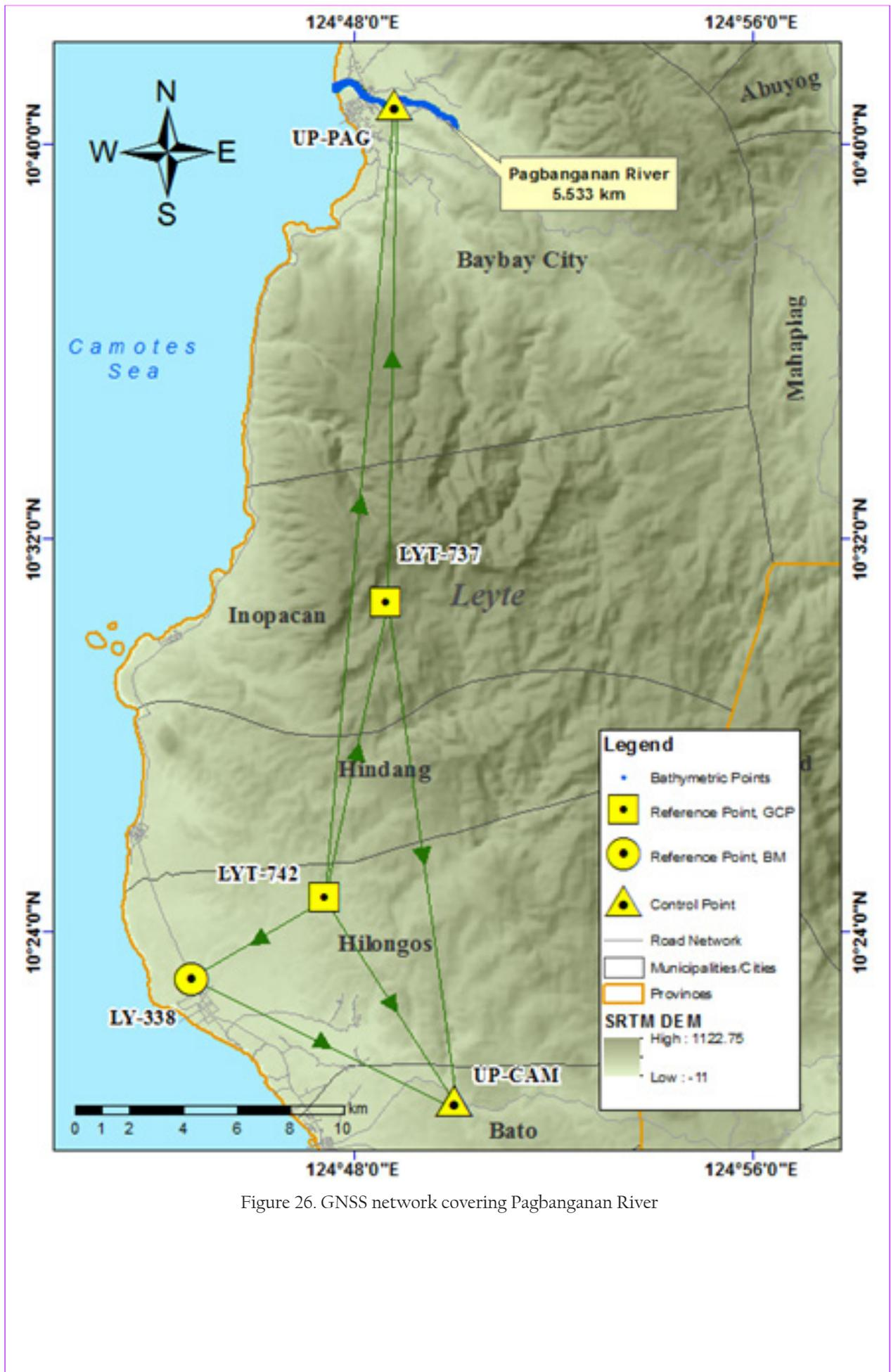
Figure 26. GNSS network covering Pagbanganan River
