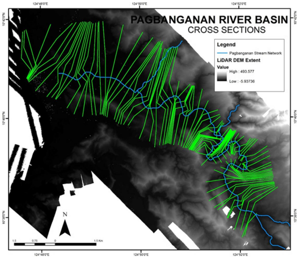
Figure 53. River cross-section of Pagbanganan River generated through Arcmap HEC GeoRAS tool
