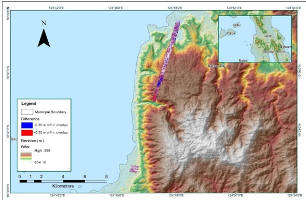
Elevation difference between flight lines
