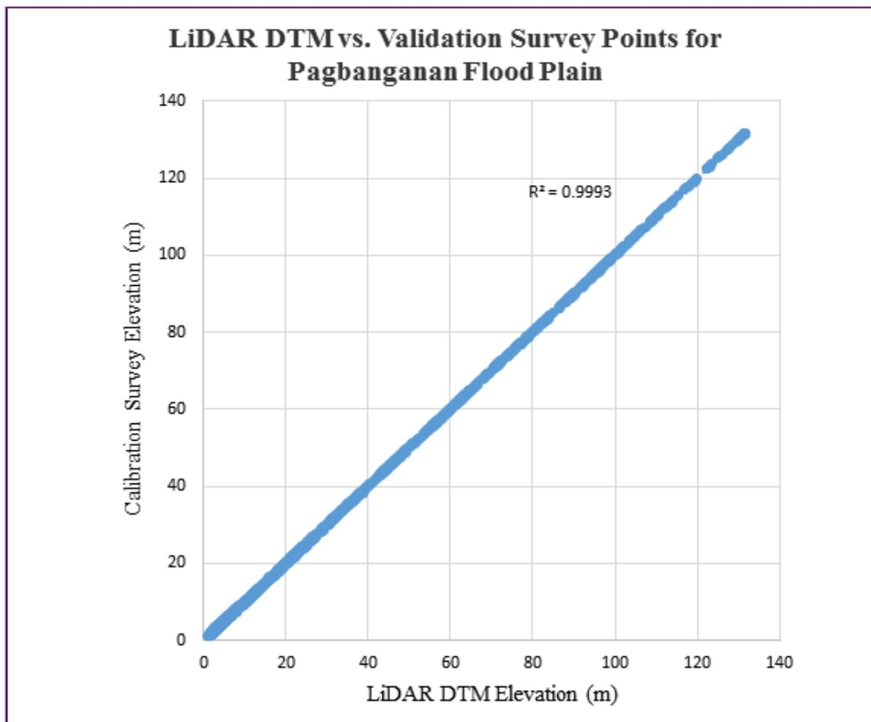
Figure 21. Correlation plot between validation survey points and LiDAR data
