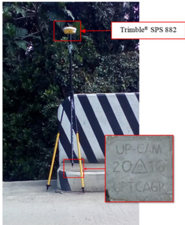
Figure 30. GNSS receiver set-up, Trimble® SPS 882, at UP-CAM, located at the approach of Cambanog Bridge in Brgy. Naga, Municipality of Bato, Leyte
