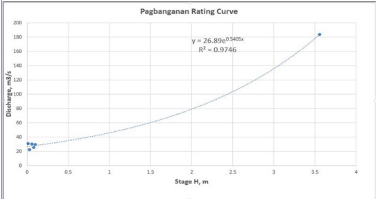
Figure 44. Rating curve at Dungcaan Bridge
