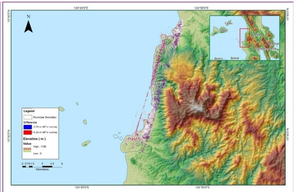
Elevation difference between flight lines
