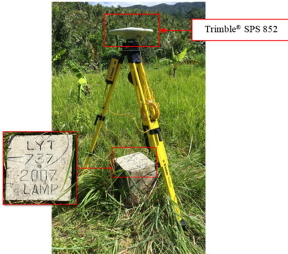
Figure 27. GNSS base set-up, Trimble® SPS 852, at LYT-737, located at the back of Cabulisan Elementary School in Brgy. Cabulisan, Municipality of Inopacan, Leyte
