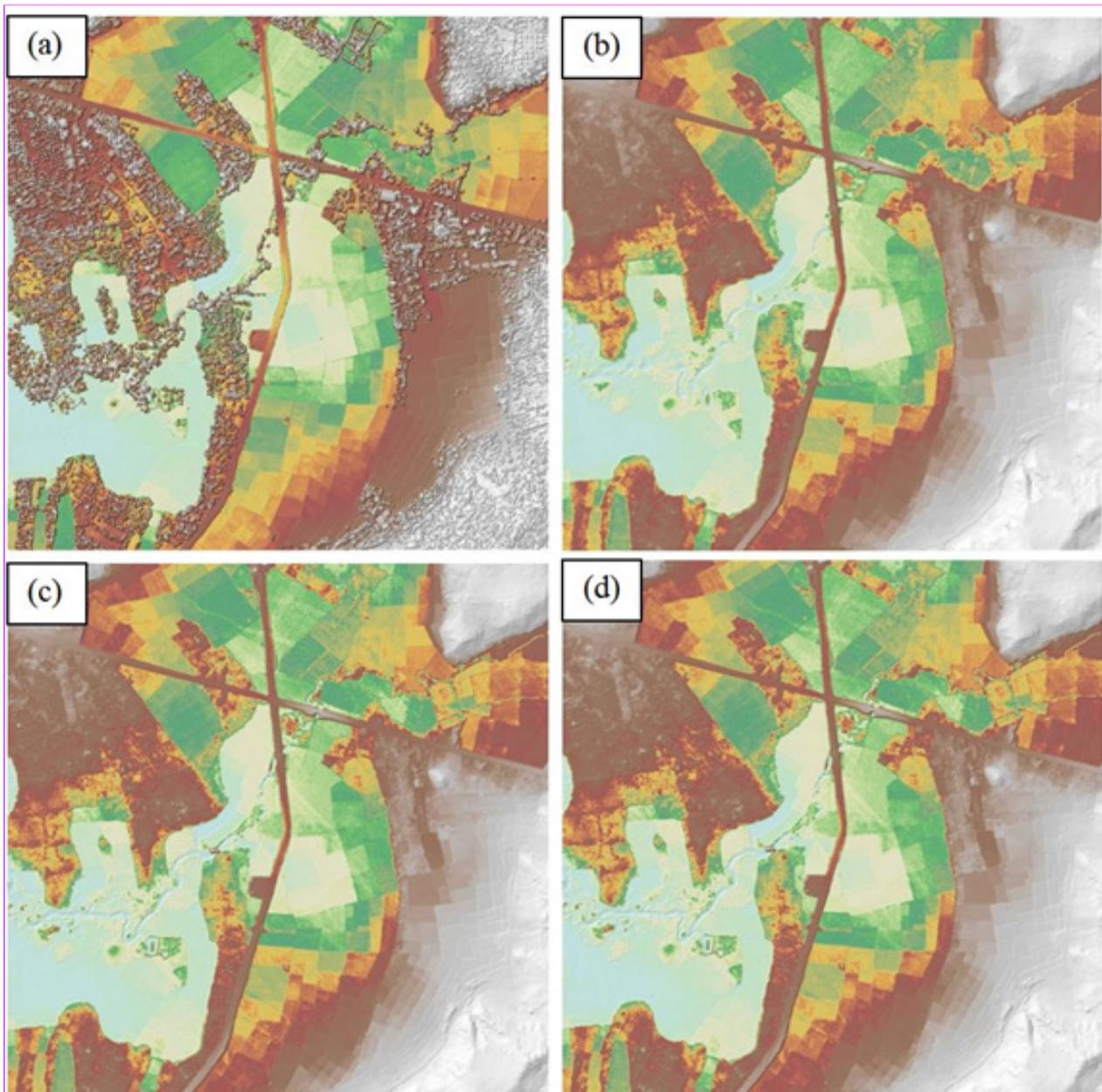
Figure 16. The production of last return DSM (a) and DTM (b), first return DSM (c) and secondary DTM (d) in some portion of Pagbanganan Floodplain.
