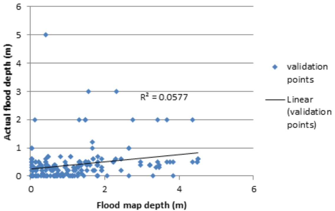
Figure 76. Flood map depth vs. actual flood depth for 5-year RP validation
