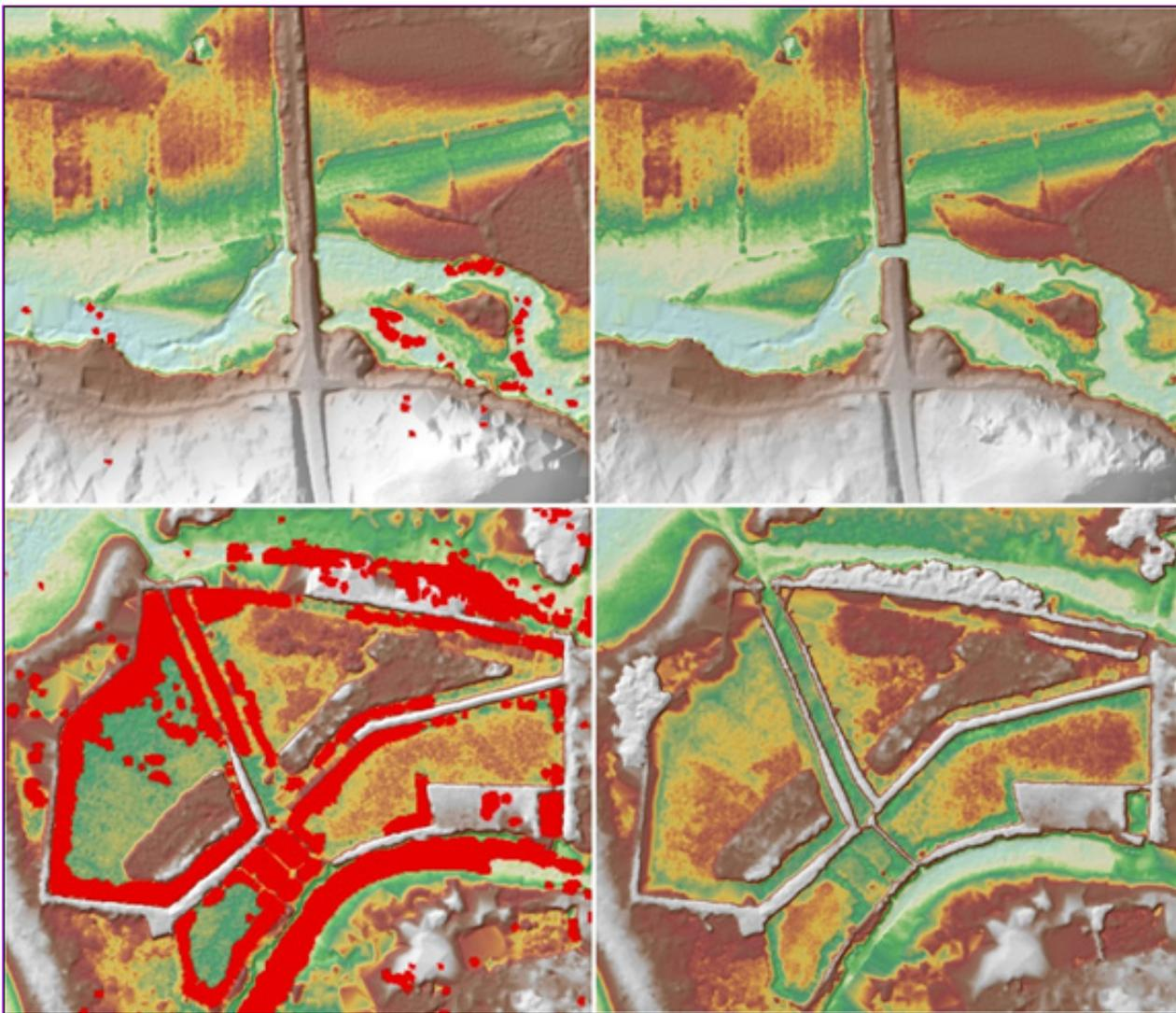
Figure 17. Portions in the DTM of Pagbanganan flood plain—a bridge before (a) and after (b) manual editing; and a fishpond before (c) and after (d) data retrieval and interpolation
