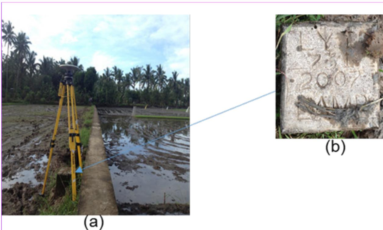
Figure 3. GPS set-up over LYT-731 in Brgy. Kansungka, Baybay City, Leyte (a) and NAMRIA reference point LYT-731(b) as recovered by the field team
