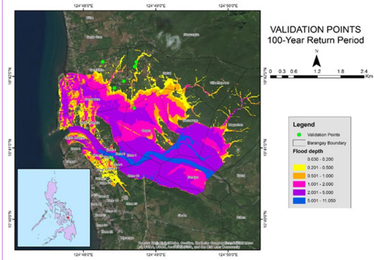
Figure 75. Validation points for 100-year flood depth map of Pagbanganan Floodplain
