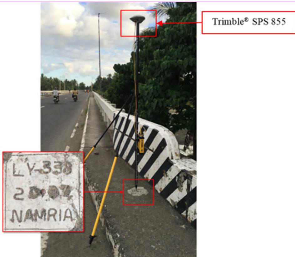
Figure 29. GNSS receiver set-up, Trimble® SPS 855, at LY-338, located at the approach of Salug Birdge along Sta. Indang-Hilongos Road in Brgy. San Juan, Municipality of Hilongos, Leyte
