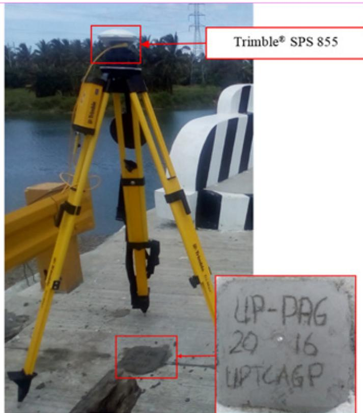
Figure 31. GNSS receiver set-up, Trimble® SPS 855, at UP-PAG, located at Pagbanganan Bridge approach in Brgy. Poblacion Zone 12, City of Baybay, Leyte
