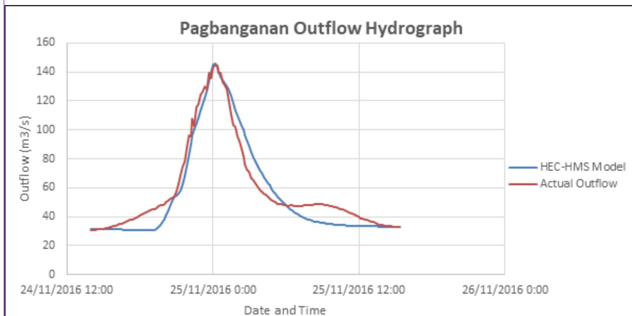
Figure 55. Outflow hydrograph of Pagbanganan produced by the HEC-HMS model compared with observed outflow
