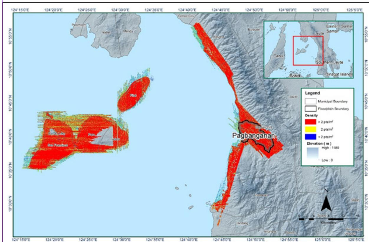
Figure 11. Pulse density map of merged LiDAR data for Pagbanganan Floodplain
