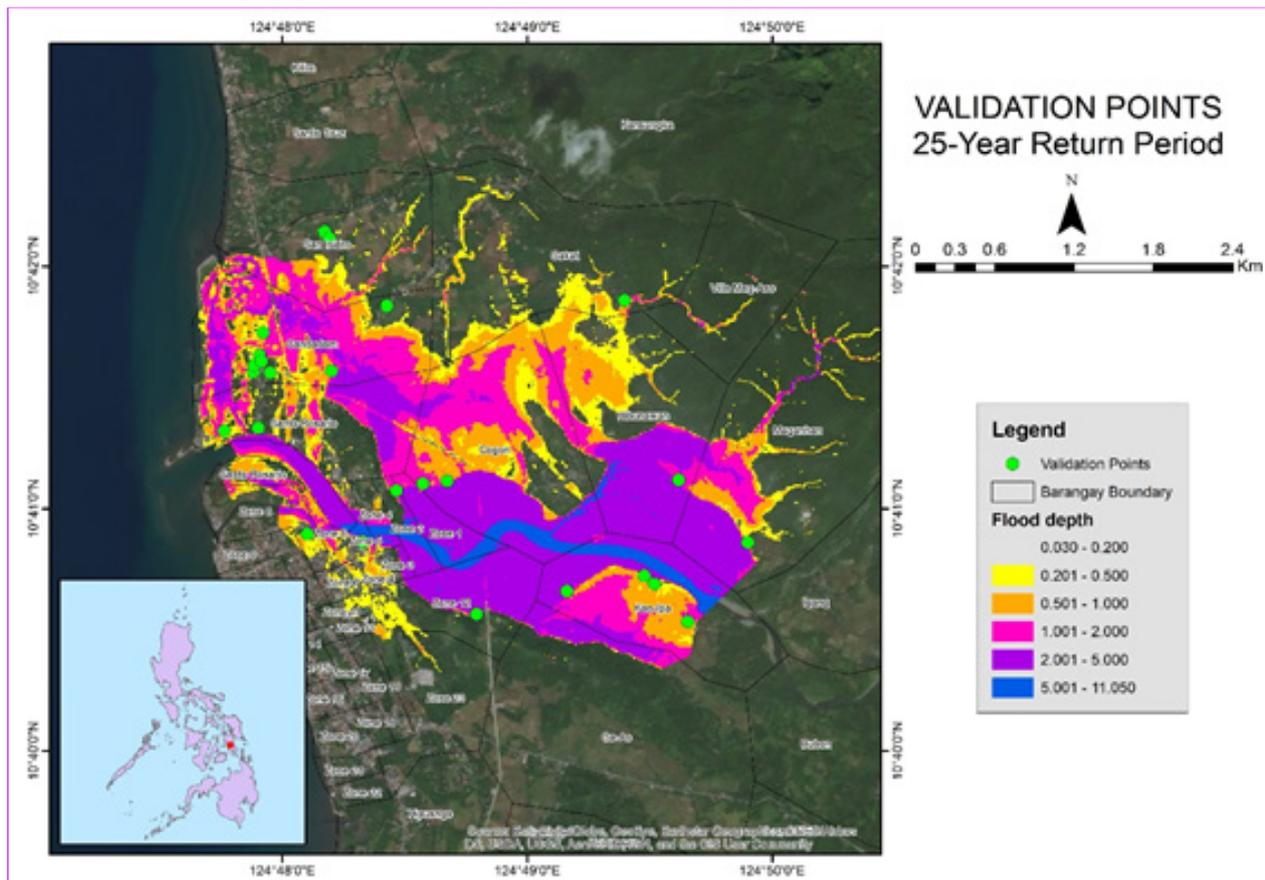
Figure 74. Validation points for 25-year flood depth map of Pagbanganan Floodplain
