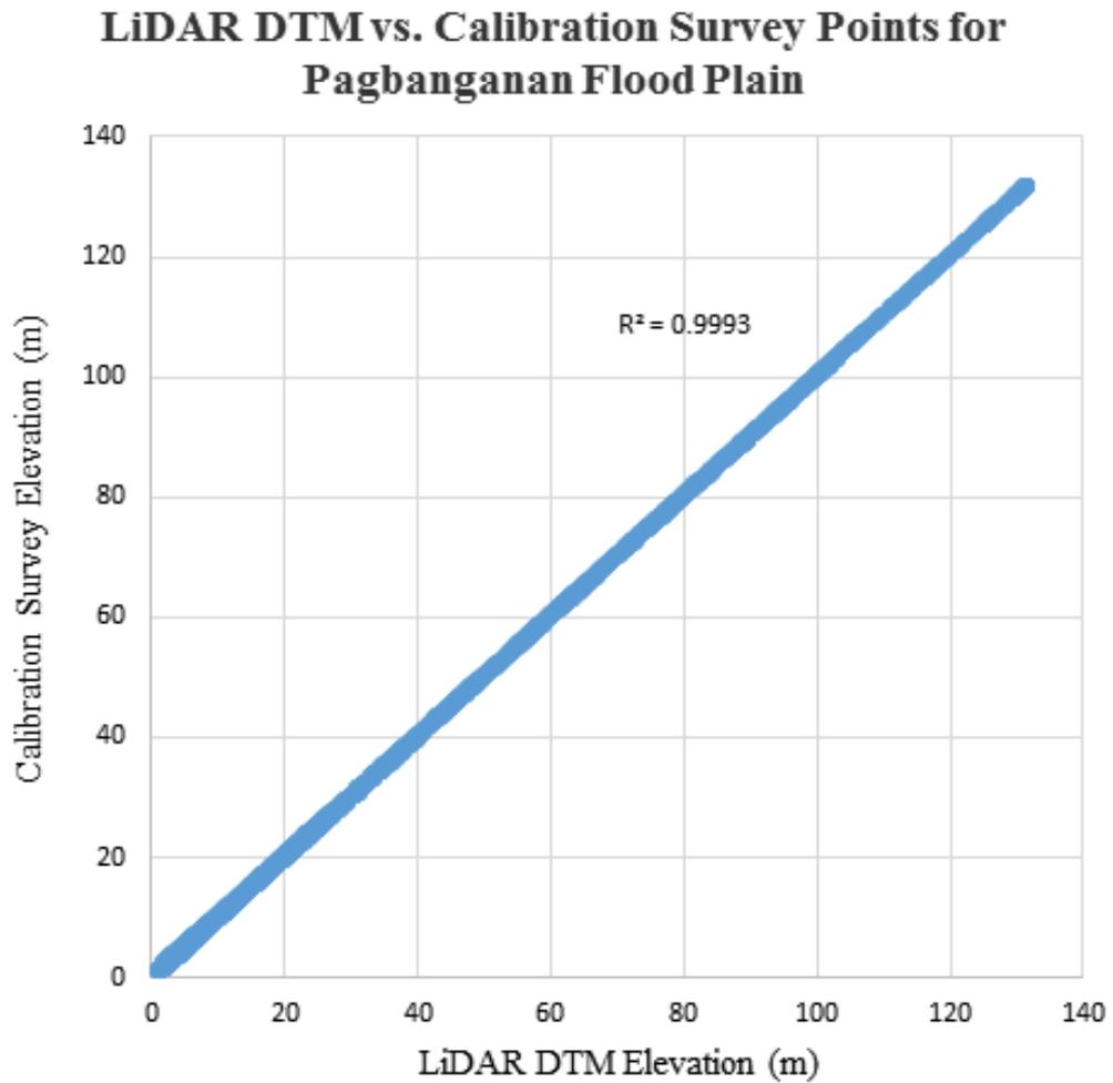
Figure 20. Correlation plot between calibration survey points and LiDAR data
