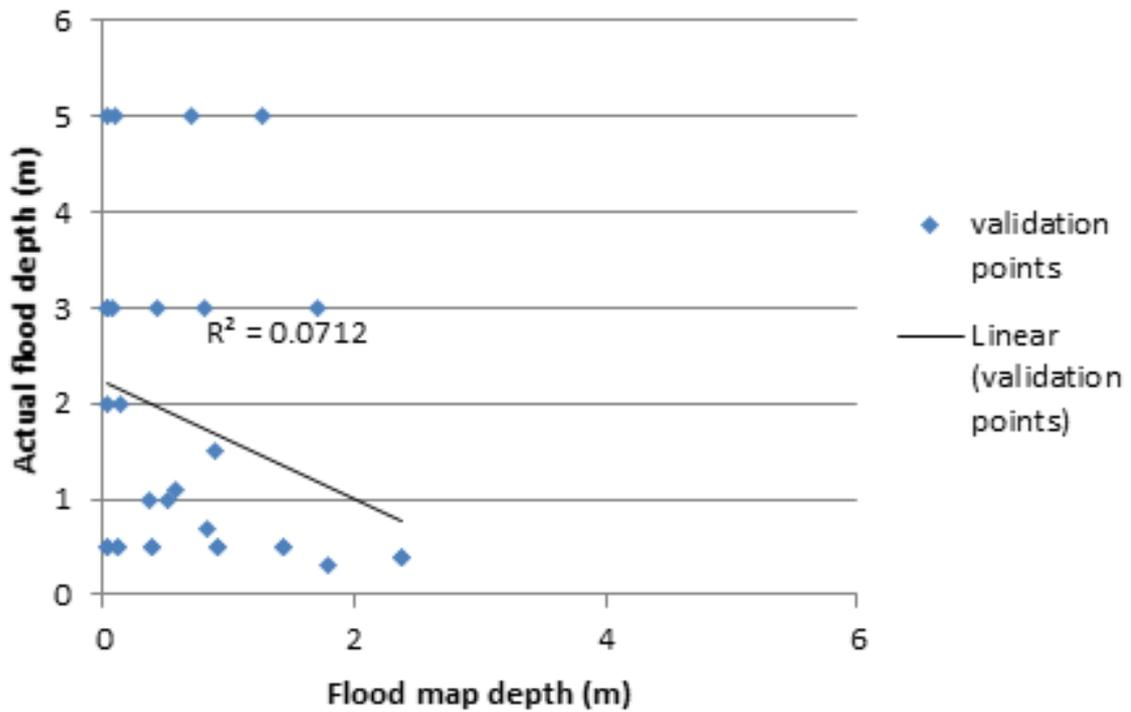
Figure 77. Flood map depth vs. actual flood depth for 25-year RP validation
