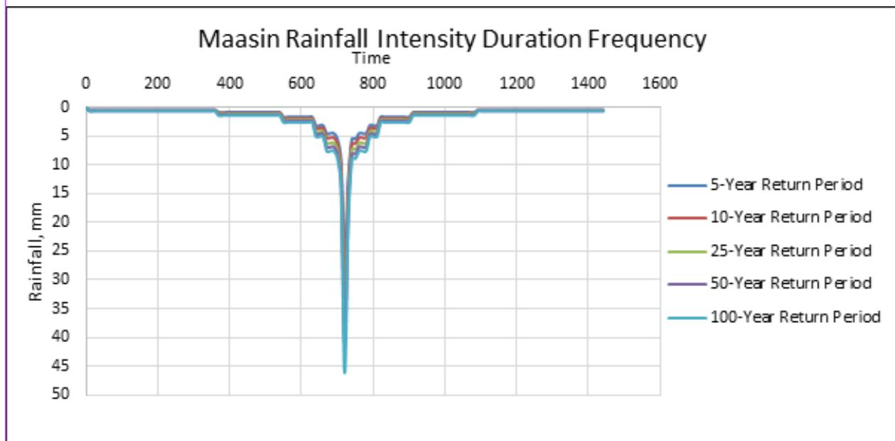
Figure 47. Synthetic storm generated for a 24-hr period rainfall for various return periods
