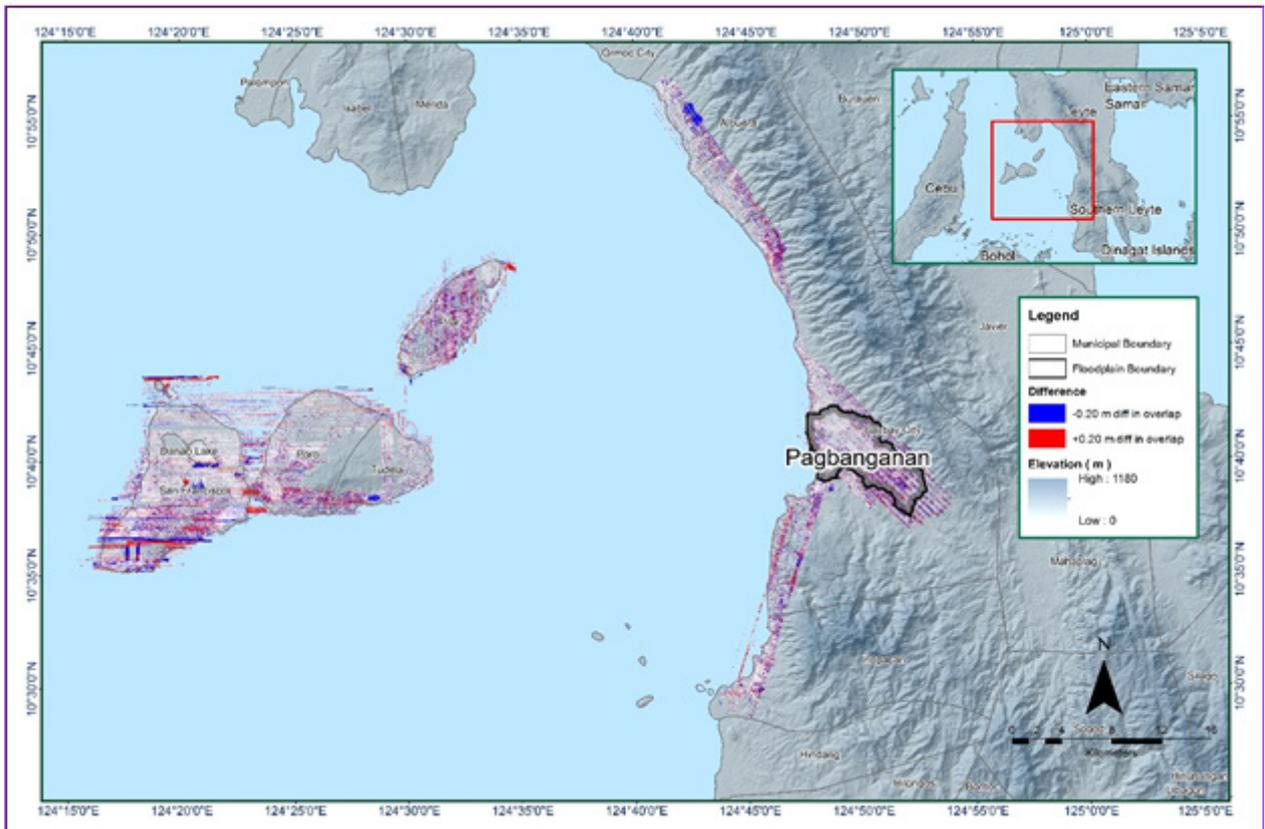
Figure 12. Map of elevation difference between flight lines for Pagbanganan Floodplain
