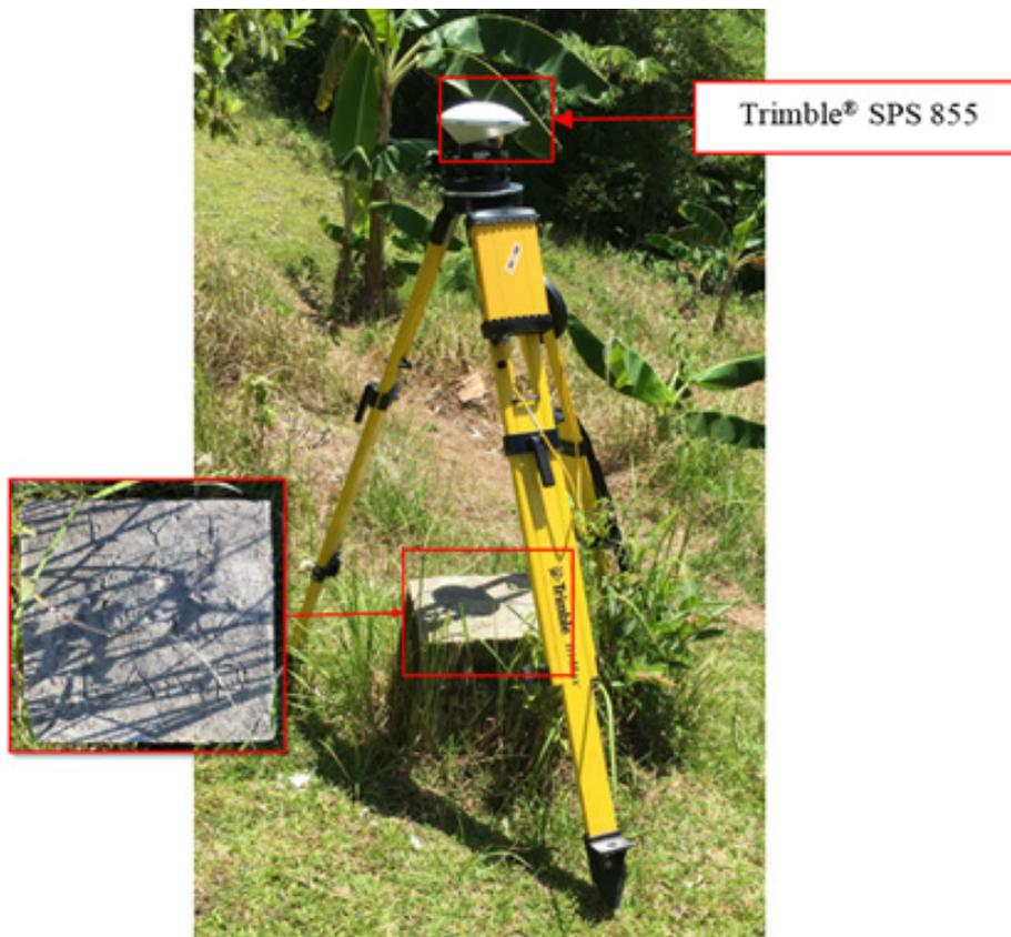
Figure 28. GNSS base set-up, Trimble® SPS 855, at LYT-742, located near a chapel and basketball court in Brgy. Tambis, Municipality of Hilongos, Leyte
