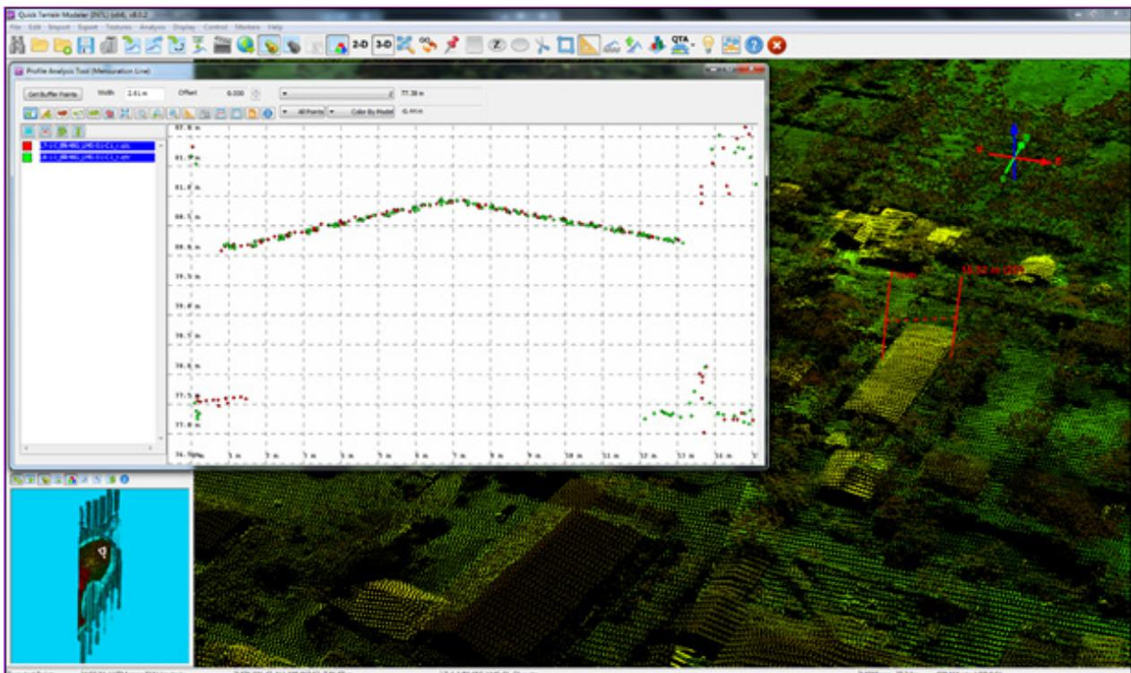
Figure 13. Quality checking for a Pagbanganan flight 8407AC using the Profile Tool of QT Modeler
