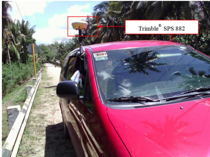
Figure 37. Validation points acquisition survey set up along Pagbanganan River Basin
