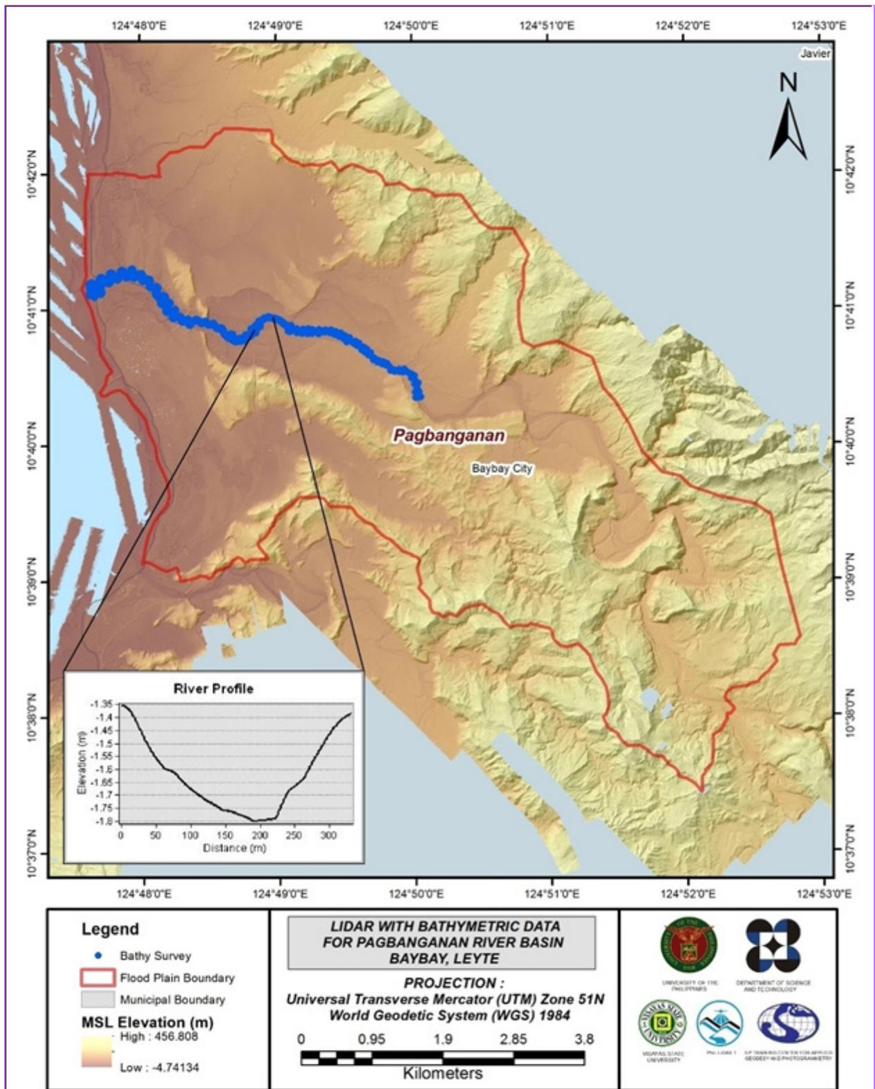
Figure 22. Map of Pagbanganan Floodplain with bathymetric survey points shown in blue
