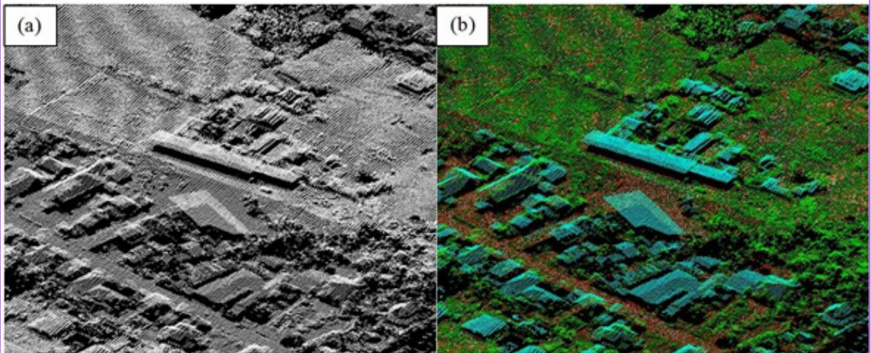
Figure 15. Point cloud before (a) and after (b) classification.
