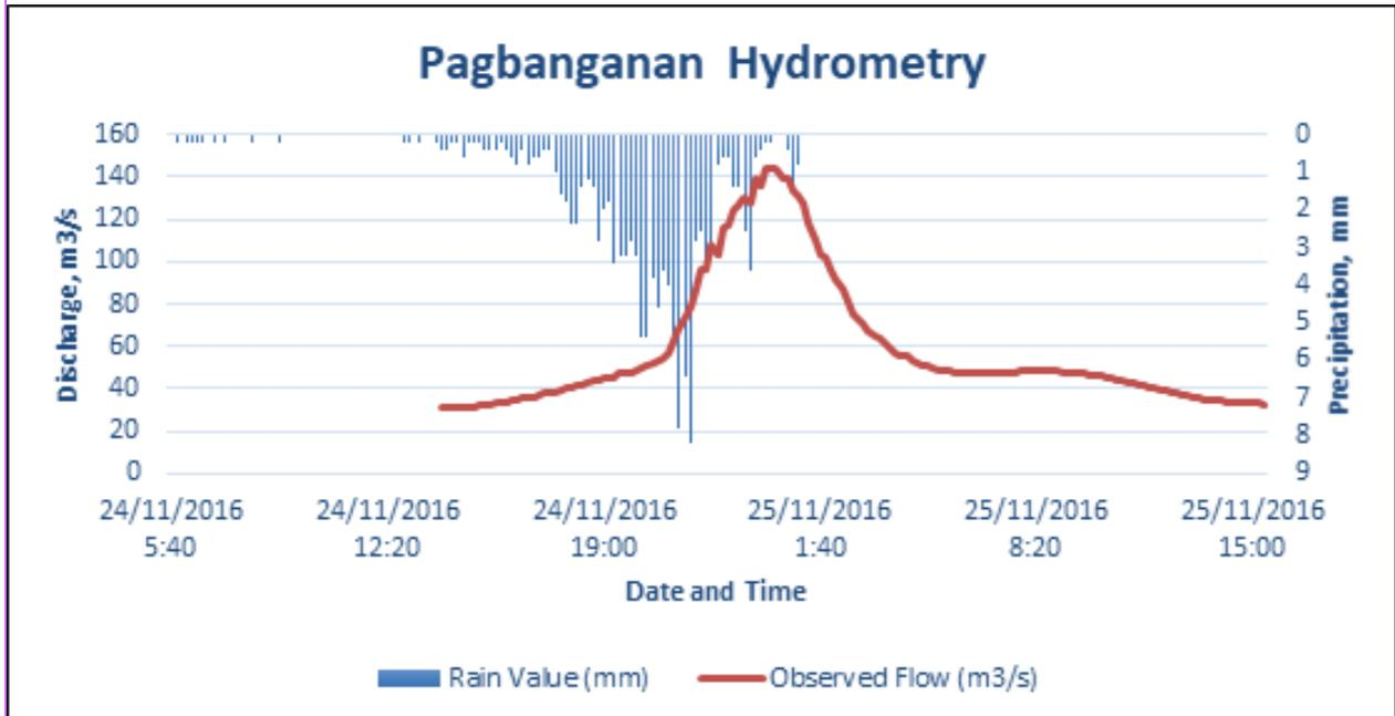
Figure 45. Rainfall and outflow data at Pagbanganan used for modeling
