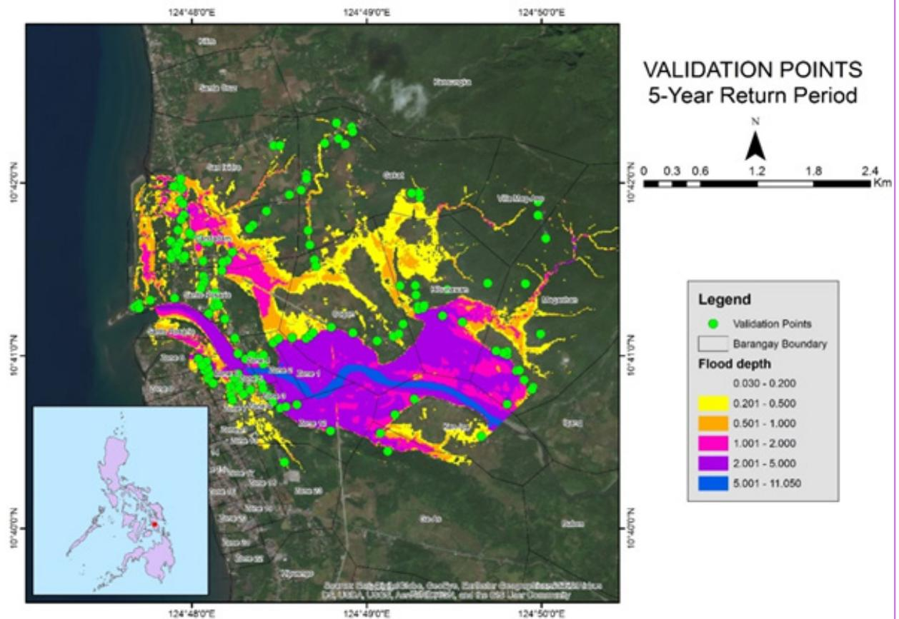
Figure 73. Validation points for 5-year flood depth map of Pagbanganan Floodplain
