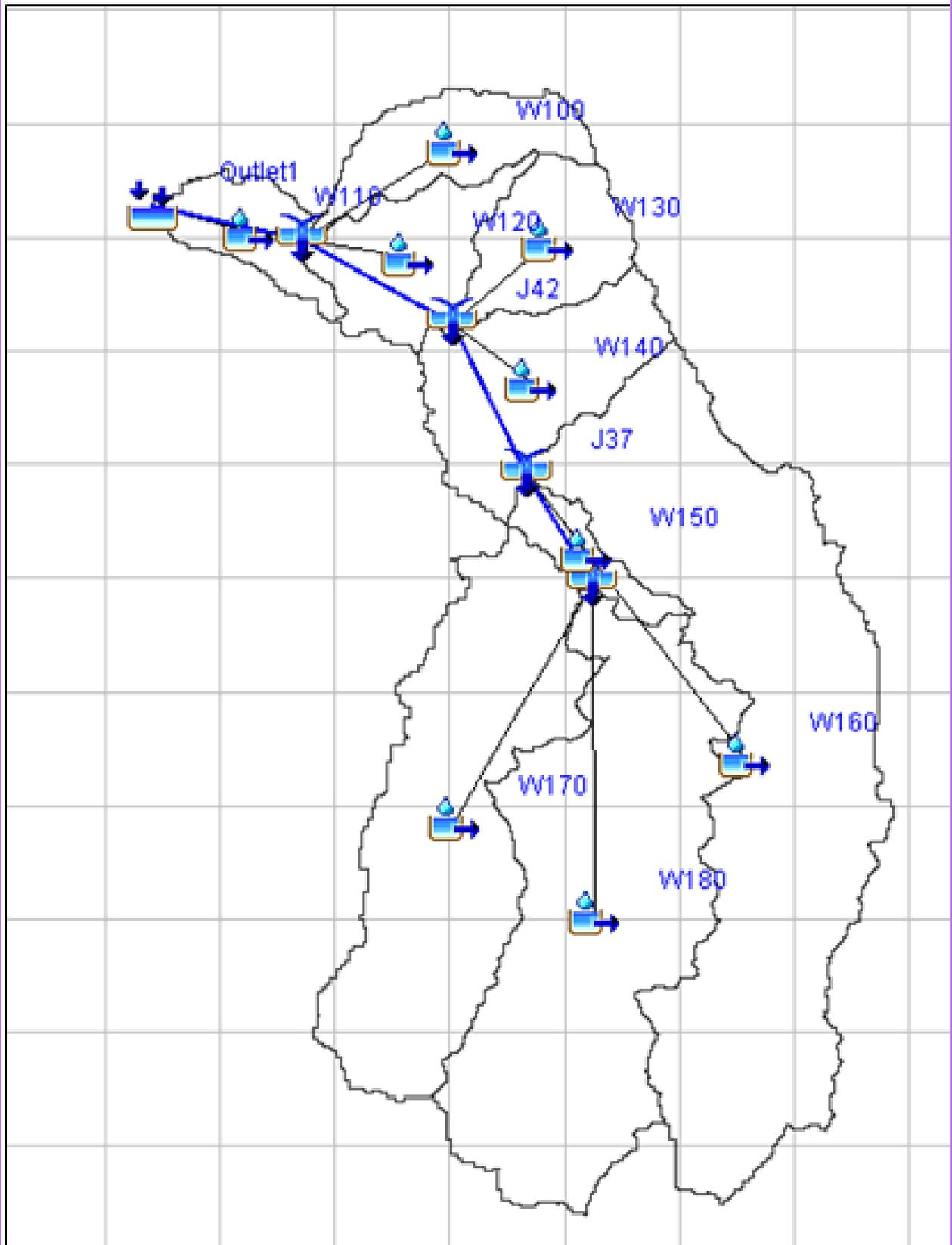
Figure 52. The Pagbanganan River Basin model generated using HEC-HMS
