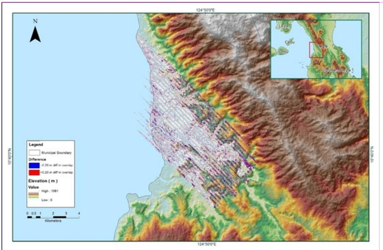
Elevation difference between flight lines
