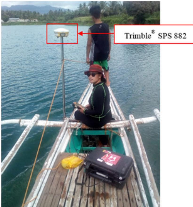
Figure 39. Bathymetric survey set-up in Pagbanganan River
