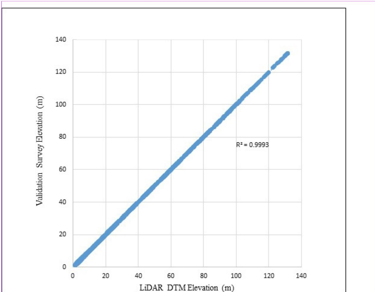
Figure 26. Correlation plot between validation survey points and LiDAR data
