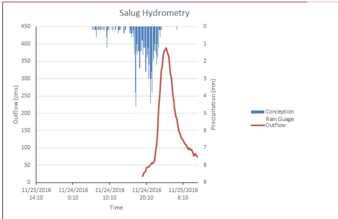
Figure 50. Rainfall and outflow data at Salug Bridge used for modeling
