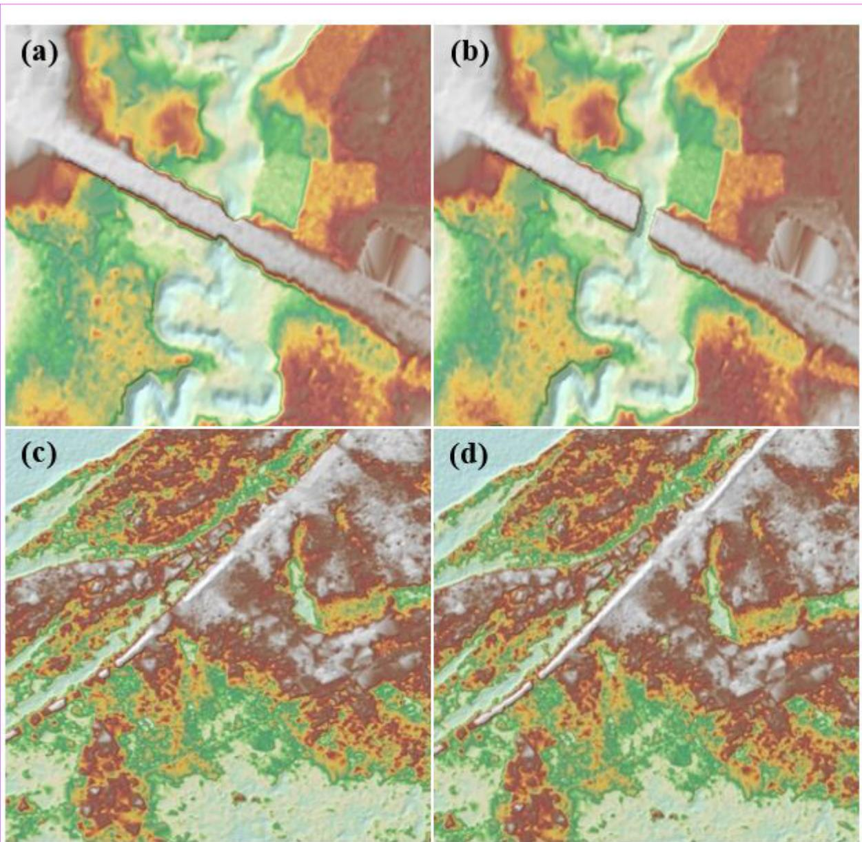
Figure 22. Portions in the DTM of Salug Floodplain – a bridge before (a) and after (b) manual editing; a road before (c) and after (d) data retrieval
