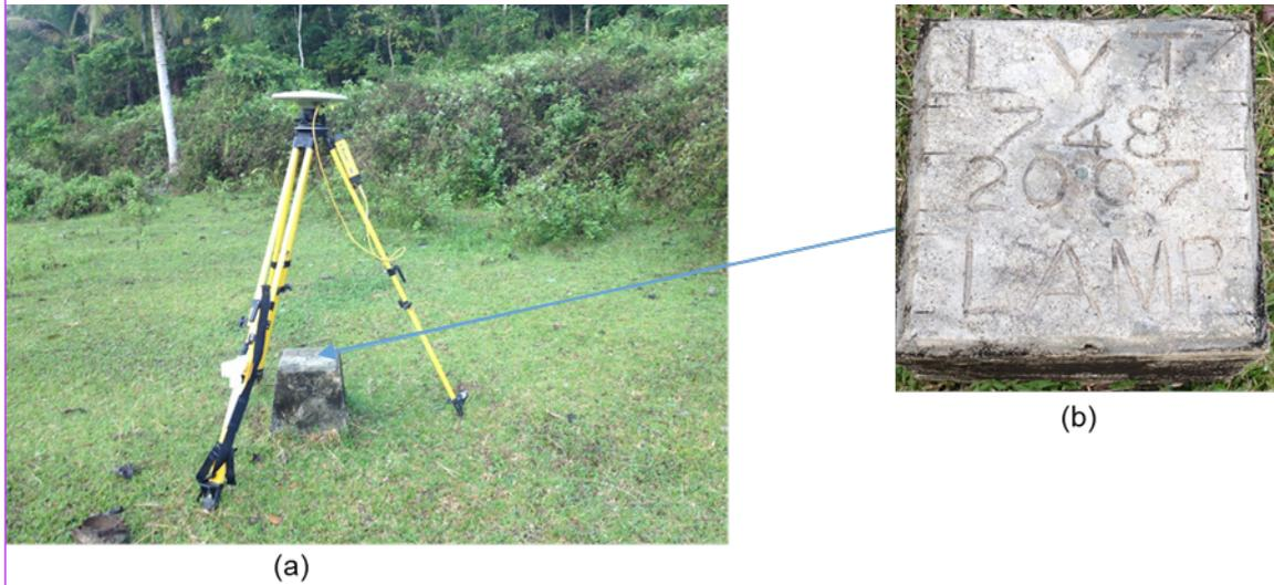
Figure 5. GPS set-up over LYT-748 at the back of Hitoog Elementary School, Brgy. Hitoog, Municipality of Matalom, Leyte (a) and NAMRIA reference point LYT-748 (b) as recovered by the field team
