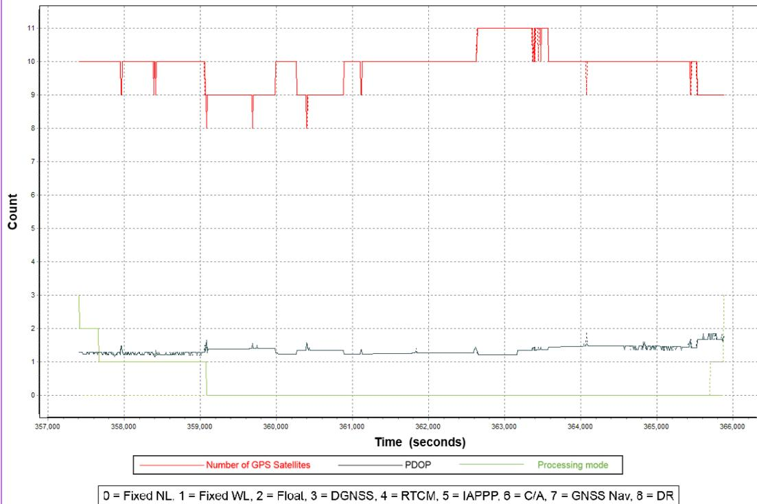
Figure 10. Solution Status parameters of Salug Flight 7754A.
