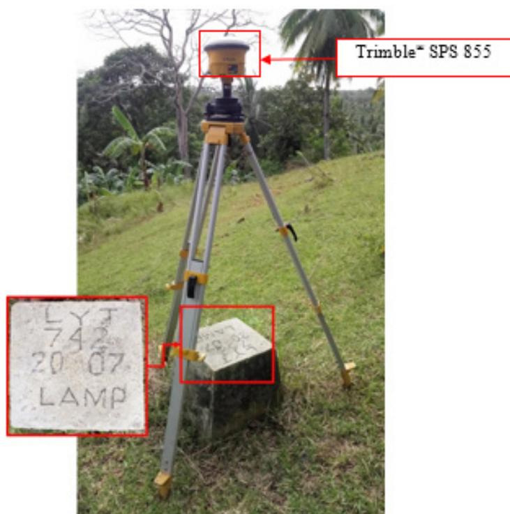
Figure 32. GNSS base set up, Trimble<sup>®</sup> SPS 855, at LYT-742, located near a chapel and basketball court in Brgy. Tambis, Municipality of Hilongos, Leyte
