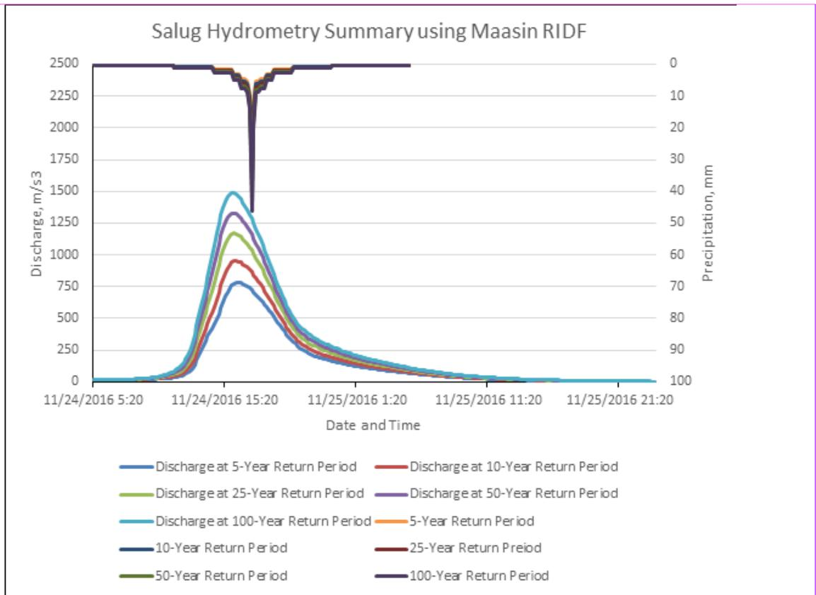
Figure 61. Outflow hydrograph at Salug Station generated using Tacloban RIDF simulated in HEC-HMS
