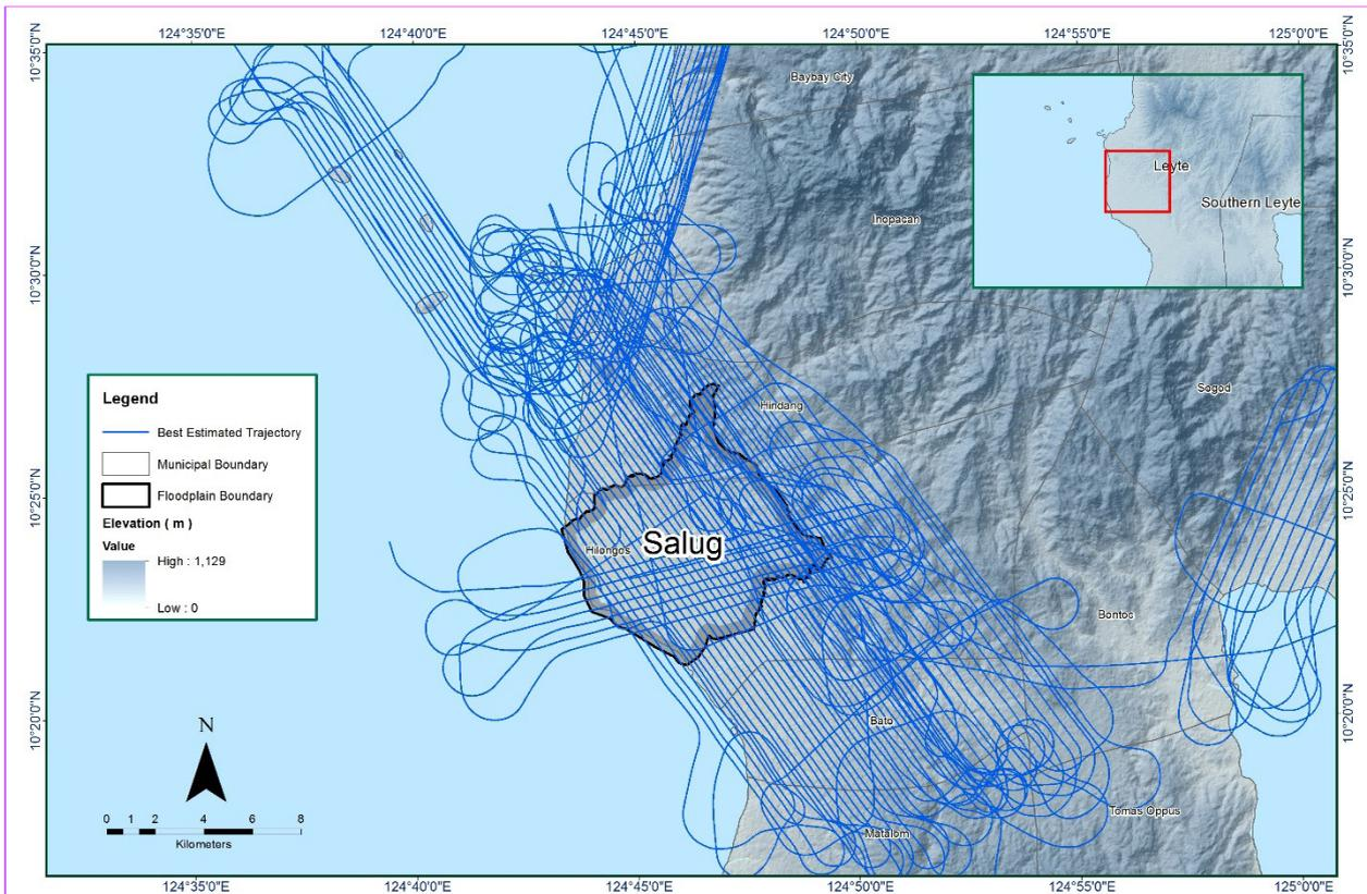
Figure 11. Best estimated trajectory of LiDAR missions conducted over Salug Floodplain
