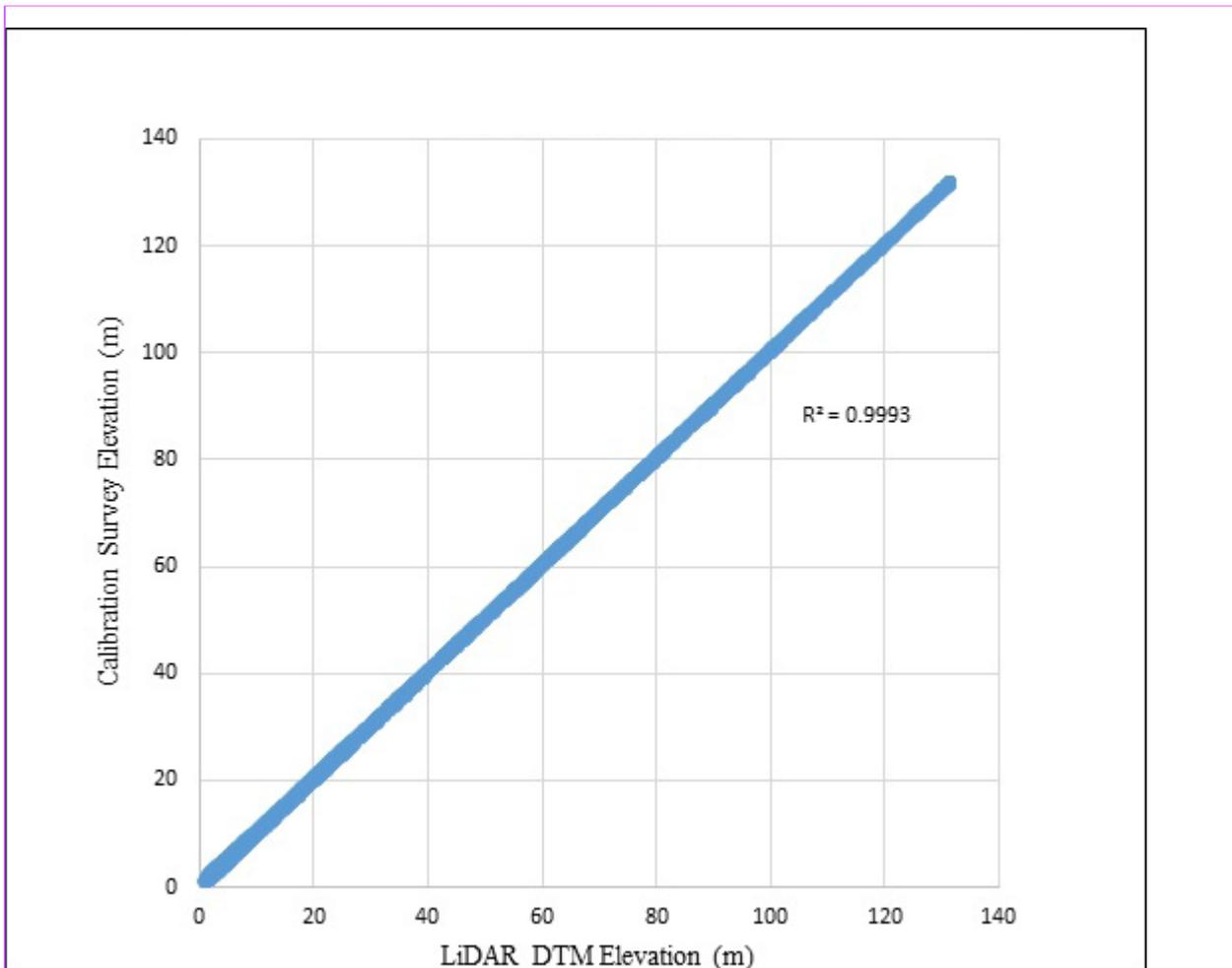
Figure 25. Correlation plot between calibration survey points and LiDAR
