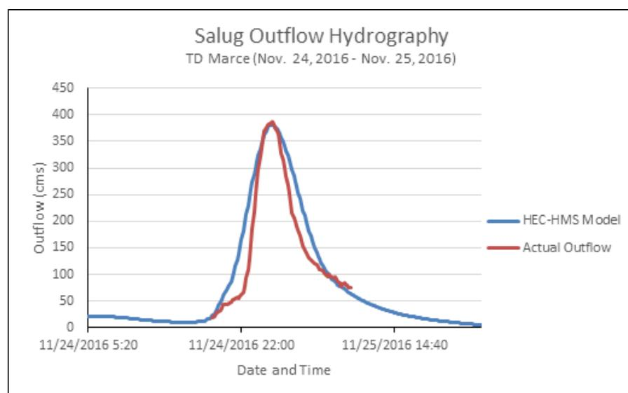
Figure 60. Outflow hydrograph of Salug Bridge generated in HEC-HMS model compared with observed outflow. Enumerated in Table 33 are the adjusted ranges of values of the parameters used in calibrating the model.
