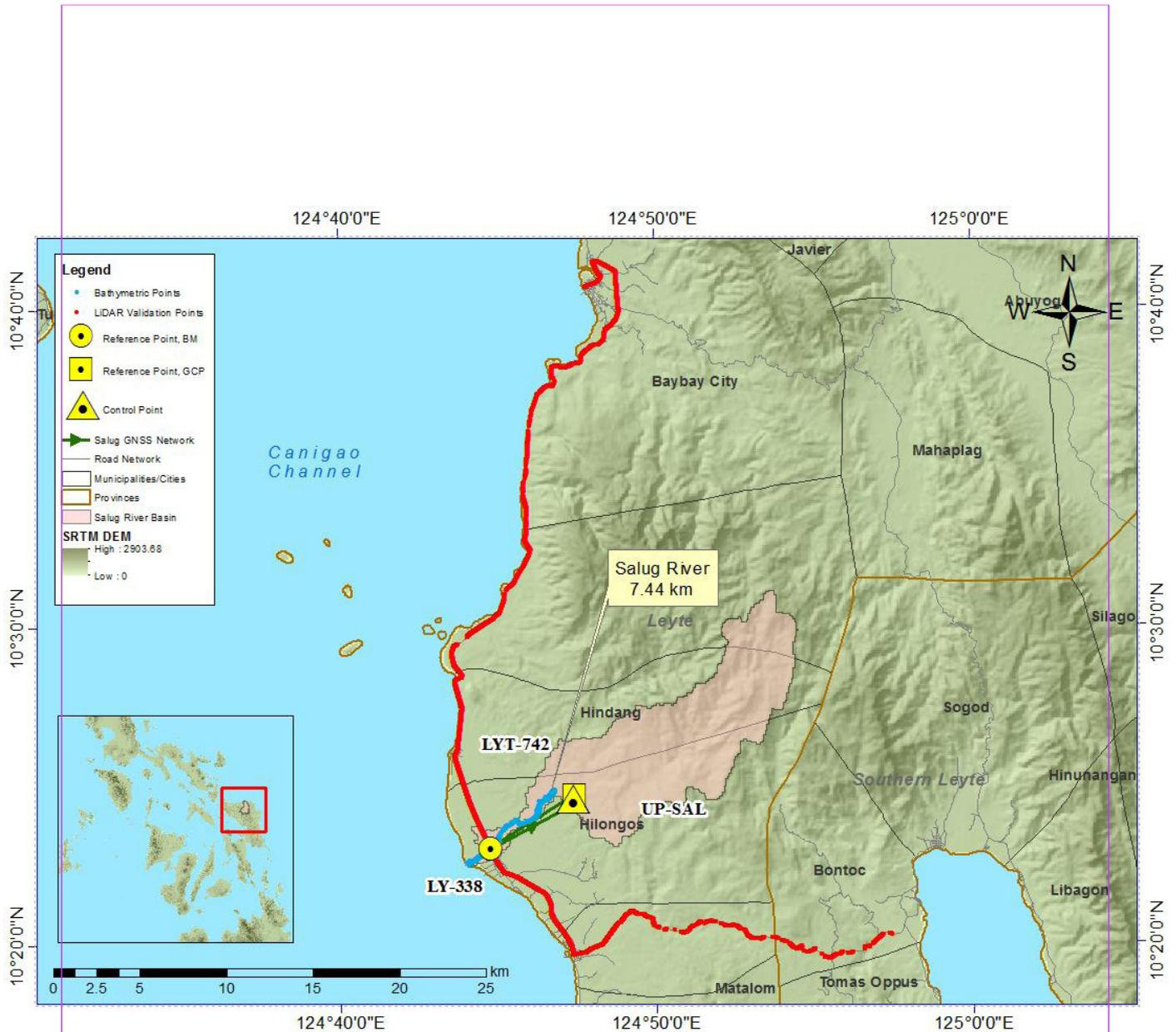
Figure 30. Extent of the bathymetric survey (in blue) in Salug River and the LiDAR data validation survey (in red)
