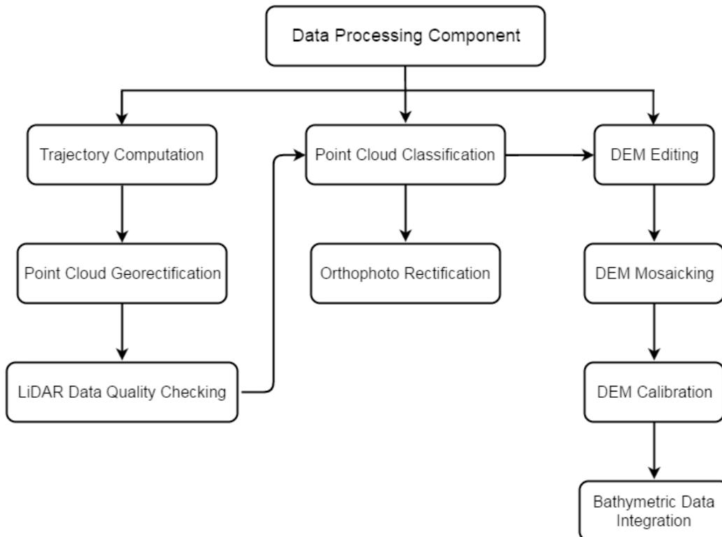
Figure 8. Schematic diagram for Data Pre-Processing Component
