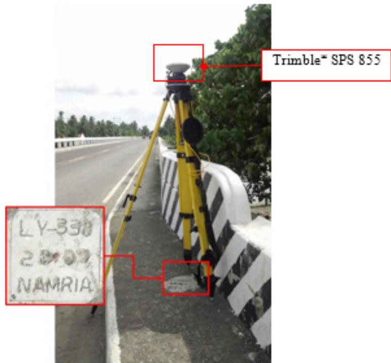
Figure 33. GNSS receiver set up, Trimble® SPS 855, at LY-338, located at the approach of Salug Birdge along Sta. Indang-Hilongos Road in Brgy. San Juan, Municipality of Hilongos, Leyte
