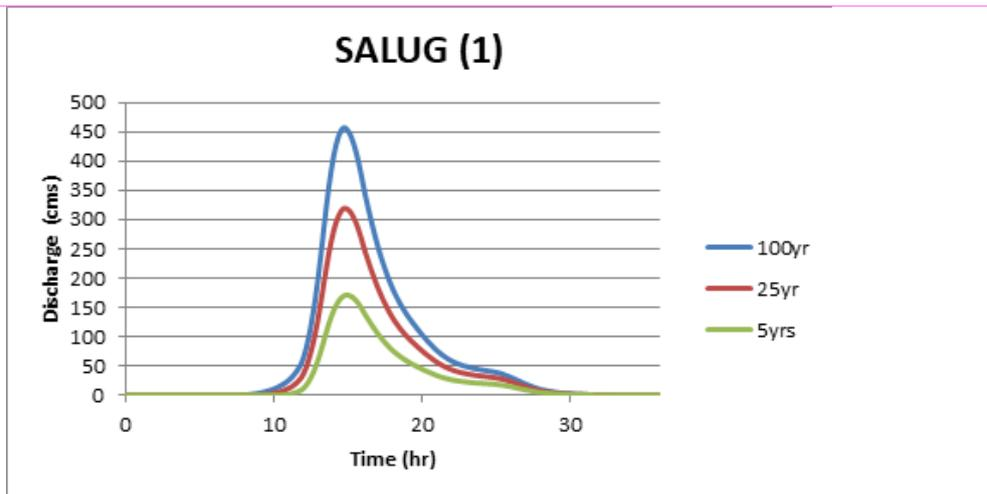
Figure 62. Salug River (1) generated discharge using 5-, 25-, and 100-year Tacloban City rainfall intensity-duration-frequency (RIDF) in HEC-HMS
