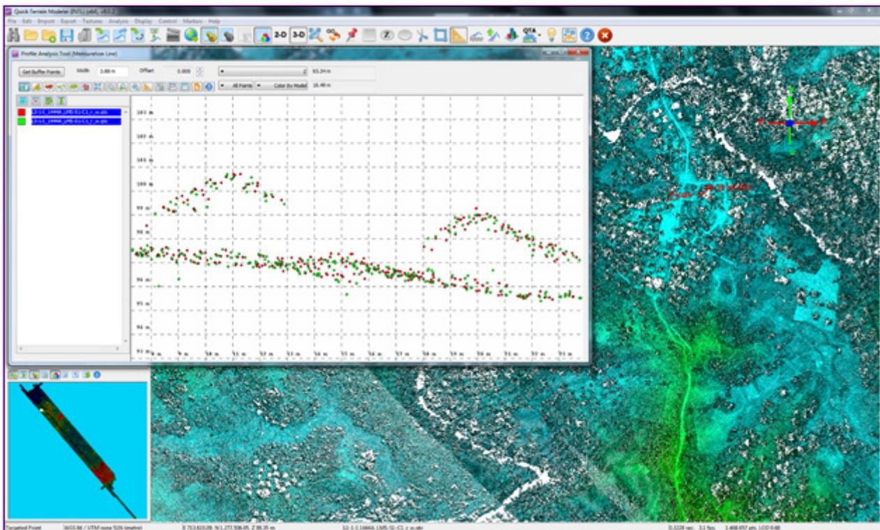
Figure 19. Quality checking for Silaga flight 14444A using the Profile Tool of QT Modeler
