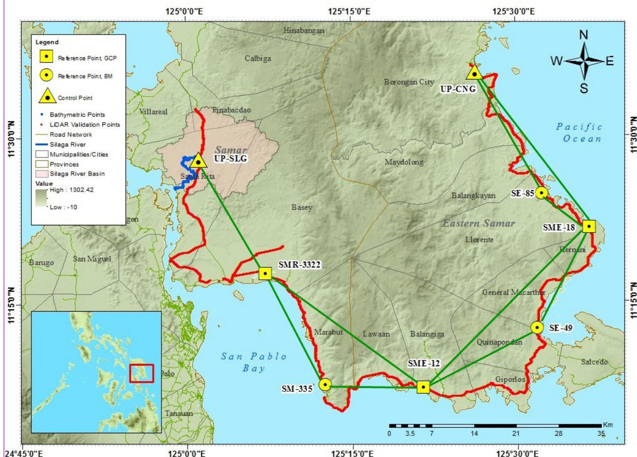
Figure 33. Extent of the bathymetric survey (in blue line) in Silaga River and the LiDAR data validation survey (in red).
