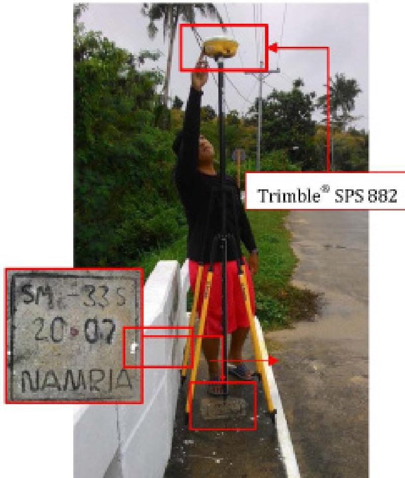
Figure 40. The GNSS (Trimble® SPS 882) base occupation , at SM-33S, located in Brgy. Pinalanga in the Municipality of Marabut, Samar.
