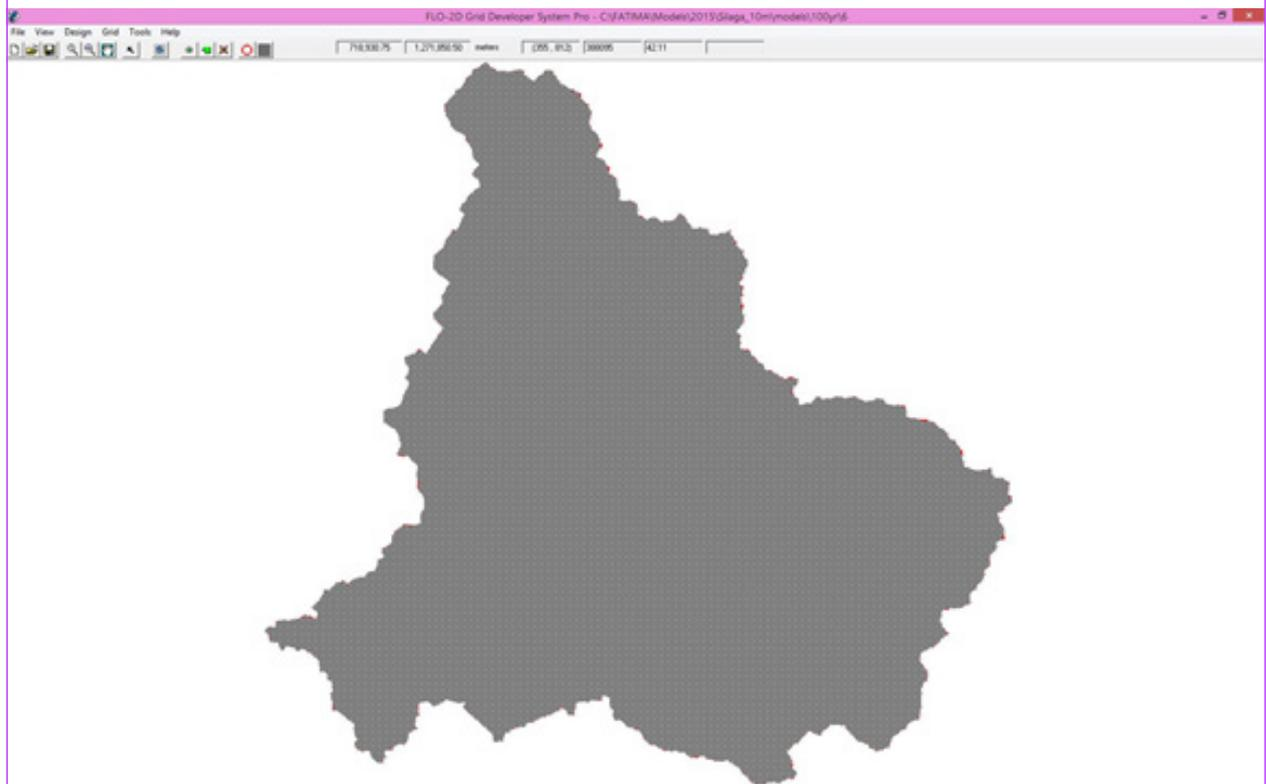
Figure 66. A screenshot of the river sub-catchment with the computational area to be modeled in FLO-2D Grid Developer System Pro (FLO-2D GDS Pro)
