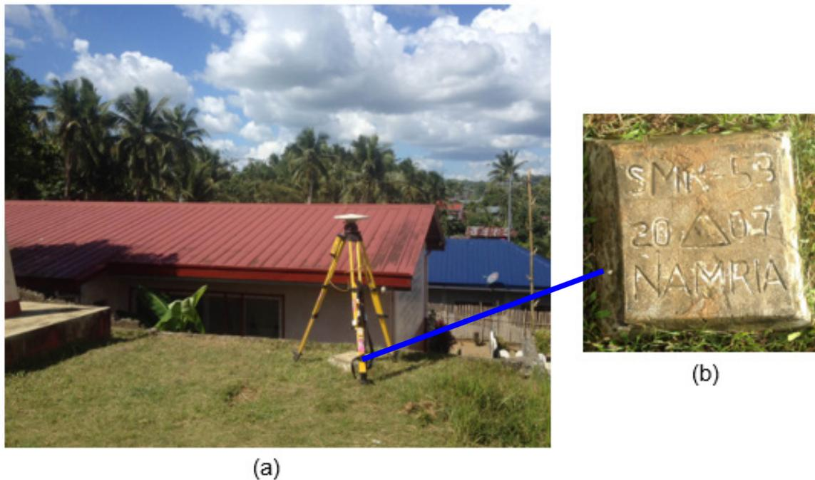
Figure 3. Photo (A) shows the GPS set-up over SMR-53 located near the flagpole of San Isidro Elementary School, Brgy. San Isidro, Santa Rita, Samar; while Photo (B) depicts the close-up view of NAMRIA reference point SMR-53 as recovered by the field team.
