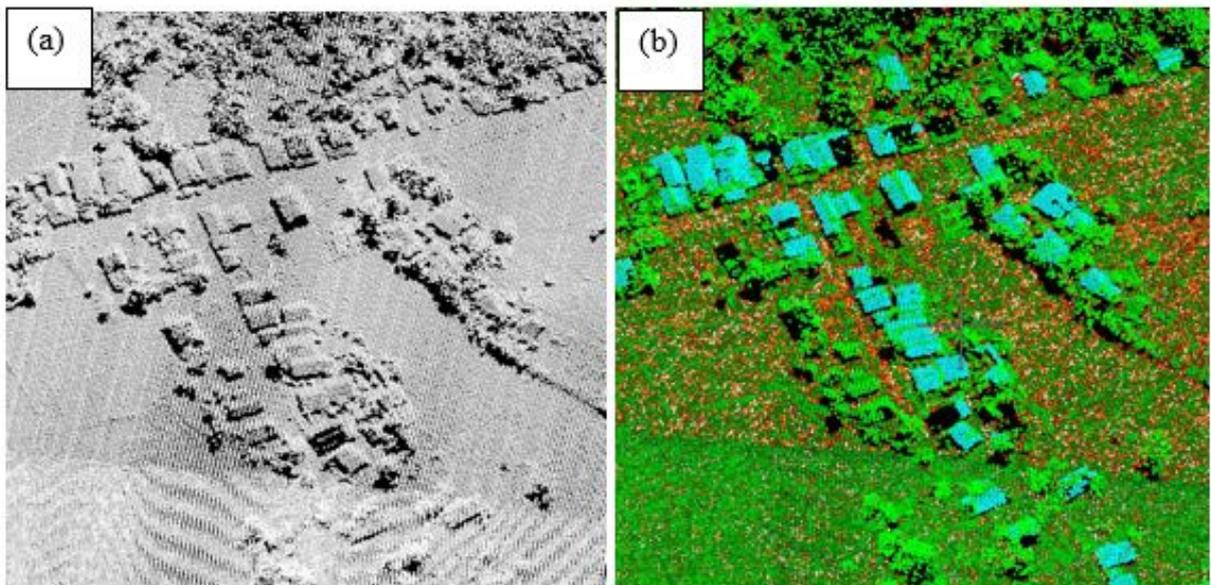
Figure 21. Point cloud before (a) and after (b) classification
