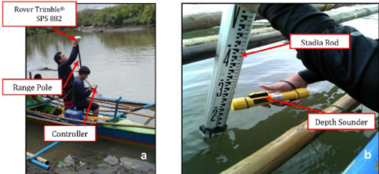
Figure 51. Photos showing (a) setup for the Bathymetric Survey in Silaga River; (b) use of portable sounder in measuring the deeper parts of the river.
