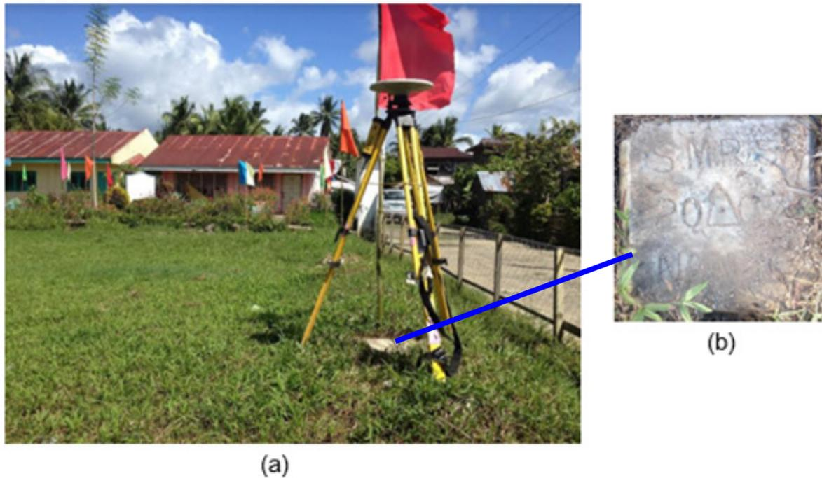
Figure 5. Photo (A) shows the GPS set-up over SMR-58 located inside Serum Elementary School, Brgy. Serum, Basey; while Photo (B) depicts a close-up view of NAMRIA reference point SMR-58 as recovered by the field team.
