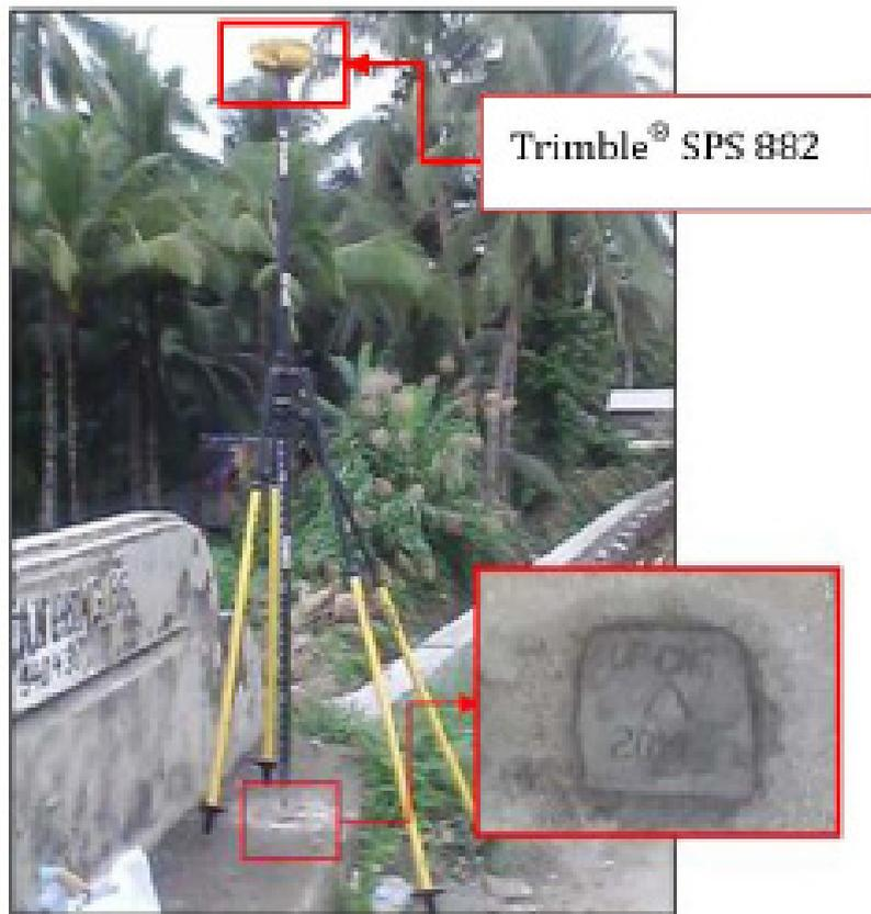
Figure 41. The GNSS receiver occupation, Trimble® SPS 882, at UP-CNG, located at the approach of Can-Obing Bridge in Brgy. Can-Abong, Borongan City, Eastern Samar.
