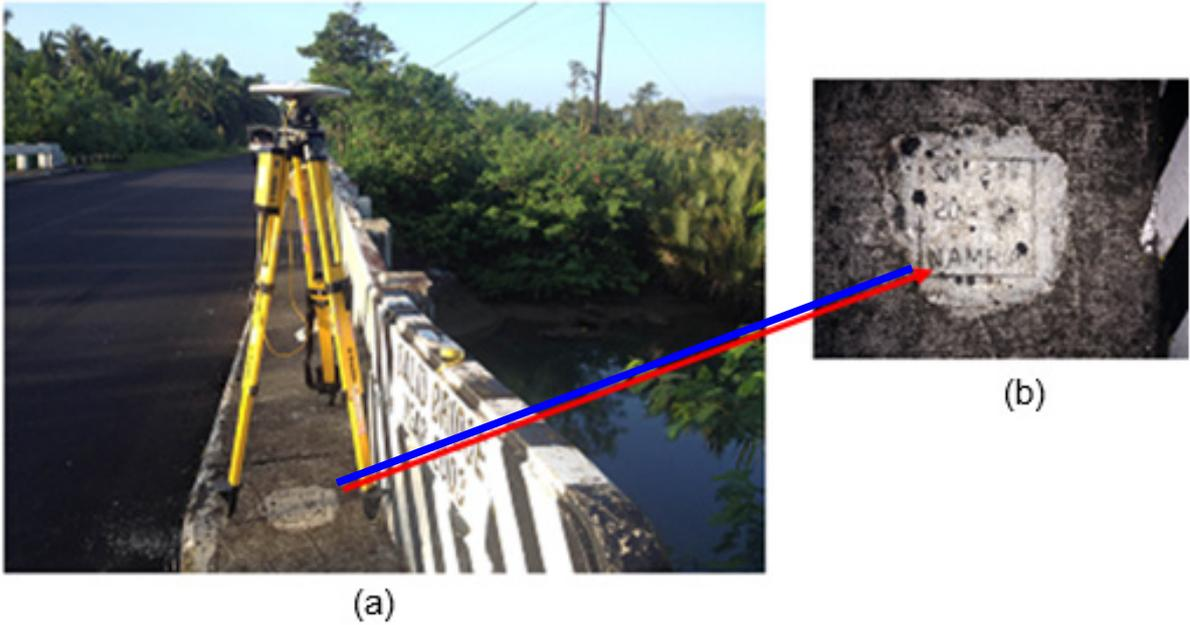
Figure 6. Photo (A) shows the GPS set-up over SM-286 located at Dalid Bridge along the National Highway in Brgy. San Pascual, Sta. Rita, Samar; while Photo (B) offers a close-up view of NAMRIA reference point SM-286 as recovered by the field team.
