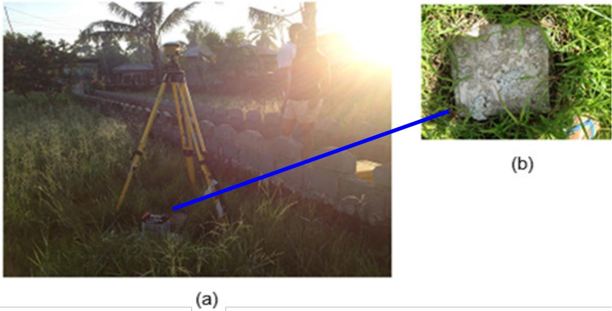
Figure 4. Photo (A) shows the GPS set-up over SMR-56 located inside Cabacungan Elementary School, Brgy. Cabacungan, Sta. Rita, Samar; while Photo (B) presents a close-up view of NAMRIA reference point SMR-56 as recovered by the field team.
