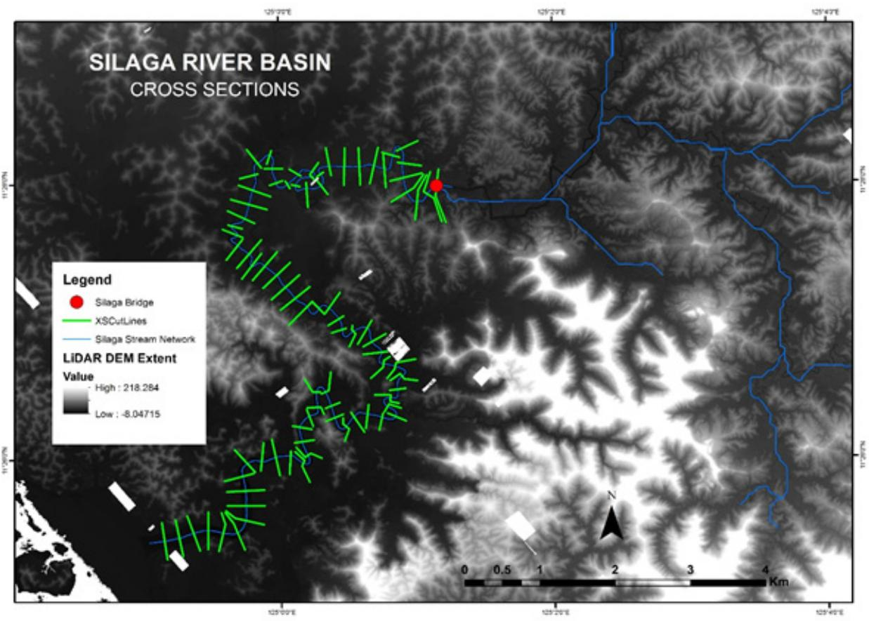
Figure 65. River cross-section of the Silaga River through the ArcMap HEC GeoRas tool
