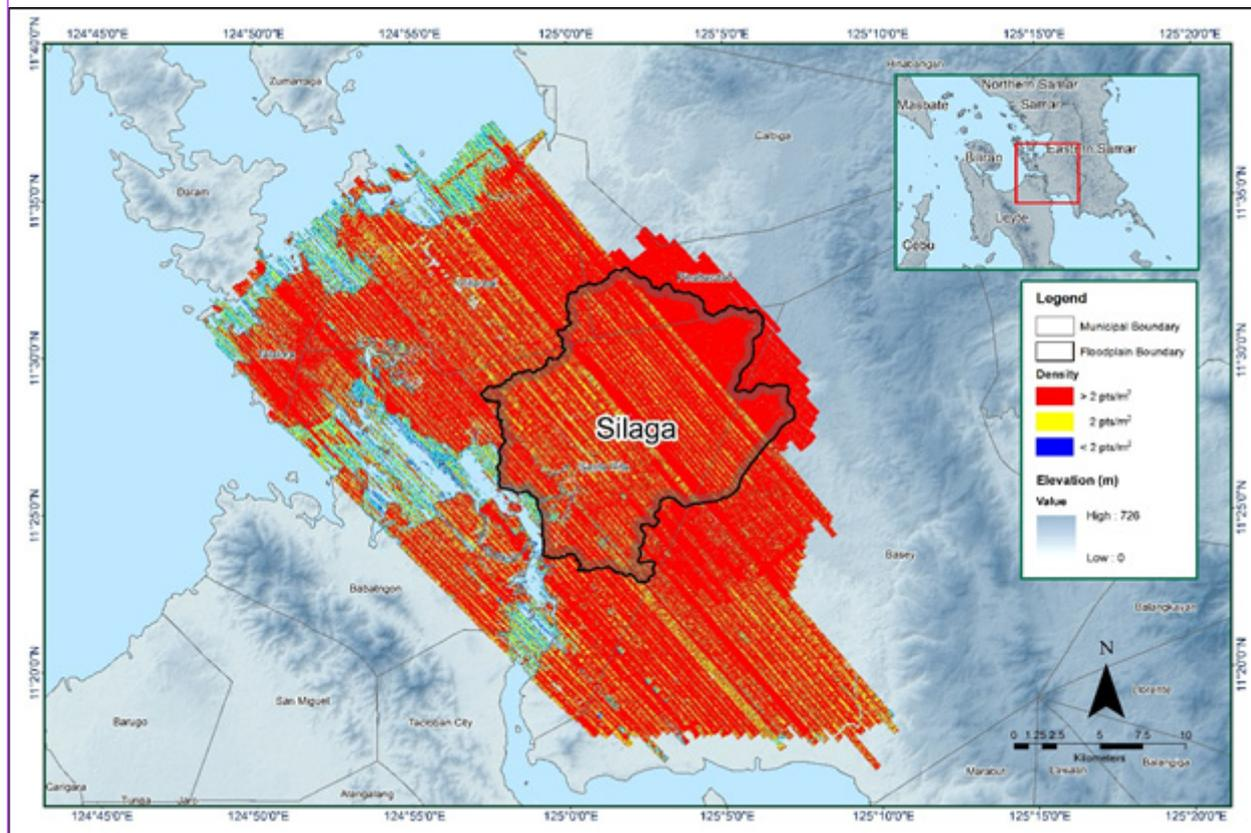
Figure 17. Pulse density map of merged LiDAR data for Silaga floodplain.
