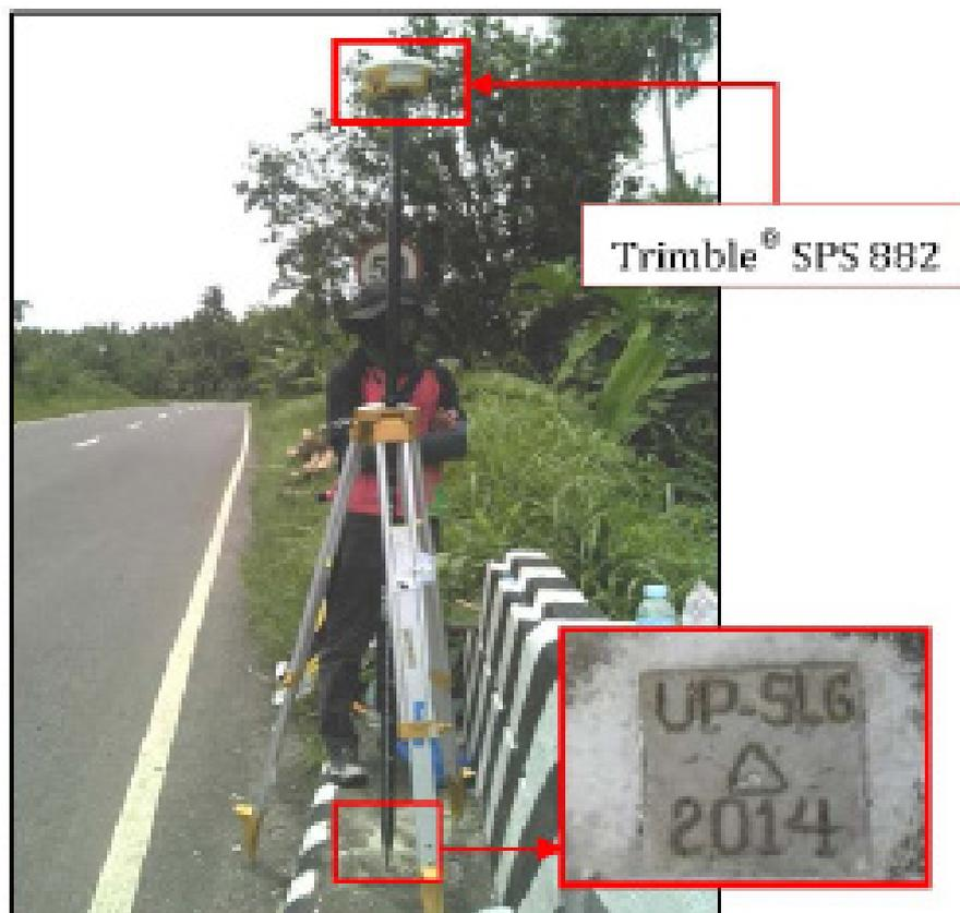
Figure 42. The GNSS receiver occupation, Trimble® SPS 882, at UP-SLG, located at the approach of Silaga Bridge in Brgy. Tominamos in the Municipality of Sta Rita, Samar.
