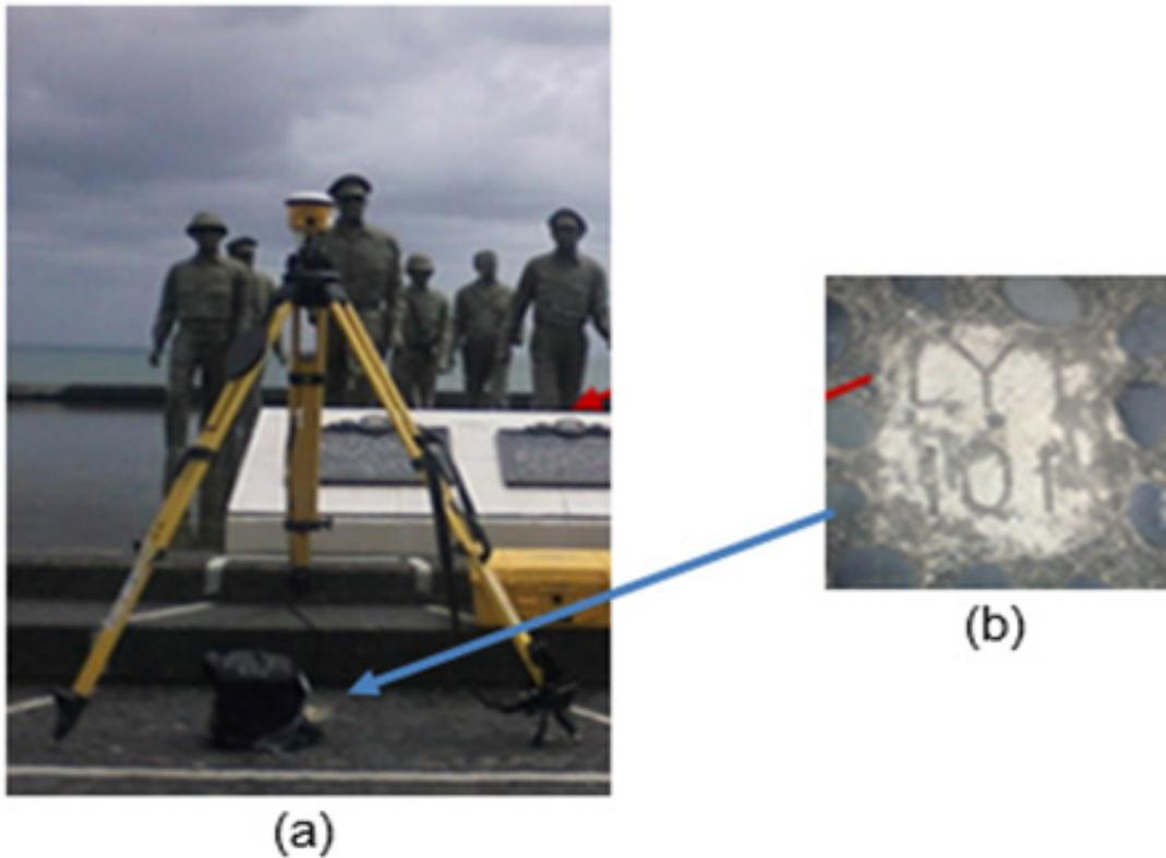
Figure 8. Photo (A) depicts the GPS set-up over LYT-101 located within the premises of MacArthur’s Landing Memorial Park, Palo, Leyte; while Photo (B) shows a close-up view of NAMRIA reference point LYT-101 as recovered by the field team.
