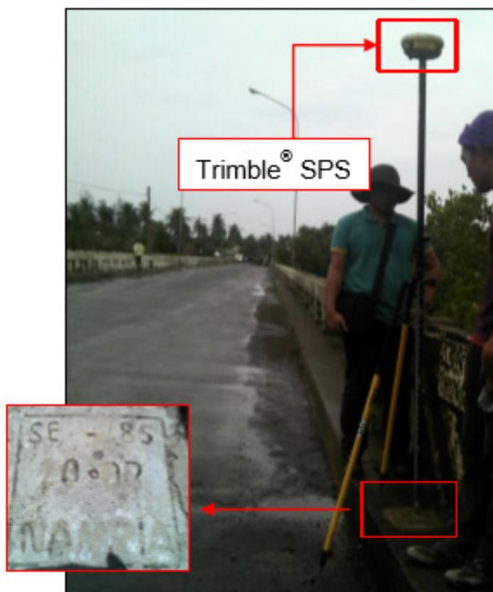
Figure 36. The GNSS (Trimble® SPS 882) receiver setup at SE-85, located at the approach of Llorente Bridge in Brgy. II, Municipality of Llorente, Eastern Samar
