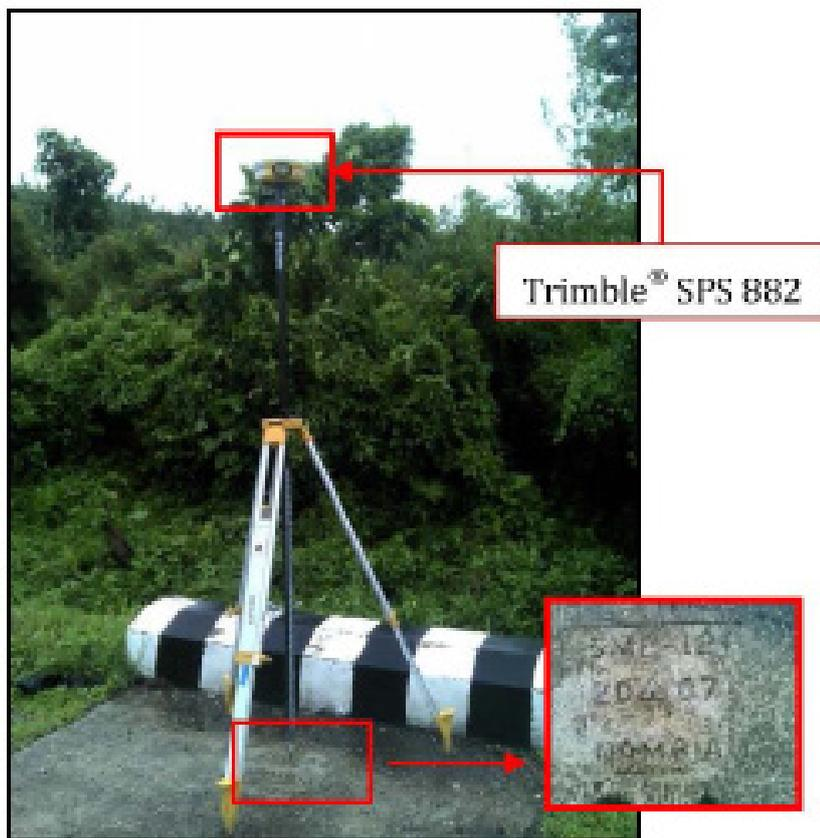
Figure 37. The GNSS (Trimble® SPS 882) receiver occupation, at SME-12, located in Brgy. San Miguel, Municipality of Balangiga, Eastern Samar.
