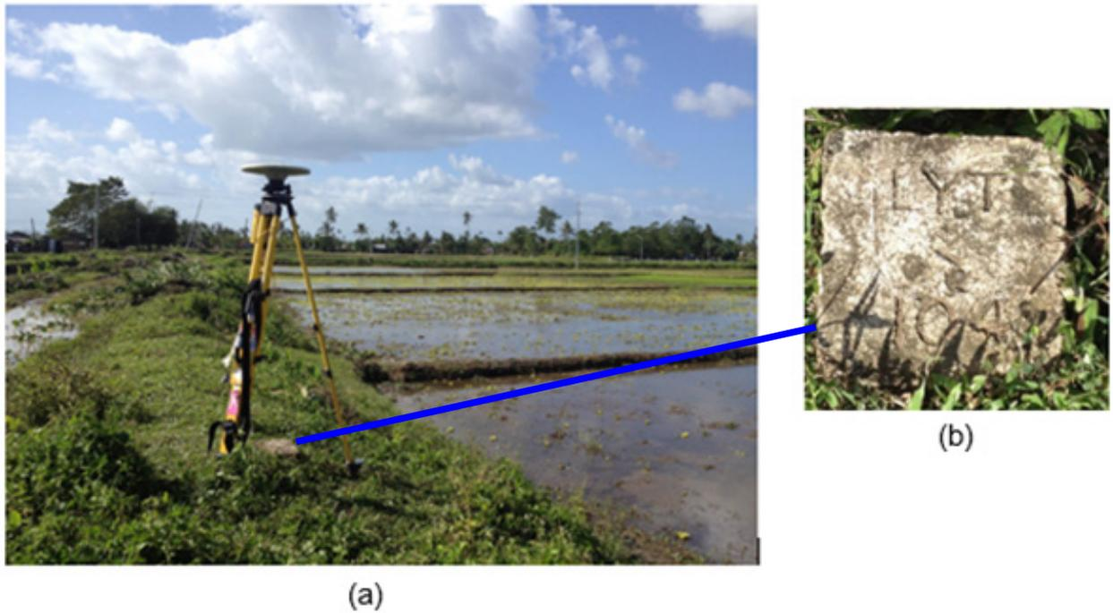
Figure 9. Photo (A) displays the GPS set-up over LYT-104 located and reestablished along a rice paddy trail, approximately 90 meters from the centerline, east side of Pastrana-Santa Fe Road, District IV, Pastrana, Leyte; while Photo (B) shows a close-up view of NAMRIA reference point LYT-104 as recovered by the field team.
