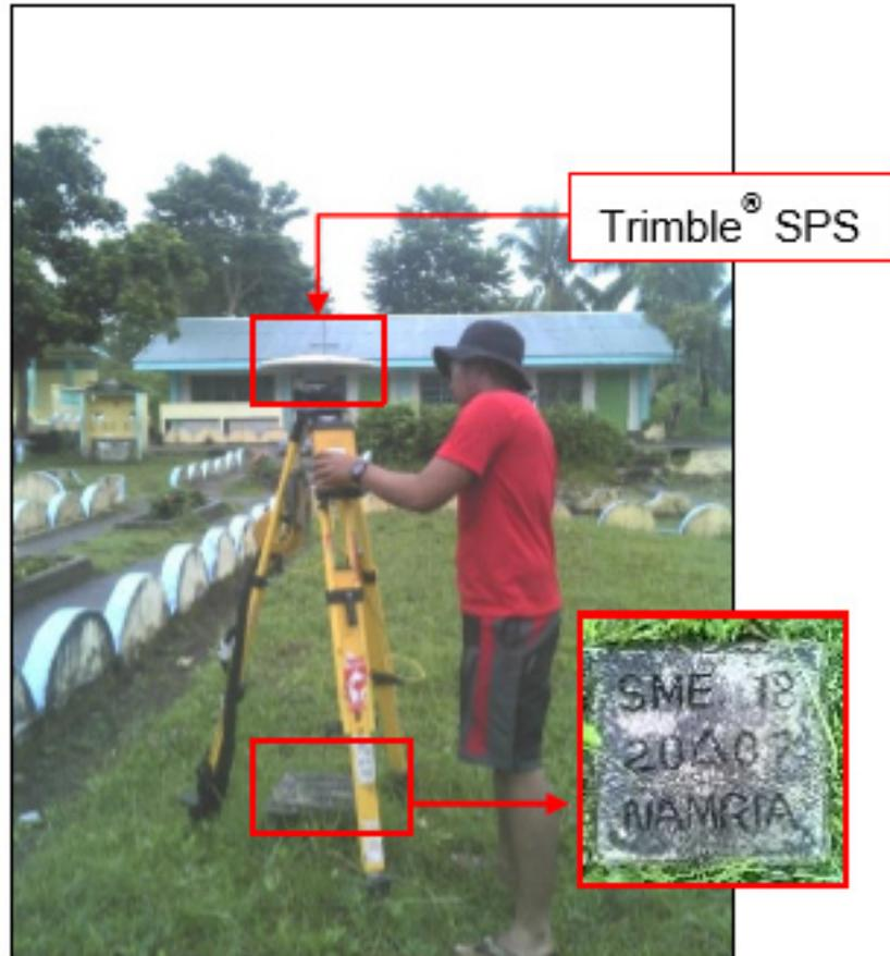
Figure 35. The GNSS base receiver setup, Trimble® SPS 852, at SME-18, located inside San Jose Elementary School, Brgy. Canciledes in the Municipality of Hernani, Eastern Samar.
