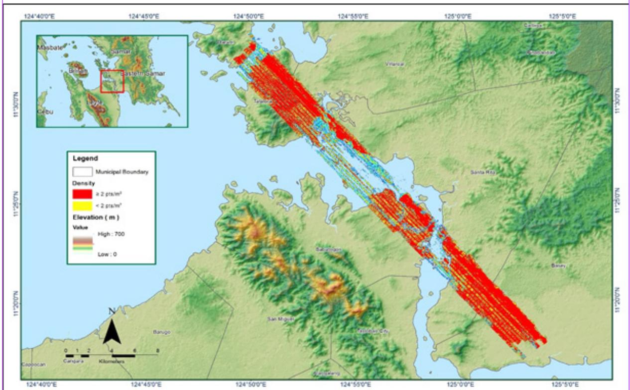
Figure A-8.27. Density map of merged LiDAR data
