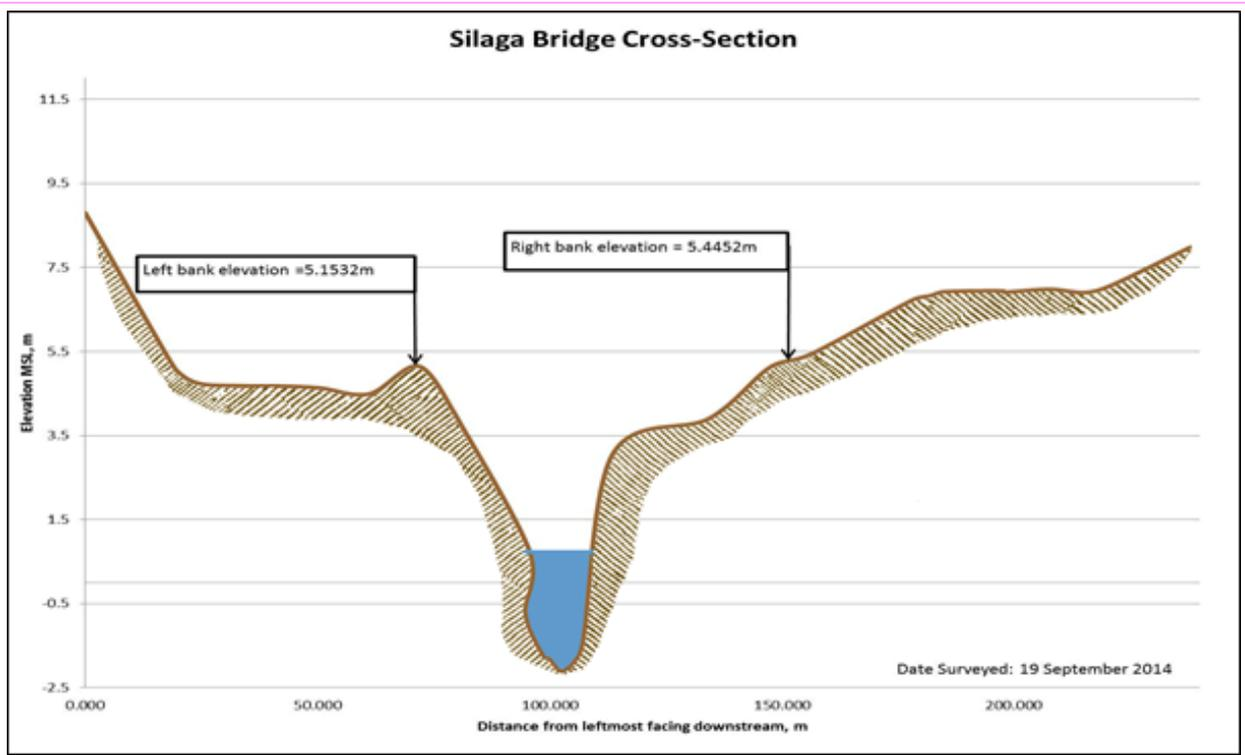
Figure 55. Cross-section plot of the Silaga Bridge
