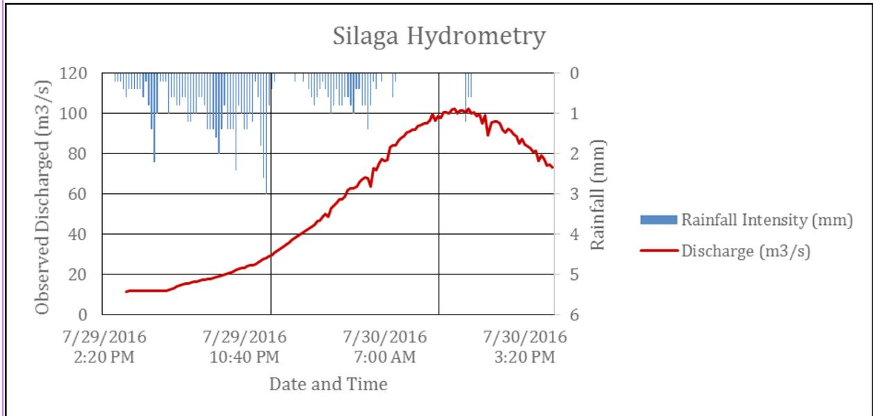
Figure 57. Rainfall and outflow data of the Silaga River Basin, which was used for modeling.
