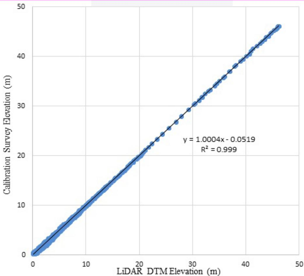
Figure 28. Correlation plot between calibration survey points and LiDAR data.
