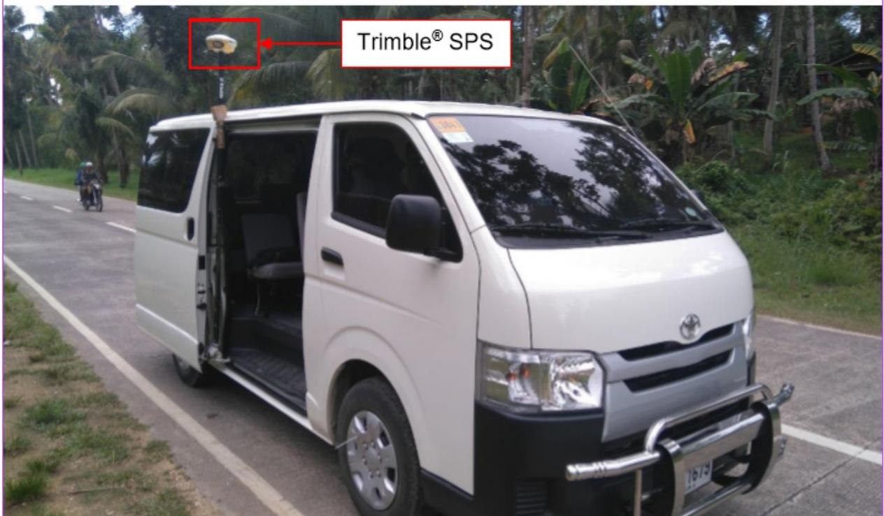
Figure 49. The validation point acquisition survey setup using a GNSS receiver fixed in a van along the Silaga River Basin
