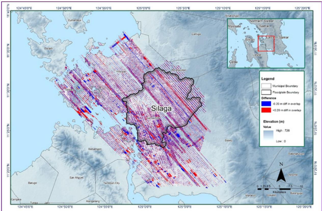
Figure 18. Elevation Difference Map between flight lines for Silaga Floodplain Survey.
