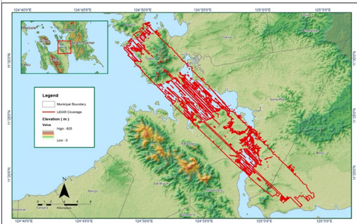
Figure A-8.32. Coverage of LiDAR data
