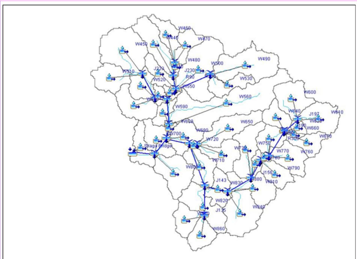
Figure 64. Silaga river basin model generated in HEC-HMS
