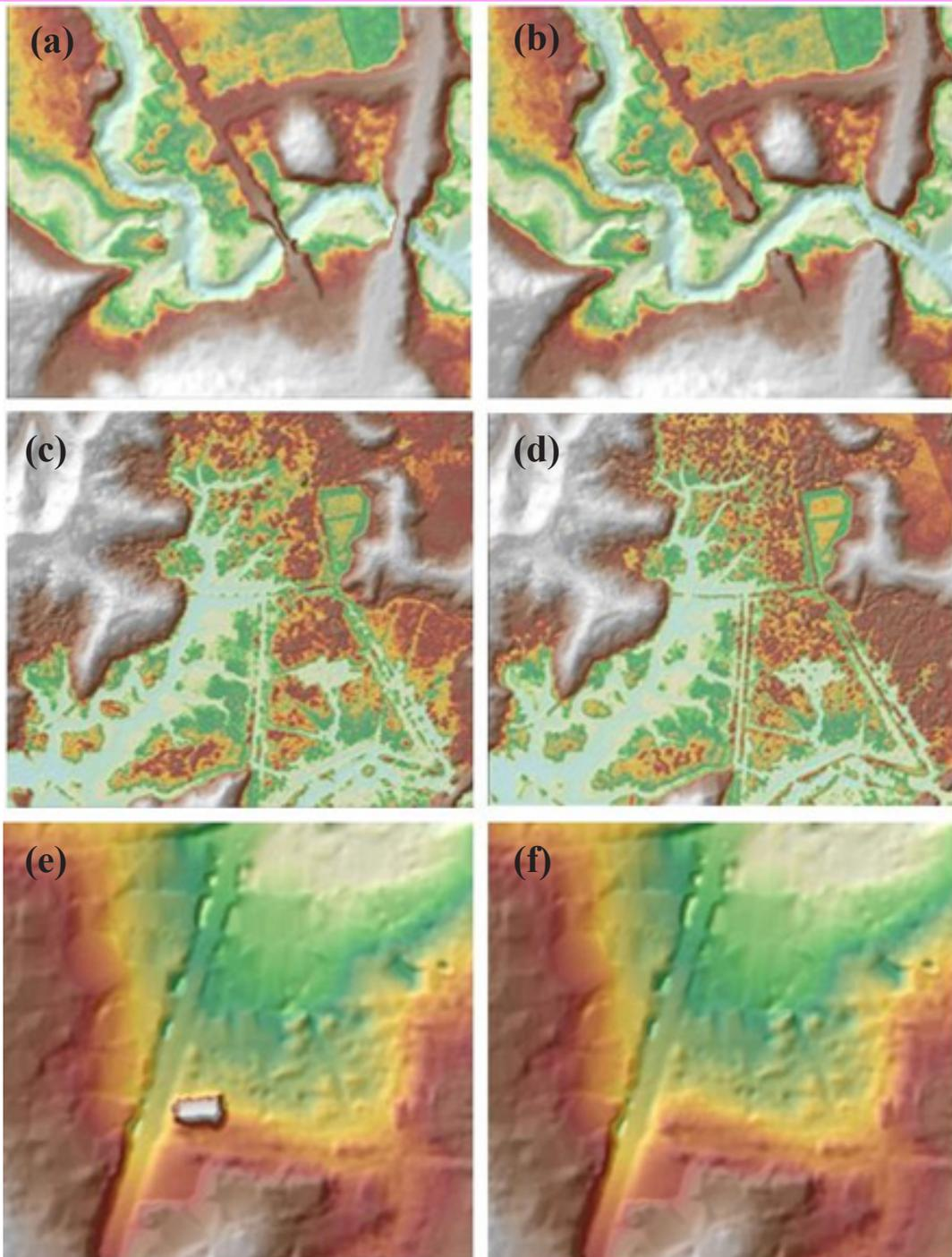
Figure 25. Portions in the DTM of Silaga Floodplain – a bridge before (a) and after (b) manual editing; a paddy field before (c) and after (d) data retrieval; and a building before (e) and after (f) manual editing.
