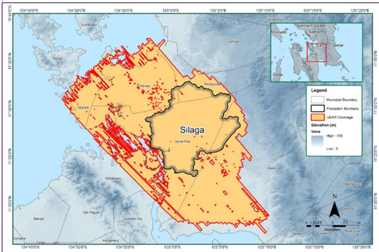
Figure 15. Boundaries of the processed LiDAR data on top of a SAR Elevation Data over Silaga Floodplain.
