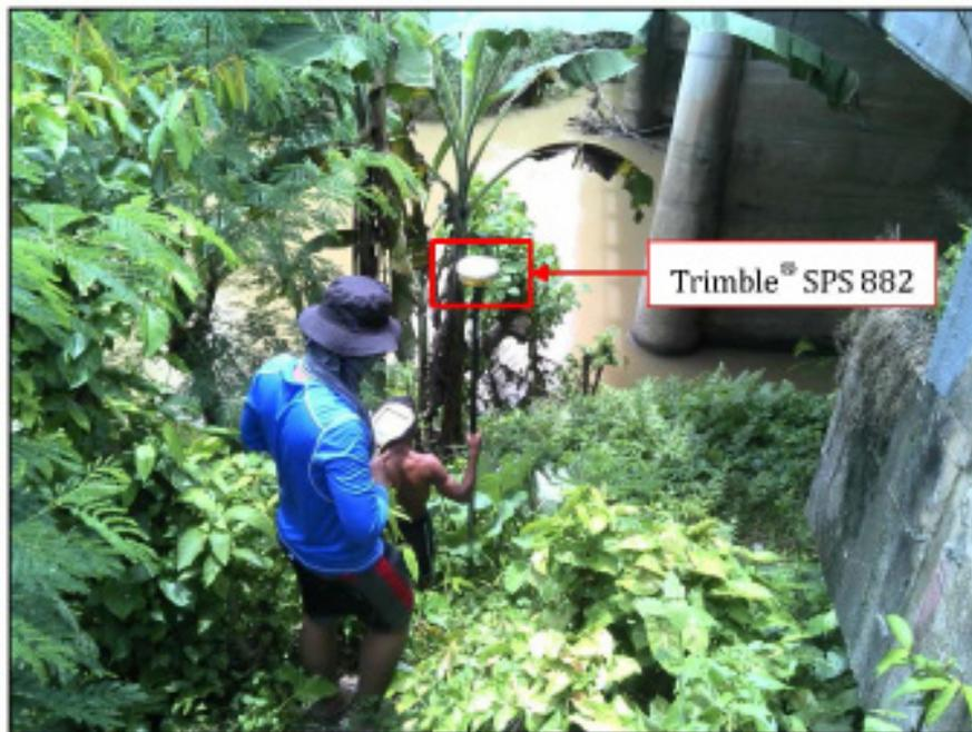
Figure 44. The Cross-section survey conducted at Silaga Bridge in Brgy. Tominamos, Sta. Rita, Samar.
