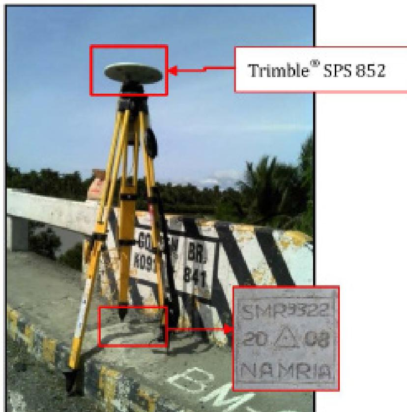
Figure 38. The GNSS (Trimble® SPS 852) base occupation at SMR-3322, located at the approach of Golden Bridge in Brgy. Binongtu-an in the Municipality of Basey, Samar.
