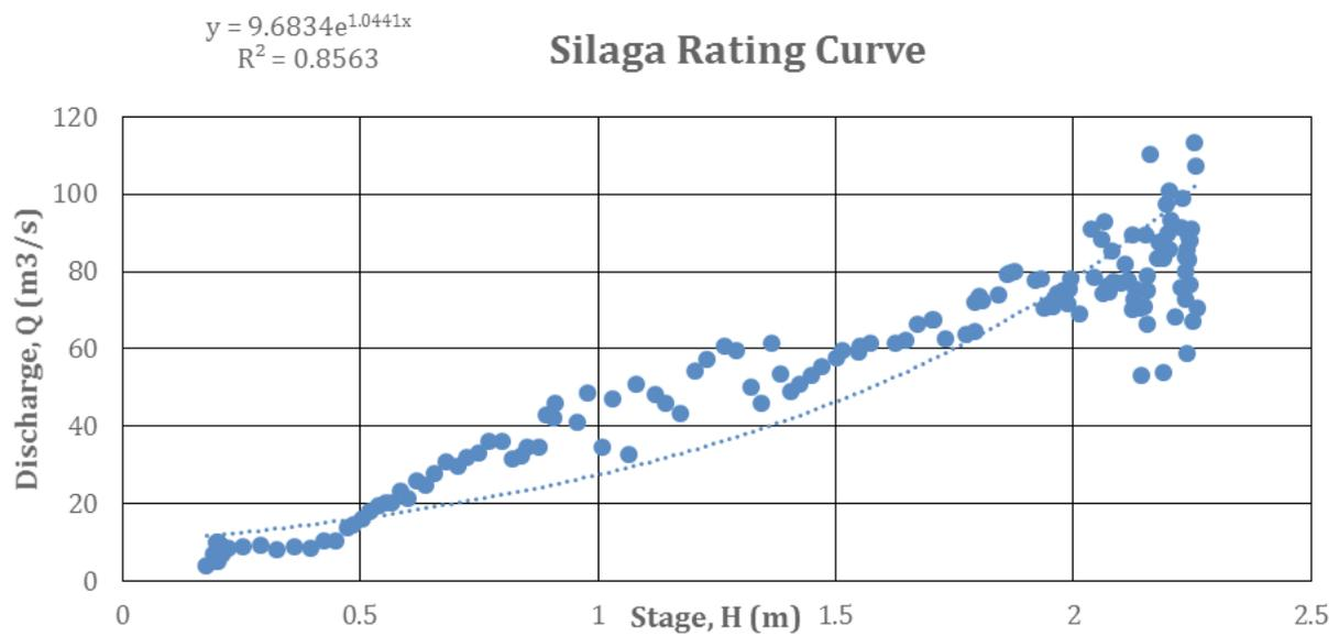
Figure 56. Rating curve of the Silaga Bridge in Sta. Rita, Samar.
