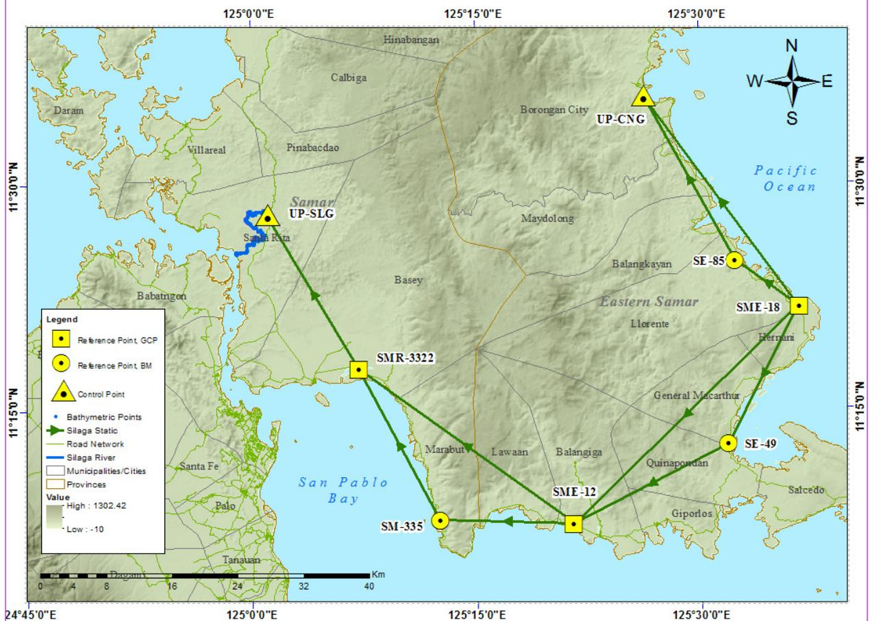
Figure 34. The GNSS Network established in the Silaga River Survey.
