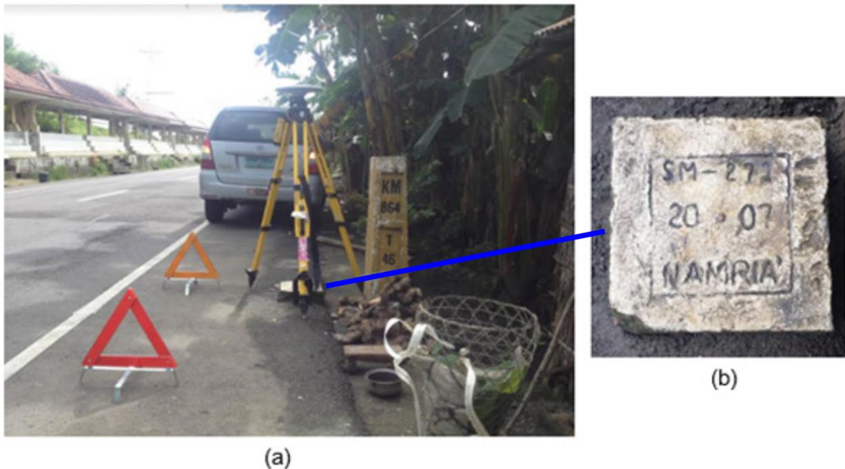
Figure 7. Photo (A) depicts the GPS set-up over SM-271 located beside Kilometer Post 864 along the right side of the National Highway, Bgry. Laygayon, Pinabacdao, Samar; while Photo (B) shows a close-up view of NAMRIA reference point SM-271 as recovered by the field team.
