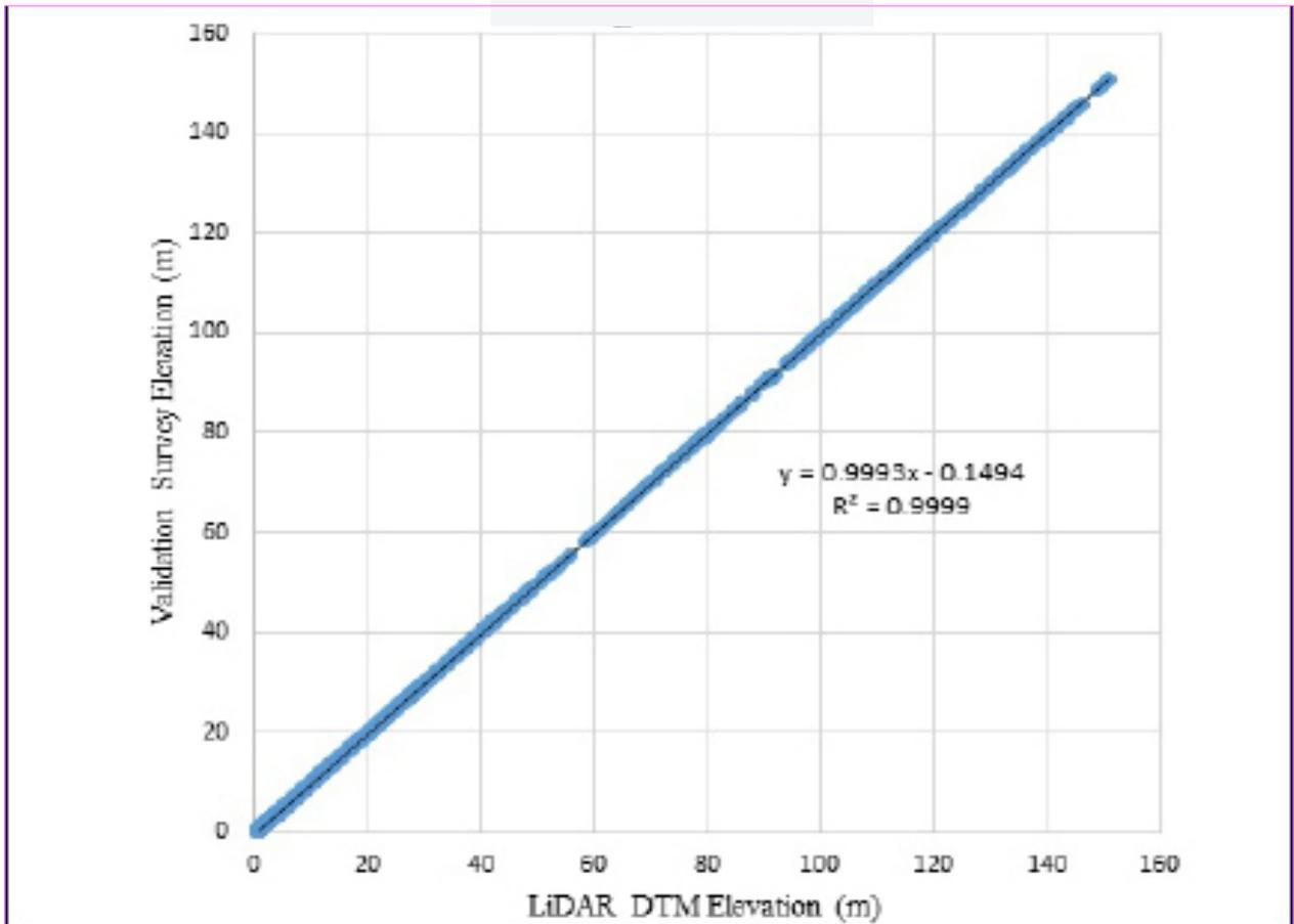
Figure 29. Correlation plot between validation survey points and LiDAR data.
