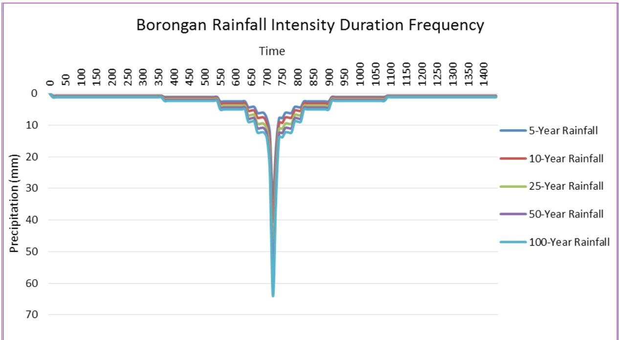
Figure 52. The synthetic storm generated for a 24-hour period rainfall for various return periods.
