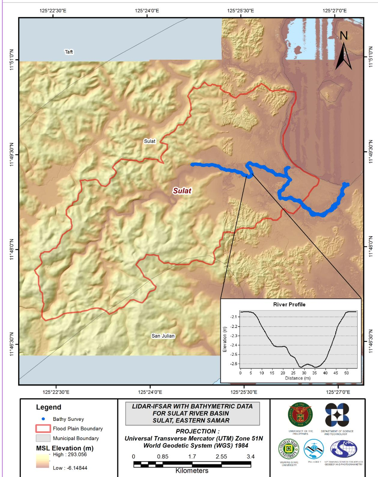
Figure 25. Map of Sulat floodplain with bathymetric survey points in blue.
