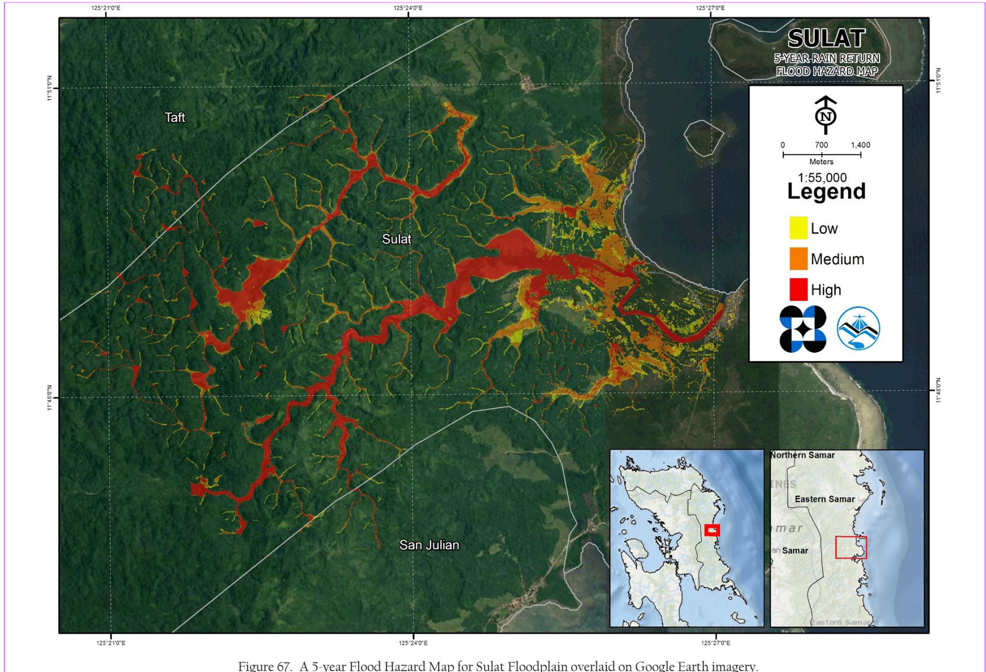
Figure 67. A 5-year Flood Hazard Map for Sulat Floodplain overlaid on Google Earth imagery.
