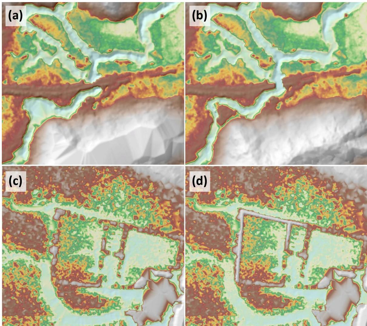
Figure 20. Portions in the DTM of the Sulat Floodplain – a bridge before (a) and after (b) manual editing; a paddy field before (c) and after (d) data retrieval.
