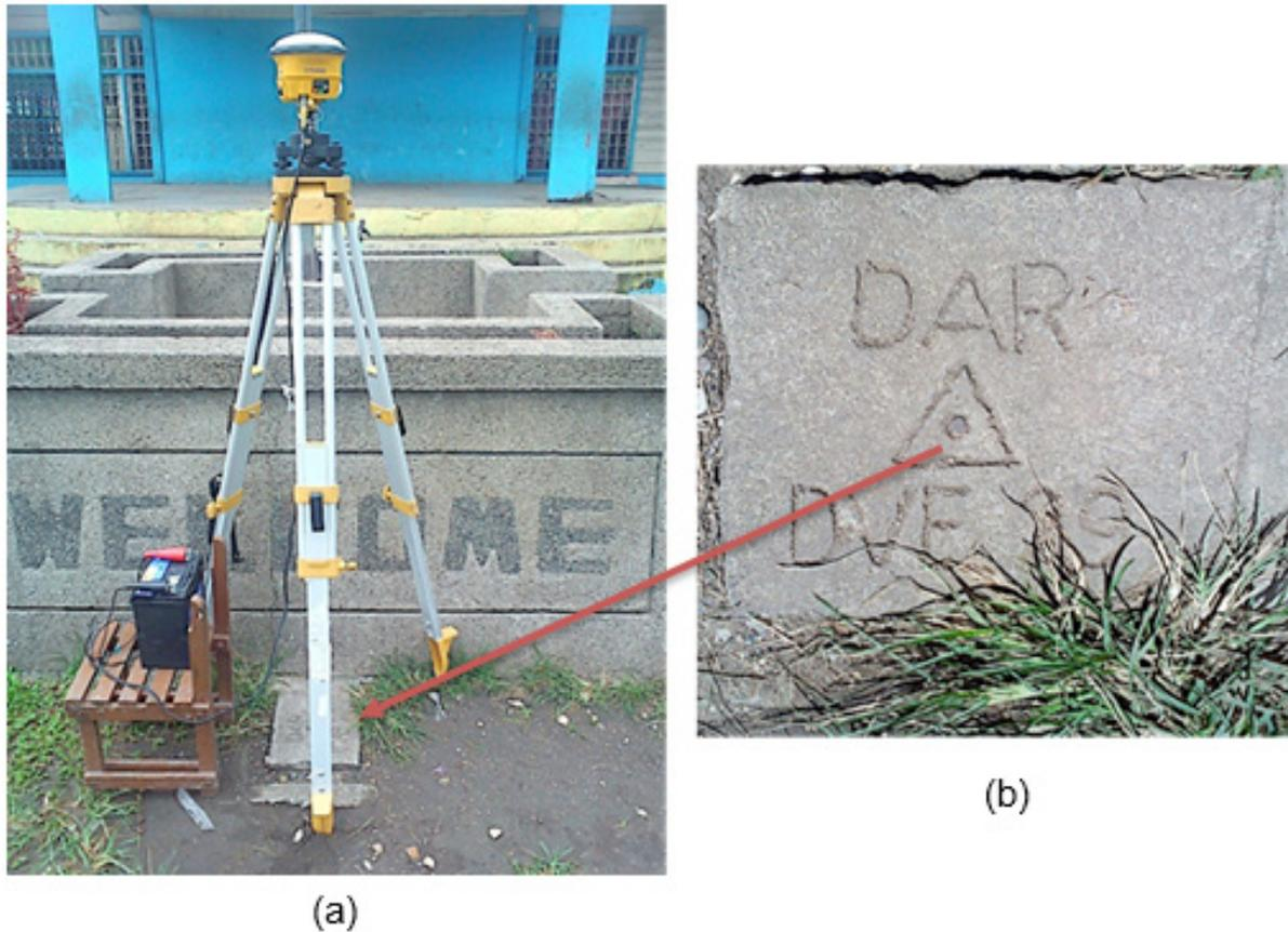
Figure 4. GPS set-up over SE-16 located in front of the flagpole of Gregorio Moralizon Elementary School II (a) and NAMRIA reference point DVE-19 (b) as recovered by the field team.
