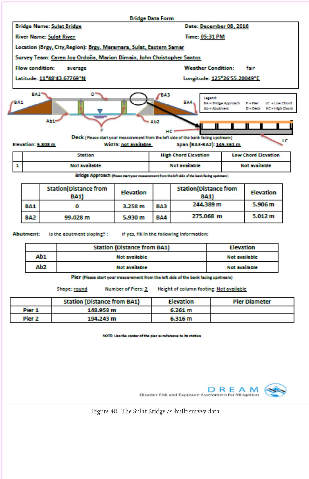
Figure 40. The Sulat Bridge as-built survey data.
