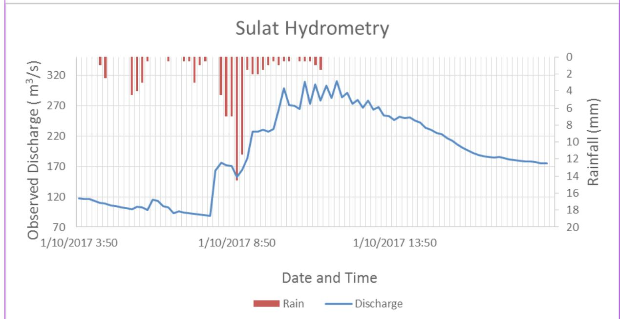
Figure 50. Rainfall and outflow data at Sulat Bridge, which was used for modeling.
