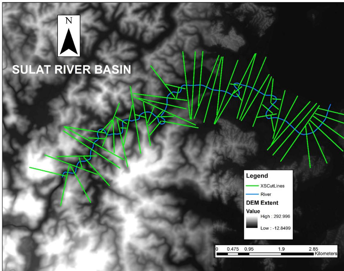
Figure 58. River cross-section of the Sulat River through the ArcMap HEC GeoRas tool.
