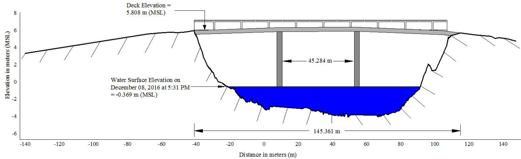
Figure 39. The Sulat Bridge cross-section diagram.
