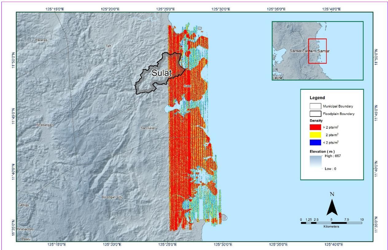
Figure 12. Pulse density map of the merged LiDAR data for Sulat floodplain..
