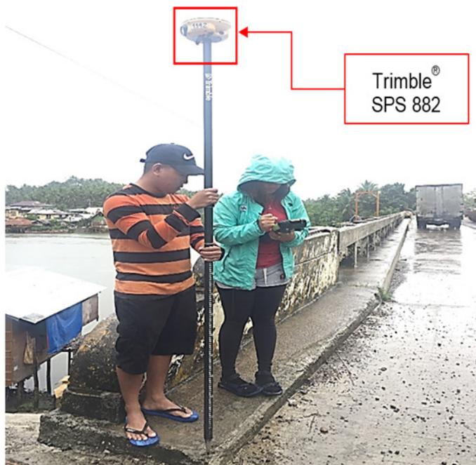
Figure 37. As-built survey conducted at Sulat Bridge.
