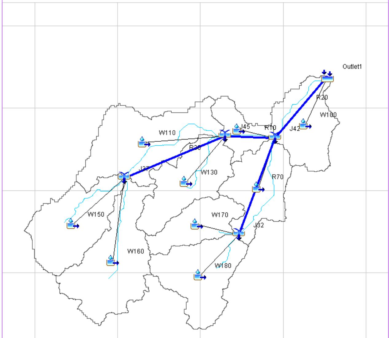
Figure 57. Sulat river basin model generated in HEC-HMS.
