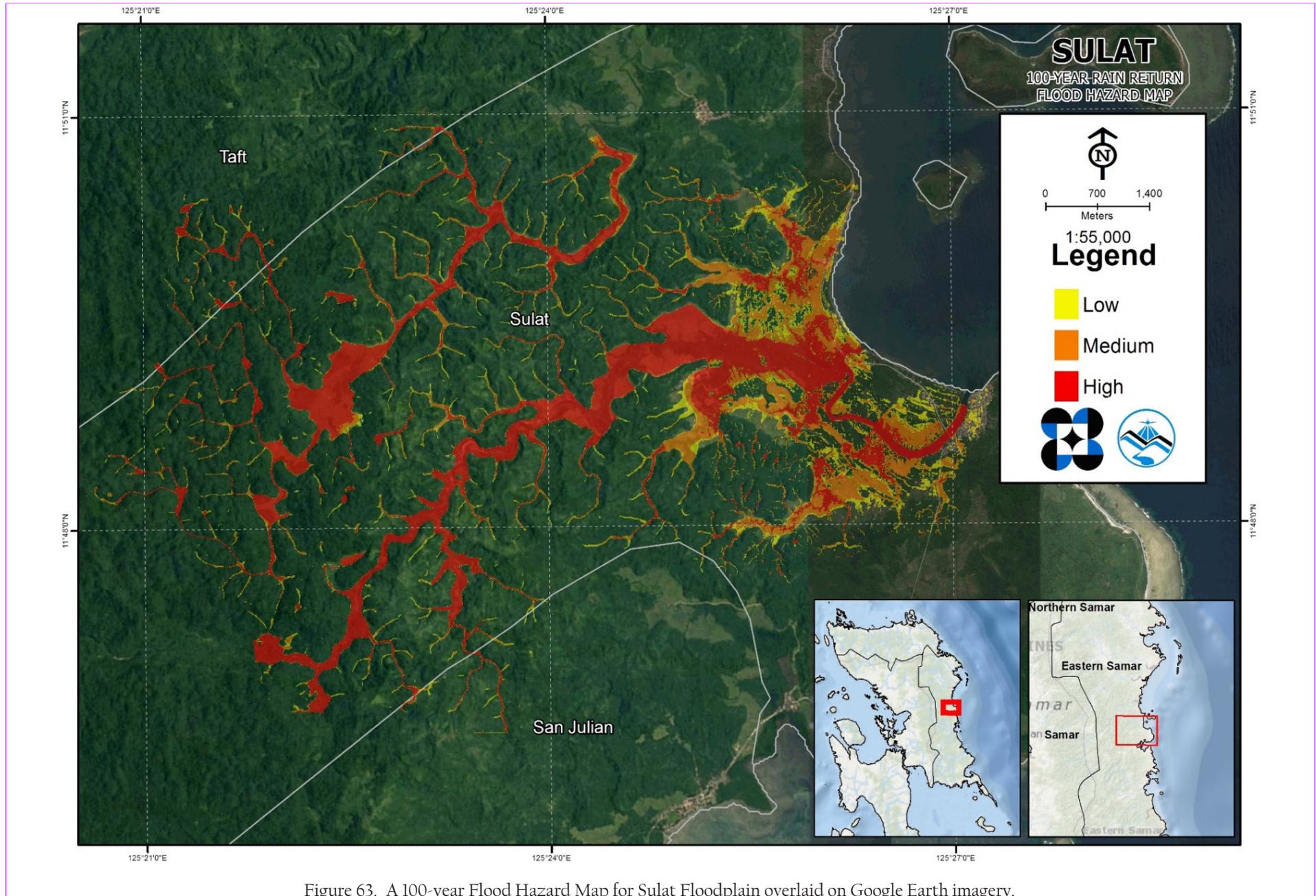
Figure 63. A 100-year Flood Hazard Map for Sulat Floodplain overlaid on Google Earth imagery.
