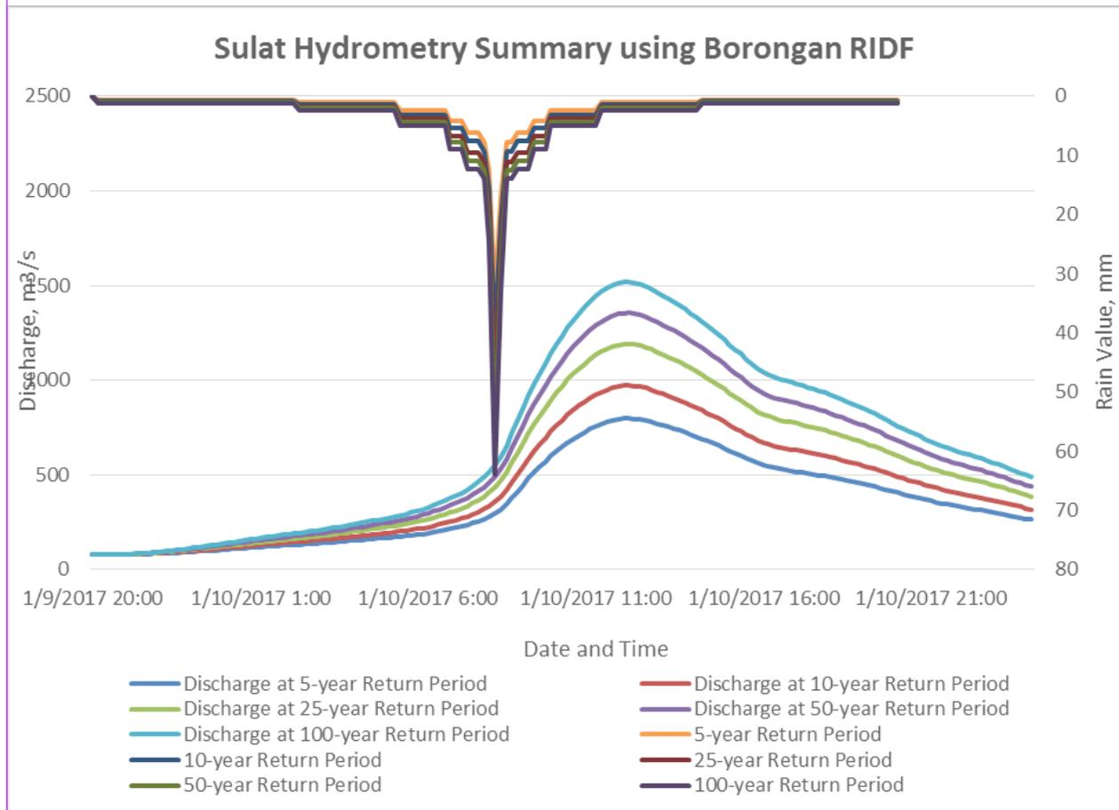
Figure 61. The Outflow hydrograph at the Sulat Station, generated using the Borongan RIDF simulated in HEC-HMS.
