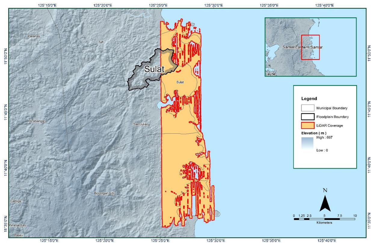
Figure 10. Boundaries of the processed LiDAR data over the Sulat Floodplain.
