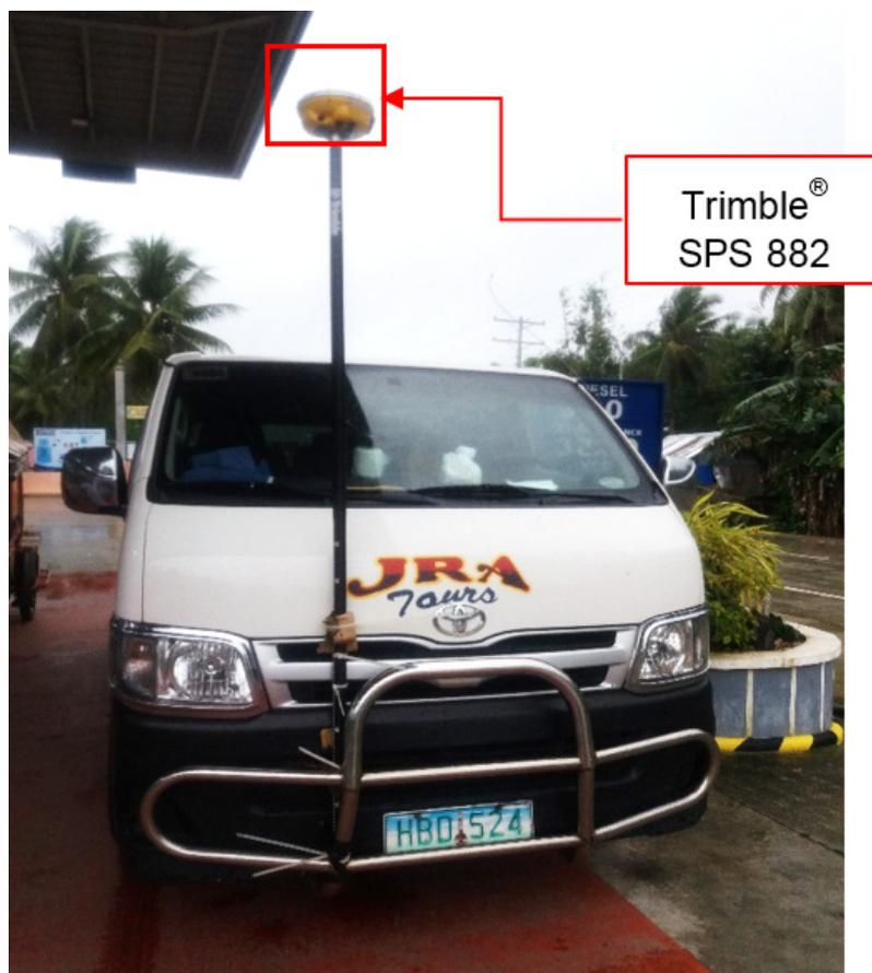
Figure 42. GNSS Receiver Trimble® SPS 882 installed on a vehicle for Ground Validation Survey.
