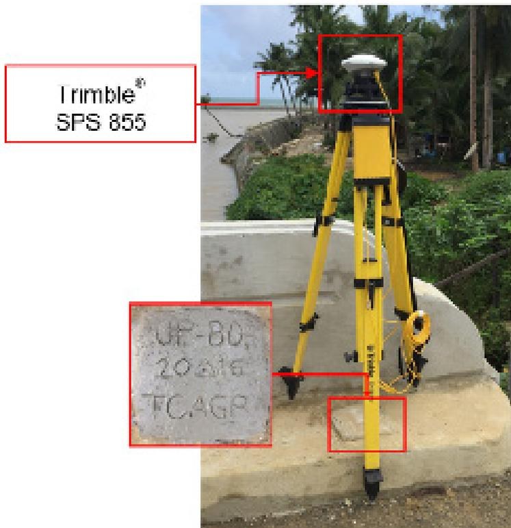
Figure 33. GNSS receiver set up, Trimble® SPS 855, at UP-BOR, located at the approach of Can-Obing Bridge in Brgy. Can-Abong, Borongan City, Eastern Samar
