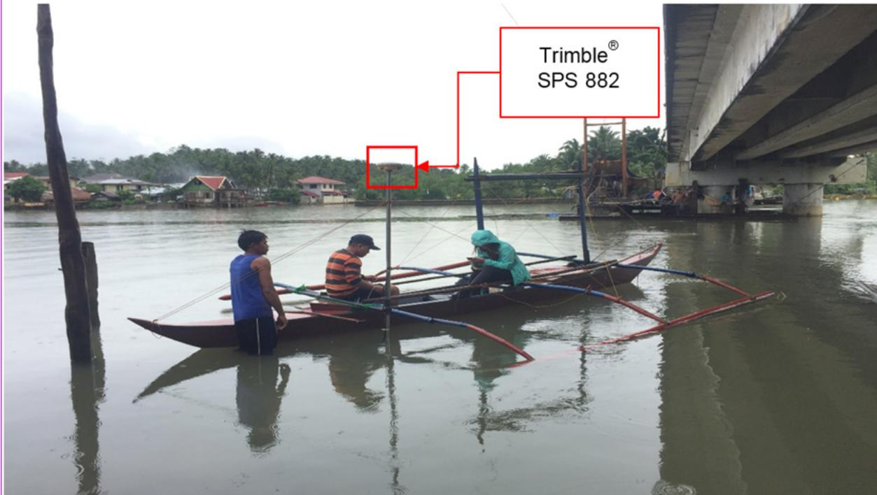
Figure 44. Set up of the bathymetric survey at Sulat River using Trimble® SPS 882 in GNSS PPK survey technique.
