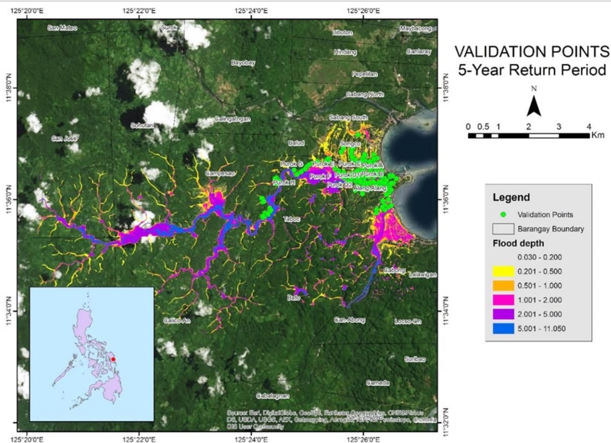
Figure 78. Validation Points for a 5-year Flood Depth Map of the Sulat Floodplain.
