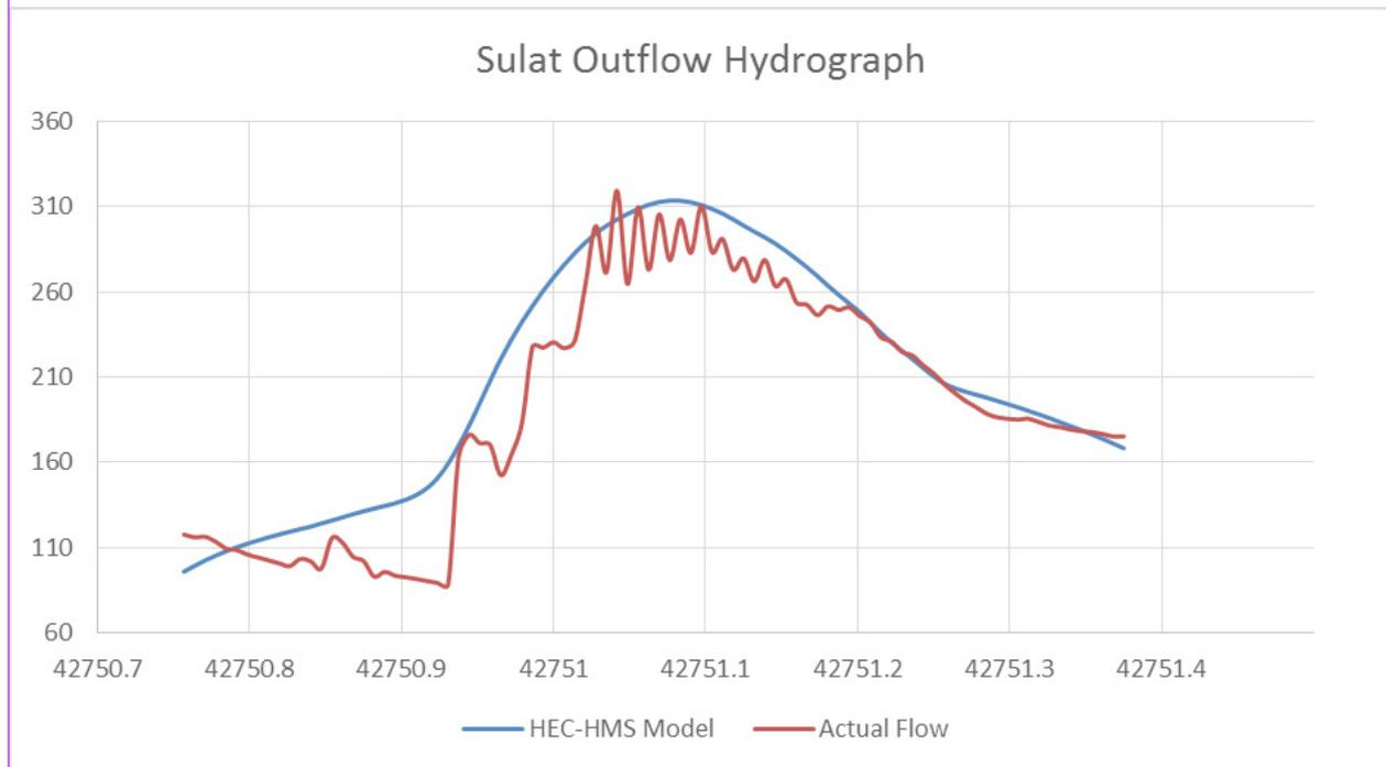
Figure 60. Outflow Hydrograph of Sulat produced by the HEC-HMS model compared with observed outflow.
