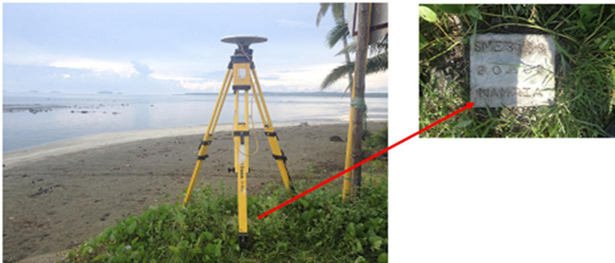
Figure 3. GPS set-up over SME-3139 located along the highway in Brgy. Sto. Nino, Sulat, Eastern Samar (a) and NAMRIA reference point SME-3139 (b) as recovered by the field team.
