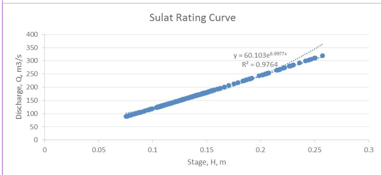
Figure 49. The rating curve at Sulat Bridge, Sulat, Samar.
