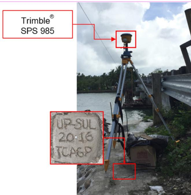
Figure 34. GNSS receiver set up, Trimble® SPS 985, at UP-SUL, located at the approach of Sulat Bridge in Brgy. Maramara, Municipality of Sulat, Eastern Samar
