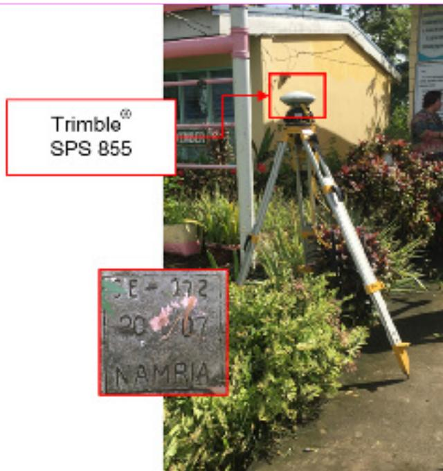
Figure 32. GNSS receiver set up, Trimble® SPS 855 at SE-172, located in Brgy. Nato, Municipality of Taft, Eastern Samar
