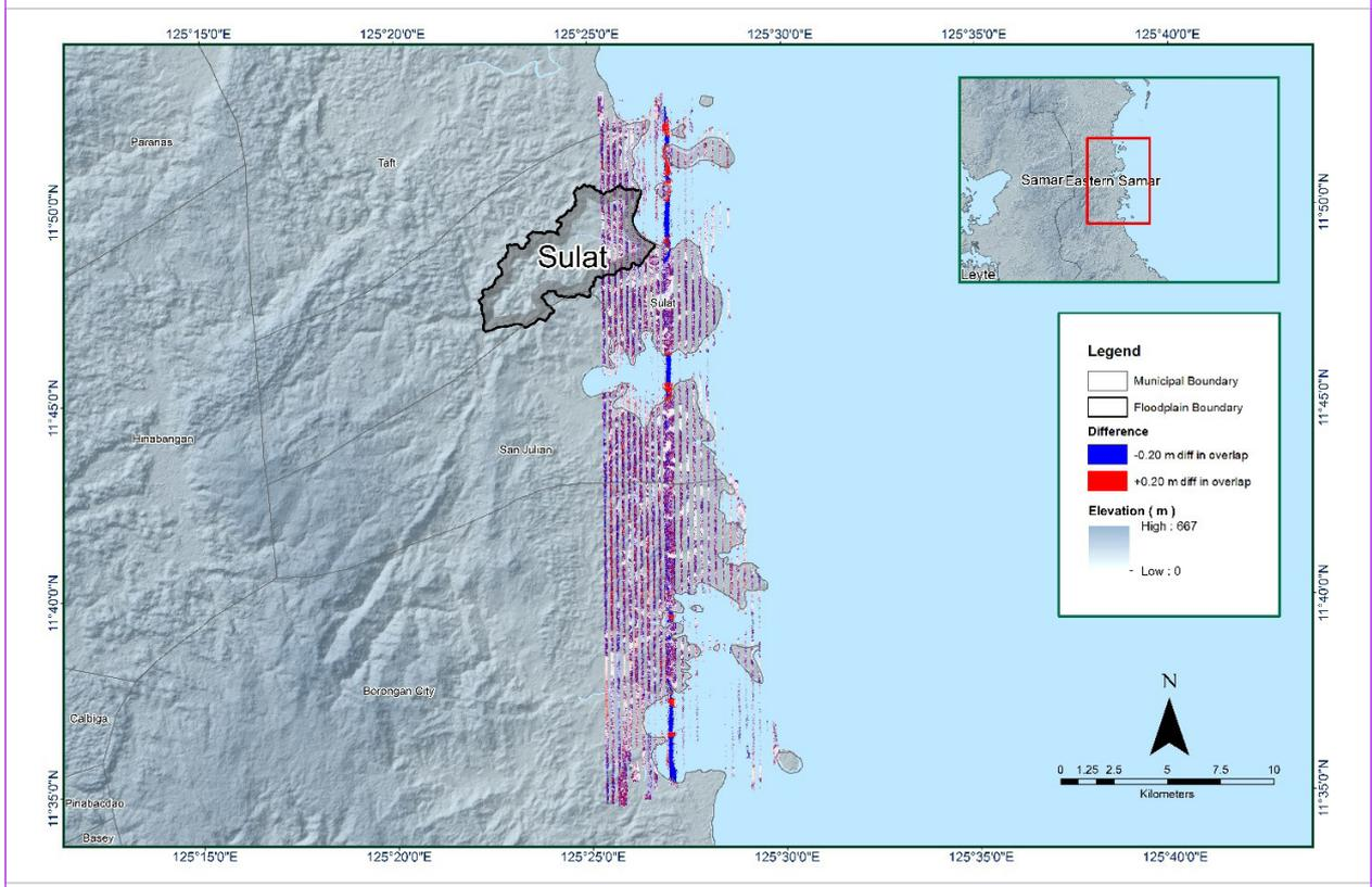
Figure 13. Elevation difference Map between flight lines for the Sulat Floodplain Survey.
