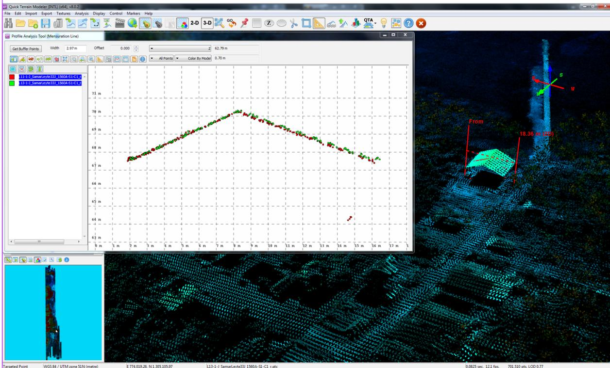
Figure 14. Quality checking for Sulat flight 1560A using the Profile Tool of QT Modeler.
