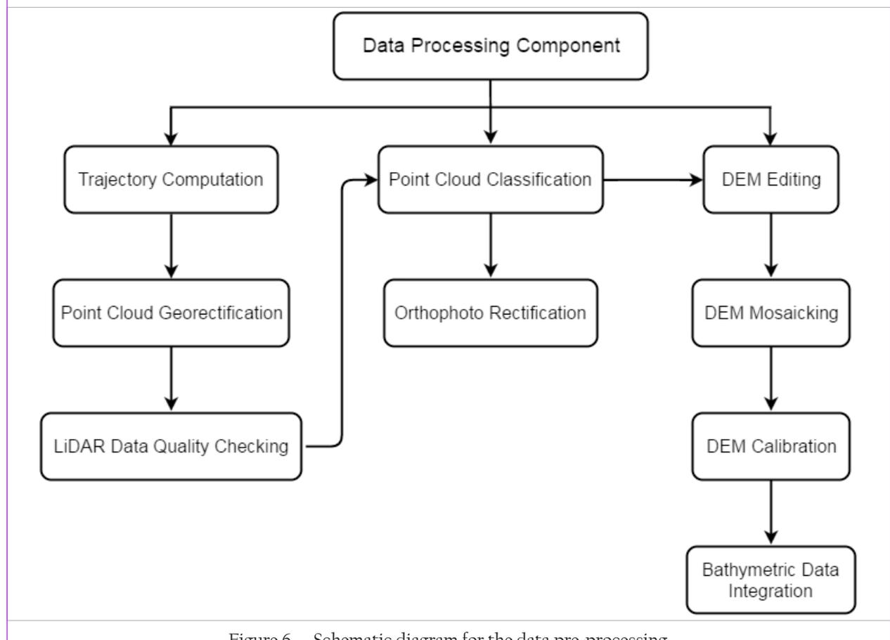
Figure 6. Schematic diagram for the data pre-processing.
