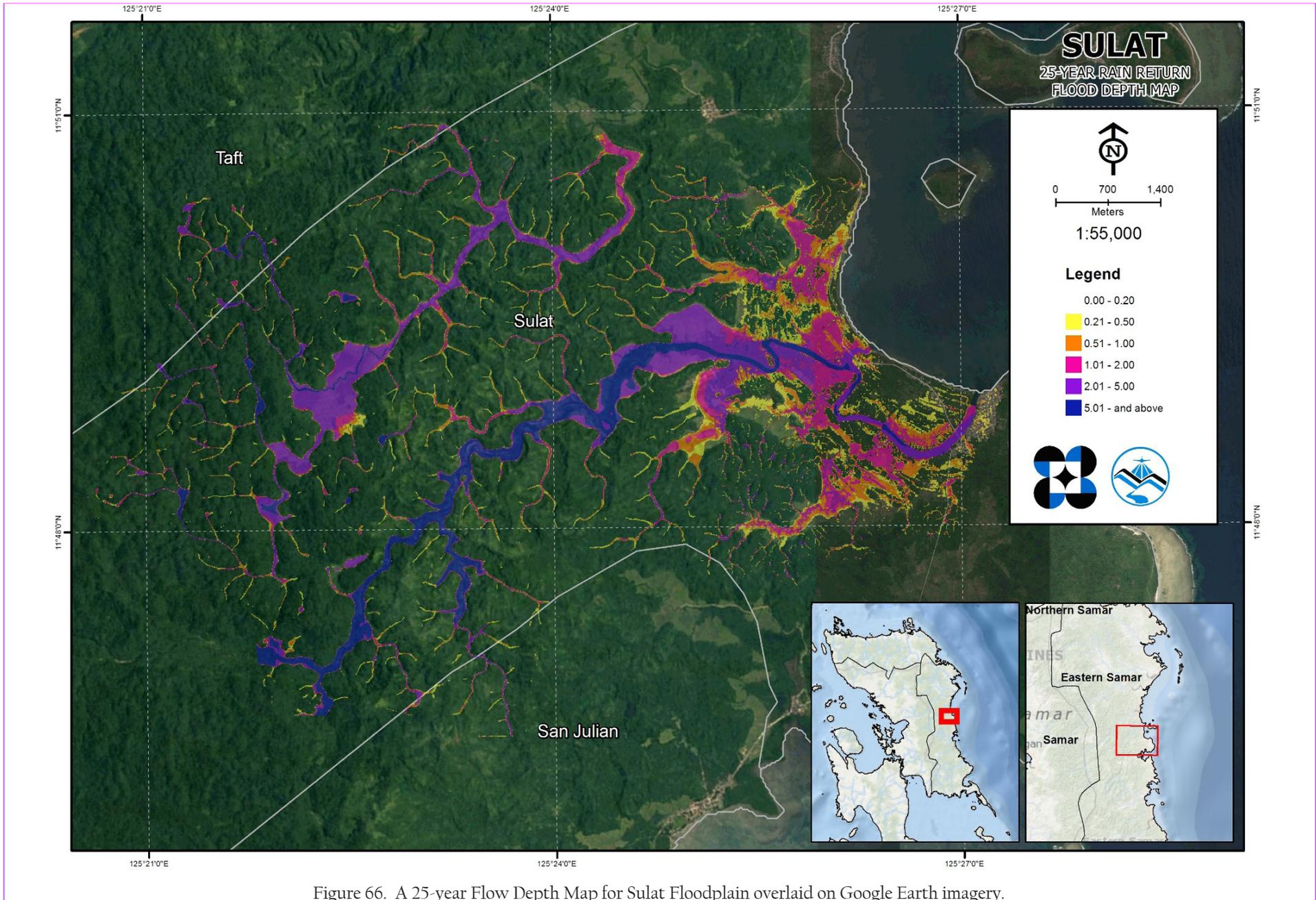
Figure 66. A 25-year Flow Depth Map for Sulat Floodplain overlaid on Google Earth imagery.
