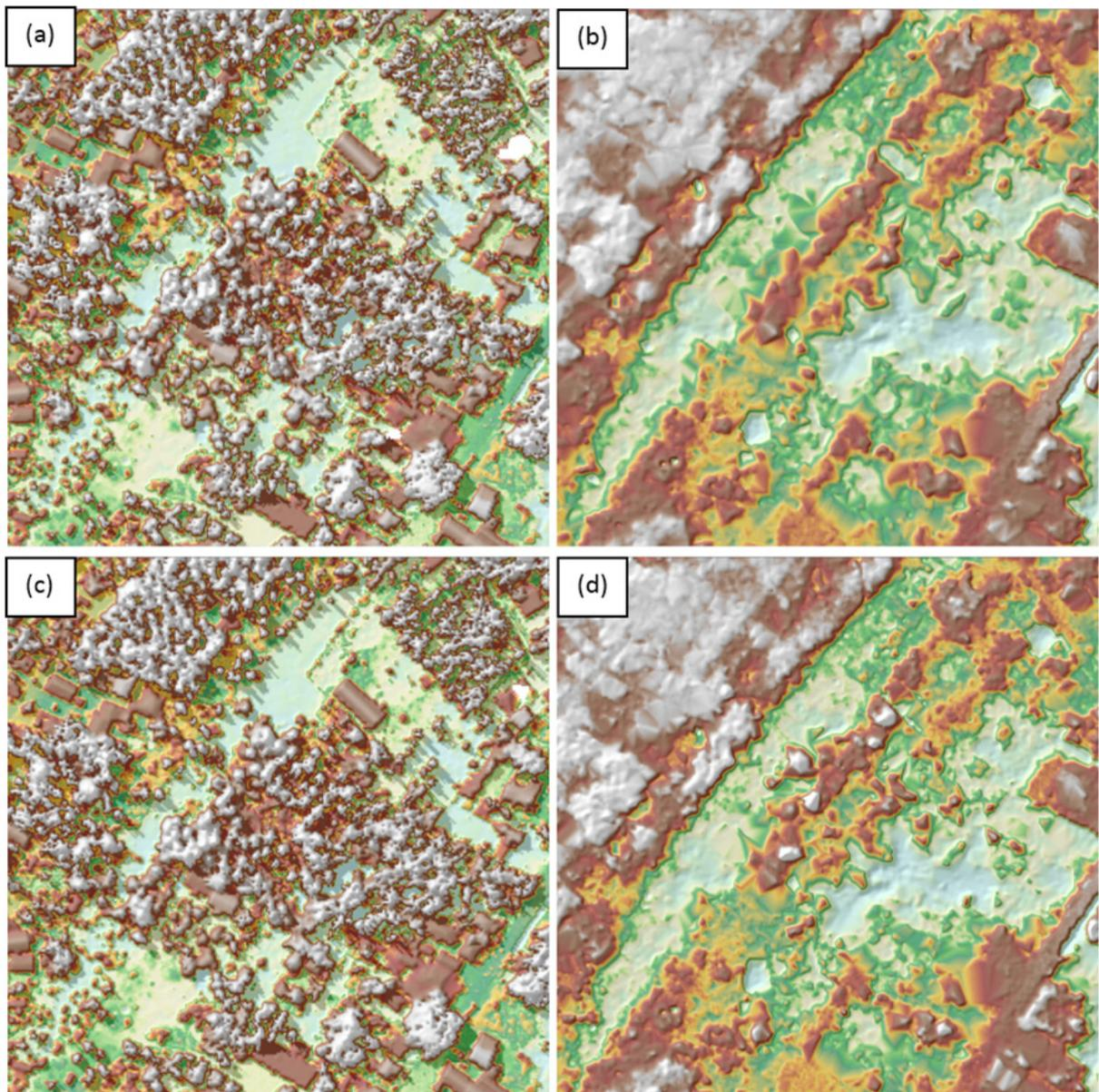
Figure 17. The production of last return DSM (a) and DTM (b), first return DSM (c) and secondary DTM (d) in some portion of Sulat floodplain.
