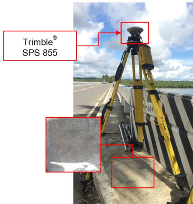
Figure 35. GNSS receiver setup, Trimble® SPS 855, at UP-ULO-2, located at the approach of Can-Avid Bridge in Brgy. Canteros, Municipality of Can-Avid, Eastern Samar
