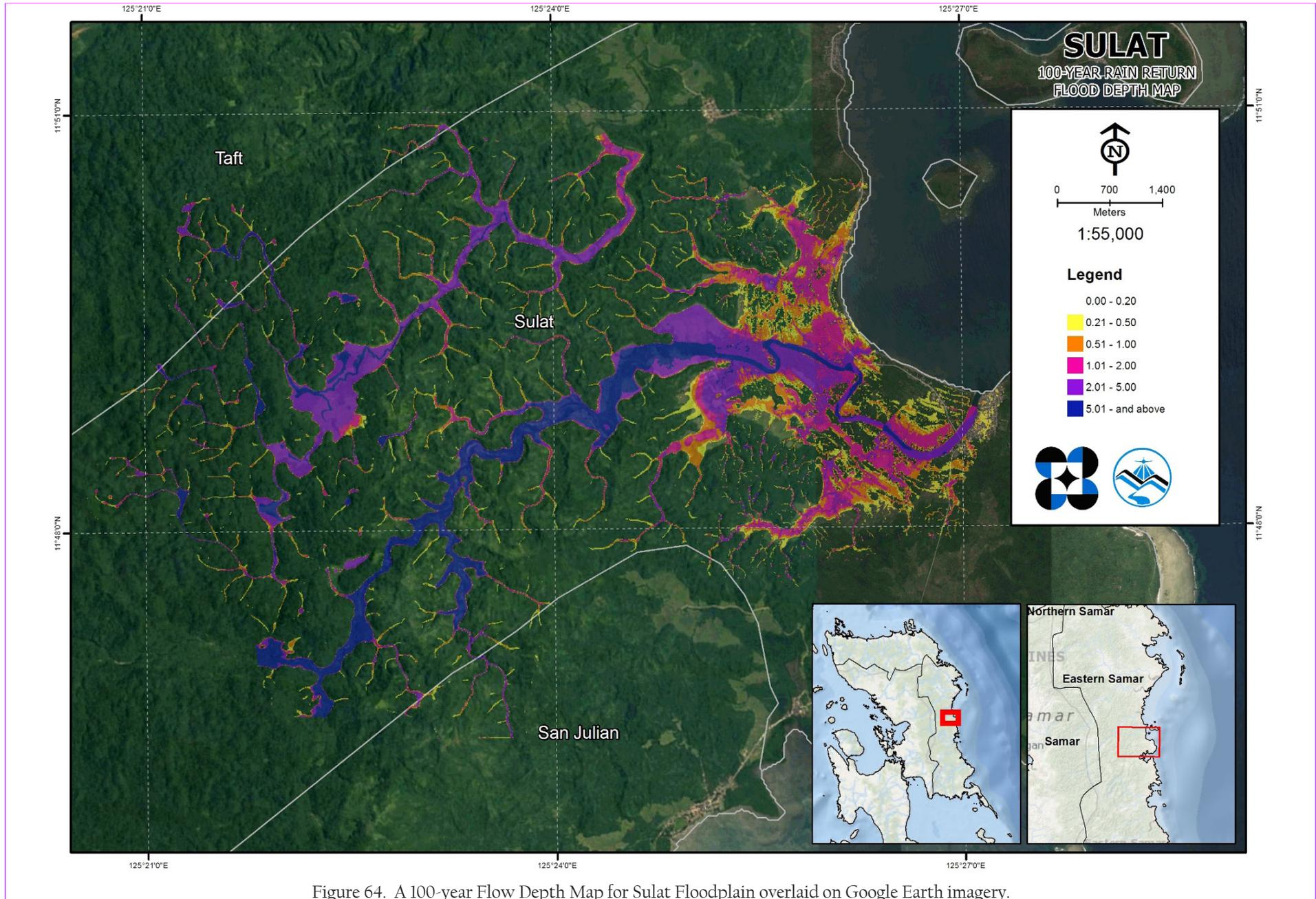
Figure 64. A 100-year Flow Depth Map for Sulat Floodplain overlaid on Google Earth imagery.
