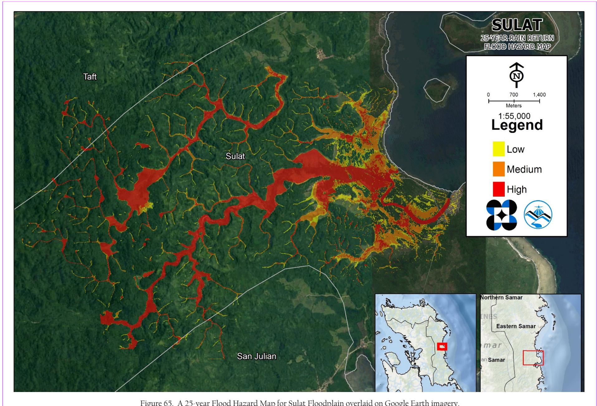
Figure 65. A 25-year Flood Hazard Map for Sulat Floodplain overlaid on Google Earth imagery.
