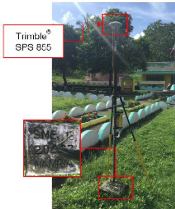
Figure 30. GNSS base set up, Trimble® SPS 852, SME-18, located within the grounds of San Jose Elementary School in Brgy. Canciledes, Municipality of Hernani, Eastern Samar
