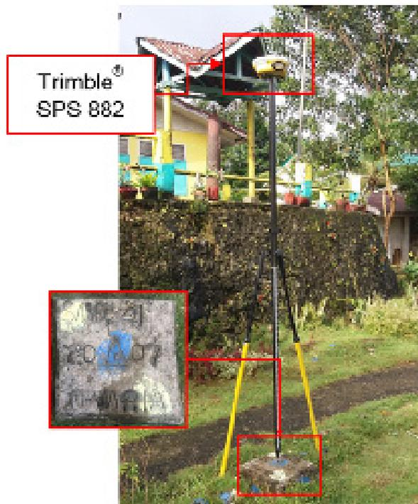
Figure 31. GNSS receiver set up, Trimble® SPS 882, at SMR-41, located in Brgy. Fatima, Municipality of Hinabangan, Samar.
