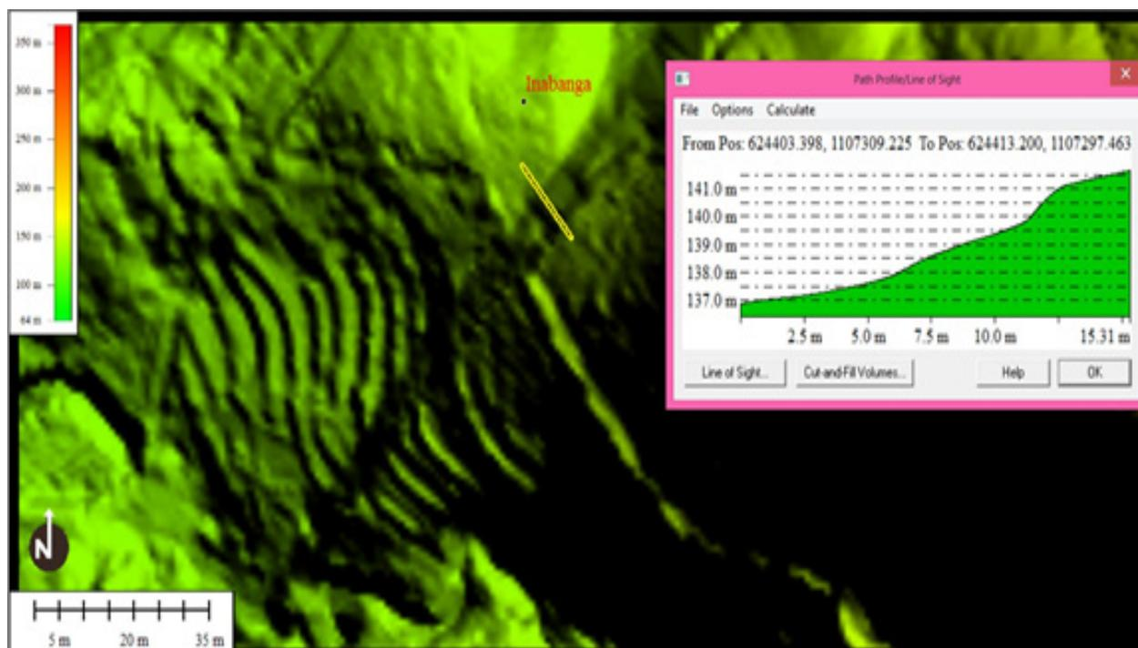
Figure 47. Profile view of the yellow line in the DTM, showing the 4m uplift in Inabanga
