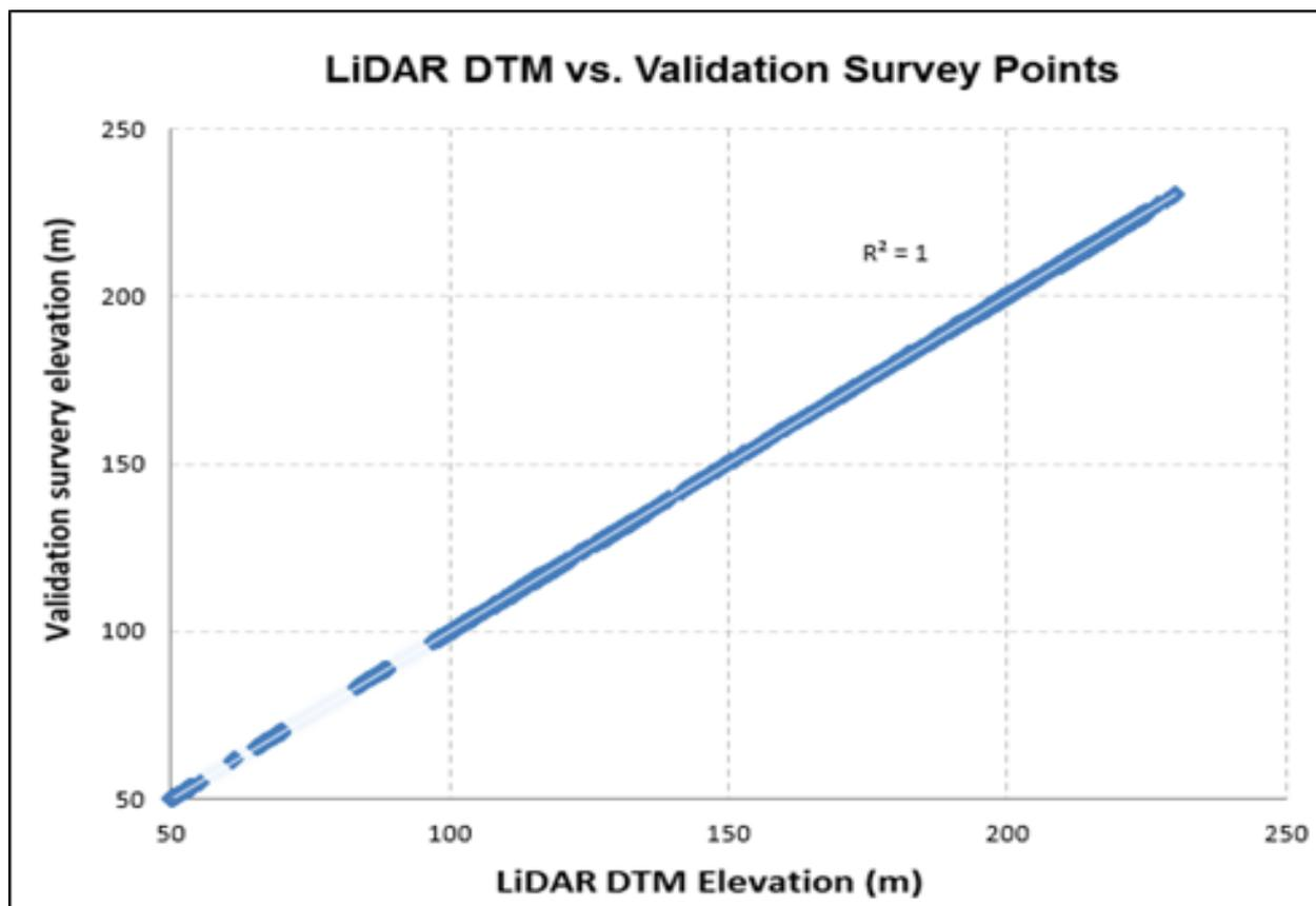
Figure 39. One-one Correlation plot between topographic and LiDAR data
