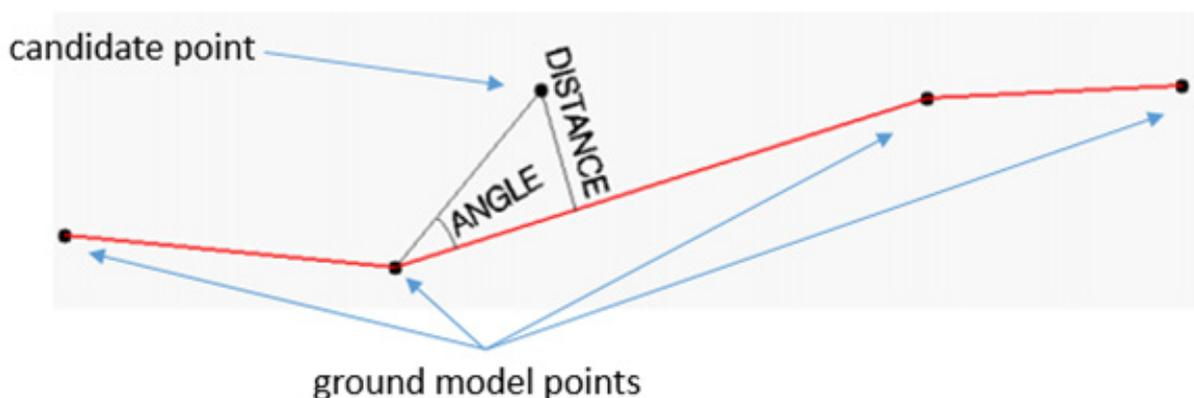
Figure 13. Ground classification technique employed in Terrascan
