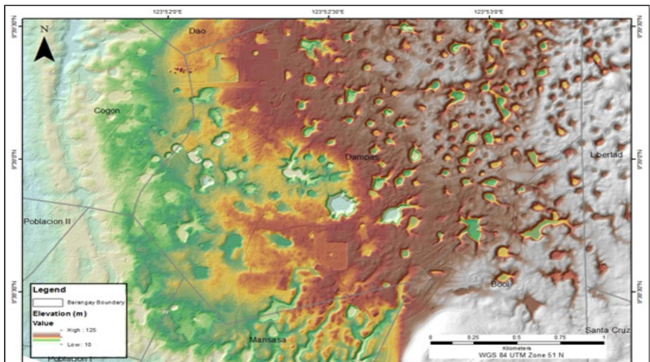
Figure 45. Final DTM in Tagbilaran showing presence of sink holes
