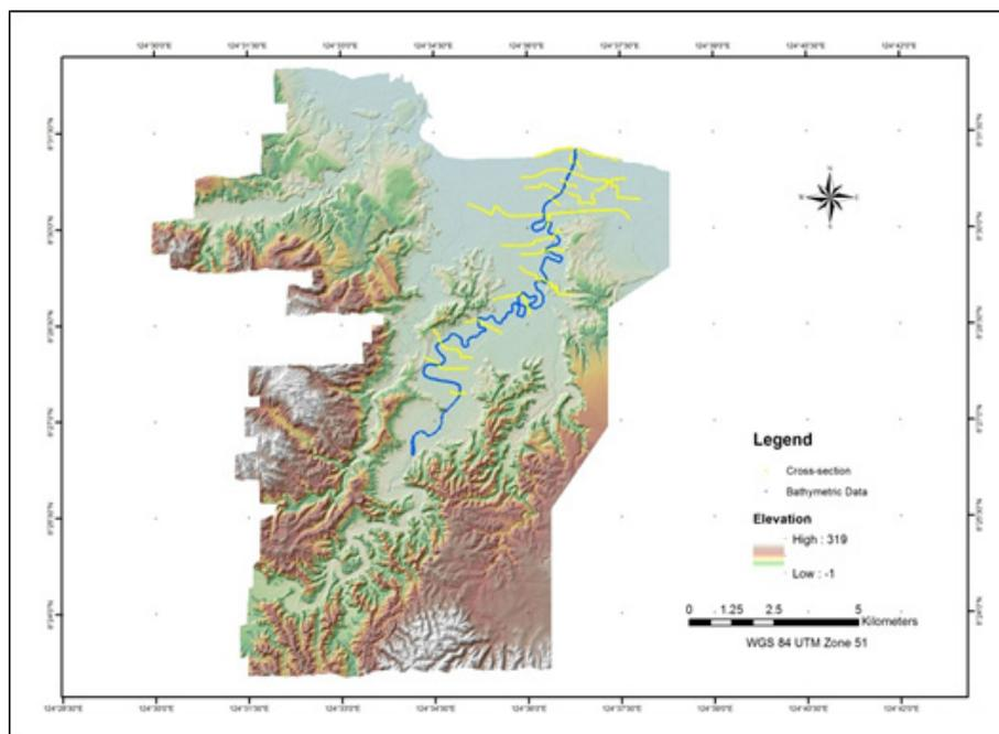
Figure 40. Final DTM of Iponan with validation survey shown in blue
