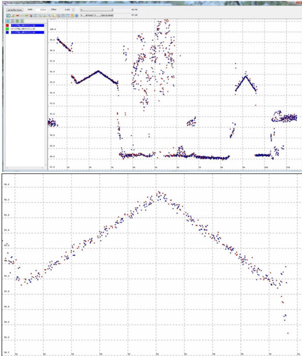
Figure 15. Profile over roof planes (a) and a zoomed-in profile on the area encircled in yellow (b)
