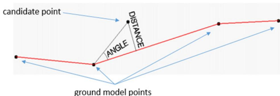
Figure 16. Ground classification technique employed in Terrascan
