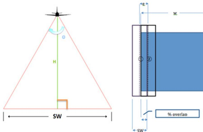
Figure 9. Concept of LiDAR data acquisition parameters
