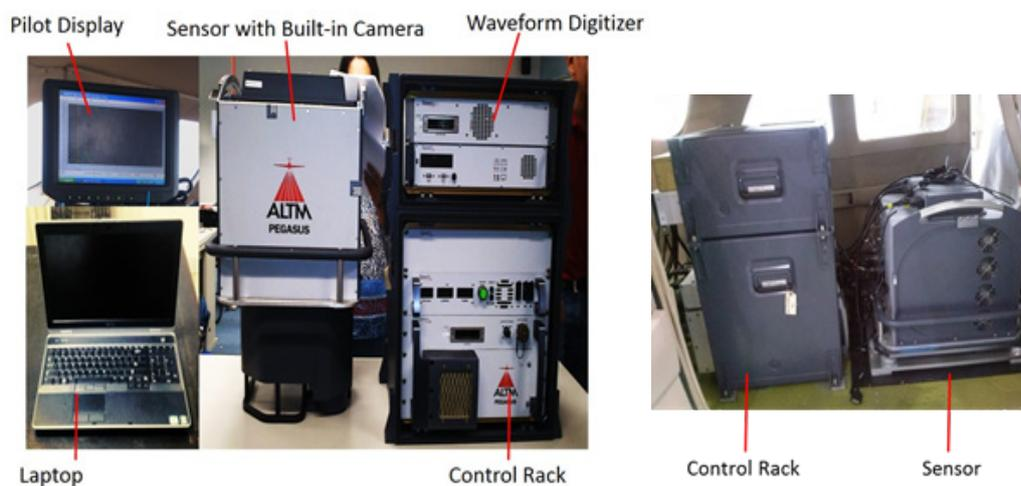
Figure 11. The ALTM Pegasus System: a) parts of the Pegasus system, b) the system as installed in Cessna T206H
