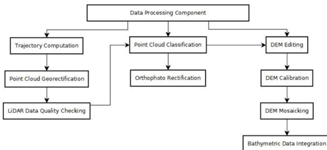
Figure 12. Schematic diagram of the data processing
