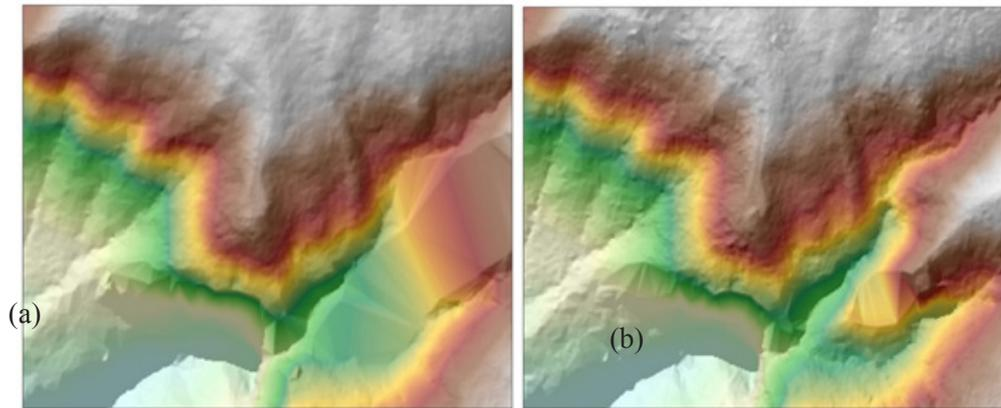
Figure 17. Resulting DTM of ground classification using the default parameters (a) and adjusted parameters (b)
