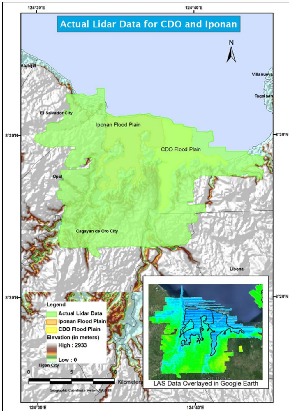
Figure 23. Cagayan de Oro and Iponan floodplain data acquisition LAS output
