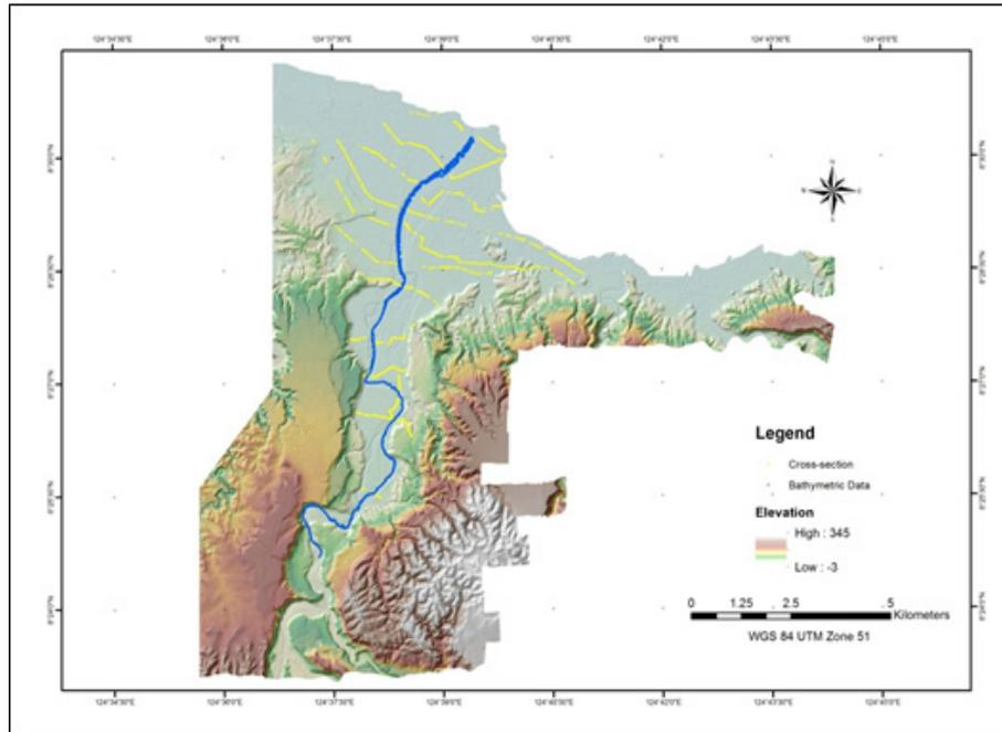
Figure 39. Final DTM of Cagayan de Oro with validation survey shown in blue
