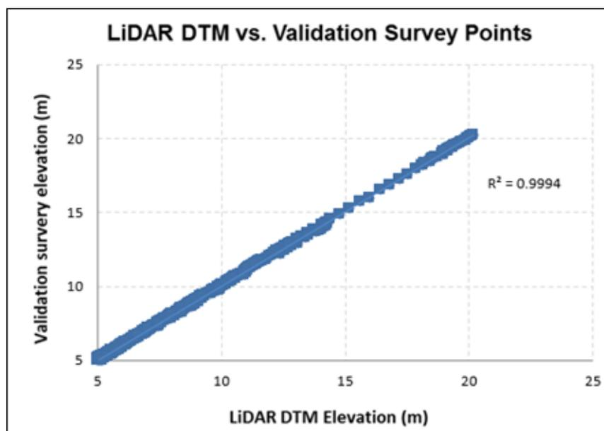
Figure 30. One-one Correlation plot between topographic and LiDAR data
