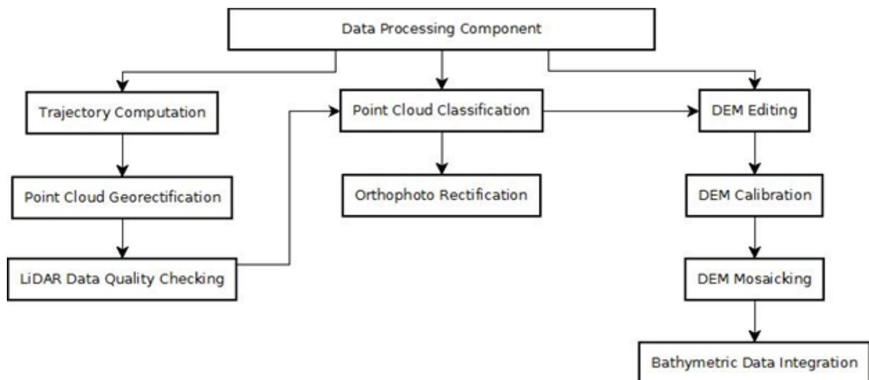
Figure 9. Schematic diagram of the data processing
