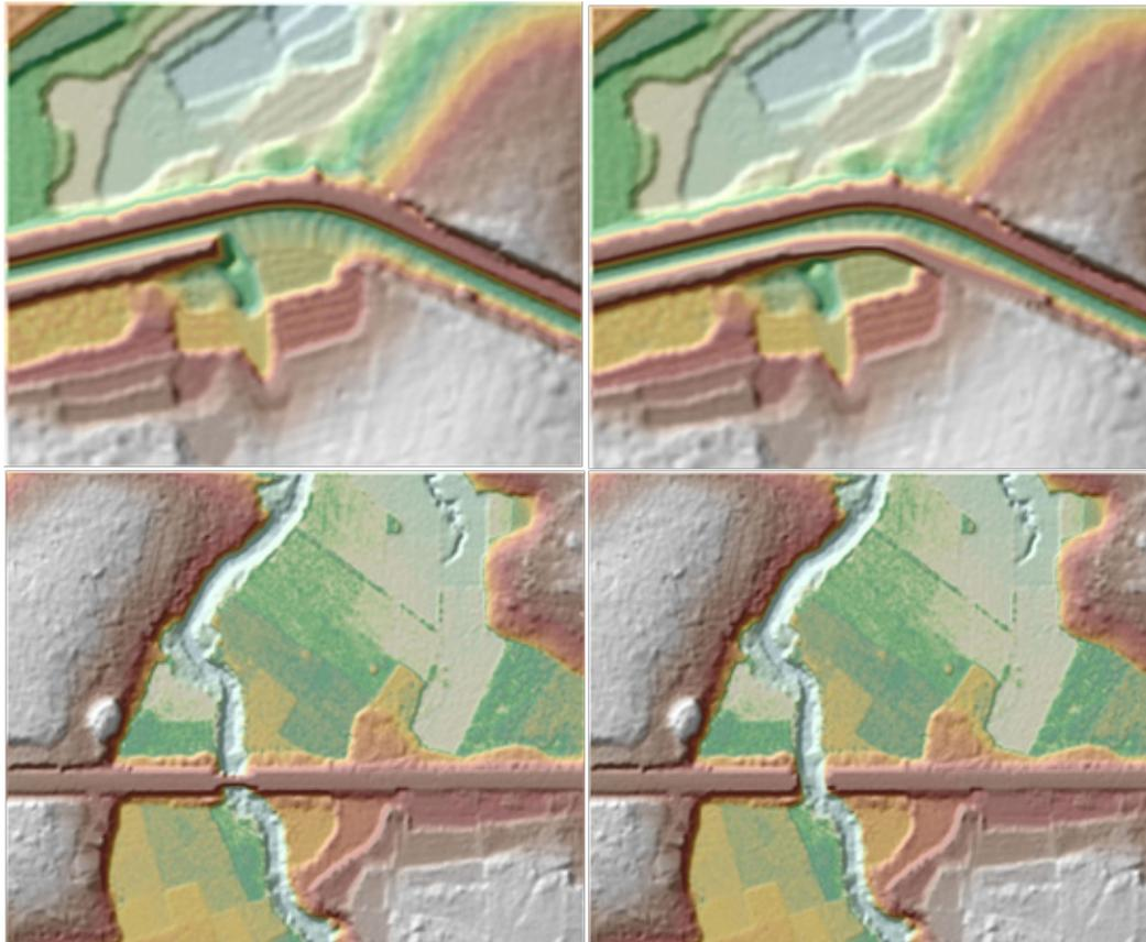
Figure 28. Images of DTMs before and after manual editing. Image (a) shows an embankment that might have been cut by the classification routine while image (b) shows the changes in the same area after manual editing. Image (c) and (d) show an example of a stream
