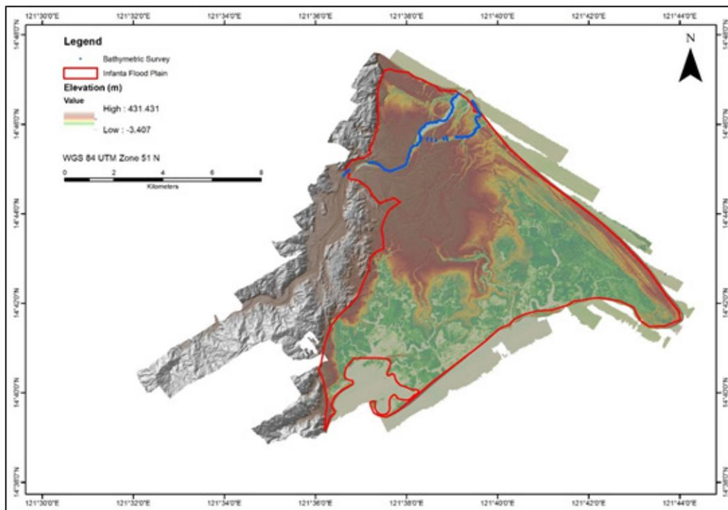
Figure 31. Final DTM of Infanta with validation survey shown in blue
