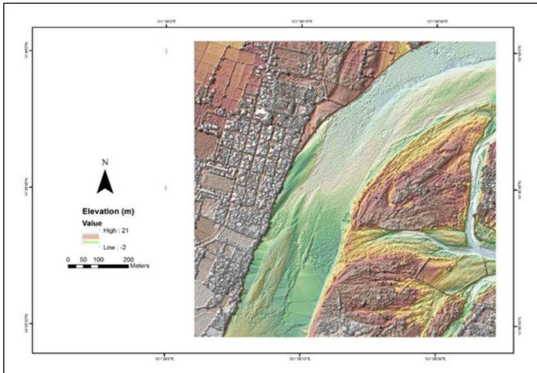
Figure 33. Sample 1x1 Square Kilometer DSM.
