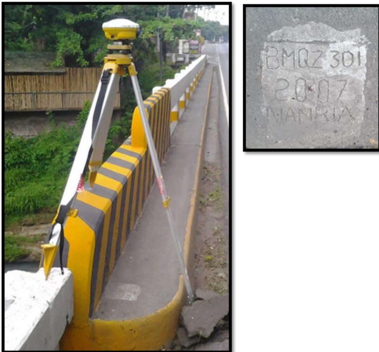
Figure 18. NAMRIA control station MSE-3241 is located along the national highway on the SE corner of Masin bridge (106+600) in Candelaria, Quezon.
