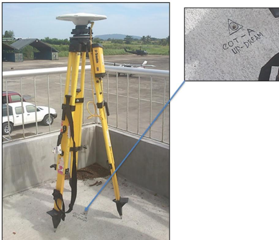
Figure 19. Ground Base Station Observation at COT-A located inside the premises of Cotabato Airport
