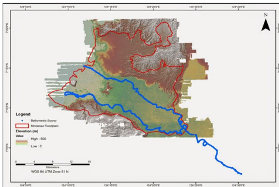
Figure 34. Final DTM of Mindanao with validation survey shown in blue
