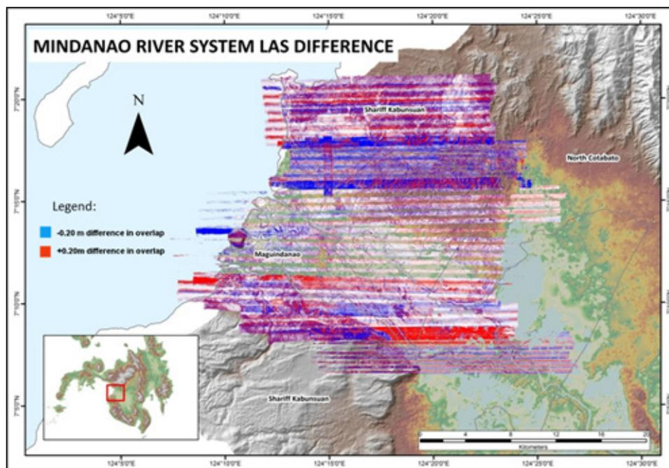
Figure 27. Elevation difference map between flight lines
