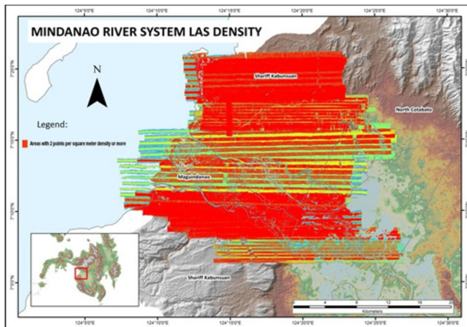
Figure 26. Density map of merged LiDAR data for the Mindanao mission
