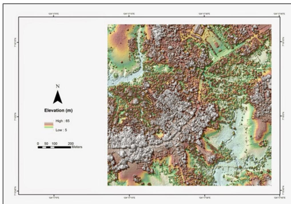
Figure 36. Sample 1x1 square kilometer DSM
