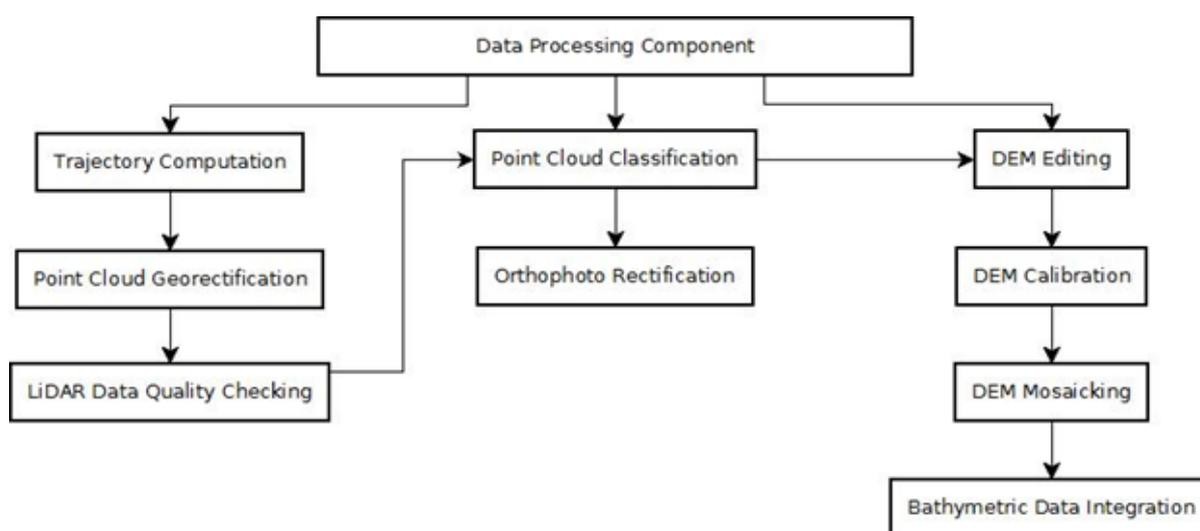
Figure 10. Schematic diagram of the data processing
