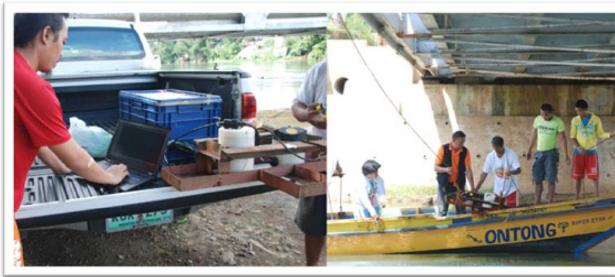
Figure 13. Deployment of ADCP with Depth Gauge below the Baloi Bridge, in Agus River, Lanao del Norte
