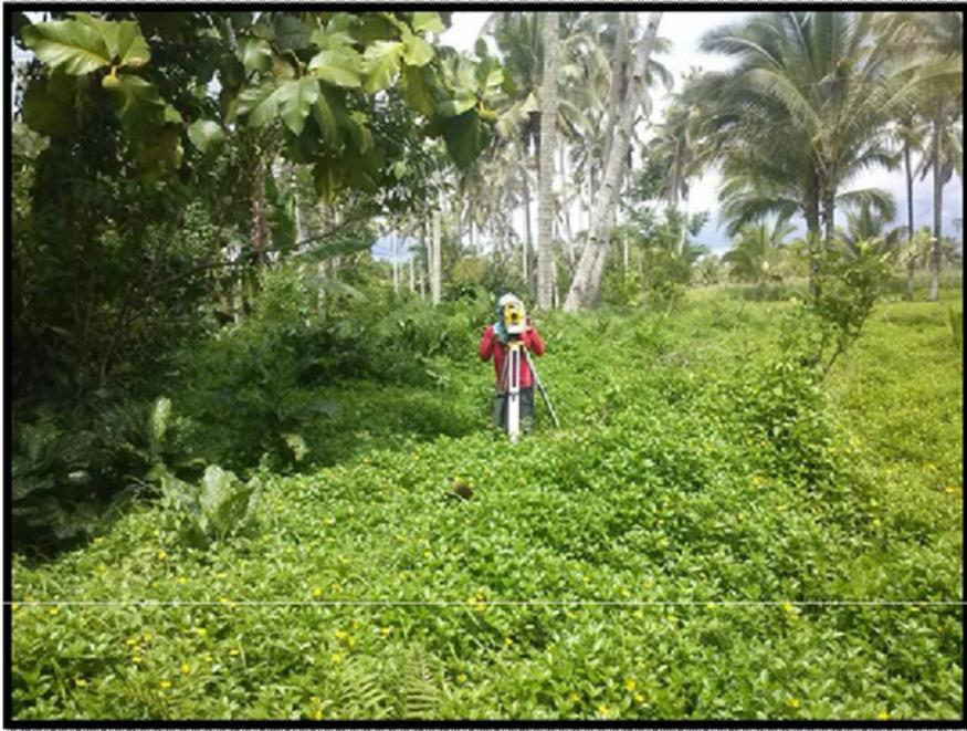
Figure 18. Conducting cross-section survey using Hi-Target Prism less at cross-section 4 at Brgy. Adapun-Ali, Baloi
