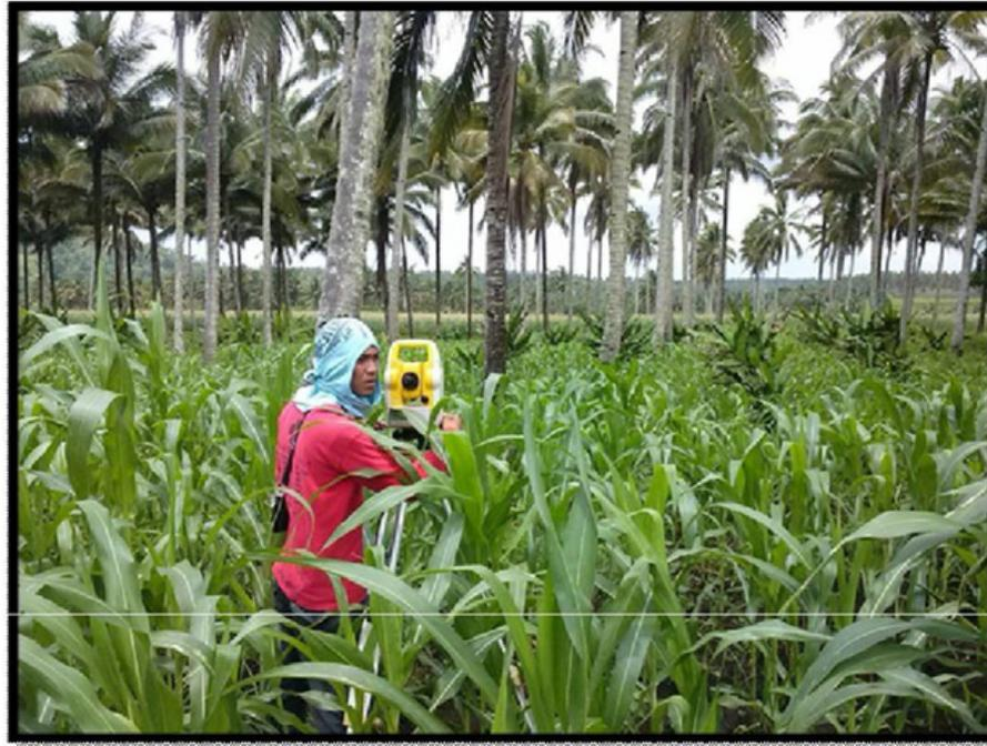
**Figure 15.** Conducting cross-section survey using Hi-Target Prism less at cross-section 4 at Brgy. Batolacongan, Baloi
