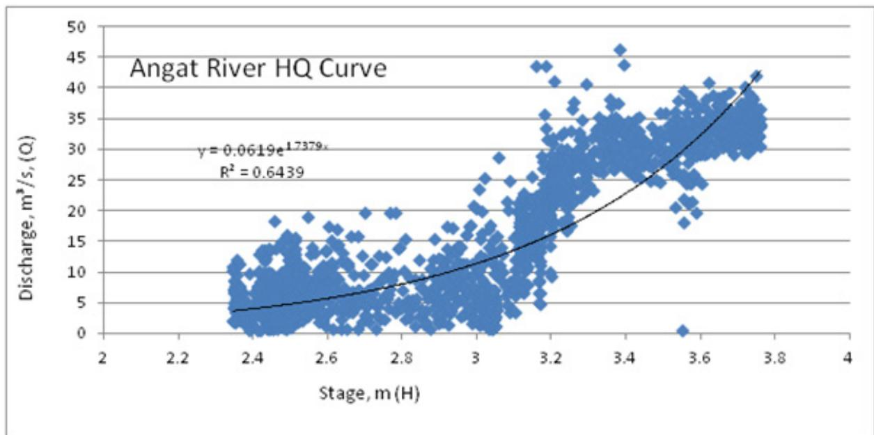
Figure 38. Stage-discharge computation in Brgy. Parulan, Plaridel
