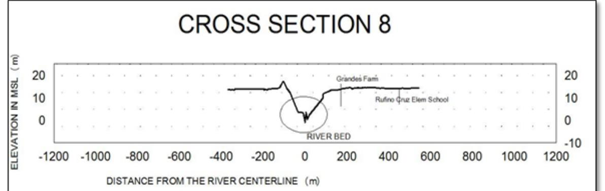
Figure 21. Cross-section 8 at Angat River
