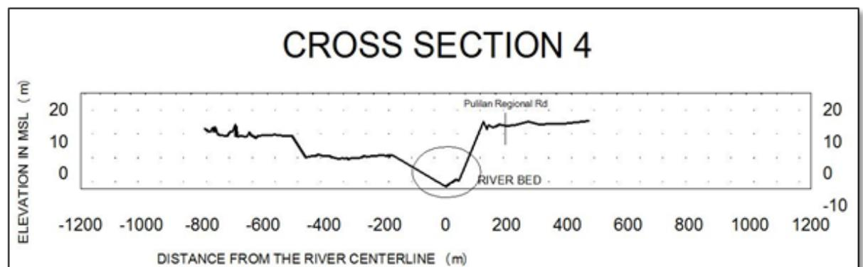
Figure 17. Cross-section 4 at Angat River
