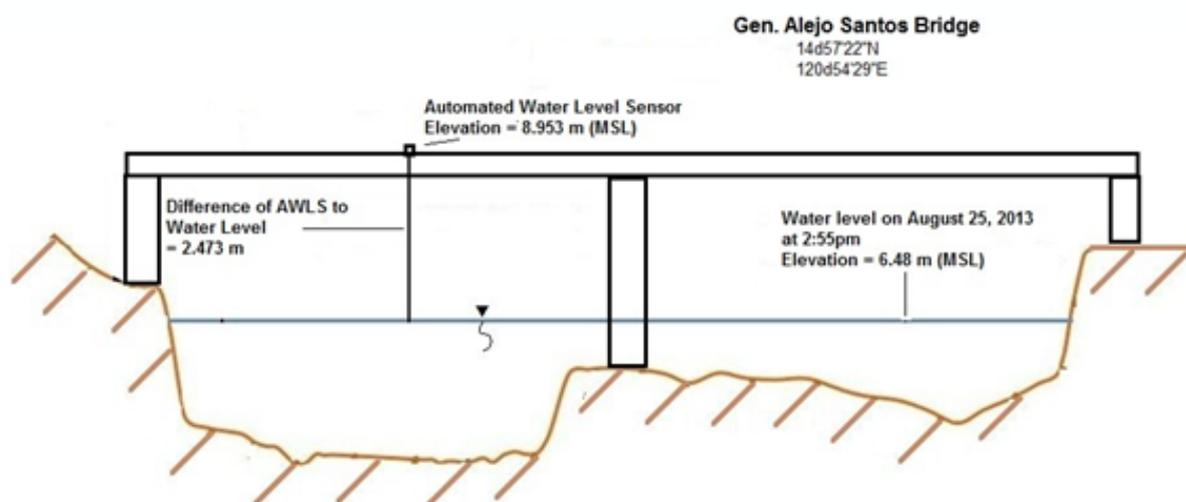
Figure 45. Cross-section diagram of Alejo Santos Bridge
