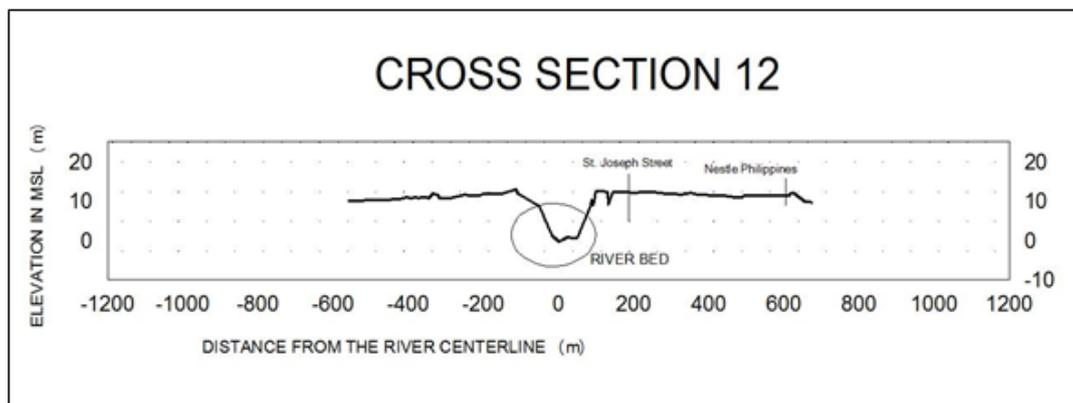
Figure 25. Cross-section 12 at Angat River
