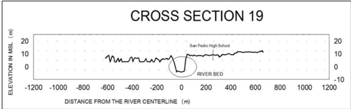
**Figure 30.** Cross-section 19 at Angat River
