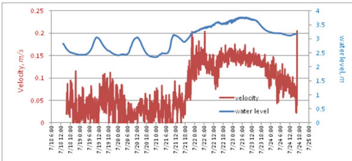
Figure 35. Relationship between velocity and stage in Brgy. Parulan, Plaridel
