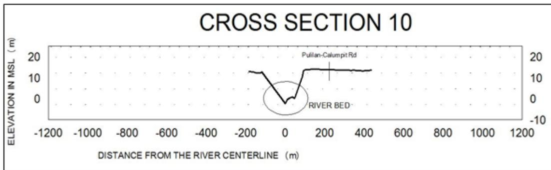
Figure 23. Cross-section 10 at Angat River
