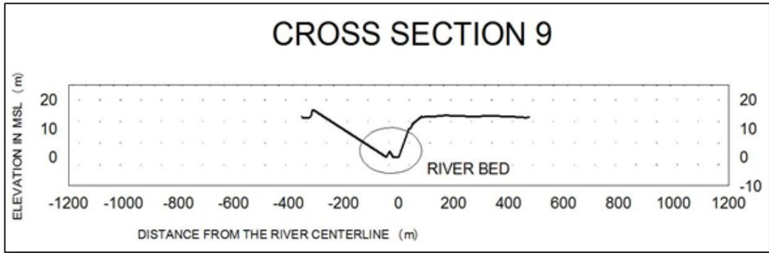
Figure 22. Cross-section 9 at Angat River
