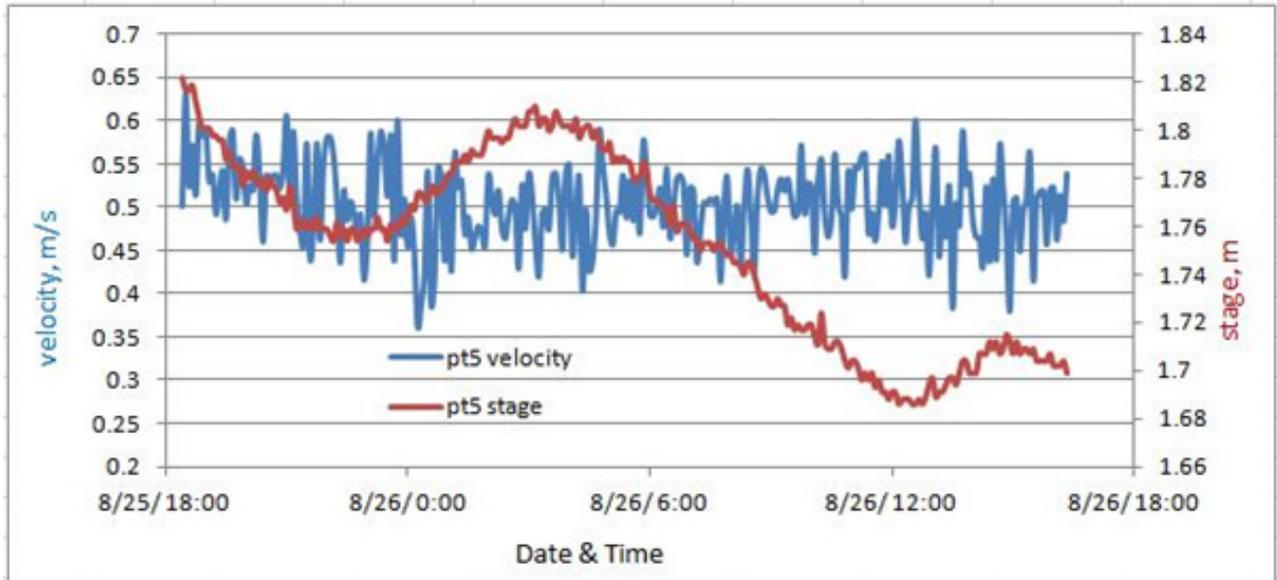
Figure 47. Relationship between velocity and stage in Brgy. Caniogán, Calumpit
