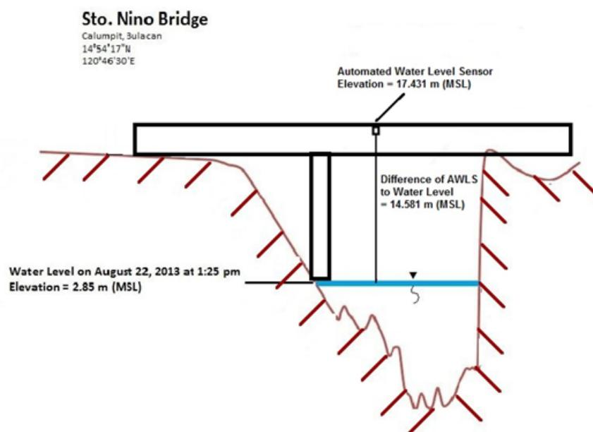
**Figure 44.** Cross-section diagram of Sto. Nino Bridge
