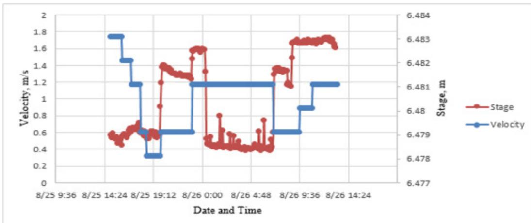
Figure 50. Relationship between stage and velocity in Brgy. Bustos, Bulacan
