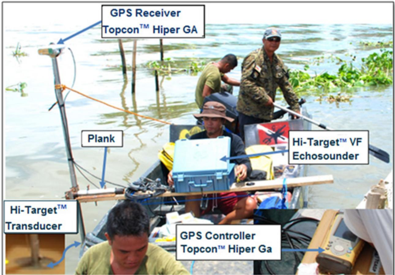
Figure 33. Bathymetric survey setup
