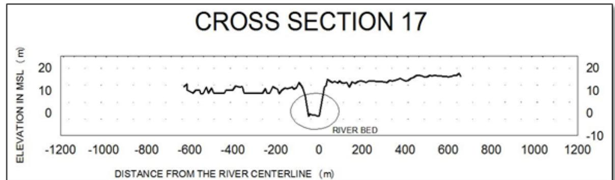
Figure 28. Cross-section 17 at Angat River
