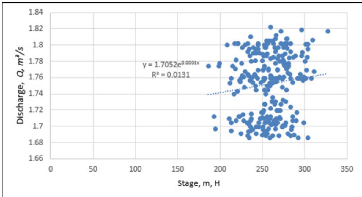
Figure 48. Stage-discharge computation at Sto.Nino Bridge in Brgy. Caniogán, Calumpit, Bulacan
