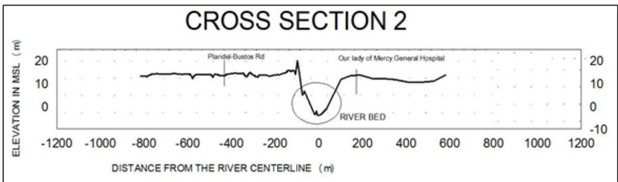
Figure 15. Cross-section 2 at Angat River
