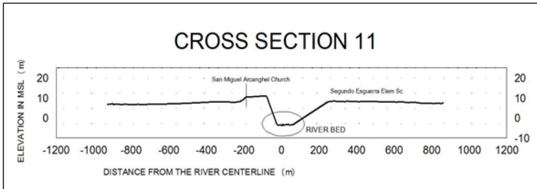
Figure 24. Cross-section 11 at Angat River
