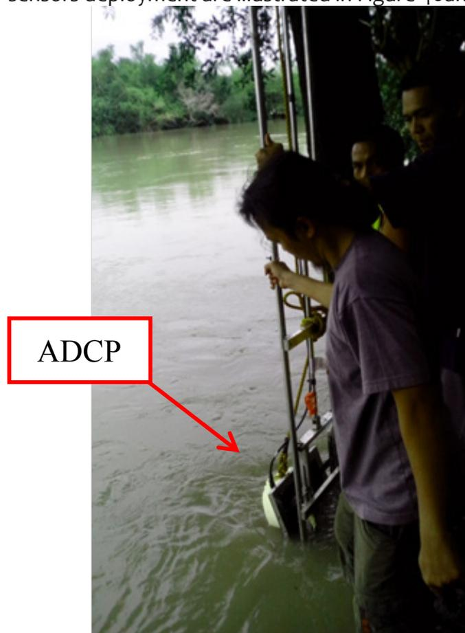
**Figure 40.** Deployment of ADCP and depth gauge in Brgy. Parulan in Plaridel, Bulacan
