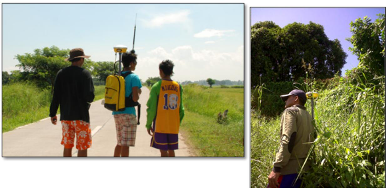
**Figure 12.** Cross-section teams conducting PPK GNSS survey
