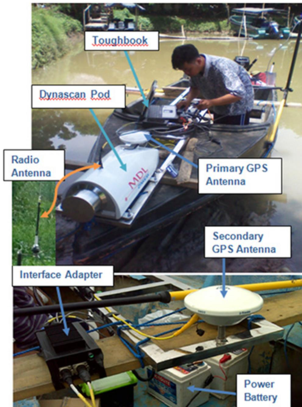
**Figure 31.** The MDL Dynascan™ installed on one end of the boat for the river bank profile surveys of Angat River
