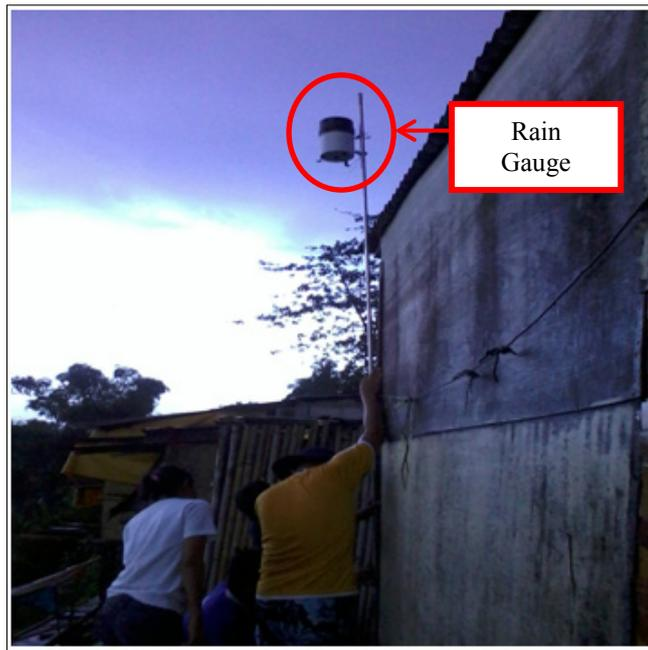
**Figure 41.** Rain gauge deployment in Brgy. Parulan, Plaridel
