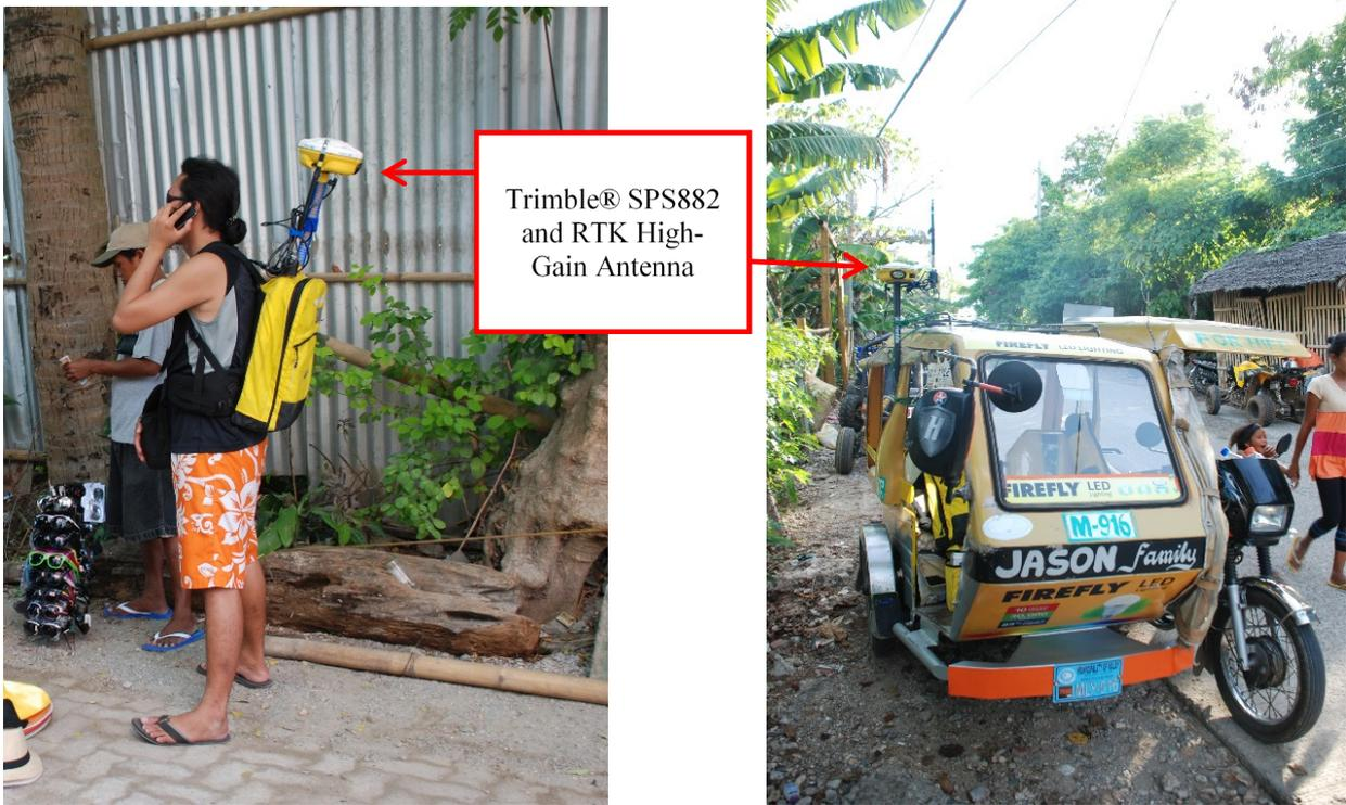
**Figure 18.** Validation Points Acquisition Survey using GNSS RTK technique by traversing the length of roads (a) by foot (b) as installed on a motorized vehicle
