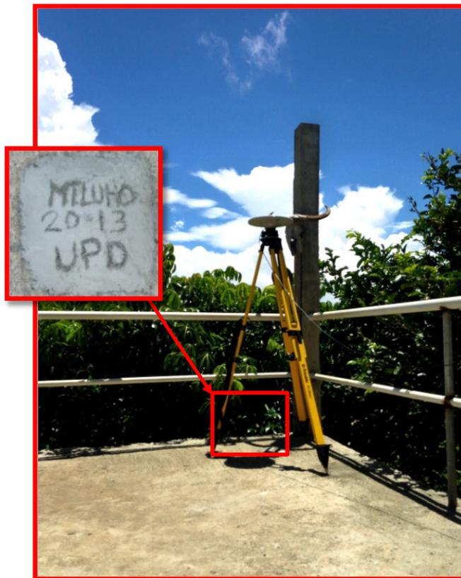
Figure 13. Static GNSS observation at Mt. Luho in Boracay Island, Malay, Aklan
