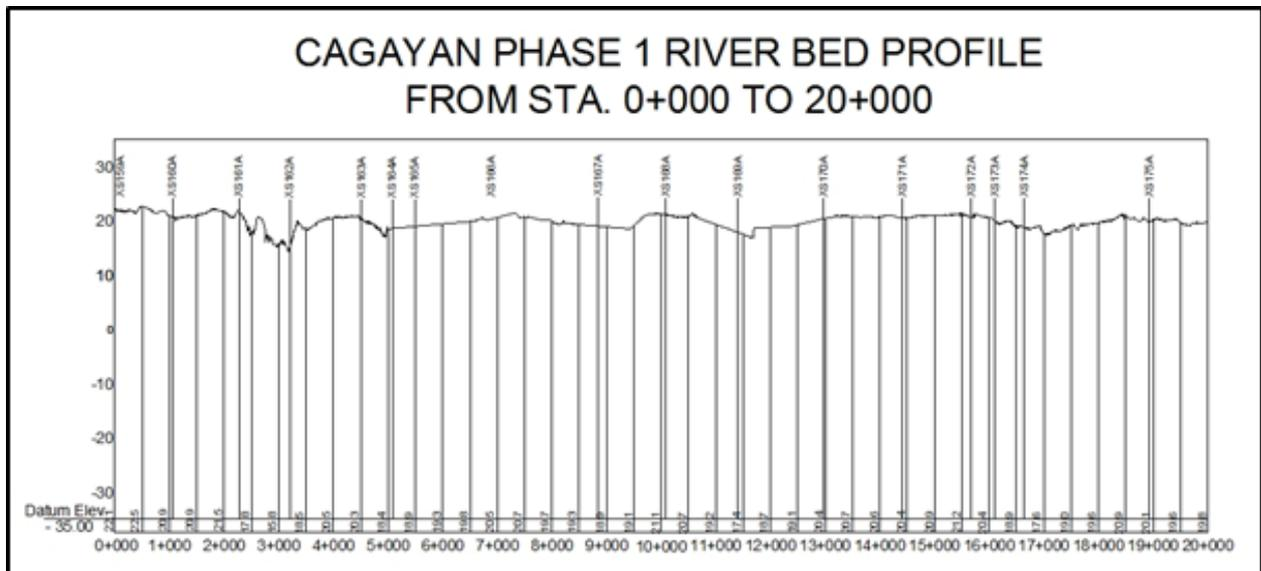
Figure 76. Bathymetry center line from Nagtipunan to Maddela in Quirino
