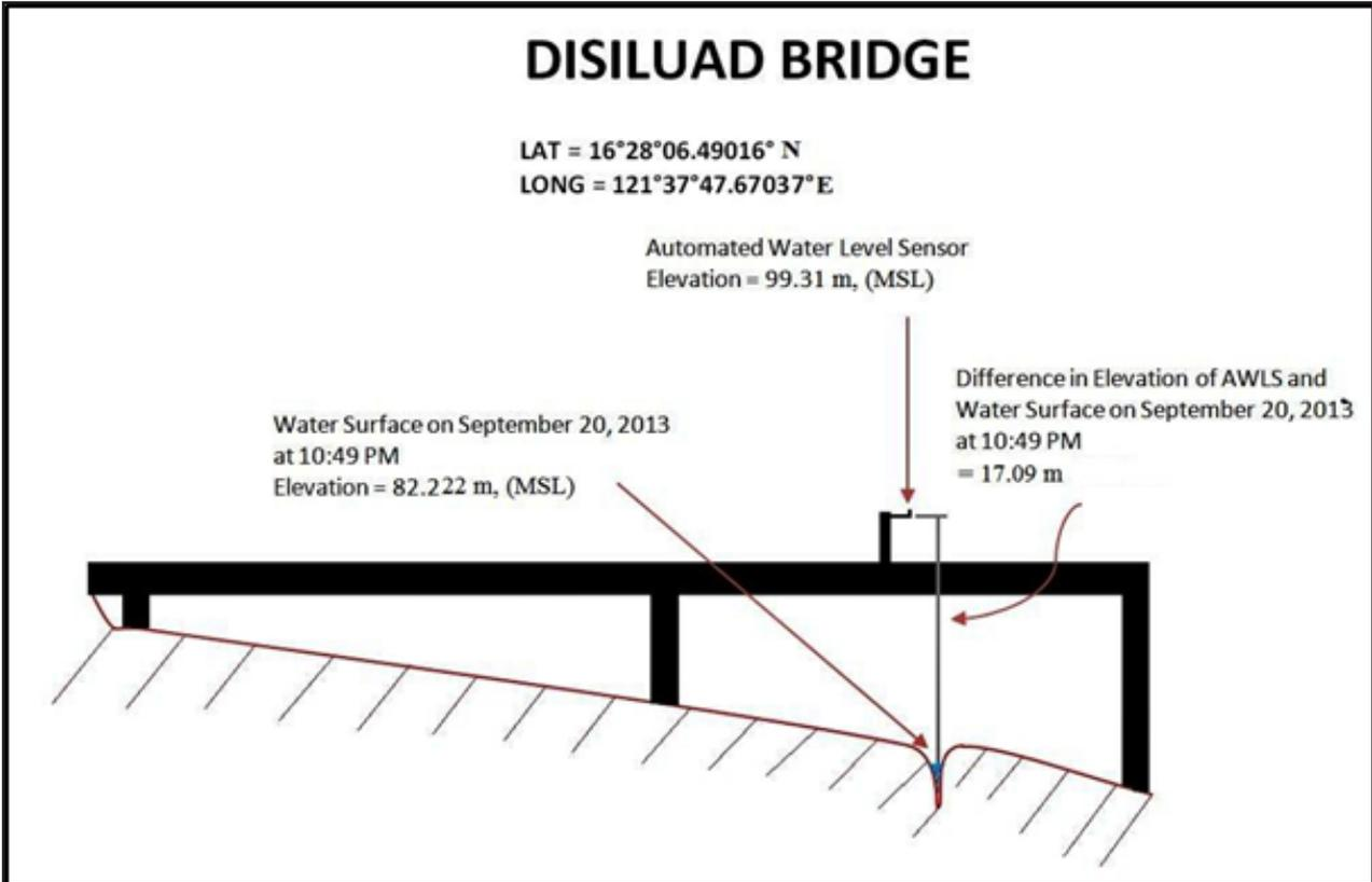
Figure 40. Disilud Bridge Cross-Section Diagram
