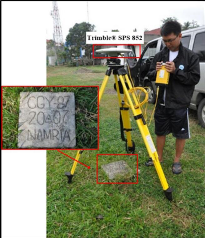
Figure 18. Trimble® SPS 985 setup at CGY-87 in Gattaran, Cagayan
