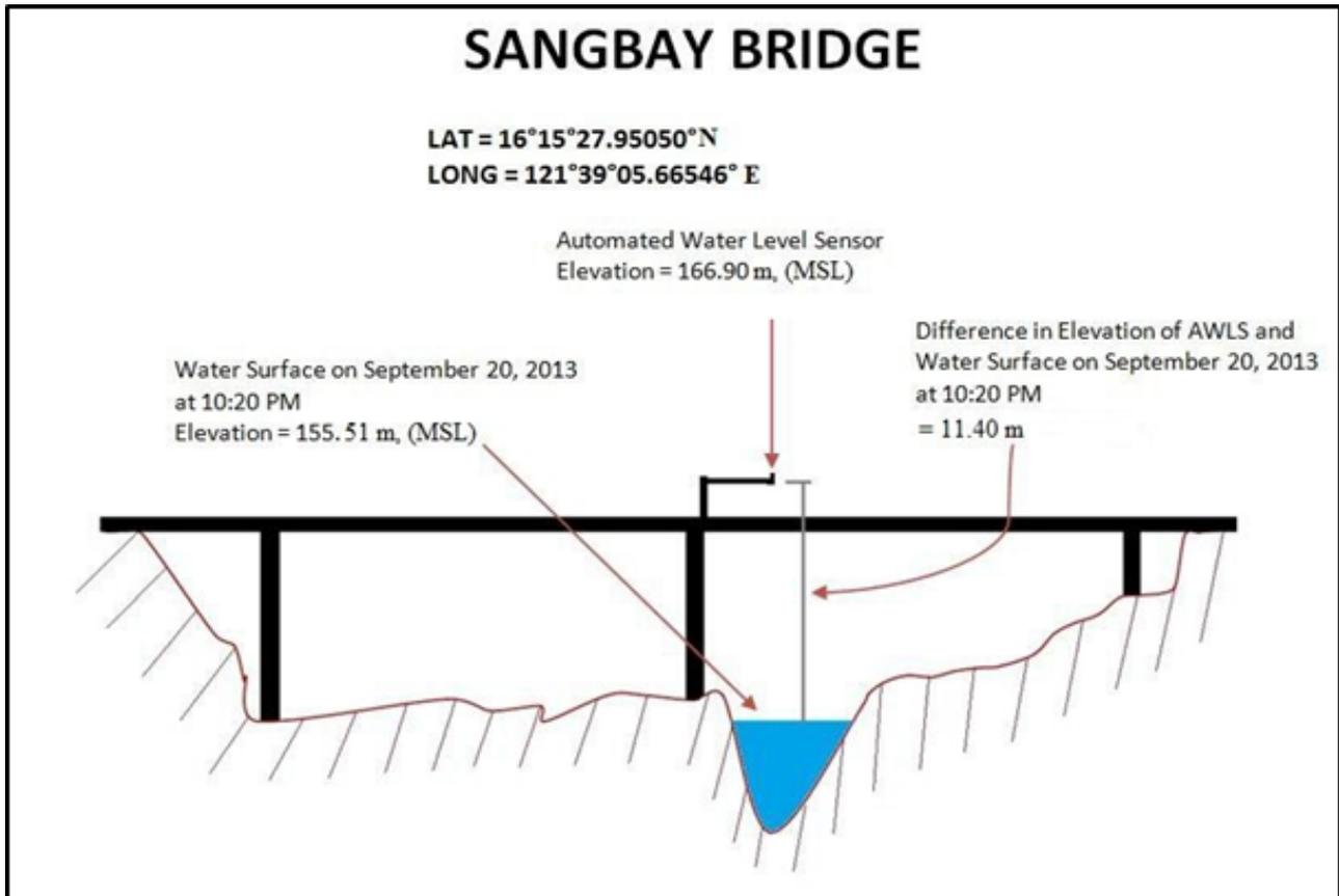
Figure 49. Sangbay Bridge Cross-Section Diagram
