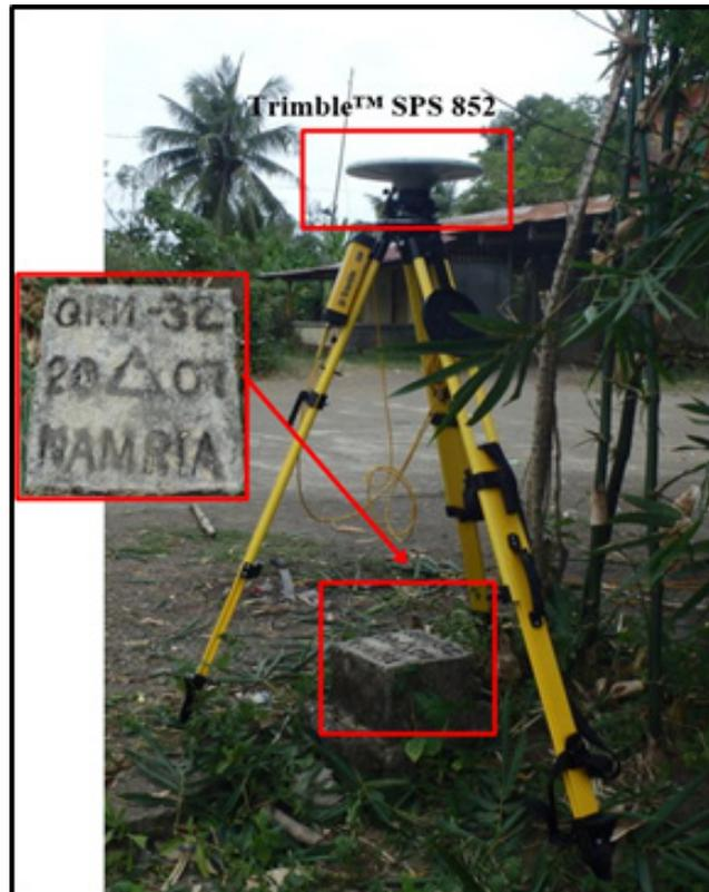
**Figure 27.** GNSS receiver set up, Trimble® SPS 852 at QRN-32, Brgy. Liwayway Diffun, Quirino
