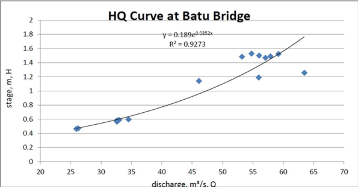
**Figure 99.** Relationship between stage and discharge in Batu Bridge within the observation period
