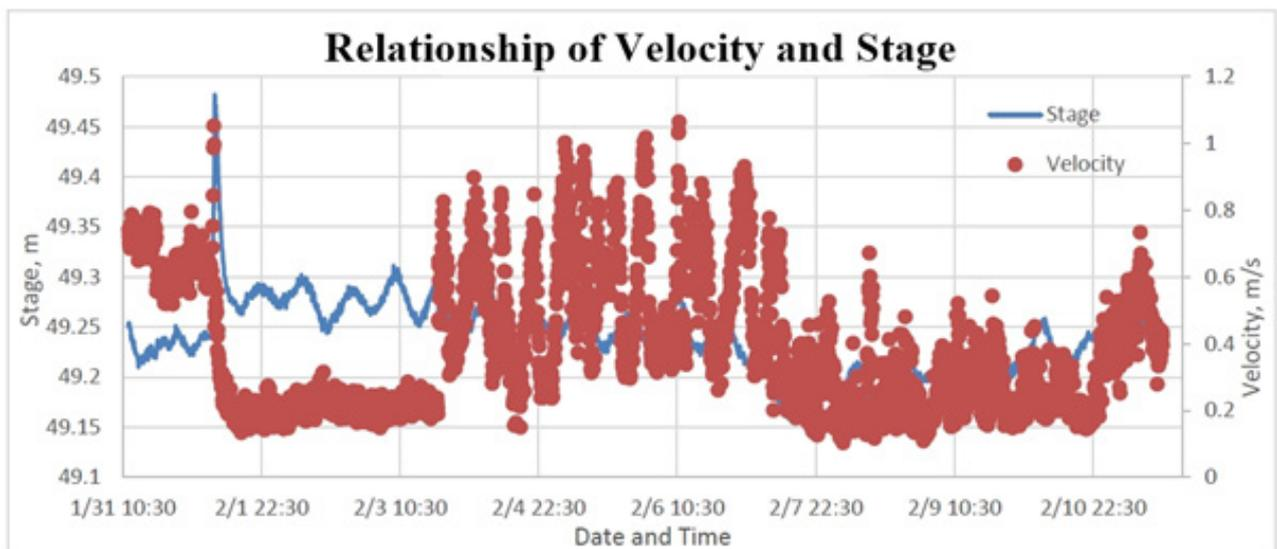
**Figure 131.** Relationship between velocity and stage in Mallig Bridge within the observation period
