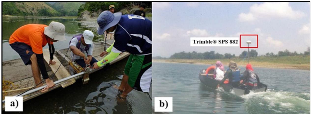
Figure 75. Bathymetric survey (Phase 3) setup on a boat (a) Quirino and (b) Isabela
