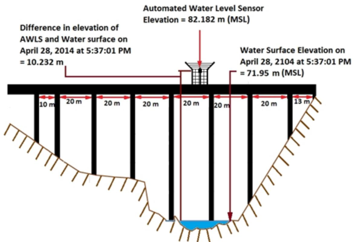
Figure 61. Santiago Bridge Cross-Section Diagram
