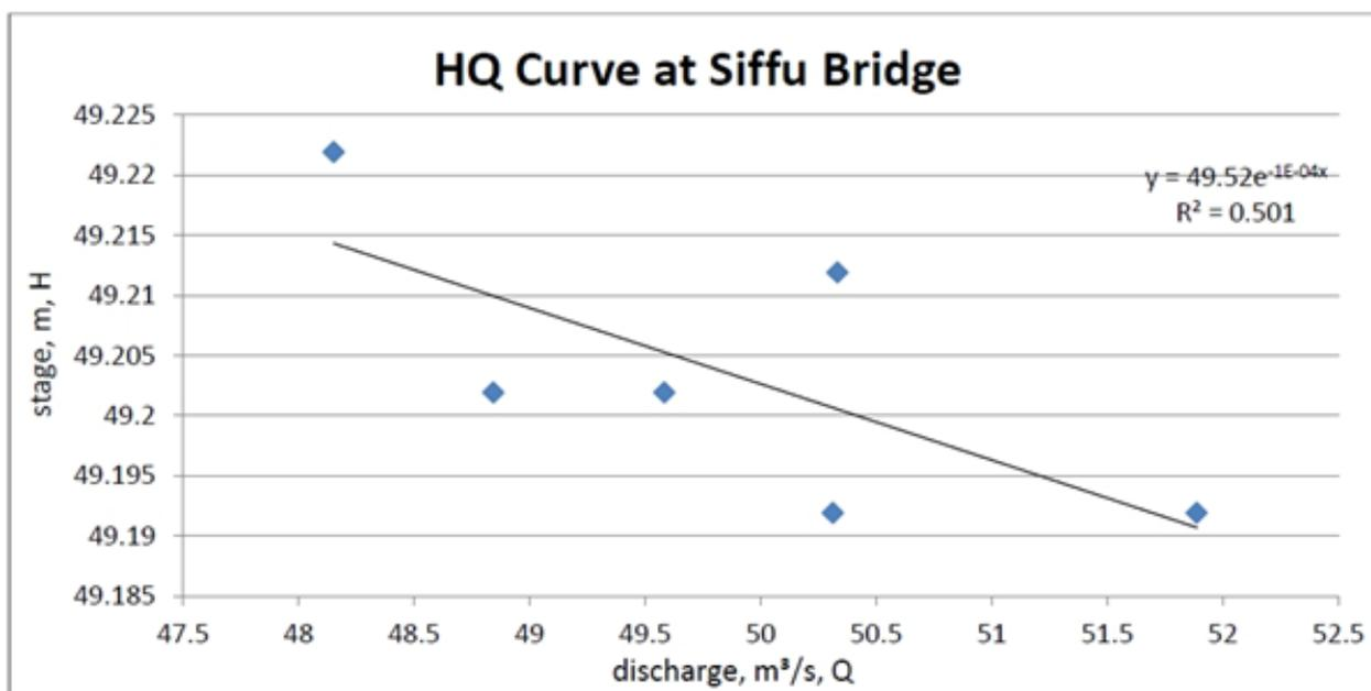
**Figure 119.** Relationship between stage and discharge in Siffu Bridge within the observation period
