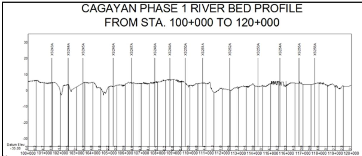
Figure 69. Bathymetry center line from the Municipalities of Iguig and Solana to Amulung in Cagayan
