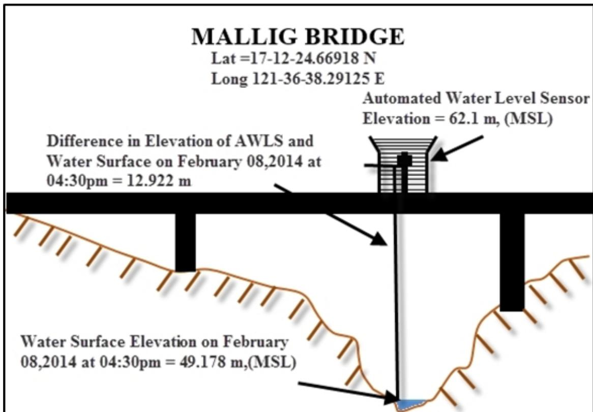
Figure 57. Mallig Bridge Cross-Section Diagram
