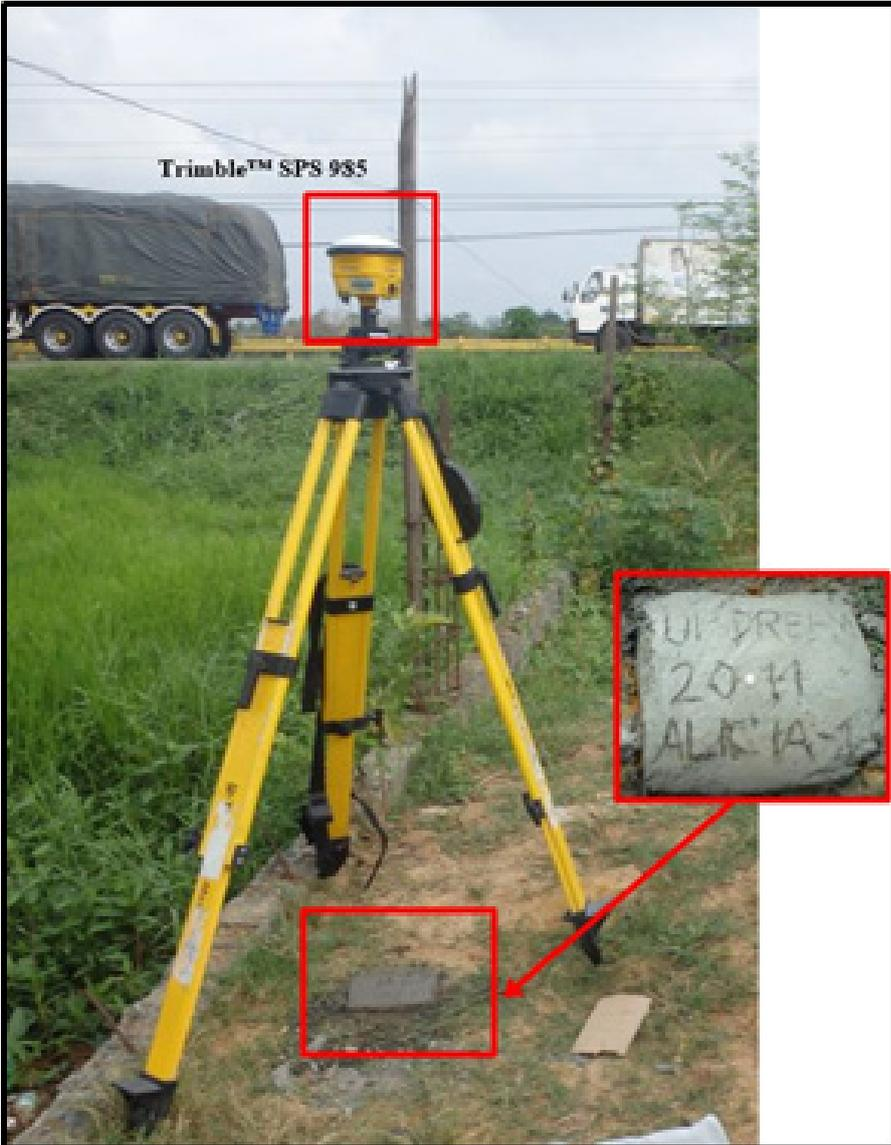
Figure 29. GNSS receiver set up, Trimble® SPS 985 at ALICIA-1, Alicia, Isabela
