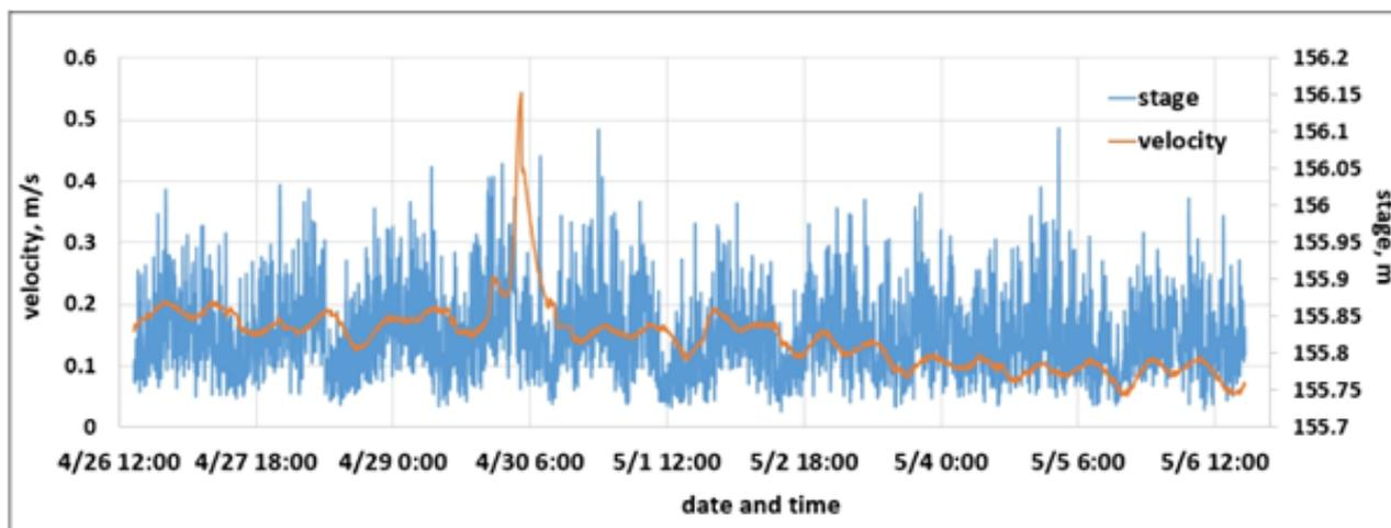
Figure 143. Relationship between velocity and stage in Sangbay Bridge within the observation period
