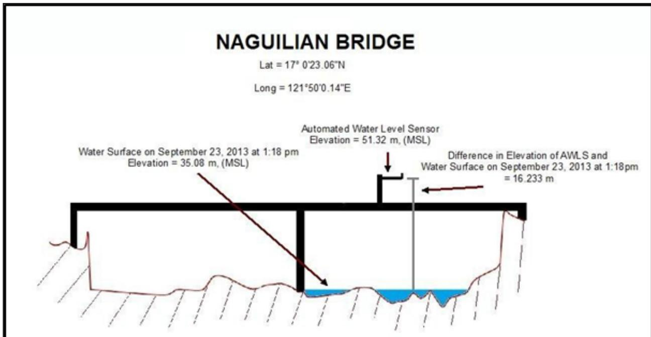
Figure 46. Naguilian Bridge Cross-Section Diagram
