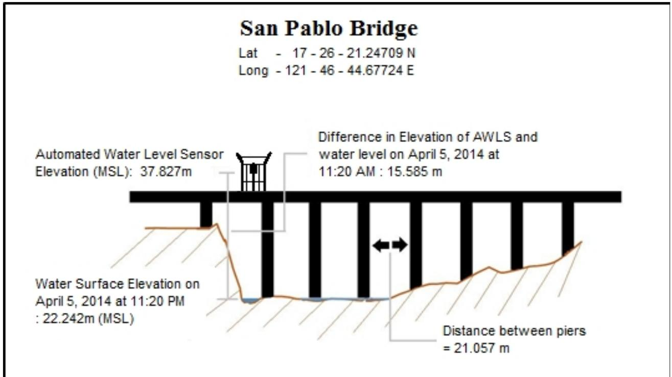
Figure 55. San Pablo Bridge Cross-Section Diagram
