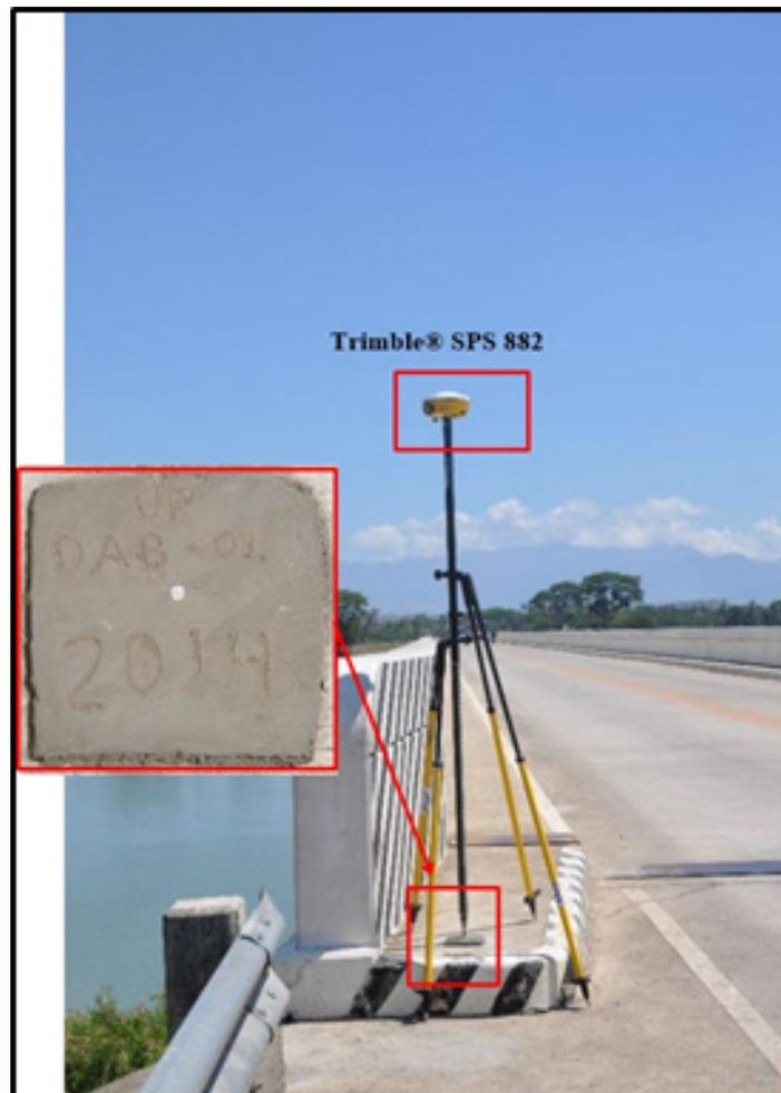
**Figure 19.** GNSS receiver set up, Trimble® SPS 882 at UP DAB-1 2014 at Delfin Albano Bridge, Delfin Albino, Isabela
