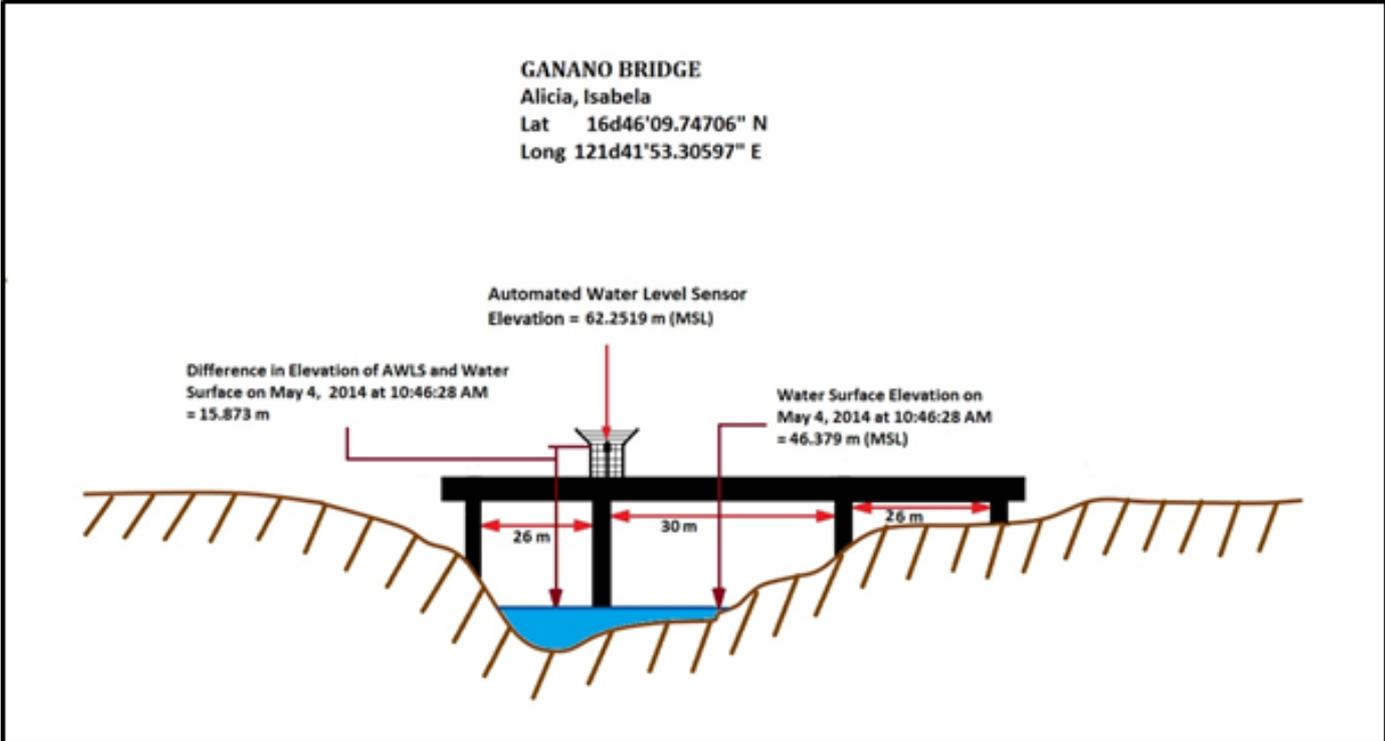
Figure 59. Ganano Bridge Cross-Section Diagram
