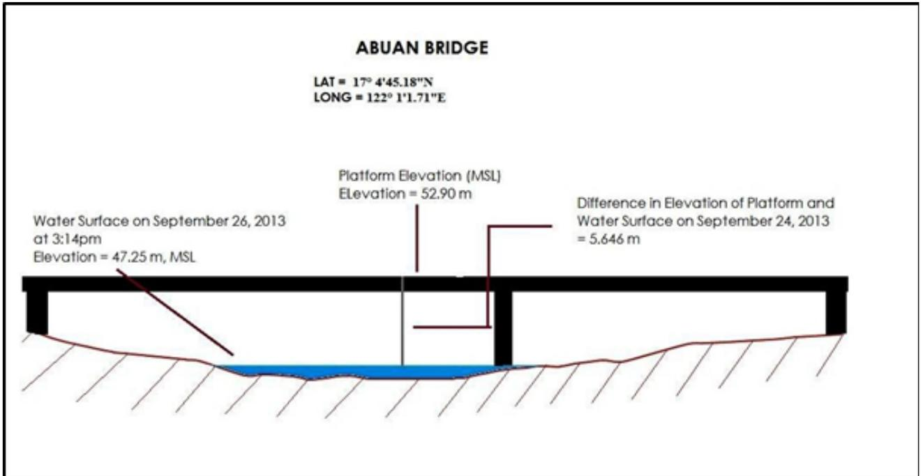
Figure 37. Abuan Bridge Cross-Section Diagram
