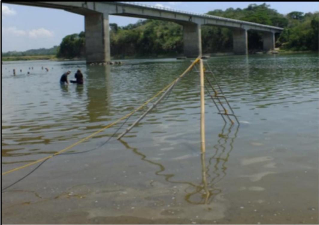
**Figure 90.** Deployed ADCP at Malalam Bridge, Isabela
