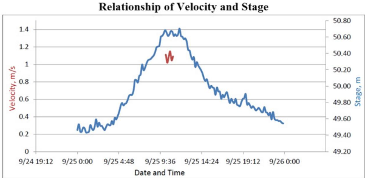
Figure 104. Relationship between velocity and stage in Magat (Aurora) Bridge within the observation period
