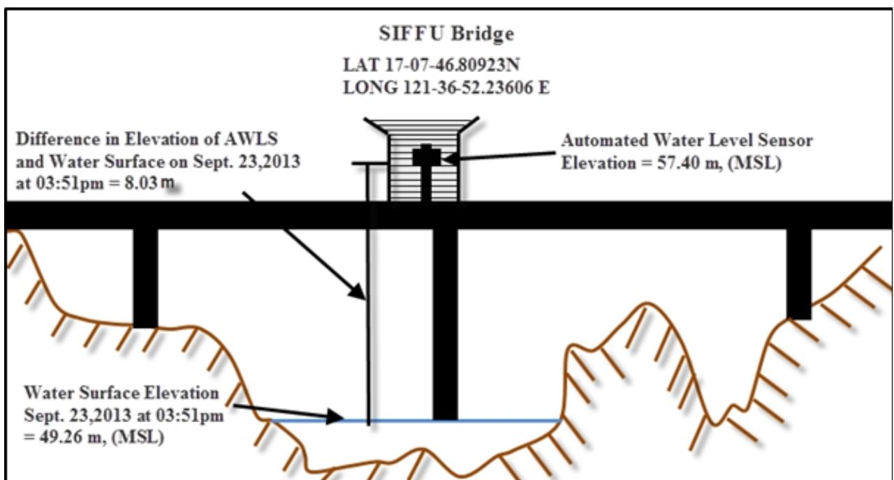
Figure 50. Siffu Bridge Cross-Section Diagram
