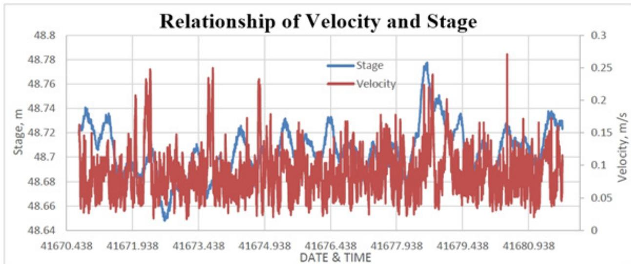
**Figure 129.** Relationship between velocity and stage in Magat (Aurora) Bridge within the observation period
