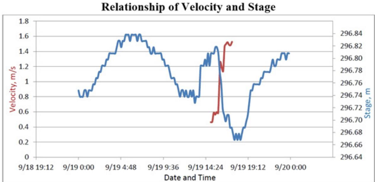
Figure 96. Relationship between velocity and stage in Batu Bridge within the observation period
