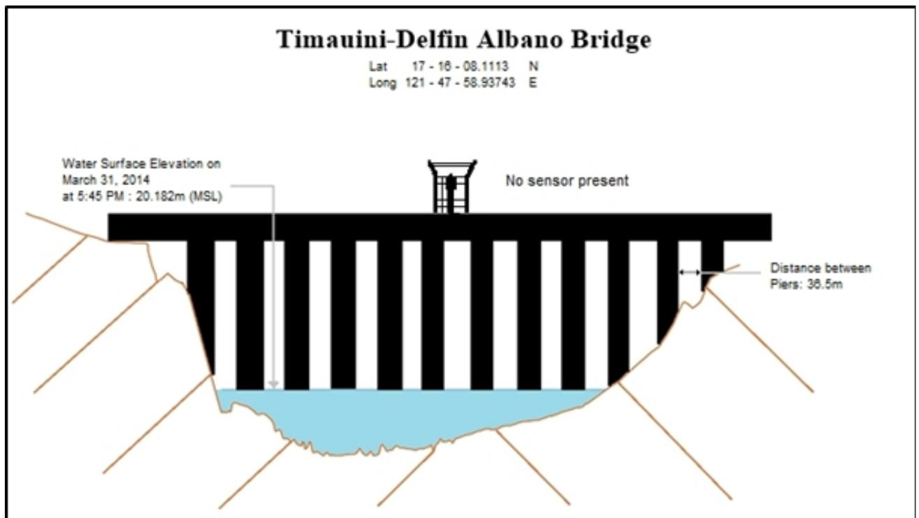
Figure 56. Timauni-Delfin Albano Bridge Cross-Section Diagram
