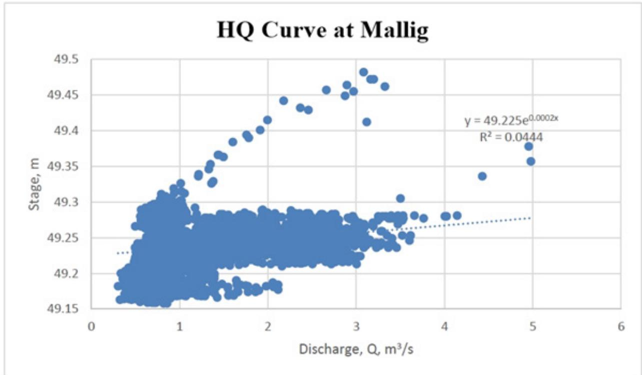
Figure 132. Relationship between stage and discharge in Mallig Bridge within the observation period
