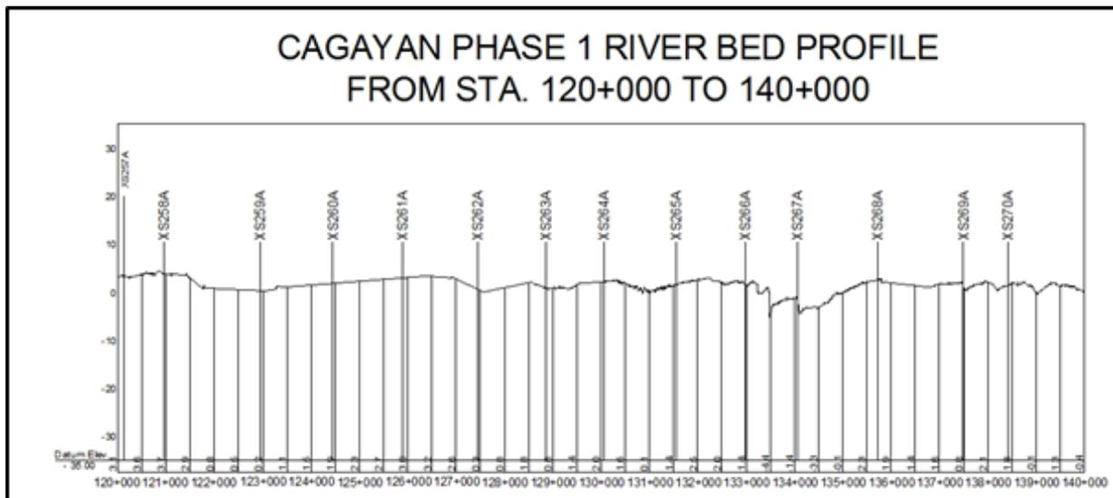
Figure 70. Bathymetry center line from the Municipality of Amulung to Aparri in Cagayan
