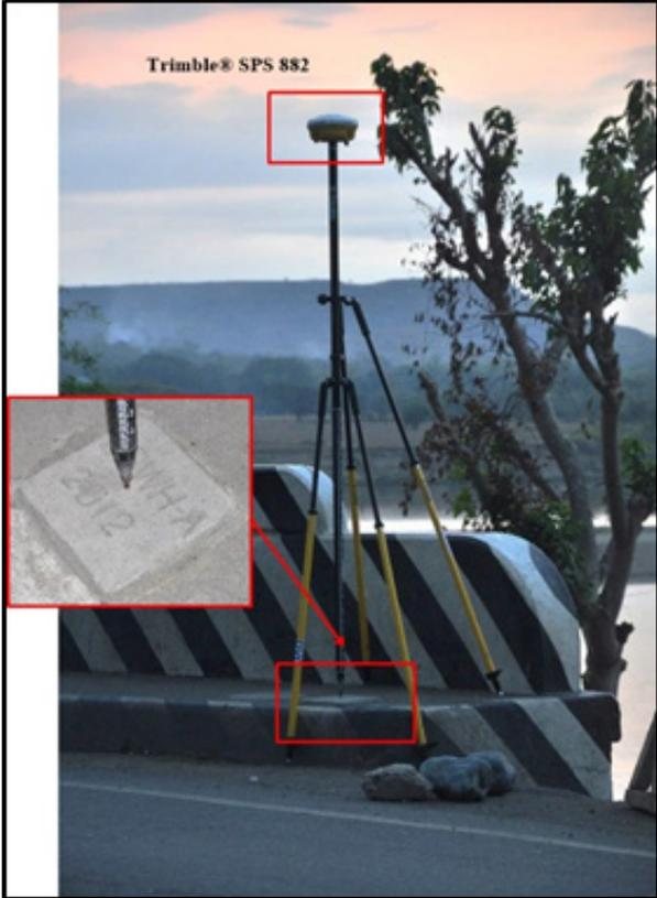
Figure 20. Trimble® SPS 882 setup at DPWH-A 2012, at Buntun Bridge, Tuguegarao City, Cagayan
