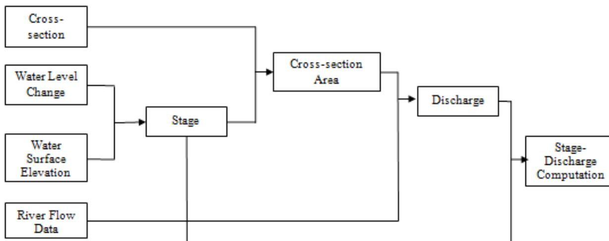
**Figure 7.** Flow Chart for Stage-Discharge Correlation Computation
