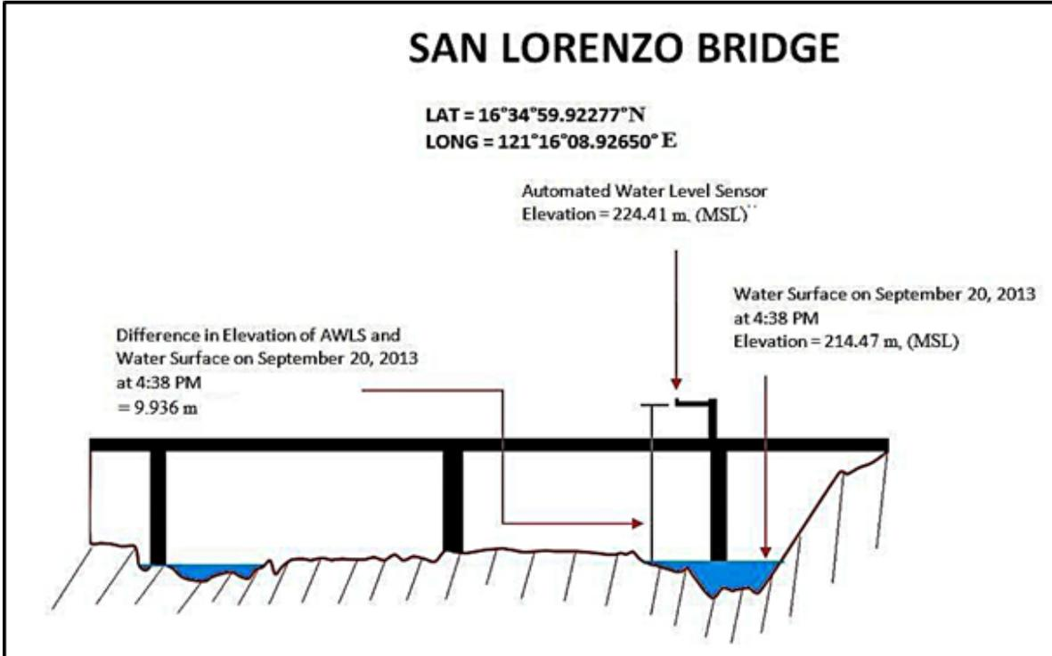
Figure 48. San Lorenzo Bridge Cross-Section Diagram
