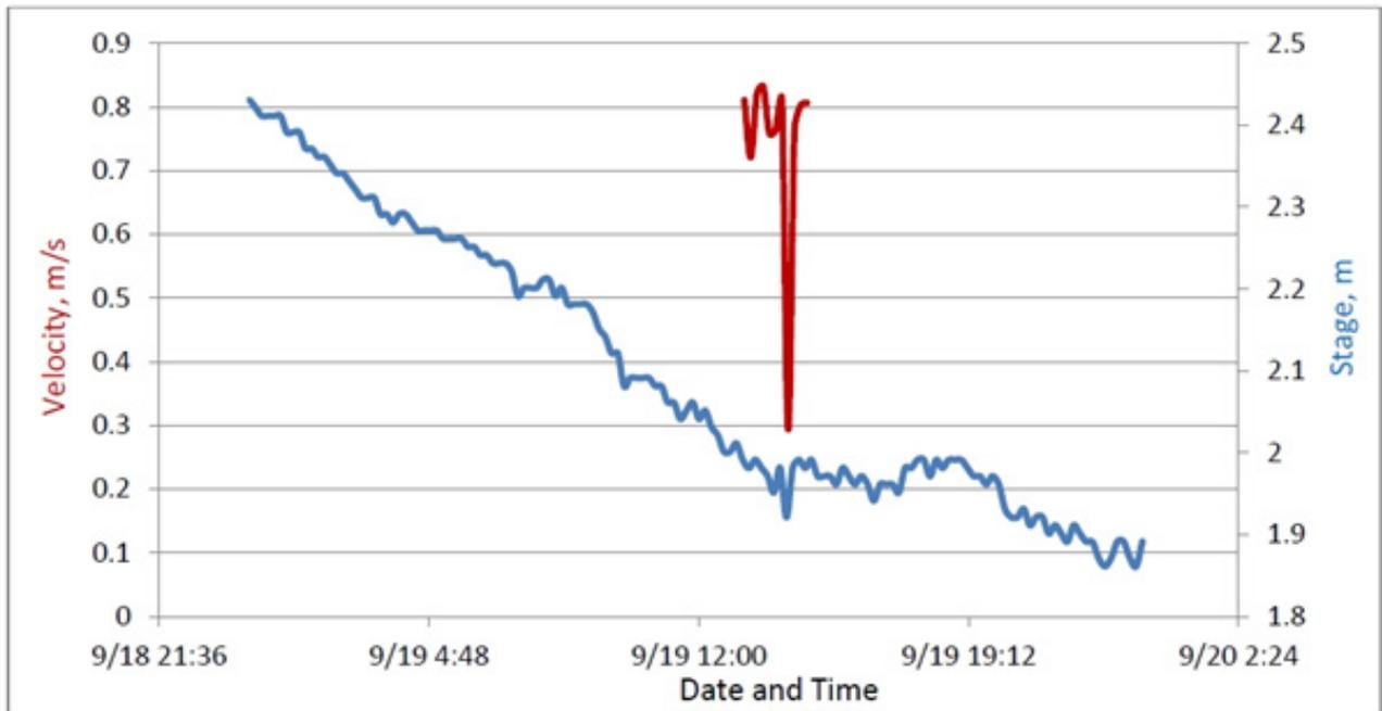
**Figure 100.** Relationship between velocity and stage in Lucban Bridge within the observation period
