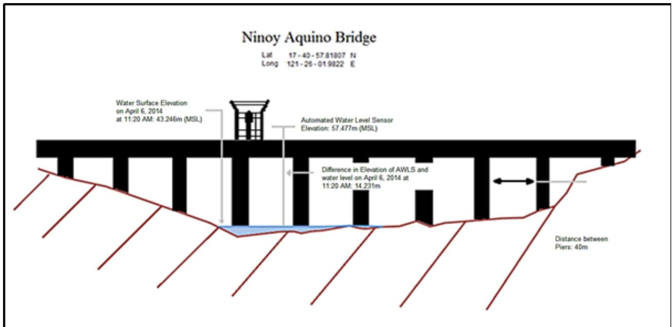
Figure 53. Ninoy Aquino Bridge Cross-Section Diagram
