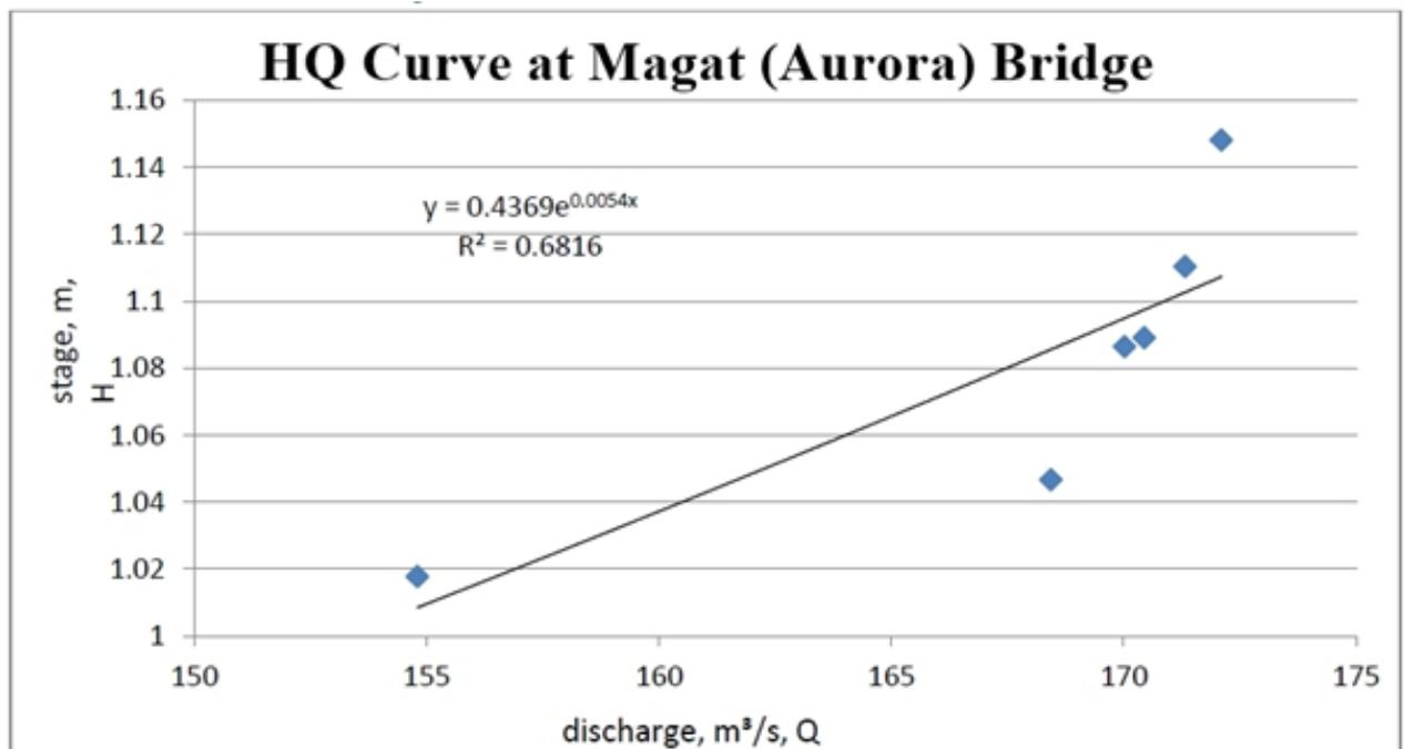
Figure 107. Relationship between stage and discharge in Magat (Aurora) Bridge within the observation period
