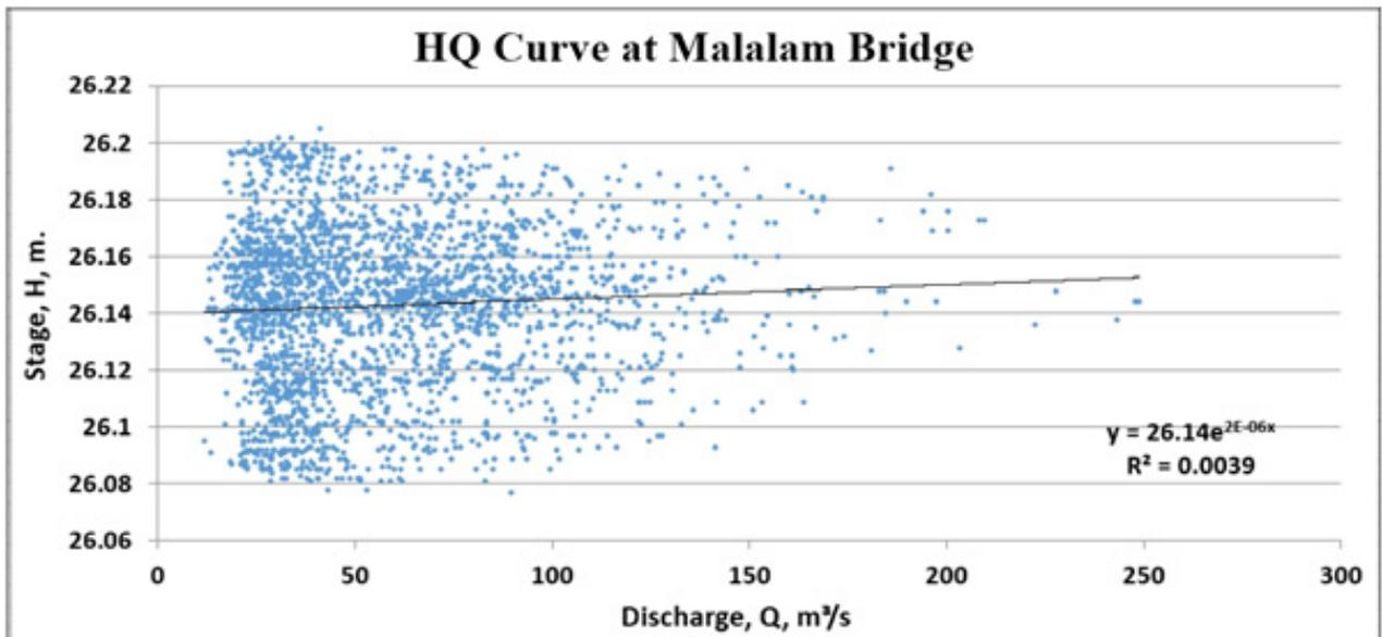
Figure 138. Relationship between stage and discharge in Malalam Bridge within the observation period
