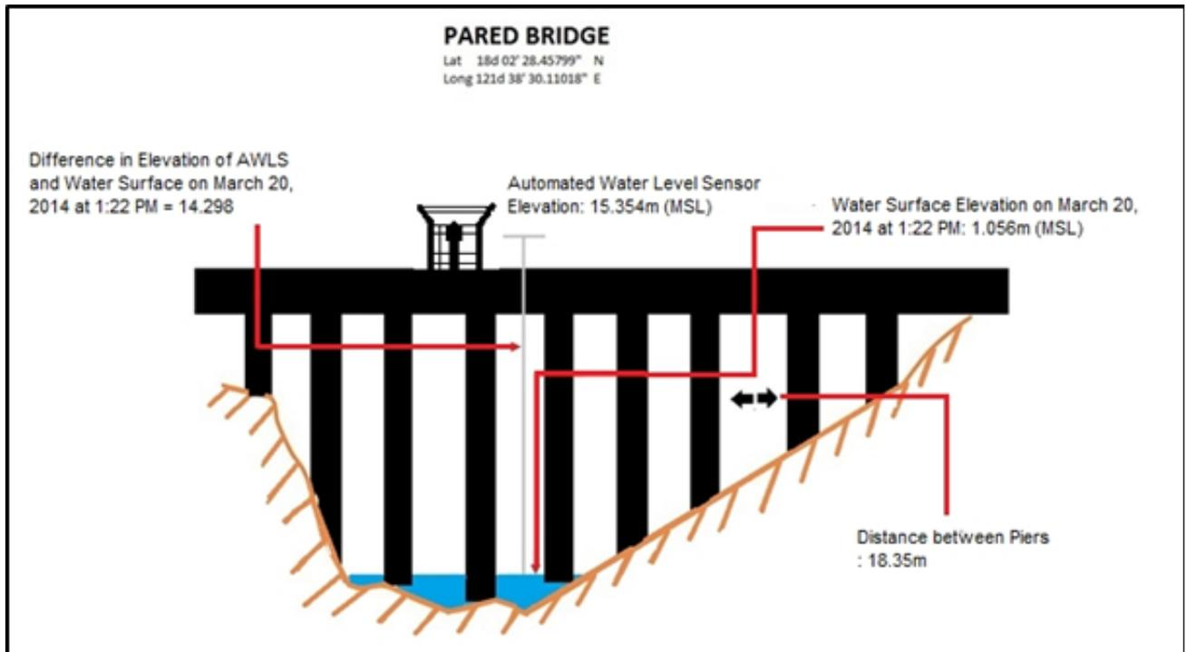
Figure 54. Pared Bridge Cross-Section Diagram
