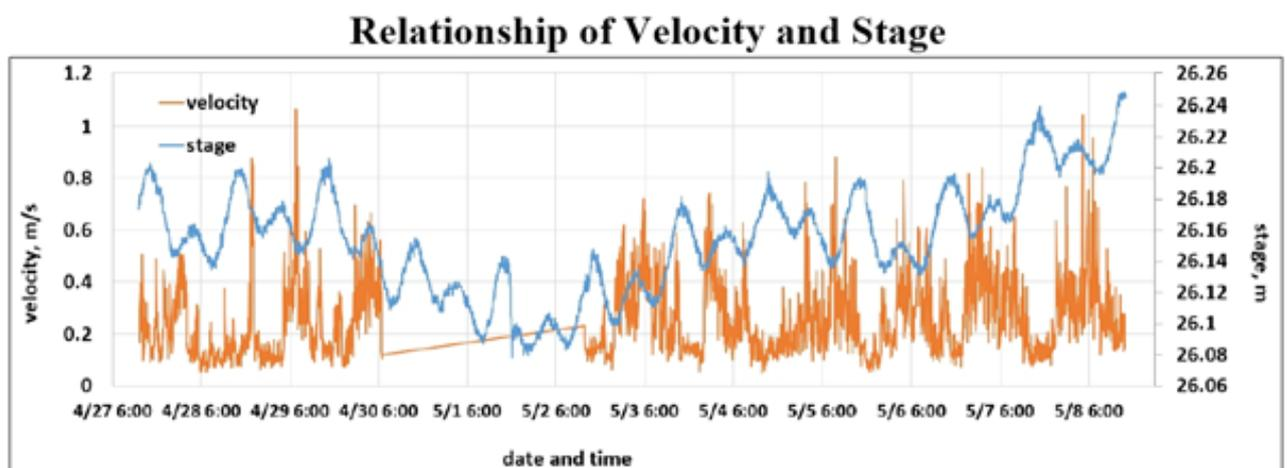
**Figure 135.** Relationship between velocity and stage in Malalam Bridge within the observation period
