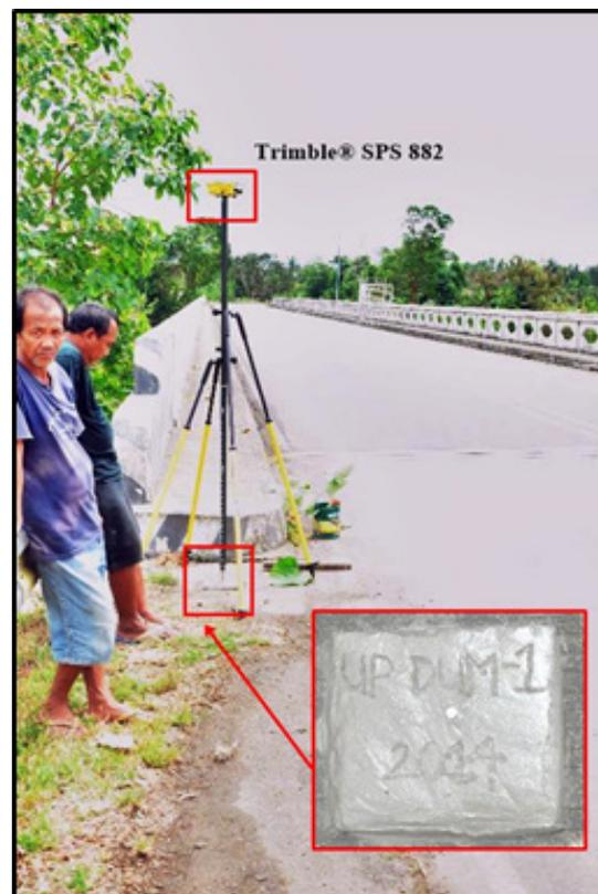
**Figure 23.** GNSS base set up, Trimble® SPS 882, at UP DUM-1, at Dummum Bridge in Gattaran, Cagayan
