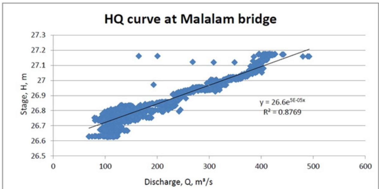
Figure 111. Relationship between stage and discharge in Malalam Bridge within the observation period
