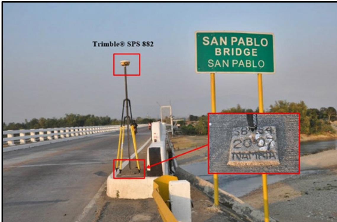
Figure 15. GNSS receiver set up, Trimble® SPS 882 at SB-254 at San Pablo Bridge in San Pablo, Isabela
