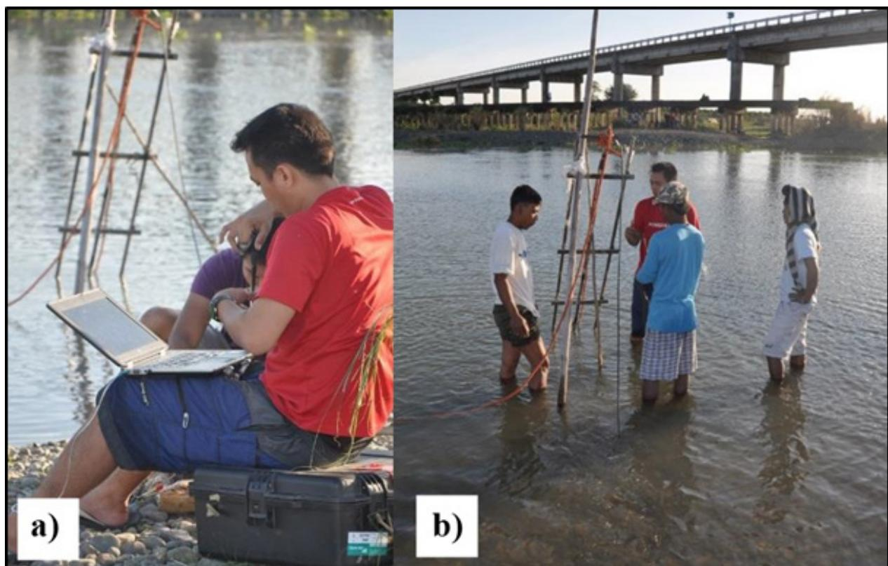
**Figure 89.** At Magat River (Aurora Bridge) (a) Setting up both Depth gauge and ADCP (b) Deployment of ADCP
