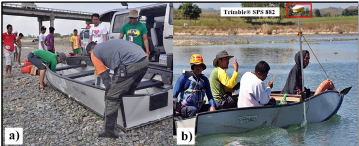
**Figure 71.** Bathymetric survey at Magat River using portable boat borrowed from PDRRMC. (a) Assembling the boat in preparation for the survey (b) Gathering bathymetric data using OHMEX™ single beam echosounder with mounted Trimble® SPS 882
