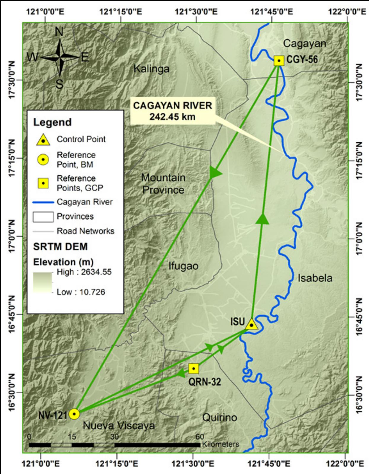
Figure 13. GNSS Network of the initial survey in Cagayan River Basin
