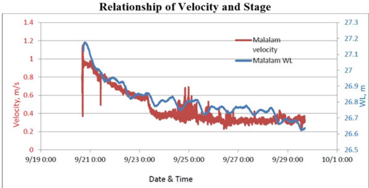
Figure 108. Relationship between velocity and stage in Malalam Bridge within the observation period
