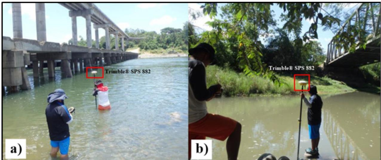
**Figure 36.** Cross section Survey during Cagayan River Survey Phase 3 on April 28 - May 8, 2014 at (a) Dalibubon Bridge and (b) President Bridge
