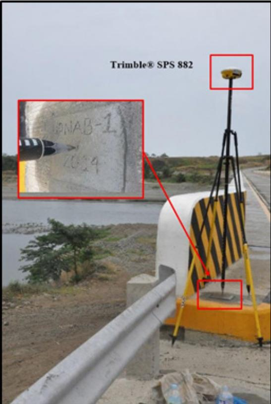
Figure 21. GNSS base set up, Trimble® SPS 882, at UP NAB-1 in Ninoy Aquino Bridge, Brgy. San Luis, Tuao, Cagayan
