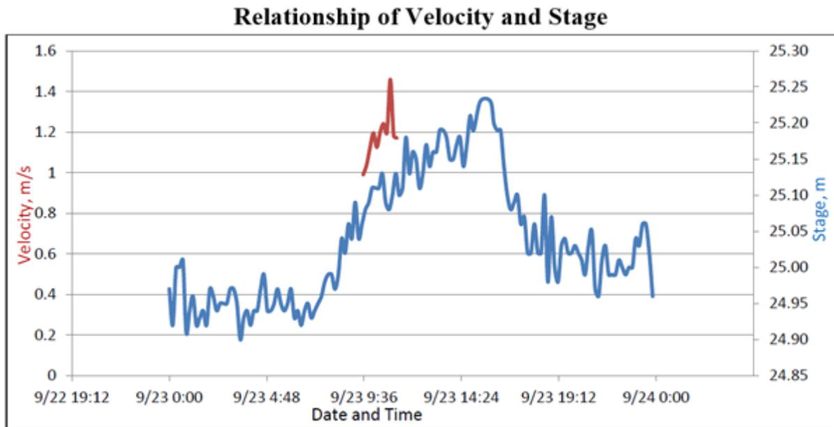
Figure 92. Relationship between velocity and stage in Arkon Bridge within the observation period
