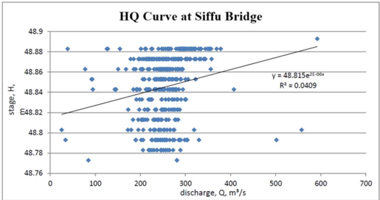
**Figure 134.** Relationship between stage and discharge in Siffu Bridge within the observation period
