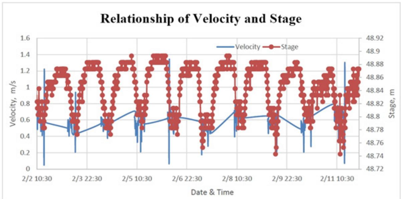
Figure 133. Relationship between velocity and stage in Siffu Bridge within the observation period
