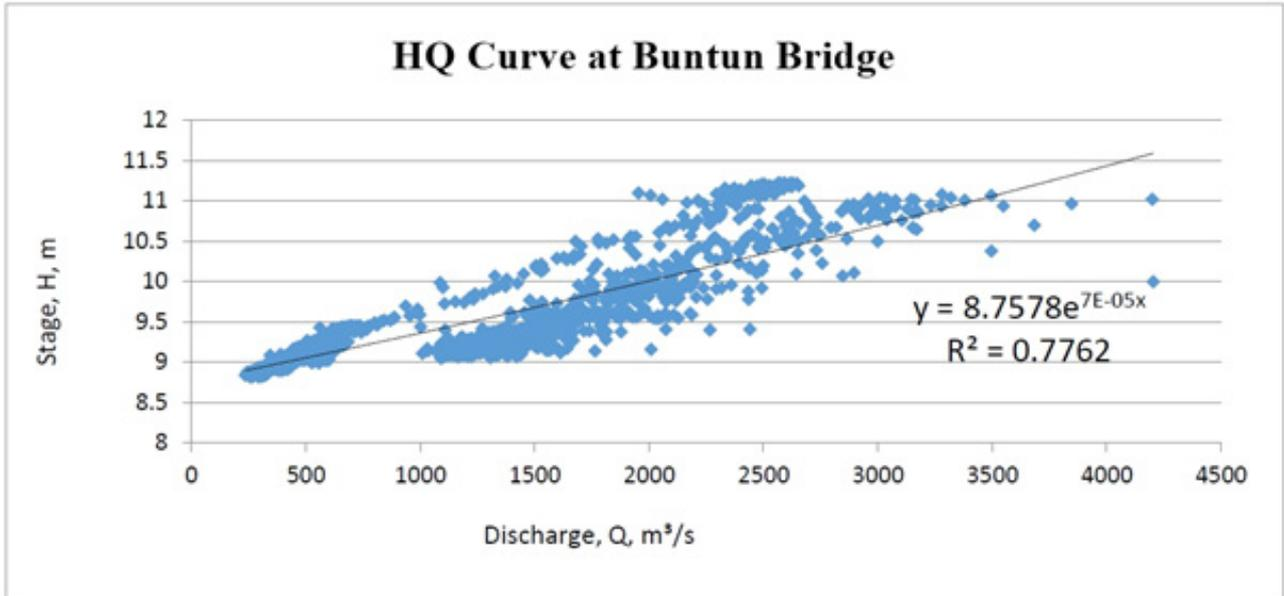
Figure 123. Relationship between stage and discharge in Buntun Bridge within the observation period
