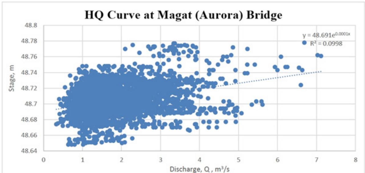
**Figure 130.** Scatter plot showing the relationship between stage and discharge in Magat (Aurora) Bridge within the observation period
