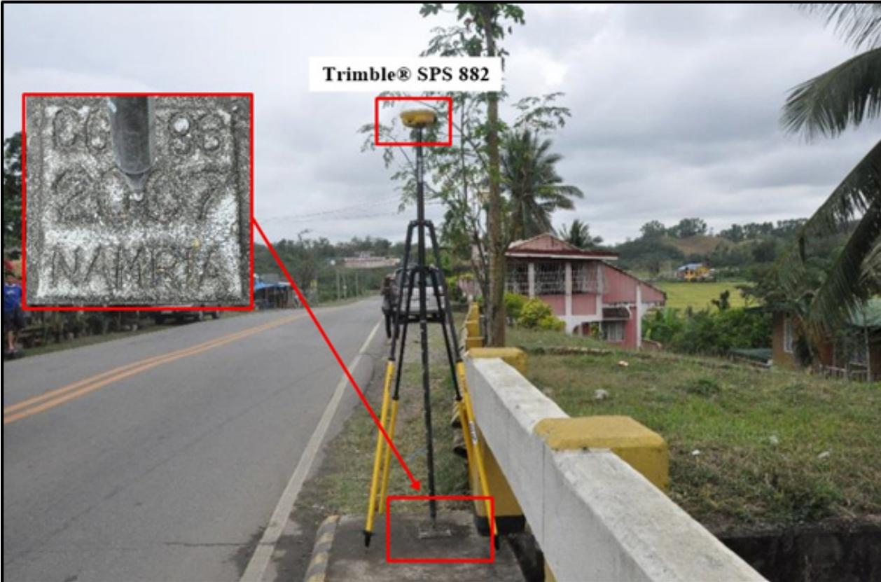
**Figure 24.** Trimble® SPS 882 setup at CG - 186, at Magapit Bridge, Brgy. Magapit, Lal-lo, Cagayan
