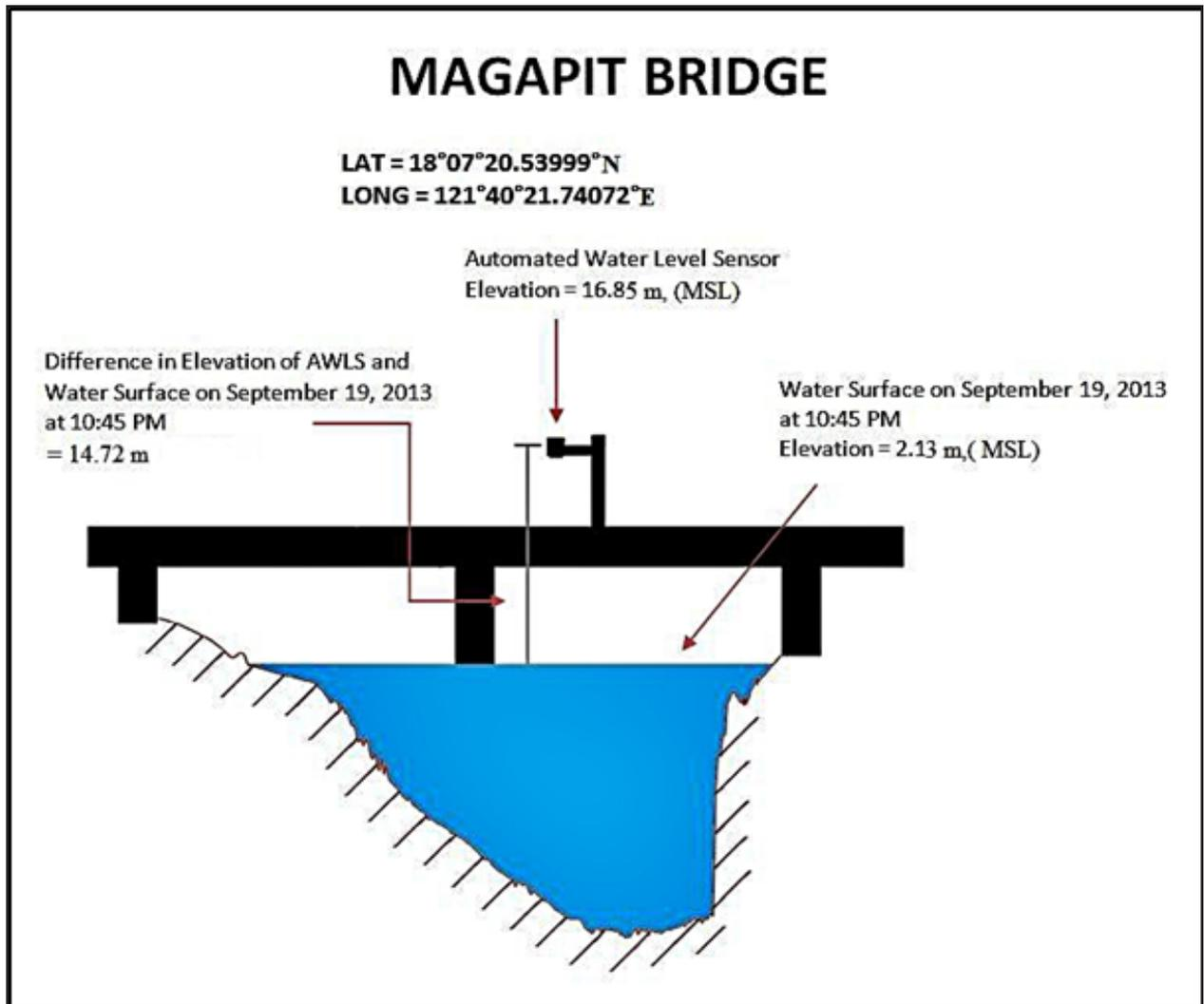
Figure 43. Magapit Bridge Cross-Section Diagram
