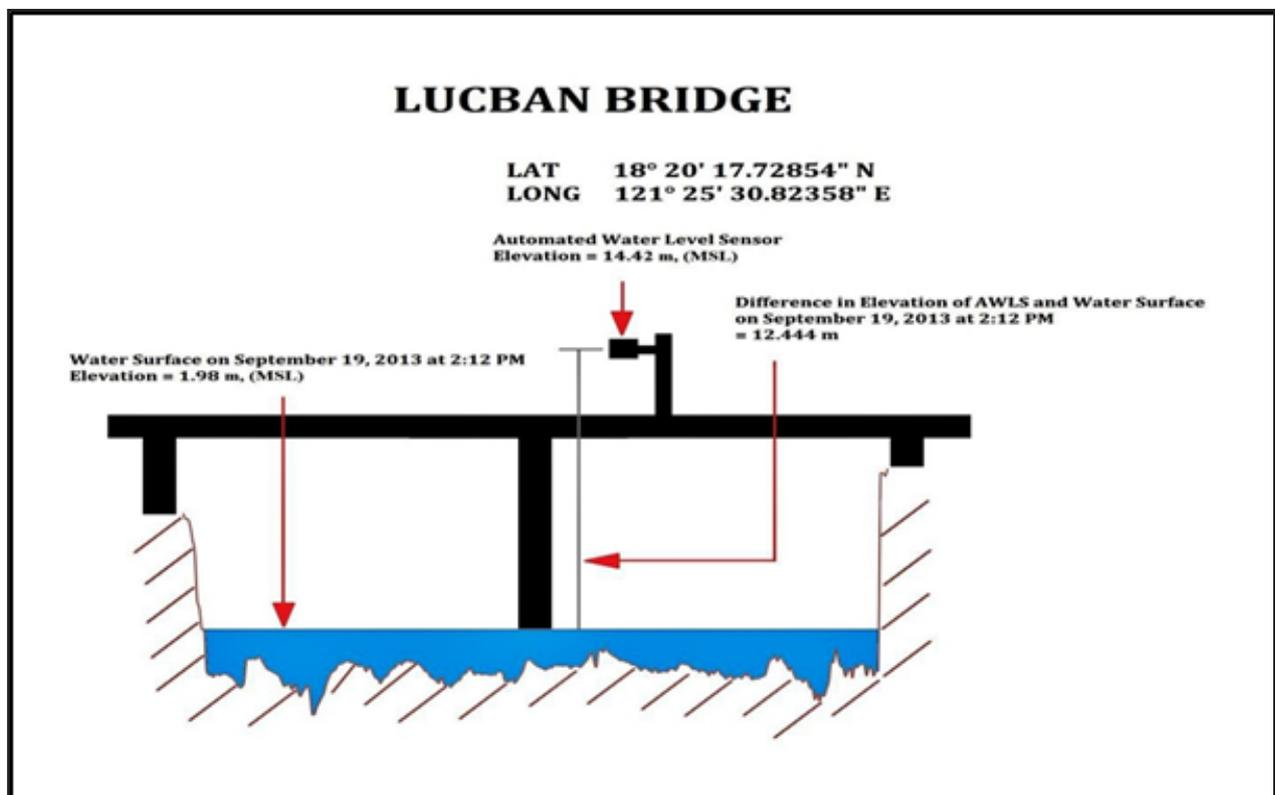
Figure 42. Lucban Bridge Cross-Section Diagram
