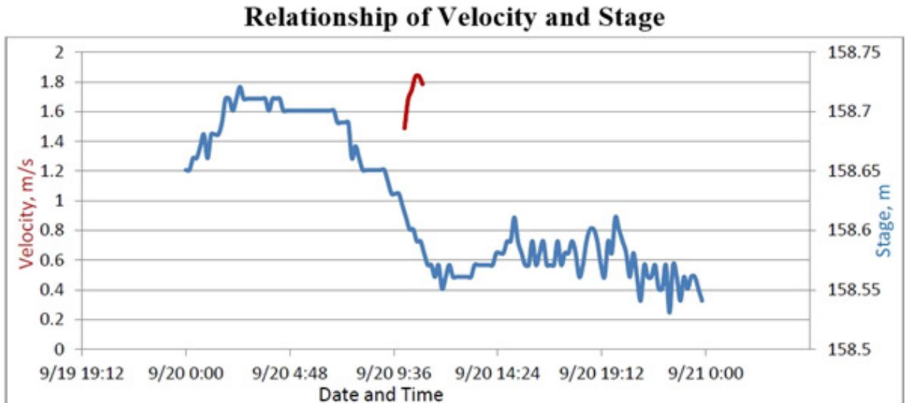
Figure 112. Relationship between velocity and stage in Sangbay Bridge within the observation period
