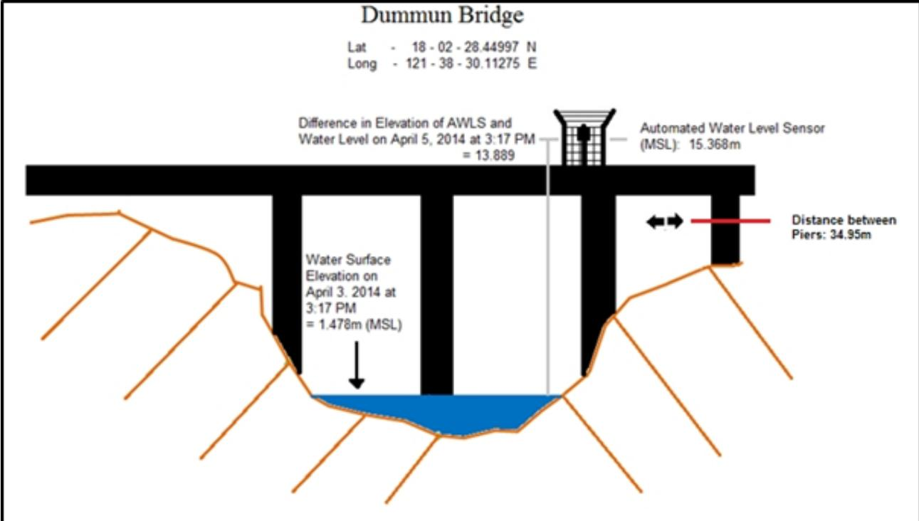
Figure 52. Dummun Bridge Cross-Section Diagram
