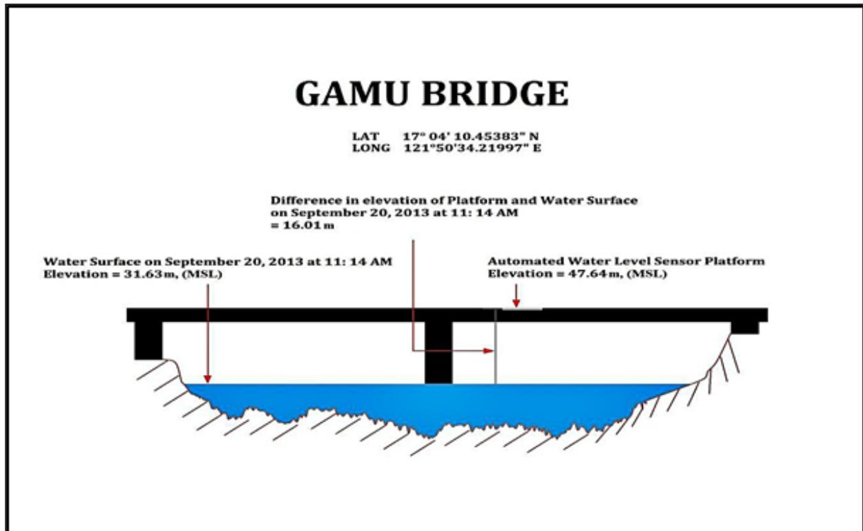
Figure 41. Gamu Bridge Cross-Section Diagram
