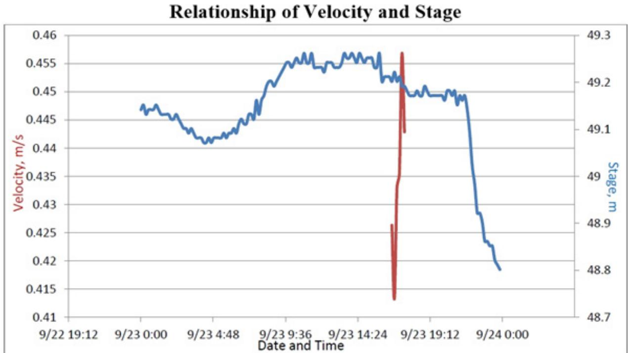
Figure 116. Relationship between velocity and stage in Siffu Bridge within the observation period
