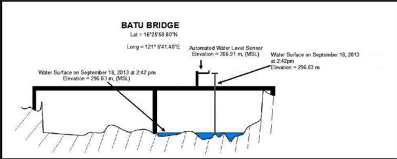
Figure 39. Batu Bridge Cross-Section Diagram
