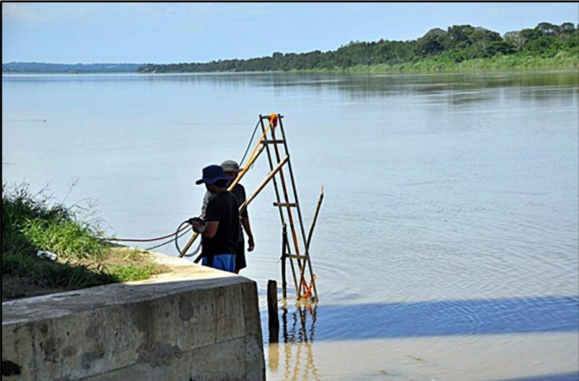
Figure 87. ADCP and Depth Gauge Deployment along Magapit Bridge
