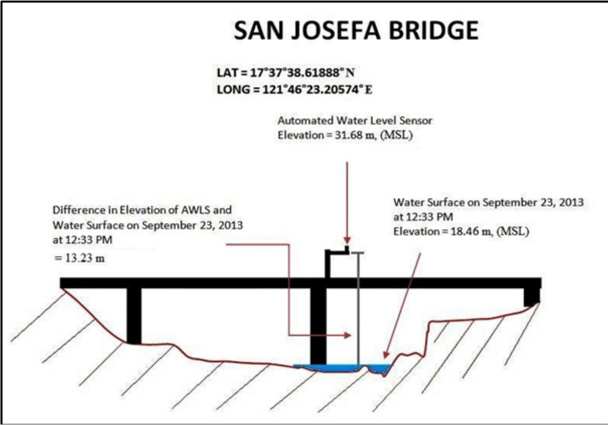
Figure 47. San Josefa Bridge Cross-Section Diagram
