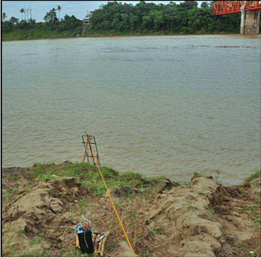
Figure 86. ADCP and Depth Gauge Deployment along Gamu Bridge
