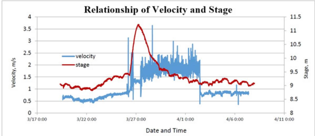
Figure 120. Relationship between velocity and stage in Buntun Bridge within the observation period
