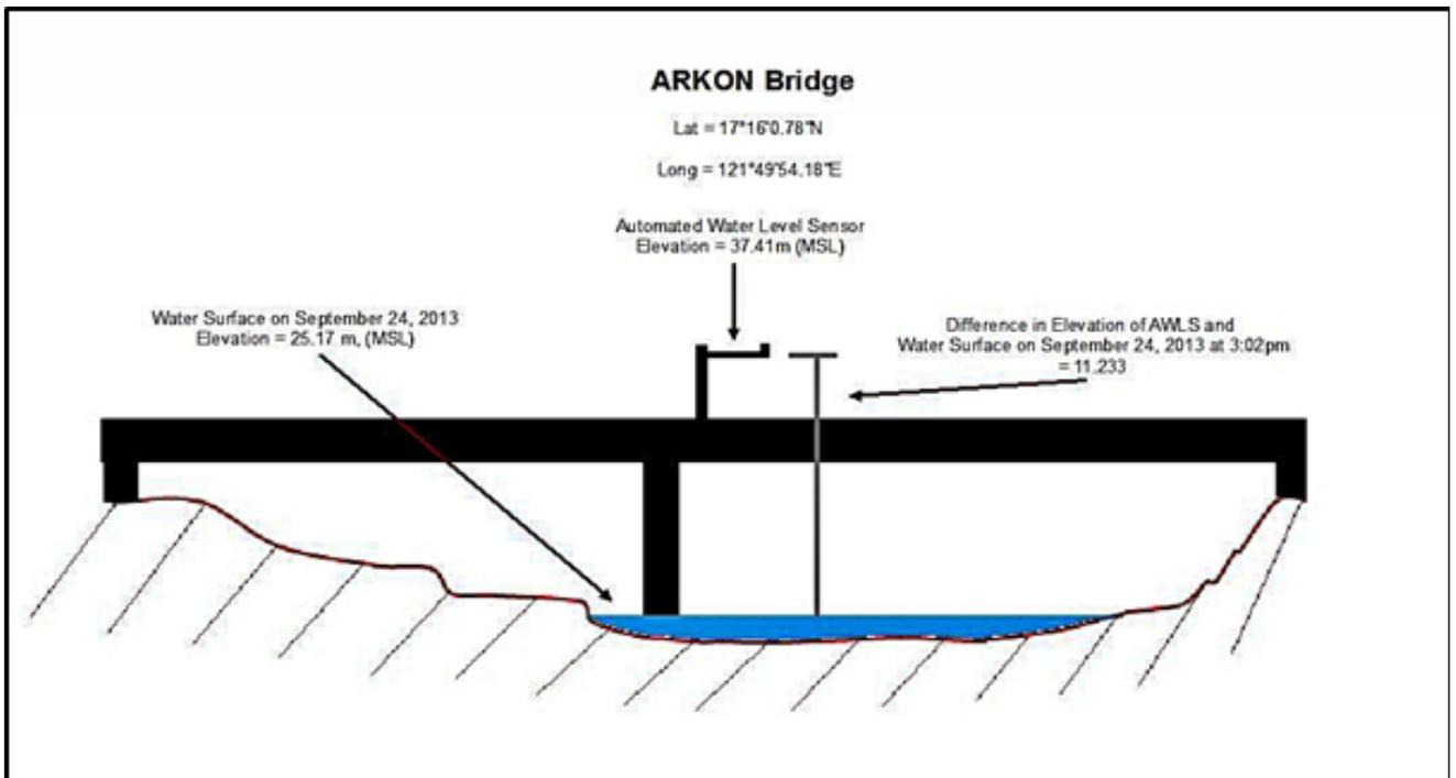
Figure 38. Arkon Bridge Cross-Section Diagram
