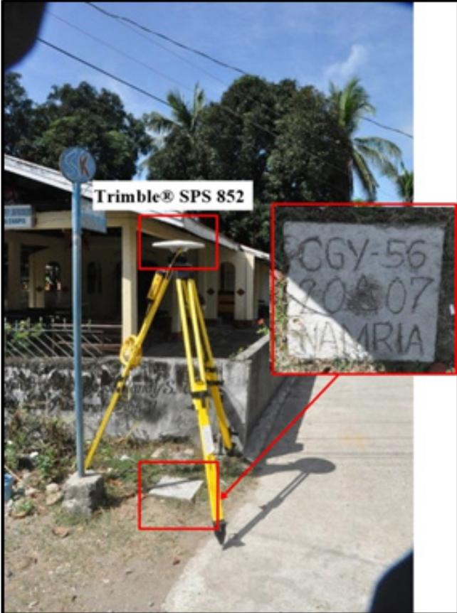
Figure 17. GNSS base set up, Trimble® SPS 852 at CGY-56 in Tuguegarao City, Cagayan
