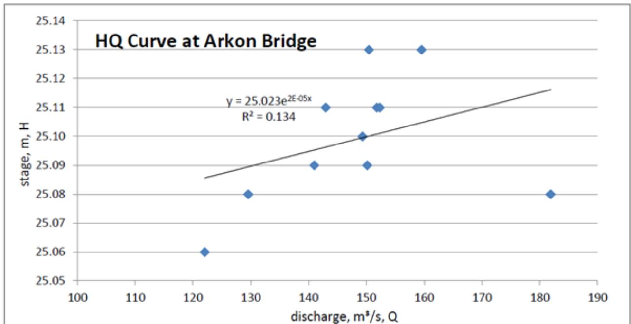
Figure 95. Relationship between stage and discharge in Arkon Bridge within the observation period
