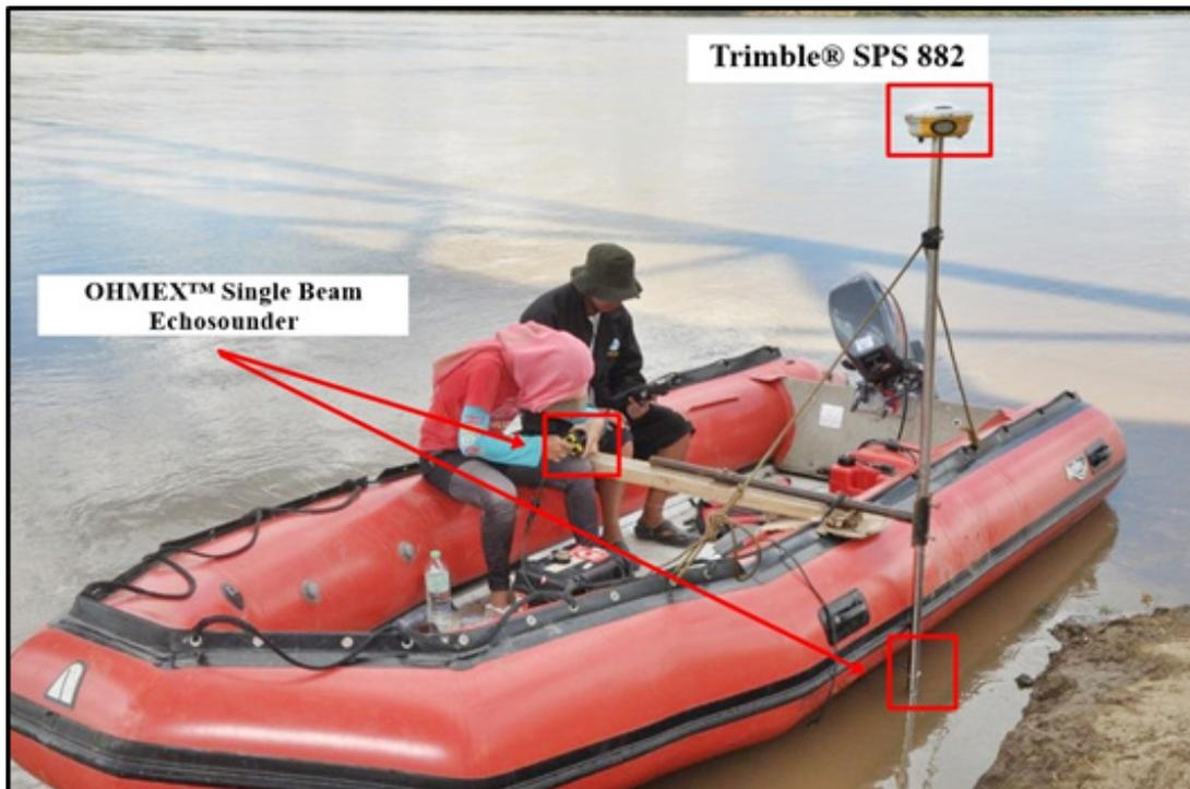
Figure 63. Bathymetric survey (Phase 1) setup with installed Ohmex™ Single Beam Echosounder and mounted Trimble® SPS 882
