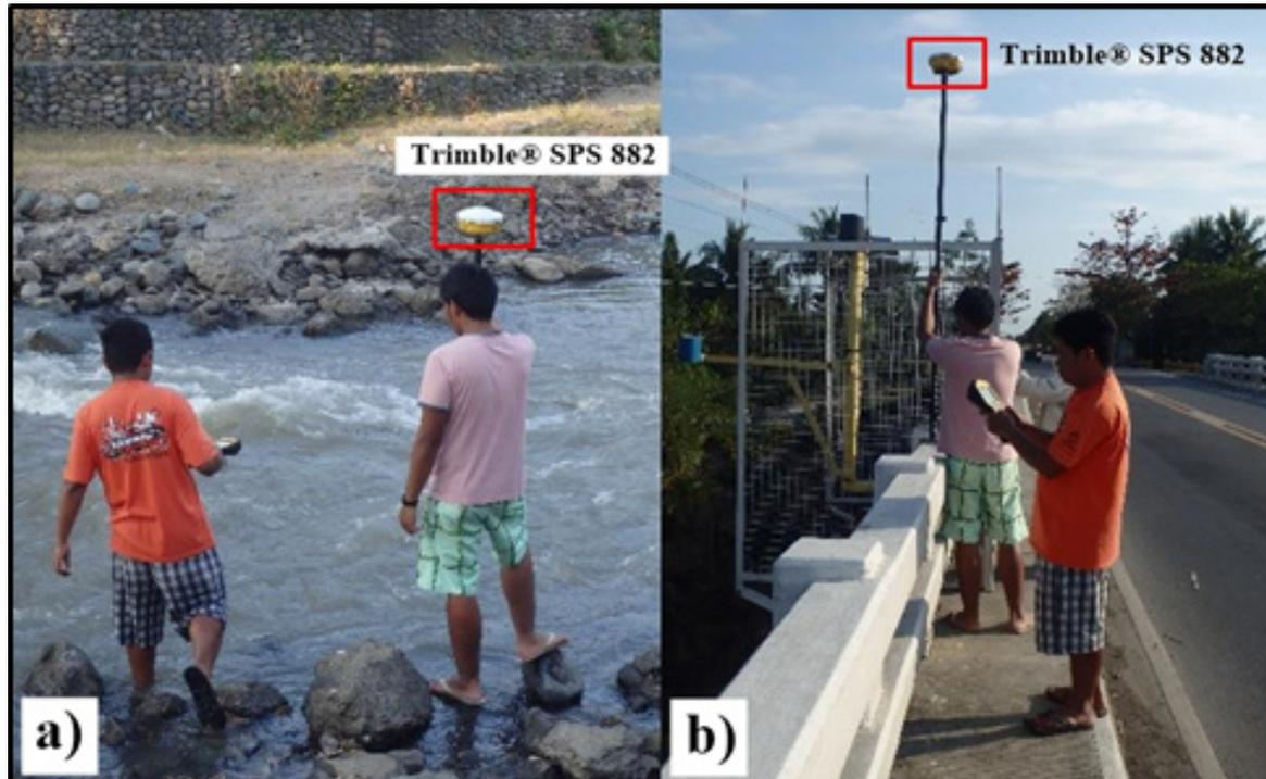
**Figure 35.** Actual cross section survey in Mallig bridge during Cagayan River Survey Phase 2 on January 29-February 12, 2014 (a) Gathering of data from the right bank of river (b) Gathering data for sensor elevation
