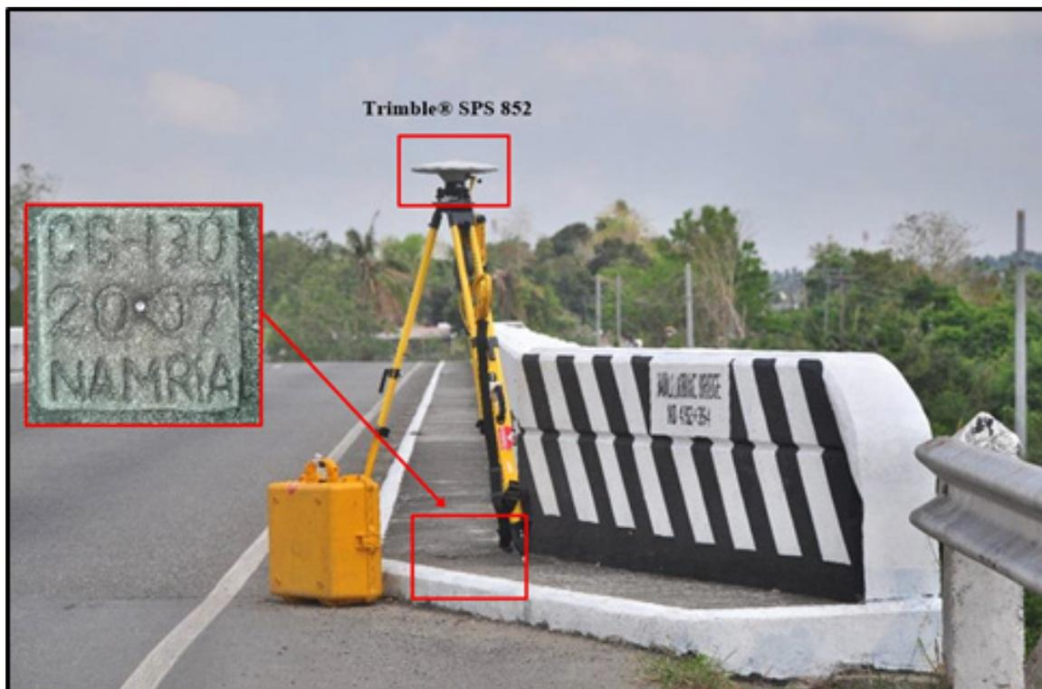
Figure 16. Trimble® SPS 852 setup at CG-130 in Iguig, Cagayan
