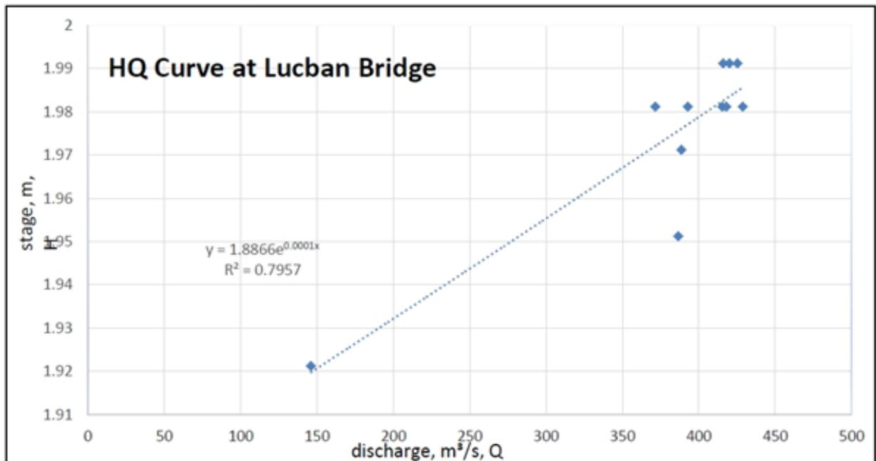
Figure 103. Relationship between stage and discharge in Lucban Bridge within the observation period
