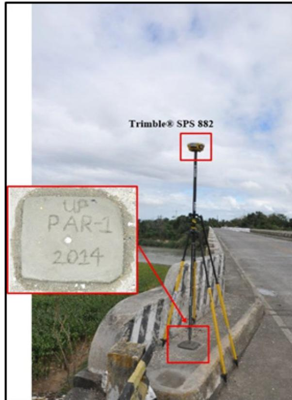
**Figure 22.** Trimble® SPS 882 setup at UP PAR-1, at Pared Bridge, Brgy. Pared, Alcala, Cagayan
