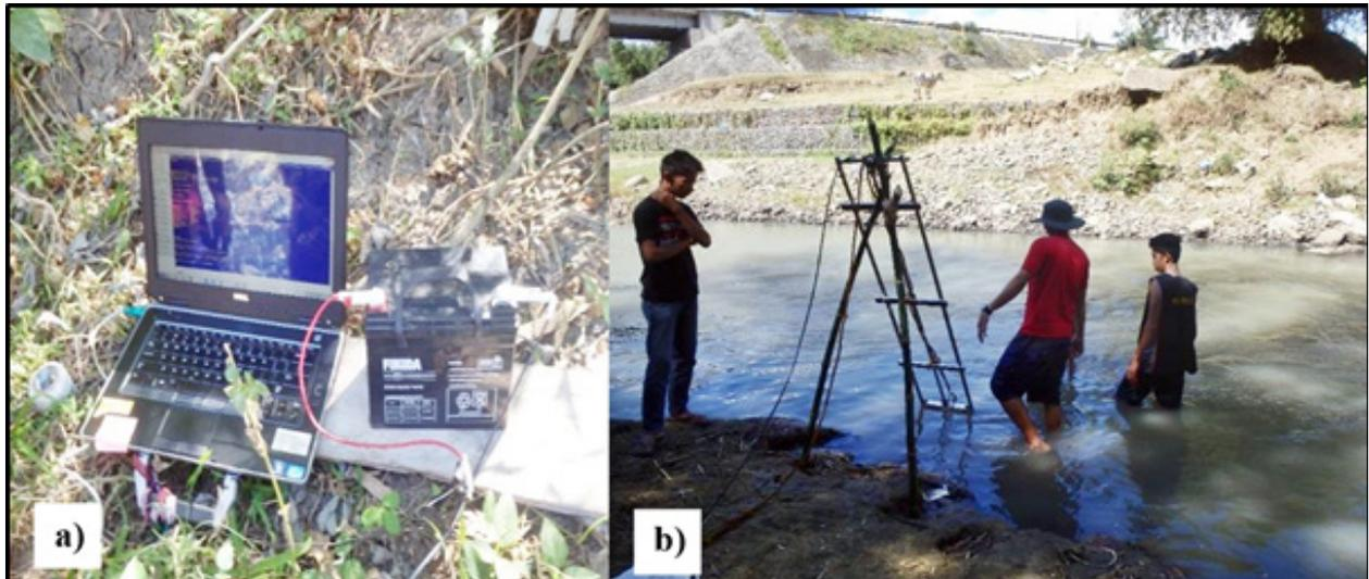
**Figure 88.** At Mallig River (a) setting up the ADCP (b) deployment of ADCP in Mallig River
