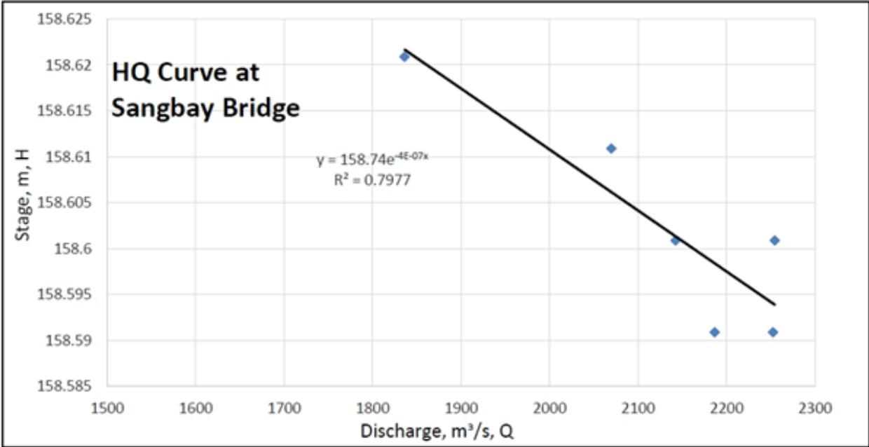
Figure 115. Relationship between stage and discharge in Sangbay Bridge within the observation period
