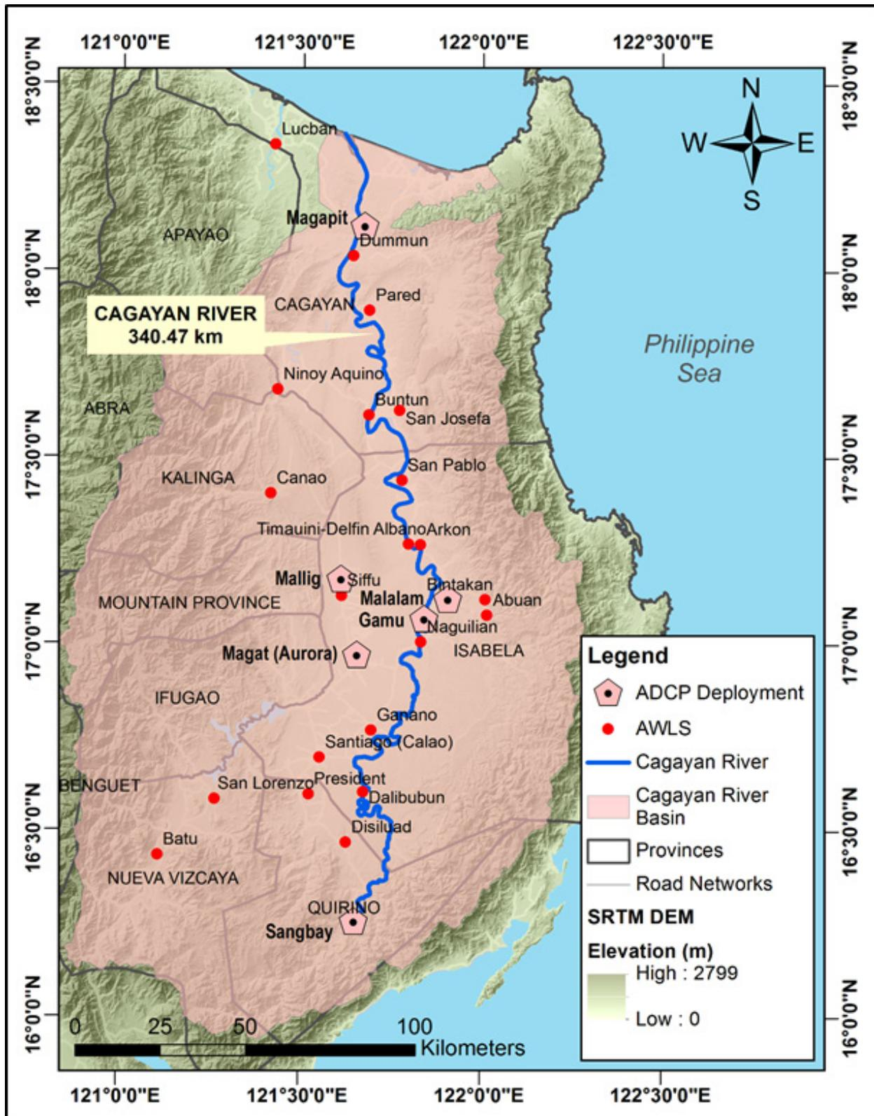
Figure 83. Location of the deployed ADCP during the Cagayan River Survey
