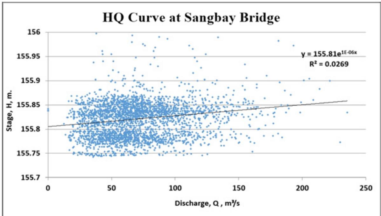
Figure 146. Relationship between stage and discharge in Sangbay Bridge within the observation period
