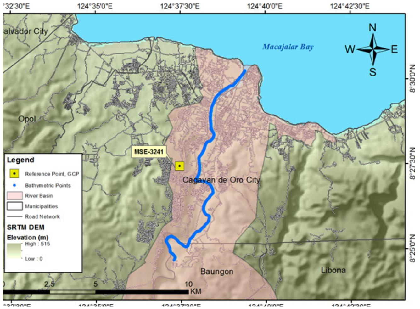
Figure 32. Bathymetry Survey along Cagayan de Oro River
