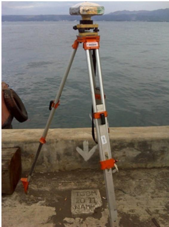
**Figure 12.** Static GNSS observation on TGBM inside Macabalan Port
