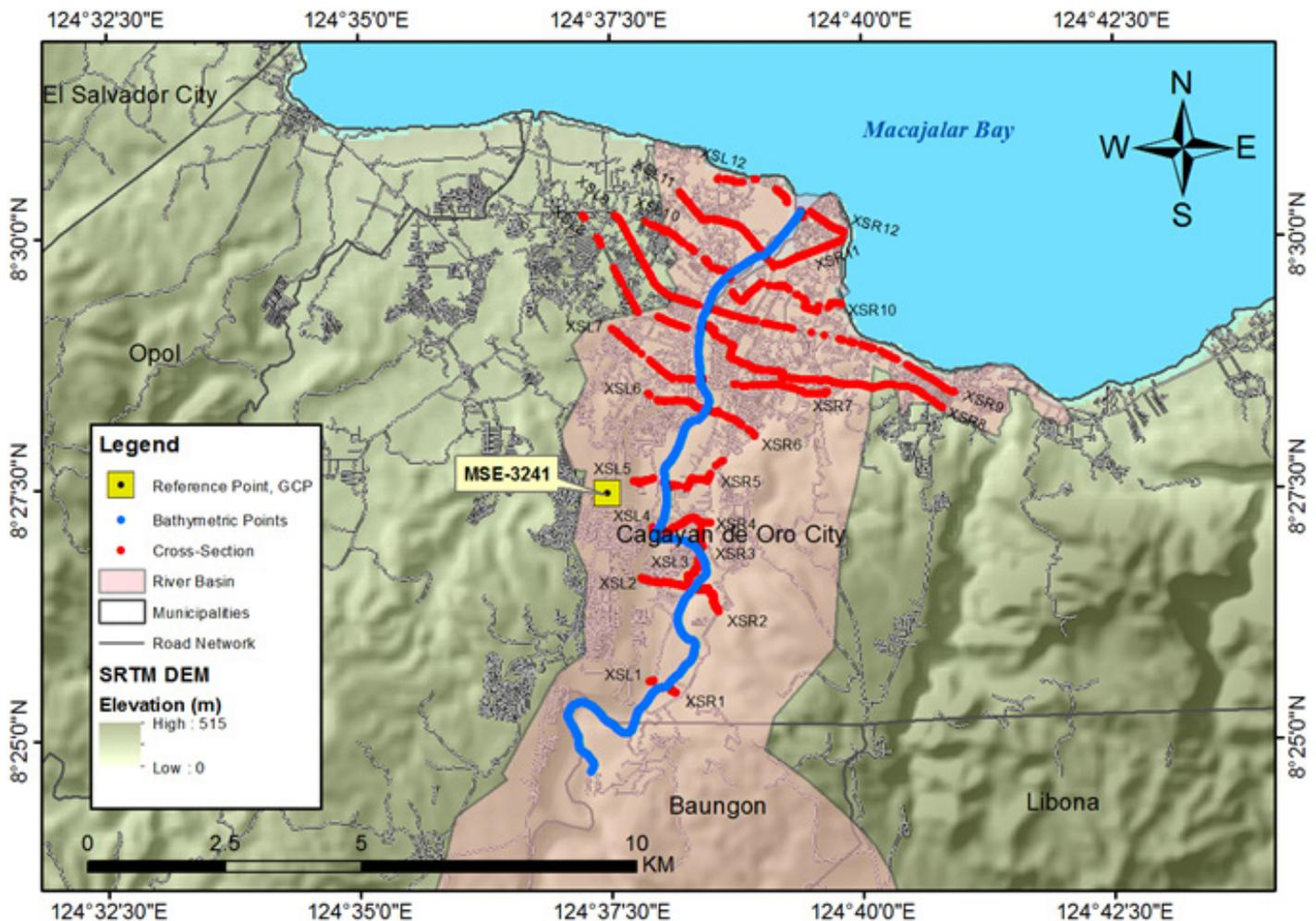
Figure 14. Cross-Section Survey for Cagayan de Oro River
