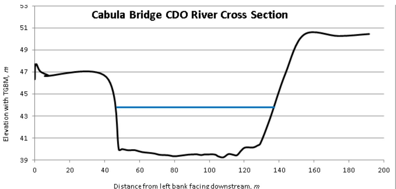
**Figure 35.** Relationship between the stage and the cross section at Cabula Bridge
