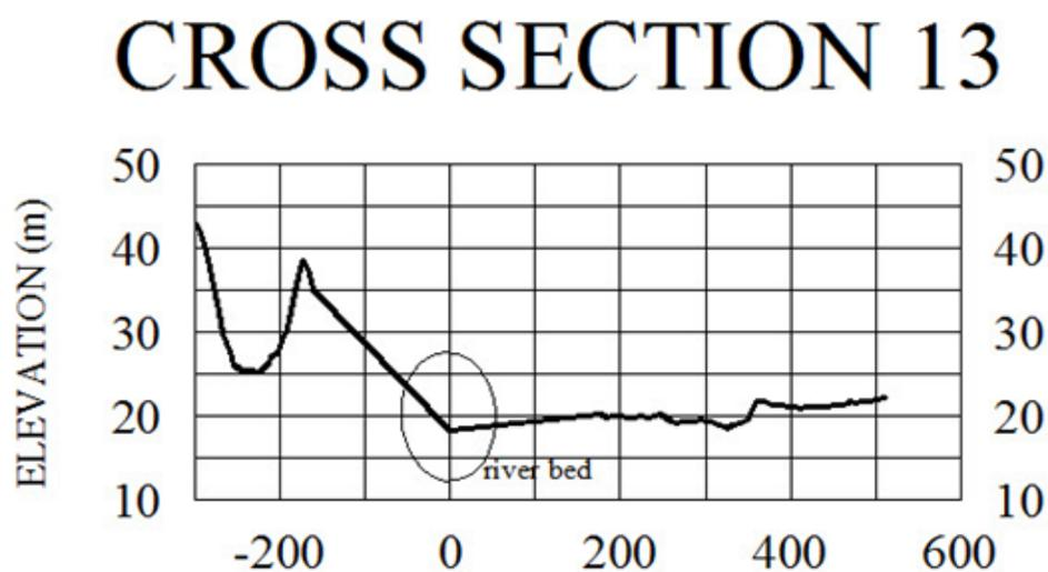
Figure 53. Cross section 13 of Hijo survey area
