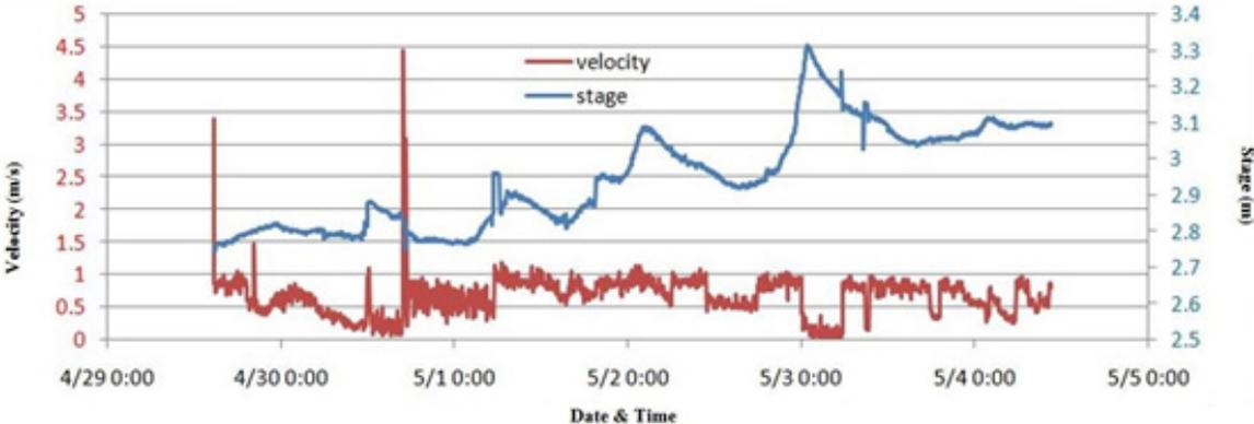
Figure 21. Stage vs velocity graph for Hijo River within the observation period
