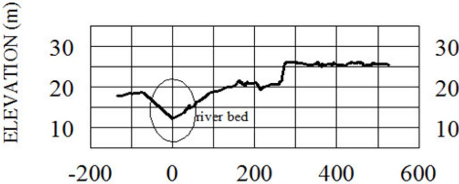
Figure 55. Cross section 15 of Hijo survey area
