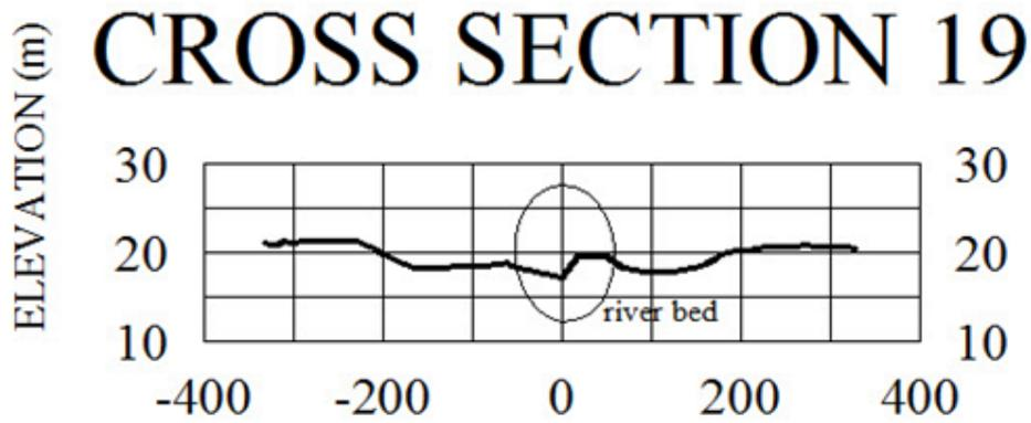
Figure 59. Cross section 19 of Hijo survey area
