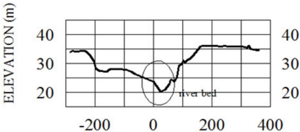
Figure 45. Cross section 5 of Hijo survey area
