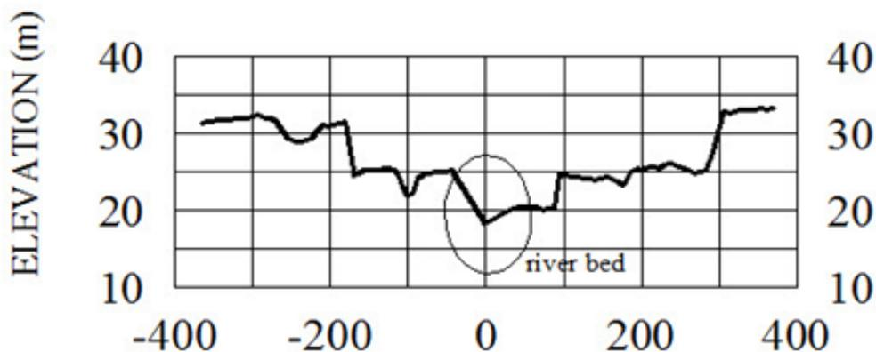
Figure 47. Cross section 7 of Hijo survey area
