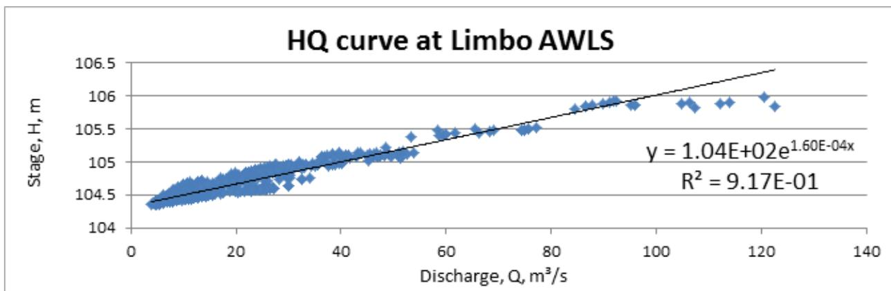
Figure 29. Stage-discharge computation in Brgy. Limbo, Maco
