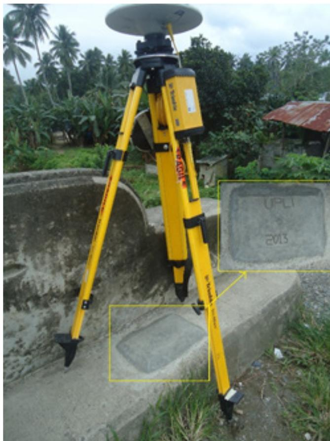
**Figure 13.** Static GNSS observation at UP-Li in Brgy. Limbo, Maco
