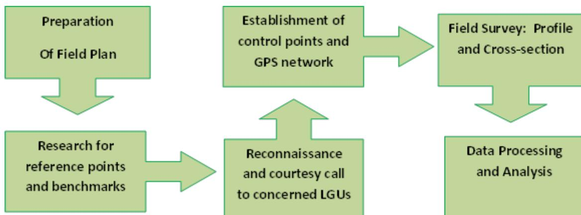
Figure 31. Flowchart of the field survey
