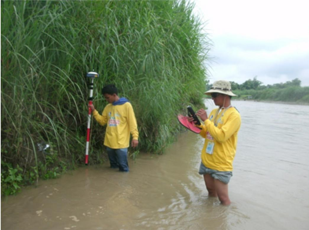
**Figure 38.** Profile team recording a reading during the profile survey of Hijo River
