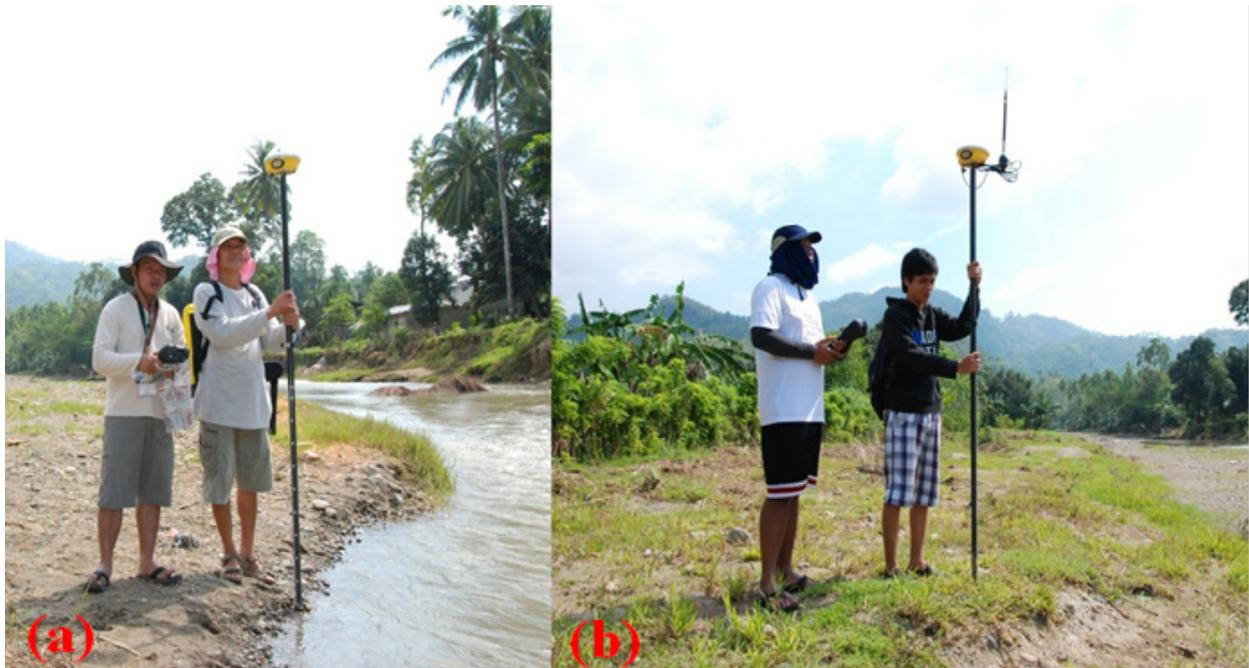
Figure 25. Profile Survey Team Conducting PPK and RTK GNSS Survey
