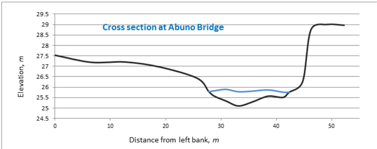
**Figure 46.** Cross section at the ADCP deployment site in Brgy. Abuno
