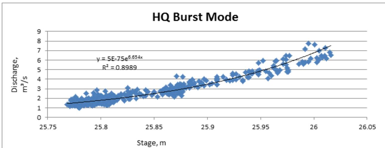
**Figure 50.** Stage-discharge computation in a burst mode along Iligan River from the ADCP deployed in Brgy. Abuno
