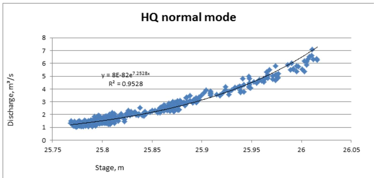
**Figure 49.** Stage-discharge computation in a normal mode along Iligan River from the ADCP deployed in Brgy. Abuno
