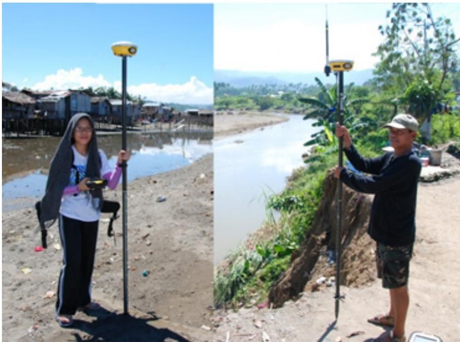
**Figure 13.** Cross Section Survey using PPK and RTK Surveying technique.
