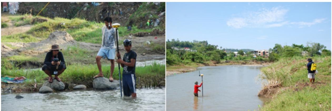
**Figure 35.** Manual bathymetric survey using PPK GNSS technique
