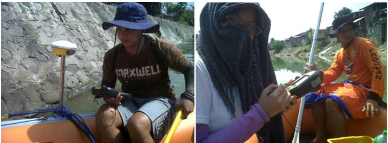
**Figure 34.** Bathymetric survey setup using Trimble®SPS 882 mounted on top of the OHMEX™ Transducer
