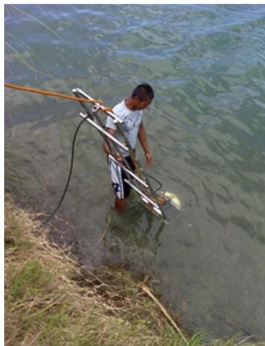
**Figure 27.** A local hire fixing the position of the Acoustic Doppler Current Profiler along the bank of Ilog-Hilabangan River in Brgy. Camansi, Kabankalan City
