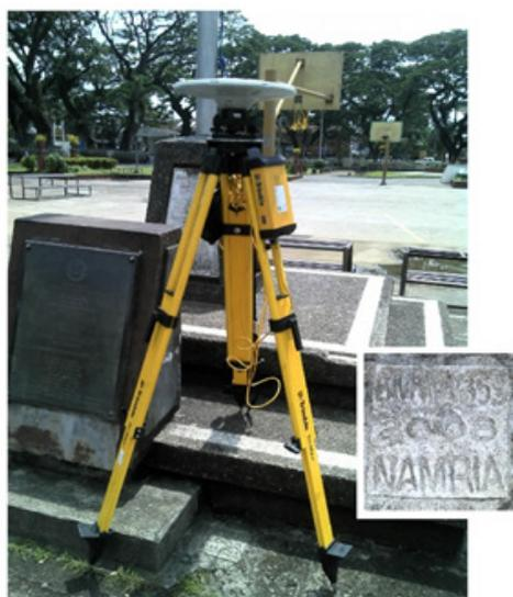
**Figure 31.** PPK base station at BM-NW 353 located in front of the old Municipal Hall of Kabankalan City
