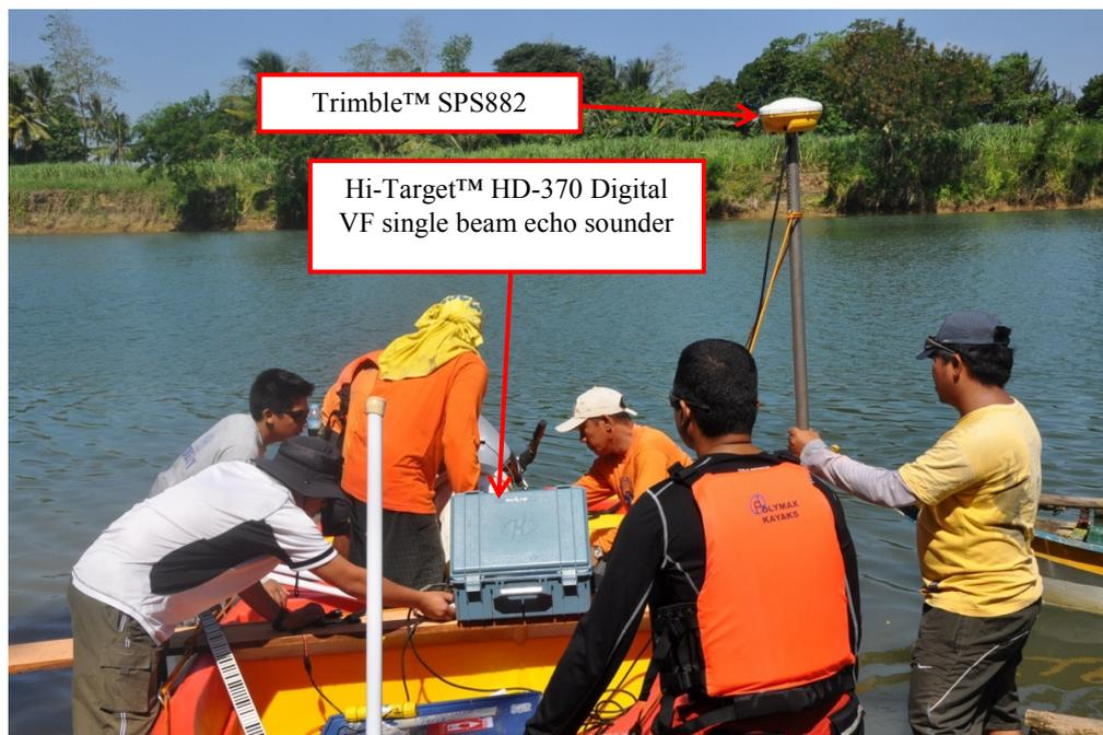
**Figure 18.** The set-up of instruments for the bathymetry survey with the Trimble® SPS882 mounted on top of the Hi-Target™ Transducer
