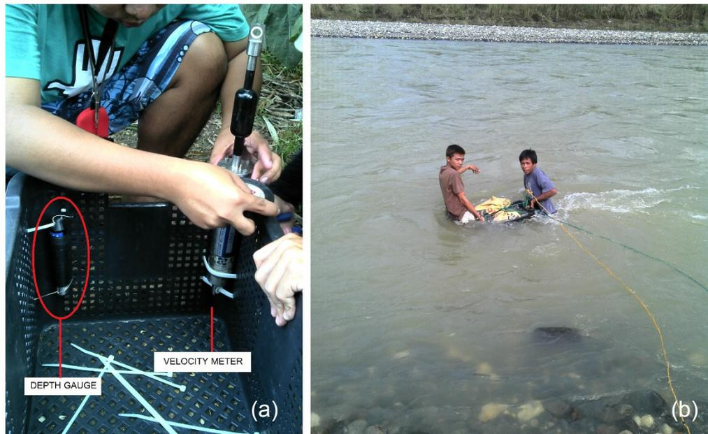
**Figure 33.** (a) Velocity Meter and Depth Gauge set-up (b) Deployment site of the Velocity Meter at Hilabangan Bridge, Kabankalan City, Negros Occidental
