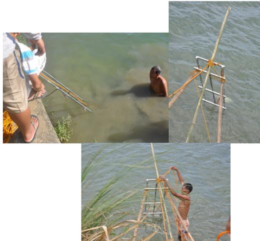
**Figure 26.** A series of images of ADCP deployment on the bank of Ilog-Hilabangan River in Brgy. Camansi, Kabankalan City
