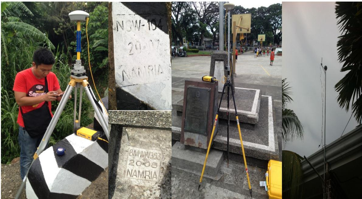
Figure 49. Reference point, Benchmark and established point: a.) NGW 104 for Reference point, b.) NGW 353 for Benchmark and c.) Internet Base Satellite System.
