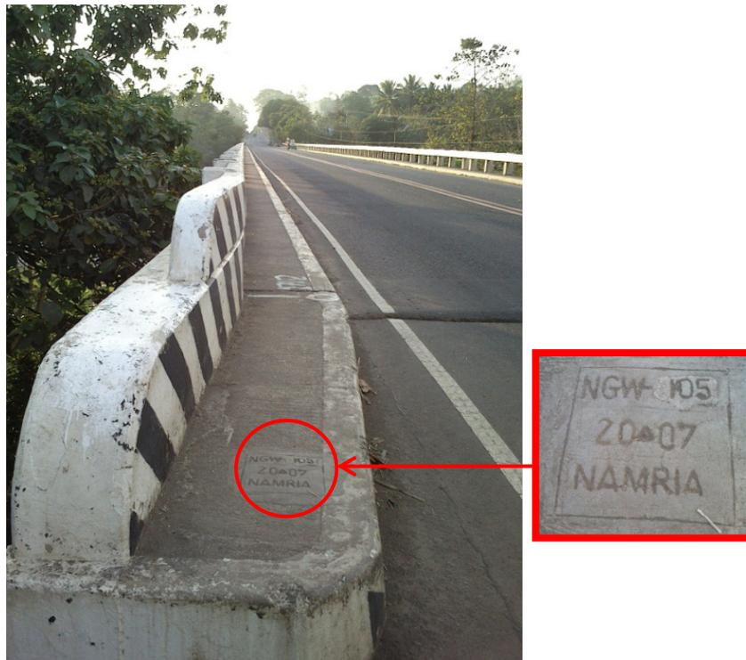
Figure 15. NGW-105 is located in Ilog-Hilabangan Bridge that was also used to establish a GNSS Network
