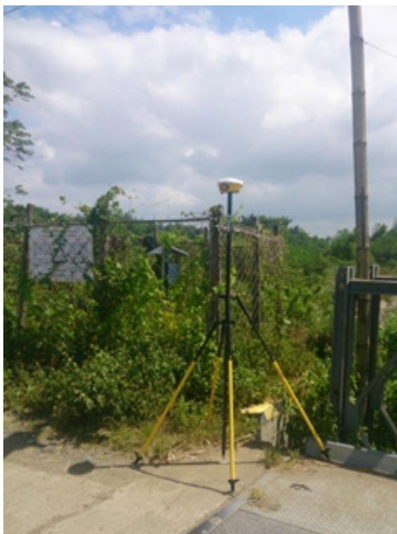
**Figure 10.** Static GNSS observation at Cahigon Bridge in Maasin
