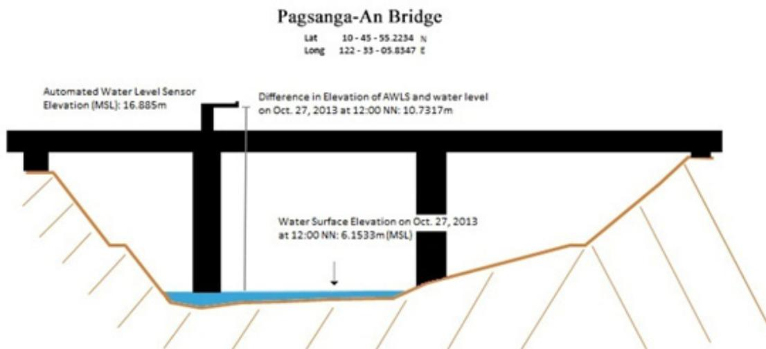
Figure 18. Pagsanga-An Bridge along Tigum River in Pavia, Iloilo
