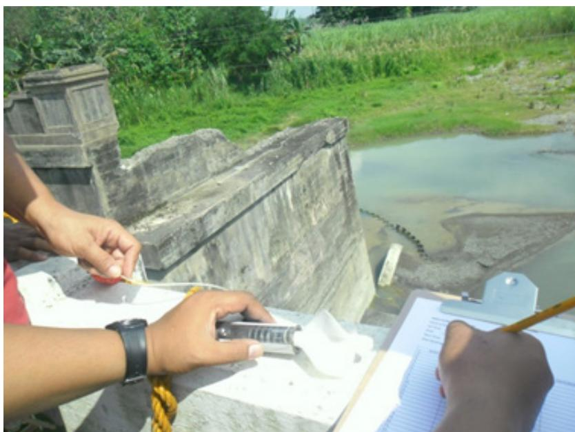
**Figure 20.** Flow measurements using a rotor-type flow meter
