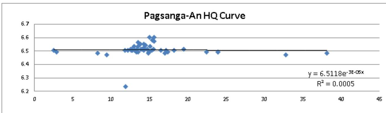
**Figure 30.** HQ Curve for Pagsanga-An Bridge
