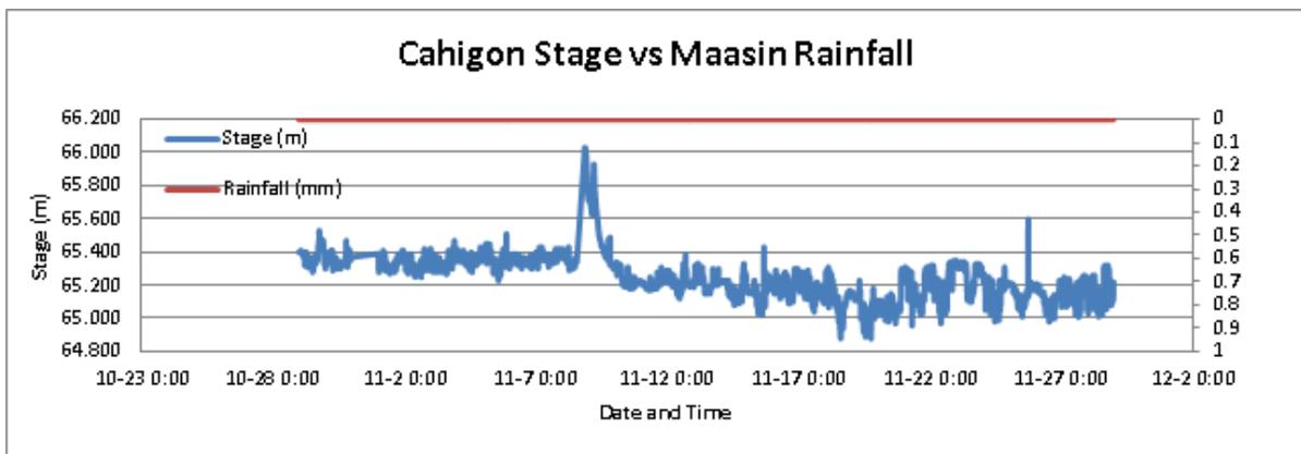
Figure 23 .Stage vs Rainfall for Cahigon Bridge
