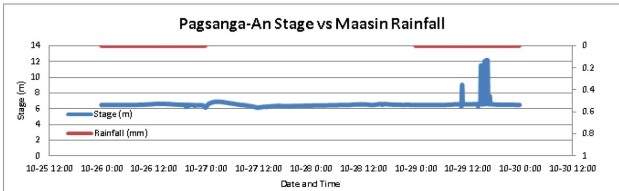
**Figure 28.** Stage vs Rainfall at Maasin for Pagsanga-An Bridge
