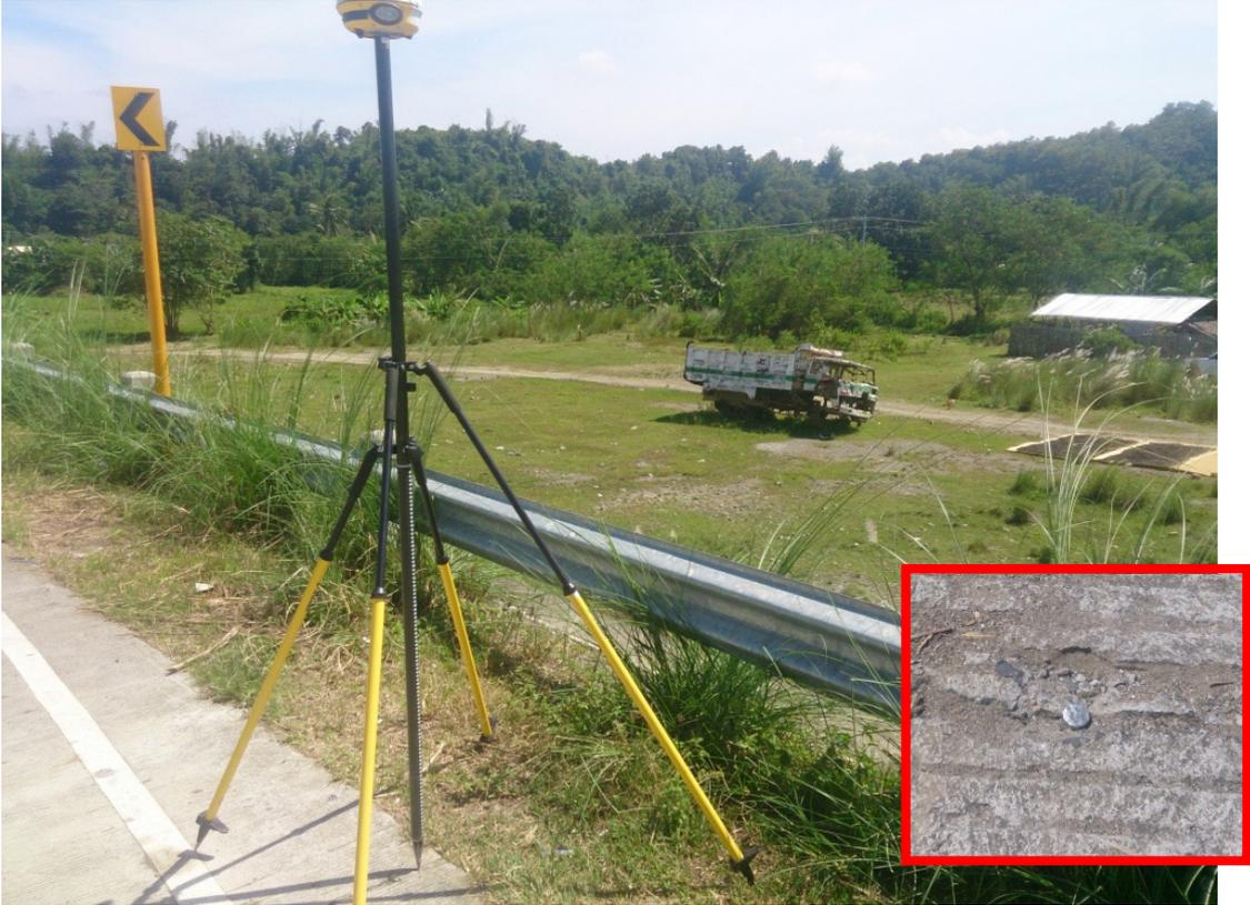
Figure 13. Static GNSS observation at Nichols Bridge in Alimodian
