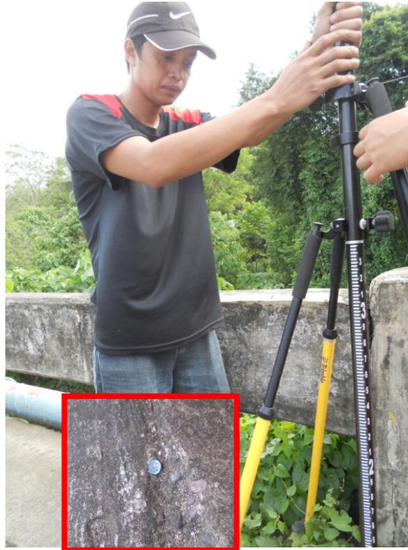
Figure 15. Static GNSS observation at San Miguel Bridge, San Miguel
