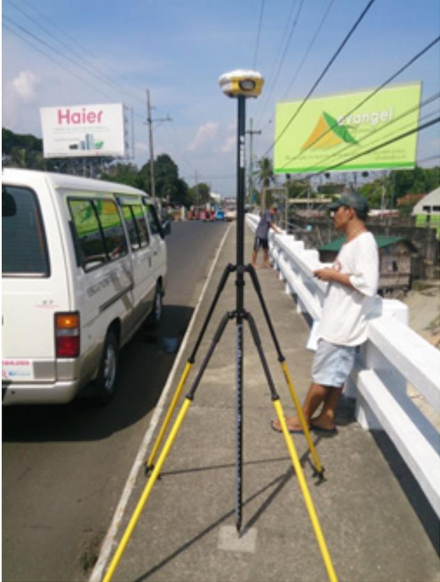
Figure 11. Static GNSS observation at control point J-11 1999 in Jaro Bridge in Iloilo City
