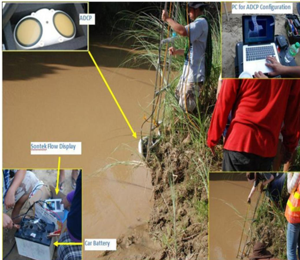
Figure 39. First deployment of Acoustic Doppler Current Profiler at Bulao Bridge
