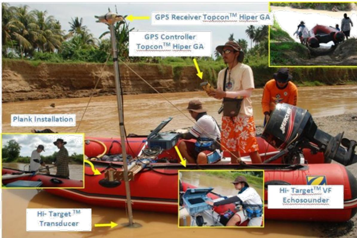
Figure 30. Bathymetric survey setup
