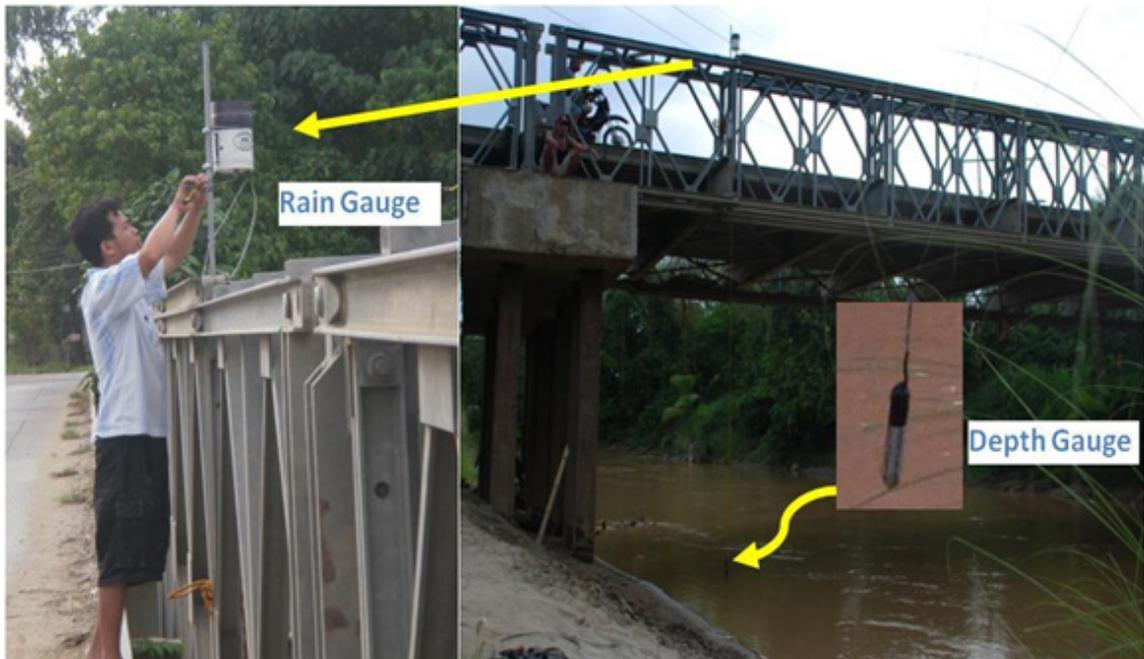
Figure 38. Rain gauge and depth gauge deployment at Bulao Bridge
