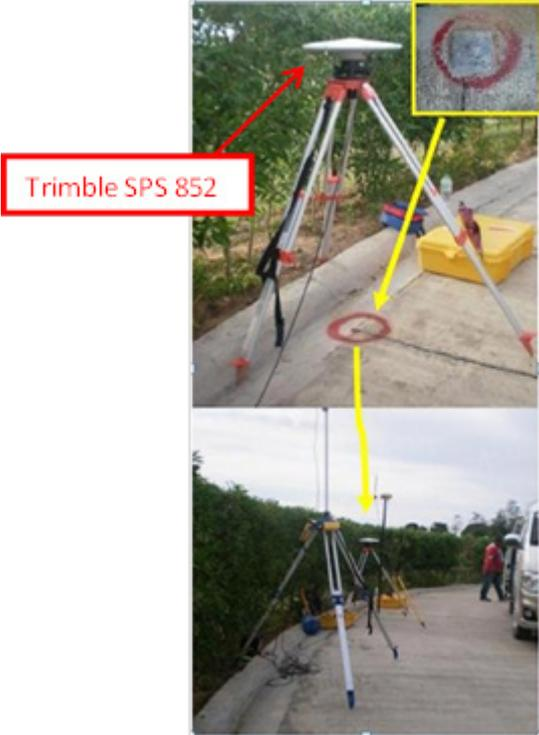
**Figure 13.** Static GNSS observation at a control point at Golden Heaven Cemetery, Cagayan De Oro City
