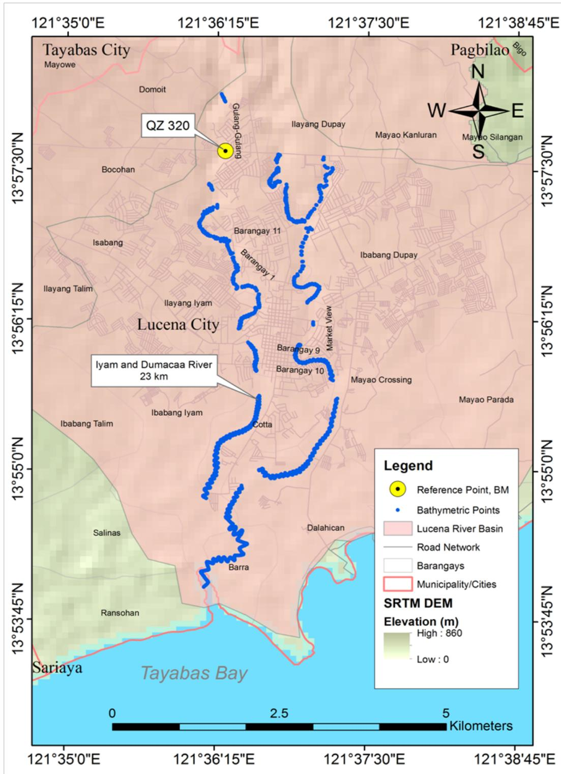
Figure 14. Bathymetric data in Iyam and Dumacaa River
