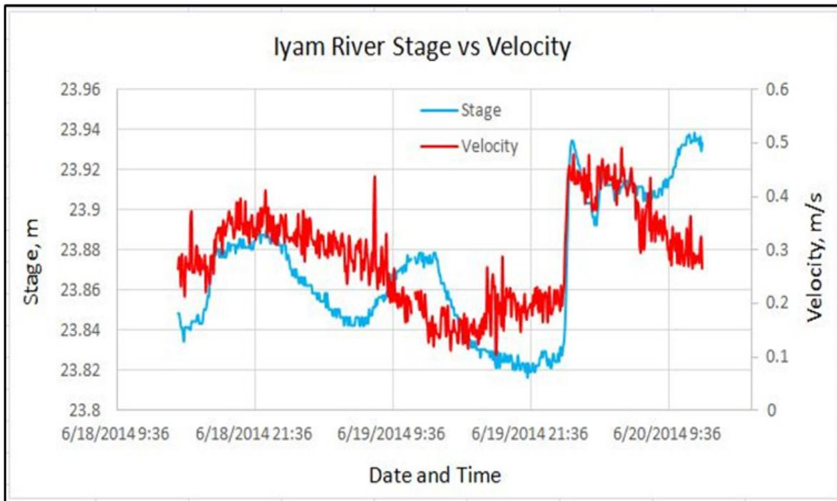
Figure 32. Iyam River stage vs. velocity graph
