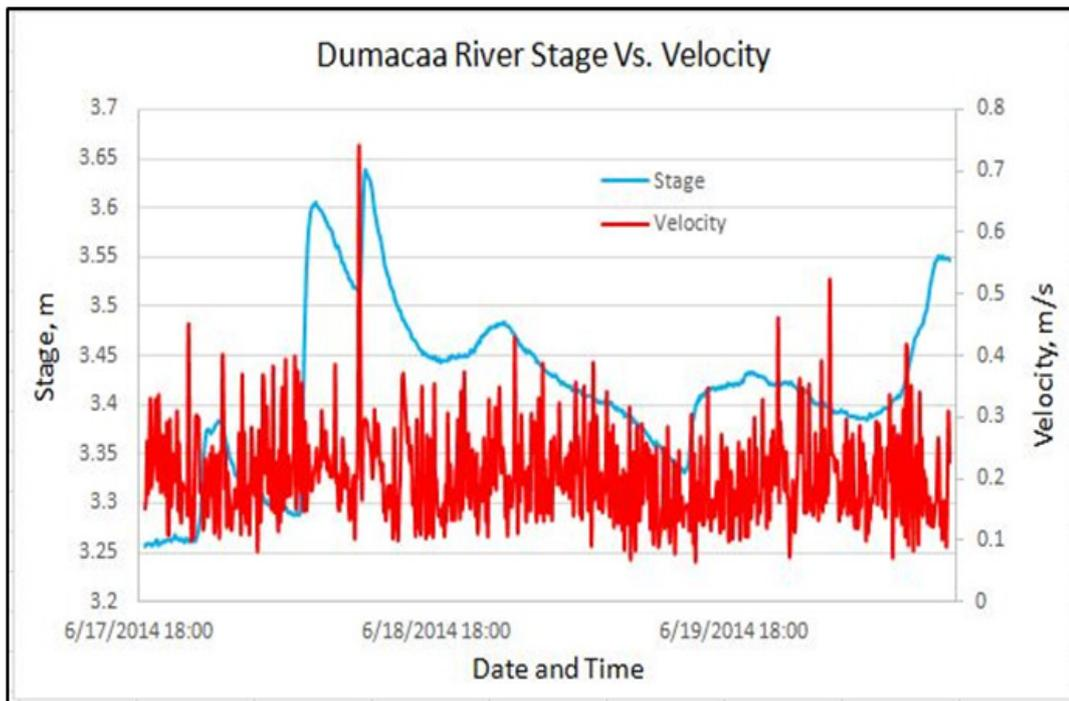
Figure 27. Dumacaa River stage vs velocity graph
