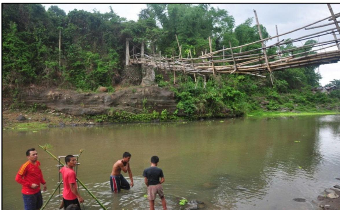
**Figure 18.** ADCP with Depth Gauge deployed along Iyam River in Brgy. Gulang-Gulang, Lucena
