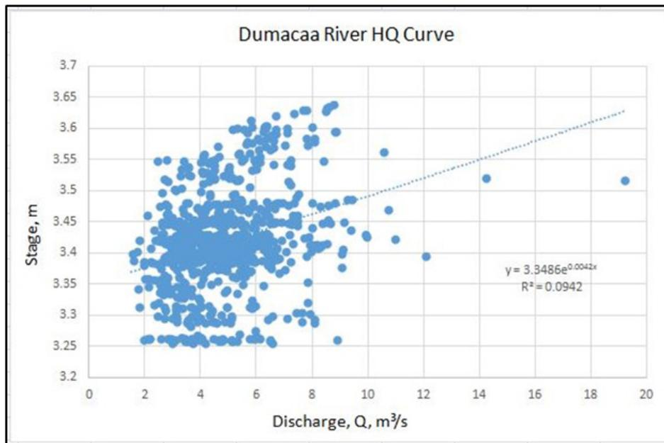
**Figure 29.** Stage-discharge computation at Dumacaa River
