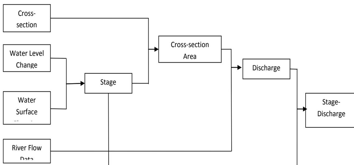
**Figure 7.** Flow Chart for Stage-Discharge Correlation Computation
