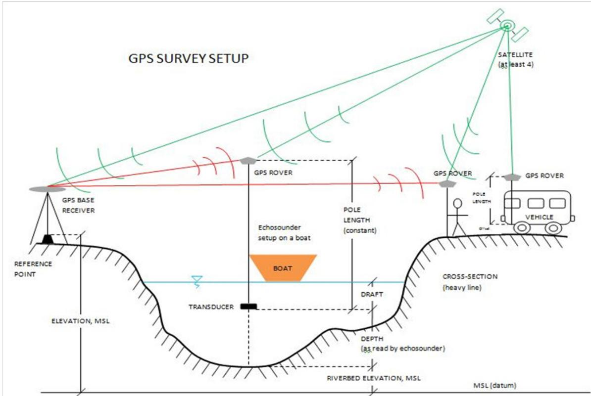
Figure 8. Setup for GNSS Surveys
