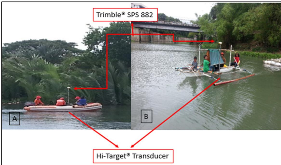
Figure 13. Bathymetry survey setup
