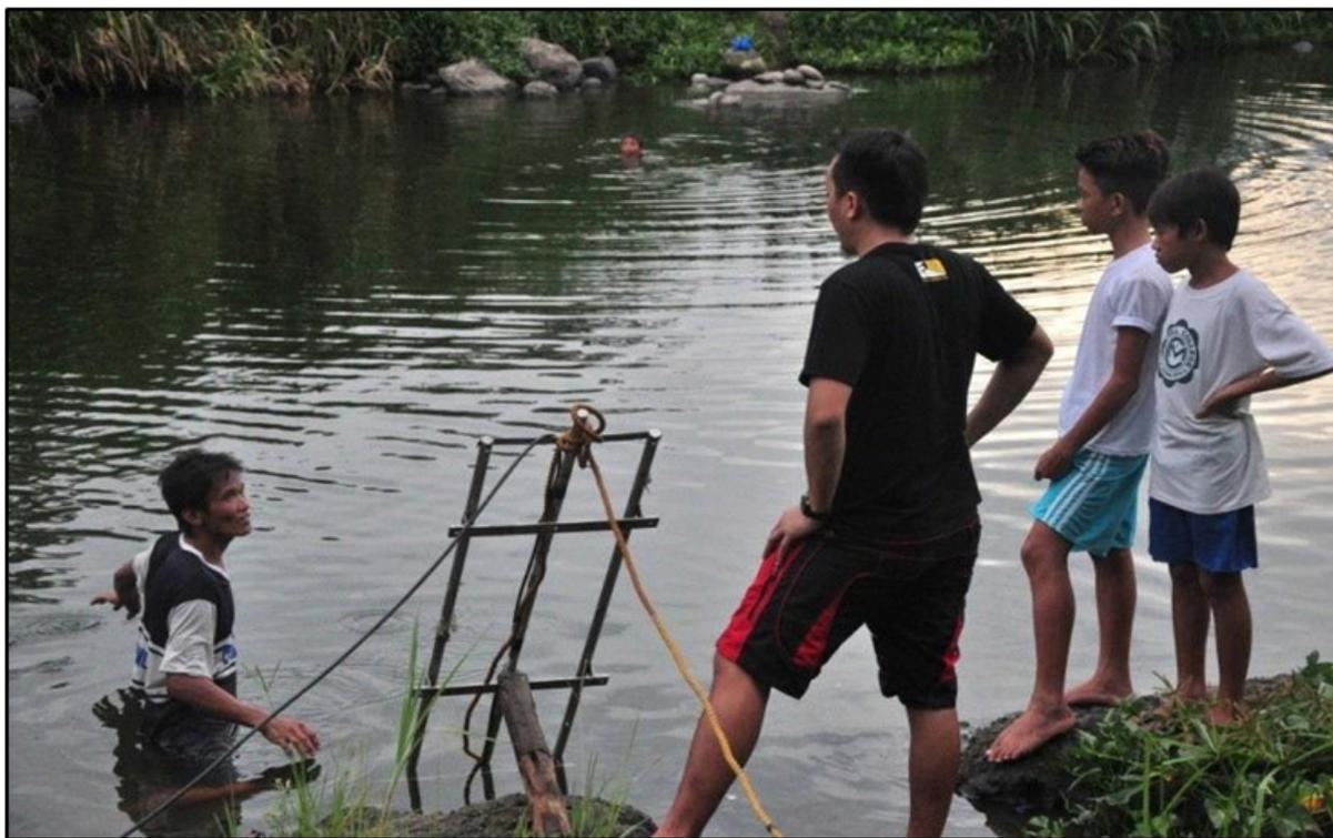
**Figure 16.** ADCP with Depth Gauge deployed along Dumacaa River in Brgy. Ibabang Dupay, Lucena
