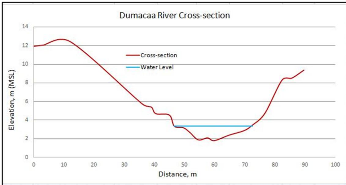
Figure 25. Dumacaa River cross-section plot
