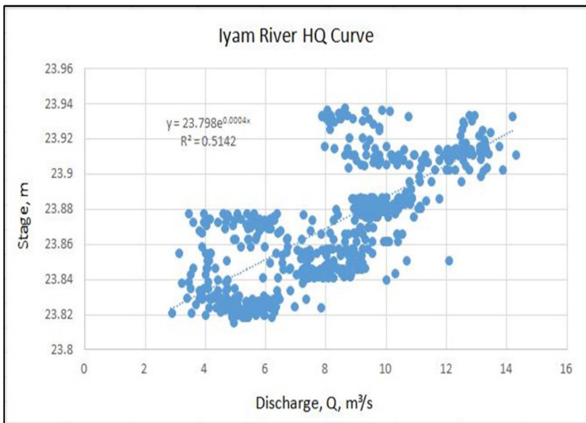
Figure 34. Stage-discharge computation at Iyam River
