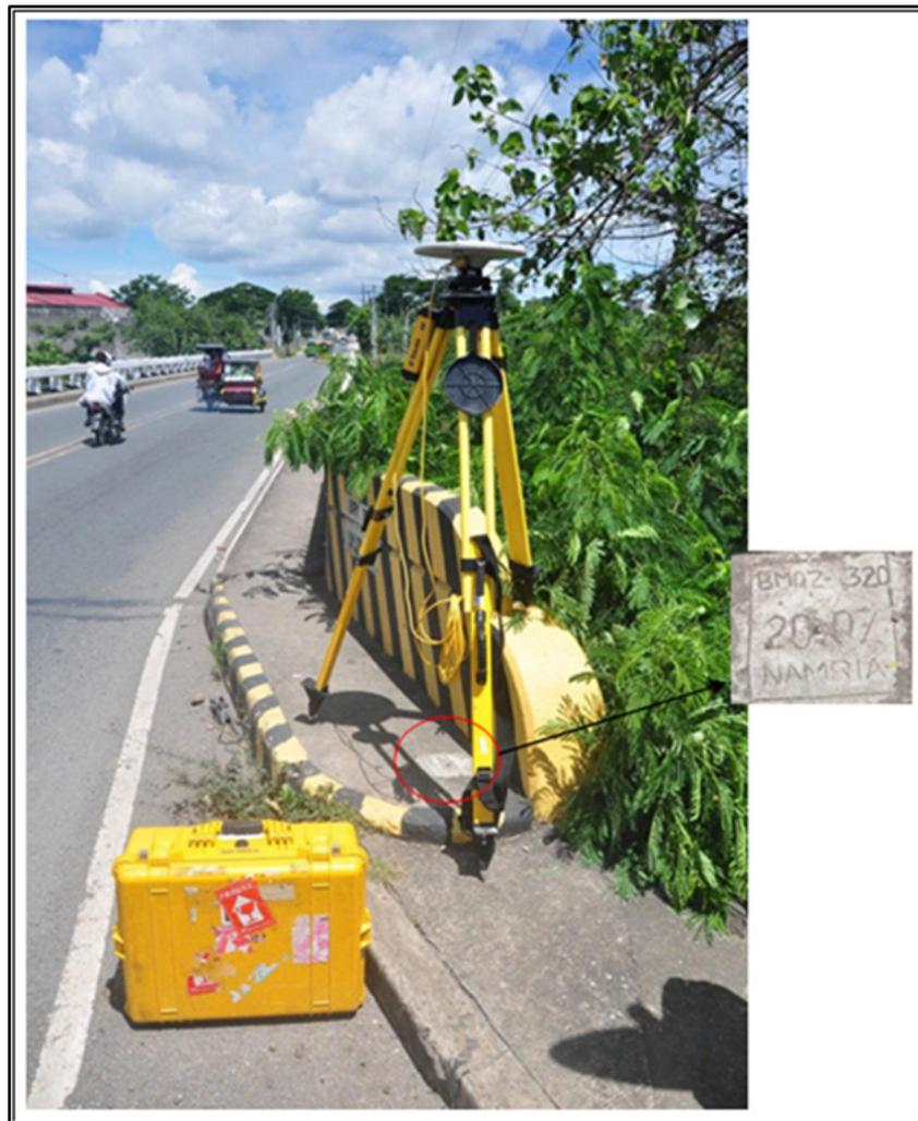
**Figure 12.** Static GNSS observation at BMQZ-320 at Iyam Bridge, Lucena City
