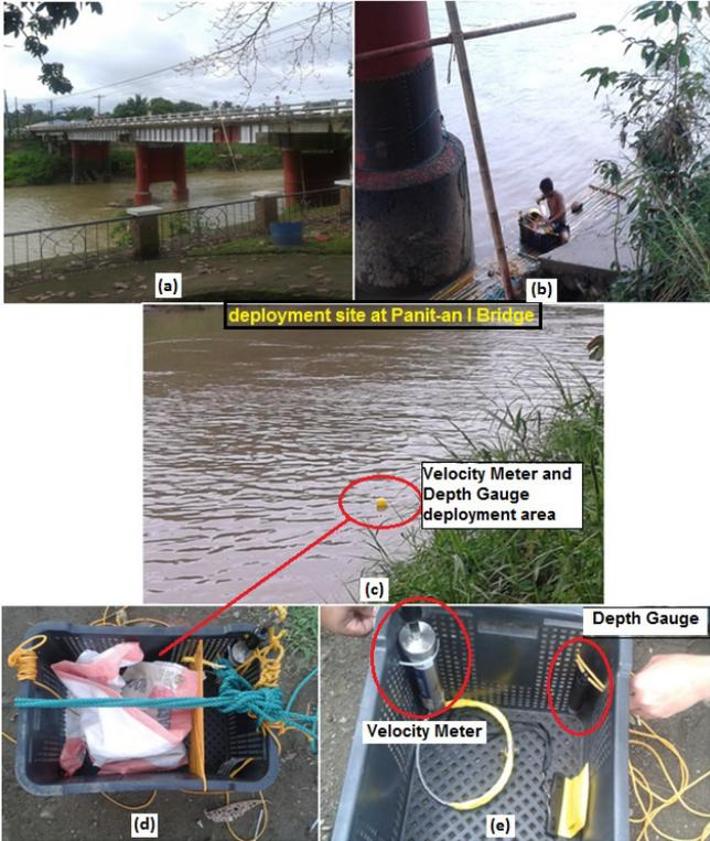
Figure 19. Deployment of Velocity Meter and Depth Gauge (a) Panit-an Bridge, (b) Preparation of the deployment site, (c) buoy tied to the crate, (d) & (e) actual set-up of the depth gauge and velocity meter
