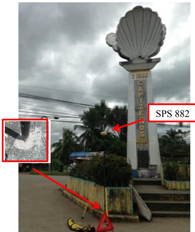
**Figure 12.** Static GNSS observation at CP-175, a benchmark at Barangay Lanot, Roxas City, Capiz
