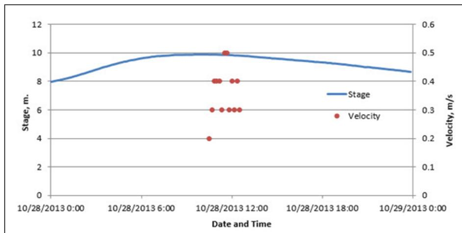
**Figure 31.** Relationship between Water Velocity and Stage at Sigma Bridge
