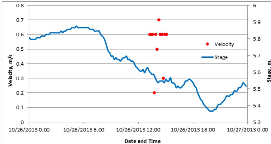
Figure 35. Relationship between Water Velocity and Stage at Maayon Bridge
