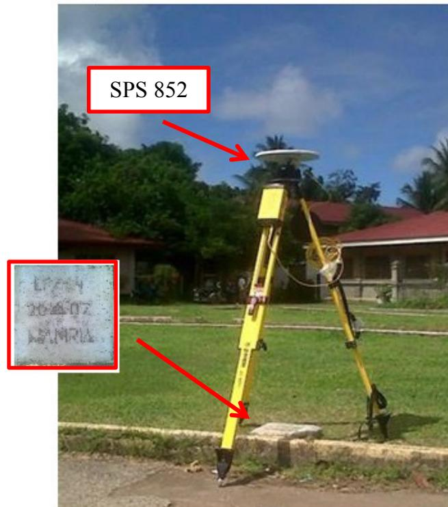
**Figure 13.** GNSS observation at a reference point, CPZ 14 at Pan-ay church, Panay, Capiz
