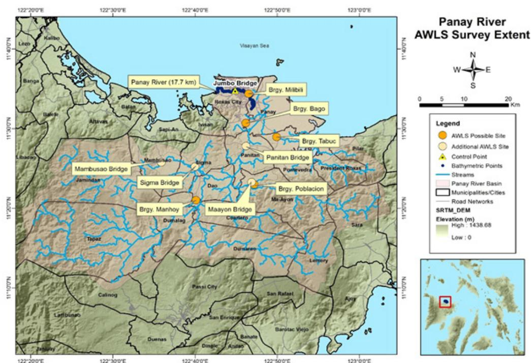
**Figure 37.** Possible sites for Automated Water Level Sensor (AWLS) installation along Panay River System
