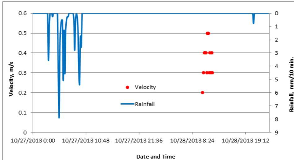
Figure 32. Relationship between Water Velocity and Rainfall at Sigma Bridge
