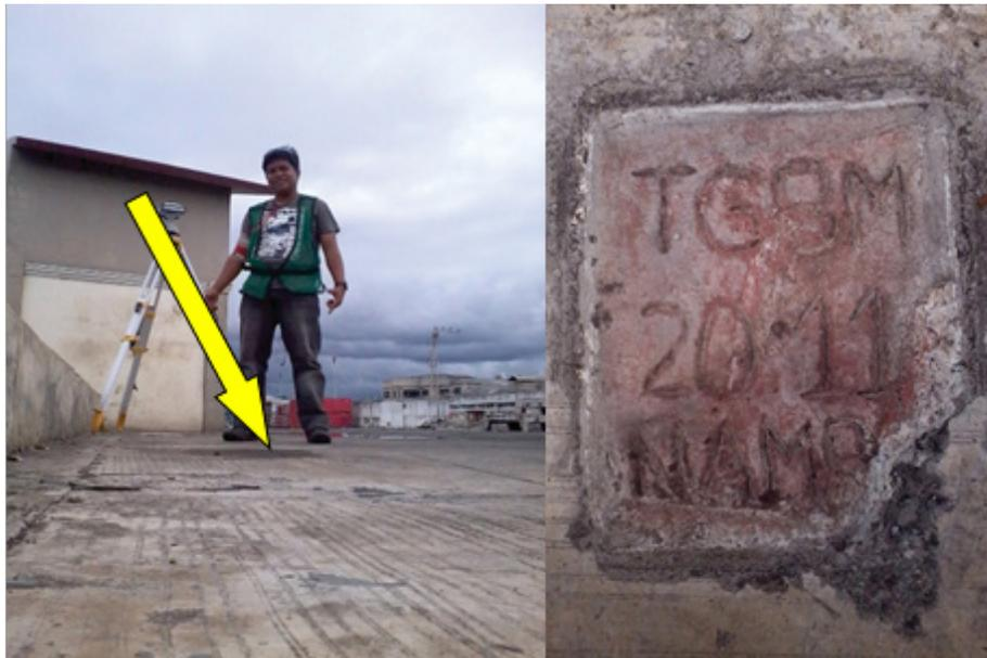
**Figure 4:** Static observation on TGBM inside Macabalan Port
