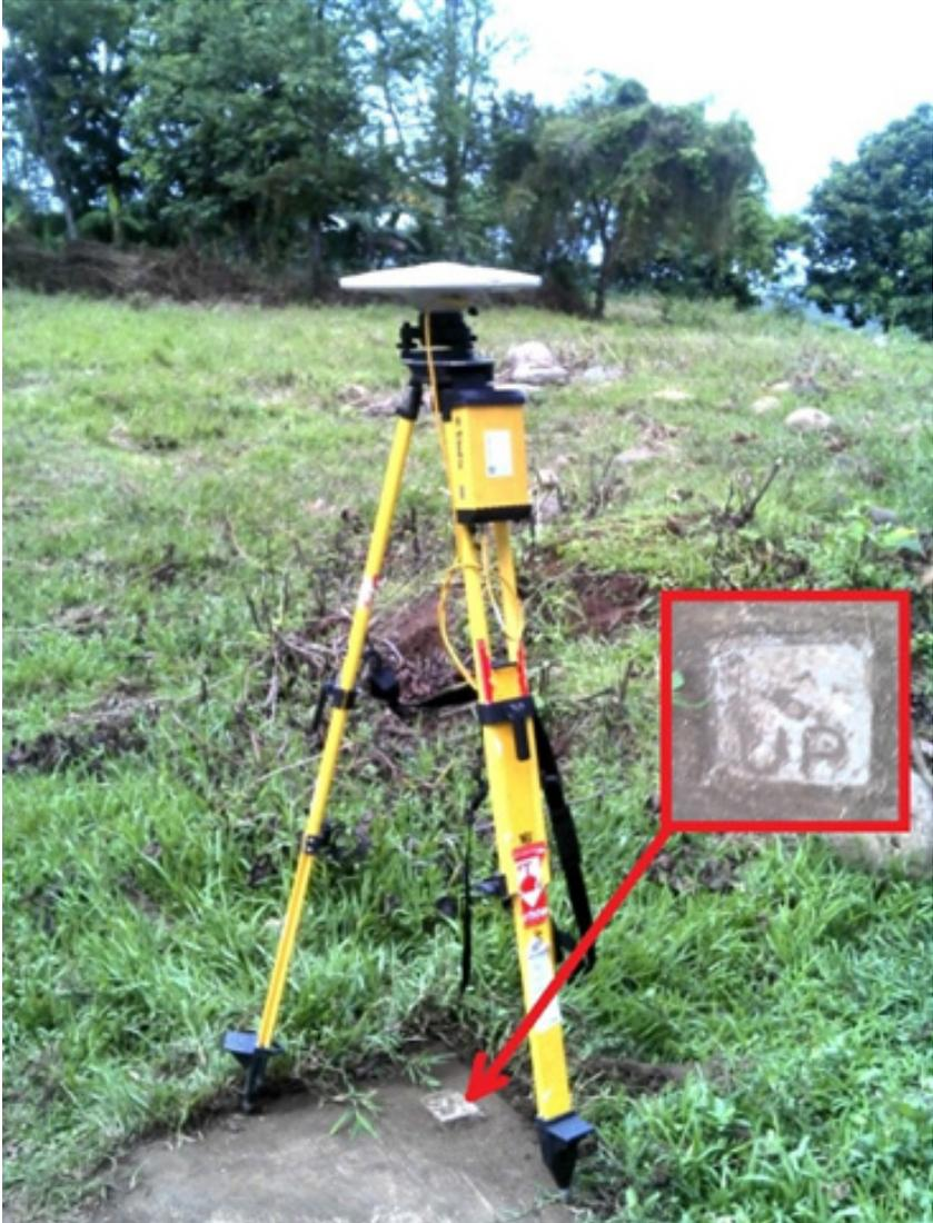
Figure 13. Static GNSS observation on UP established control point (UP-TAG)
