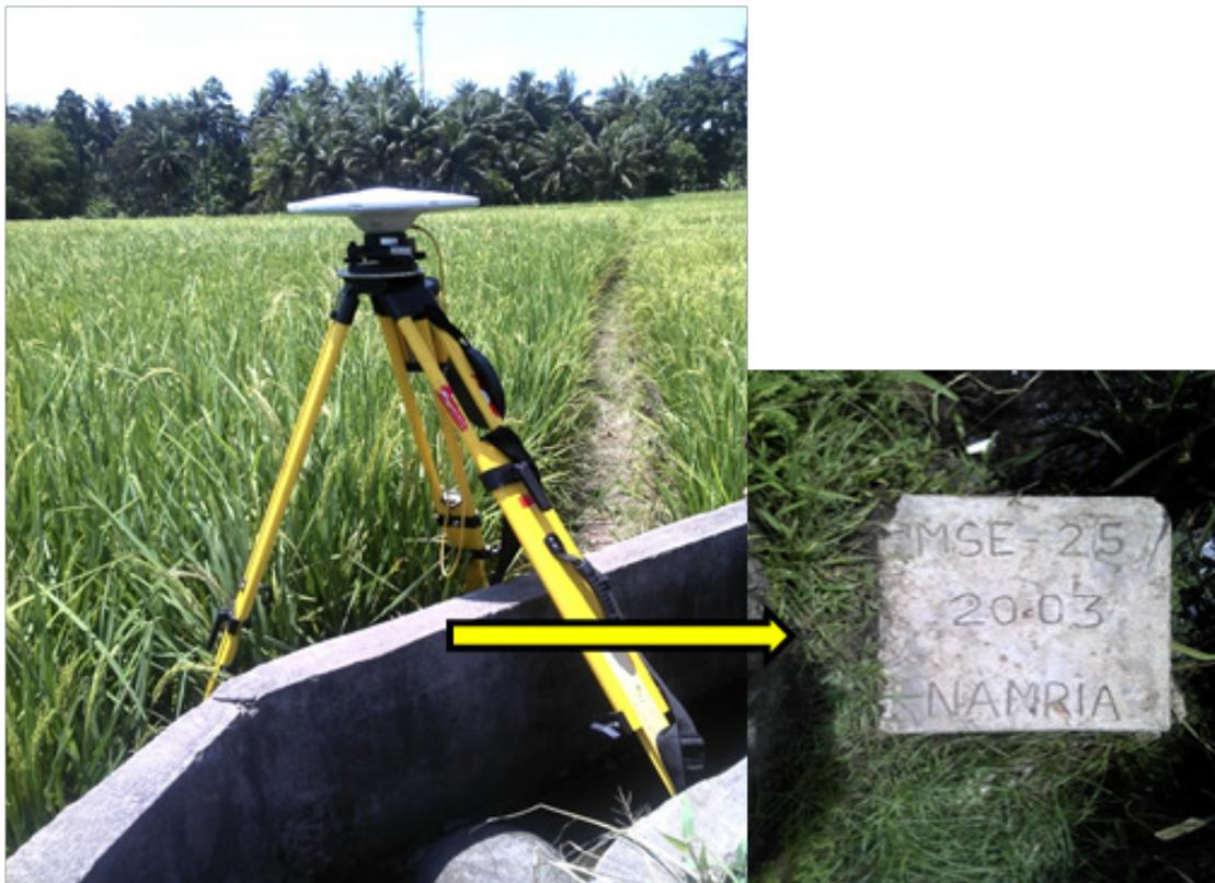
**Figure 12.** Static GNSS observation on MSE-25 beside a concrete irrigation canal in Brgy. Poblacion, Villanueva, Misamis Oriental
