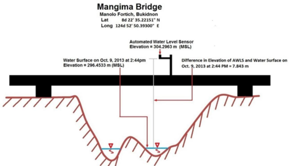
Figure 35. Cross-section diagram of Mangima Bridge
