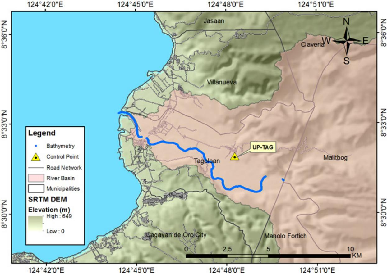
Figure 17. Bathymetry Survey along Tagoloan River
