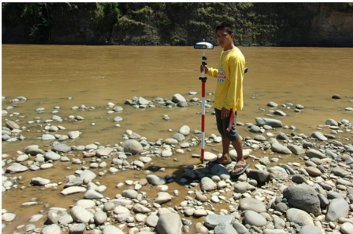
**Figure 9:** PT member conducting a profile survey in Tagoloan River
