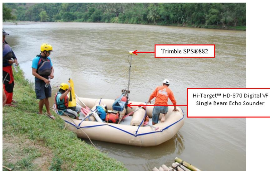
**Figure 15.** Bathymetric survey setup using Trimble SPS™ 882 mounted on top of the Hi-Target™ Transducer
