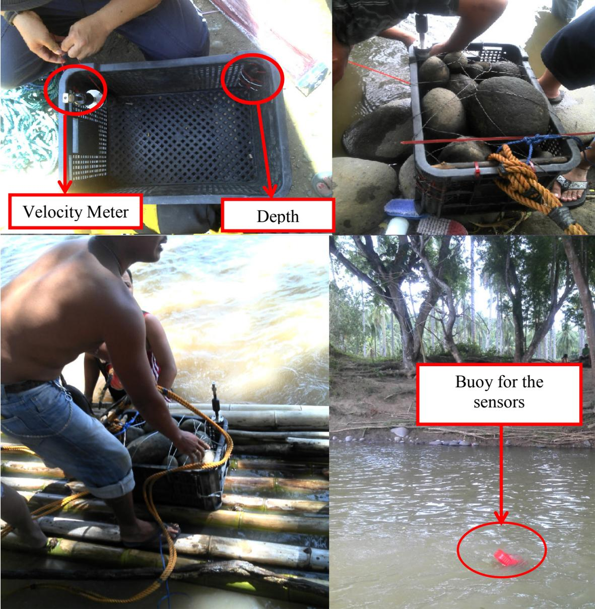
Figure 22. A series of picture displaying the components and deployment of the velocity meter and depth gauge in Tagoloan River, Brgy. Sta Ana, Tagoloan City
