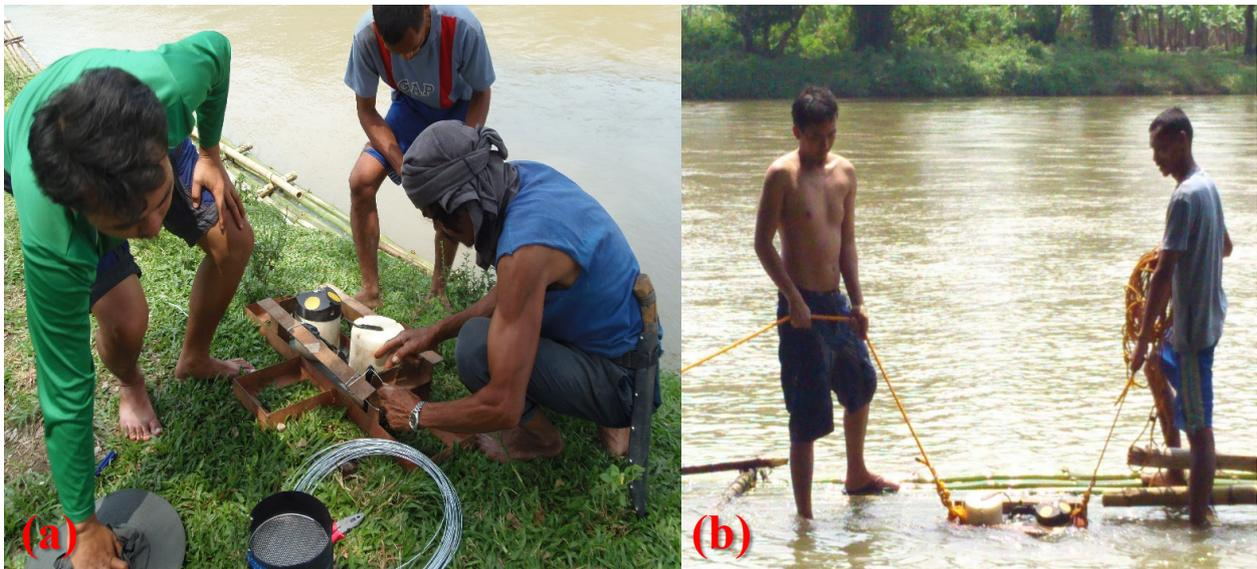
Figure 38. (a) Setting up of ADCP with depth gauge.
