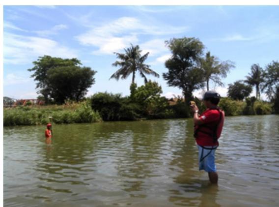
**Figure 16.** Manual bathymetric survey using PPK GNSS technique along Brgy. Poblacion, Tagoloan City
