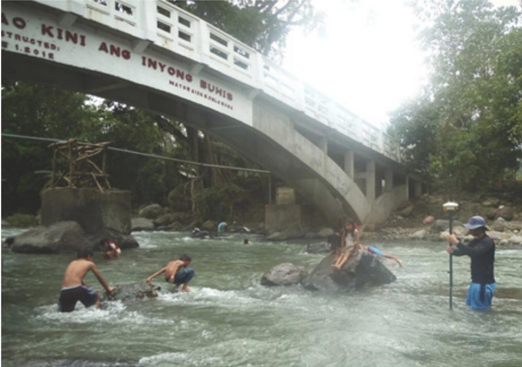
Figure 30. Cross-section survey at Arch Bridge
