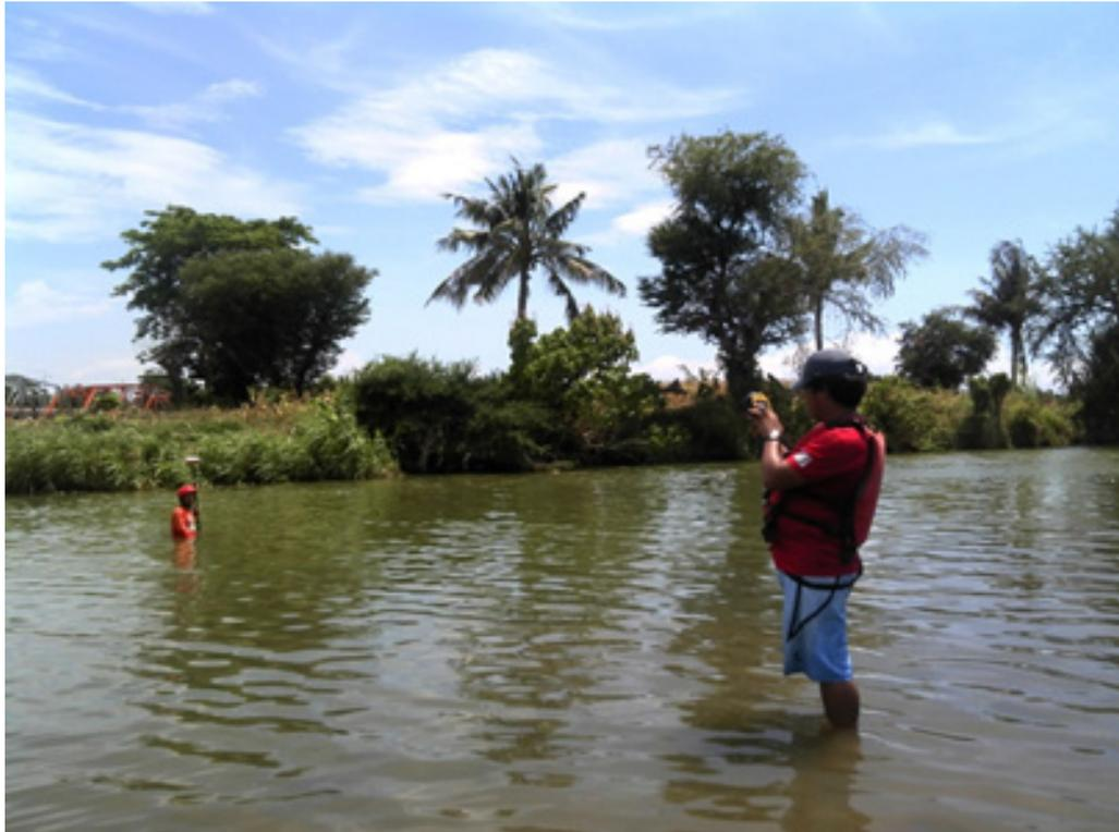
**Figure 51.** Survey team conducting bathymetry survey using PPK GNSS technique along cross section 17 to 19
