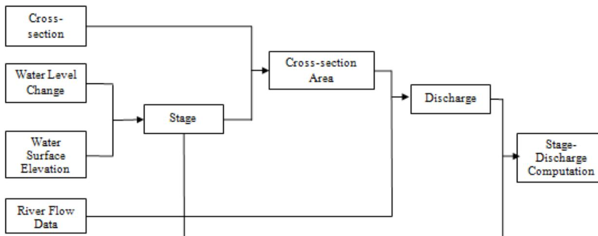
**Figure 6.** Flow Chart for Stage-Discharge Correlation Computation
