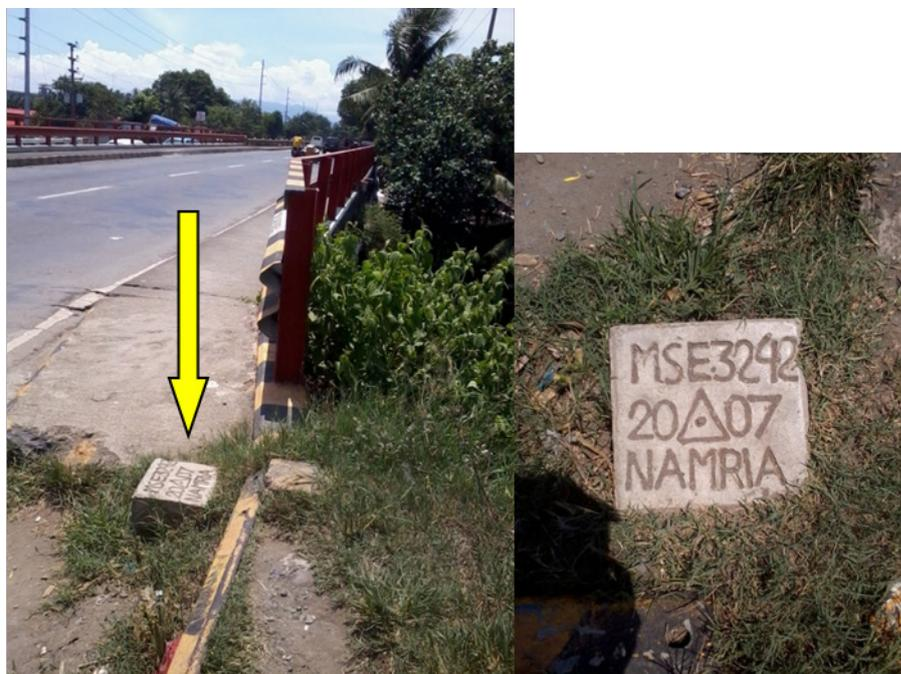
**Figure 6:** MSE-3242 at the foot of Umalag Bridge, Brgy. Tablon, Cagayan de Oro City was used during the static observation
