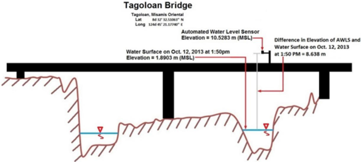
Figure 36. Cross-section diagram of Tagoloan Bridge
