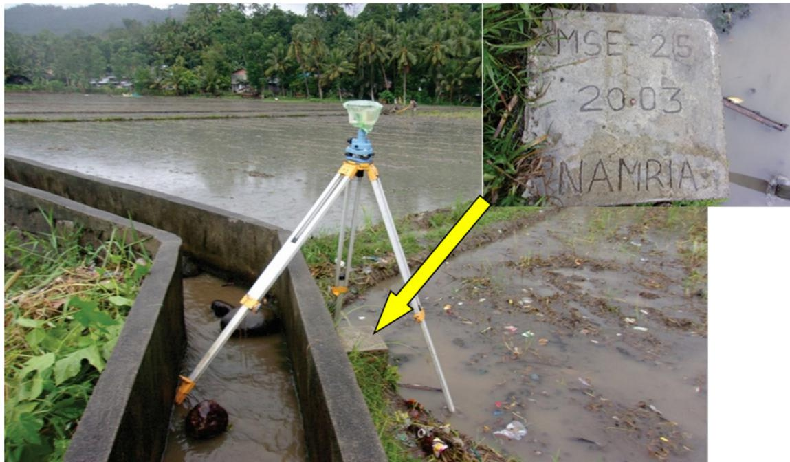
**Figure 5:** Static observation on MSE-25 beside a concrete irrigation canal at Brgy. Poblacion, Villanueva, Misamis Oriental
