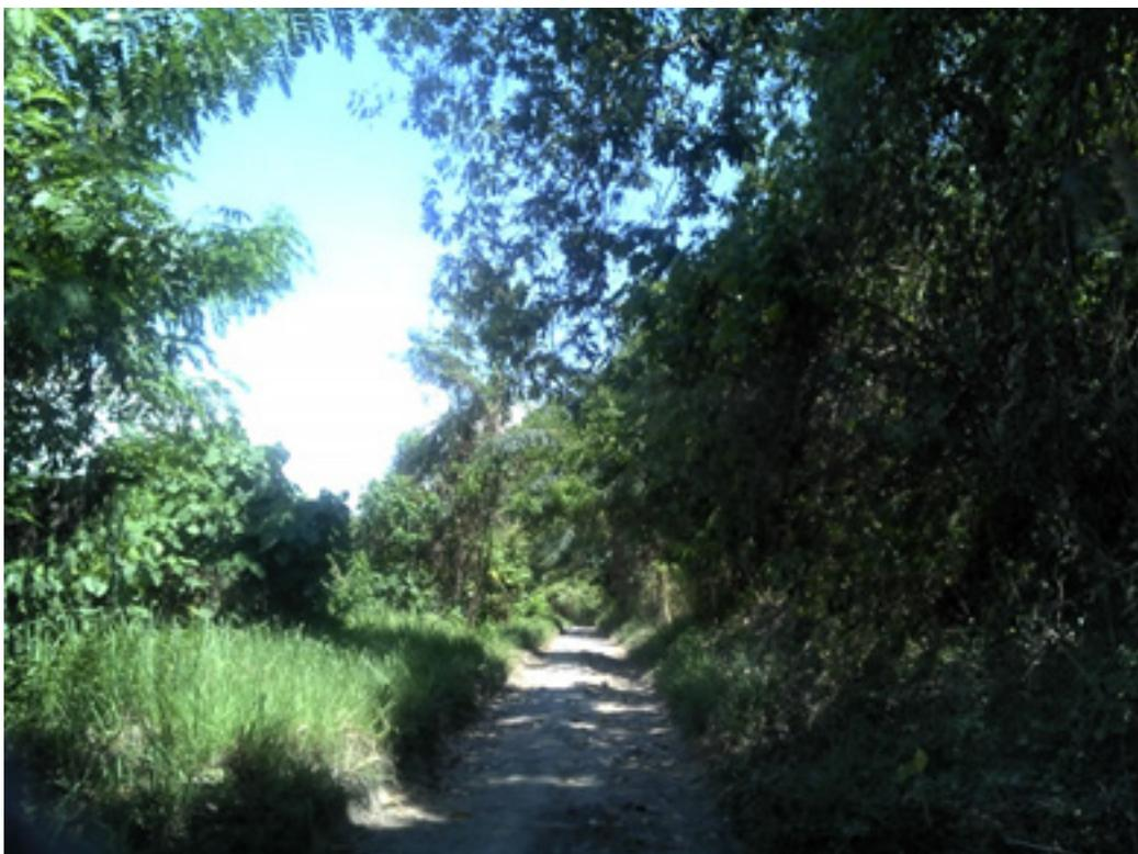
**Figure 52.** Canopy cover along roads made it difficult to conduct LiDAR validation survey using PPK GNSS technique on a continuous topo method
