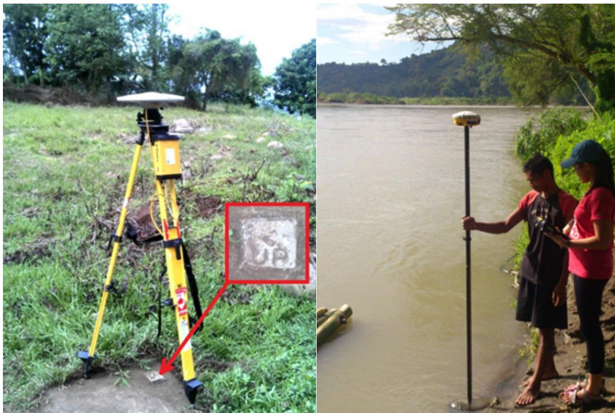
**Figure 26.** (left) GNSS base station at UP-Tagoloan located in Brgy. Sta Ana, Tagoloan City (right) Measuring the Water Surface Elevation using a DGPS
