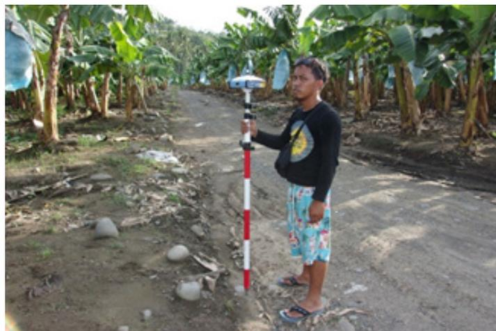
**Figure 10:** CST member holding an antenna during the conduct of cross-section survey inside a banana plantation
