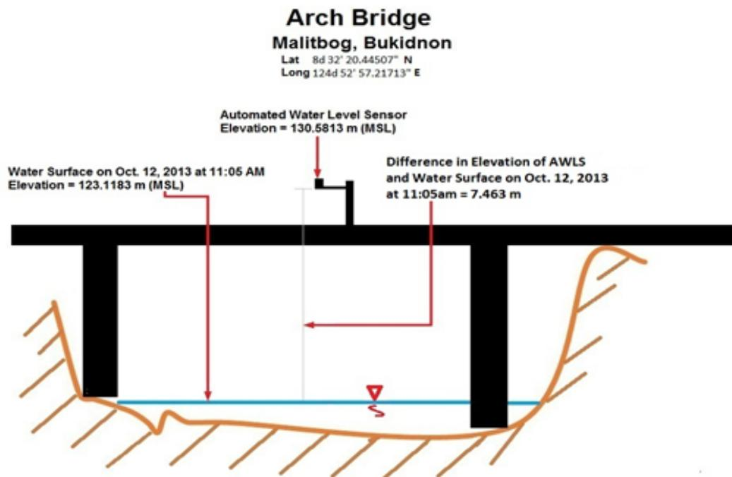
Figure 34. Cross-section diagram of Arch Bridge
