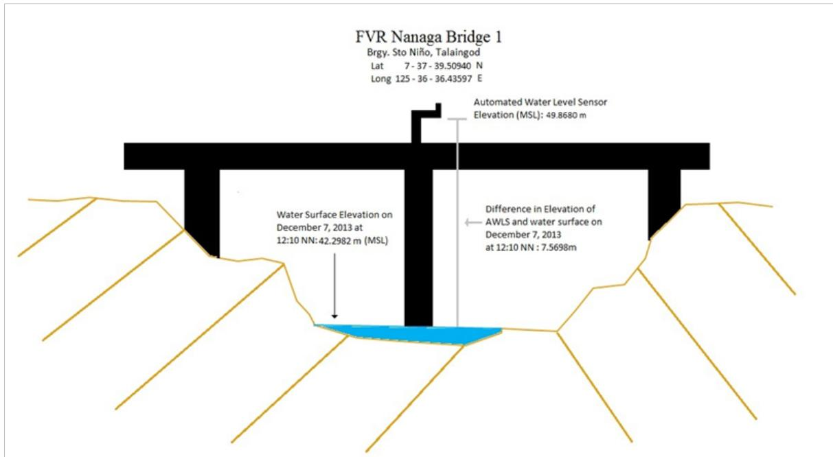
**Figure 54.** Cross-section diagram of FVR Nanaga Bridge 1, Brgy.Sto. Niño, Talaingod
