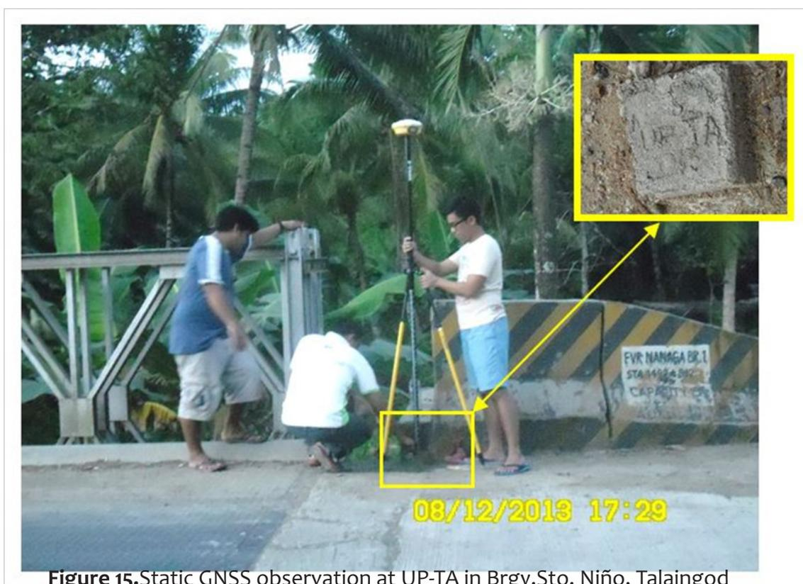
**Figure 15.** Static GNSS observation at UP-TA in Brgy.Sto. Niño, Talaingod
