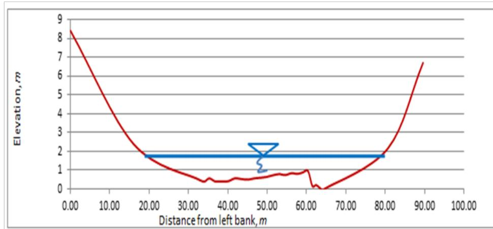
**Figure 59.** Graph showing the stage and cross-section along the ADCP deployment in Brgy. Pagsabangan, Tagum City
