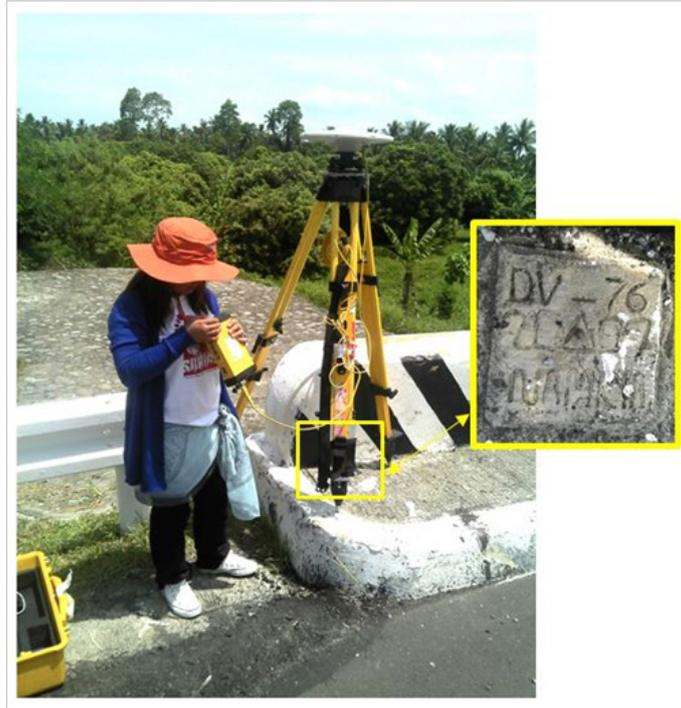
**Figure 13.** Static GNSS observation at DV-76 in Guadalupe Bridge, Tagum City
