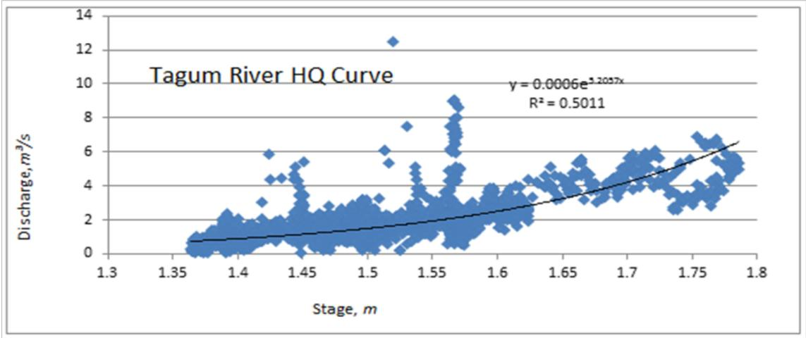
Figure 63. Relationship between stage and discharge
