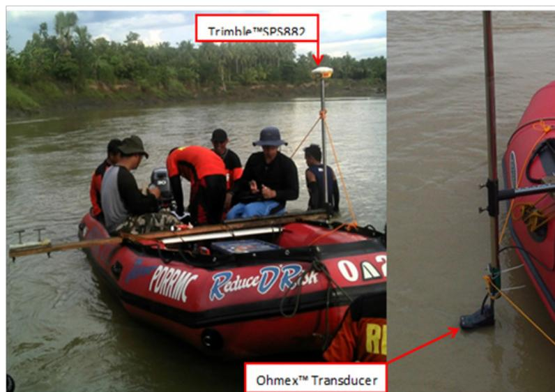
**Figure 18.** Bathymetric survey setup on a rubber boat
