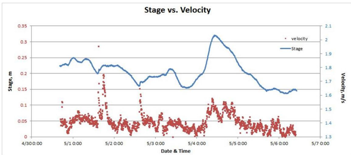
Figure 61. Relationship between velocity and stage
