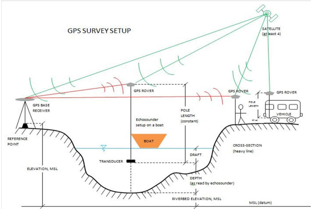
Figure 8. Setup for GNSS Surveys
