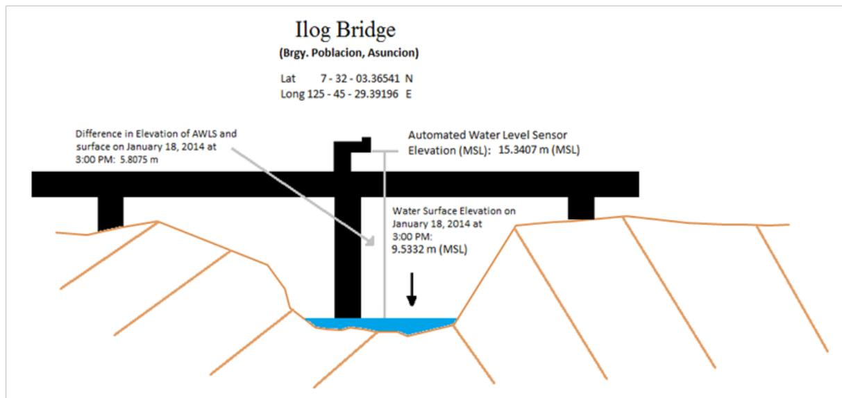
**Figure 55.** Cross-section diagram of Ilog Bridge, Brgy.Poblacion, Asuncion
