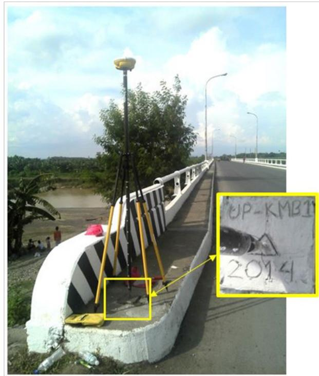
**Figure 17.** Static GNSS observation at UP-KMB1 in Brgy. Pag-Asa, Kapitalong
