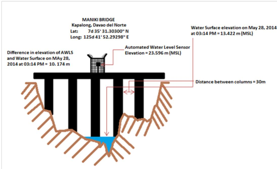
Figure 56. Cross-section diagram of Maniki Bridge, Brgy. Pag-Asa, Kapalong
