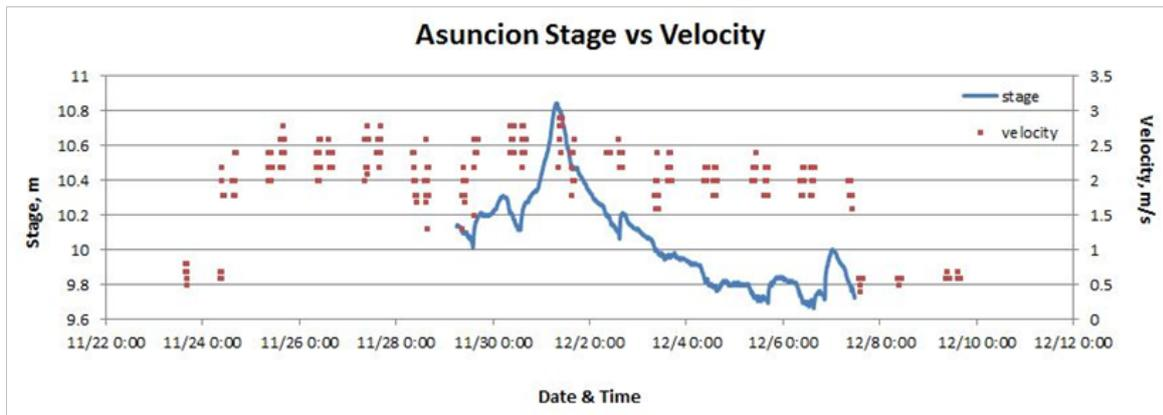
Figure 74. Stage vs. Velocity graph in Asuncion
