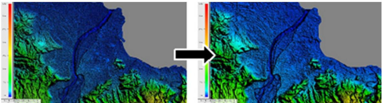
Figure 8. The 1-meter resolution LiDAR data resampled to a 10-meter raster grid in GIS software to ensure that values are properly adjusted.
