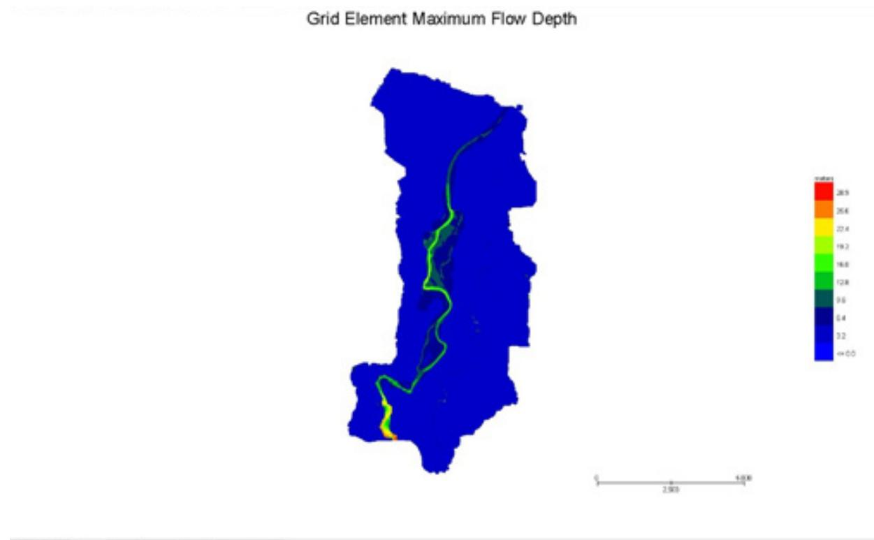
Figure 26. Cagayan de Oro floodplain generated flow depth map using FLO-2D Mapper
