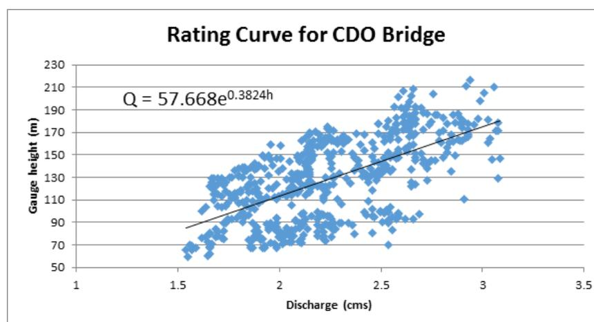
Figure 13. Water level vs. Discharge Curve for Waan Bridge, Cagayan
