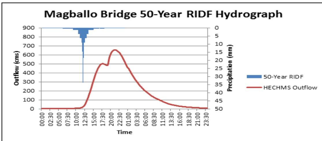
Figure 42. Magballo Bridge outflow hydrograph generated using the Dumaguete 50-Year RIDF inputted in WMS and HEC-HMS Basin Model.
