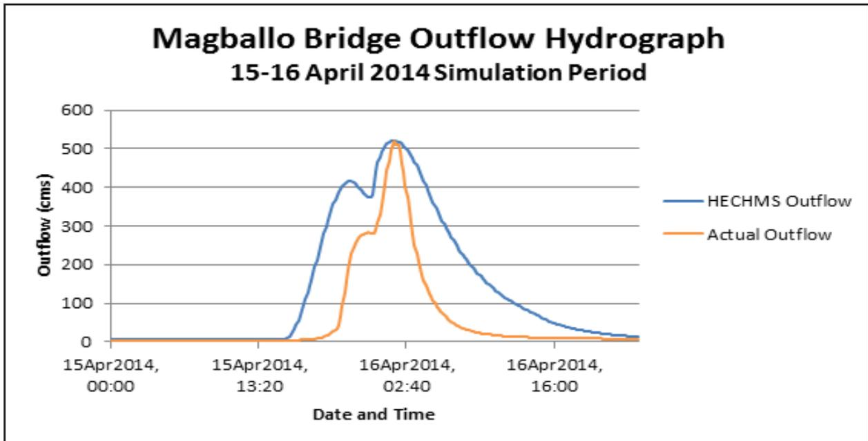
Figure 32. Outflow Hydrograph produced by the HEC-HMS model compared with observed outflow.
