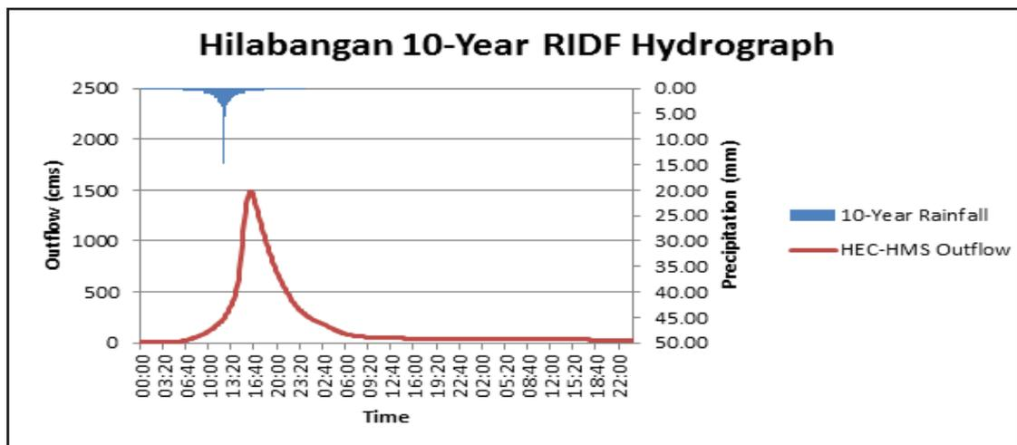
Figure 35. Hilabangan Bridge outflow hydrograph generated using the Negros 10-Year RIDF inputted in WMS and HEC-HMS Basin Model.
