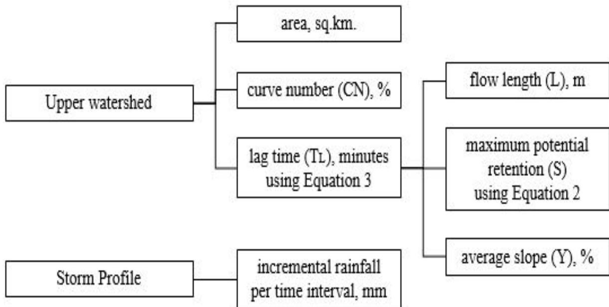
Figure 20. Different data needed as input for HEC-HMS discharge simulation using Dr. Horritt’s recommended hydrology method.
