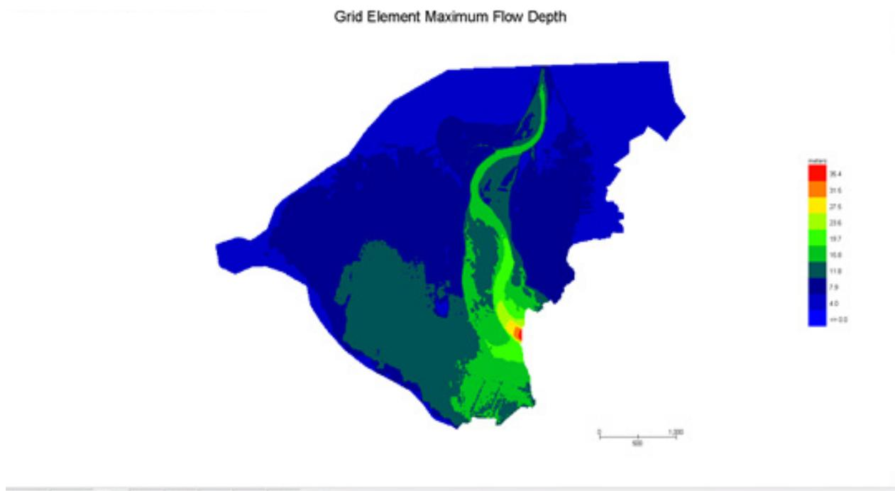
Figure 29. Hilabangan floodplain generated flow depth map using Flo-2D Mapper
