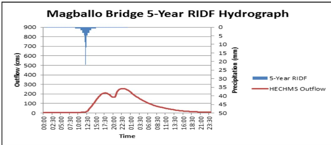
Figure 39. Magballo Bridge outflow hydrograph generated using the Dumaguete 5-Year RIDF inputted in WMS and HEC-HMS Basin Model.
