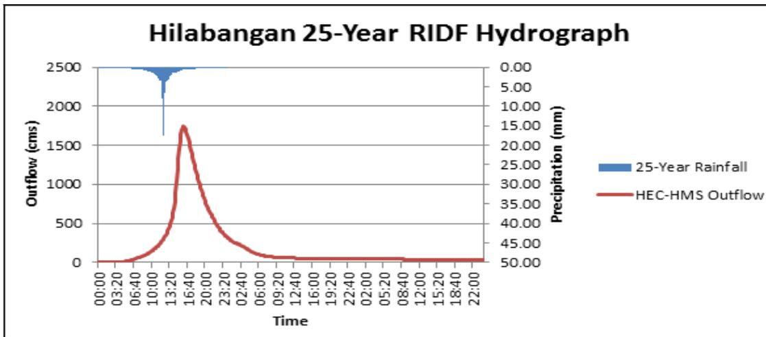
Figure 36. Hilabangan Bridge outflow hydrograph generated using the Negros 25-Year RIDF inputted in WMS and HEC-HMS Basin Model.
