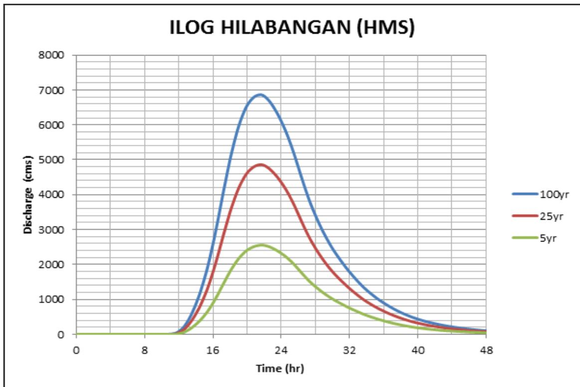
Figure 44. Outflow hydrograph generated for Ilog Hilabangan using the Iloilo Station 5-, 25-, 100-Year RIDF in HEC-HMS
