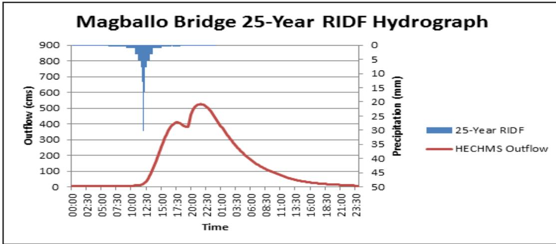
Figure 41. Magballo Bridge outflow hydrograph generated using the Dumaguete 25-Year RIDF inputted in WMS and HEC-HMS Basin Model.
