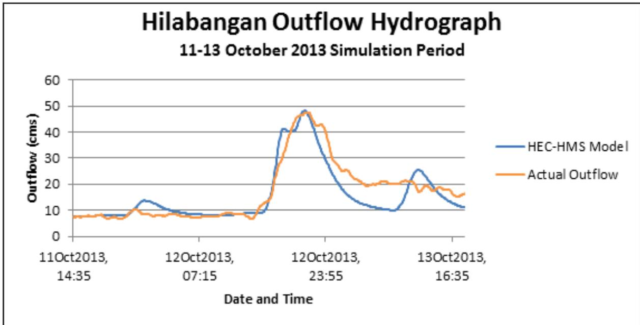
Figure 31. Outflow Hydrograph produced by the HEC-HMS model compared with observed outflow.
