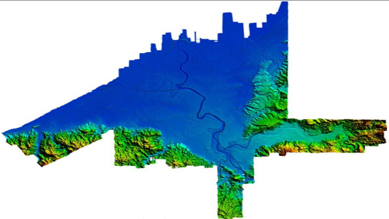
Figure 7. Digital Elevation Model (DEM) of the Hilabangan River Basin using Light Detection and Ranging (LiDAR) technology
