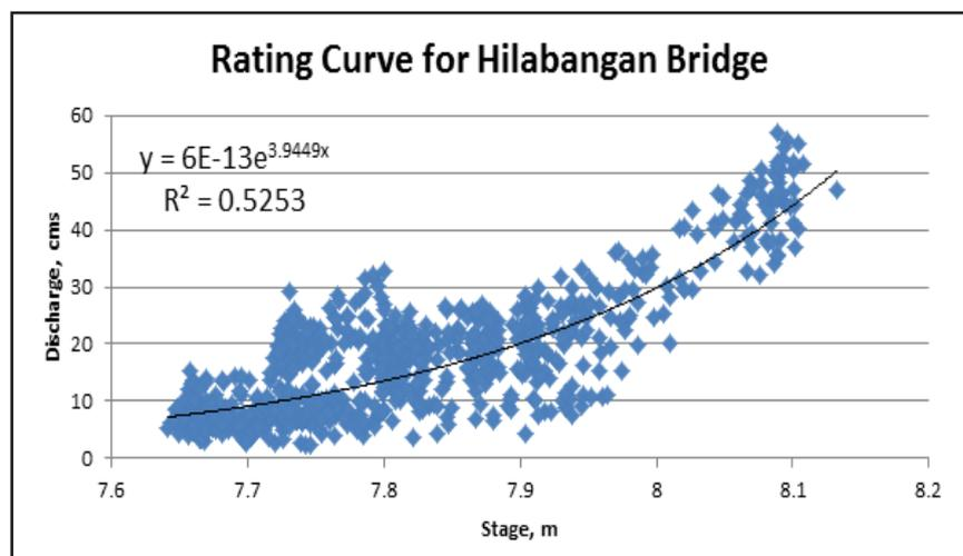
Figure 15. Water level vs. Discharge Curve for Hilabangan Bridge
