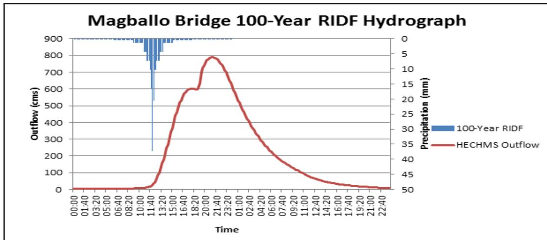
Figure 43. Magballo Bridge outflow hydrograph generated using the Dumaguete 100-Year RIDF inputted in WMS and HEC-HMS Basin Model
