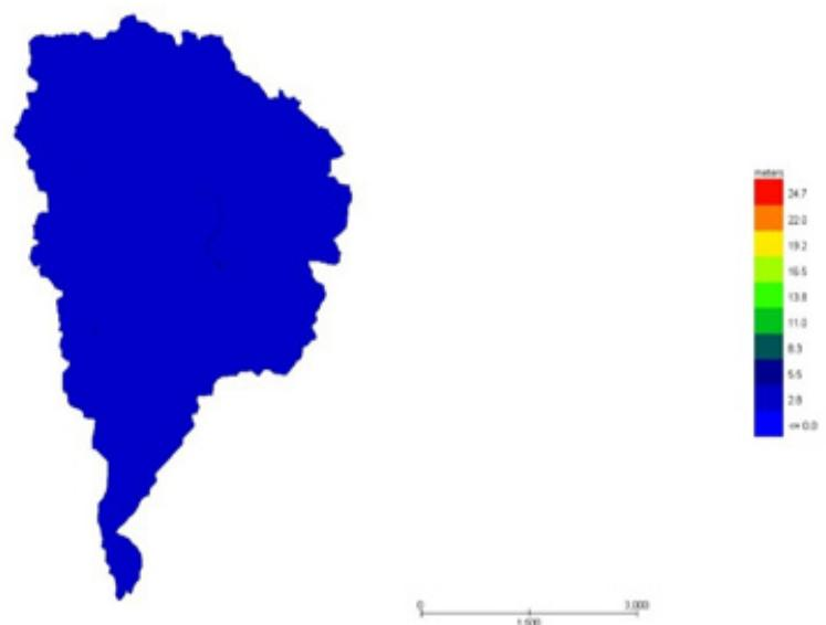
Figure 30. Mag-asawang Tubig floodplain generated flow depth map using FLO-2D Mapper
