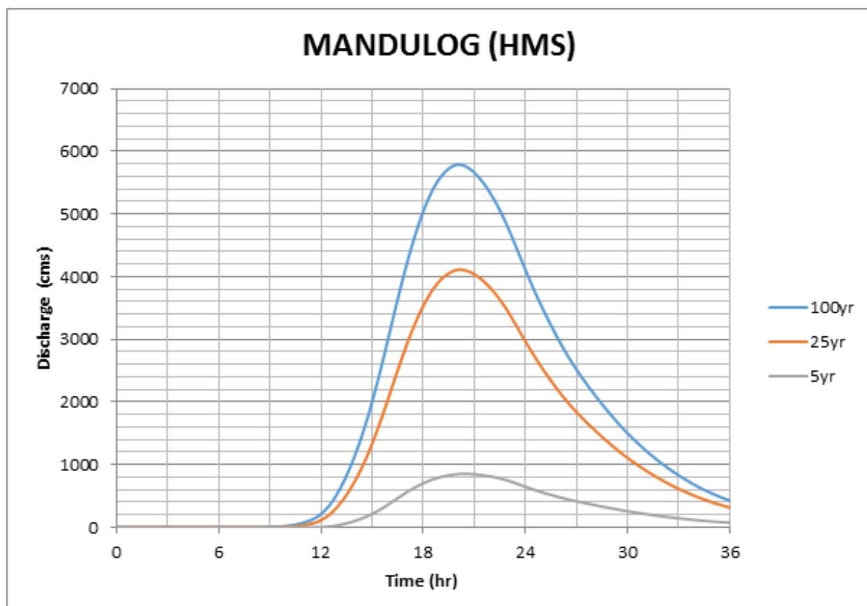
Figure 35. Outflow hydrograph generated using the Mandulog 5-, 25-, 100-Year RIDF in HEC-
