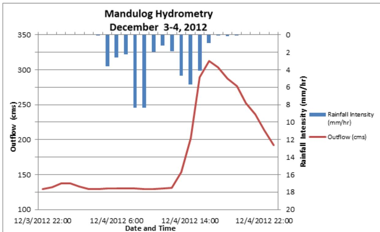
Figure 10. Mandulog Bridge 2 rainfall and outflow data used for modeling.
