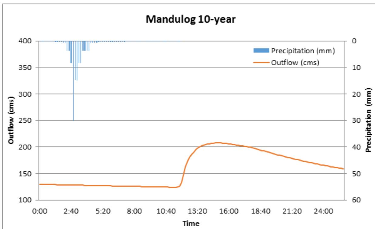
Figure 31. Outflow hydrograph generated using the Mandulog 10-Year RIDF in HEC-HMS.
