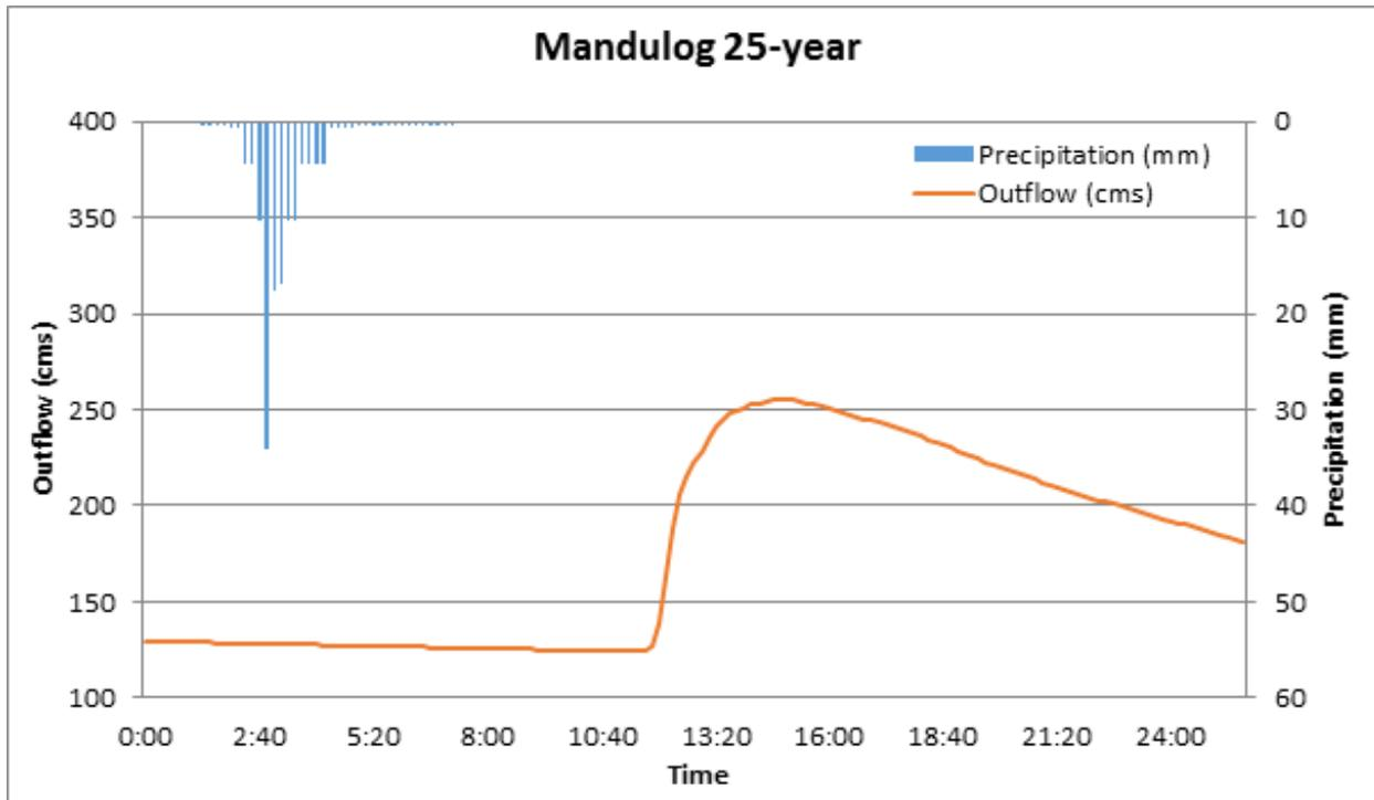
Figure 32. Outflow hydrograph generated using the Mandulog 25-Year RIDF in HEC-HMS.
