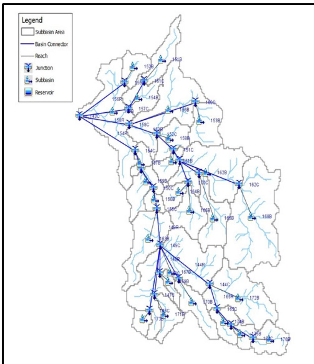
Figure 15. Mandulog HEC-HMS Model domain generated by WMS
