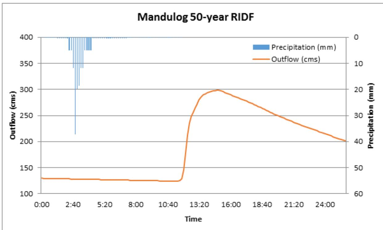
Figure 33. Outflow hydrograph generated using the Mandulog 50-Year RIDF in HEC-HMS.
