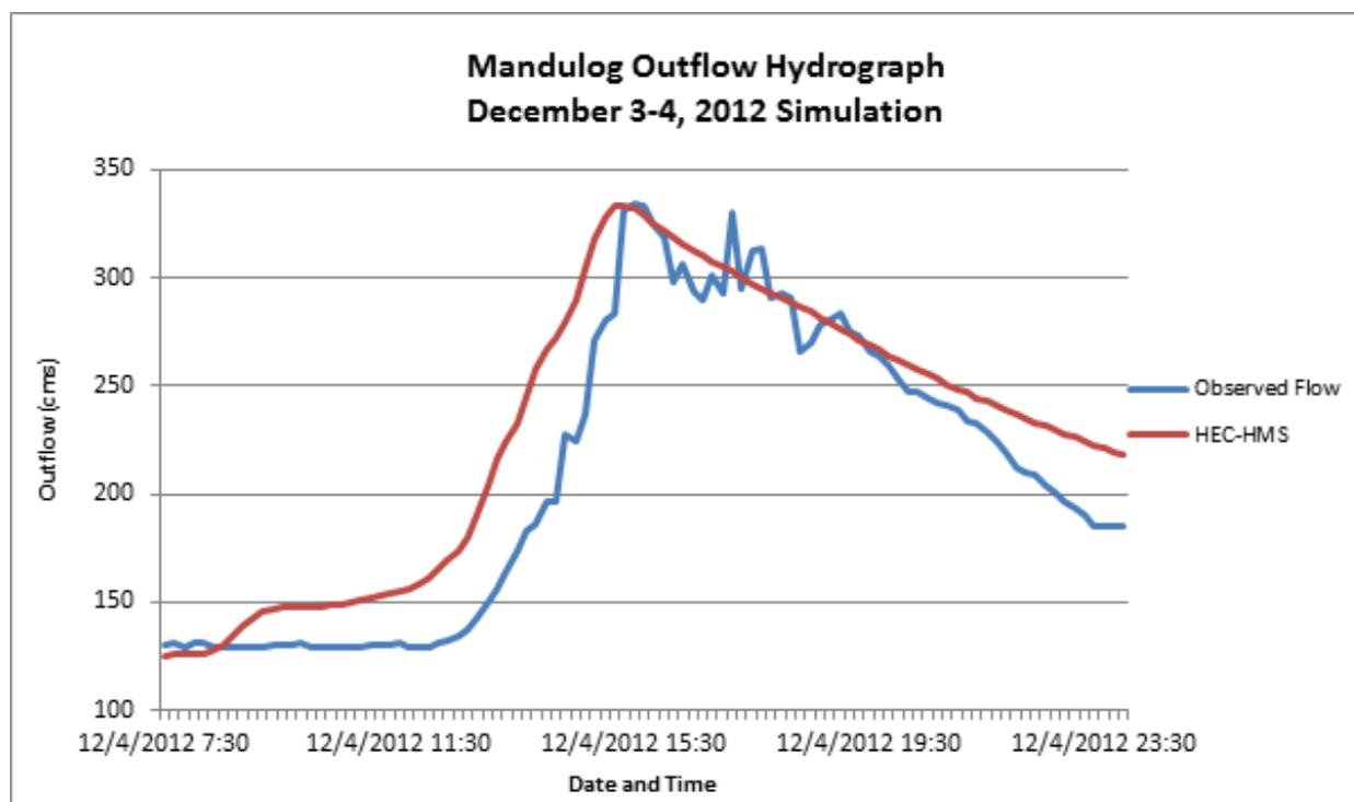
Figure 28. Outflow Hydrograph produced by the HEC-HMS model compared with observed outflow.
