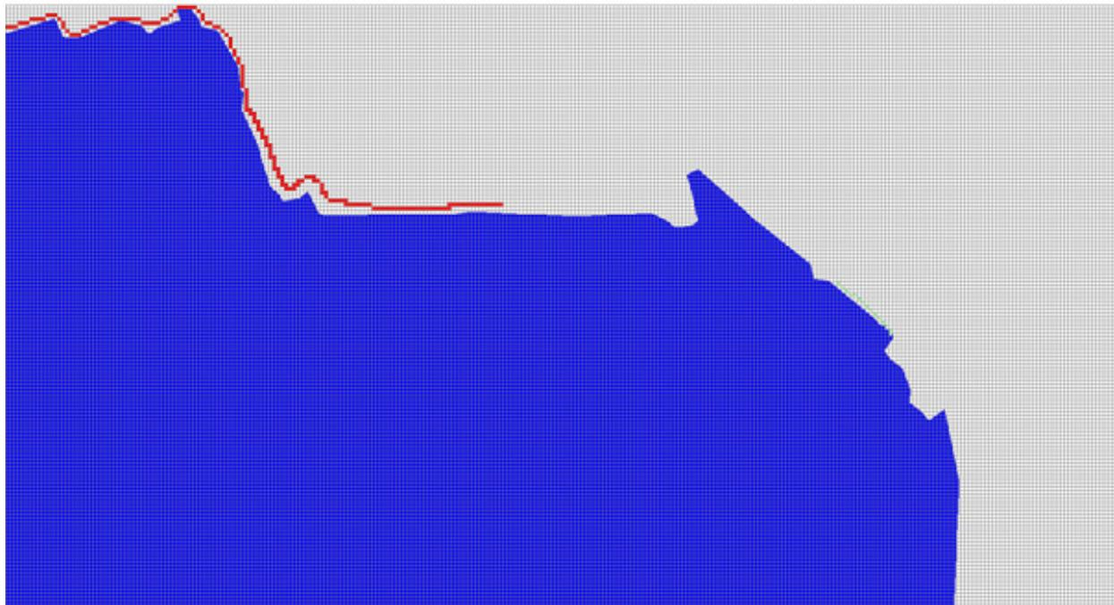
Figure 20. Screenshot showing how boundary grid elements are defined by line
