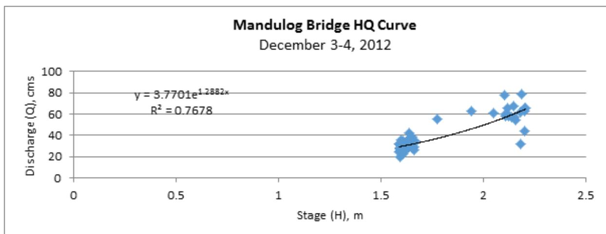
Figure 13. Water level vs. Discharge Curve for Mandulog Bridge 2
