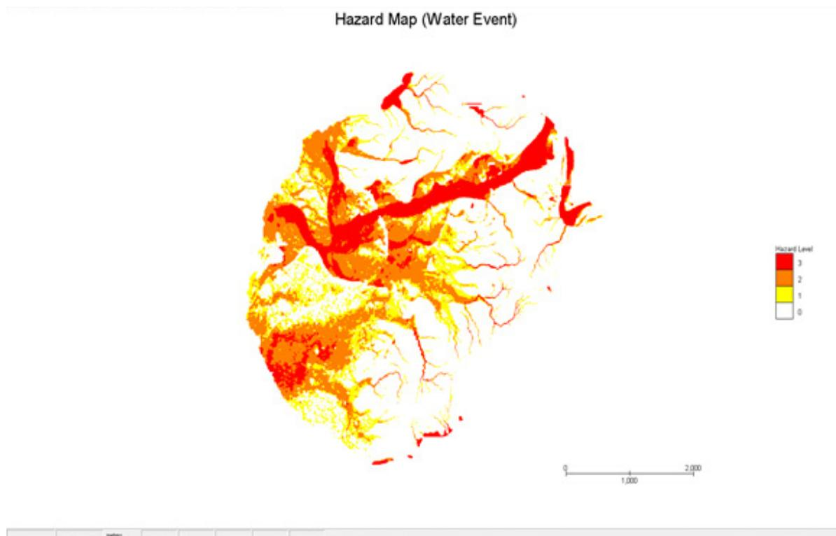
Figure 25. Mandulog Floodplain Generated Hazard Maps using FLO-2D Mapper
