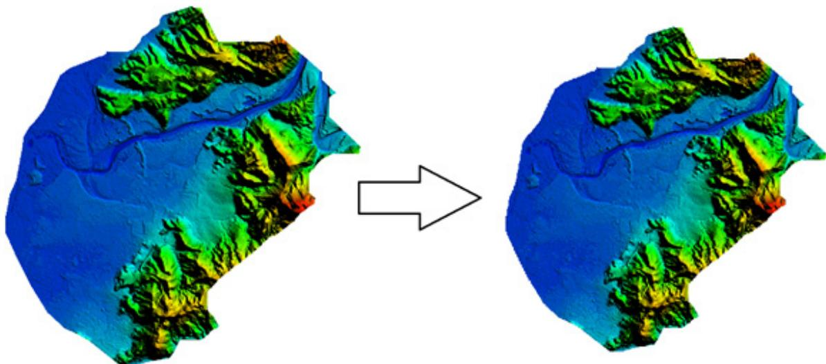
Figure 8. The 1-meter resolution LiDAR data resampled to a 10-meter raster grid in GIS software to ensure that values are properly adjusted.
