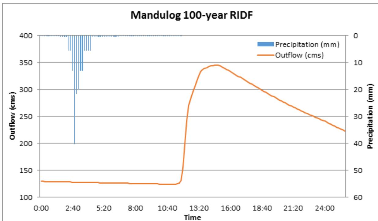
Figure 34. Outflow hydrograph generated using the Mandulog 100-Year RIDF in HEC-HMS.
