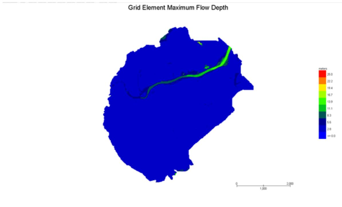
Figure 26. Mandulog floodplain generated flow depth map using FLO-2D Mapper
