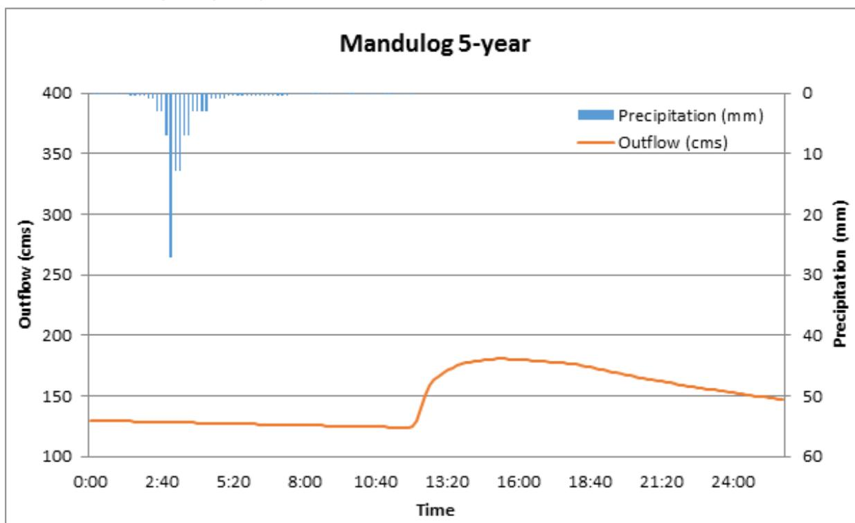
Figure 30. Outflow hydrograph generated using the Mandulog 5-Year RIDF in HEC-HMS.
