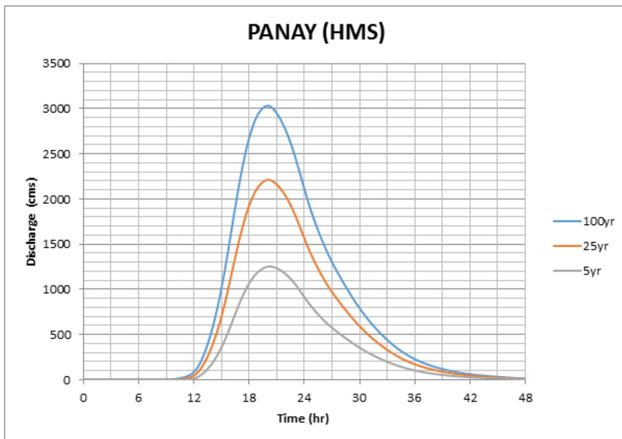
Figure 43. Outflow hydrograph generated for Tara, Panay using the Roxas 5-, 25-, and 100-year Rainfall Intensity Duration Frequency (RIDF) in HEC-HMS
