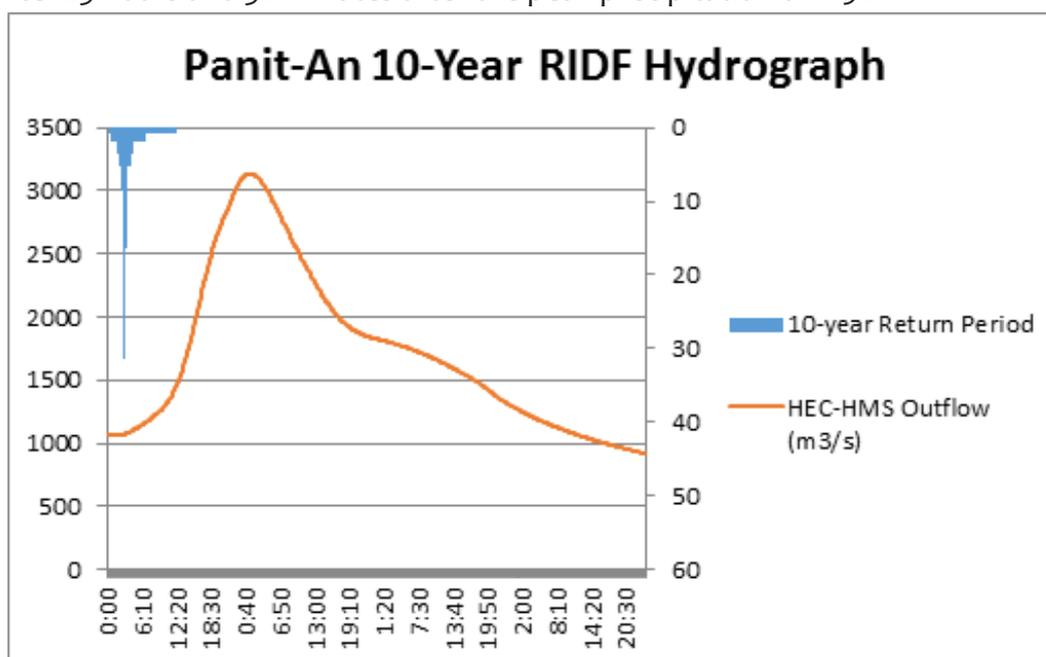
Figure 39. Outflow hydrograph generated using the Roxas 10-Year RIDF inputted in HEC-HMS
