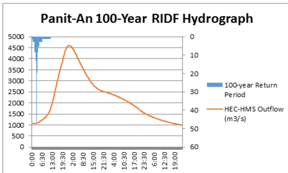
Figure 42. Outflow hydrograph generated using the Roxas 100-Year RIDF inputted in HEC-HMS
