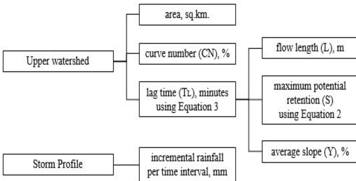
Figure 19. Different data needed as input for HEC-HMS discharge simulation using Dr. Horritt’s recommended hydrology method.
