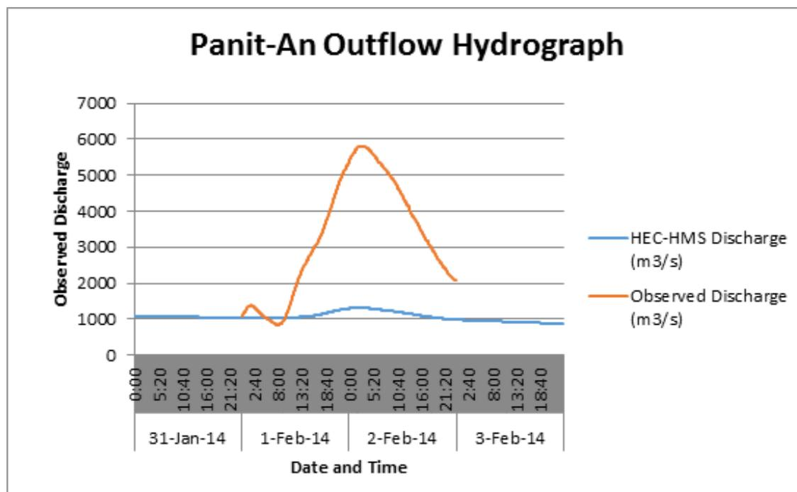
Figure 31. Outflow Hydrograph produced by the HEC-HMS model compared with observed outflow at Panit-an Bridge
