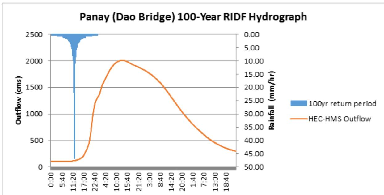
Figure 37. Outflow hydrograph generated using the Roxas 100-Year RIDF inputted in HEC-HMS
