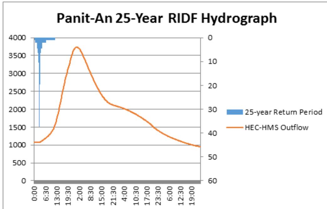
Figure 40. Outflow hydrograph generated using the Roxas 25-Year RIDF inputted in HEC-HMS
