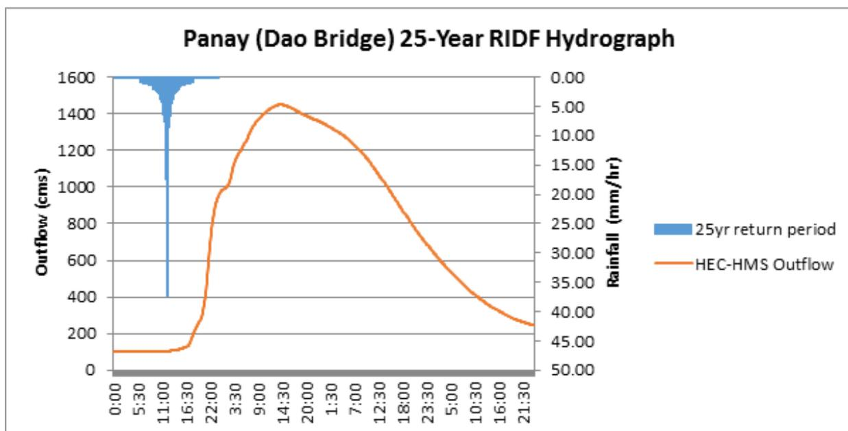
Figure 35. Outflow hydrograph generated using the Roxas 25-Year RIDF inputted in HEC-HMS
