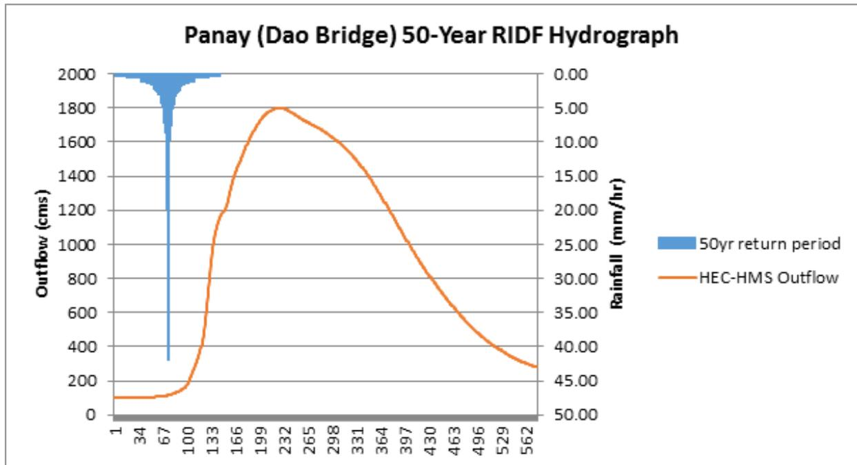
Figure 36. Outflow hydrograph generated using the Roxas 50-Year RIDF inputted in HEC-HMS
