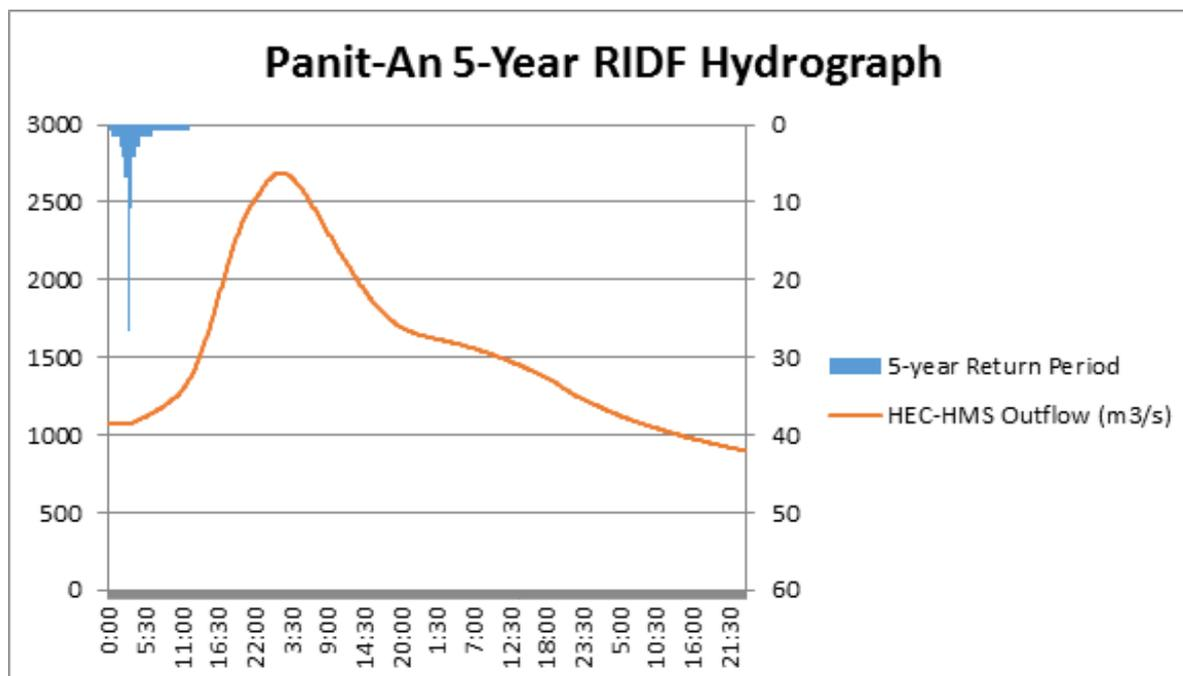
Figure 38. Outflow hydrograph generated using the Roxas 5-Year RIDF inputted in HEC-HMS
