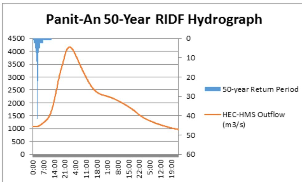
Figure 41. Outflow hydrograph generated using the Roxas 50-Year RIDF inputted in HEC-HMS
