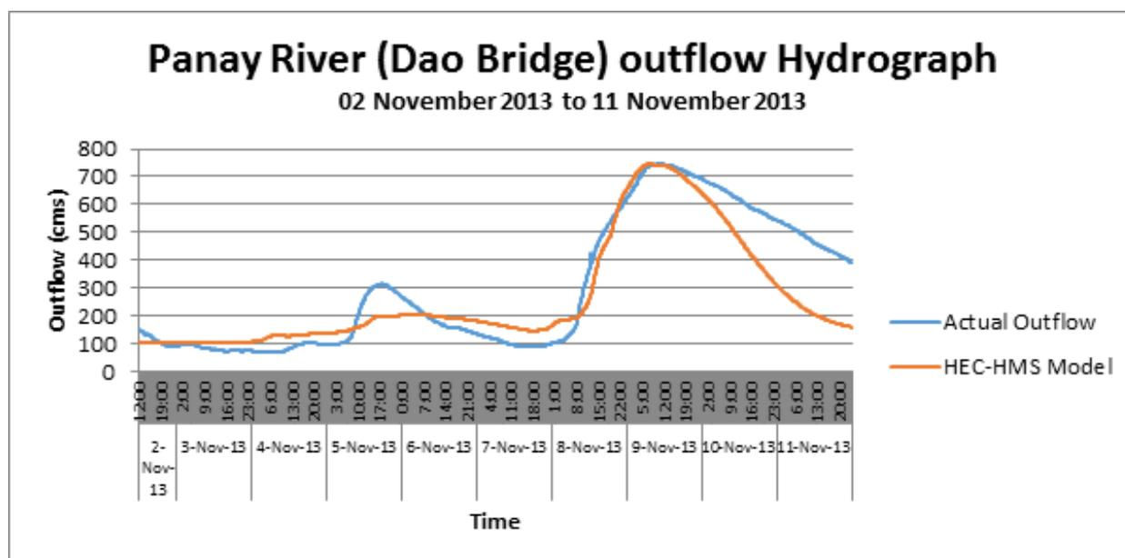
Figure 30. Outflow Hydrograph produced by the HEC-HMS model compared with observed outflow at Dao Bridge
