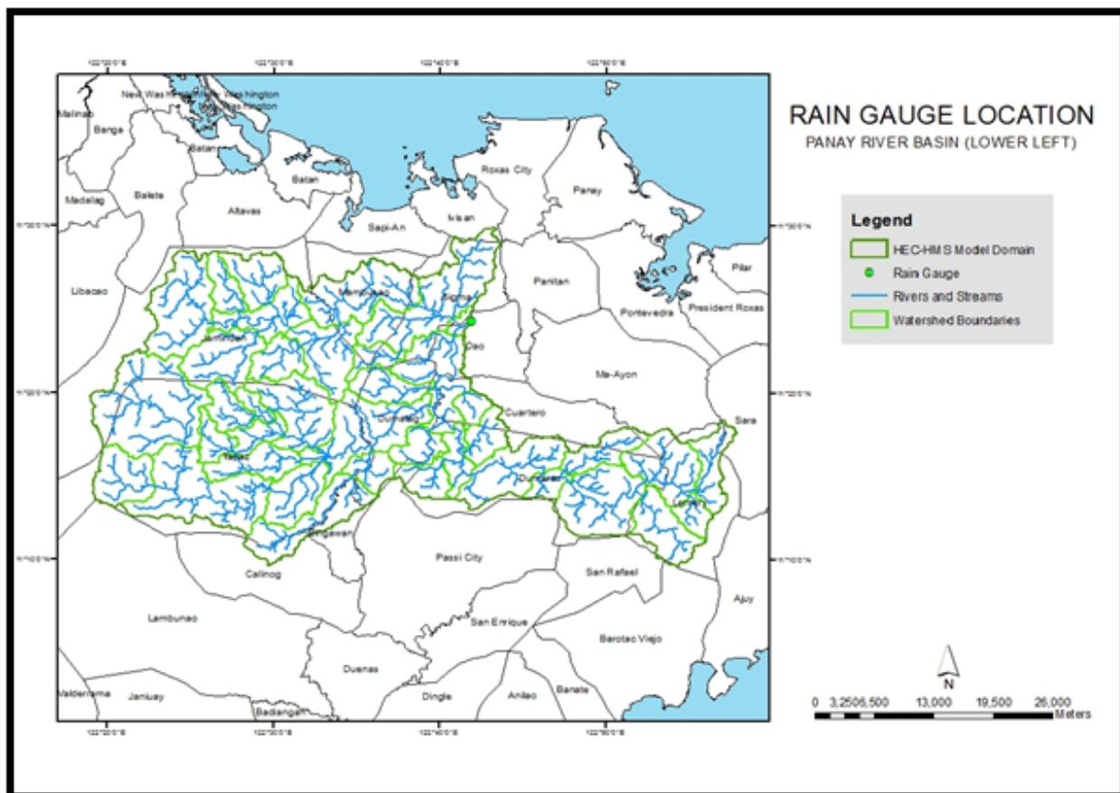
Figure 18. The location map of rain gauges used for the calibration of the Panay HEC-HMS
