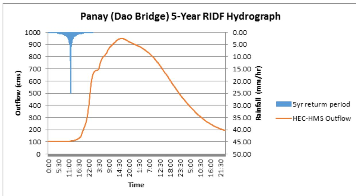
Figure 33 . Outflow hydrograph generated using the Roxas 5-Year RIDF inputted in HEC-HMS
