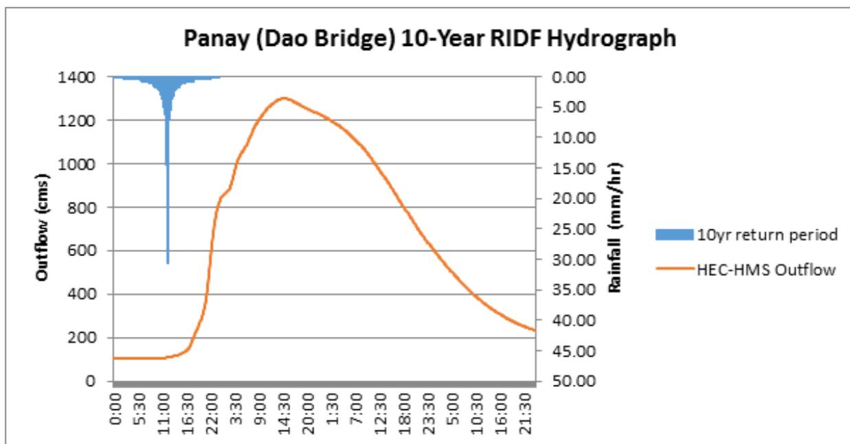
Figure 34. Outflow hydrograph generated using the Roxas 10-Year RIDF inputted in HEC-HMS
