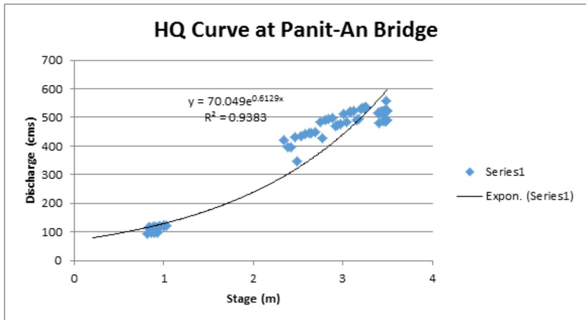
Figure 15. Water level vs. Discharge Curve for Panit-an
