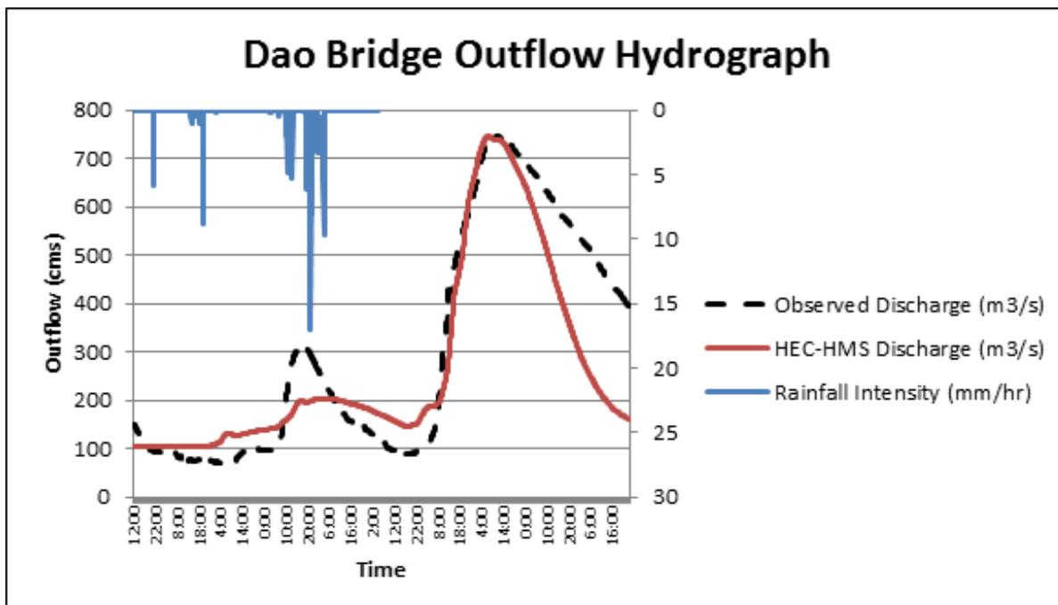
Figure 10. Rainfall and Outflow Data used for Modeling (Dao)
