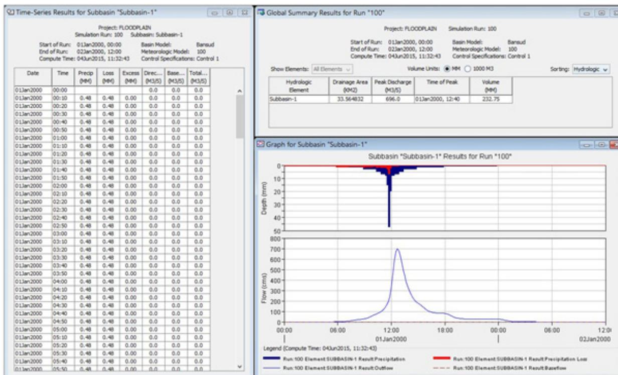
Figure 21. HEC-HMS simulation discharge results using Dr. Horritt’s Method
