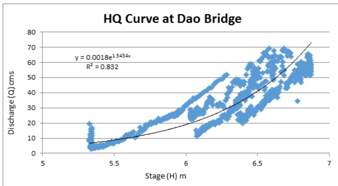
Figure 14. Water level vs. Discharge Curve for Dao Bridge
